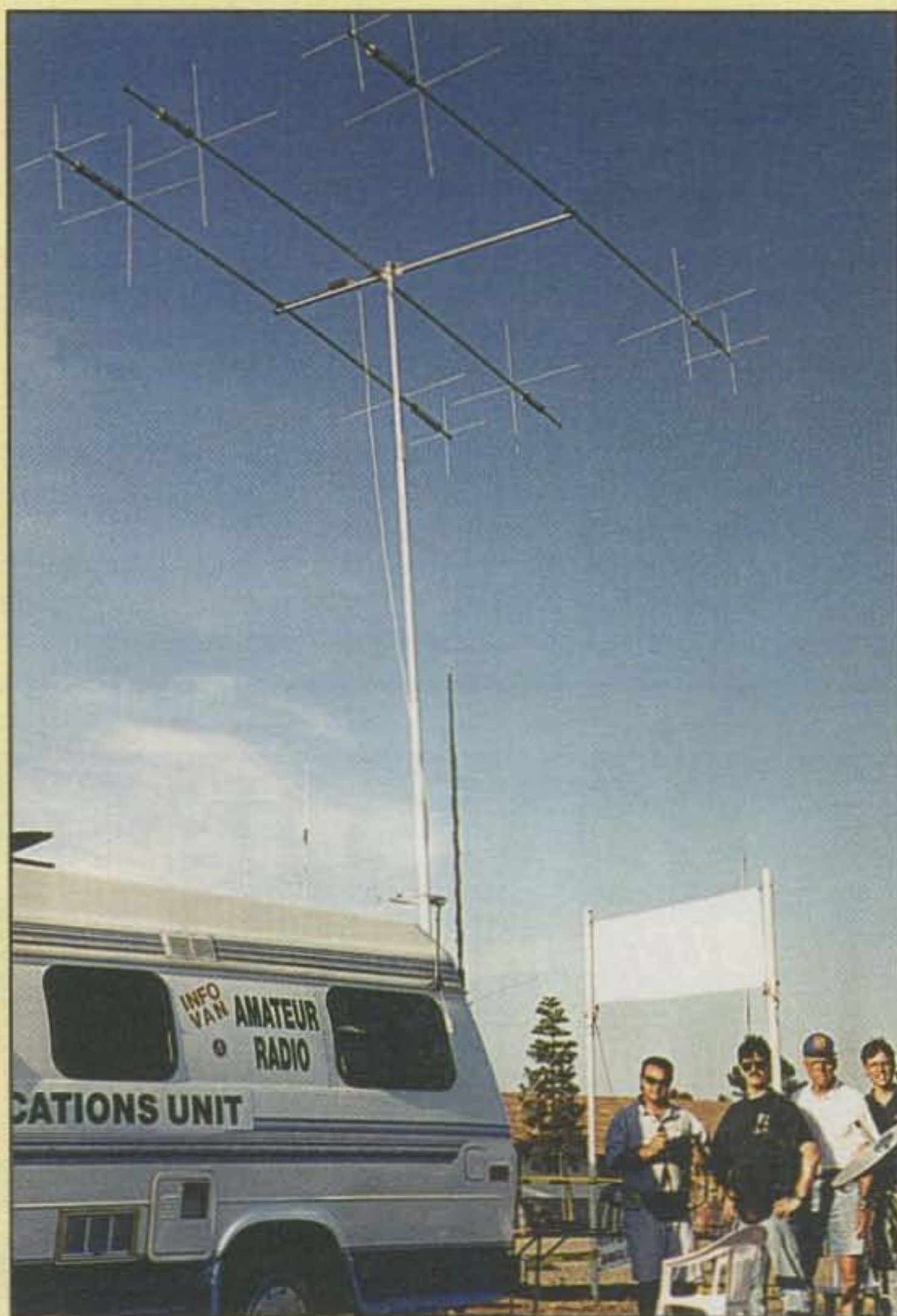
The Cushcraft MA5B "Director" mini beam is small enough to be mounted on a small rooftop or even on a (stationary) vehicle! It passed its Field Day tests with flying colors. The element at the far right in the photo is the reflector.
