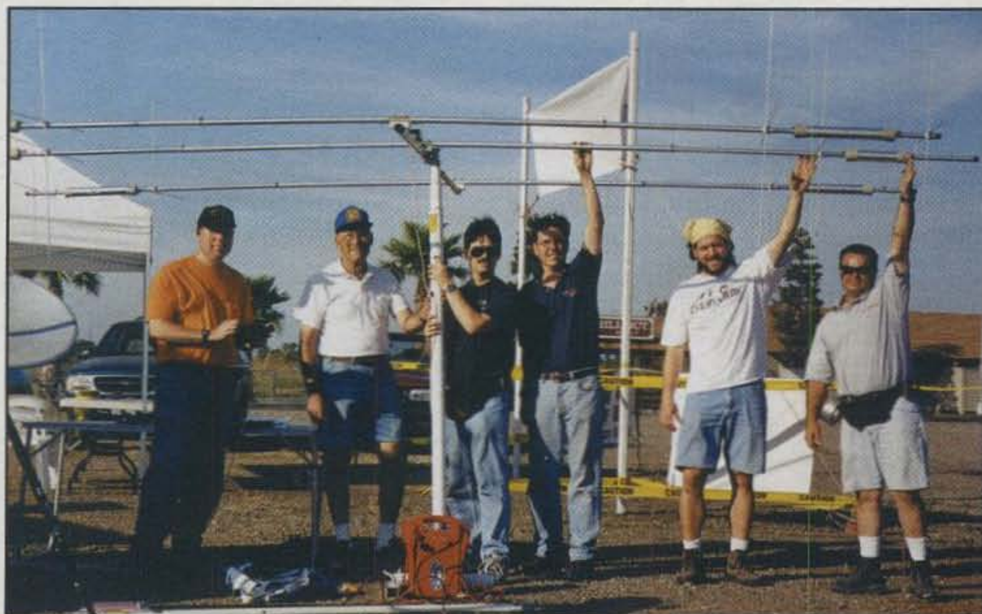
The MA5B assembled, mounted to a telescoping flagpole mast, and ready to be raised and put on the air.
