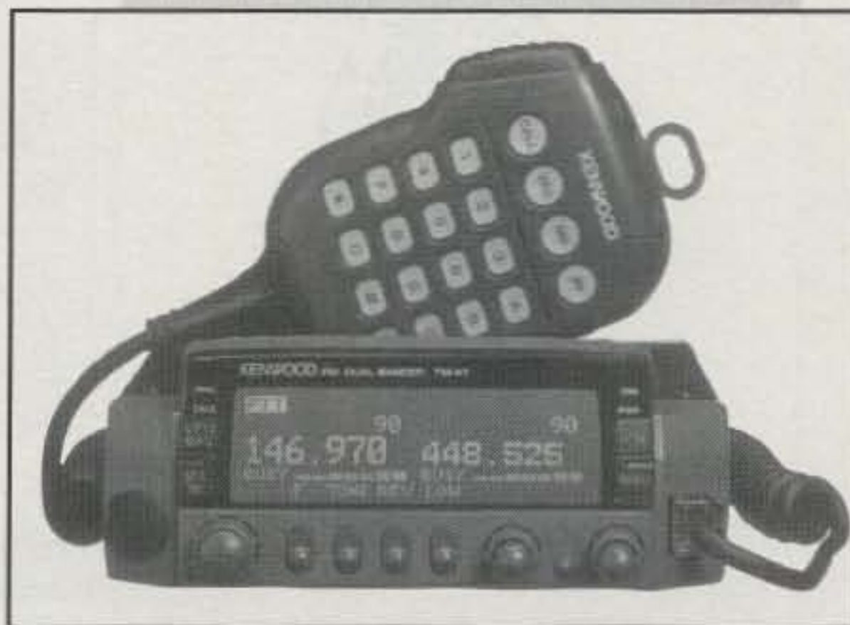
Kenwood's TM-V7A is typical of today's dual-band FM mobile rigs. Among its features is a detachable control head that lets you mount the radio under a seat or in the trunk and attach the head to the dashboard.
