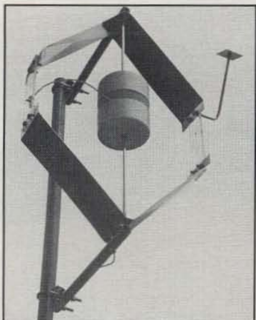
Photo 6— Antenna problems keeping you from having fun on HF? Beat the odds and have a ball with a world-famous Isotron®. A 40 or 30 meter version measures only 22" x 16" x 15", can be installed quickly (hidden?) almost anywhere, and works very well for its size. (Details in text.)
