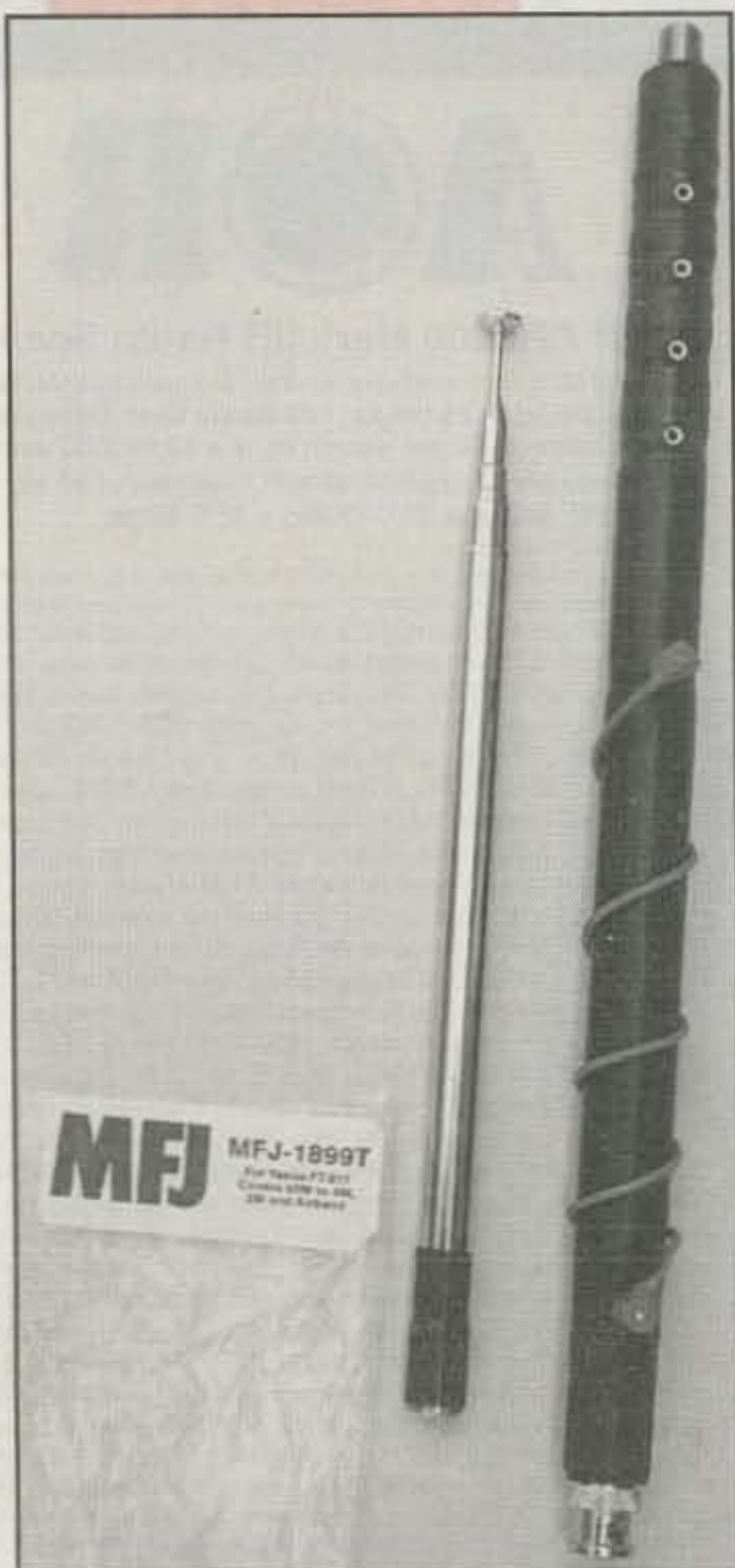
Photo 3— All bands right in your hand! This new MFJ-1899T "Walkabout" antenna covers 80 through 2 meters in a single "break apart and carry anywhere" package. Fully extended, it measures 63 inches in height. Retracted and separated, the helical base section is 12 inches long and the pull-up whip is 7 inches long.
