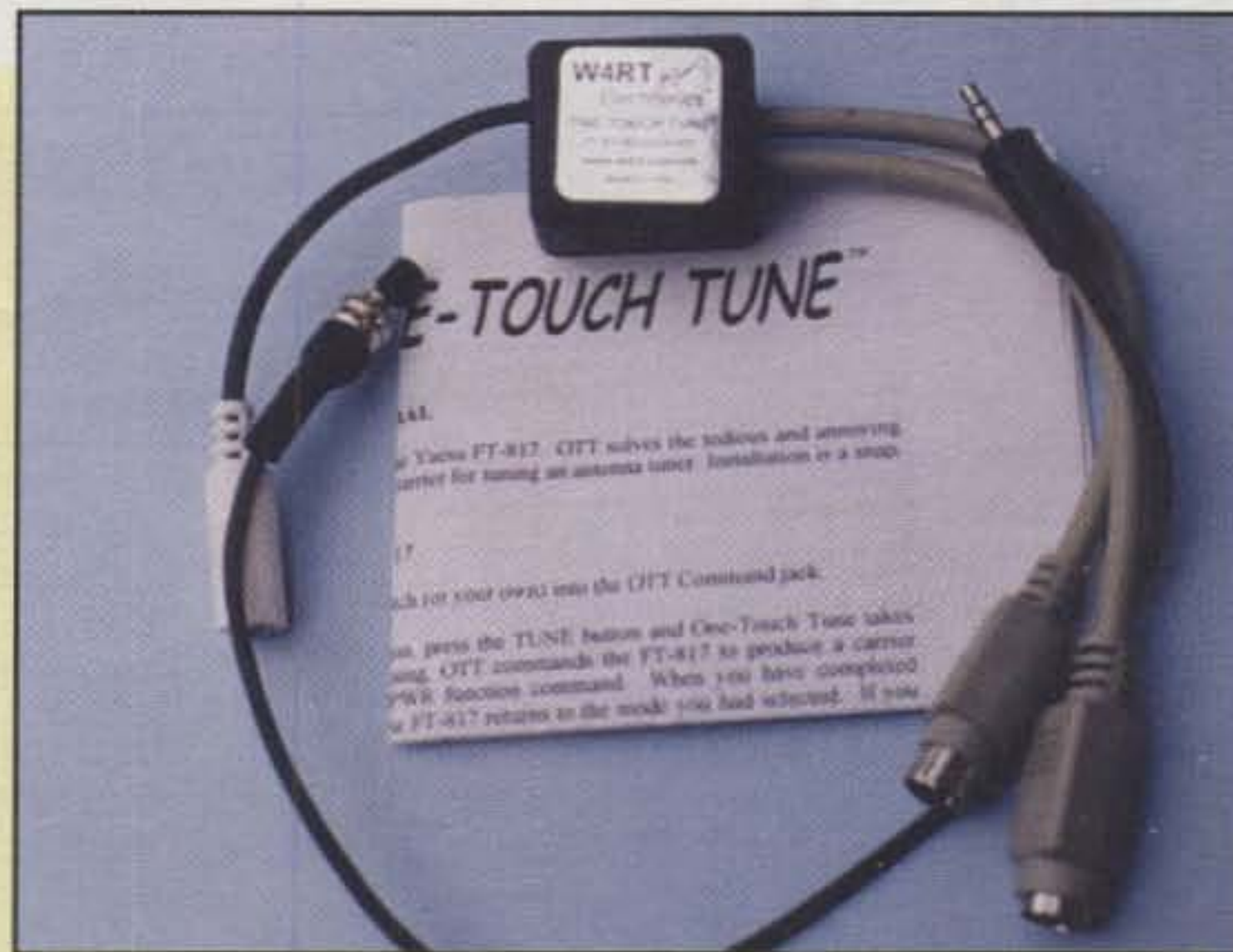
Photo 9— The new “One Touch Tune” module from W4RT Electronics. The unit plugs into sockets on the rear of the FT-817 and a press of its pushbutton or remote activation from an LDG Z11 tuner activate the rig to transmit a tune-up carrier.
