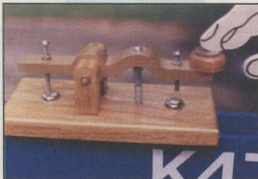
Photo 2—Close-up view of the key on the NF7E Whirligig reveals remarkable beauty. Key sports an extra-tall spring and wide gap so you can see it work from across the yard.
