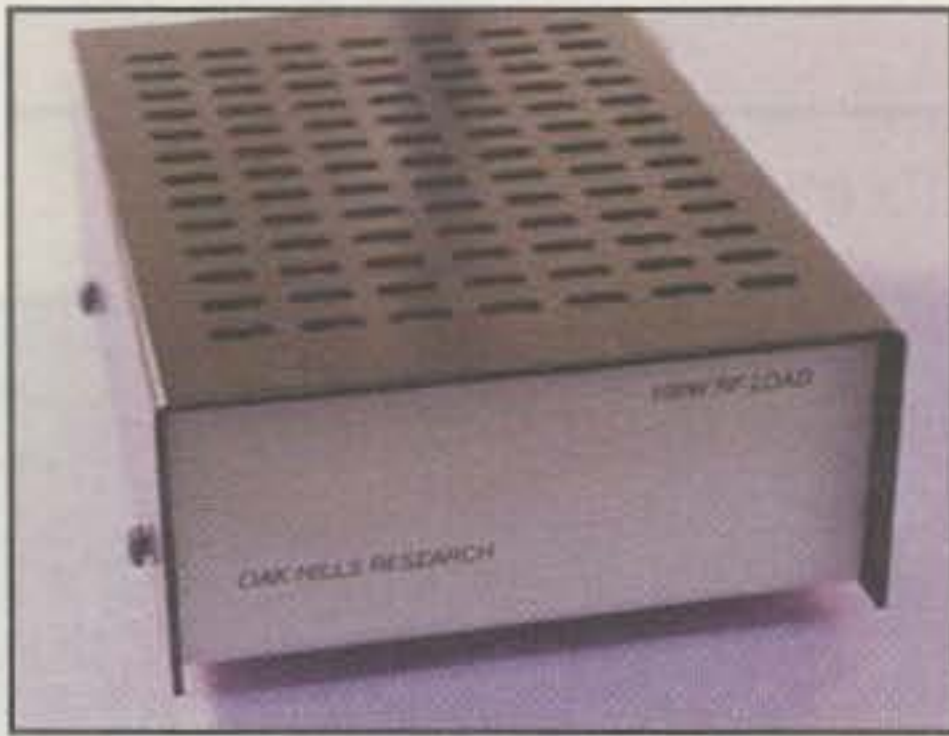
Photo C— Oak Hills Research's RFL-100 is a 100 watt RF dummy load kit for QRP (and not-so-QRP) rigs. The load kit provides a 50 ohm resistive load to 144 MHz, and offers 100 watts continuous power dissipation. (Photo from Oak Hills Research website)
