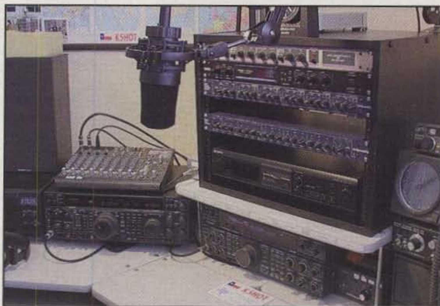
Photo A— Shown is a "stacked rack" with some high-end Symetrix audio processing products installed in the radio hamshack of David Boehner, K5HOT, as posted to the Symetrix website. The photo shows the Symetrix 528E Voice Processor and 551E 5-Band Parametric Equalizer, used with the AKG microphone and a Kenwood TS950SDX transceiver. (Photo from Symetrix website)
