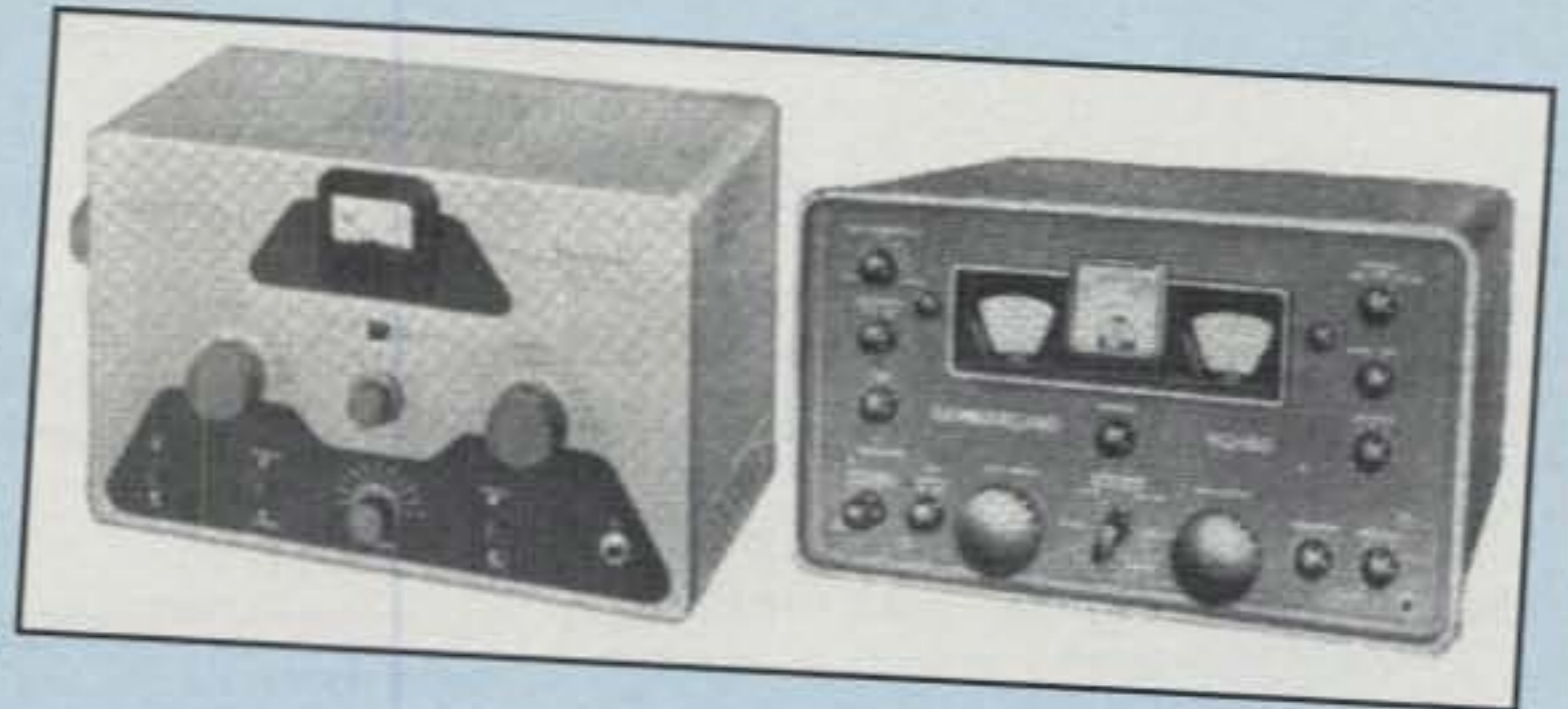
Photo B— There is no better way to enjoy CW operation on 30 meters than with an old-time transmitter and receiver. The transmitters usually sport wide-range circuits that resonate on 10.1 MHz without "mods." The receivers typically "drop down" in performance on the upper bands, but work fine on 10.1 MHz. Very nice!
