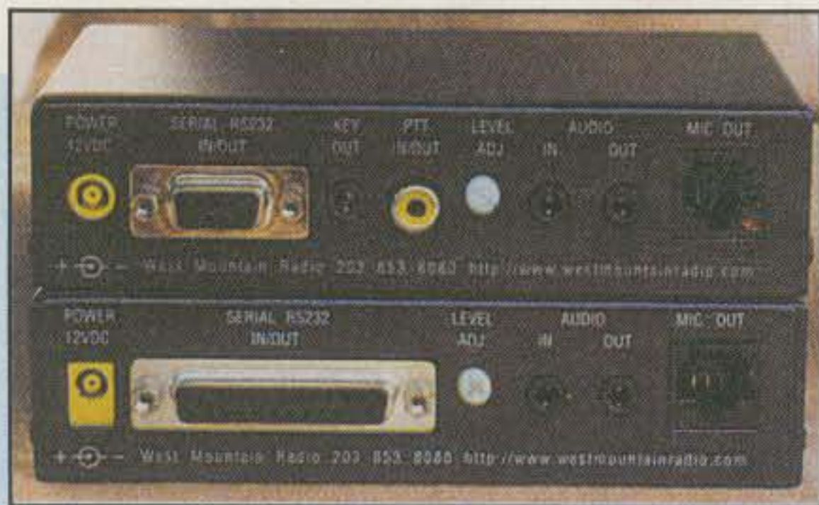
Rear view of the RIGblaster (bottom) and RIGblaster Plus (top) show additional jacks added on the Plus version. See text for details.
