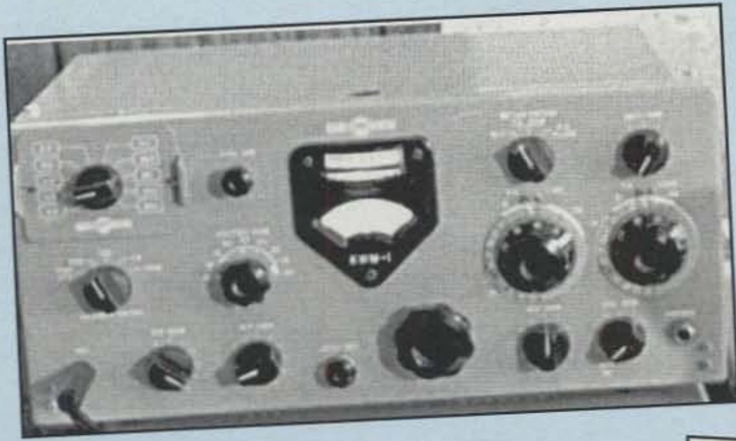
Photo A— When refurbished and modified for WARC band operation, some classic vacuum-tube transceivers produce marvelous, unequalled SSB signals. This Collins KWM-1, with its 3.1 kHz mechanical filter, is proof of that, and WARC conversion simply involves adding one crystal to its oscillator's bandswitch.
