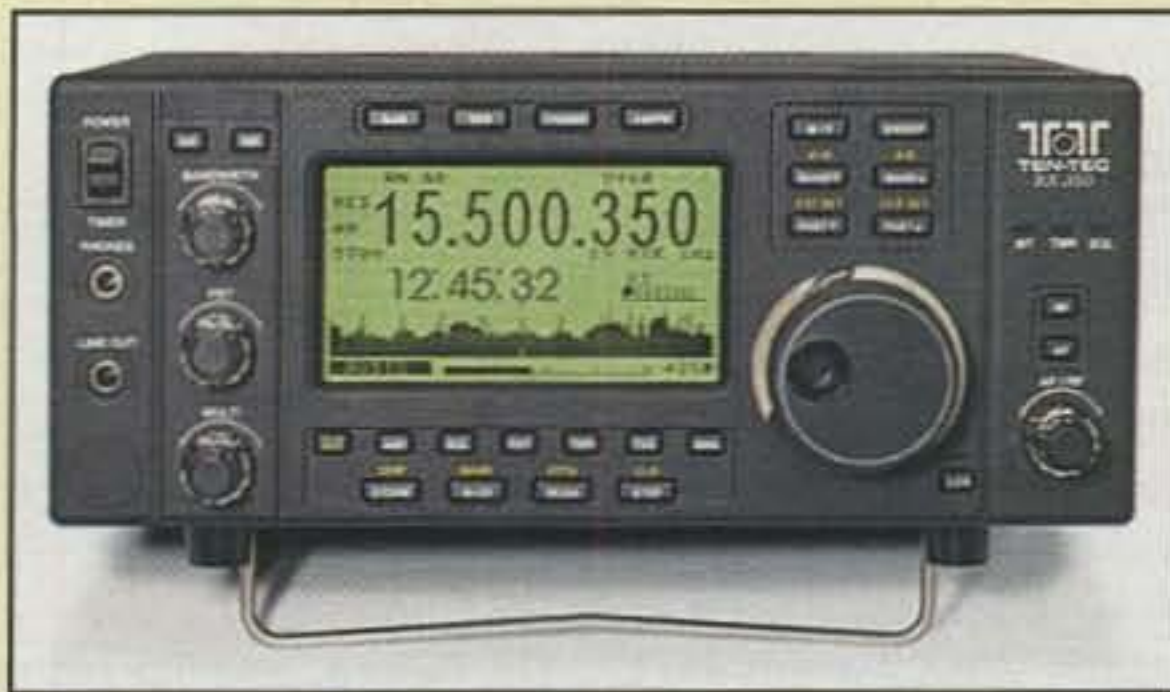
Photo A— Here's a front view of Ten-Tec's full-featured HF DSP shortwave receiver, the RX-350. The RX-350 features a clean, modern look featuring a large multifunction LCD graphics panel for display of all receiver functions, with pushbutton operation of major receiver controls from the front panel. (Photo courtesy Ten-Tec)
