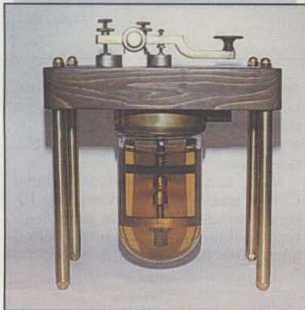
Photo 12— Some spark keys have large contacts, some even have heat sinks, but the contacts on this marvel made by The Massie Wireless Telegraph Company are immersed in a beaker of oil. The whole operating desk and the floor beneath it probably flashed when this thing was in action! (Photo courtesy K9WDY)
