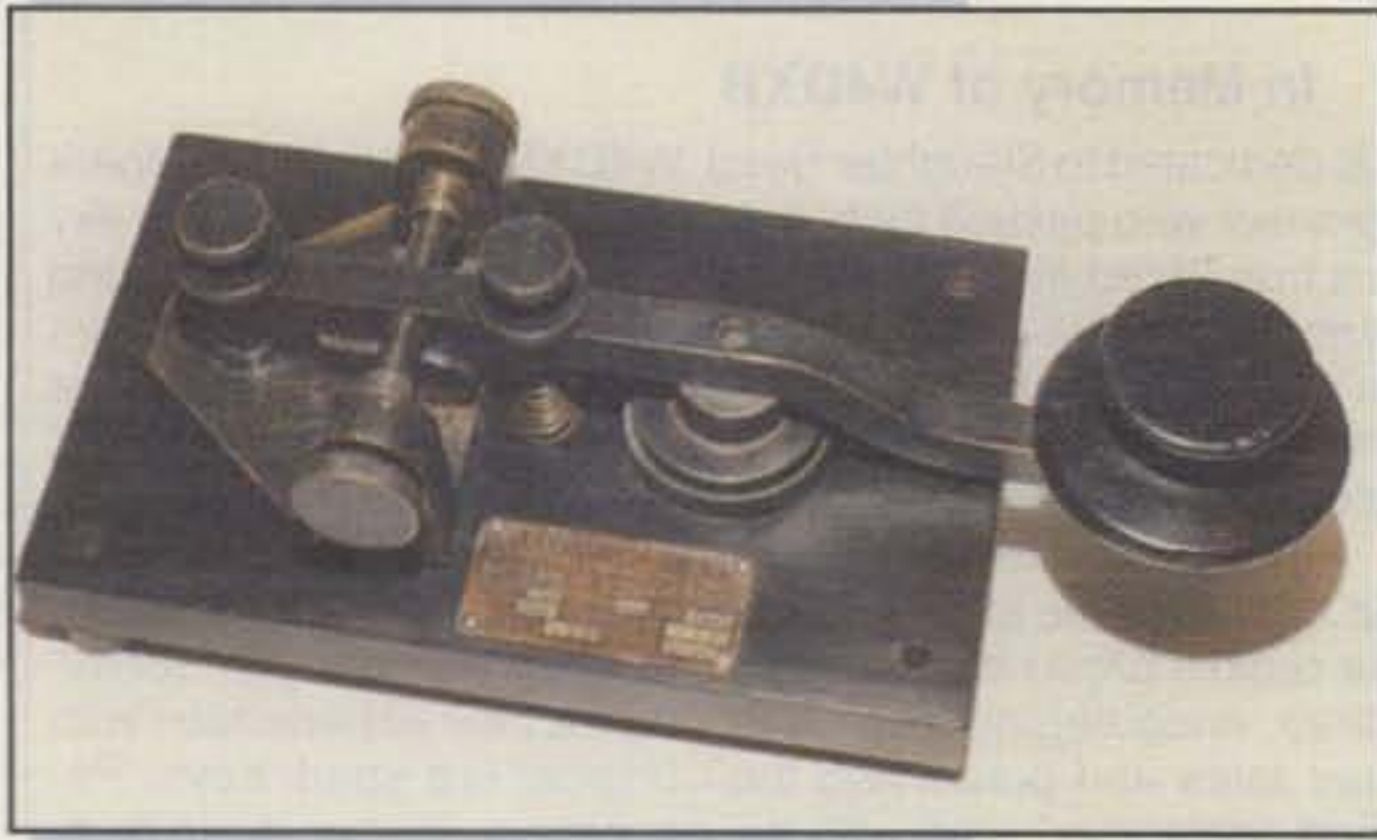
Photo 11— Spark keys such as this heavy-duty item made by the Marconi Wireless Telegraph Company of America are immediately recognized by their huge contacts. Every one is an important piece of history, and tales of use from their owners are equally important aspects of history. (Photo courtesy K9WDY)
