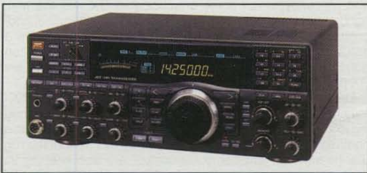
The JRC JST-245 is a powerful, almost 200 watt output transceiver that covers HF plus 6 meters and has a triple-conversion receiver and great-sounding transmit audio.
