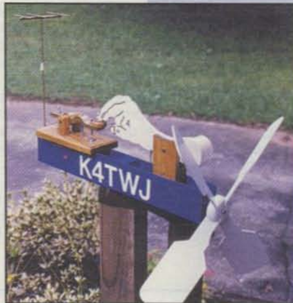
Photo 13— Here is the perfect QTH marker for your yard or driveway—a Wind Key made by Bob Wertz, NF7E. Wind turns the propeller, which drives the hand up and down to activate the key, which is a beautiful humpback type with large, wide-spaced contacts. Wind Keys are available directly from NF7E. (Details in text.)
