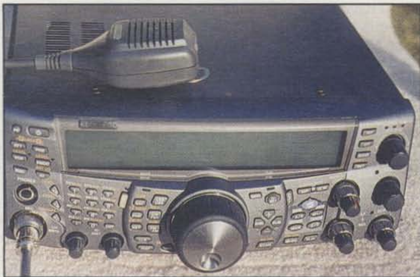
The Kenwood TS-2000 HF/VHF/UHF multi-mode base or mobile transceiver can be special ordered with the 1240–1300 MHz band factory-installed (designated the TS-2000X).
