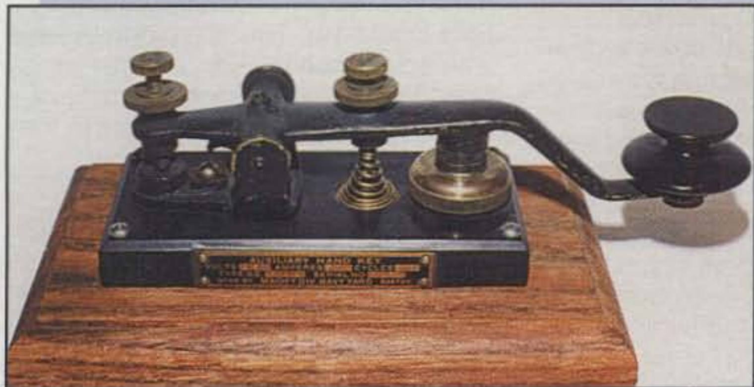
Photo 9— This rescued-from-extinction Boston Navy Yard spark key was made around 1910 and used with fire-breathing spark transmitters of the same period. Notice the massive contacts on this key. They are rated at 50 amperes and can be field-replaced when burned out from high current. (Photo courtesy master key collector Gil Schlehman, K9WDY)
