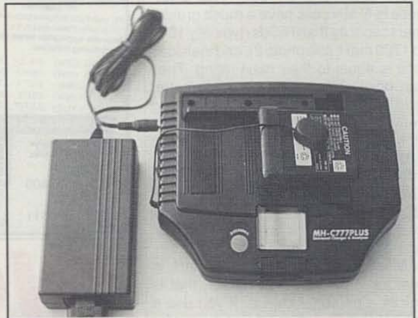
Photo 5—The Maha MHC777 Plus with sliding contacts and temperature sensor in place and charging a Kenwood PB-22 battery pack. Notice use of a pack's top contacts permits quick-charging both NiCd packs and/or battery trays filled with NiMH cells.
