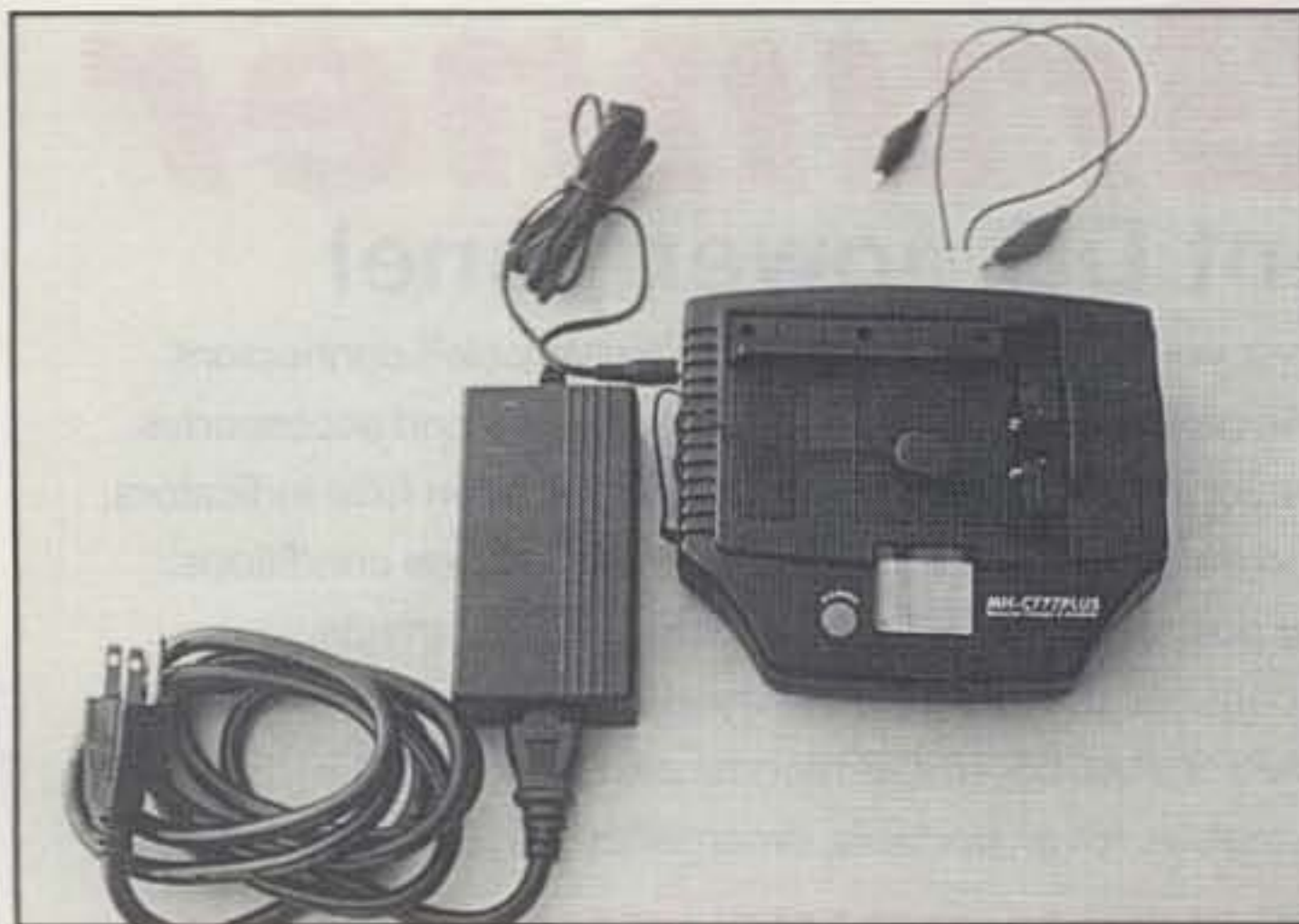
Photo 4—The Maha MH777 Plus charger sports microprocessor control, sliding contacts to mate with various battery packs, a magnetic base to hold the pack in place, and a snap-on temperature sensor. It is elaborate!
