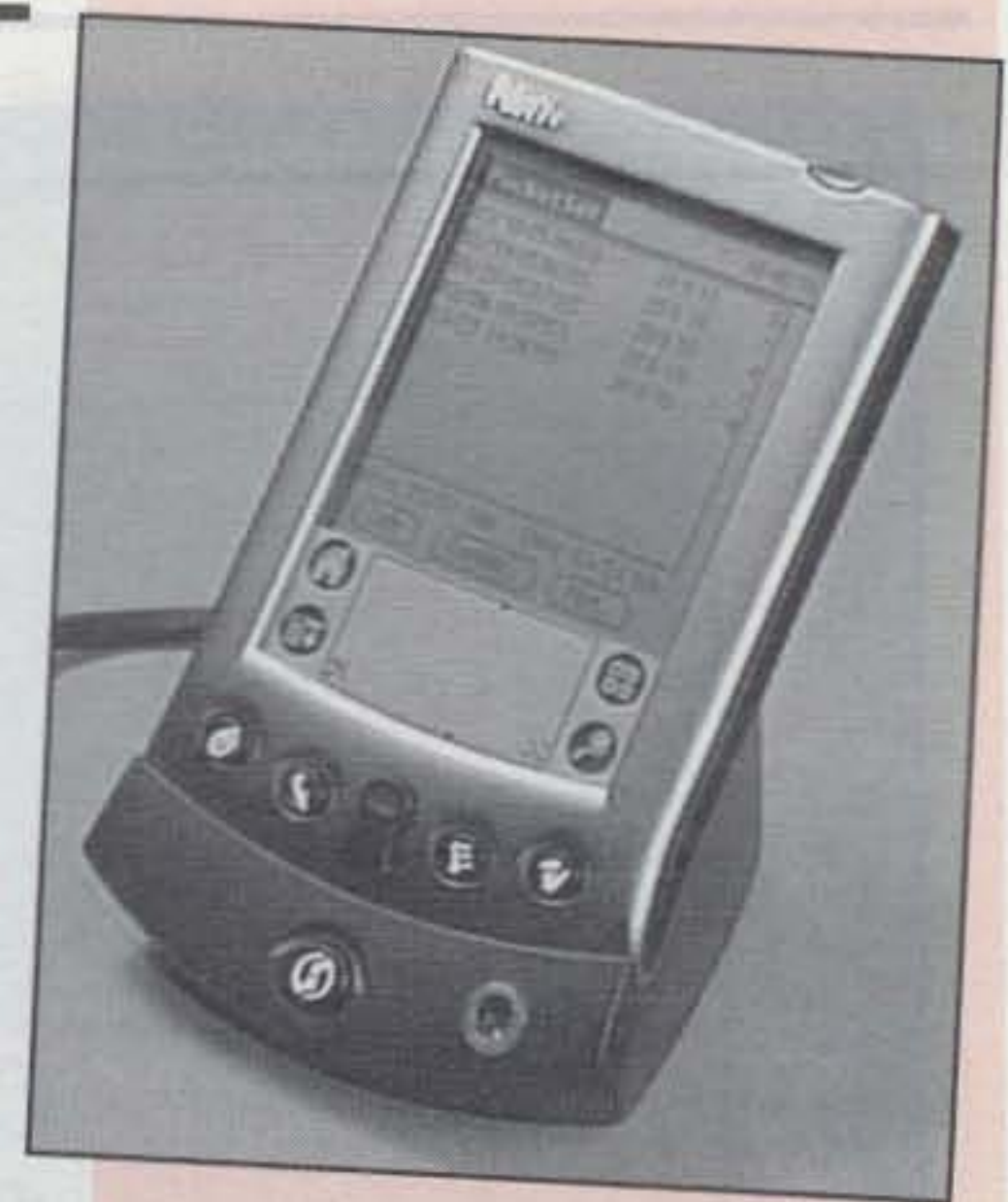
Fig. 3— The Palm inside its HotSync cradle. The cradle is used to transfer data between your computer and the Palm, via the RS-232 port. Shown on the screen is a table of International Space Station passes that will be visible from my QTH during March 2002, computed by PocketSat.
