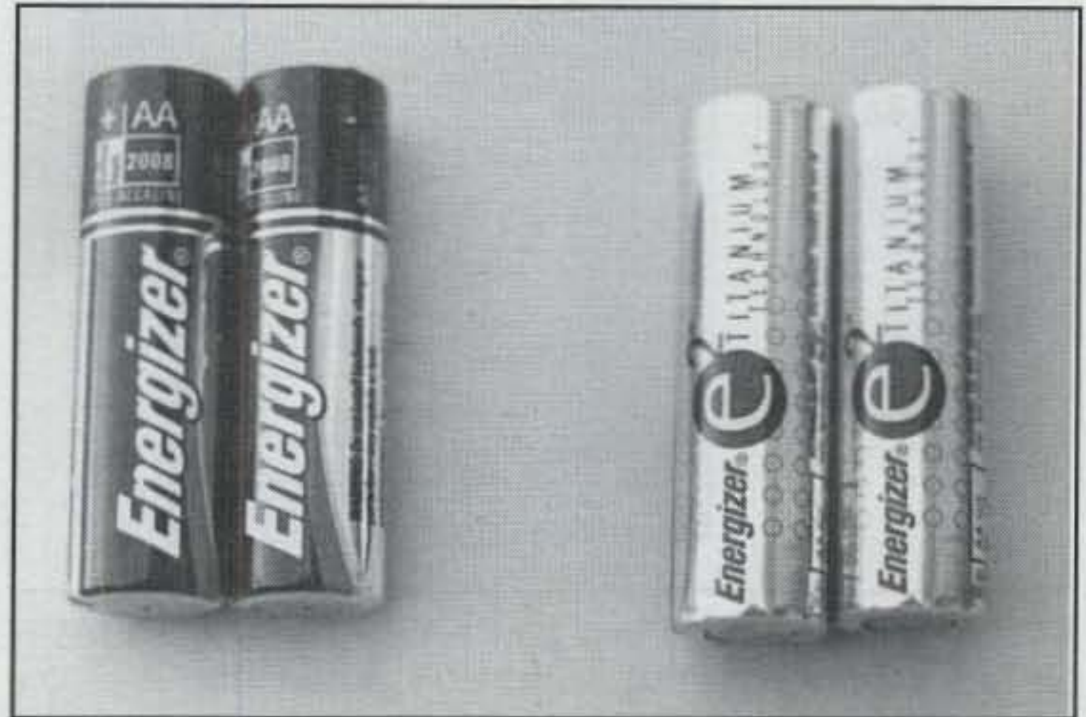
Photo 1—Two popular, stout-hearted versions of alkaline cells are Eveready's Energizer and E 2 Titanium shown here. Both types have the same total capacity of 2850 maH, but the E 2 Titanium is designed for heavier current loads and thus is more attractive for use in high-power talkies and transceivers.
