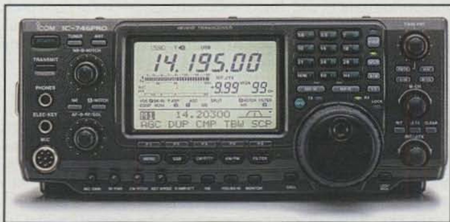
ICOM has upgraded the IC-746 to an IC-746 PRO, adding 32-bit IF-DSP, variable-level noise blanker, SSB/CW synchronous tuning, selectable digital IF filters, automatic notch filter, and even a built-in RTTY demodulator and decoder.
