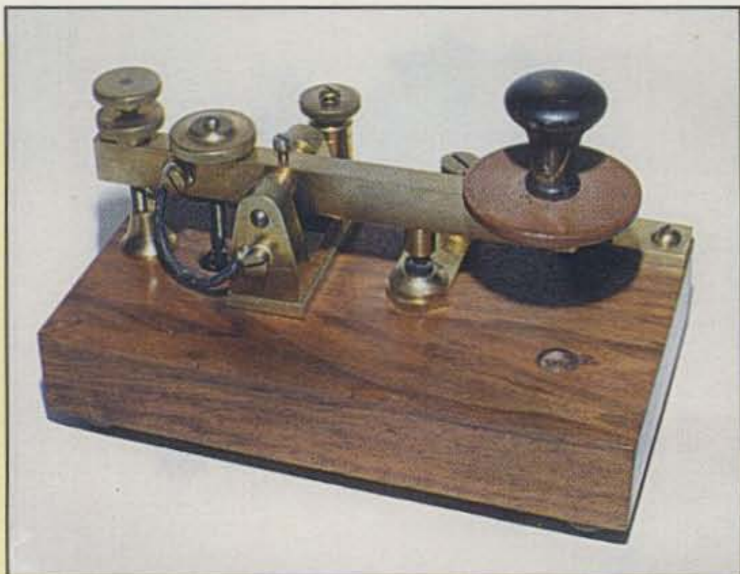
Photo 6— This DuCretet and Rogers pump key glows with the look of old-time telegraphy in a European railroad depot. The fulcrum assembly and rear “pull down” tension spring in particular reflect classic British influence.
