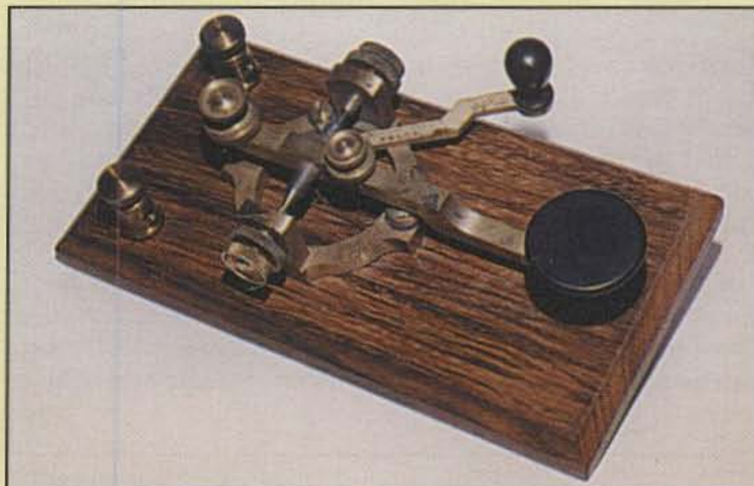
Photo 5— The look of old wild west telegraphy flourishes from every viewing angle of this classic Patrick and Carter hand key. Notice its oval base, pressed-into-arm trunion/pivot pin, and step-lever arm, all indicative of a pre-1900 item.
