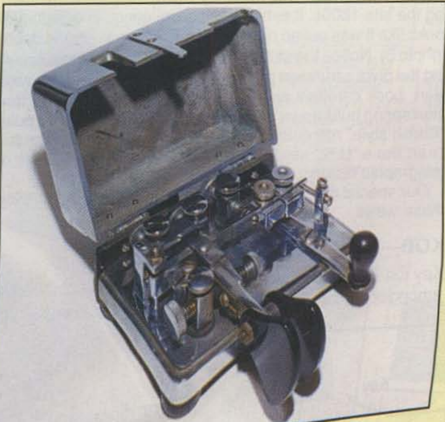
Photo 3— This palm-size bug was designed by a railroad telegrapher during the 1920s, and a small number were made for landline telegraphers and radio amateurs. and you will see it is akin to a regular telegraph key and around each other to reduce the complexity of the key collector
