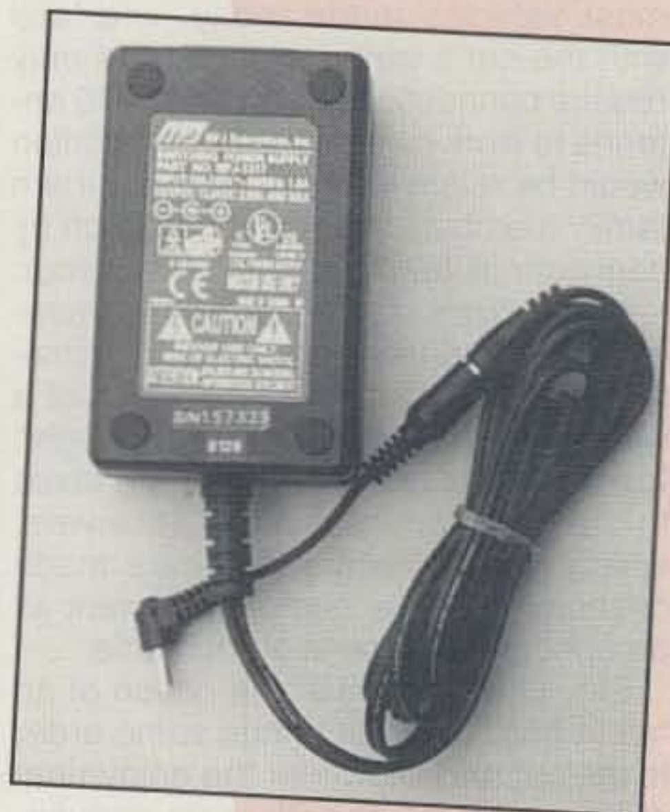
Photo 1— The new pocket-size MFJ-1317 switching-type power supply is a gem! Unit measures only 1.4"H x 2.5"W x 4.0"D and delivers 13.8 volts DC at up to 2.89 amps—enough "juice" to power all your QRP gear simultaneously. Power supply is also equipped with a cable and mini-coaxial plug to fit the FT-817.
