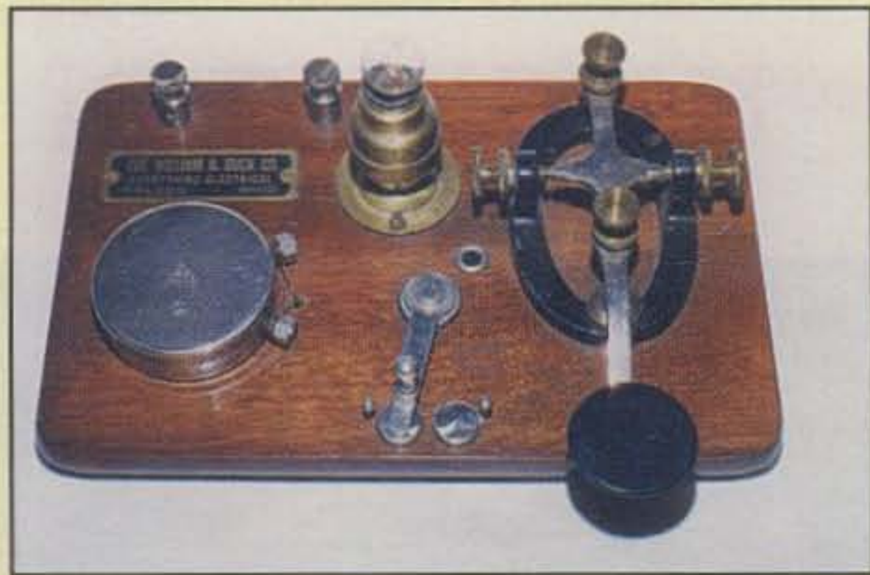
Photo 9— This later KOB with buzzer was designed more for radio than telegraph practice and was made by the William B. Duck Company. This famous manufacturer was also well known for its loose couplers, crystal sets, and other spark-era apparatus.
