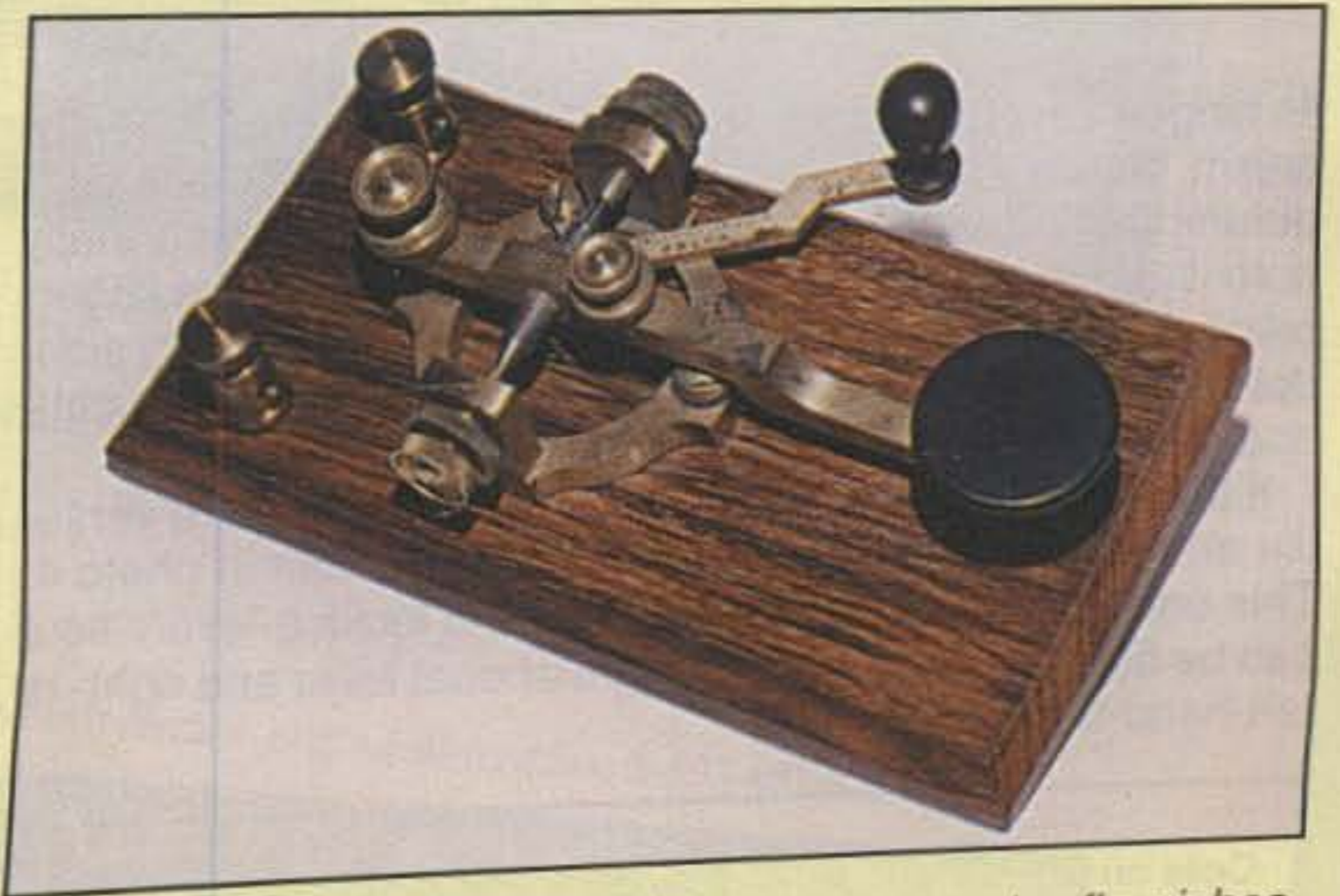
Photo 5— The look of old wild west telegraphy flourishes from every viewing angle of this classic Patrick and Carter hand key. Notice its oval base, pressed-into-arm trunnion/pivot pin, and step-lever arm, all indicative of a pre-1900 item.
