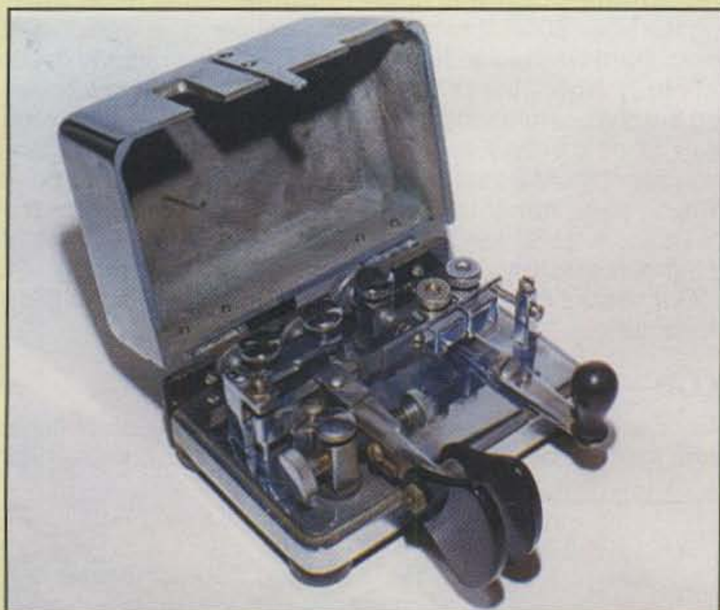
Photo 3— This palm-size bug was designed by a railroad telegrapher during the 1920s, and a small number were sold to both landline telegraphers and radio amateurs. Study the mechanism, and you will see it is akin to a regular bug with its parts folded around each other to reduce size. (Photos 3 through 9 courtesy dedicated key collector Gil Schlehman, K9WDY)
