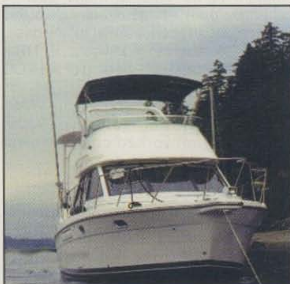
Photo A— Fluidmotion Antenna Systems has introduced its SteppIR series remotely adjustable antennas, which are available as a dipole (shown here being used as a vertical antenna on a boat) or as a 2- or 3-element Yagi. The antennas are unique in that they allow for continuous frequency coverage between 20 and 6 meters. Price ranges from about $440 for the dipole to $1000 for a 3-element beam. (Photo from the Fluidmotion website)
