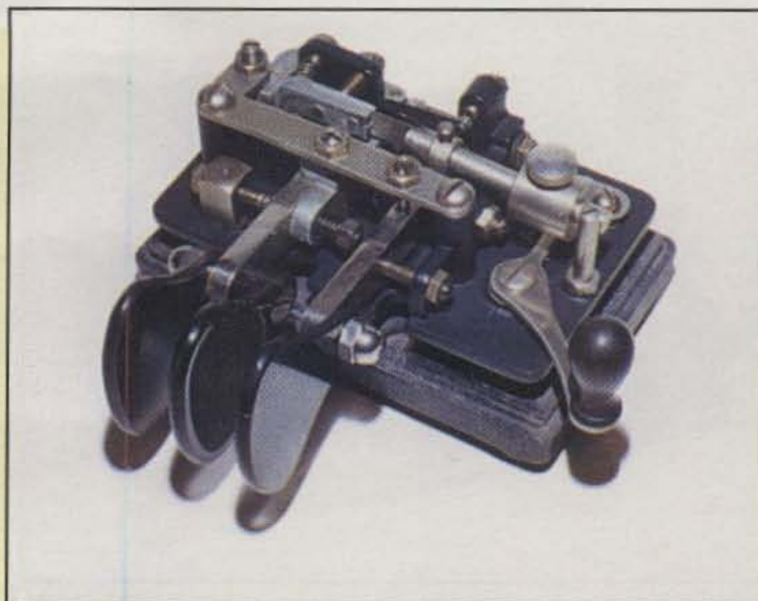
Photo 4— A slightly later version of the 73 bug with its cover fully removed for study. Notice this version's mechanism is similar to the earlier version, but includes interchangeable parts that can be shifted around or "field configured" to produce a single- or dual-lever, right- or left-hand bug.
