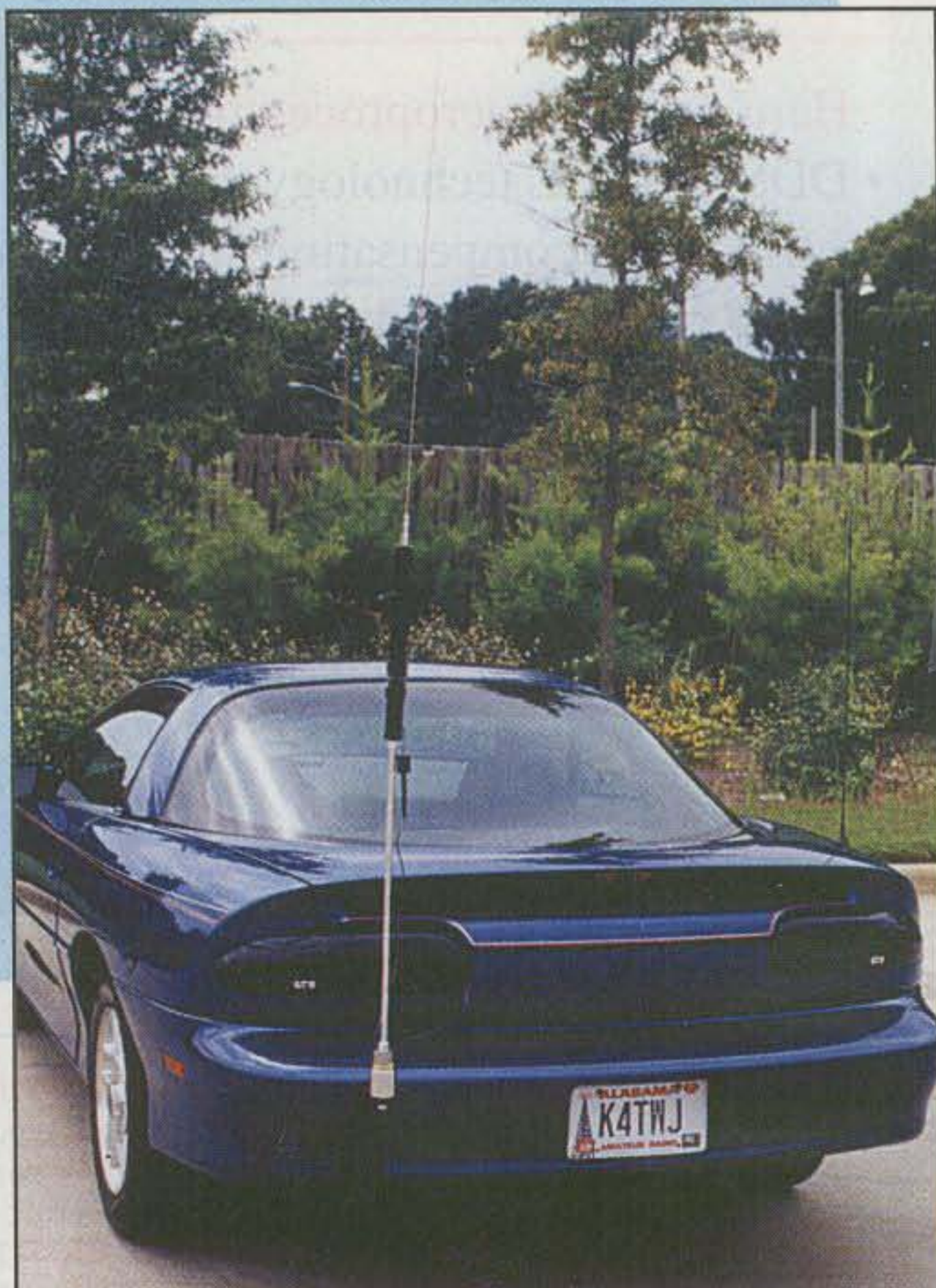
Photo 1— Red hot and cooking best describes the appearance and performance of the new tall version of the W6MMA Super Antenna. It stands 9 feet high from street to tip, covers 40 through 6 meters, and gives my Camaro real globe-spanning horsepower.
