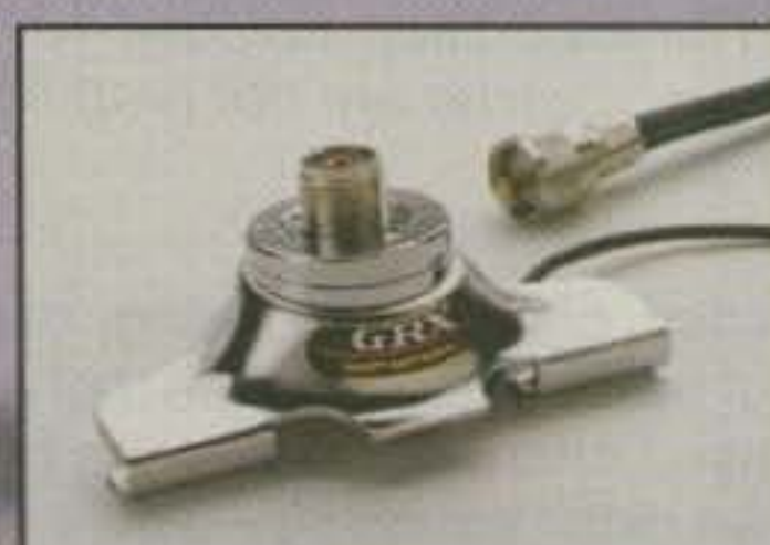
COMET GR-5M Low-profile, stainless steel trunk lip mount. Offset washers provide for up to 17 deg vertical adjustment of antenna. 16'9" of deluxe cable included, 18" mini RG-188A/U style coax for easy entry thru the weather seal. Gold-plated SO-239/PL-259 connectors.
