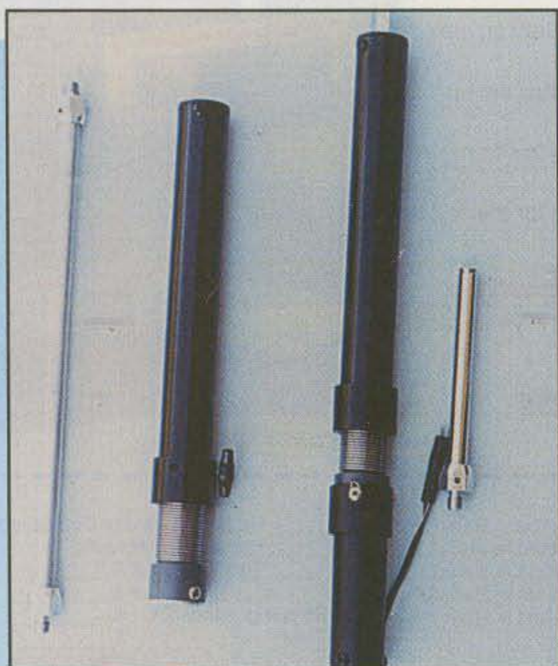
Photo 2— The sections used to make a break-down and carry-anywhere version of the W6MMA Super Antenna include (left to right) 12 inch base mast, 12 inch MP1 or 18 inch MP2 coil, and 44 inch/5 inch pull-up whip. (Discussion in text.)
