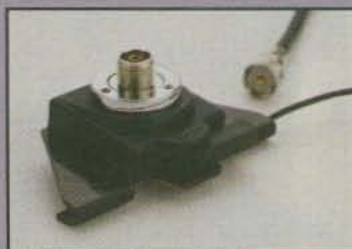
COMET CQ-5M Low-profile, "quick-disconnect" trunk lip mount. For quick storage, or theft prevention, the antenna and connector are disengaged from the mount base with the release of a lever. Offset washers provide up to 17 deg vertical antenna adjustment. Includes 16'9" of deluxe cable, 18" of mini RG-188A/U style coax for easy entry thru the weather seal. Gold-plated SO-239/PL-259 conns.
