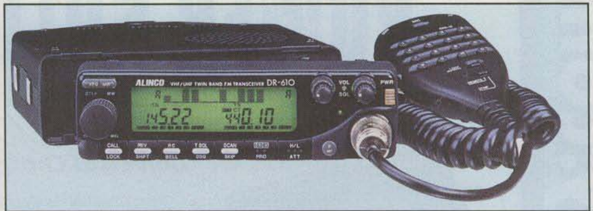
One of the advantages of a detachable head is that you can mount the "box" that contains the radio under a seat, in the trunk, or under the dash. The Alinco DR-610T VHF/UHF FM dual-band mobile/base transceiver allows you to do just that. (Photo courtesy Alinco)
