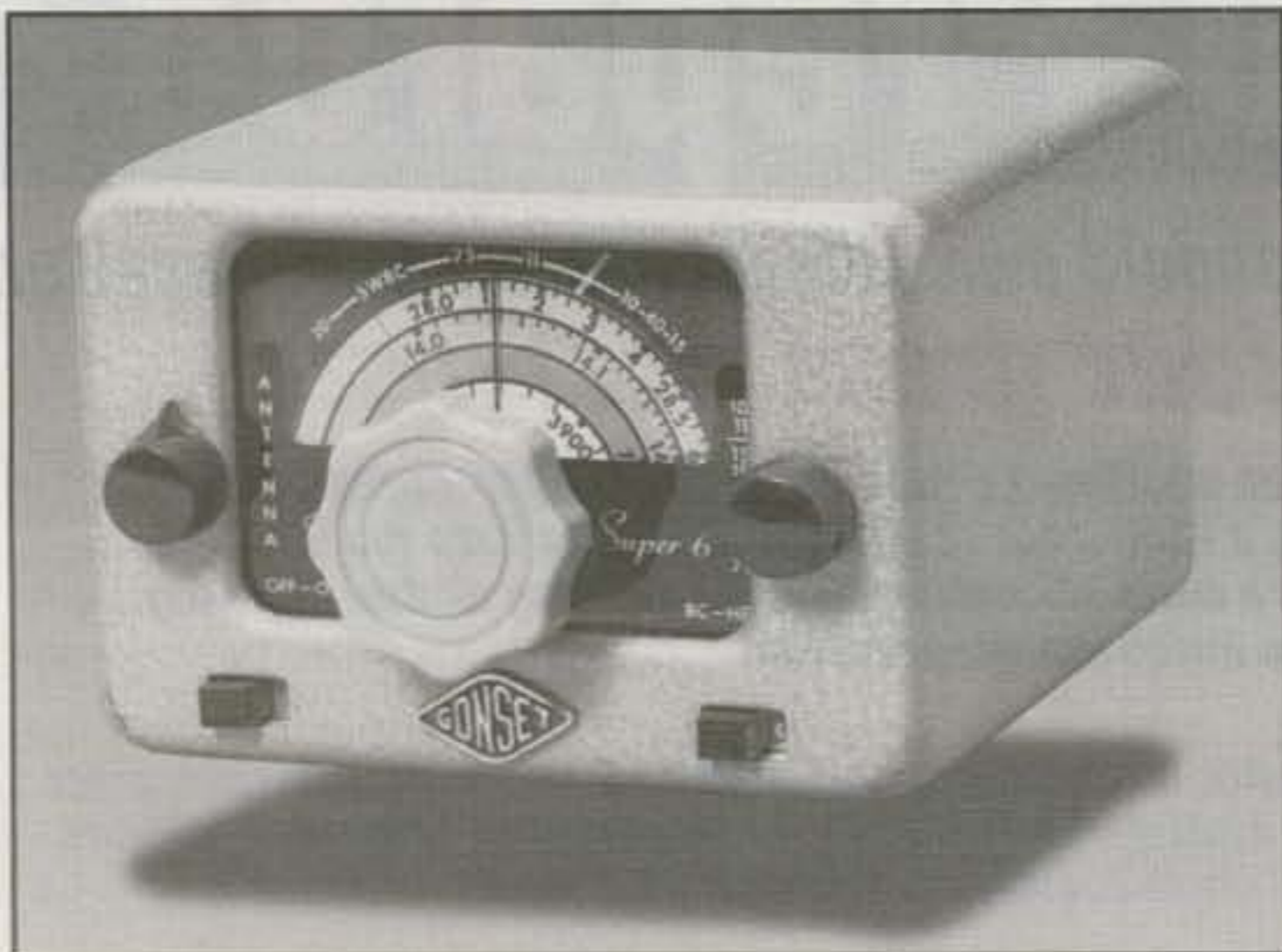
Photo 2—Gonset Super 6. Whether strapped to the steering column or mounted beneath the dashboard, Gonset converters were a mainstay of early mobile operation.
