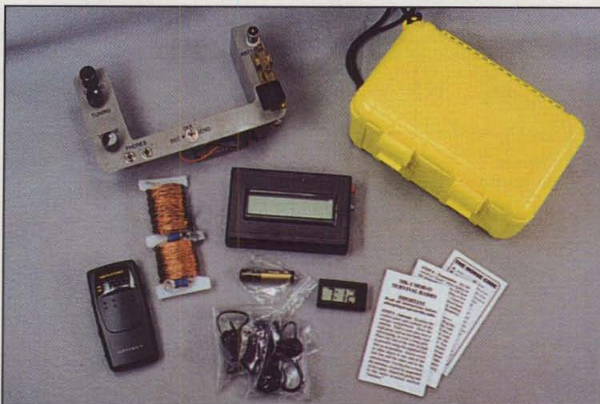
Photo 2— A closer look at the various items in the Survival Radio package built by KA6IRL. The mainframe houses the trans-receiver. Supporting items such as antenna wire, Code Reader, etc., are stored in the center cut-out. Operating instructions are in the box lid.
