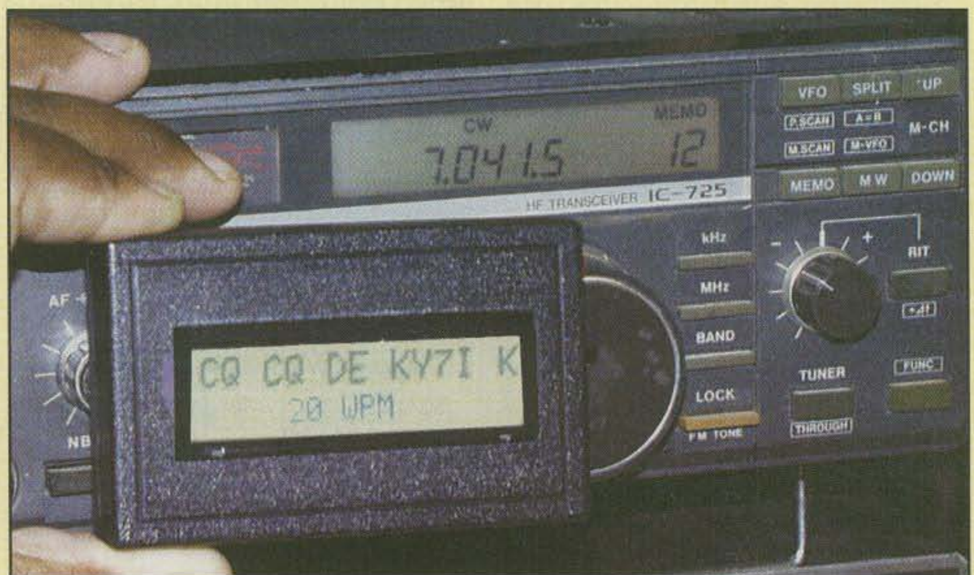
Photo B— The MFJ-461 Pocket Size Morse Code Reader lets you watch CW turn into solid text messages as the messages scroll across an easy-to-read LCD display. There are no cables to hook up, and no computer or interface is required. Simply place the unit close to your receiver speaker until the lock LED flashes in time with the CW! (Photo courtesy MFJ Enterprises)
