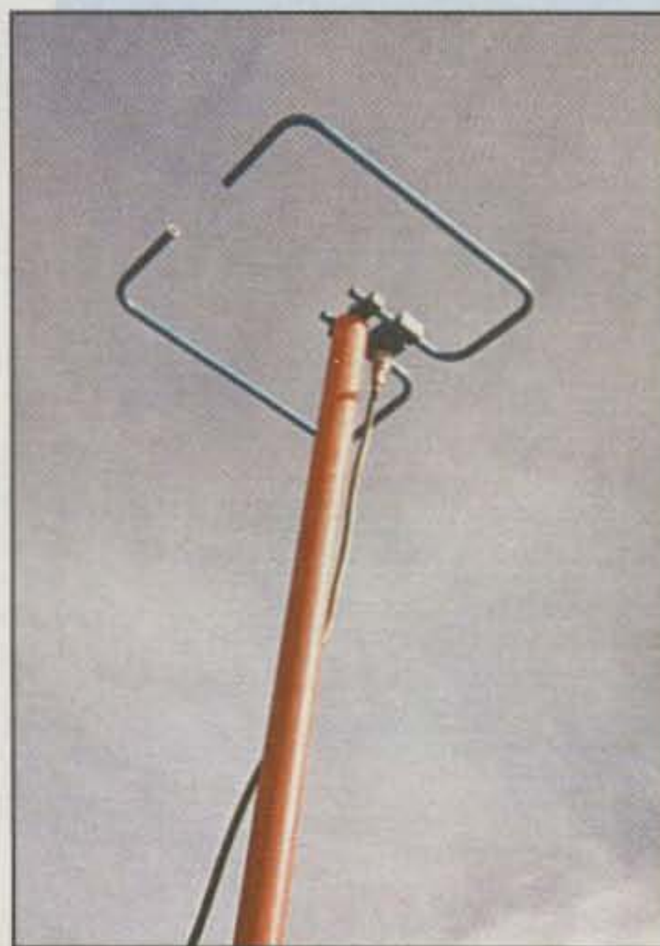
Loop antennas don't have to be round! This M 2 Sqloop is an omnidirectional, horizontally polarized antenna suitable for mobile or fixed use.
