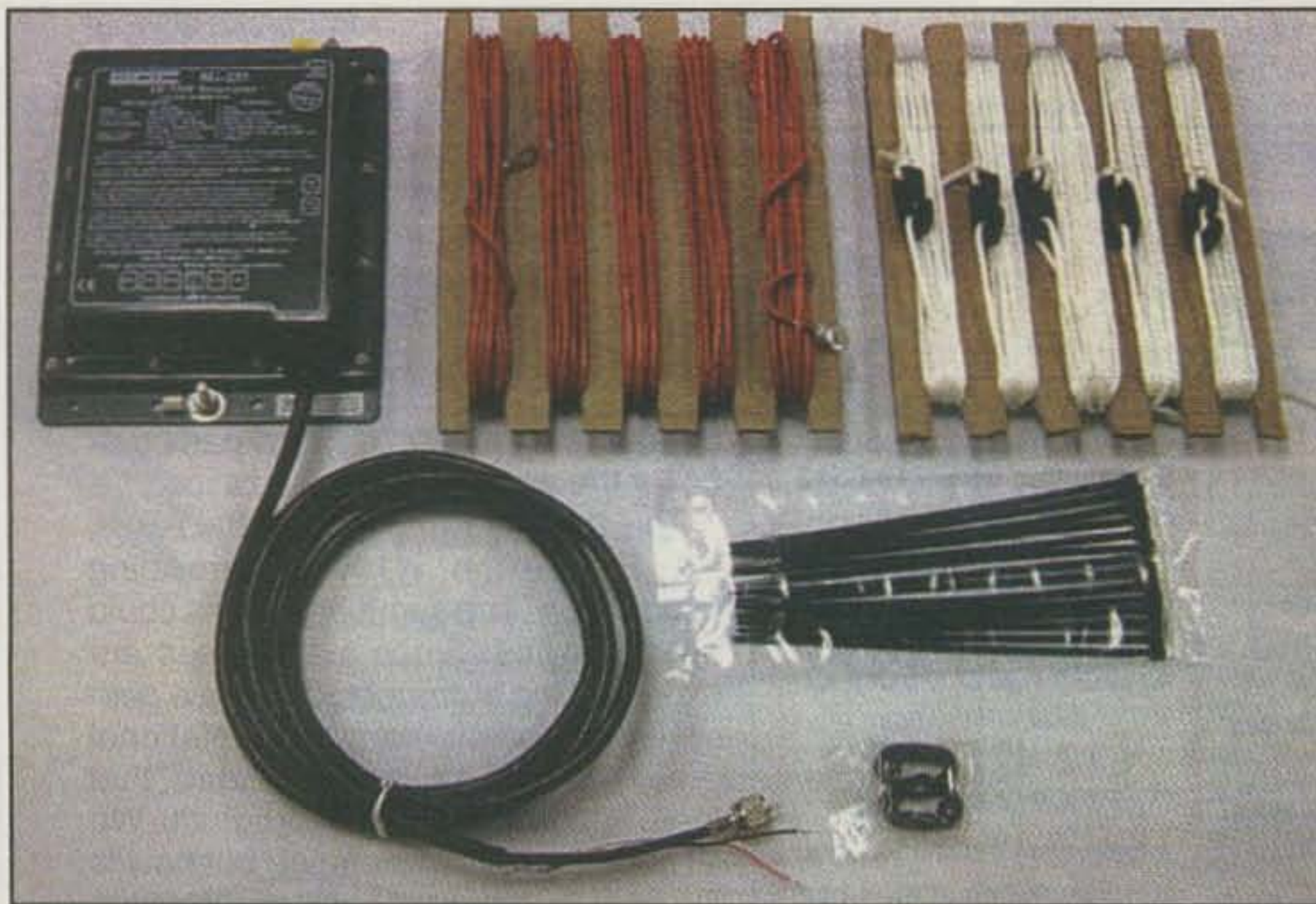
Photo D— The new configure-as-necessary Stealth portable and emergency antenna kit introduced by SGC at Dayton 2002. Kit contains SG-237 Automatic Antenna Coupler, 80 feet of insulated wire, 30 feet of support rope, 20 feet of pull-up rope, six antenna mounting clips, 12 cable ties, and instruction manual. (Photo courtesy SGC)
