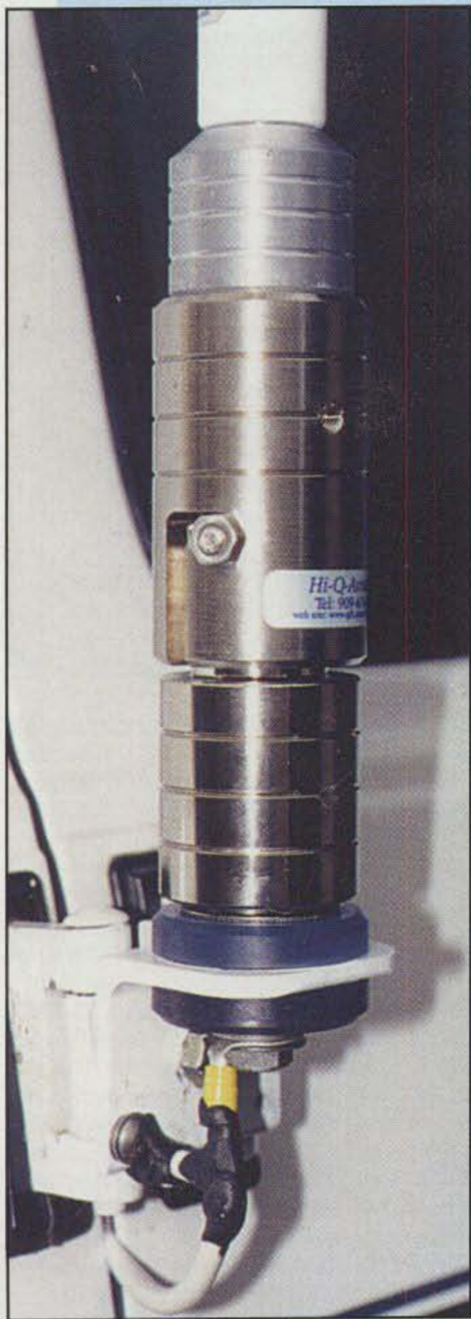
Coax Seal™ protects the coax "Y" connection.
