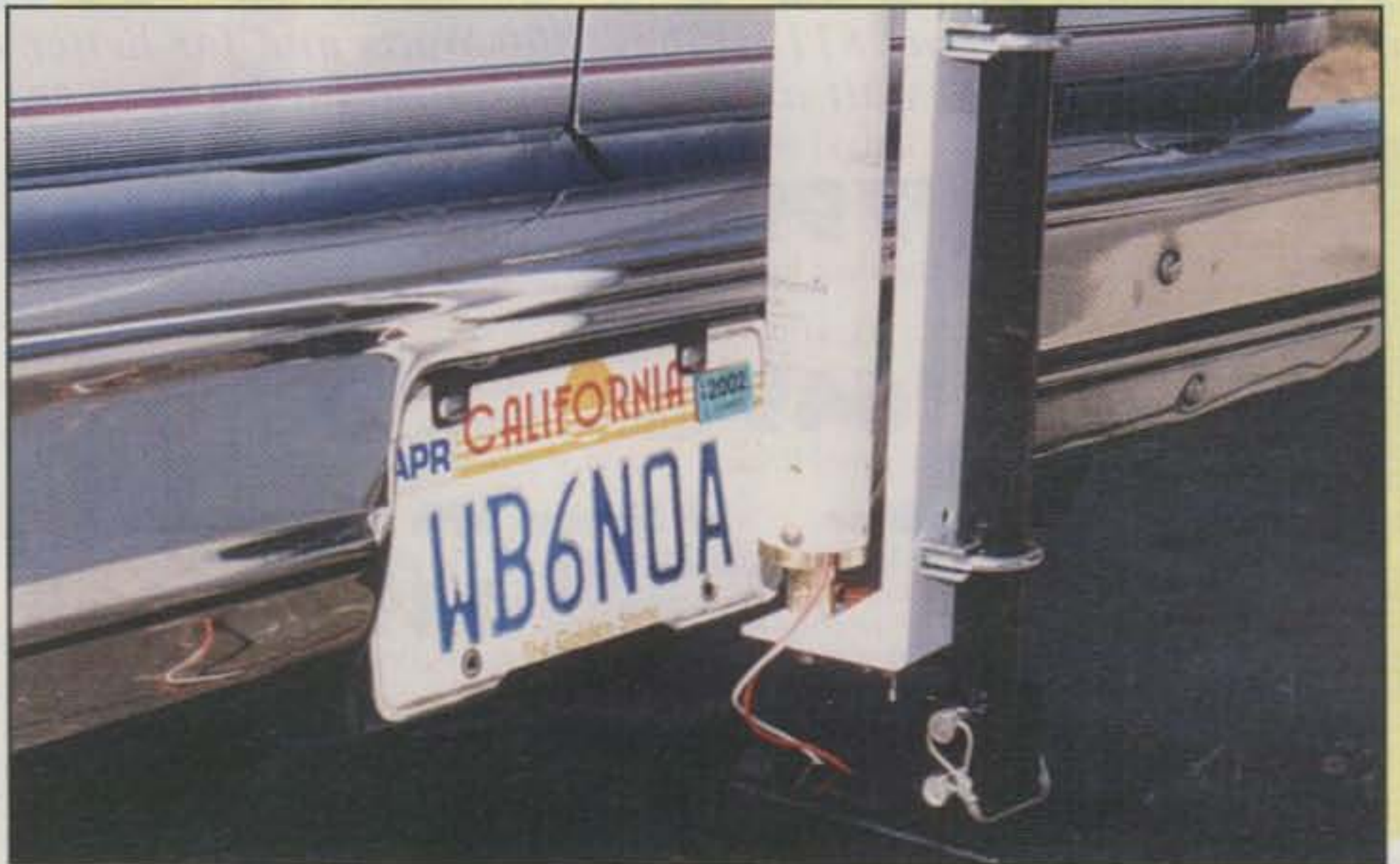
The antenna base mounts securely to the trailer-hitch receiver on the back of WB6NOA's van, which also provides an excellent point for a solid ground connection. A good ground to the vehicle chassis is essential for mobile use.
