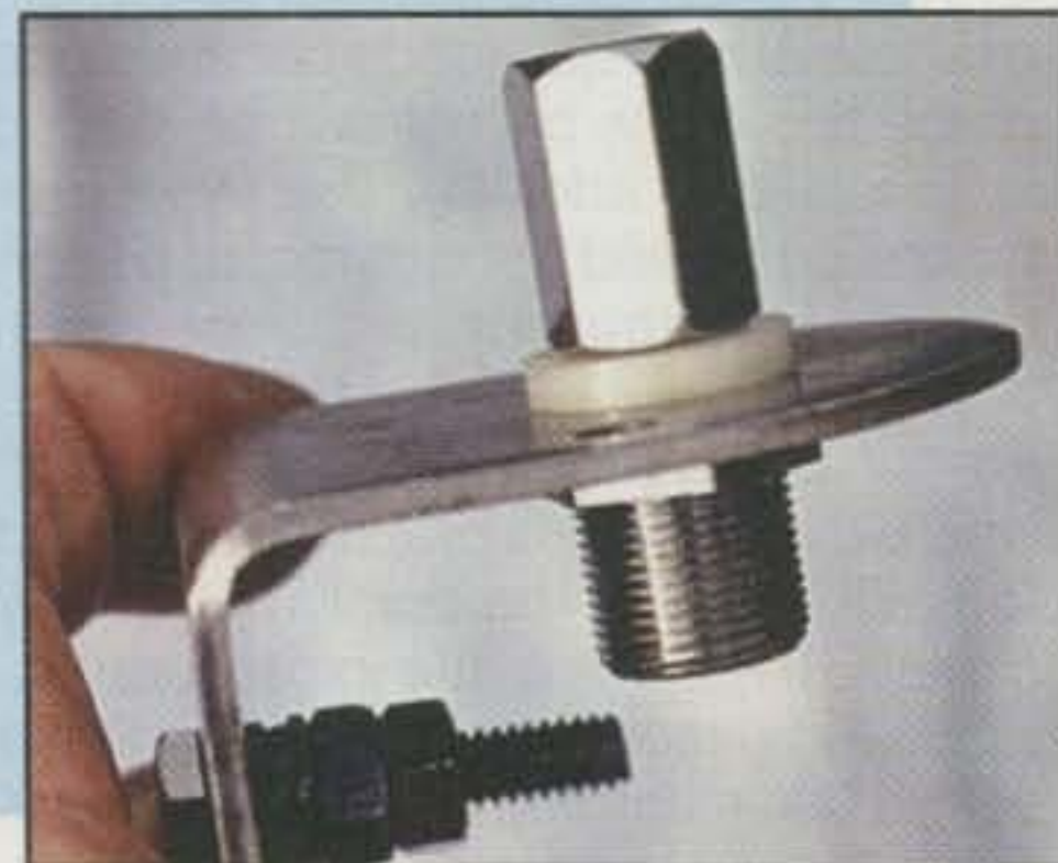
The typical, popular "L" mount with SO-239 stud adapter.
