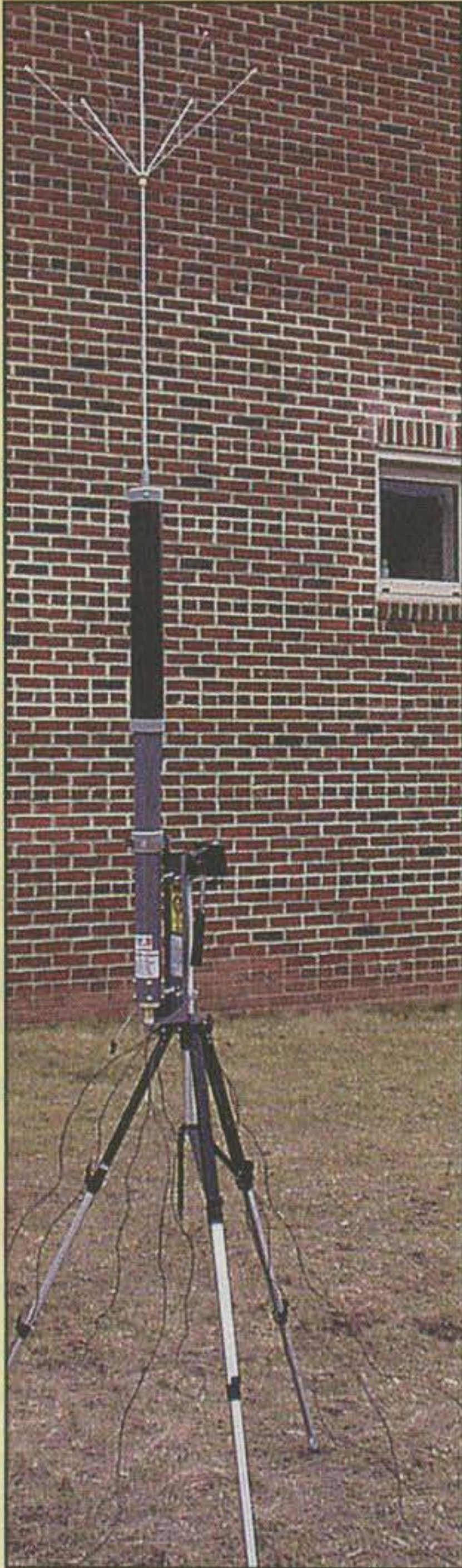
The fixed-station version of the HS-1500 MkII, the MVA, sets up quickly and easily on just about anything, including a camera tripod. (W2VU photo)
