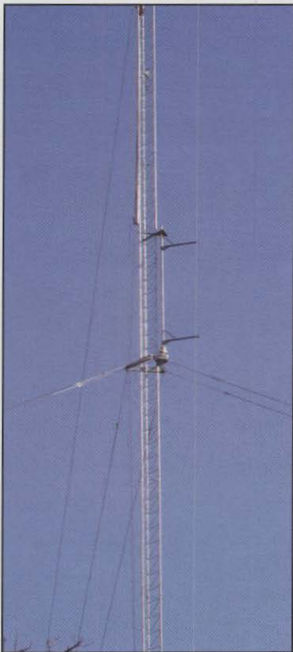
Photo B— The side arm incorporates a torque arm stabilizer.
