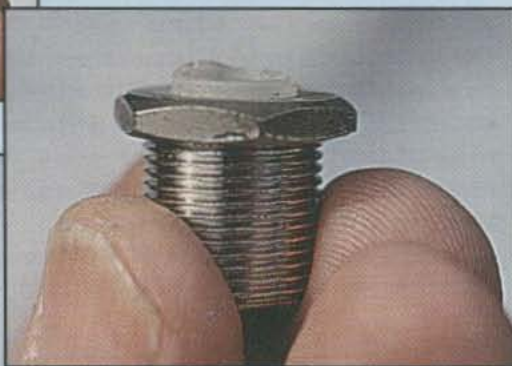
The stud failure point with tall whips at highway speeds.
