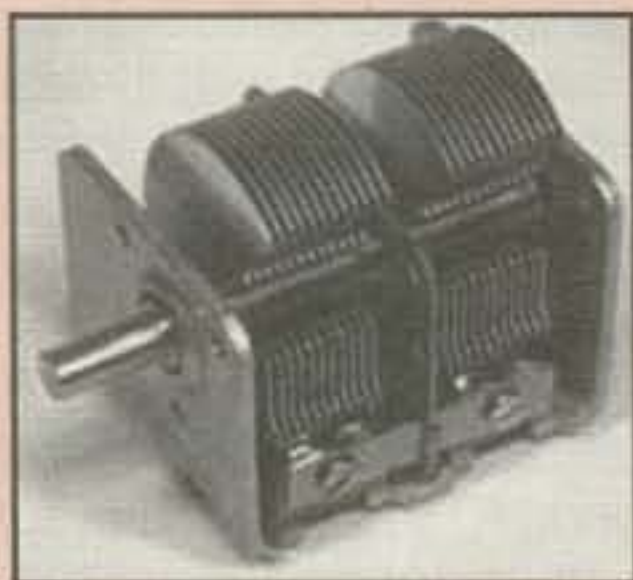
Photo A— In addition to an excellent newsletter and a large selection of books, the Crystal Set Society offers a wide array of special crystal-set-related items such as this custom-made dual-section 365 pF tuning capacitor. The "XSS" is one-stop shopping for sure.
