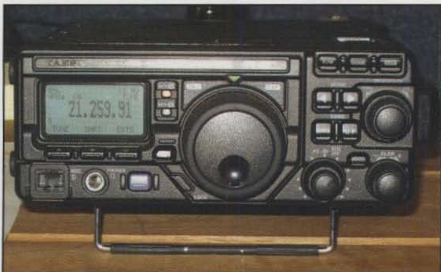
Yaesu's new FT-897, described as "an FT-817 on steroids," was one of the hits of the show. It puts out up to 100 watts when connected to conventional power sources or 20 watts on its internal NiMH batteries. The radio covers 160 meters – 70 centimeters (minus 222 MHz).
