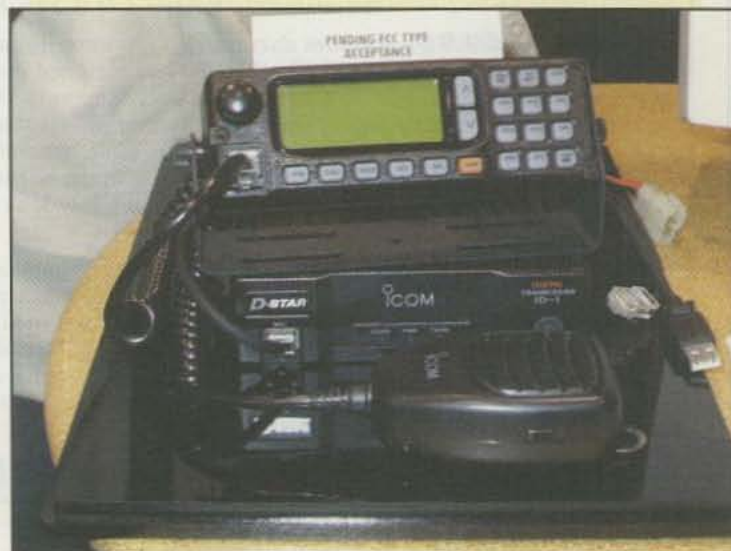
ICOM's new ID-1 digital transceiver operates on 1296 MHz as part of the new D-Star digital network that the company has been developing in conjunction with the Japan Amateur Radio League.
