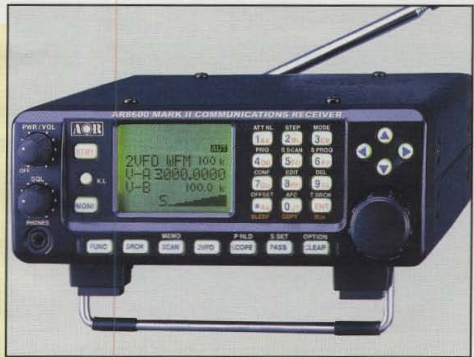
AOR's AR-8600 Mark II is a wideband receiver covering 100 kHz to 3 GHz (minus cellular). An optional NTSC video module will allow you to watch the TV signals it picks up.
