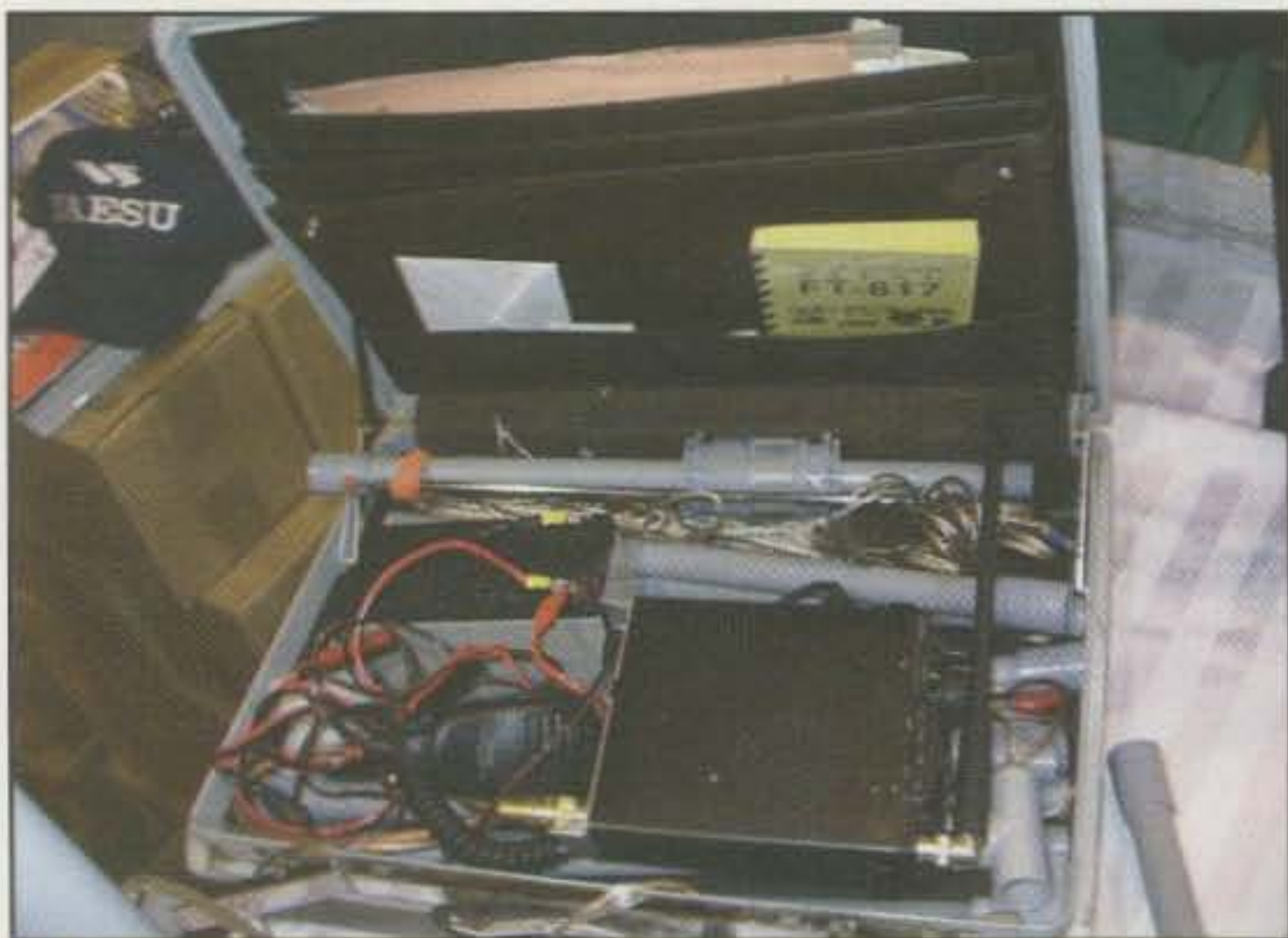
The new Minuteman antenna can be broken down, folded up, and put into a briefcase as part of an all-band "go kit" for emergencies.
