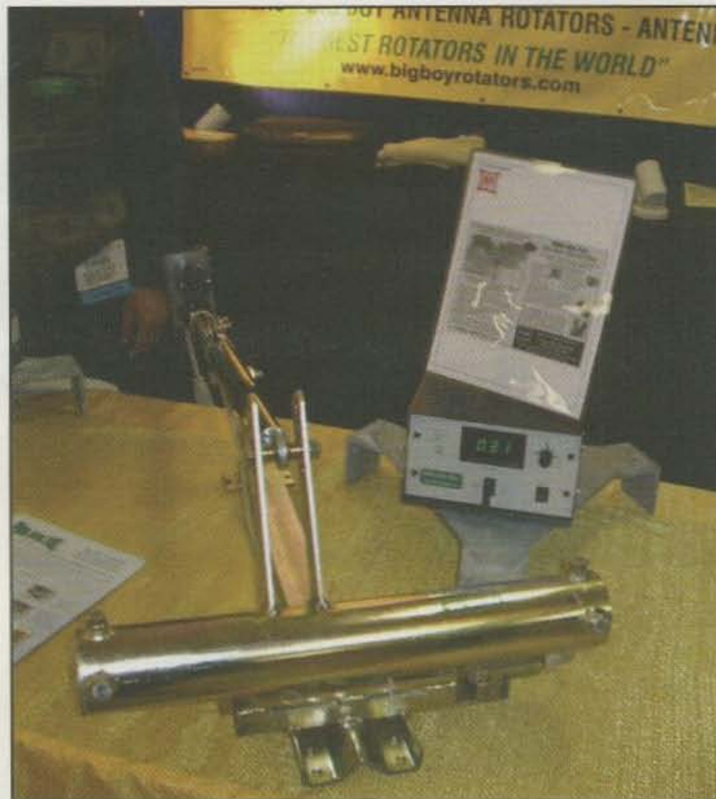
Pro.Sis.Tel of Italy has introduced its new PST 75-18 elevation rotator for EME (Earth-Moon-Earth) and satellite communications.
