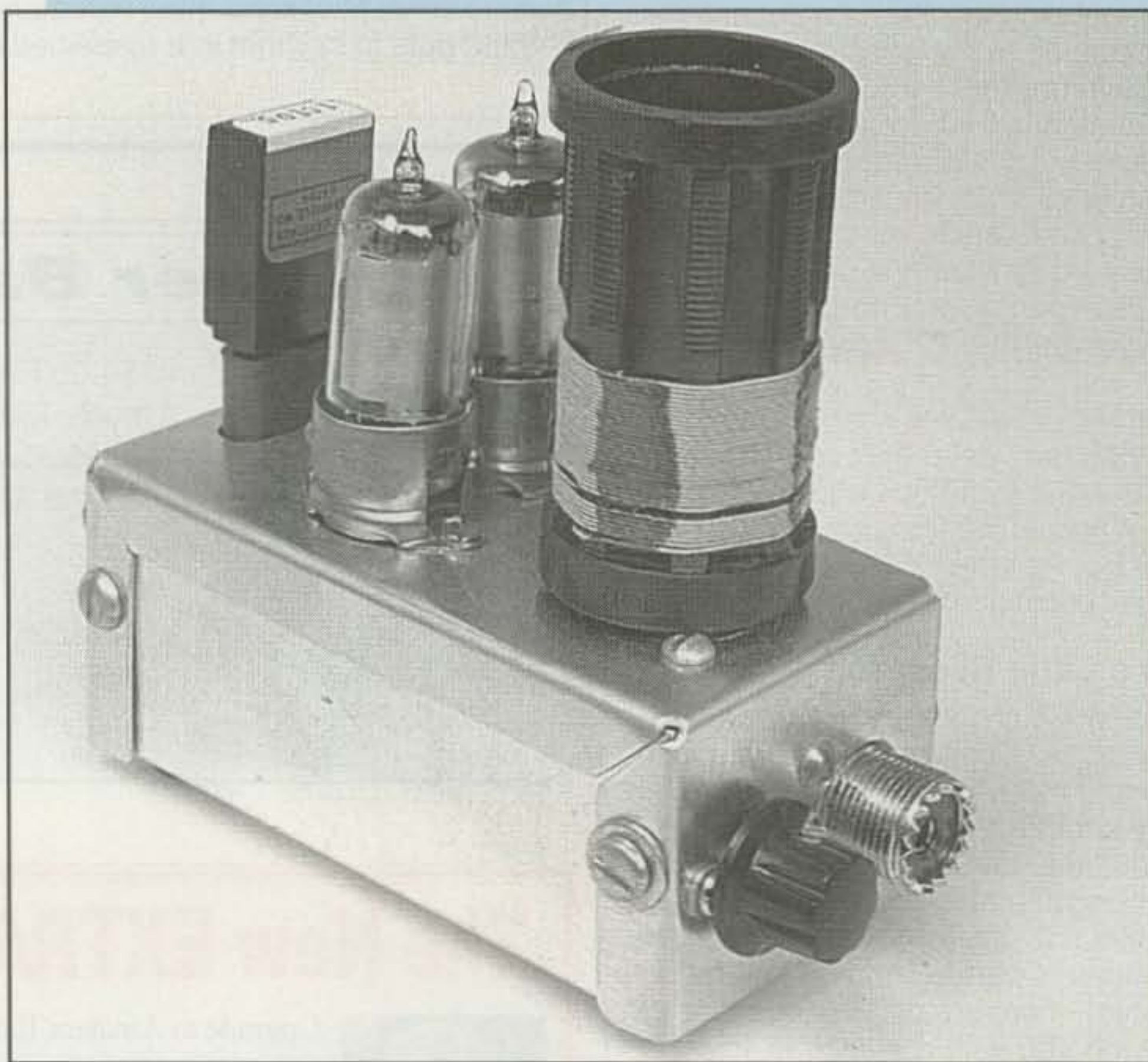
Photo A—Incredible beauty, warmth, and charm best describe this 1950s-style 1S4 transmitter. It can be configured for 80, 40, or 30 meter operation and powered by batteries or a small AC supply. It makes a great "occasional" QRP rig.
