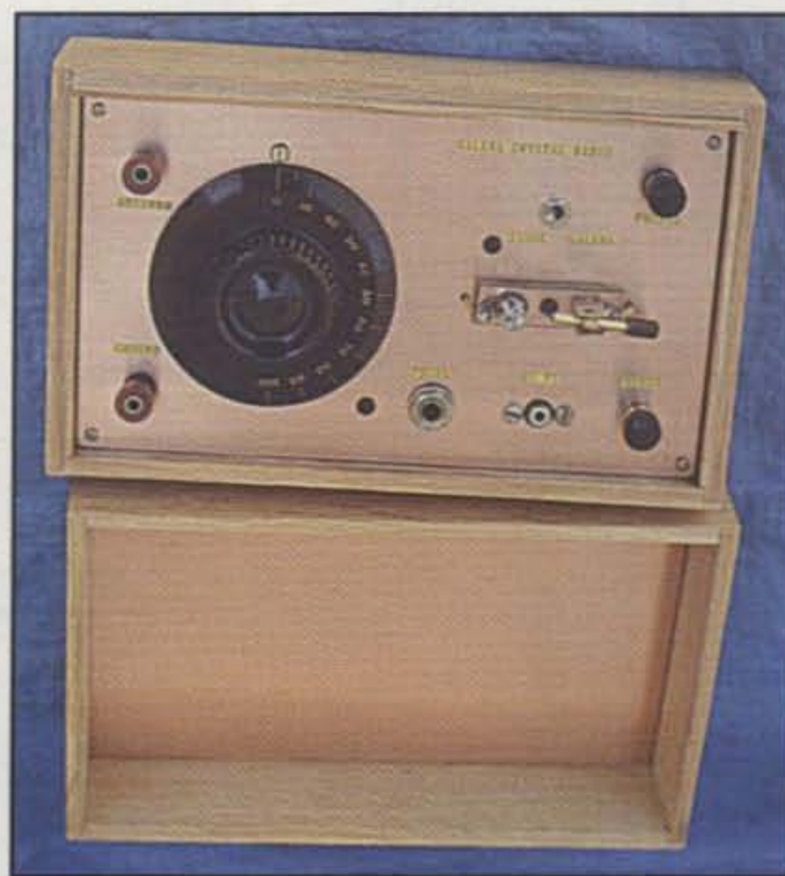
Photo B— Trim, clean crystal set homebrewed by Leonard Gardner, W2QBC. Receiver sports a genuine National "Velvet Vernier" dial, catwhisker-and-galena detector, plus gold lettering on lacquered copper panel set in a white oak case. Nice! (Photo by W2QBC)
