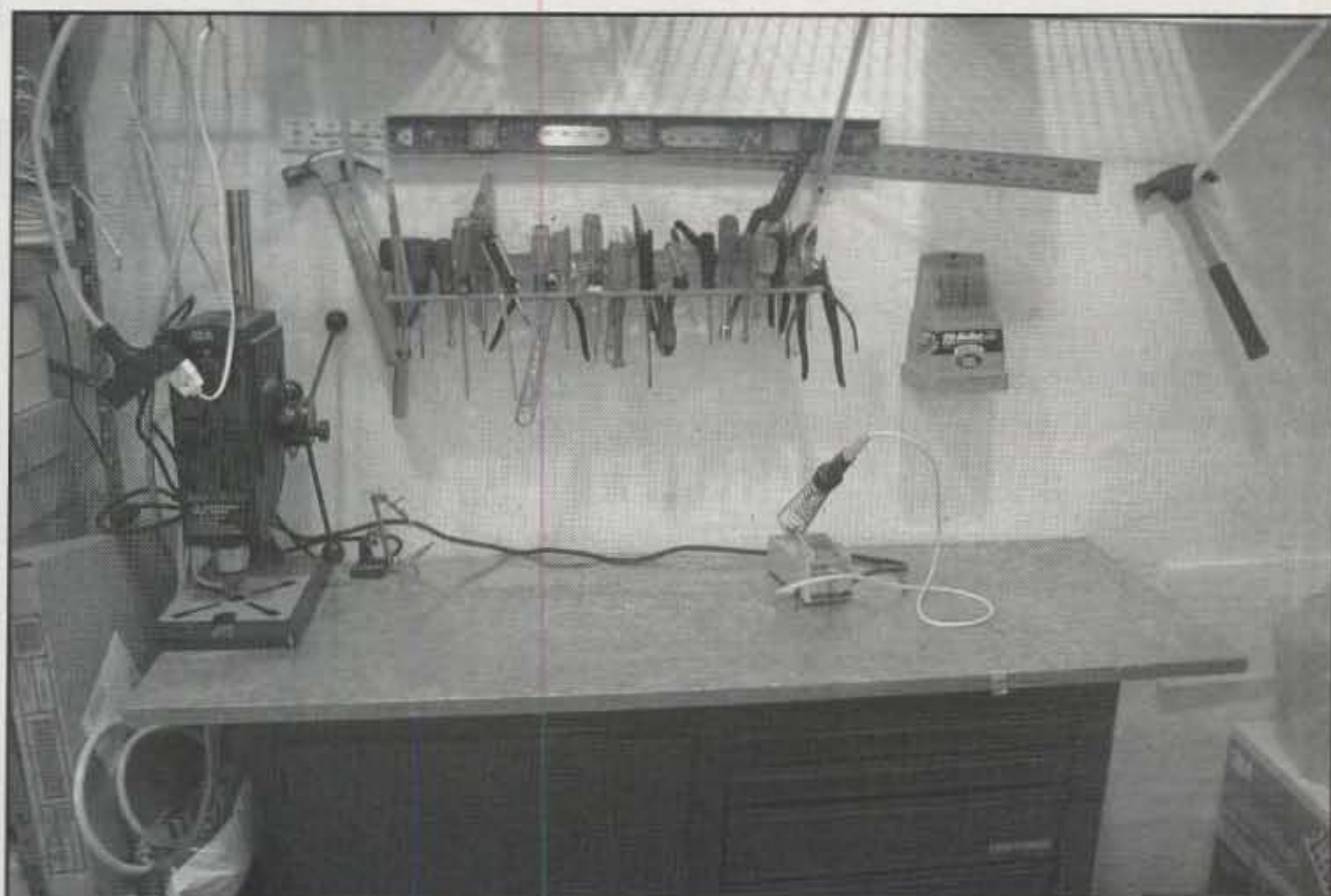
Here is the workbench and the tool rack. The soldering iron is a permanent resident at the top because it is used more than any other tool. The drill press is not used that often, but it is too tall to fit on the shelf above the bench, so it is pushed out of the way in the back corner.
