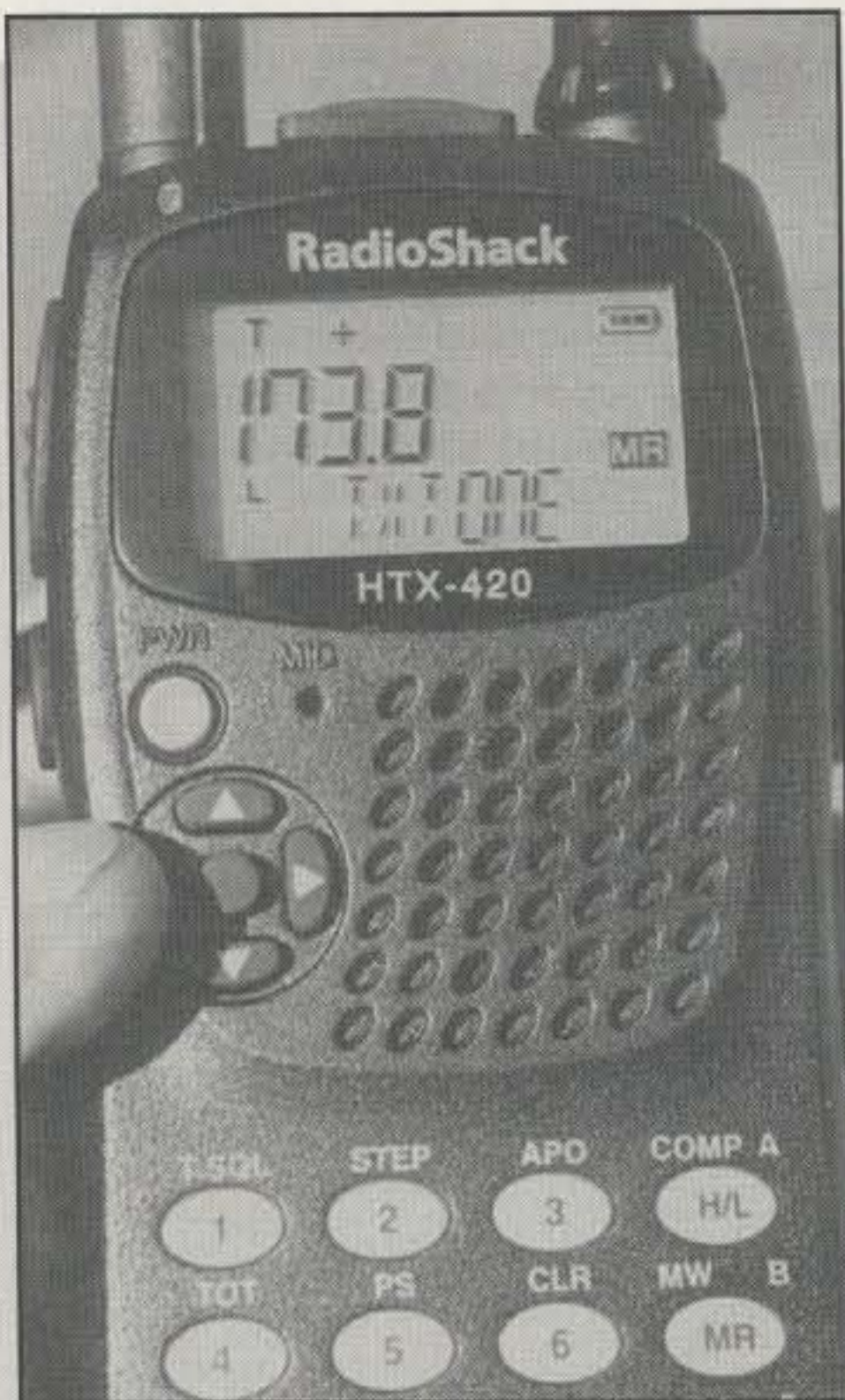
Setting CTCSS tones on the HTX-420 is easy, and the display lets you know if you are setting a transmit (TX) or receive (RX) tone.
