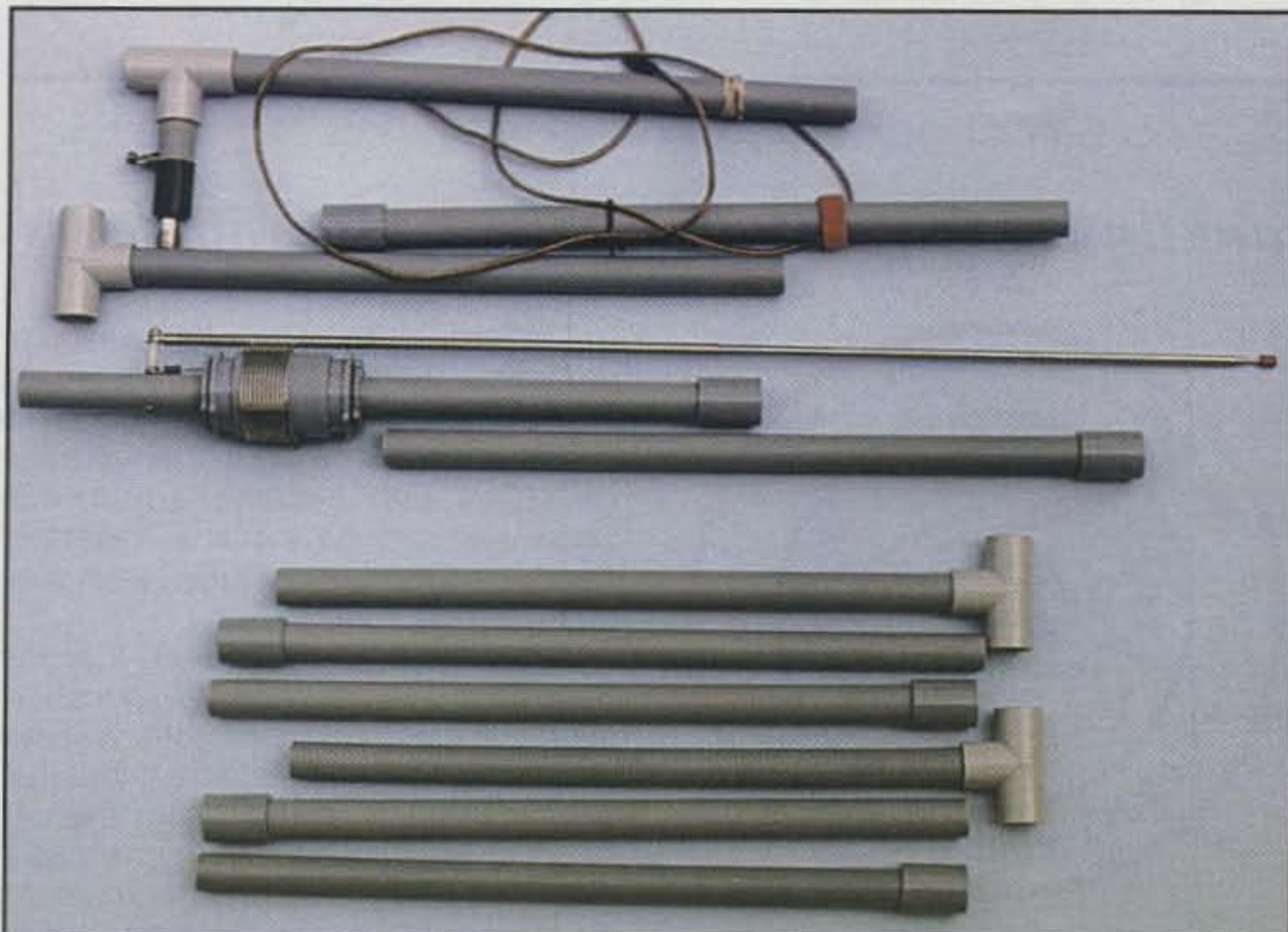
Photo G— The new MinuteMan antenna from John Bee, N1GNV, and Quicksilver Radio Products is a slip-together portable vertical antenna for 20, 17, 15, 12, and 10 meter operation. Here you see it laid out and ready for field assembly, which takes only a couple of minutes.
