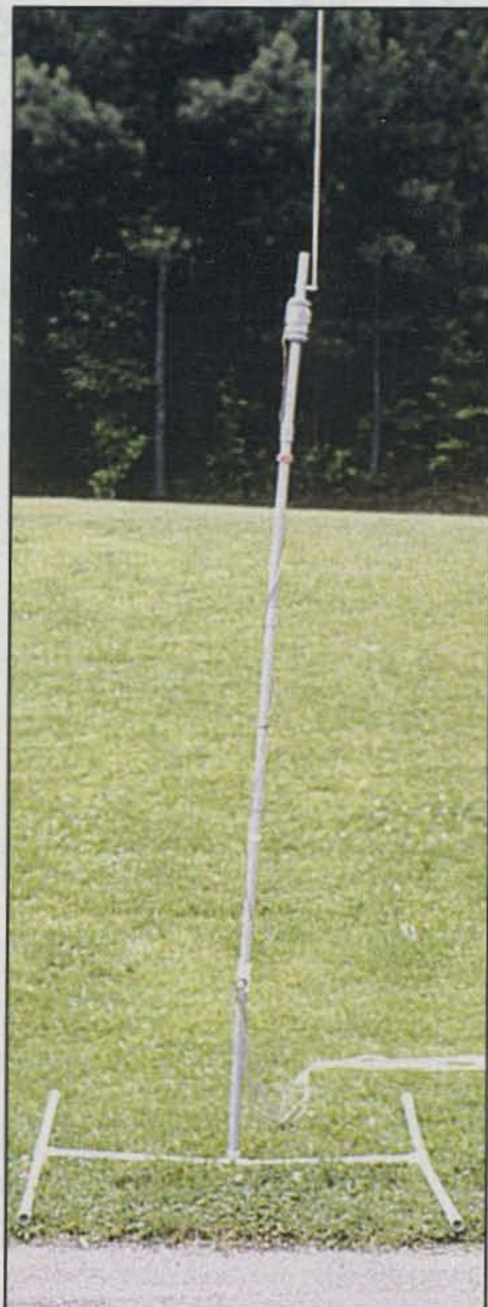
Photo H— The new MinuteMan 20 antenna assembled and ready for operation on its self-supporting base. Counterpoise wires and coax cables connect to the antenna two feet up from the base.
