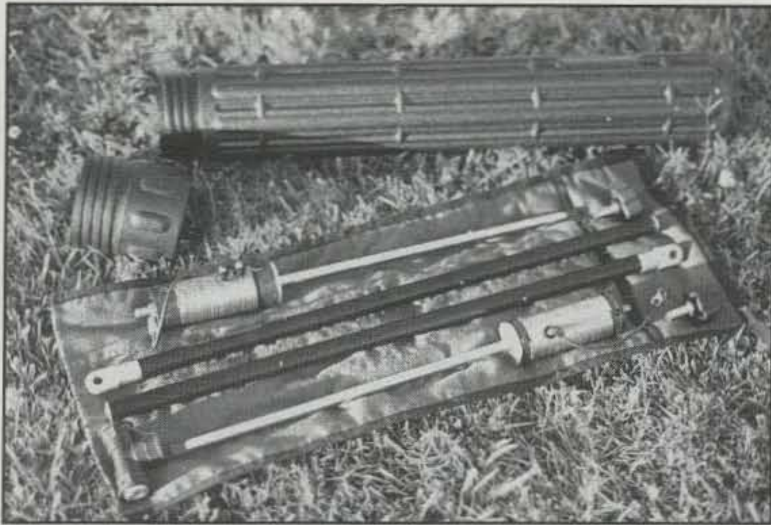
Photo F— The snap-together, multiband W3FF Buddipole antenna laid out and ready for quick field assembly. All sections store neatly in a roll-up bag, which slips into the 24 inch container at the top of the photo.
