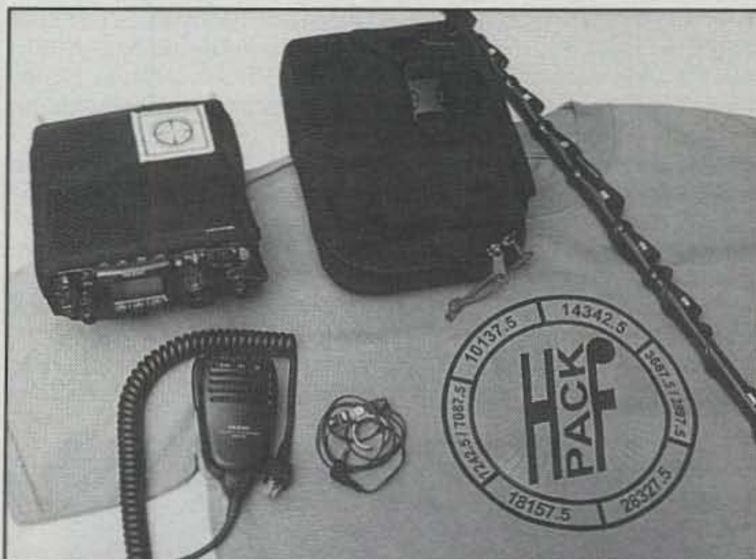
Photo D— What do you need for operating HF Pack? As shown here, the main requirements are a mini transceiver such as the FT-817, a carrying case or bag, an easy-to-carry antenna, mic, key, and short coax cable. An HF Pack T-shirt is optional, but has a noticeable advantage (see above).
