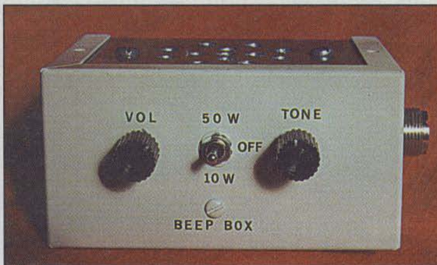
Photo A— The stand-alone Beep Box with volume and tone controls, built into a 2" x 3" x 4" minibox.
