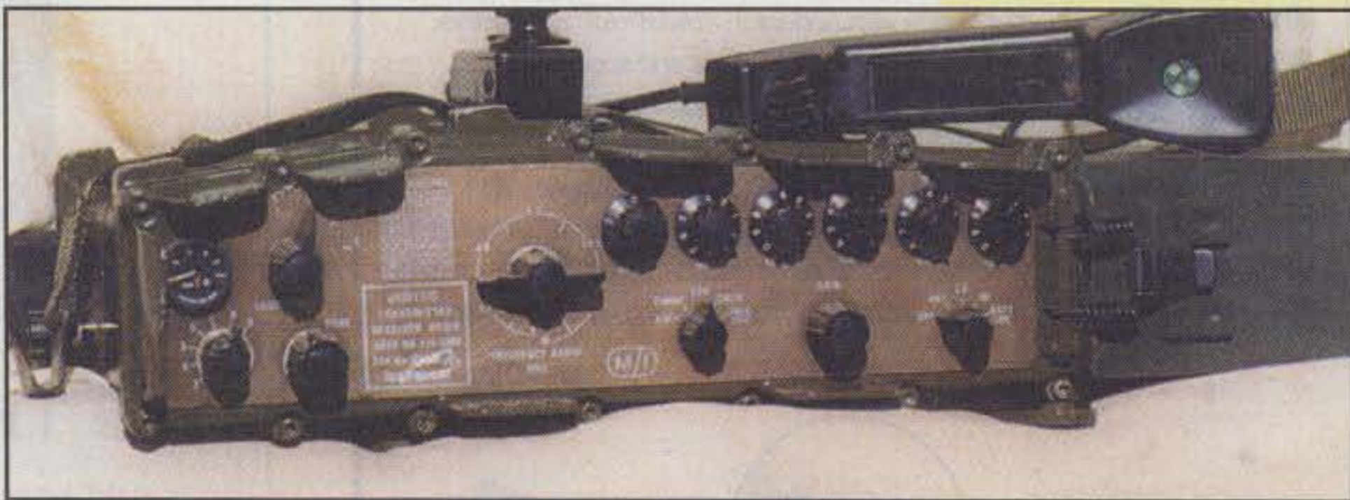
Photo B—The PRC320 HF manpack transceiver with handset and key. Battery attachment is on the right. The antenna would plug into the left-hand edge.
