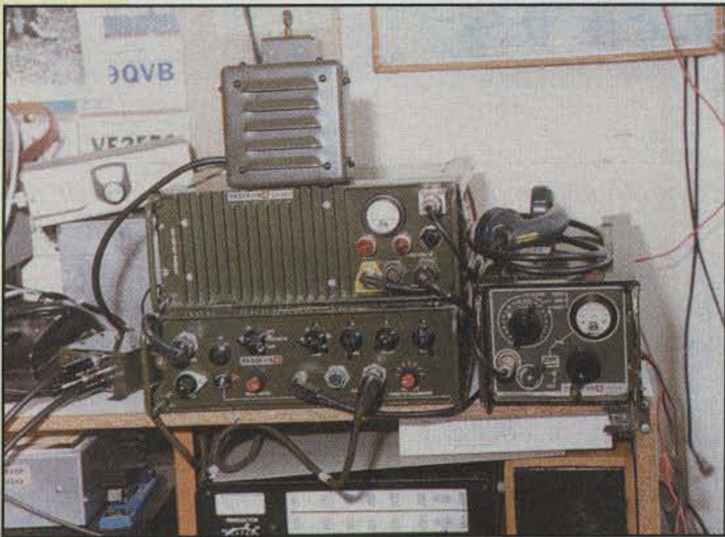
Photo D— The Redifon GR-345 with the GA-480 amplifier and ACU9 ATU in use in the author's shack.
