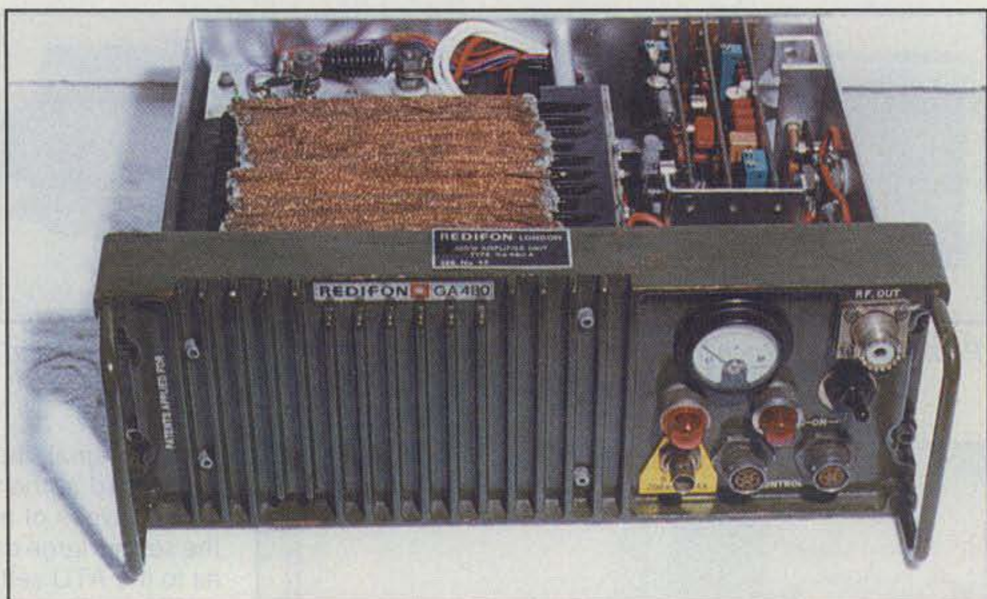
Photo E— The inside of the GA-480 amplifier showing the large heatsink (left) and driver and control boards.
