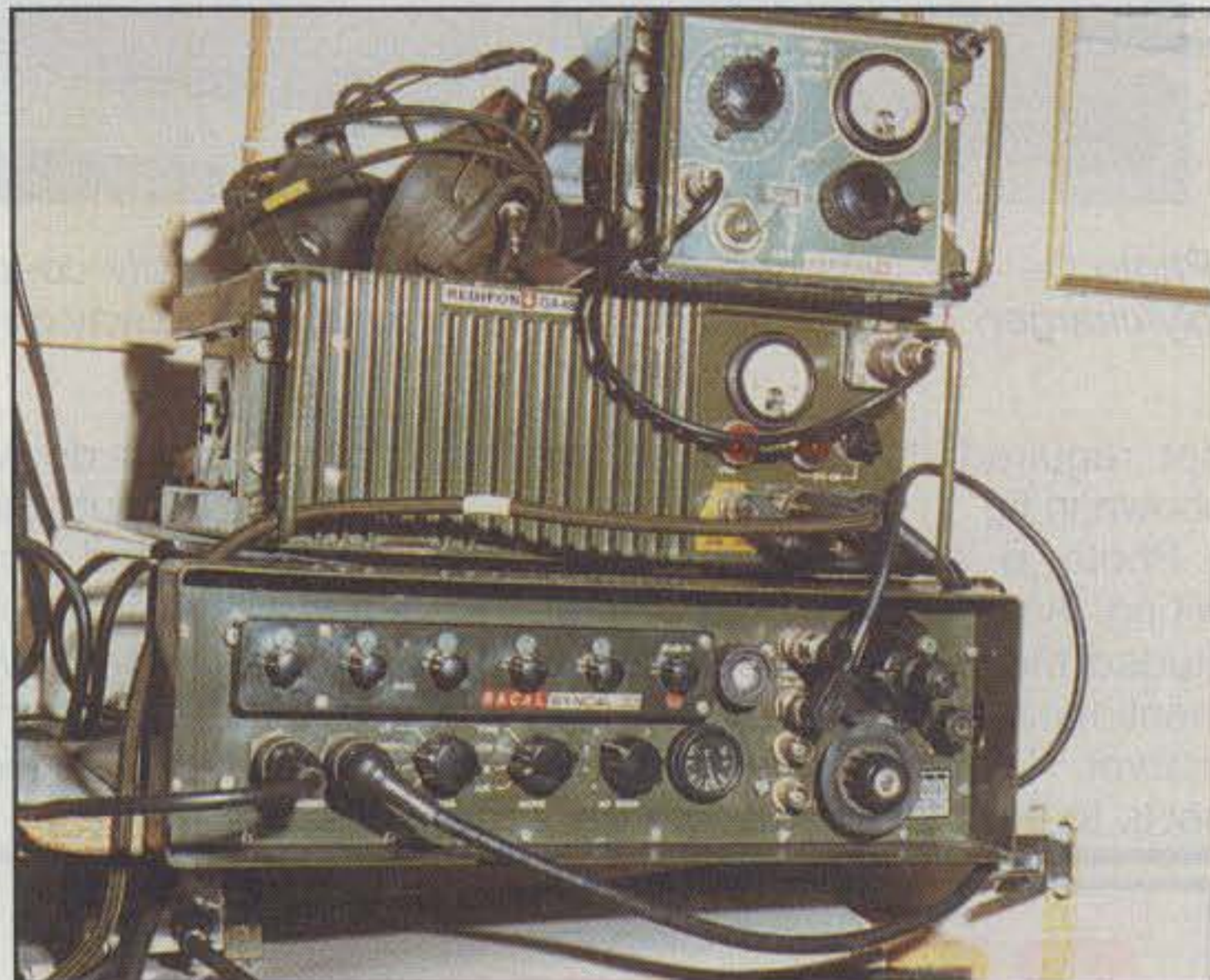
Photo A—The Racal Syncal 30 in use with the GA480 amplifier and ACU9 antenna-tuning unit.
