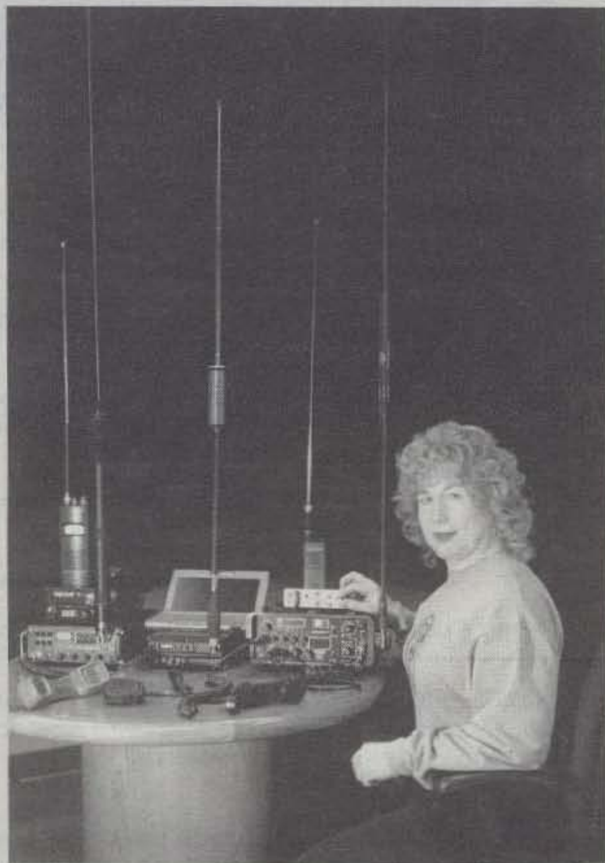
HF Pack founder Bonnie Crystal, KQ6XA, with her cool collection of backpack/HF Pack SSB transceivers. Units are (left to right) FT-817 with homebrewed docking booster; Tokyo Hi-Power HT-750 handheld for 40, 15, and 6 meters; Yaesu FT-70G; Vertex VX-1200 with laptop on top; and Kachina MP-25 with Mizuho MX-7S handheld on top. (Photo by Jessica Stevens, KF6WMMY)
