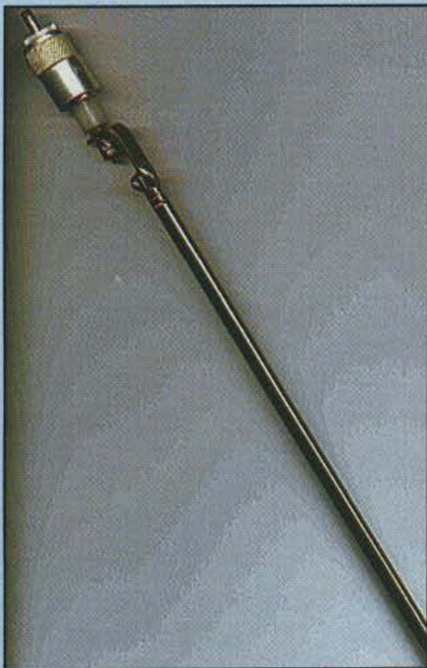
Photo C— A 6 foot whip made from a telescoping antenna goes on top of the coil. You may adjust the size of this whip as needed for a good match on your selected band.
