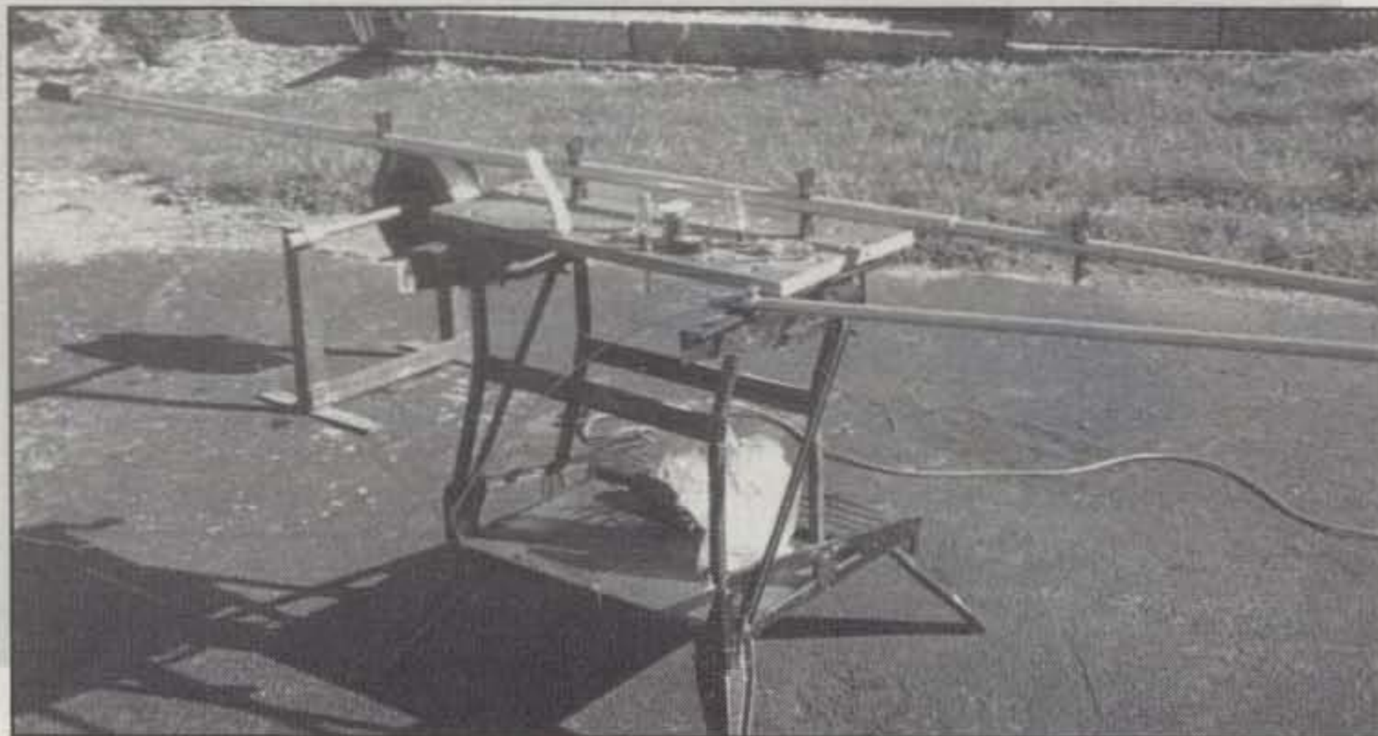
Photo D— Wire protruding from tip used to pull Poly rope through element.
