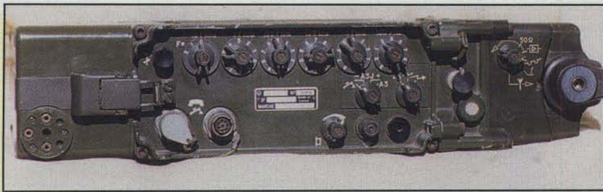
Photo C— The French TRC300 manpack transceiver with battery on the left and automatic ATU on the right.
