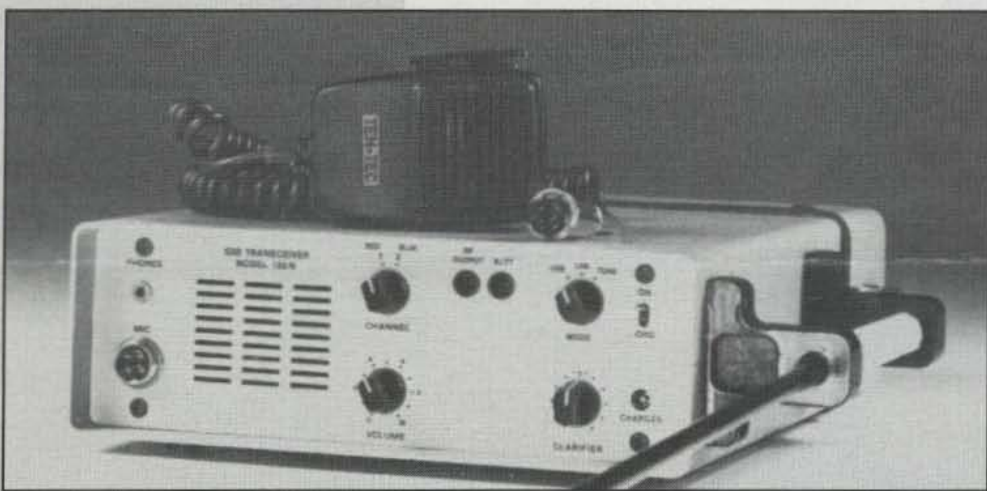
Photo 4— Little known Ten-Tec model 120 manpack HF transceiver produced during the 1980s. Although challenging to find today, the rig could prove a unique and fun item for use HF Pack'n. (Photo courtesy Ten-Tec)
