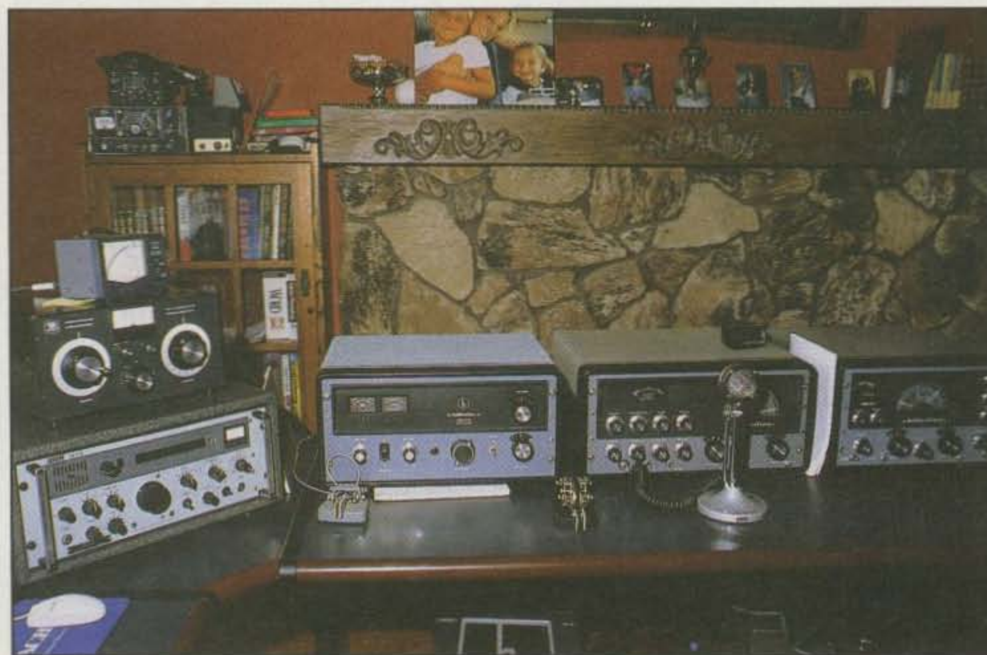
Joe's main living-room operating position including (from left) a Viking tuner atop a Racal RA-1772 shortwave receiver and a complete Hallicrafters station — an HA-33 linear amplifier, HT-32 transmitter, and SX-115 receiver.
