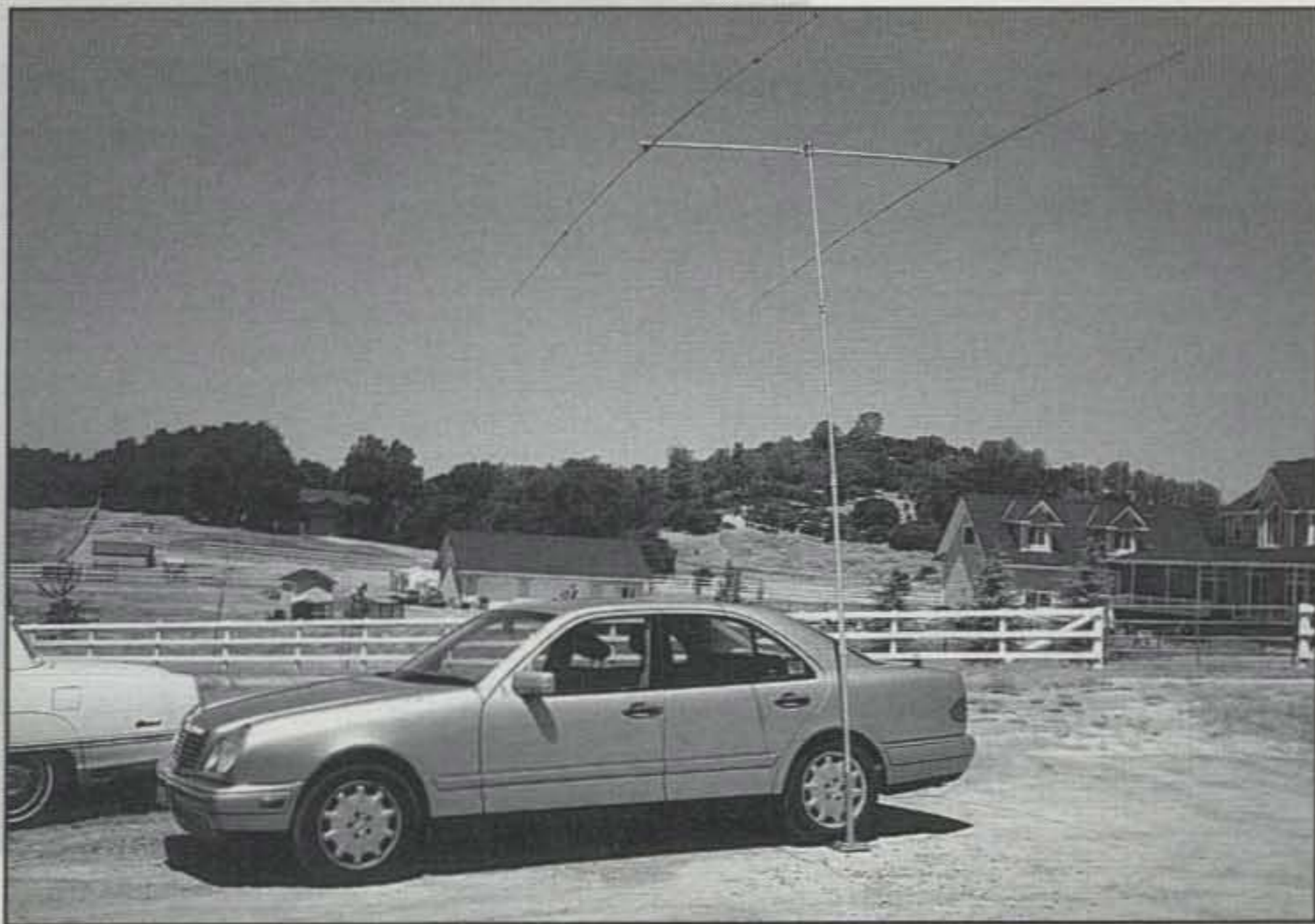
Photo 7— Within five minutes Vern, W6MMA, has assembled the minibeam, set it up for working 20 meters, and secured its mast to a drive-on mount. First class!
