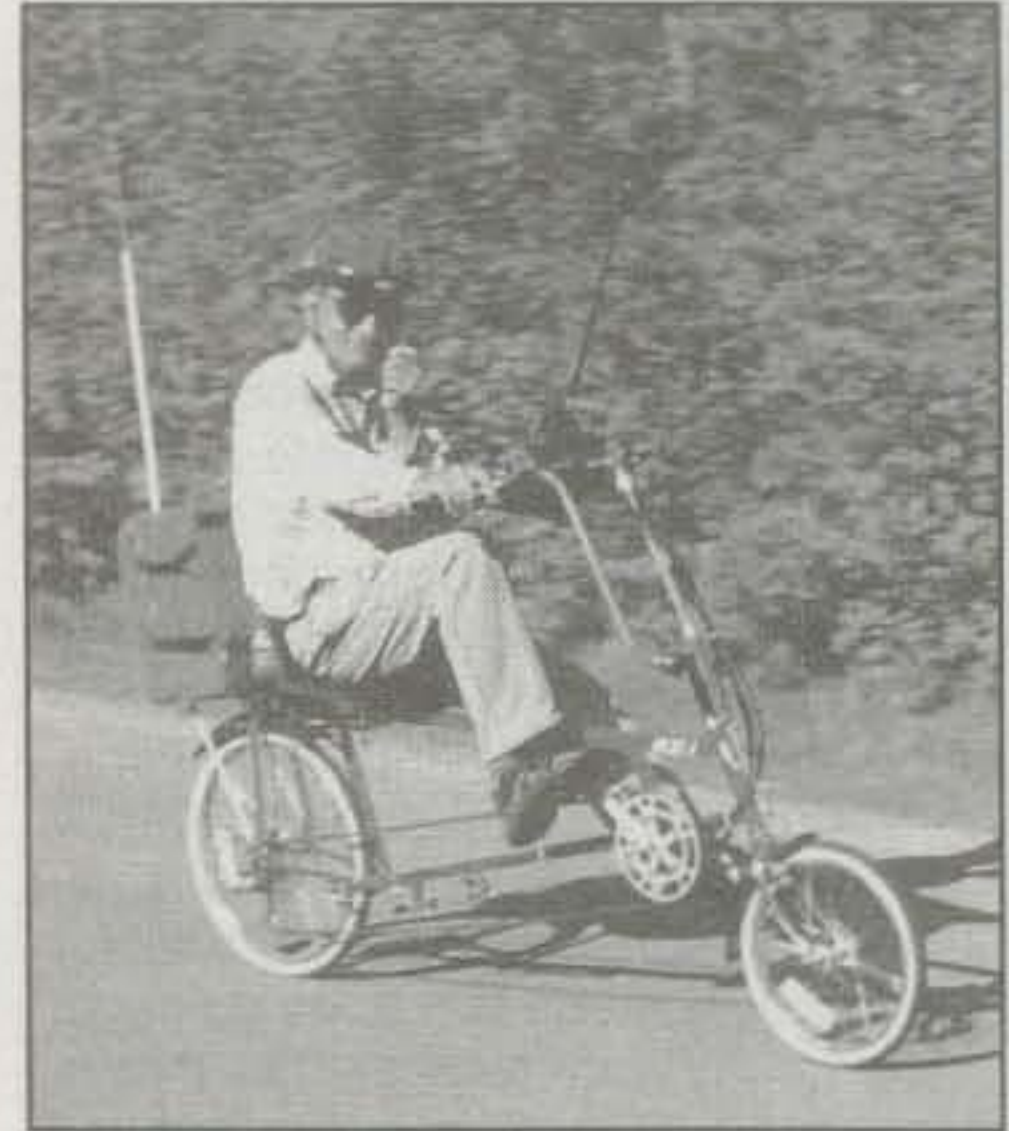
Photo 1—Mohan, VE7FM, checks in with the HF Pack group on 18.157.5 MHz while mobilizing on his “Easy Racer” recumbent bicycle. Setup consists of handlebar-mounted QRP Plus transceiver, dual-band FM talkie, GPS receiver, plus homebrew antenna and gel-cell battery. Now that's biking in style! (Photo courtesy VE7FM)
