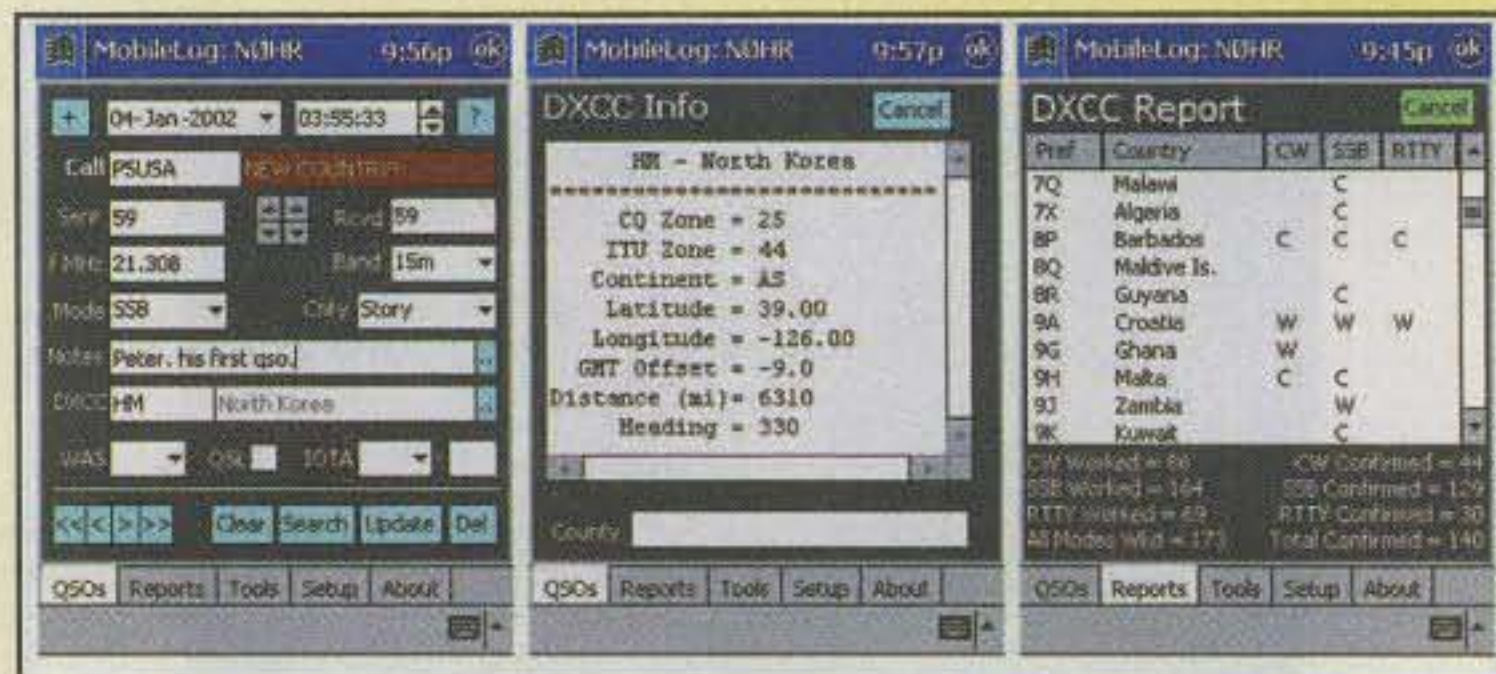
Fig. 1—Do you need a low-cost, low-power, low-weight alternative to laptop logging in the field? If you own a PocketPC, NØHR's MobileLog puts the power of a desktop logging application into the palm of your hand. You can track DXCC award status by band or mode, calculate approximate beam headings and distance to DX stations, easily search for previous QSOs, and much more. (W8FX screen capture from the NØHR website)
