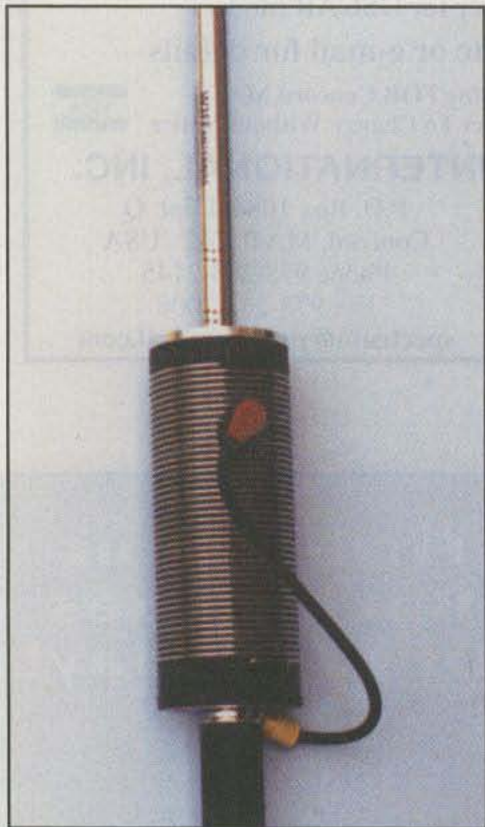
Photo B— This new "Buddipole" portable multiband dipole utilizes longer elements and fewer turns of coil wire, resulting in higher efficiency and improved performance. (Discussion in text.)
