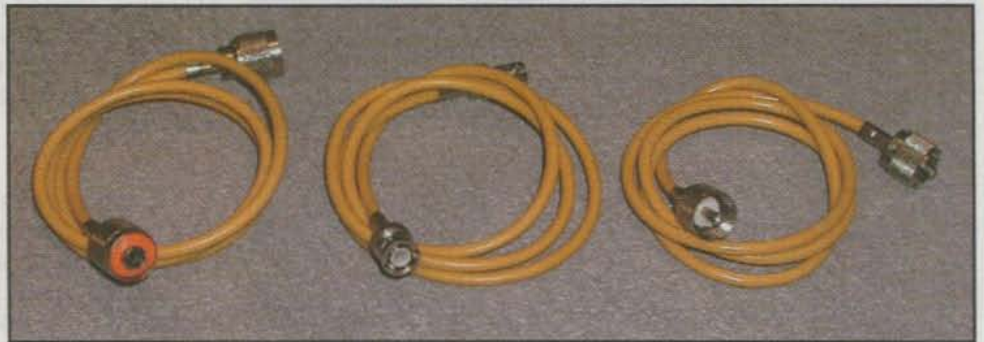
Three popular coax connectors (left to right): Type N, BNC, and "UHF." The first two are somewhat weather resistant, while the ubiquitous UHF connector is as worthless at keeping moisture out as it is at keeping impedance constant.
