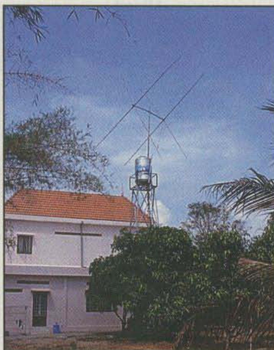
W9XK/3W2XK's homebrew tri-band quad. He says the bamboo spreaders were readily available and have survived quite well.
