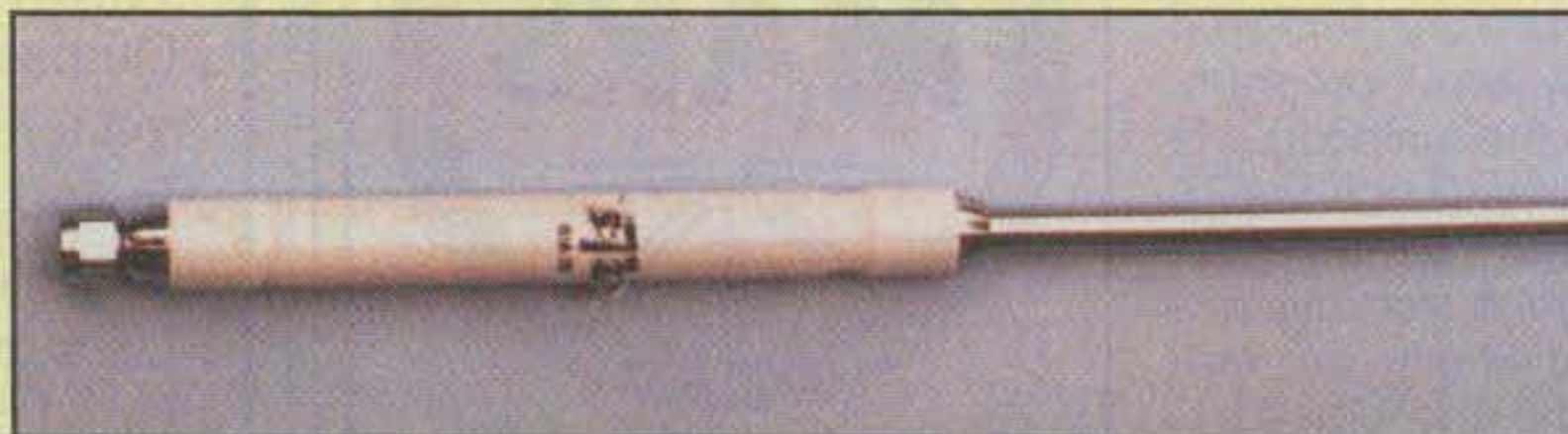
Photo A— Loading coils such as those employed in Hustler resonators are often used to reduce an antenna's physical size. The more turns of wire in the coil, the smaller the antenna element, but signal capture/radiation area and the efficiency are also reduced.
