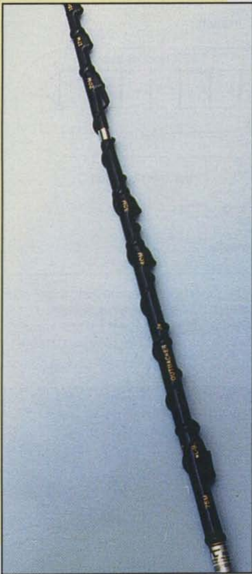
Photo D—Although not visible beneath its glossy outer cover, the popular Outbacker mobile antenna employs a helical winding as both a radiating element and a “stretched coil” for multi-band loading. Winding on lower shaft area is basically a jumper for selecting bands. (See text.)
