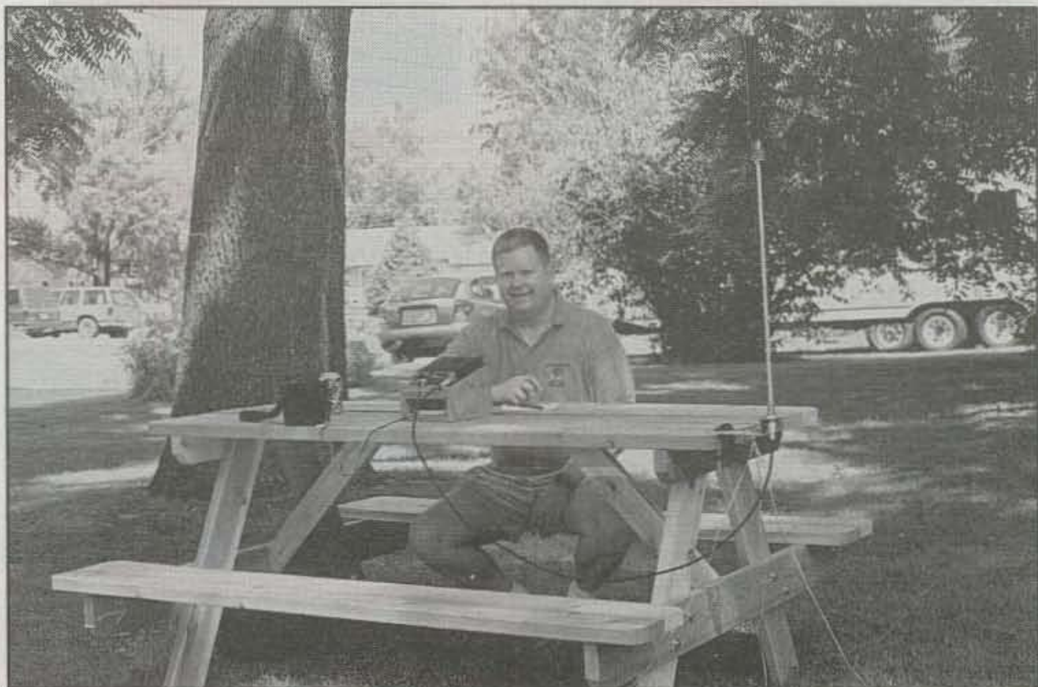
Photo 2—Mike Melland, W9WIS, enjoys camping on weekends and often calls into the HF Pack 17 and 20 meter meets while operating “Picnic Table Portable.” His gear consists of an FT-817, 7 amp battery, and W6MMA break-down MP-1 vertical with counterpoise and table-edge clamp. (Photo courtesy W9WIS)
