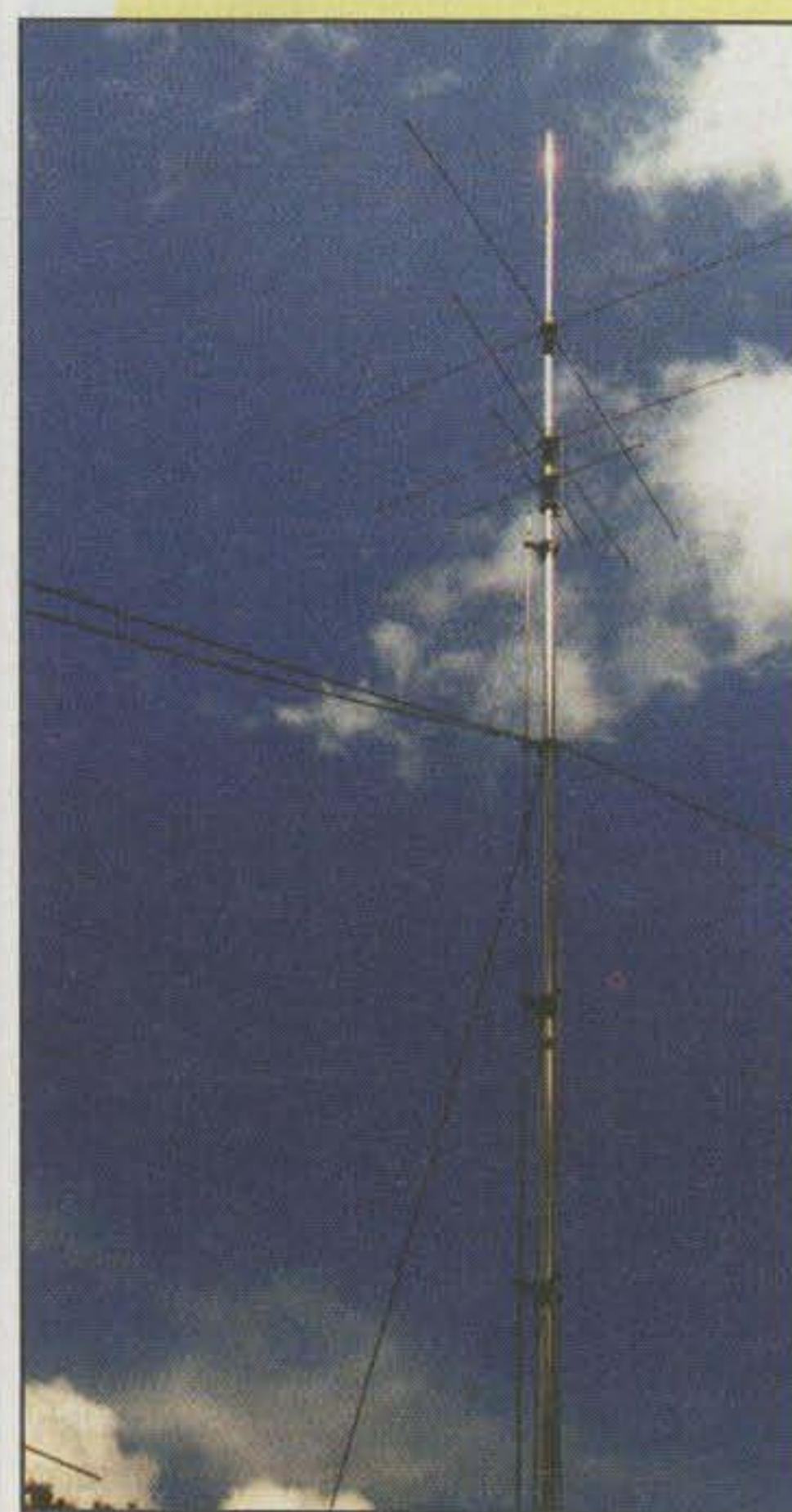
Photo E—Capacity hats such as employed on this Hy-Gain AV-640 3/8 -wave vertical are quite effective for extending an antenna's electrical height while keeping its physical height within a reasonable limit. Notice these capacity hats are used in conjunction with loading coils and are also larger rather than smaller near the top. That is because they are connected in parallel rather than in series. (Discussion in text.)
