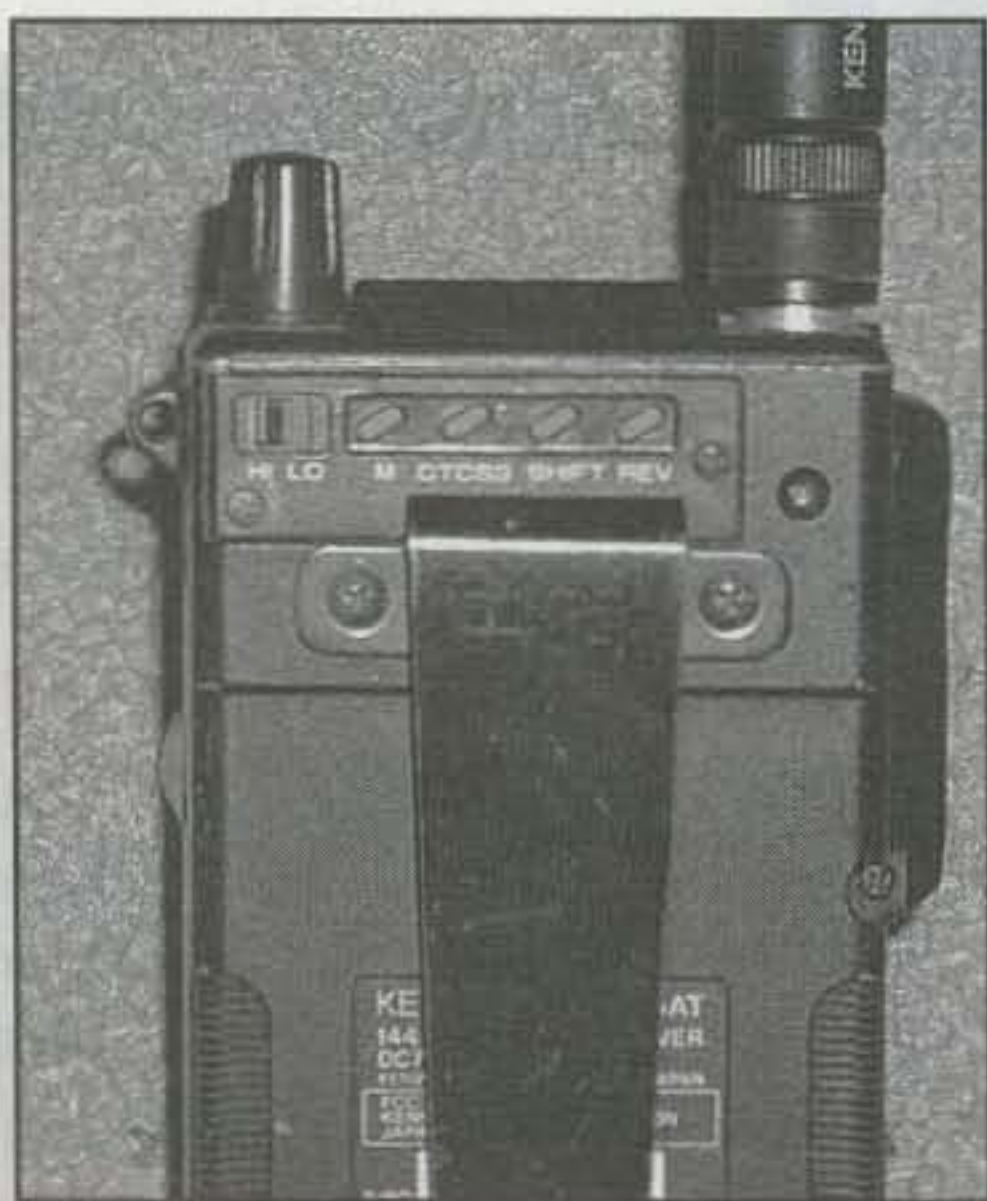
On this older rig (Kenwood TH25) the reverse switch is one of several switches located on the back of the radio above the belt clip. The reverse switch is at the far right.
