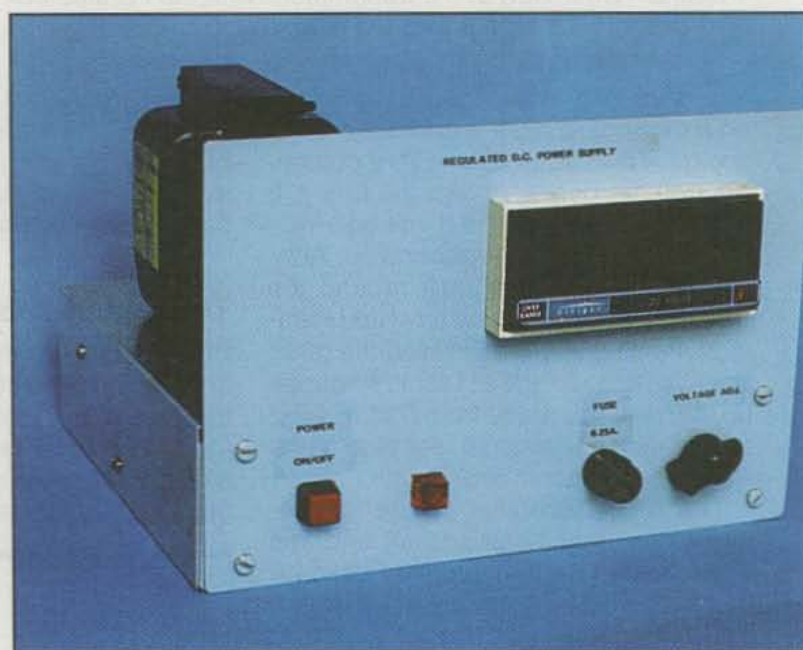
Photo A— Front view of the power supply. Controls are simple, with an on/off switch on the left and a voltage adjustment control on the lower right. The output voltage reads out on the LED display on the upper right.
