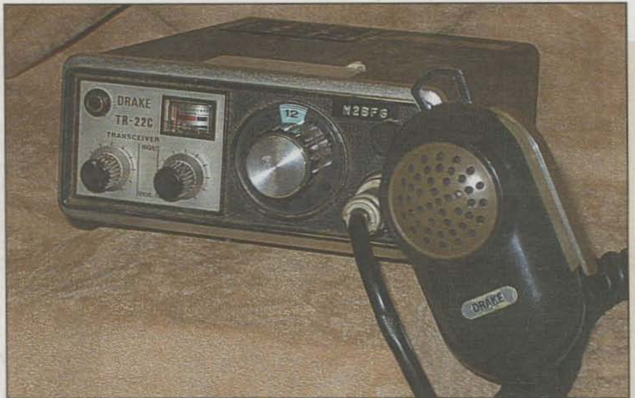
The 1970s-vintage Drake TR-22 was an early "handheld" 2 meter FM rig, with either 6 or 12 crystal-controlled channels (the TR-22C pictured here has 12) and one watt of RF out. A telescoping whip pulled out of the front, or you could plug in an external antenna in the rear. A case and shoulder strap made it portable. (Photo courtesy W2VU)
