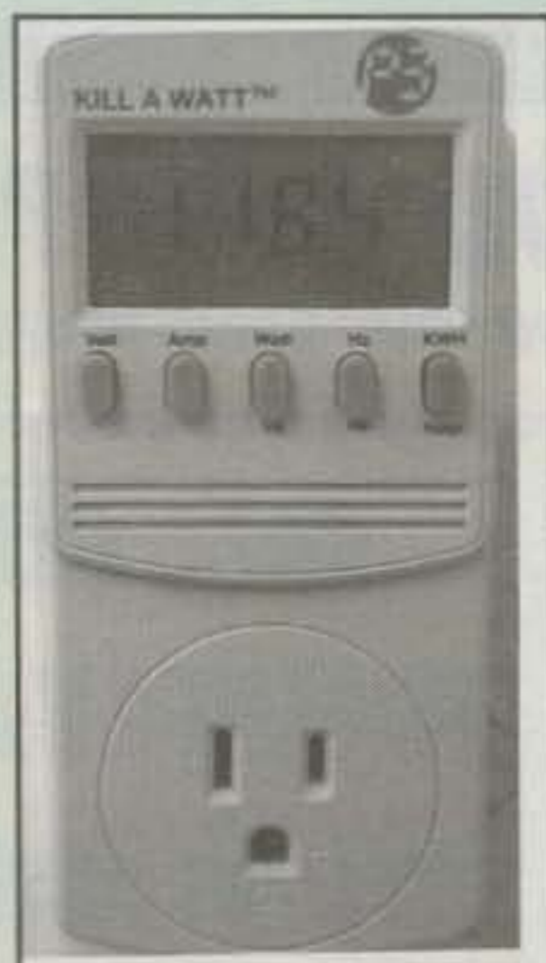
Photo 10— Have you ever wondered how much current your rig draws, how many watts your microwave oven uses, or how many kilowatt hours your energy-saving refrigerator really uses in a week or a month? This "Kill-A-Watt" meter from Radio City can reveal the answers. (Photo via Radio City)
