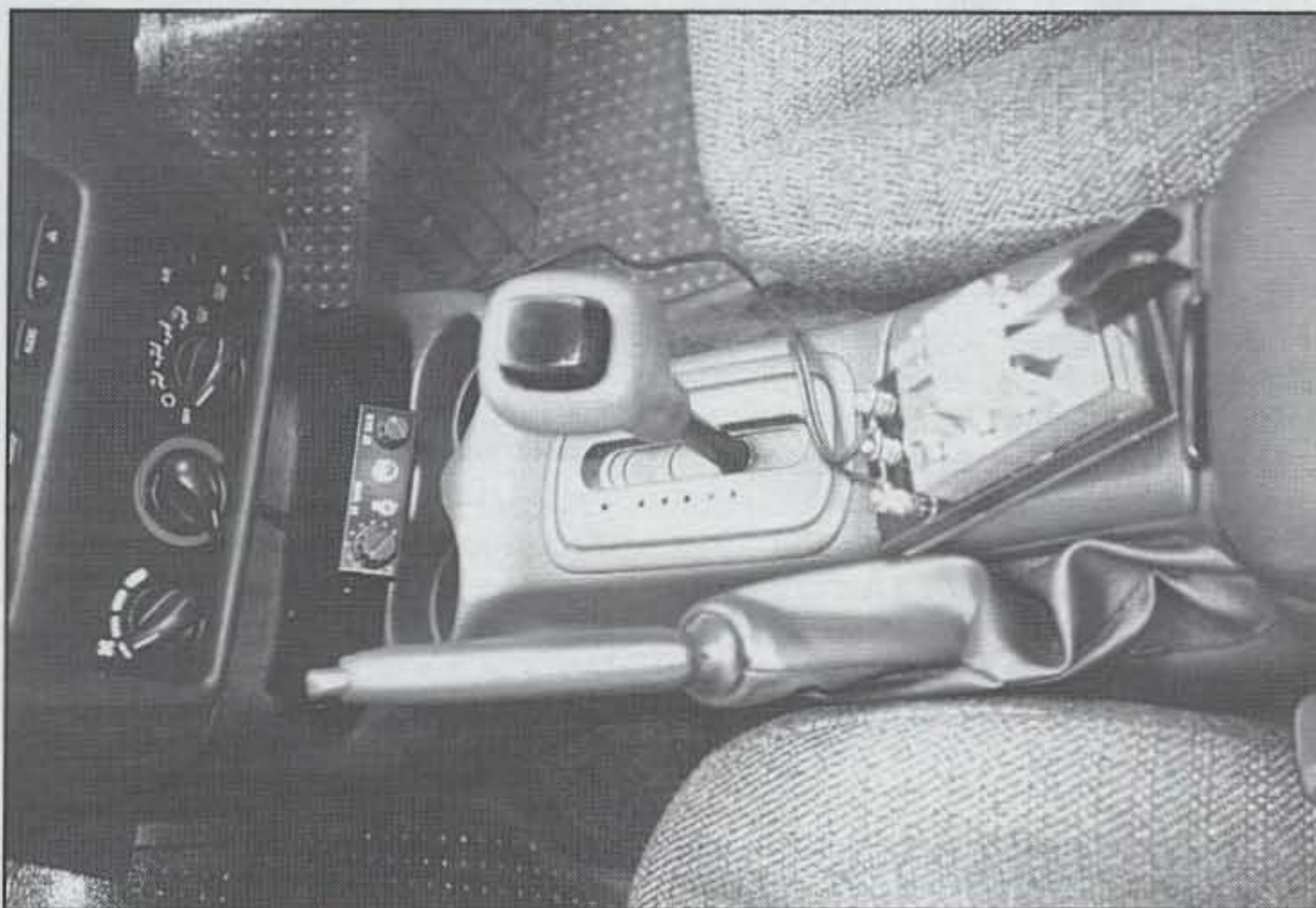
Photo A— Mobiling need not be elaborate or expensive to be fun, especially with QRP. Here a homebrewed 4 watt 30 meter transceiver (NorCal's famed "38 Special") and new K6VDH paddle (described in our March 2002 "World of Ideas" column) plus headrest-strapped speaker give WB4OEE's Cavalier a touch of real radio clout.
