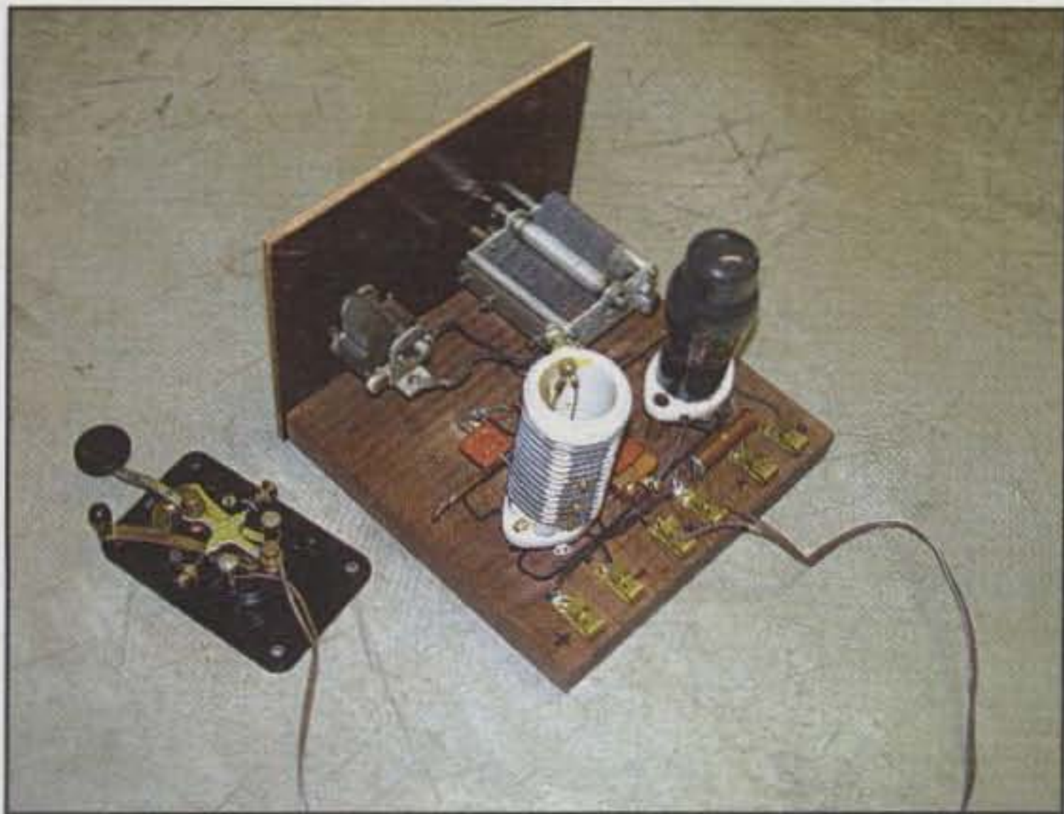
Photo B—Rear view of the transmitter. Note the Fahnestock clips for added realism.
