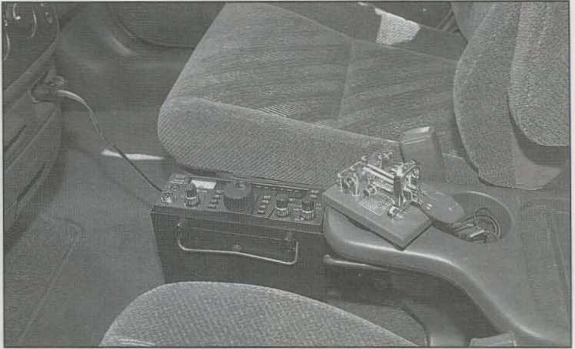
Photo D— First-class QRP mobile for sure! You are looking at the brand-new Ten-Tec Argonaut V mounted between the cockpit seats of Larry, WA4BSM's Honda minivan, and it is a romper! Like its predecessors, this heartwarming (and quite deluxe!) transceiver is destined to become a classic collectible. Notice the paddle, too; it is the prototype of a special Vibroplex/Ten-Tec dual-labeled iambic paddle that is being produced in limited quantity and available right now from Ten-Tec.
