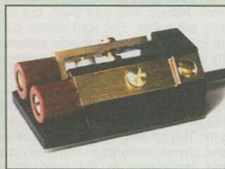
Photo 2— Here is the new "Squeeky" miniature paddle from DK1WE. Its dual levers are mounted at 45-degree angles for more comfortable use, and each lever is independently adjustable. The frame is anodized aluminum with a flat base, and the whole paddle is small enough to carry in your pocket. This handmade paddle is available from DK1WE in Germany. (Photo via DK1WE)
