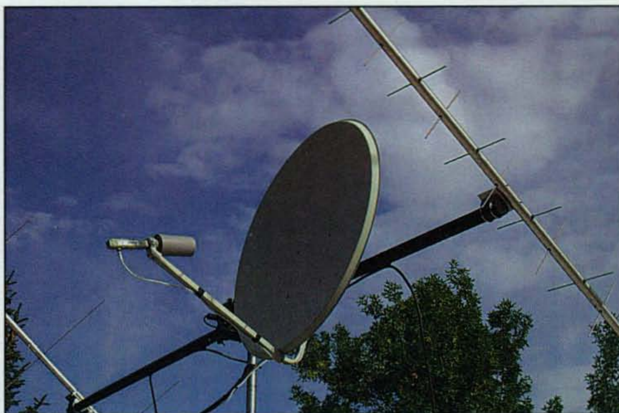
Photo F— The N3IYR S Band Antenna is produced for AO-40 work, but it can be used for any satellite or point-to-point work in the 2.4 to 2.5 GHz range. The water-proof antenna produces 25 dBi circular gain. (Photo courtesy N3IYR Antennas)
