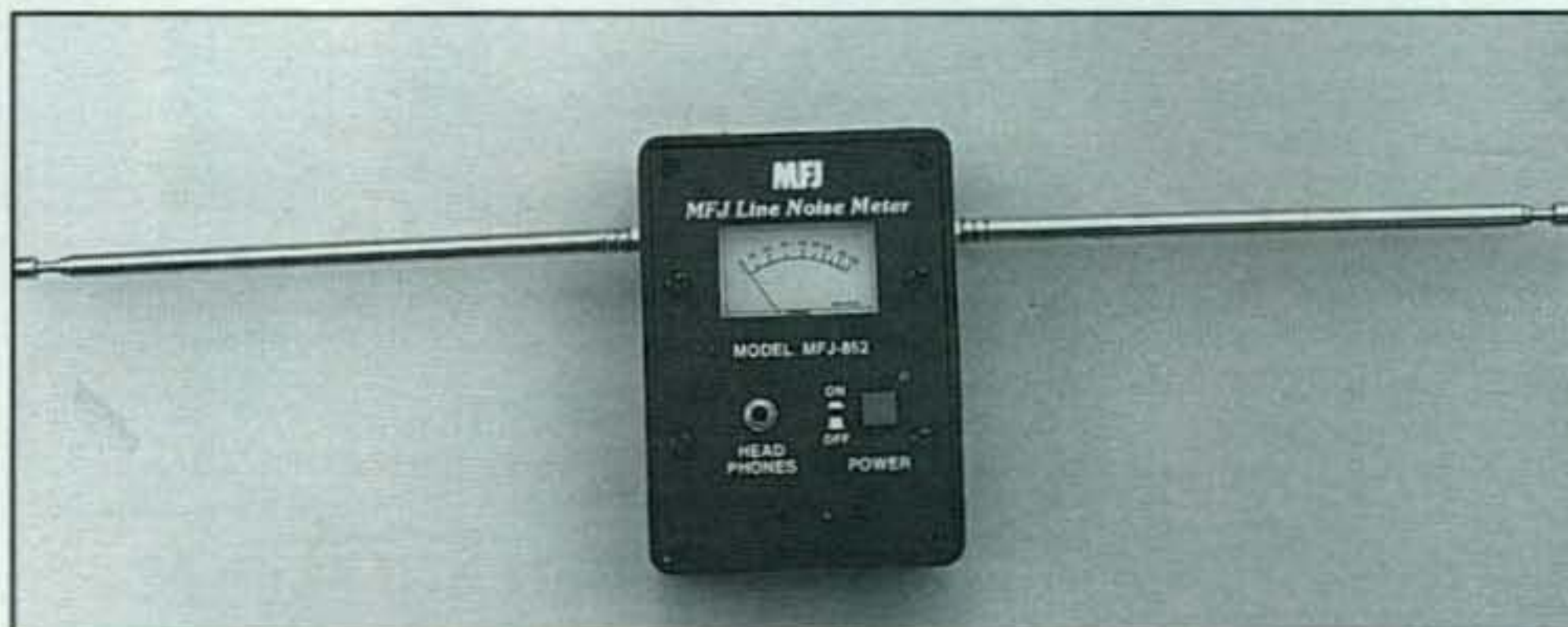
Photo C— Tracking down sources of power-line noise can prove quite a challenge. The MFJ-852 Line Noise Meter, however, cuts the pursuit down to size. The self-contained unit has a very directive antenna, level meter, and headphone socket for simultaneously monitoring noise. (Discussion in text.)
