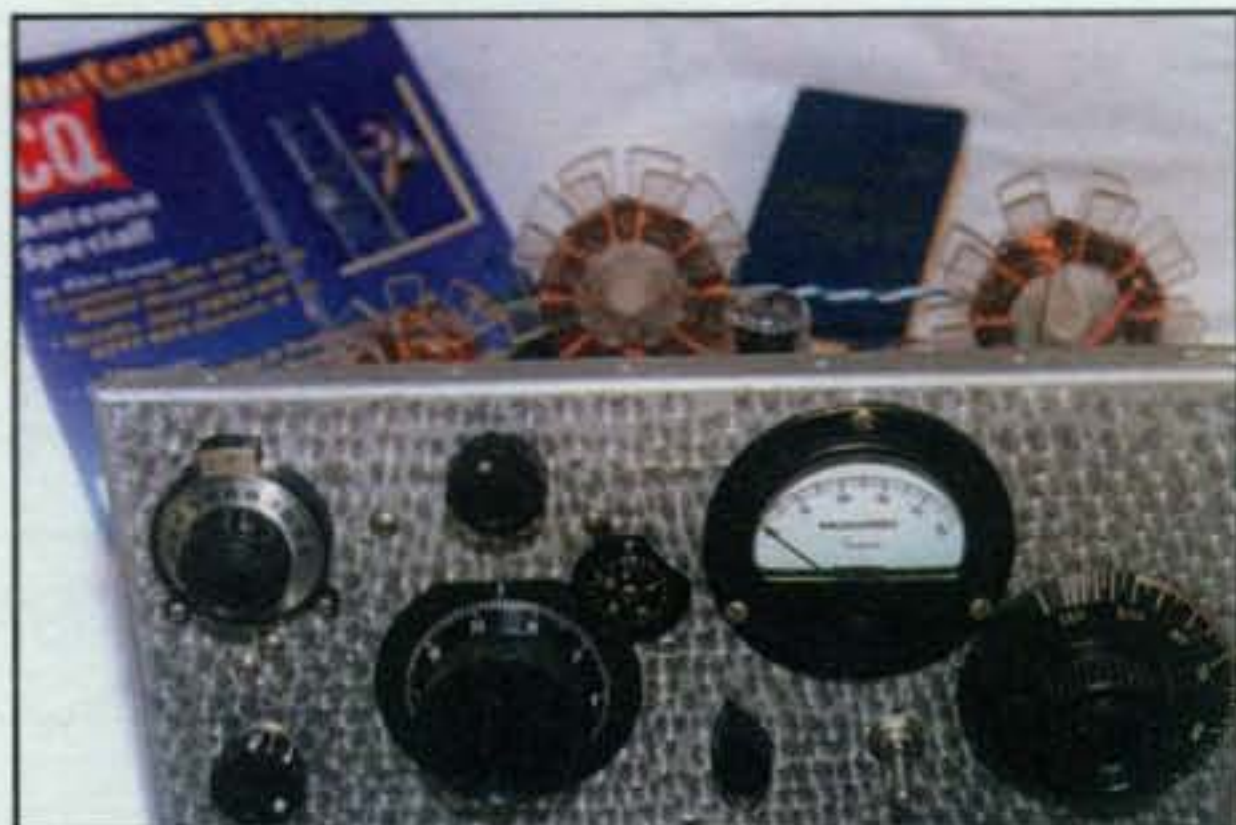
Photo A—Front view of the two-tube trans-receiver with spider-web coils built by Peter Demmer, KH6CTQ. The unit consists of a regenerative receiver and a 5 watt transmitter for 40 meters, and can be homebrewed as is or modified/expanded according to personal preference and creativity. (Photo courtesy KH6CTQ)
