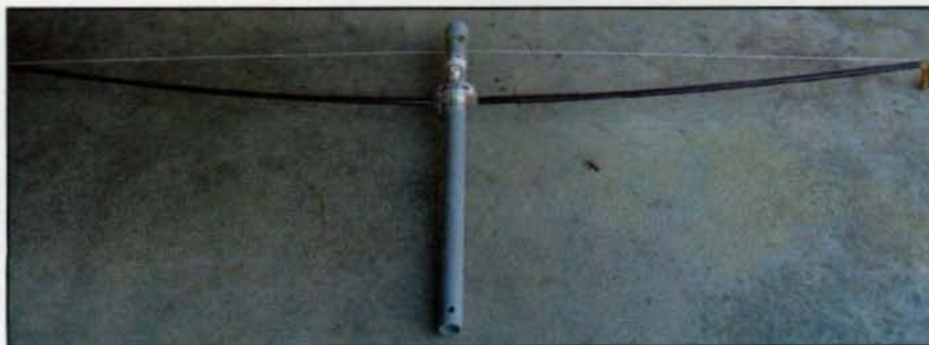
Photo 2— The Hex Beam showing the bowed spreaders installed.
