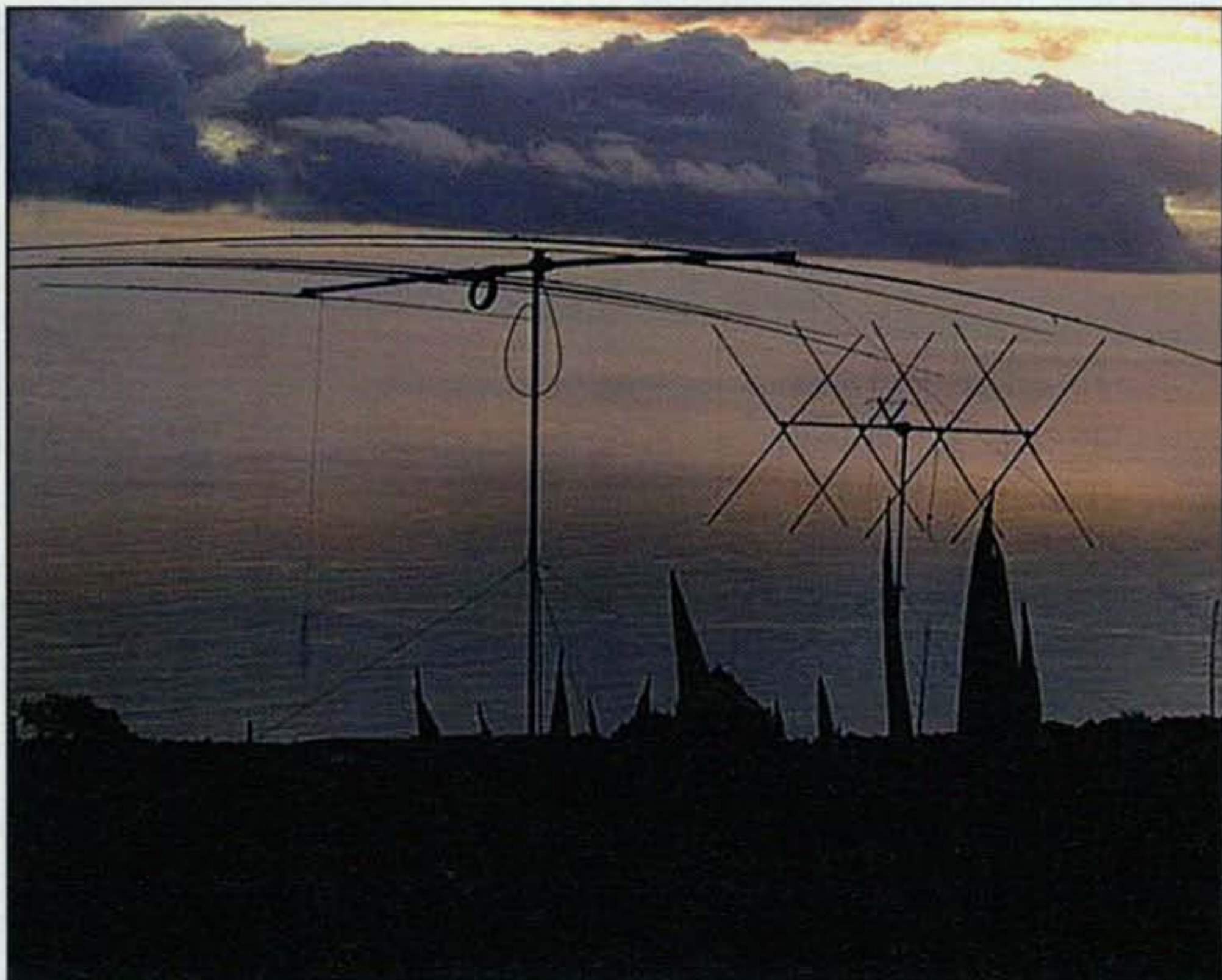
These are the two 10 meter antennas used by D44AC. They were phased, and in this photo both are pointing toward Europe.
