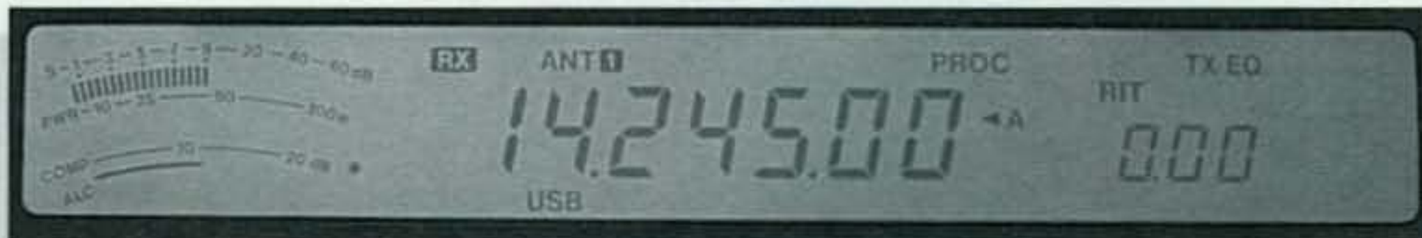
Photo A—A high (S9) level of power-line noise can mask everything on a band except the
