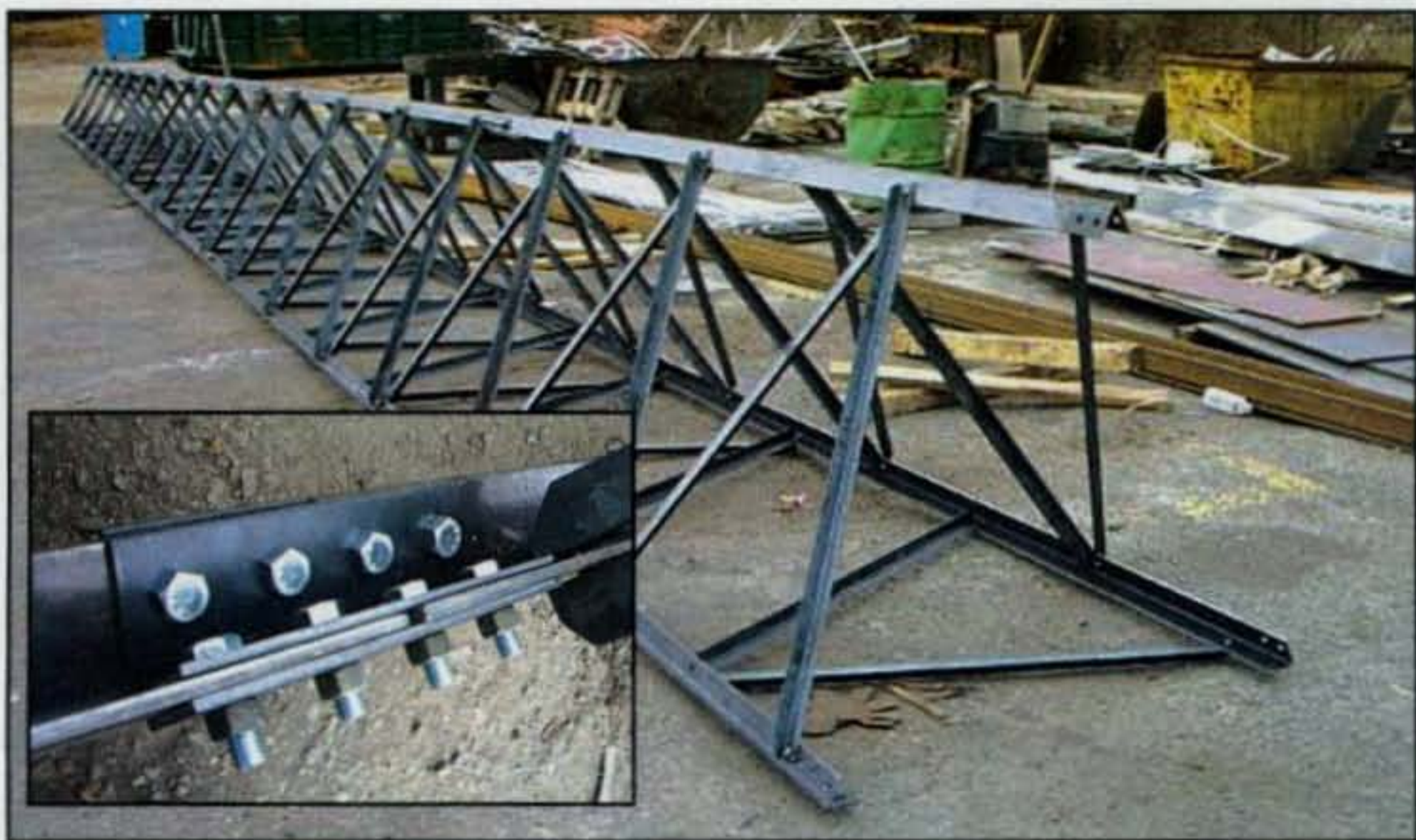
Photo G— Here's a finished AN Series Self Supporting HD-50 Tower. The rugged, lightweight, open-lattice, modular-design towers are assembled outside the company's shop to ensure everything fits together prior to full hot-dip galvanizing treatment. The inset photo details a typical section joint in a rugged AN Wireless tower. Steel plates are used on both the outside and inside of each joint, and tower sections are connected together with 24 bolts per connection to offer maximum strength. (Photos from the AN Wireless website)
