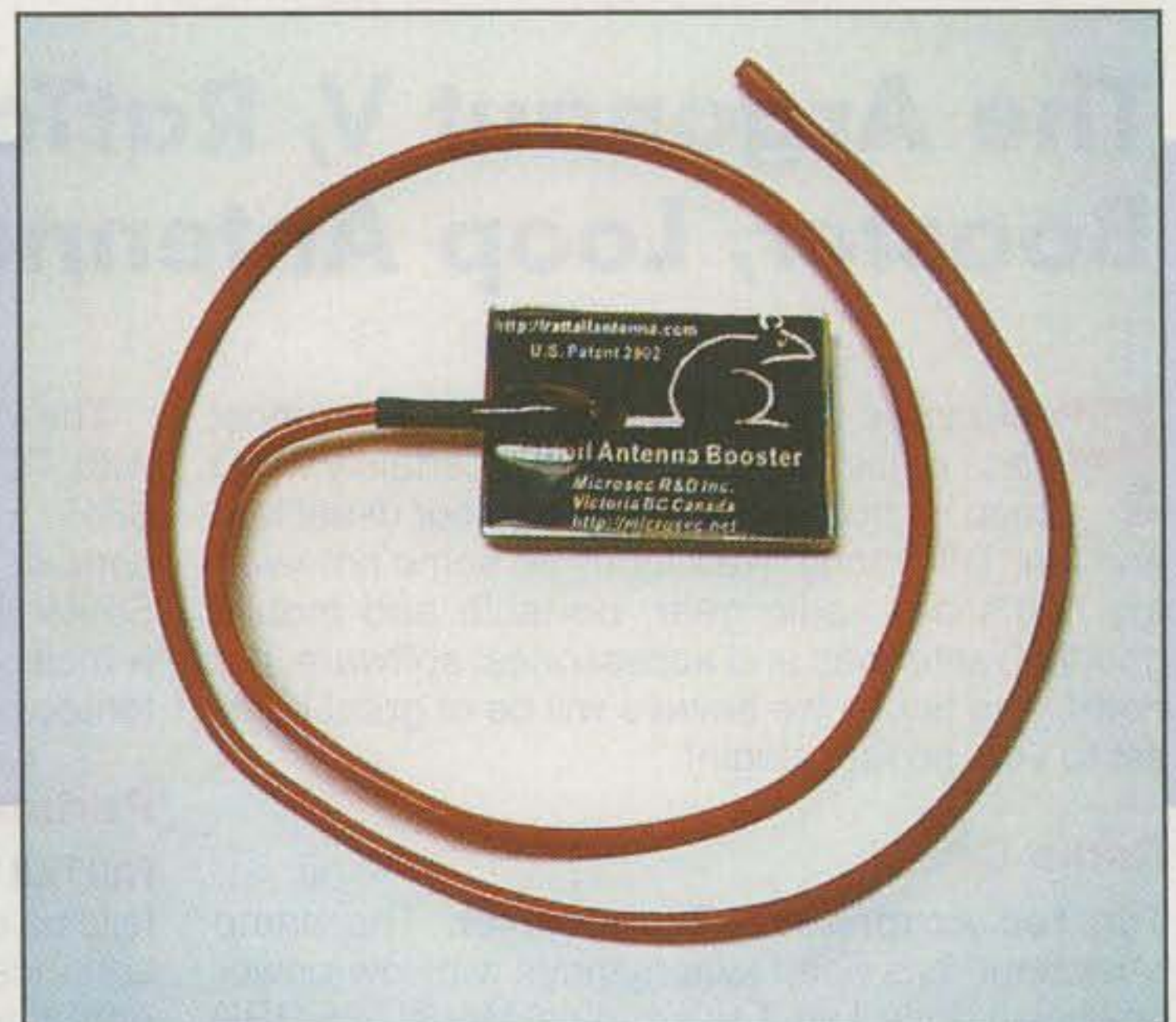
Photo C— The RatTail Antenna Booster sports a counterpoise-like "rattail" (just Velcro®), which connects to the back of the handheld radio. It rolls up for carrying in your pocket, although you can leave the rattail attached to the radio. (Photo courtesy Microsec Research and Development)
