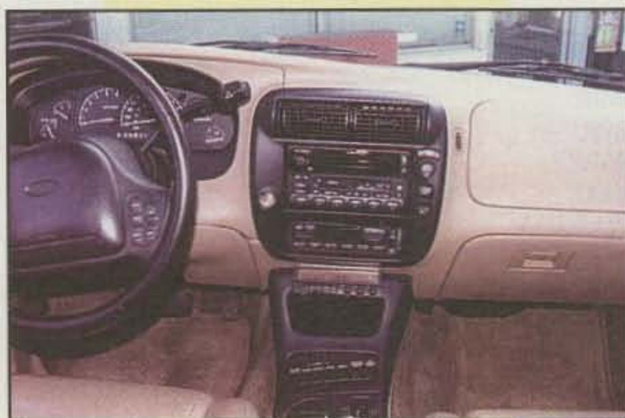
Photo 1— N6CDJ of Burbank, California did this neat installation of a Kenwood tri-band in a Ford Explorer. The control head is just below the heater controls, and the microphone stores in the center console.
