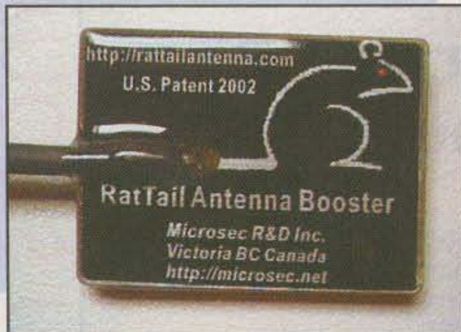
Photo B— The new RatTail Antenna Booster, offered by Microsec Research and Development, is a small device that dangles from your 2 meter handheld. The booster is claimed to increase transmitted energy by 9 to 12 dB (800 to 1600 percent) when measured at a distance of 2 km (1.2 miles) or more. Received sensitivity is also said to be increased by the same amount. (Photo courtesy Microsec Research and Development)
