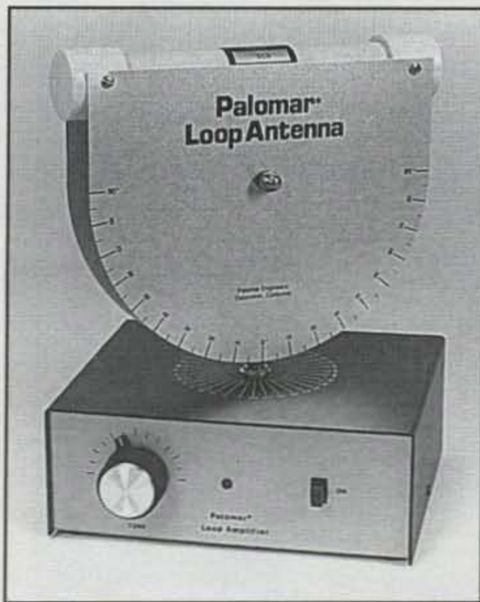
Photo D—Palomar Engineers has reintroduced its famous Loop Antenna, a "new and improved" model that has over 10 dB additional gain and sensitivity. The system consists of a loop amplifier and plug-in loops. Loops are available for the LF band, 150–550 kHz; the AM broadcast band, 530–1700 kHz; and the amateur and short-wave bands, 1700–6000 kHz. (Photo courtesy Palomar Engineers)
