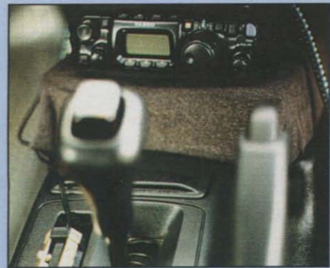
Photo 9— We often take Squeeky mobiling, as it fits perfectly into the gearshift position-display window on my Camaro, and probably many other vehicles. A thin piece of clear double-sided tape on the key's base also holds it solid to a rig case or other surface. Paddle is fitted with cable and 1/8 inch stereo plug for instant use.
