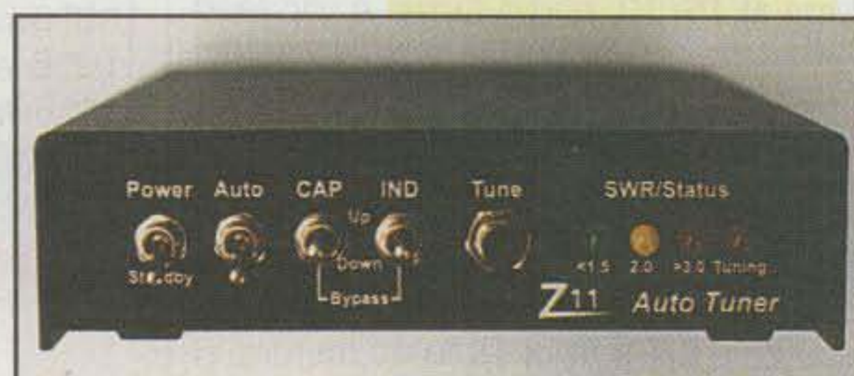
Photo 2— The very popular and widely acclaimed LDG Electronics Z11 Automatic Antenna Tuner. Unit measures 1.5"H x 5"W x 7"D, matches impedances of 6 to 800 ohms, and operates from 13 volts DC or a pair of 9 volt batteries for stand-alone activities. Note SWR-indicating LEDs on front panel. Nice!
