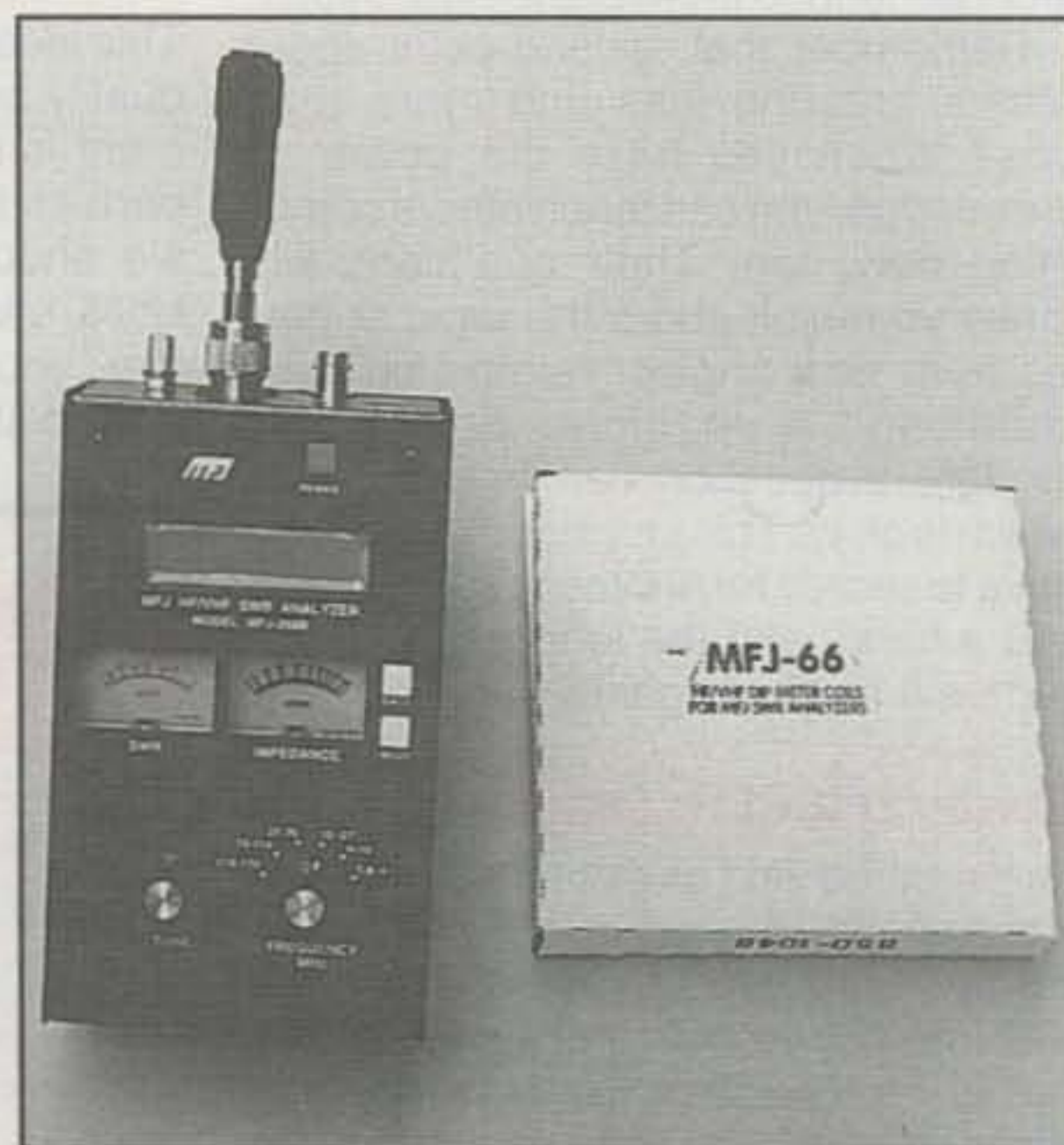
Photo A— Need a simple and convenient way to check resonance of a hand-wound coil and junk-box-obtained capacitor? An MFJ-259 Antenna Analyzer and accessory MFJ-66 Dipper Coil are the ideal solution.
