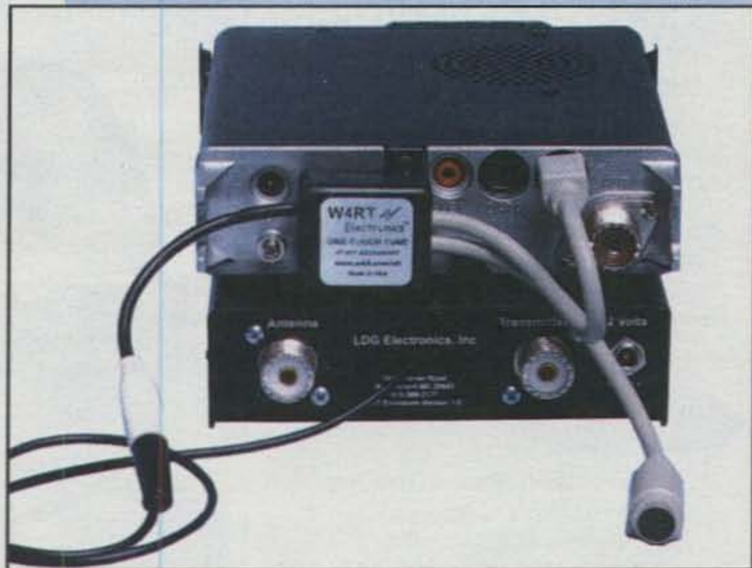
Photo 4—The W4RT Electronics One Touch Tune mod interconnecting a Z11 and FT-817. Mod is ideal for walk-and-talk HF'n where SWR changes as you move. Additional One Touch Tune modules for interfacing LDG's AT-11MP and RT-11 tuners with an FT-897 or TS-50 are also being developed by W4RT Electronics.
