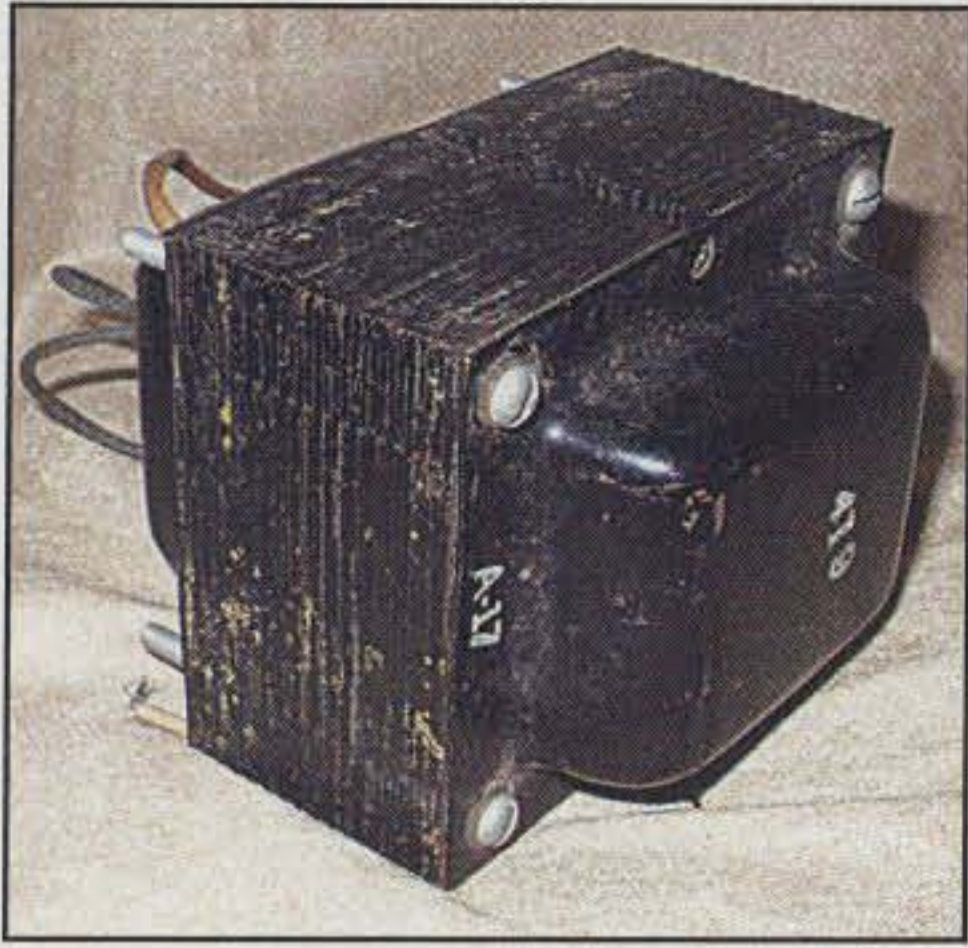
Photo D— Power transformers like the one shown here usually consist of two or three windings on a laminated iron core covered with a metal case.
