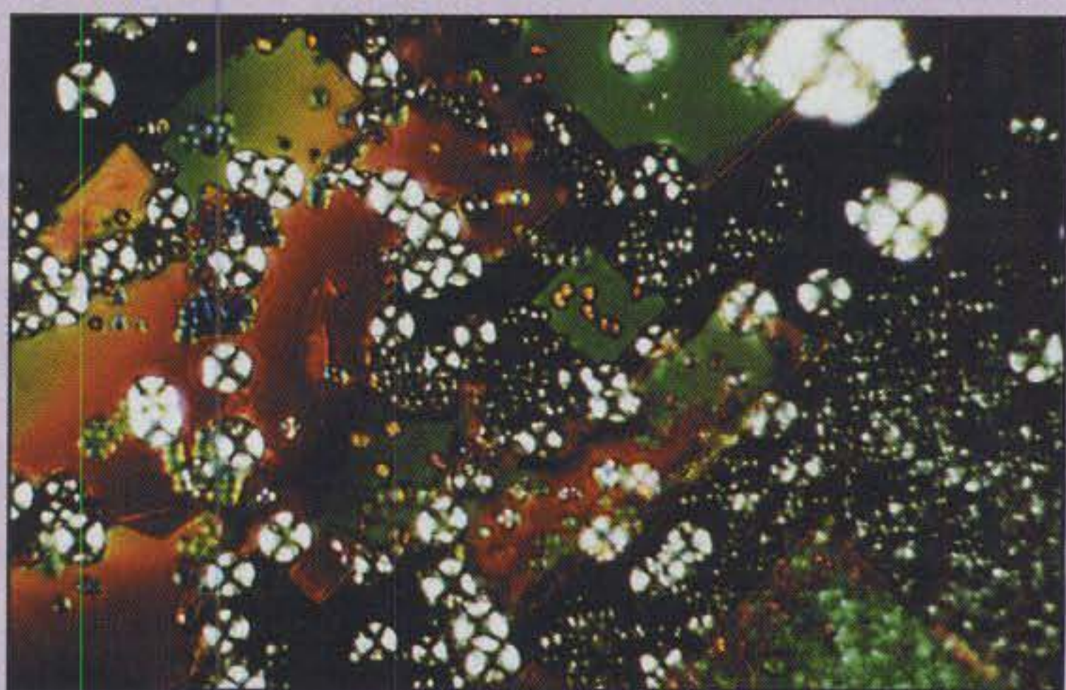
Coffee and sugar can keep you awake during a DXpedition, but if you spill it on your radio, it will creep under the steel cover and sit on the electrical contacts.
