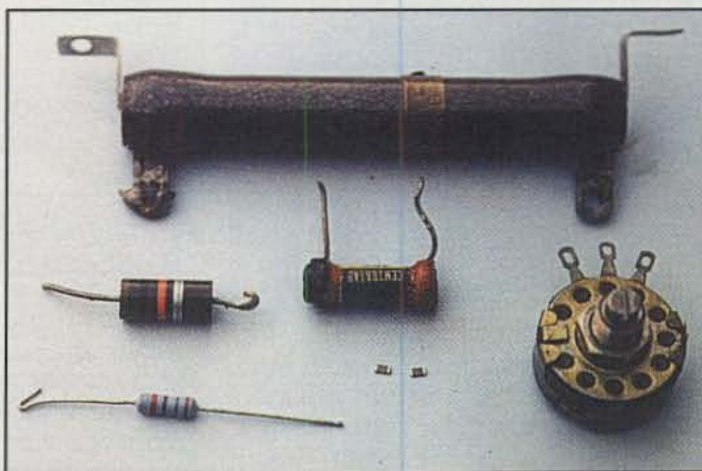
Photo A—A general sampling of resistors used in various types of electronic gear both past and present. Items shown include familiar the 1 and 2 watt leaded-type resistors (left), wire-wound 50 watt resistor (top), potentiometer (right), and classic Body-End-Dot resistor (middle). The two tiny specks appearing below the B.E.D. resistor are surface-mount "chip" resistors. Most general-purpose resistors are made of compressed carbon granules.
