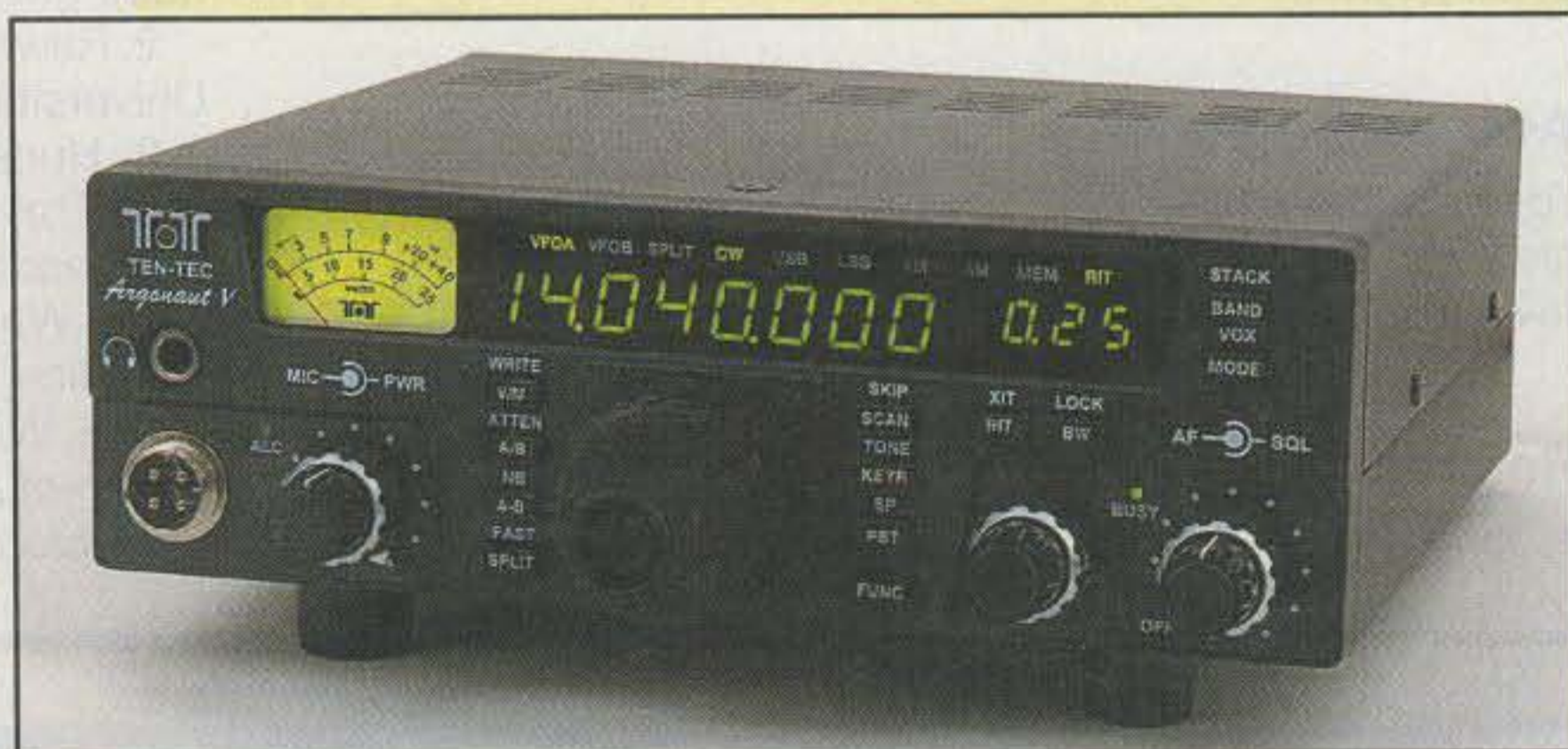
Photo A— The front panel of the Argonaut V consists of 12 buttons, two dual-concentric controls, two rotary encoders (including the main tuning control), a headphone jack, two LED indicator lights, a meter, and a three-part LED display.
