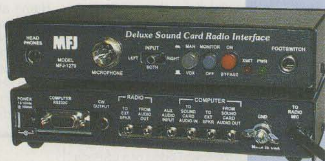
Photo B— The new MFJ-1279 Deluxe Sound Card Radio Interface boasts all the features of the popular MFJ-1275 Sound Card-to-Rig Interface, but sports several new interfacing jacks, including support for footswitch control. (Photo courtesy MFJ)
