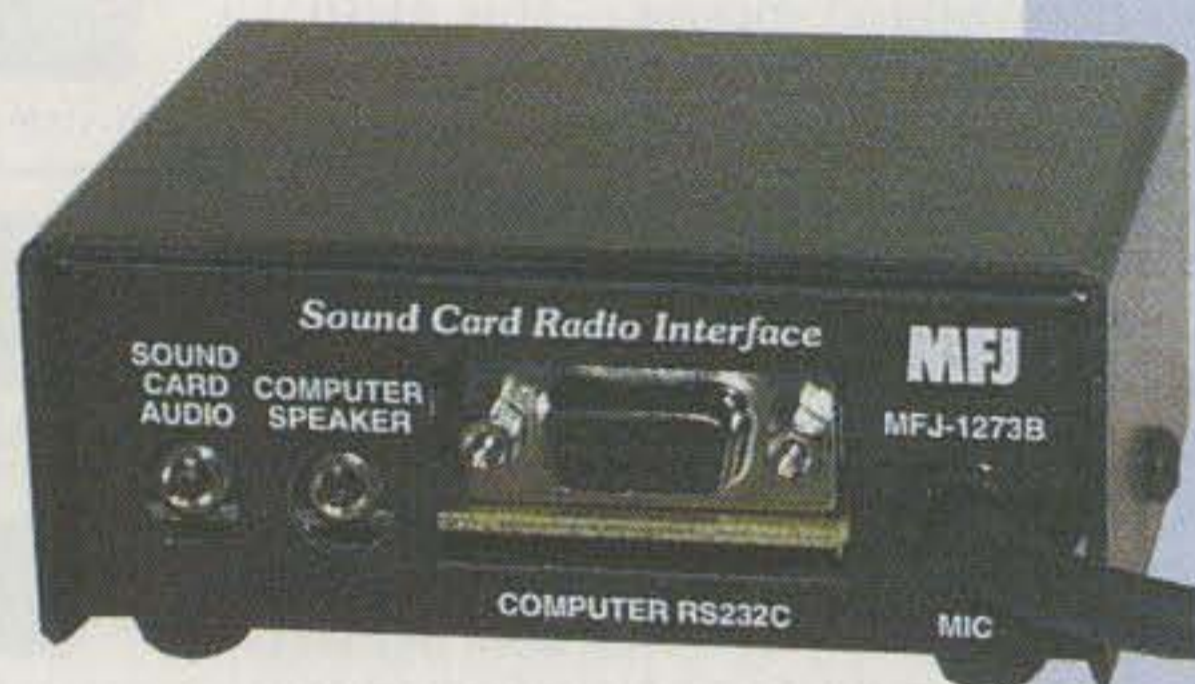
Photo C— MFJ also offers the new MFJ-1273B Digital Modes Sound Card Interface. This basic sound card interface is for those who operate mostly digital modes and who don't need a microphone input. (Photo courtesy MFJ)
