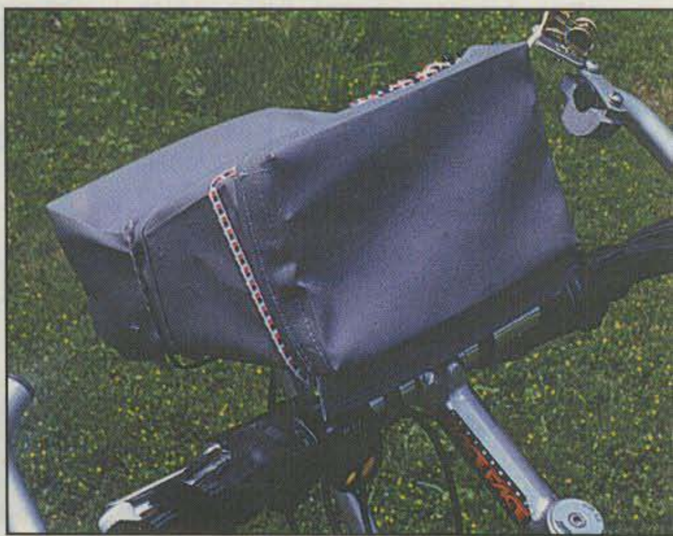
Photo 3— A custom water-repellent cover protects the transceiver during inclement weather or when traveling on dusty roads. Rig is powered from an internal battery pack, and an auxiliary battery pack rides in the saddlebag.
