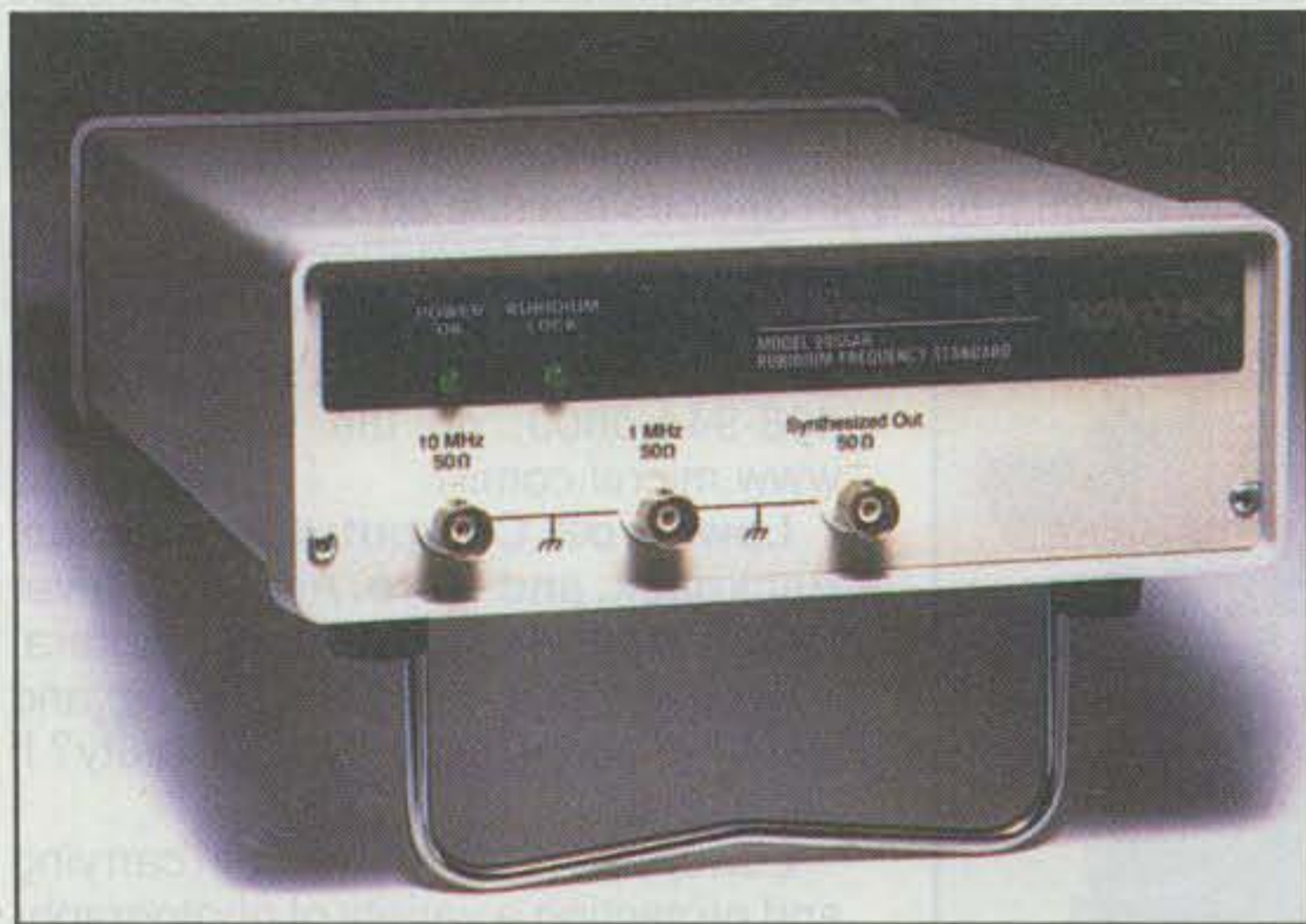
Photo E— If only the very best will do for your radio shack, Novatech Instruments offers the first-class Model 2955AR Rubidium Frequency Standard. It contains a direct digital synthesizer, locked to the atomic resonance Rubidium oscillator, providing any frequency between 100 Hz and 30 MHz in 1 μHz steps with atomic clock accuracy. (Photo courtesy Novatech)
