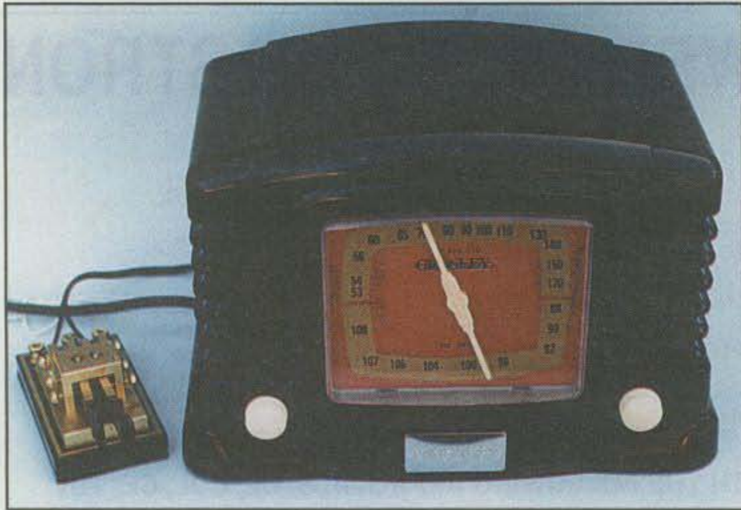
Photo B— Remember this marvelous Crosley retro radio from Universal Radio, Inc.? We highlighted it in our December 2002 “Christmas Gifts” column. We expanded it into a QRP transceiver without detracting from its original appearance, and even use its audio amplifier section to fill a room with ham band sounds.
