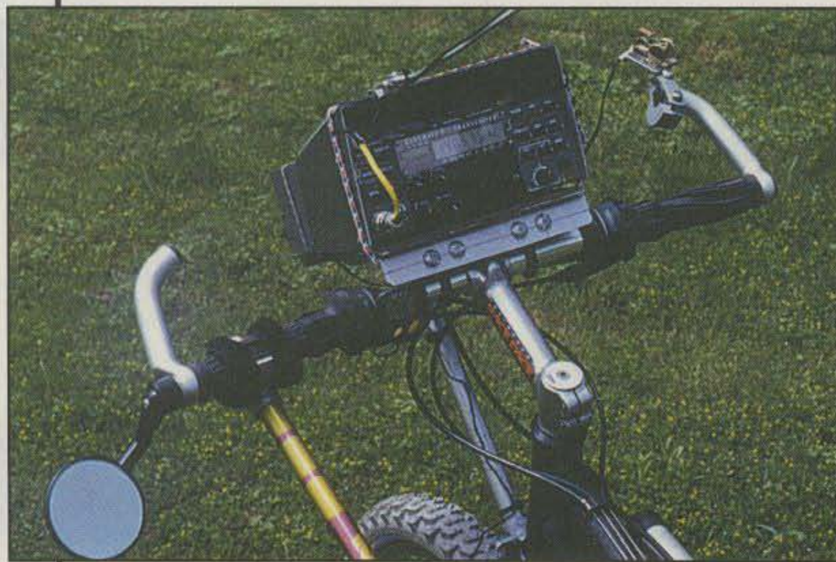
Photo 2— A closer look at the "gear end" of the VE3JC setup shows the Elecraft K2 secured to its support bracket with bungee cords. Note the mic on the boom, the tiny K9LU "Bulldog" iambic paddle on end of the right handlebar, and the tip of the parking stand rod on the left handlebar.
