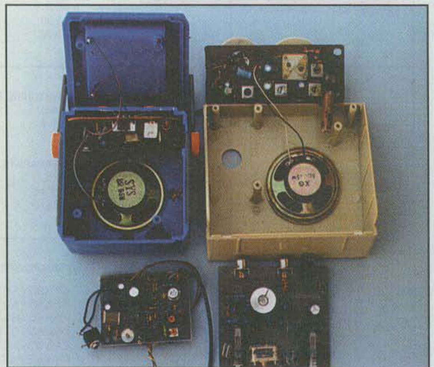
Photo E— Looking inside two small transistor radios, we see a NorCal 49er board will mount right to the speaker’s magnet with double-sided tape or fit directly into the radio’s circuit board slot (radio on left). Likewise, a Vectronics board easily mounts to the speaker’s magnet in the tan-case radio on the right. Numerous other radio/rig combinations are also possible.
