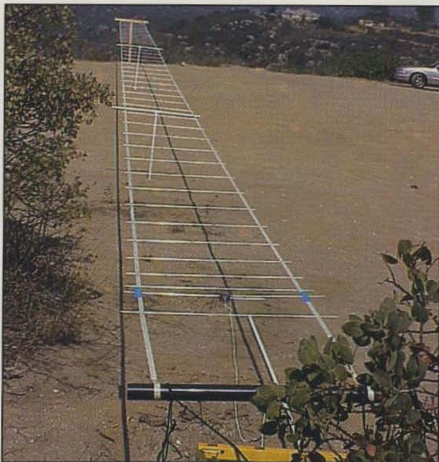
How directional is a 44-element 2 meter Yagi? Foxhunters found out the hard way on a southern California convention T-hunt. (Photo by Tom Sneden, KE6VCR)
