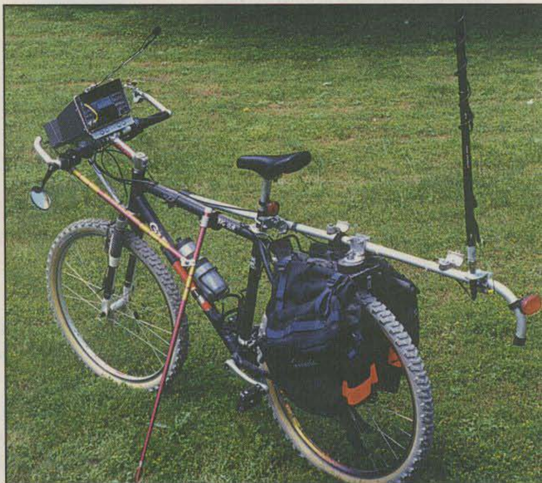
Photo 1— Now this is big-time mobiling for sure! The setup belongs to John Cumming, VE3JC, and it has traveled hundreds of miles, worked DX galore, and is also easy to duplicate. Note the Elecraft K2 transceiver sits in a handlebar-mounted and suspension-braced bracket. An Outbacker antenna is mounted to an aluminum support tube attached with L brackets to the frame of a Gary Fisher Big Sur mountain bike. (Photos 1, 2, and 3 via VE3JC)
