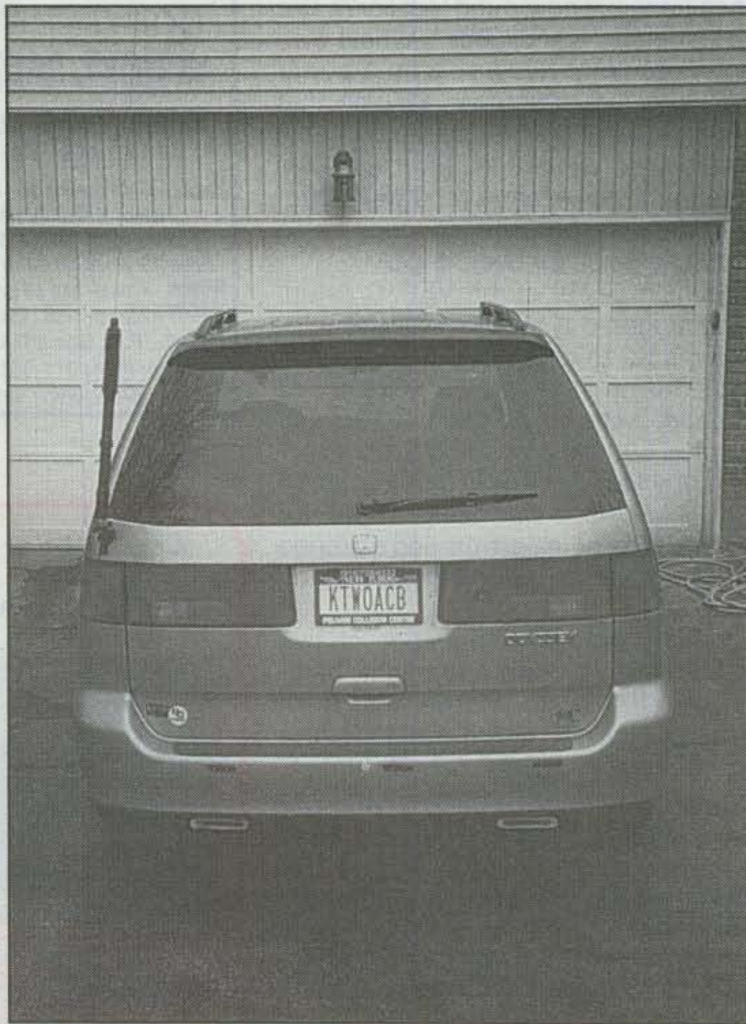
Photo 6— Rear view of the K2ACB van. The Yaesu ATAS multiband antenna mast is supported by a Diamond K-400 lip mount and almost looks like a natural part of the van's design. It is low profile and nice!
