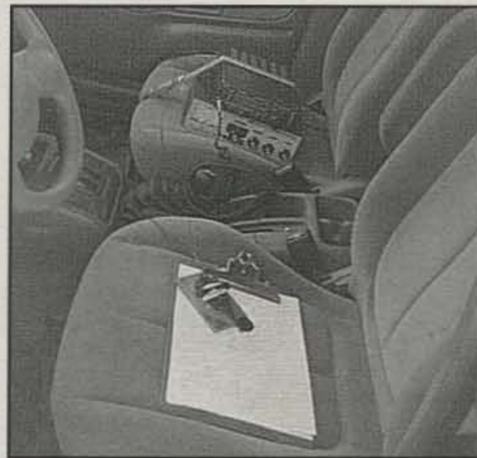
My mobile rig in a typical rental car installation. The TS-50 and MFJ tuner are strapped down in the passenger seat. The antenna is a mag-mount 20 meter Hamstick. I have used this versatile arrangement in a lot of cars to make my 11,000+ mobile contacts from 655 counties plus work 70 countries!
