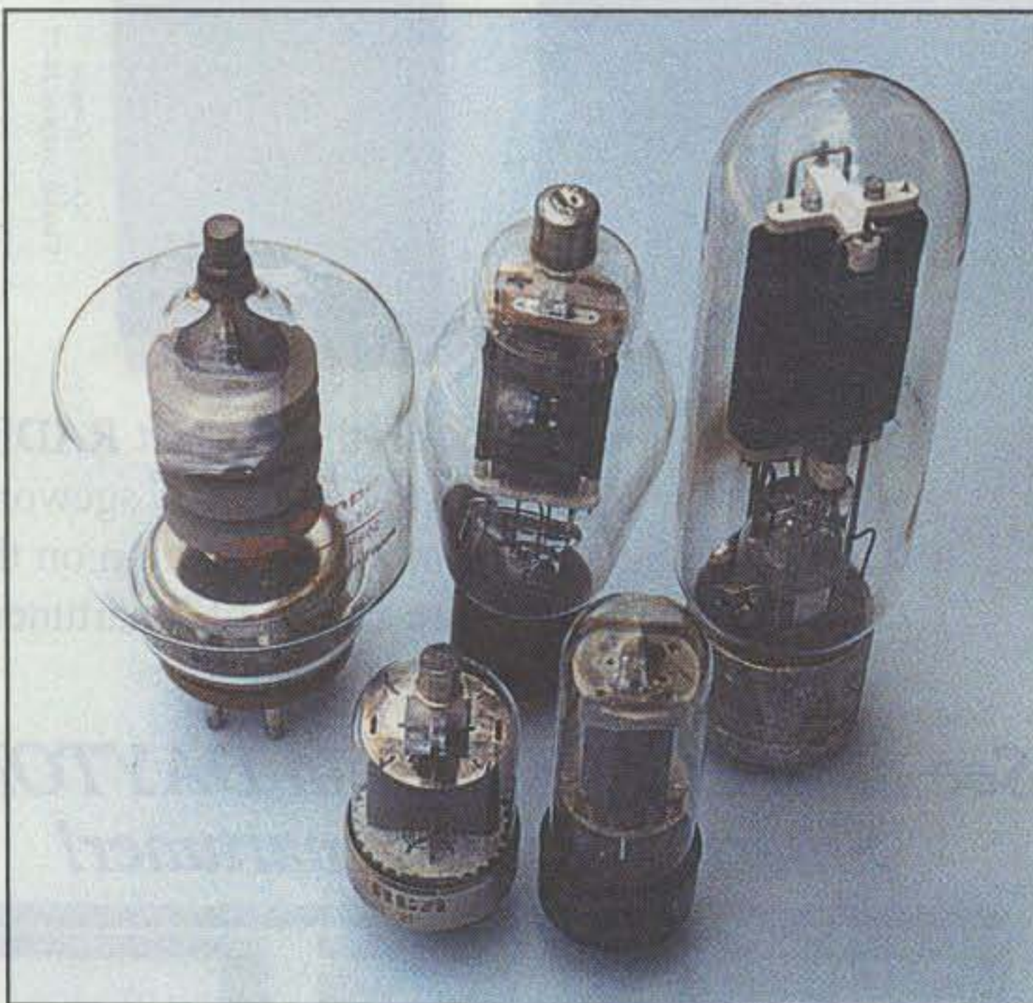
Photo A— This small sampling of vacuum tubes represents all-time transmitting favorites in amateur radio past and present. They are (left to right rear) the 3-500Z and 211, and the 811 and 211; in front are the 6146 and the 6L6. Will tubes ever become fully outdated? Let’s hope not, as they can produce beautiful, rich-sounding audio unattainable with solid-state devices.
