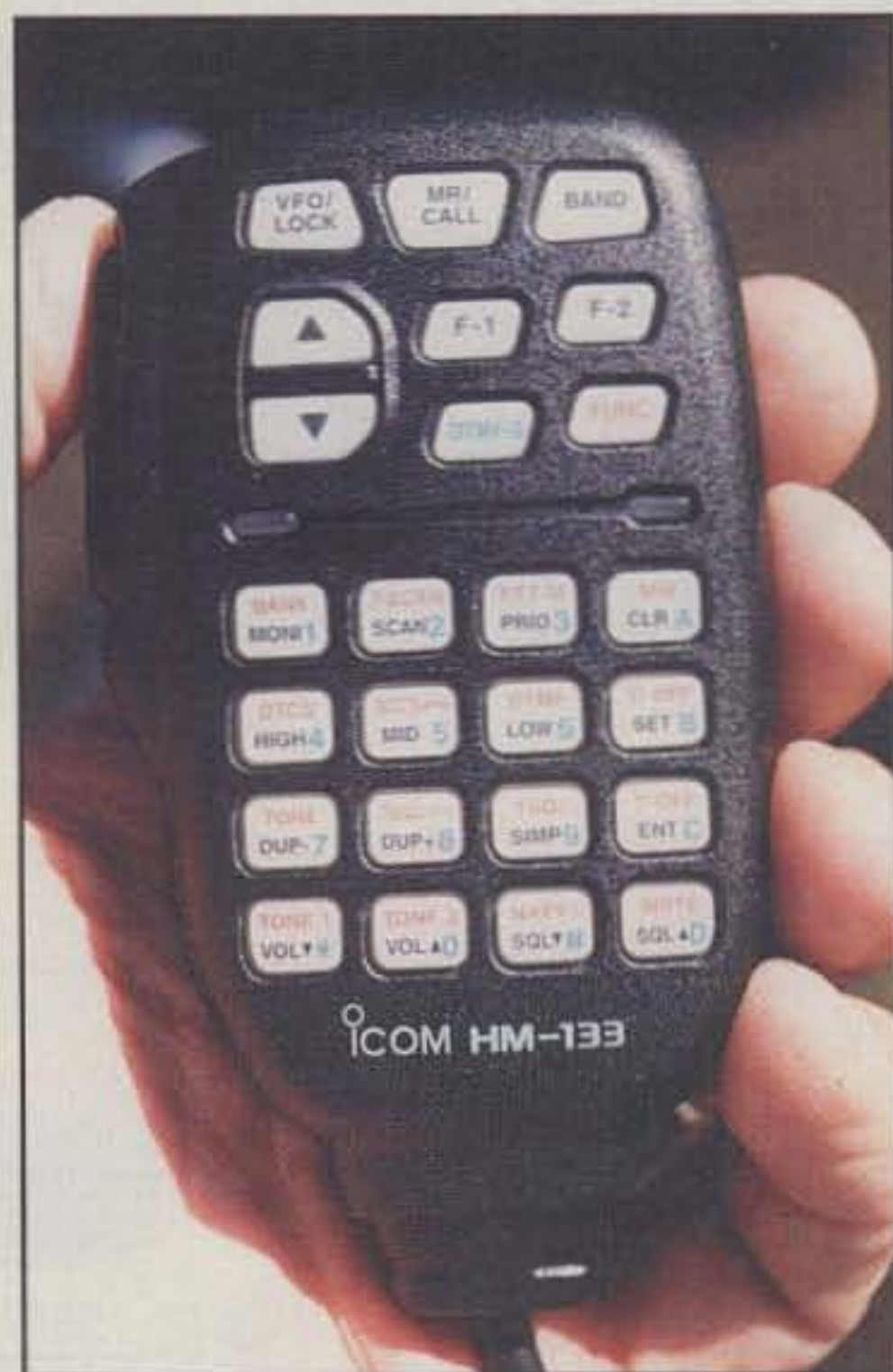
The 2720's standard microphone comes with lots of buttons, letting you control nearly all major radio functions from the microphone.
