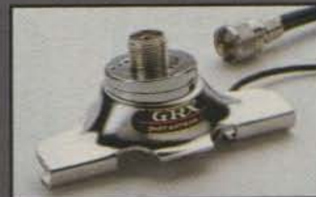
COMET GR-5M Trunk lip mount, low-profile, stainless steel. Offset washers provide up to 17 deg vertical adjustment of antenna. 16'9" of deluxe cable included, 18" of mini RG-188A/U style coax for easy entry thru the weather seal. Gold-plated SO-239/PL-259 connectors.
