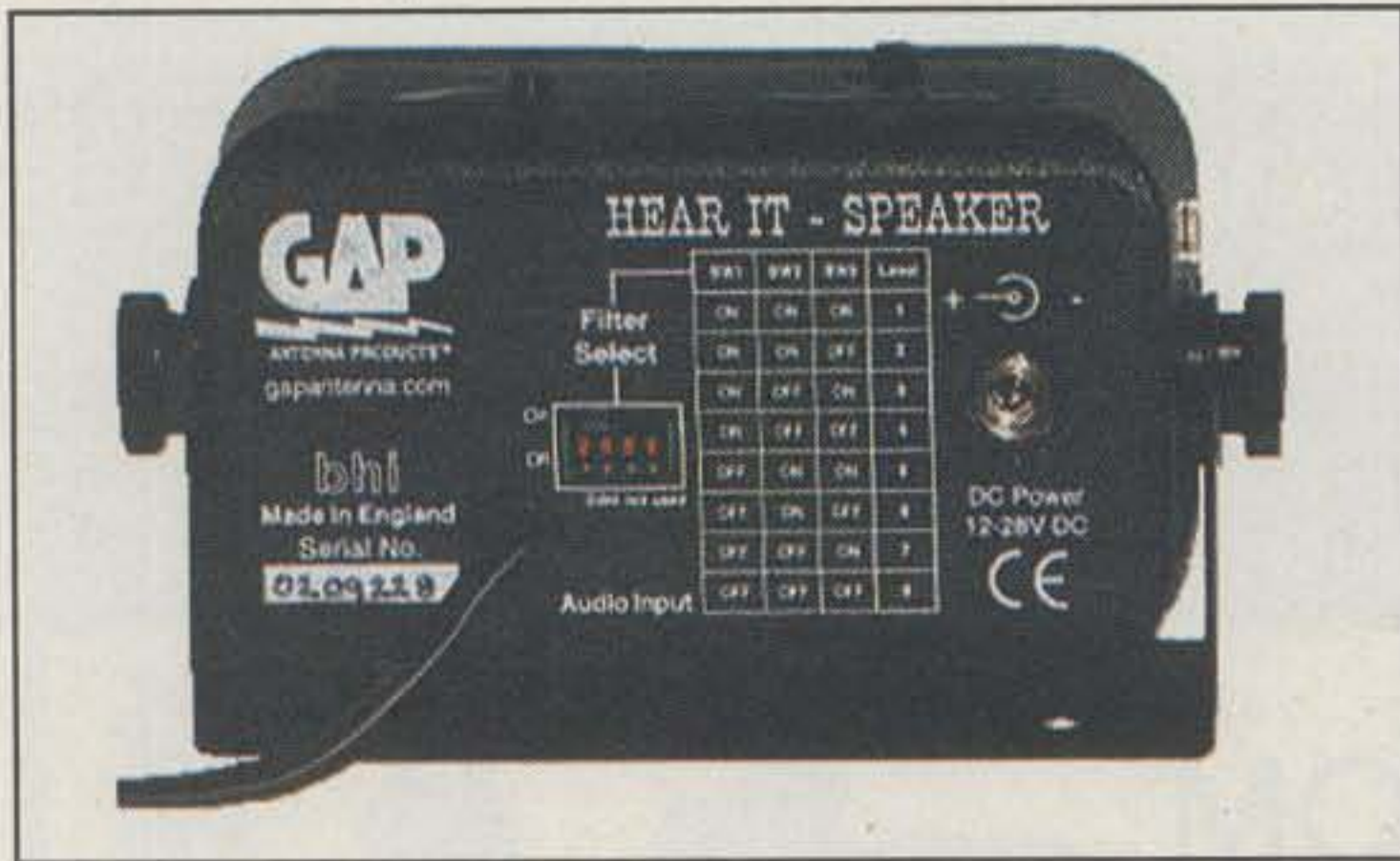
Photo B— On the back of the GAP Antennas HEAR IT SPEAKER are a set of “filter select” DIP switches to provide eight levels of noise cancellation. The switches allow the user to easily determine how much noise canceling he would like the unit to effect, level 1 giving the least amount of noise cancellation and level 8 providing the most. (Photo courtesy Gap Antennas)
