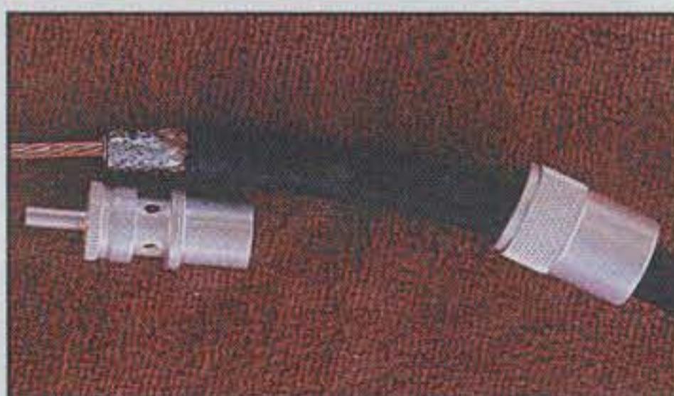
Photo 7— The tubing cutter makes removing the shield and center insulator quick and easy. Do not cut into the center conductor.
