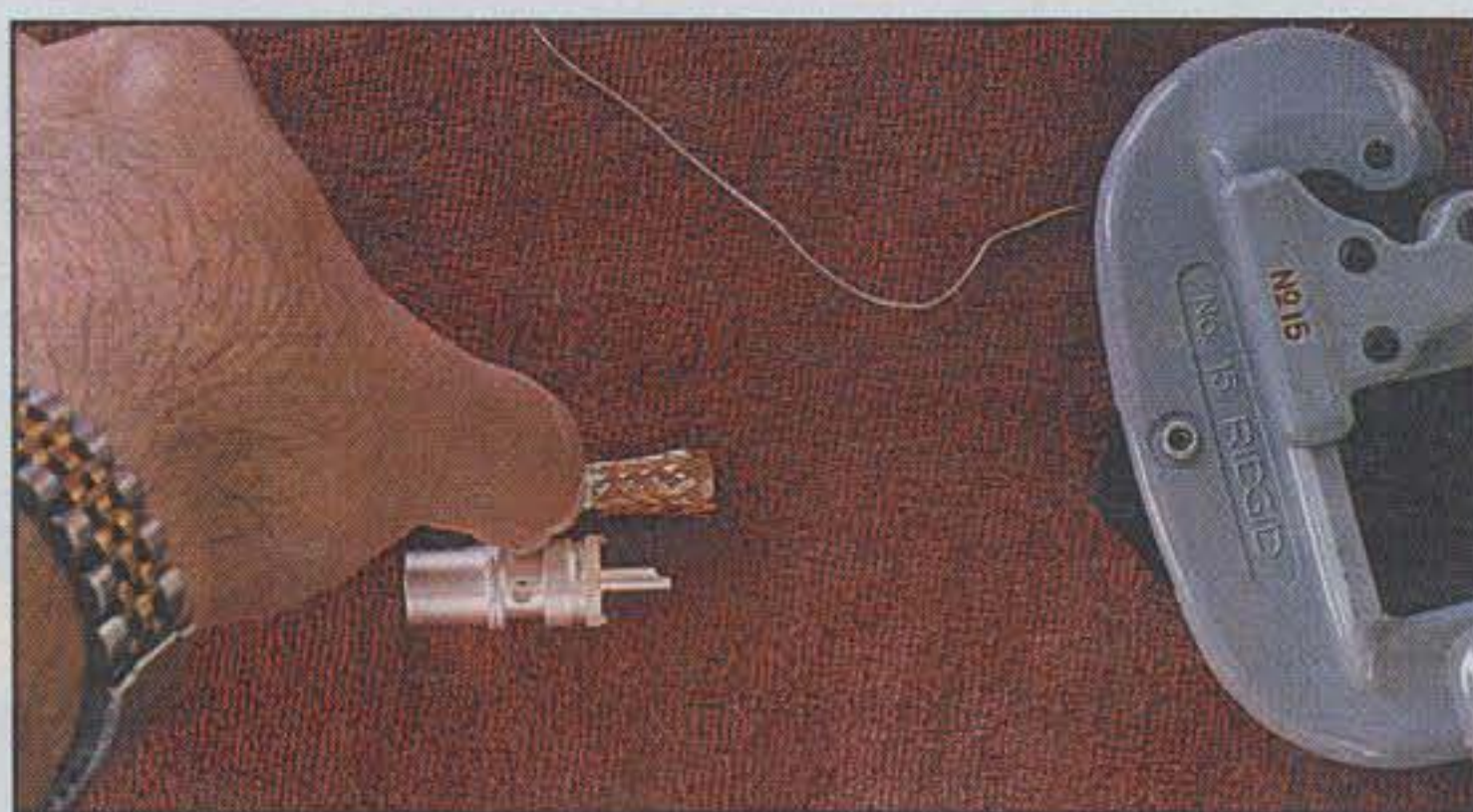
Photo 6— Again, my thumb indicates where to cut. The shield and center insulator will be cut so that the cable will fit into the connector body, and stop where the Teflon® insulator joins the connector body.
