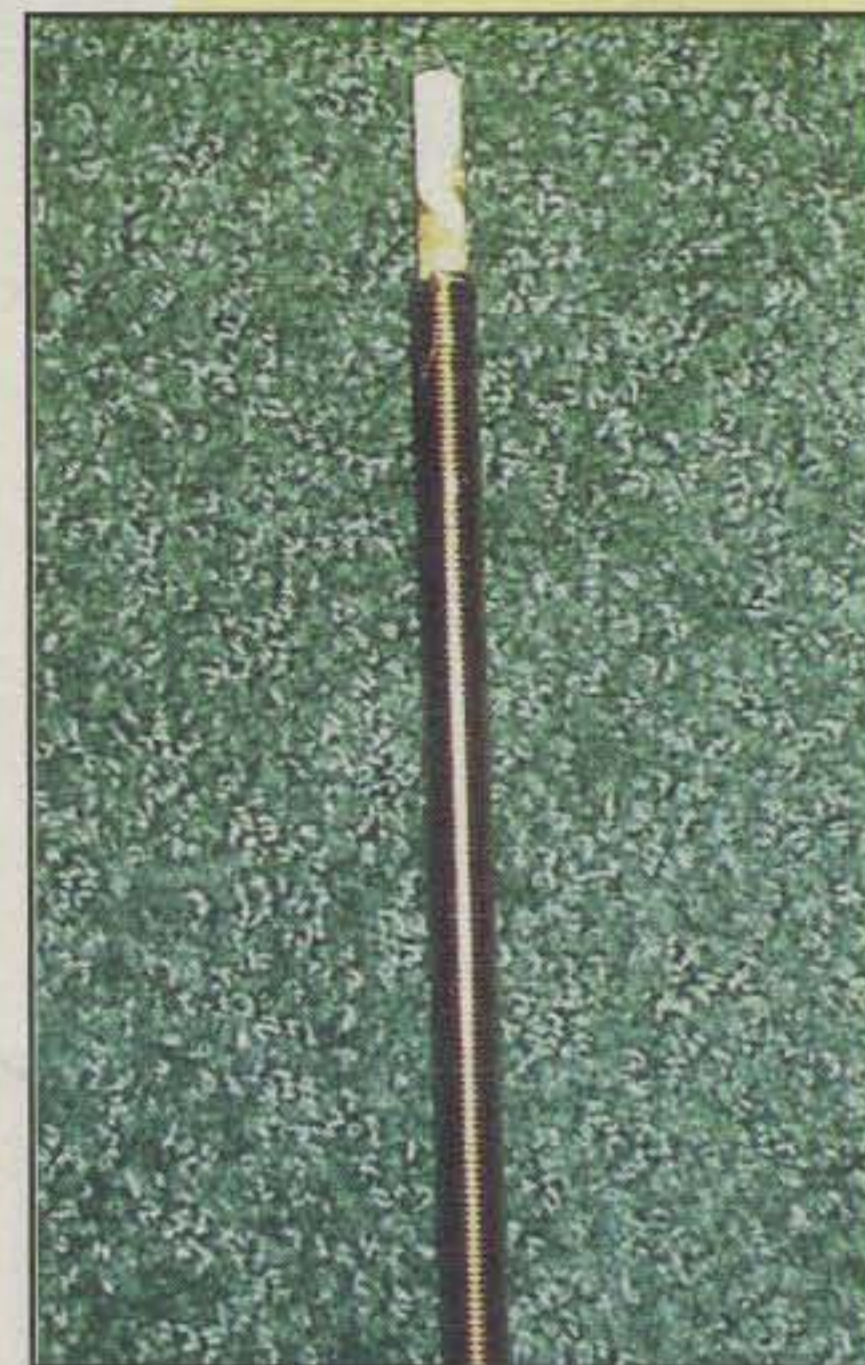
Close-up of the top of the helical winding. The last turn must be pressed flush against the turns below it to avoid corona effects from its sharp end.
