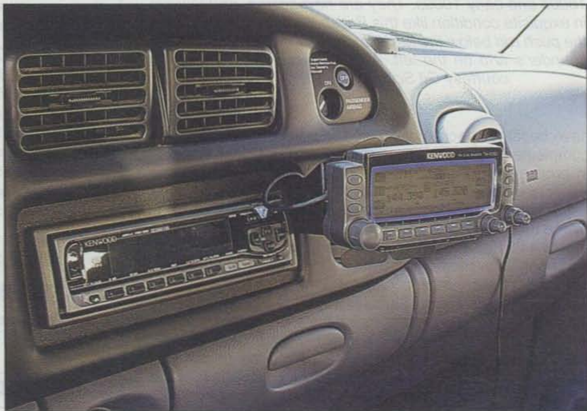
Kenwood TM-D700 control head nicely placed on a Panavise mount in 1999 Dodge Ram 2500 by KF6NXQ. (KF6NXQ photo)
