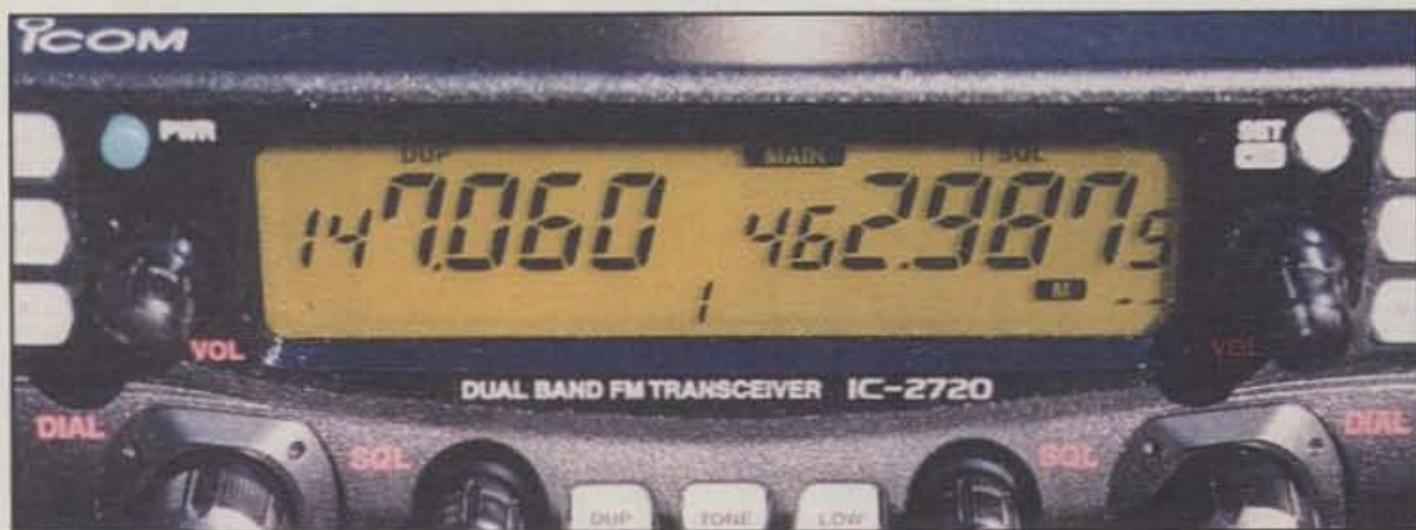
ICOM's IC-2720 true dual-band transceiver comes set up for separate installation of the radio and the control head, including an 11 foot separation cable and two separate mounts. A special mount for using the radio in one piece is an option. LCD contrast on the control head is at its best when tilted slightly down in relation to the viewer. (WB6NOA photos)
