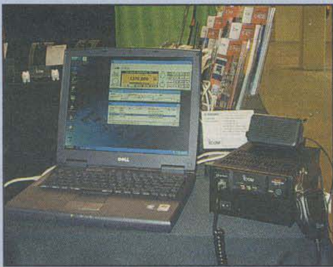
ICOM's ID-1 hooks up to a computer via a standard Ethernet connection and runs 128 kbps data as well as analog and digital voice.
