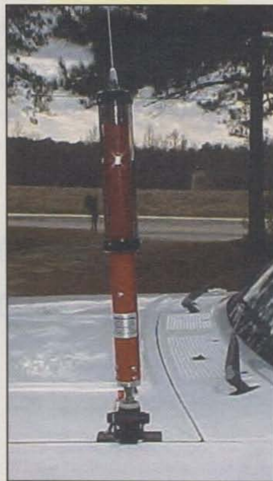
The "Little Tarheel" motorized, multi-band HF mobile antenna from Tarheel fits comfortably onto a trunk-lip mount and covers 40 through 6 meters with up to 400 watts PEP. (Photo courtesy Tarheel Antennas)
