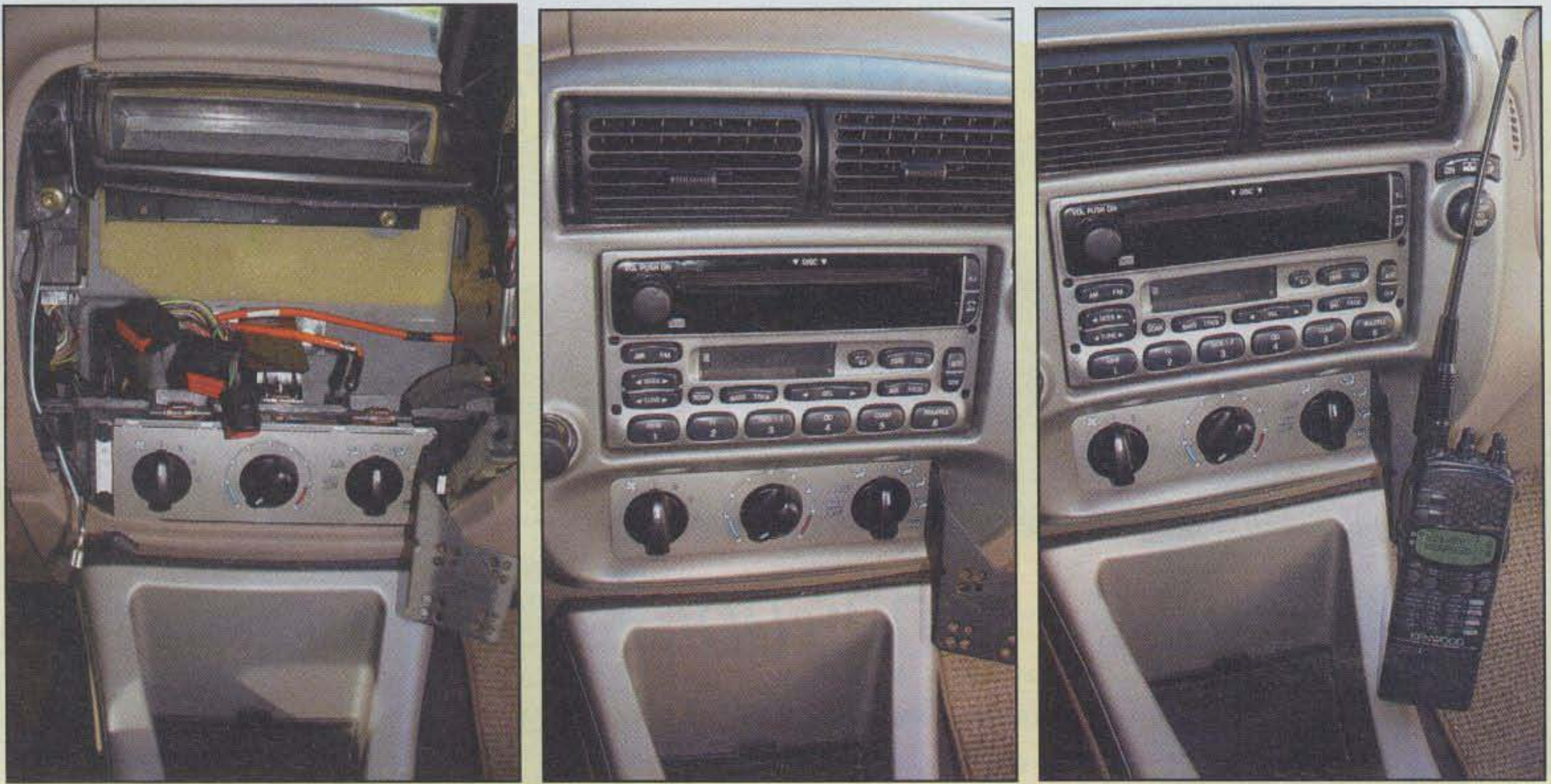
Custom-fit mounts by Panavise (and others) use existing holes for concealed mounts. Here we see "during" and "after" shots from Jeff, KF6NXQ, as he installed a Panavise mount for his HT on a 2001 Ford Explorer. Jeff reports the entire process took about 30 minutes. Panavise includes instructions with its mounts. (KF6NXQ photos)
