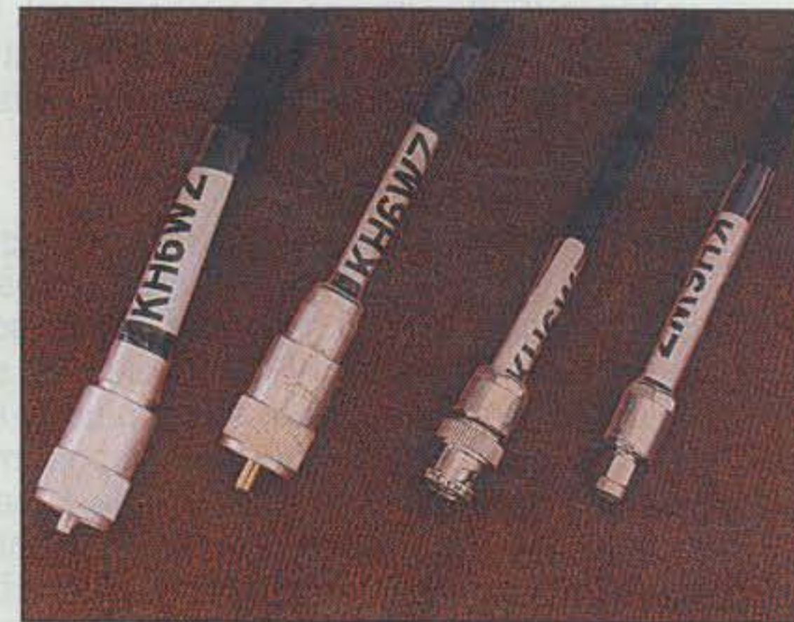
Fig. 15- All done. Left to right: PL-259 on RG-213, PL-259 with RG-8X reducer, BNC on RG-8X with SMA on RG-8X. As a final touch I added a callsign label to the cable and used heat-shrink tubing for added strain relief.
