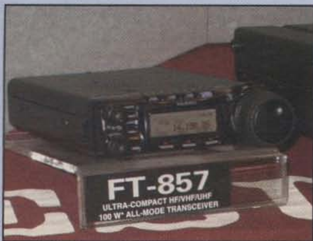
Yaesu's FT-857 is small enough to fit into a backpack, but it's a full-featured 100 watt HF/VHF/UHF all-mode radio designed primarily for mobile and portable use.
