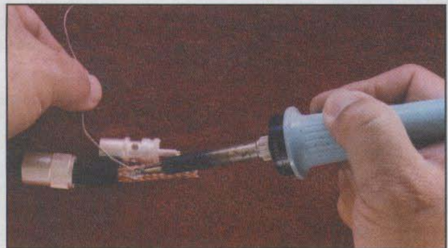
Photo 5— Tin the braid. As the solder melts into the braid, "wipe" the hot tip back and forth and along the braid, depositing a very thin film of solder on the shield. This turns the outer braid into a piece of tubing.
