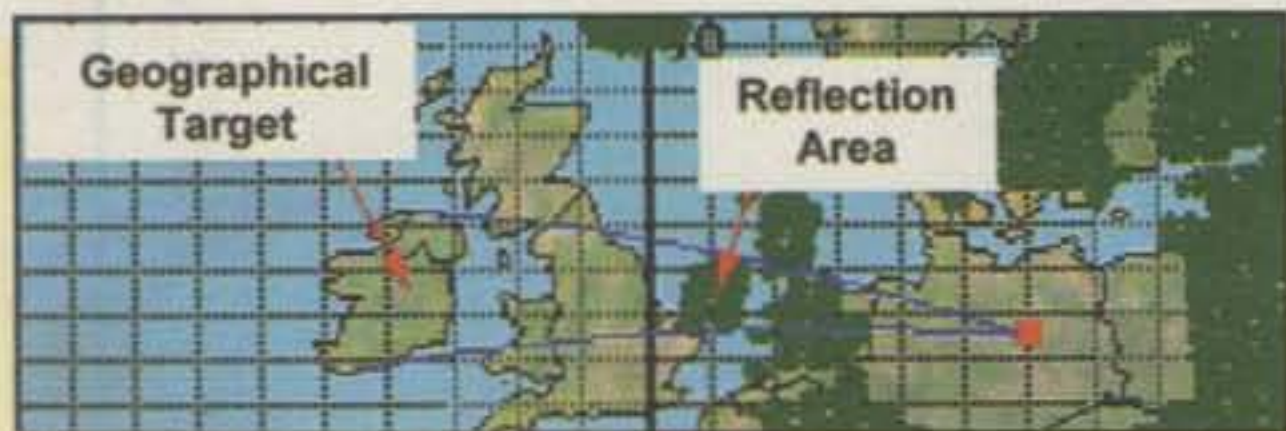
Fig. 2— Mirror image hot spots showing where you would aim your signal if you wish to work the United Kingdom.
