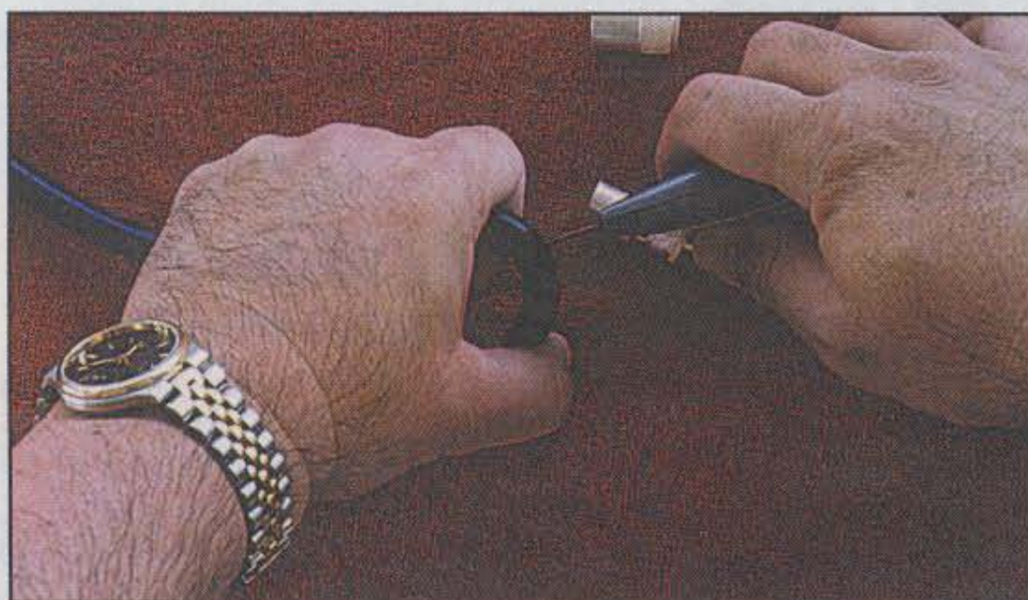
Photo 4— Carefully remove a section of the outer jacket. See text for a neat technique to prevent nicking the braid.
