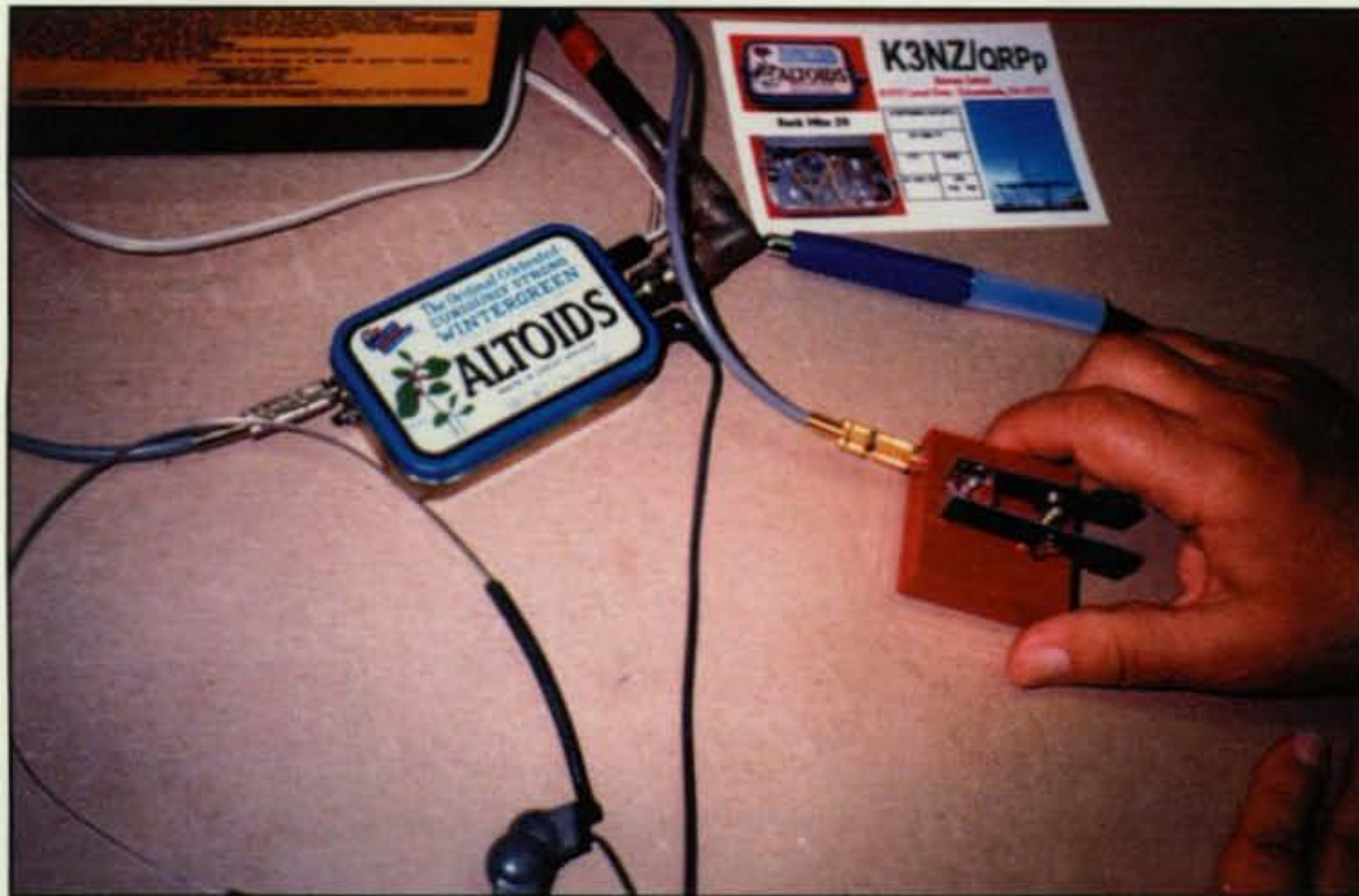
Photo B—Looking over the shoulder of Norm Zoltack, K3NZ, we see what's responsible for his attention-grabbing 20 meter signal—a little 500 milliwatt Rock Mite transceiver from Small Wonder Labs mounted in an Altoids tin. Using this gem Norm has worked 45 states and 15 countries, including a record-setting 10,000 mile CW QSO with VK4CEU in Australia. Life doesn't get much better than that!
