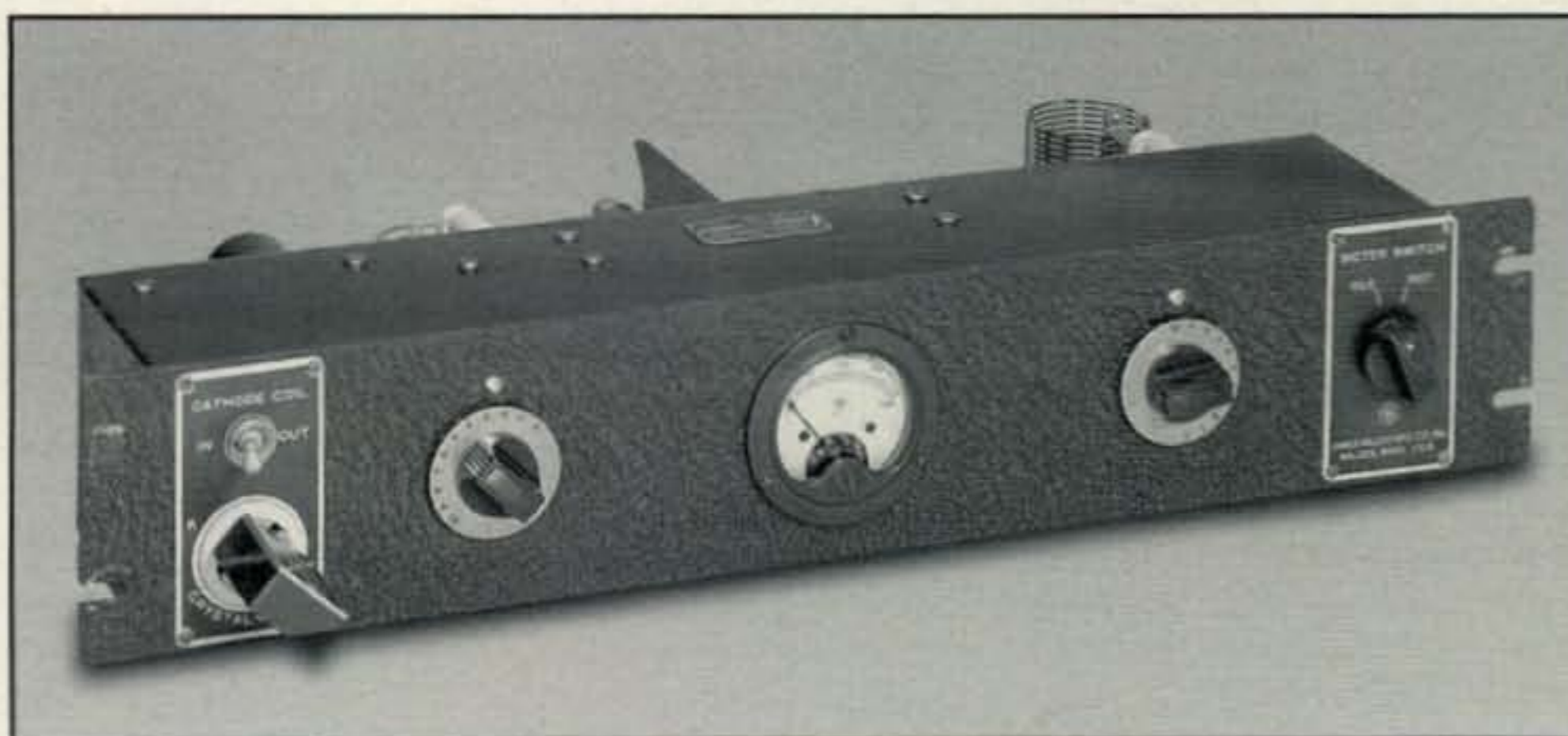
Millen 90800 Transmitter. Millen's 1946 6L6/807 transmitter owed much of its design to a pre-war magazine article. Power output was 50 watts on 80-10 meters.
