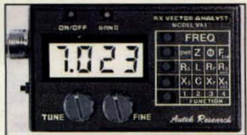
Photo F— The pocket-size Autek Research VA1 RX Vector Analyst is designed to check and adjust antennas, feedlines, and RF networks. It includes a microprocessor, A/D converters, and a low-power "transmitter" with a four-digit frequency readout, continuously variable from 0.5 to 32 MHz in six bands. (Photo from the Autek Research website)
