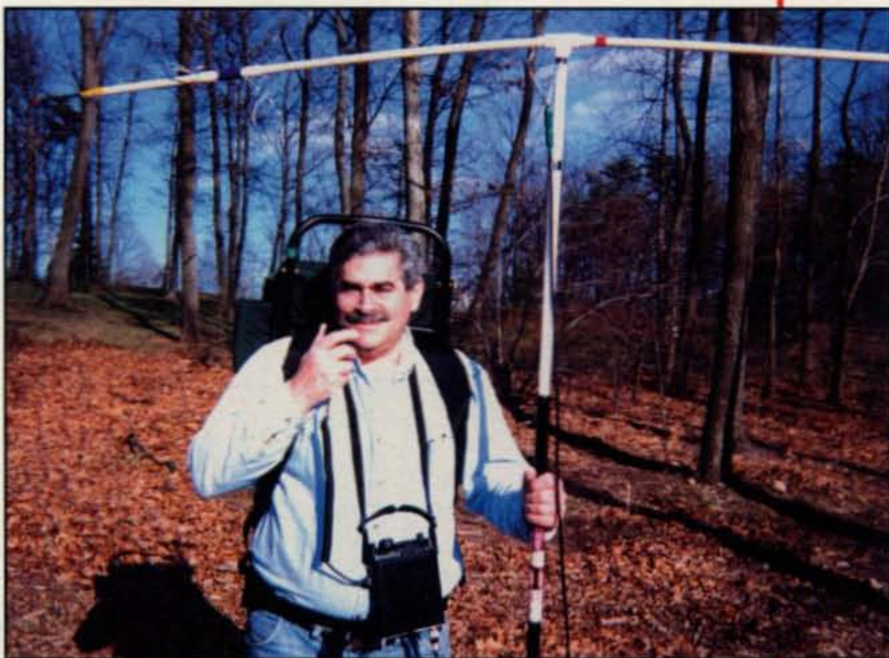
Photo A—Here's Bill Lazzaro, N2CF, hiking, hamming, and milliwatting to the max. The rig is a battery-powered FT-817 strapped around his neck, and the antenna is a popular "Buddipole" < www.buddipole.com > supported by a painter's pole that doubles as a walking stick. Bill has made numerous DX QSOs on SSB while running less than 1 watt with this setup. (Photo via N2CF)
