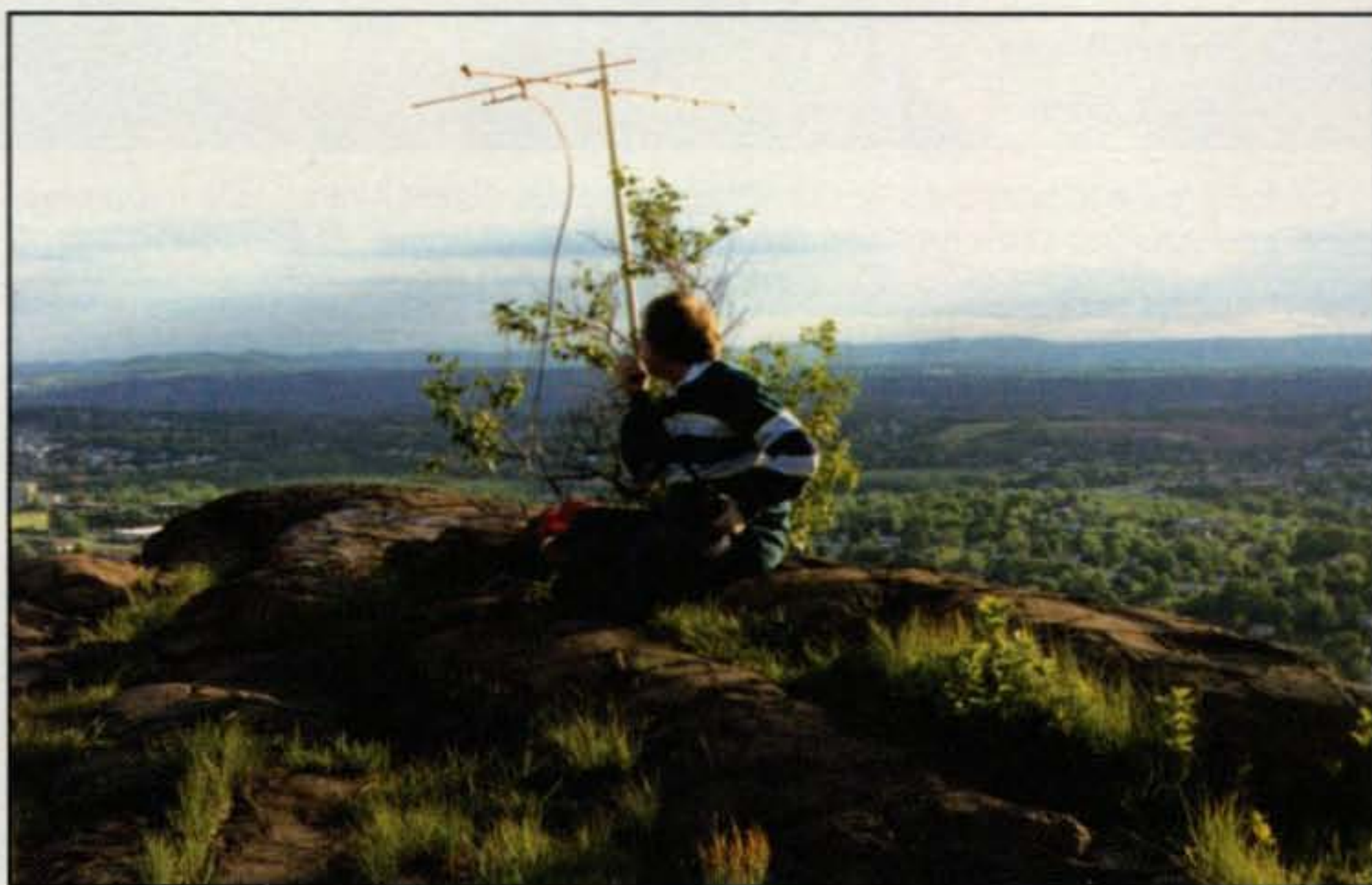
It doesn't take much to set up a very effective hilltop VHF contest station. From a location like this you can easily work several hundred miles on 2 meters with just a couple of watts and a small beam antenna.
