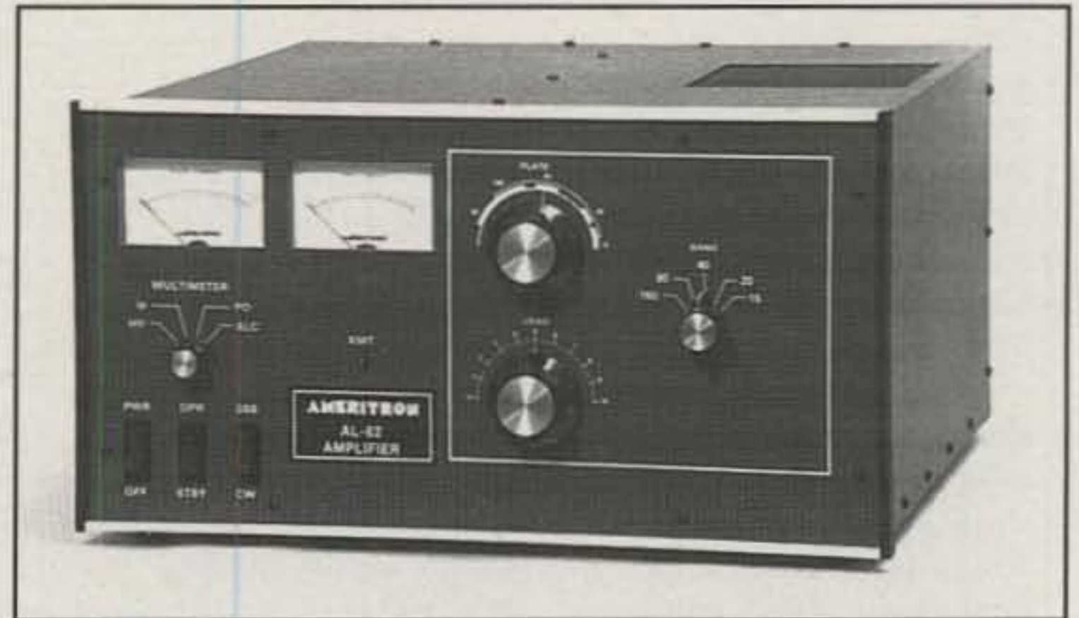
Photo A— A creditable number of modern linear amplifiers utilize grounded-grid circuit configurations for both simplicity and smooth operation. Ameritron's popular AL-82 is a good example. It uses a pair of zero-biased 3-500Z tubes to give a "barefoot" HF transceiver a band-commanding boost in signal strength. (Photo courtesy Richard Stubbs, KC5NSZ, of MFJ Enterprises)
