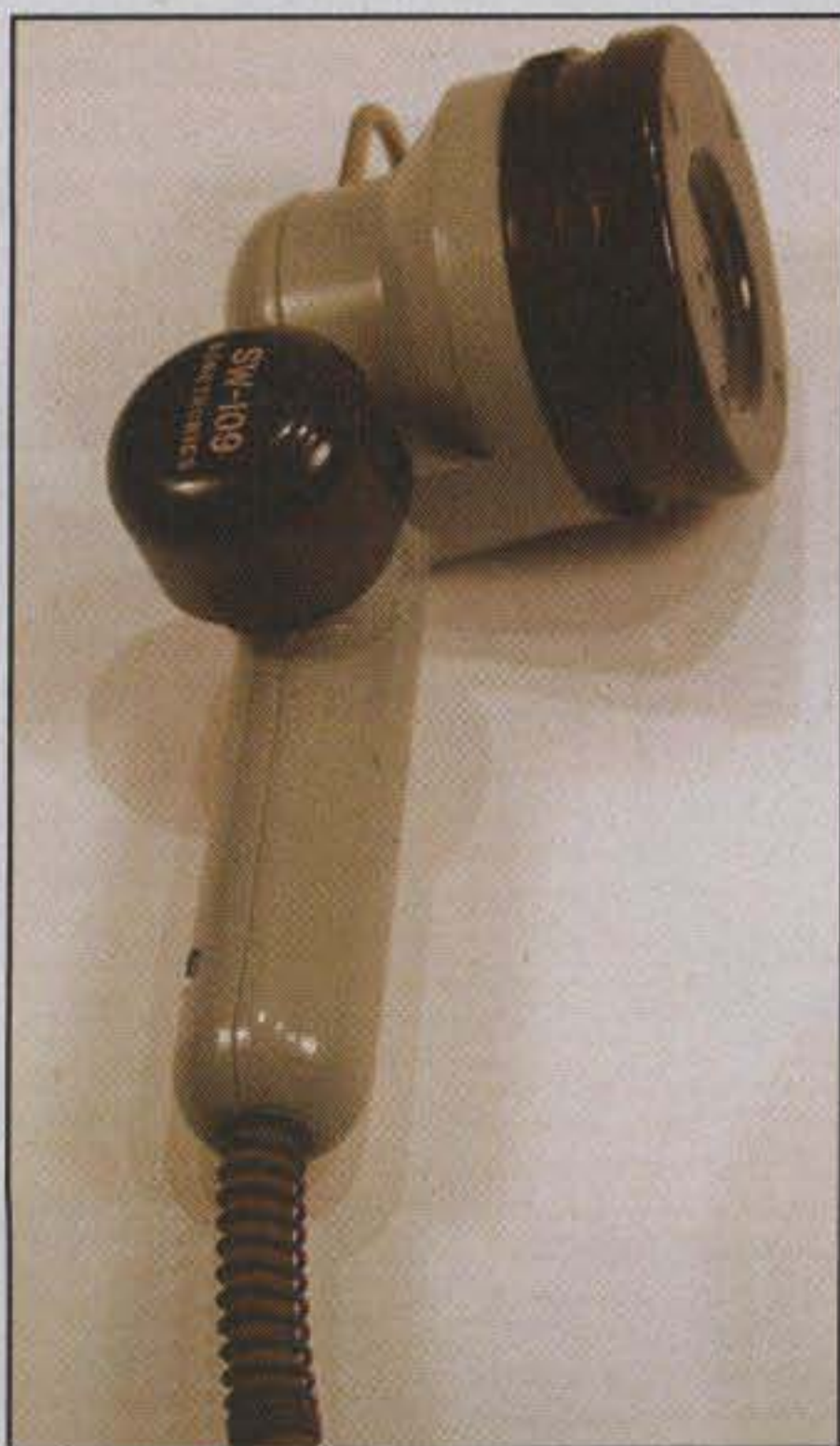
Photo G— Roaring back from extensive missions on tanks, ships, airplanes, and in police cars of yesteryear is the famous handheld version of the "Candlestick" microphone—the military T17 with unmistakable PTT switch. This captivating gem was popular during the days of AM mobiling with big-tube transmitters, Gonset receive converters, and whirring dynamotors. Totally and unquestionably awesome! (Photo via K9EID)
