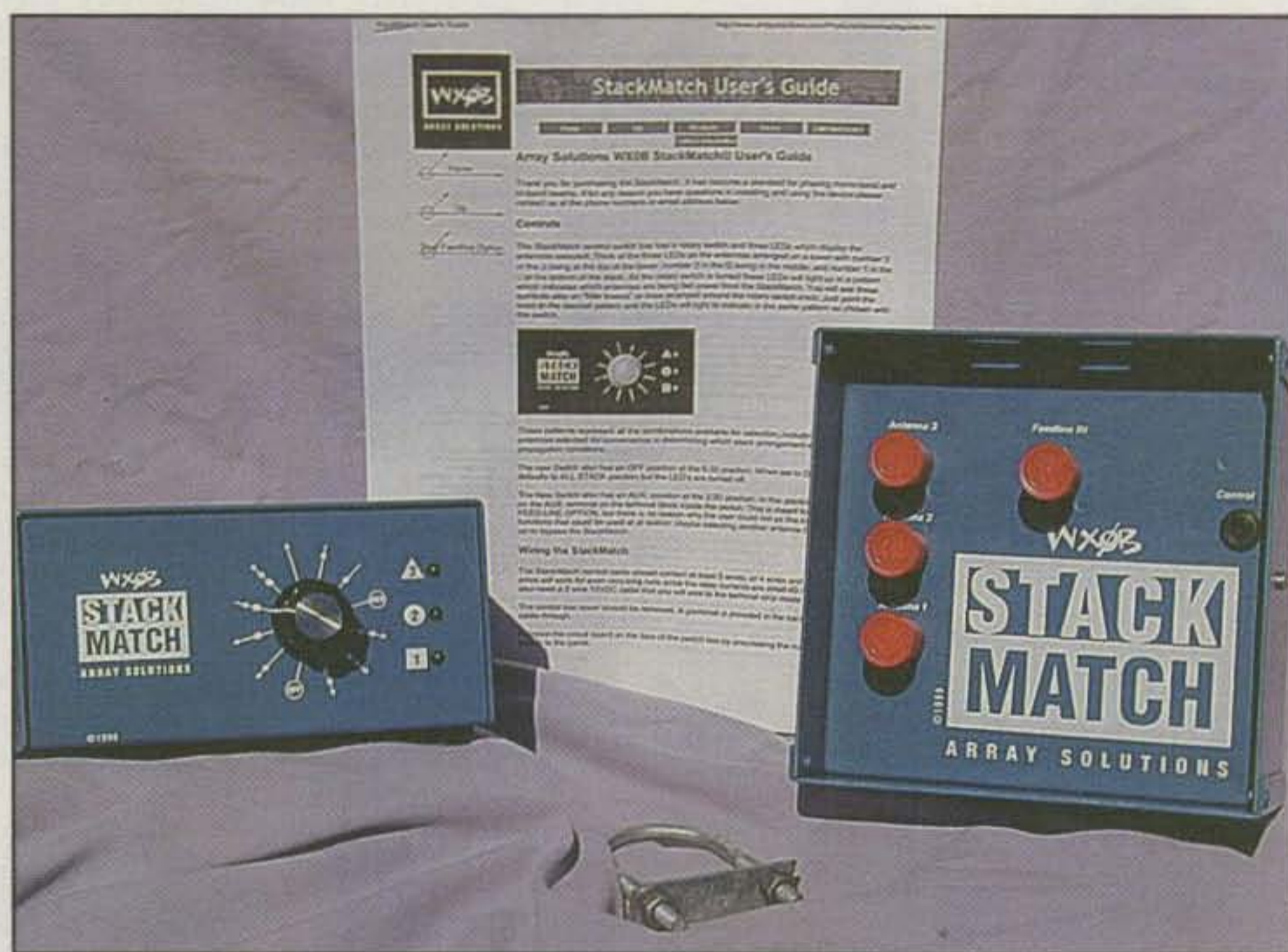
Photo A— The Array Solutions StackMatch includes a control box for inside your shack (left), an excellent manual, and the actual switchbox (right) that is mounted on the tower.
