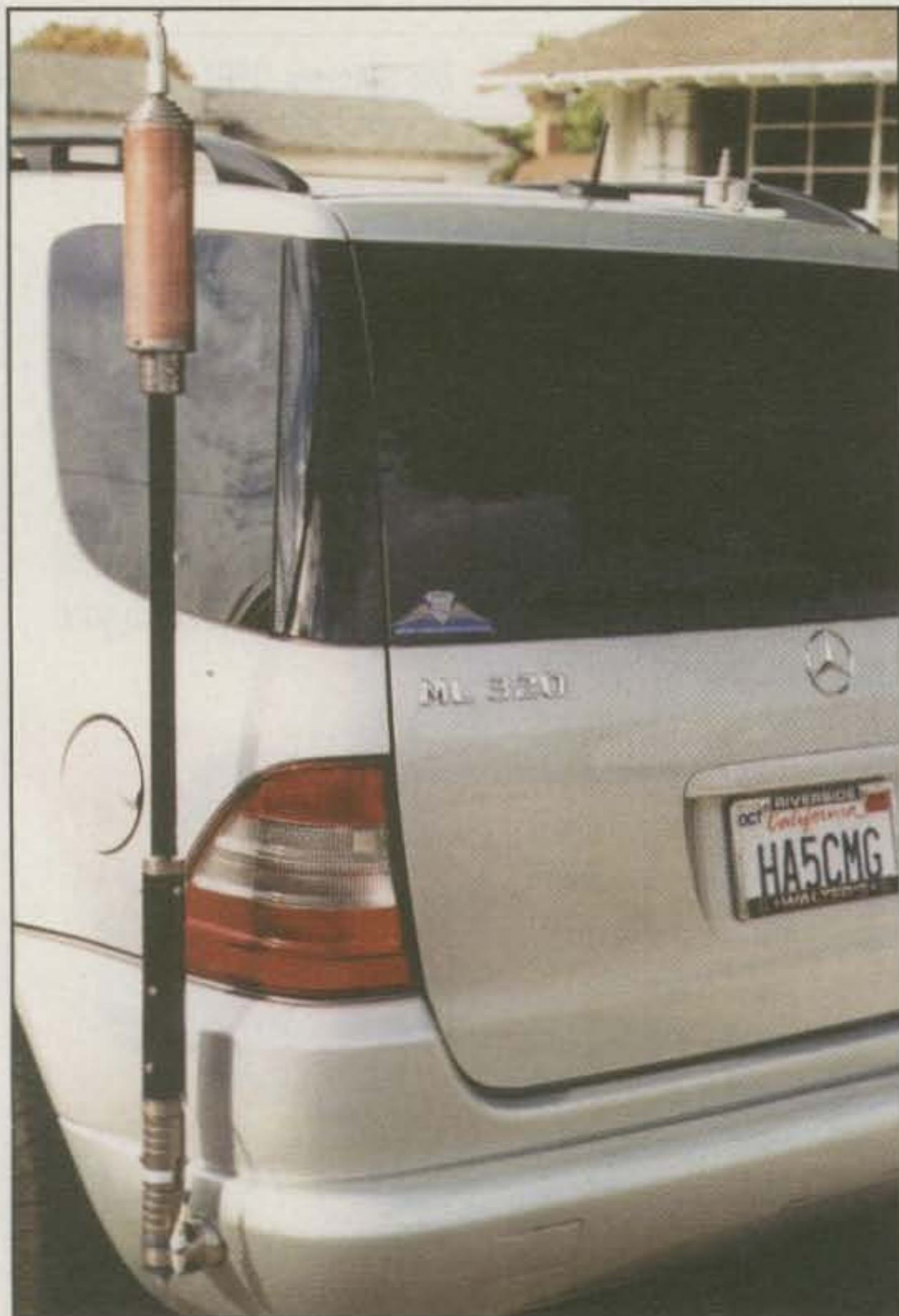
Full-size motorized HF mobile antennas, such as this Hi-Q model, have to be mounted down low, but getting the main radiating sections above the roofline makes a big difference in your signal strength.
