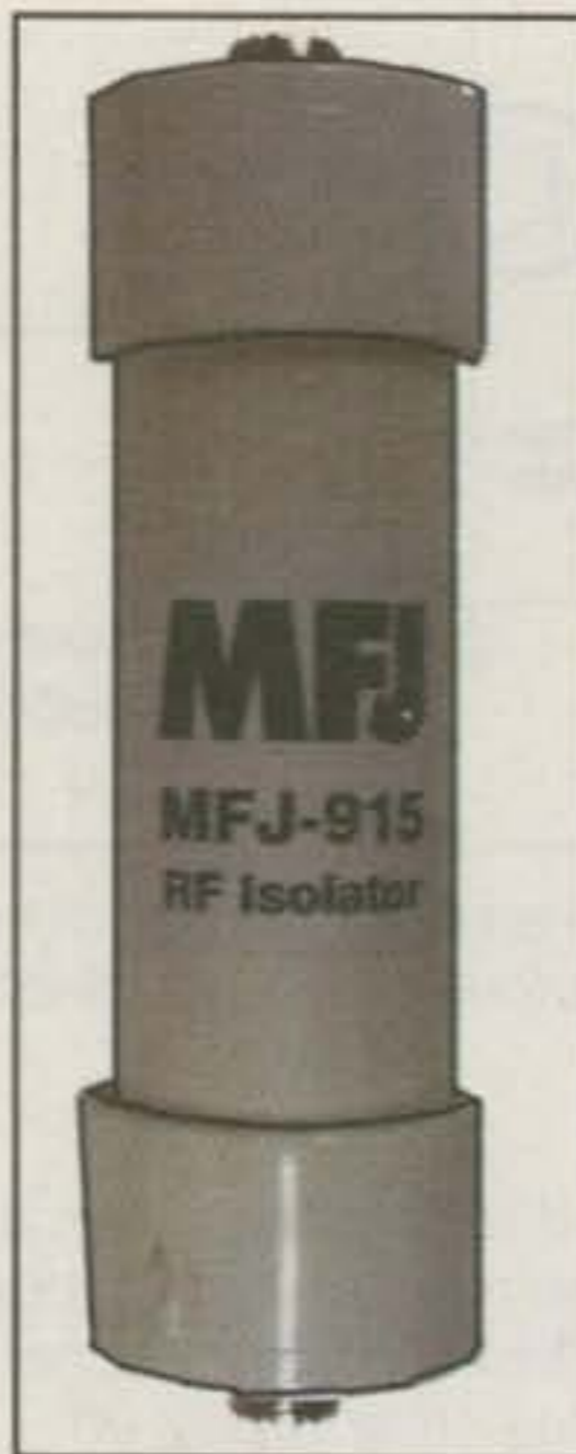
Photo B— The MFJ-915 RF Isolator is a "natural" for use with the G5RV Junior antenna. The RF Isolator is a 1:1 current balun designed to be placed in line with coax, working over the range 1.8 to 30 MHz. It reduces the stray RF often found on coax. (Photo courtesy MFJ Enterprises.)
