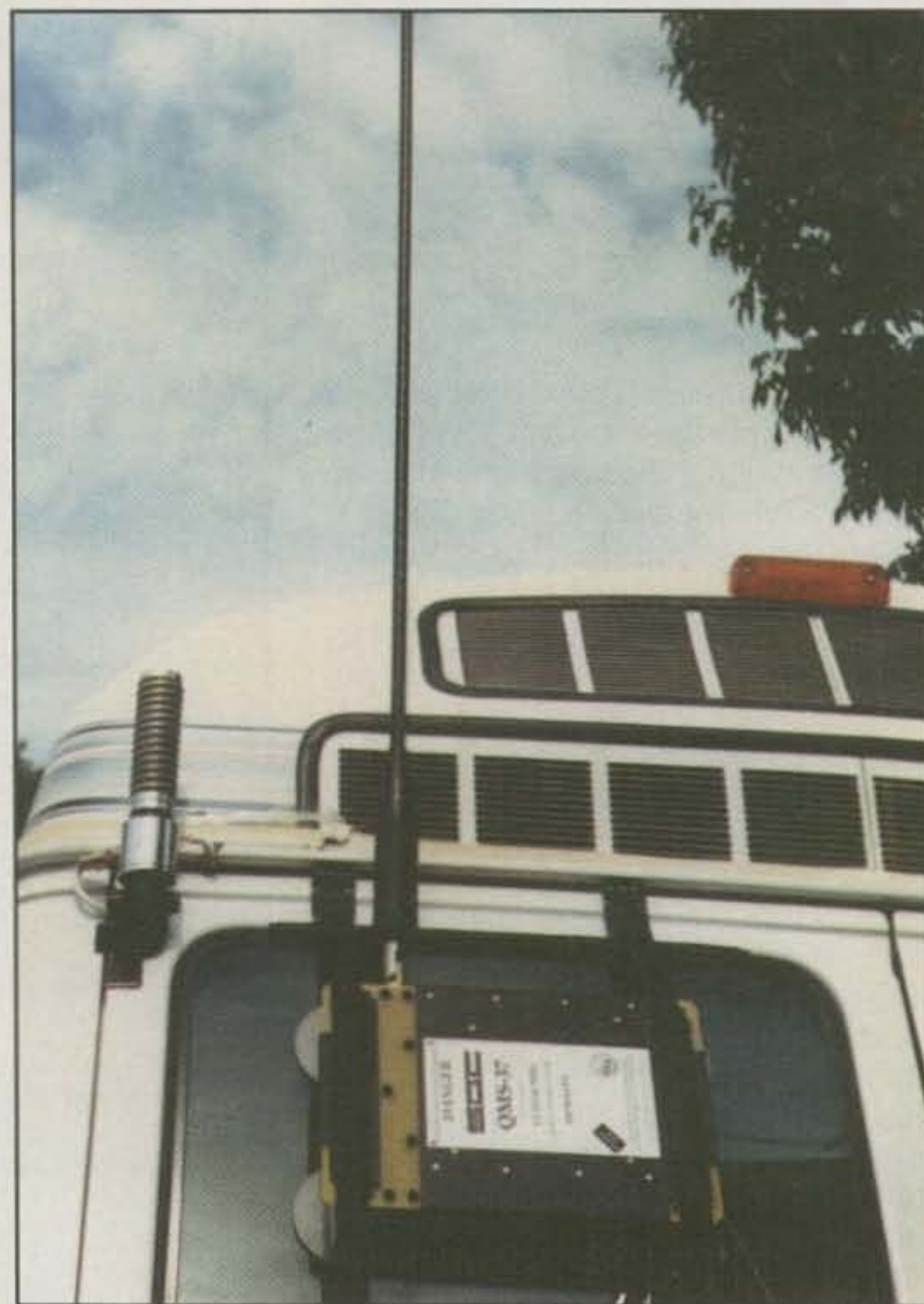
Even when you have a tuner attached directly to the antenna base, as is the case with this SGC system, "the higher the better" is still the rule.
