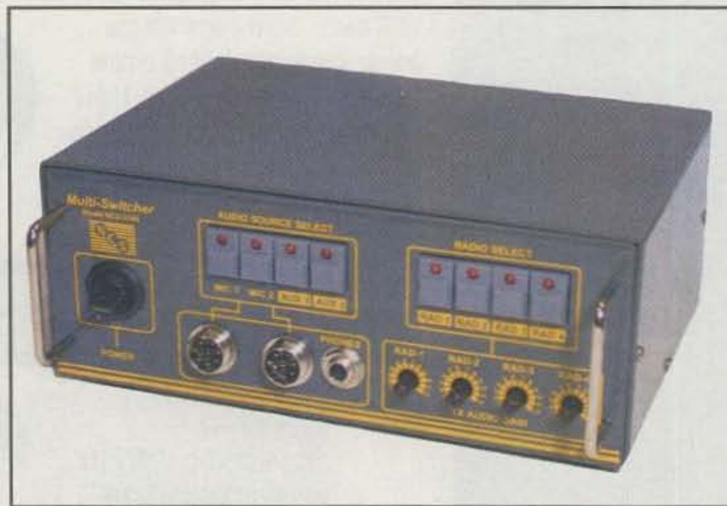
Photo A— You'll find all controls needed for full operation located on the Multi-Switcher's front panel.
