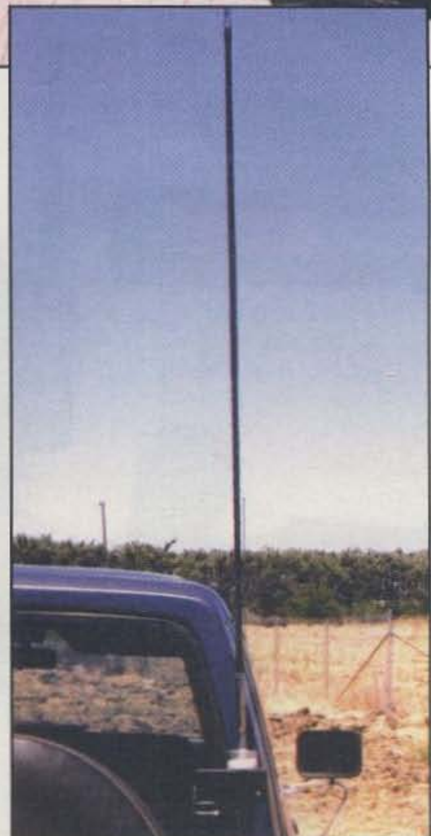
Photo 3—Here the new coil has been added to bring the resonant frequency from 7 down to 5 MHz. Clear vinyl tape keeps it from unwinding.
