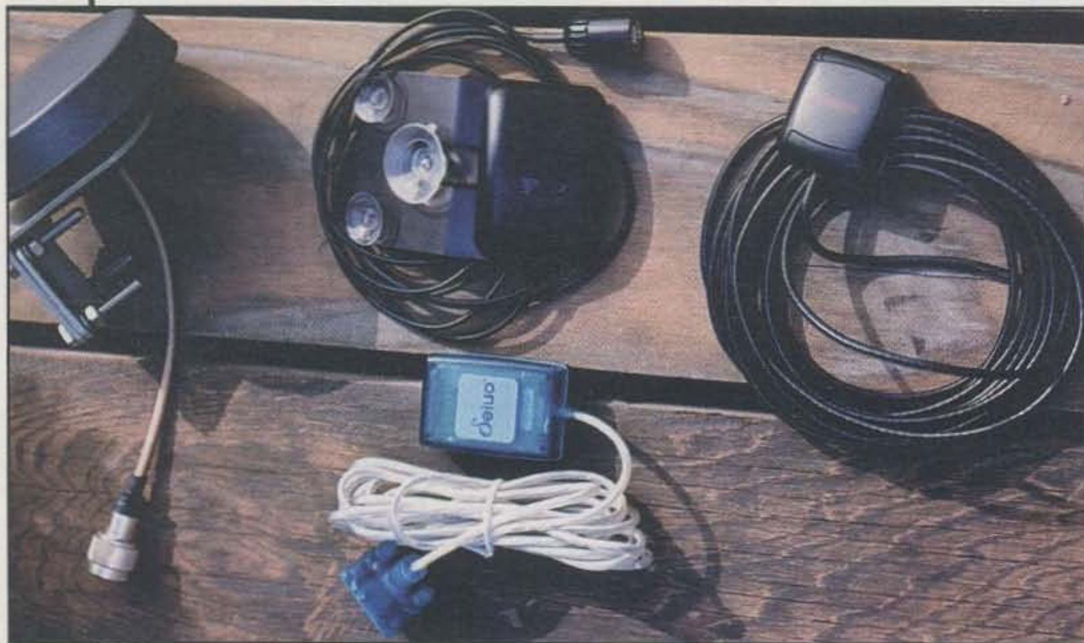
Photo A— A collection of amplified GPS antennas. The GPS module is in the lower center. It is a little magnetic box with integrated antenna and a power/data cable. It looks like a small computer mouse and does not have LCD mapping or data display.
