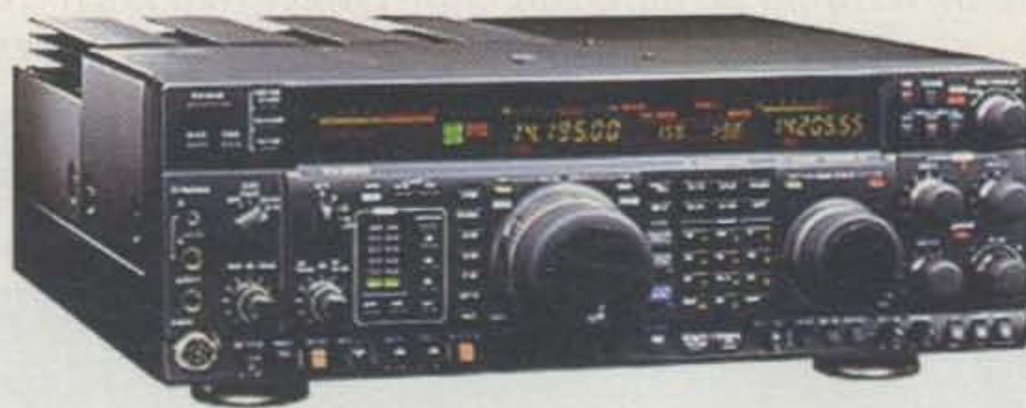
Photo A—Recognizing the superior quality of class A amplification, Yaesu includes direct front-panel selection between class B and class A operation in its popular FT-1000MP Mark V transceiver. The owner thus has a choice of high output power or an exceptionally good-sounding SSB signal, as desired.
