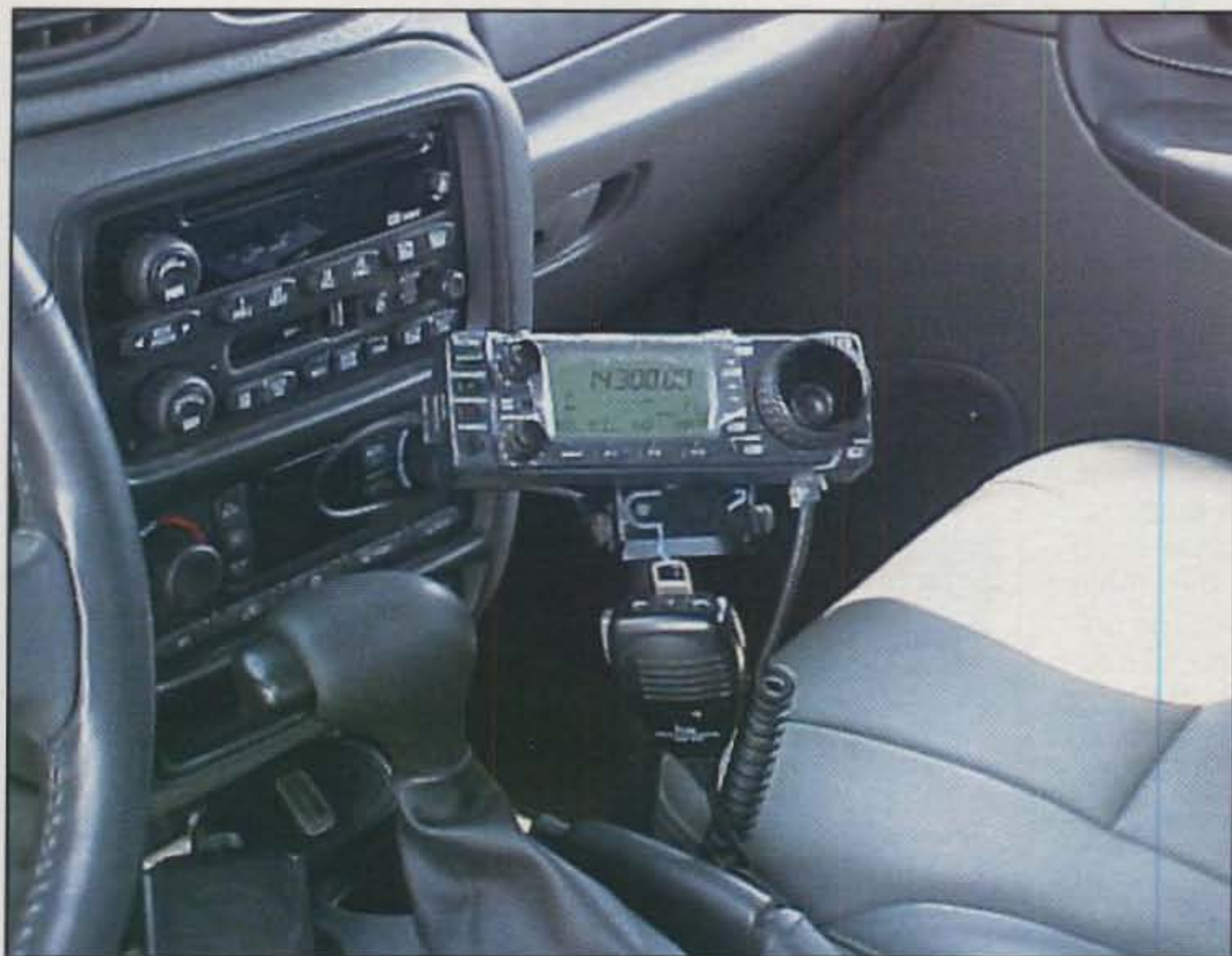
Here's KE2LJ's remote-mount setup for the popular IC-706. It's a very clean installation that's convenient for the operator. (KE2LJ photo)
