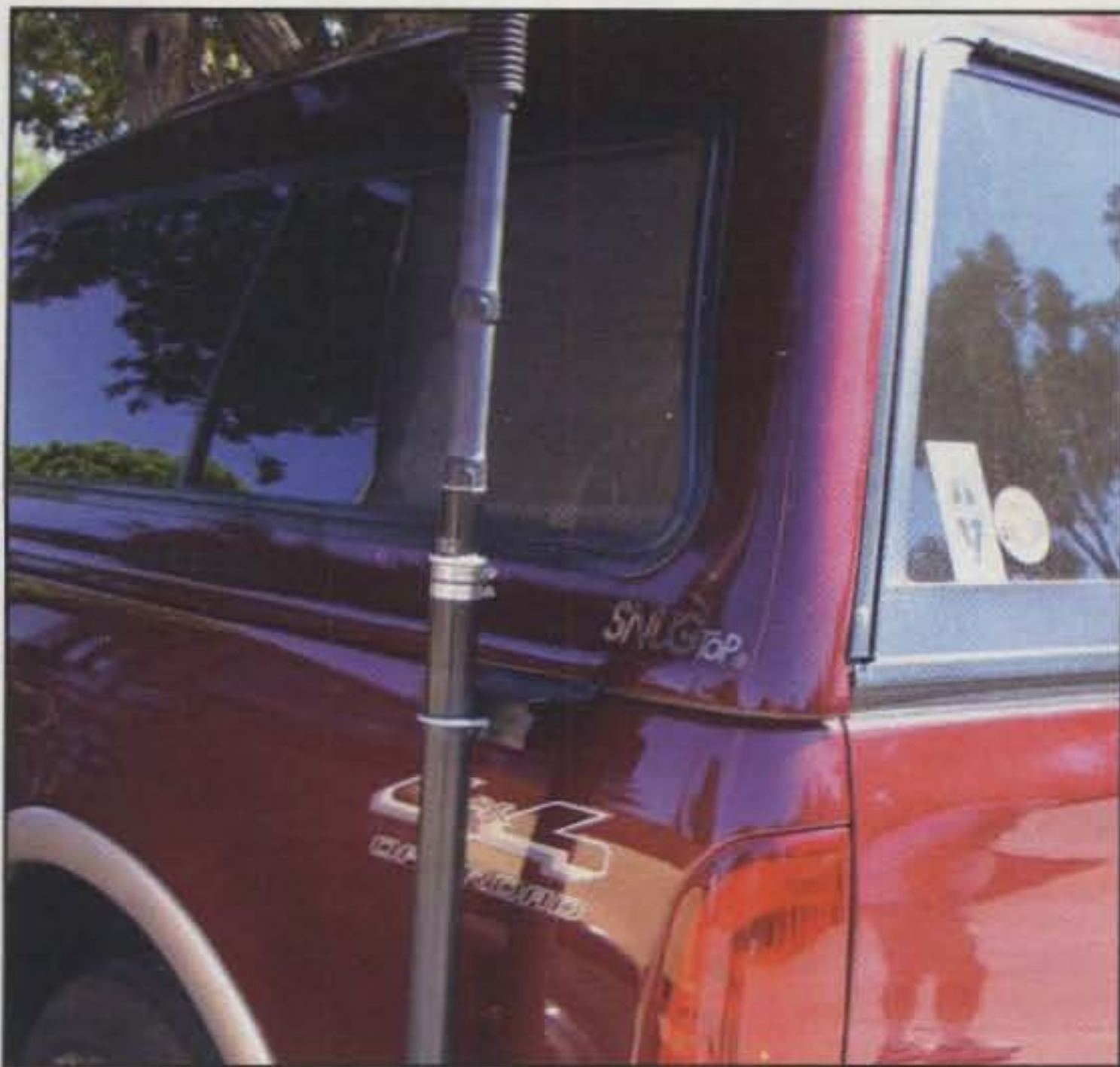
Larger antennas or heavy "screwdriver" tuners need a sturdy support. This well-designed mount for a Ford F-150 pickup appears to be strong without drilling visible holes in the truck body. (Photos by AA6JR)
