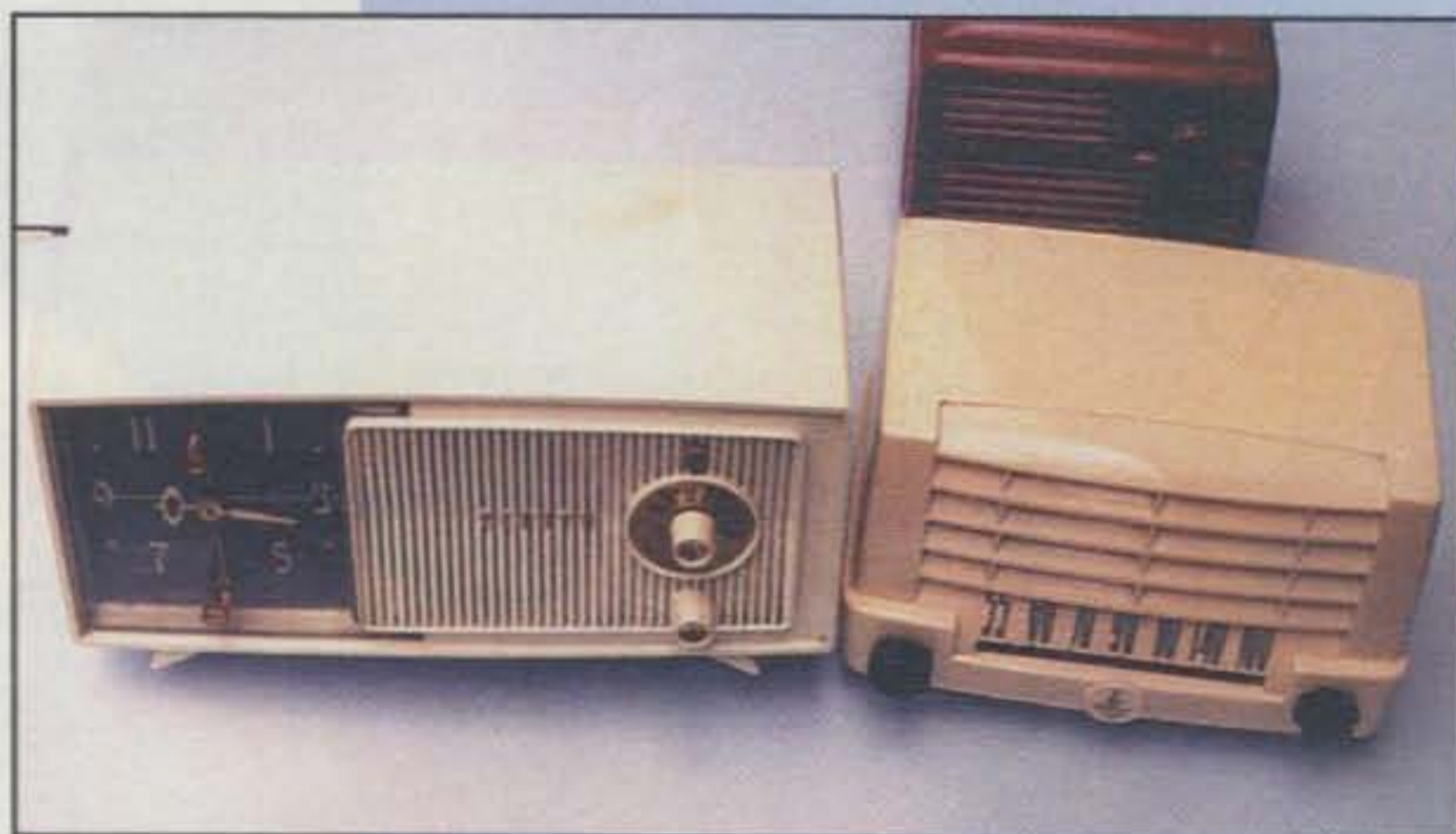
Photo A— Approximately one out of three table-model AM radios from the 1950s and '60s is a good candidate for conversion into a mini-transceiver. Here it is the rescued-from-trash-pile Emerson on the right. Why? It is small, a common style, and has a (reusable) metal chassis. The Zenith on the left is an early clock radio with a difficult-to-modify PC board, and the little red Arvin in rear has a unique reverse-reading dial—a neat collectible.
