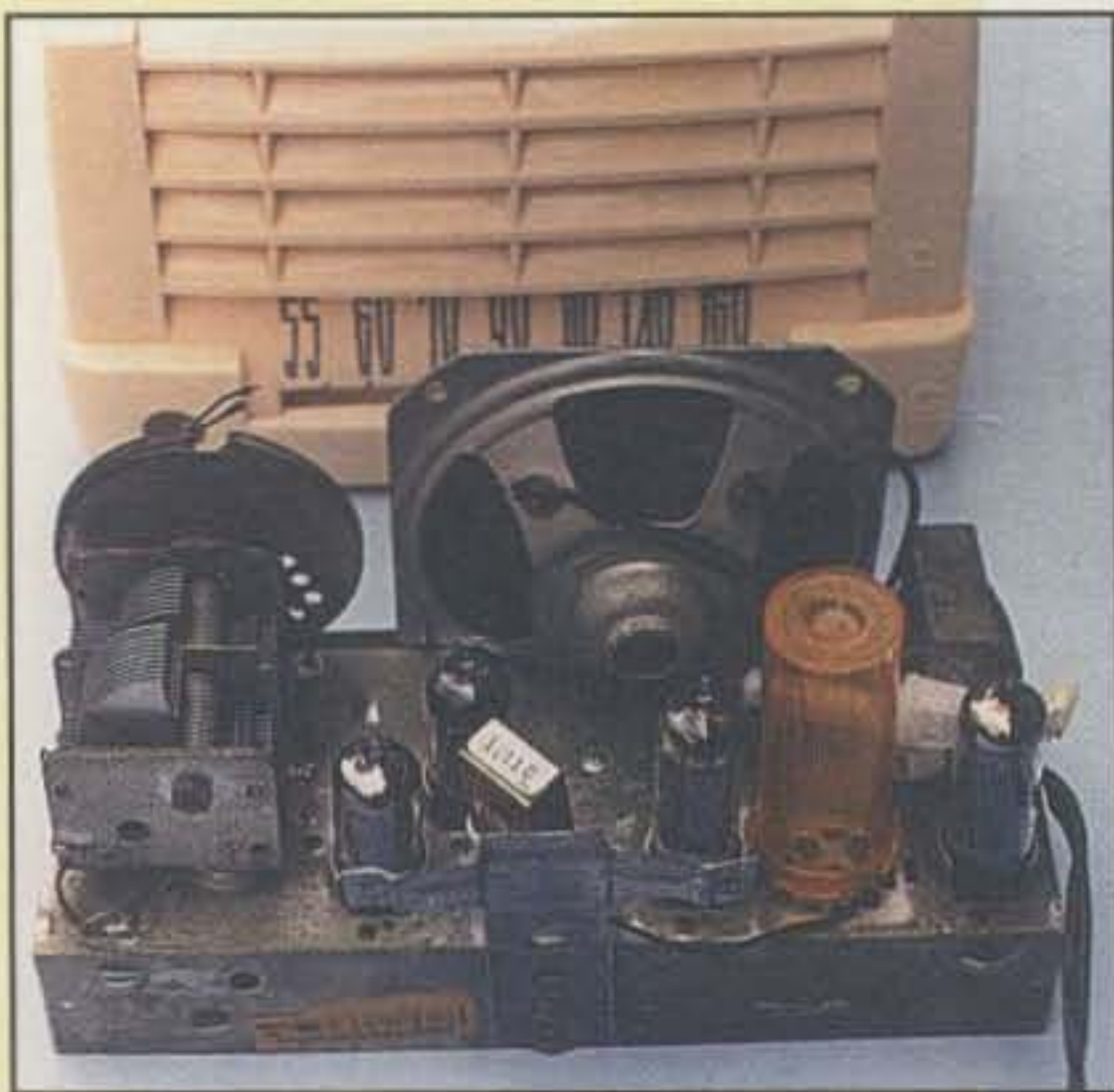
Photo D— Interior view of my rescued-from-extinction Emerson midway through conversion. A crystal socket is mounted in the space of one removed IF can; a pill-bottle coil form is mounted in place of the other IF can. The two 50C5 tubes are mounted near the rear of the chassis for maximum cooling.
