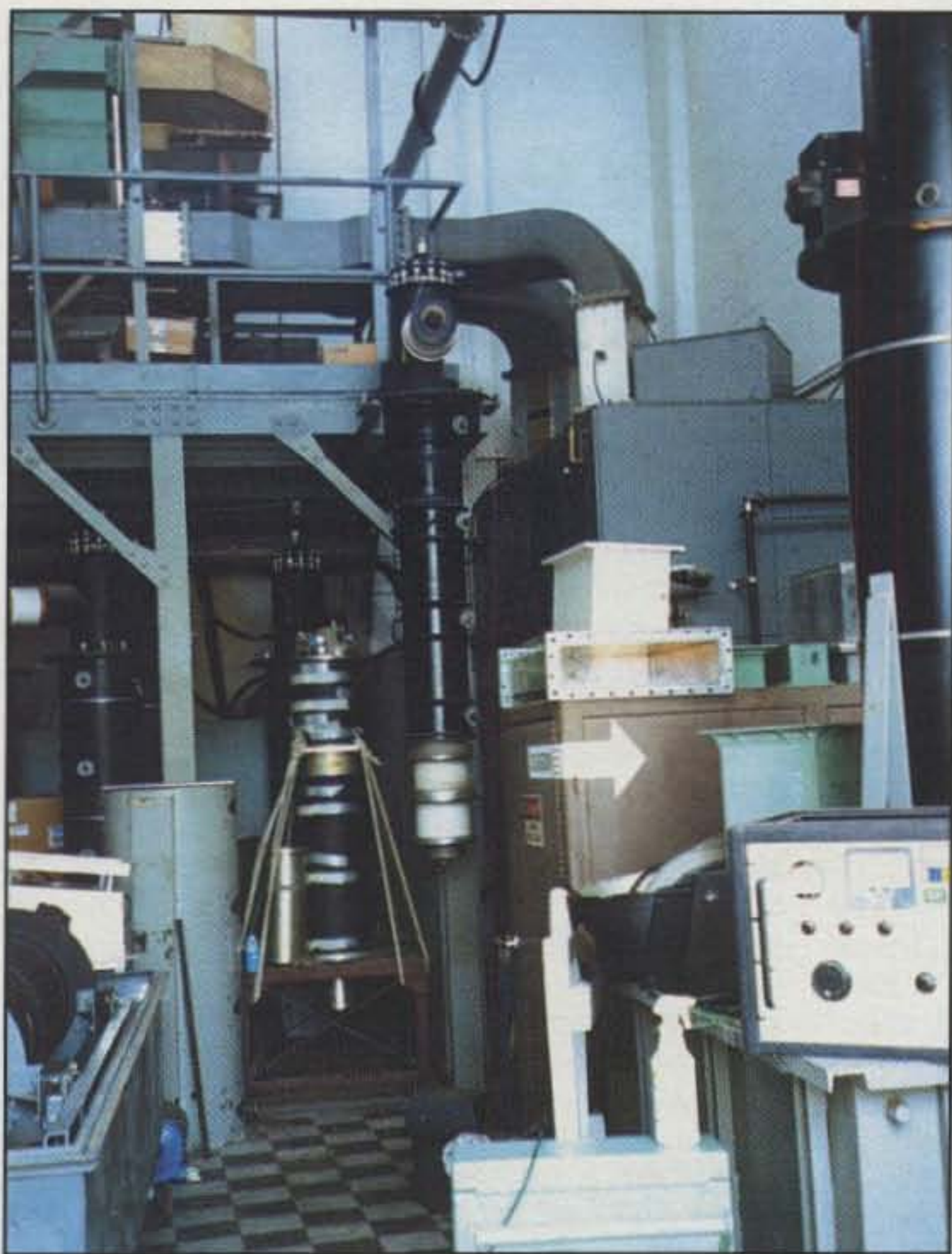
Photo 3— For atmospheric studies a 2.5 megawatt pulsed transmitter is used. This is what some spare 1 and 2.5 megawatt finals look like.
