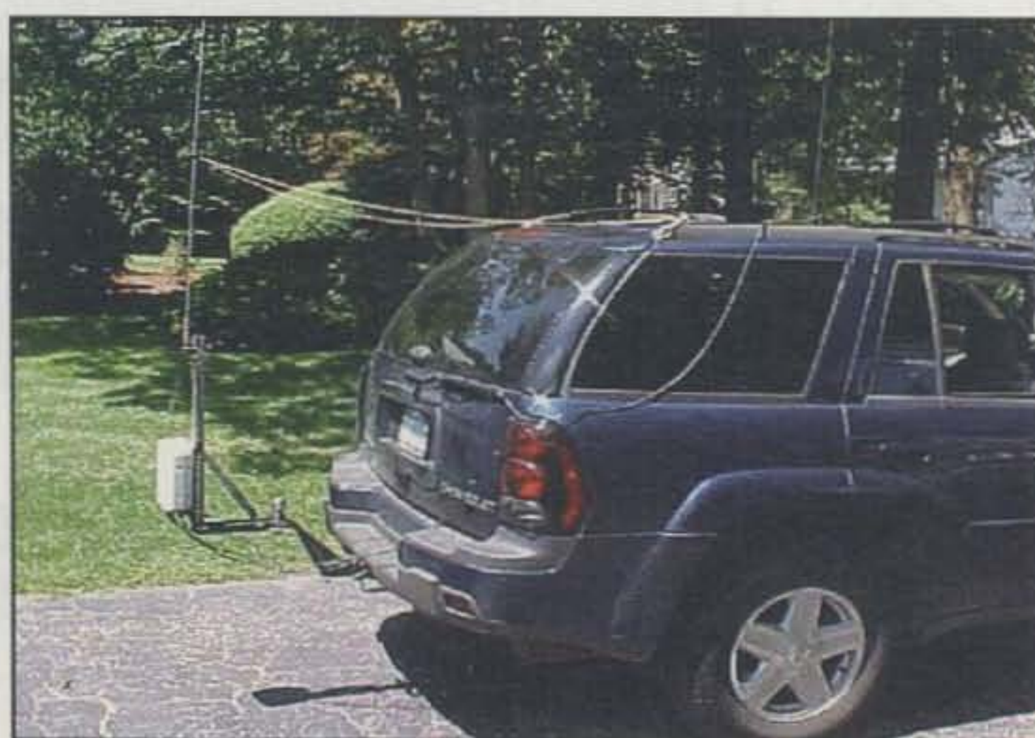
Here are ways to mount the ICOM AH-4 (or other) antenna coupler close to the antenna without drilling holes to mount the tuner in the vehicle. (KE2LJ photos)
