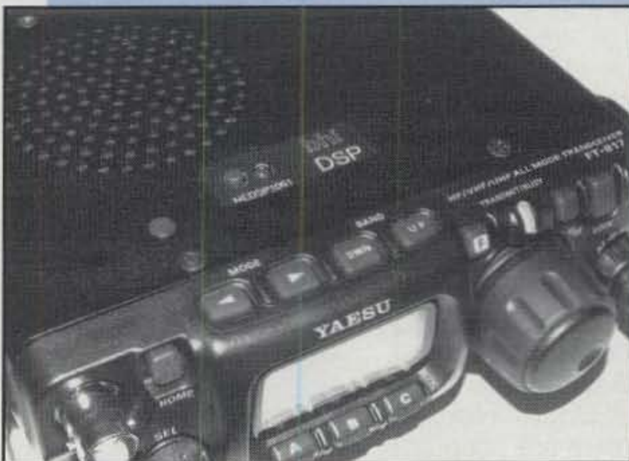
Photo B— W4RT Electronics is now installing "One Button DSP" in Yaesu's FT-817 portable transceiver, and it is hot! The unit features four levels of noise and carrier reduction that are selected by a new top-mounted pushbutton and confirmed by an LED on a small top-mounted panel. (Photo courtesy W4RT Electronics)
