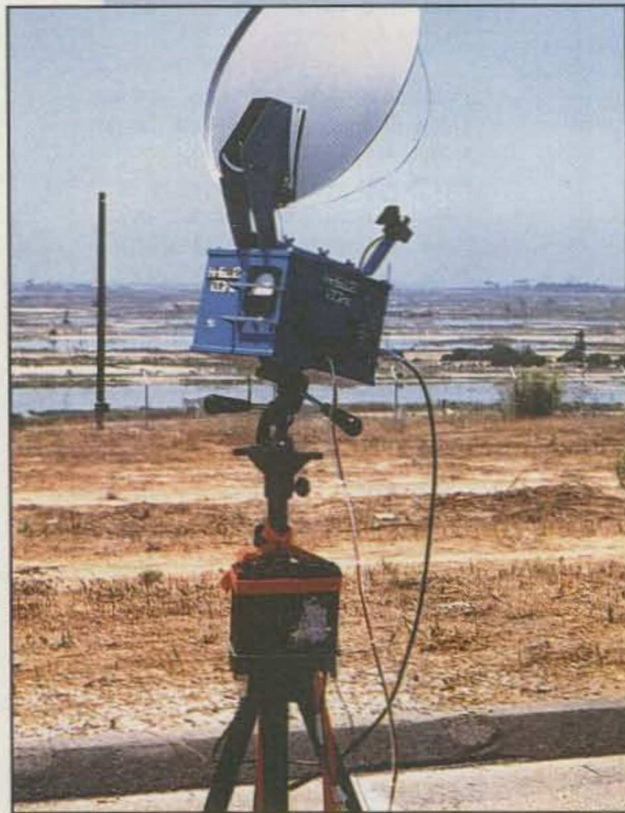
The KH6WZ 10 GHz rig looks pretty, but it didn't put out much power. A simple resistor was the downfall of the rig. "Morpheus" is being re-built yet again.
