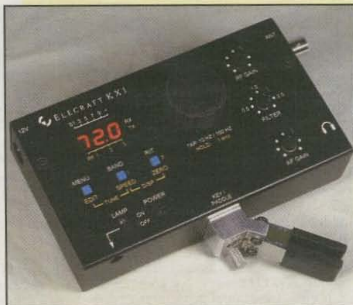
Photo 1— Nothing makes the holidays more exciting than a new transceiver, especially when it is small and affordable, like this just-announced Elecraft KX-1. The little delight sports unique design with top-mounted controls, features galore, and up to 4 watts output on 20, 40, and 30 meters.
