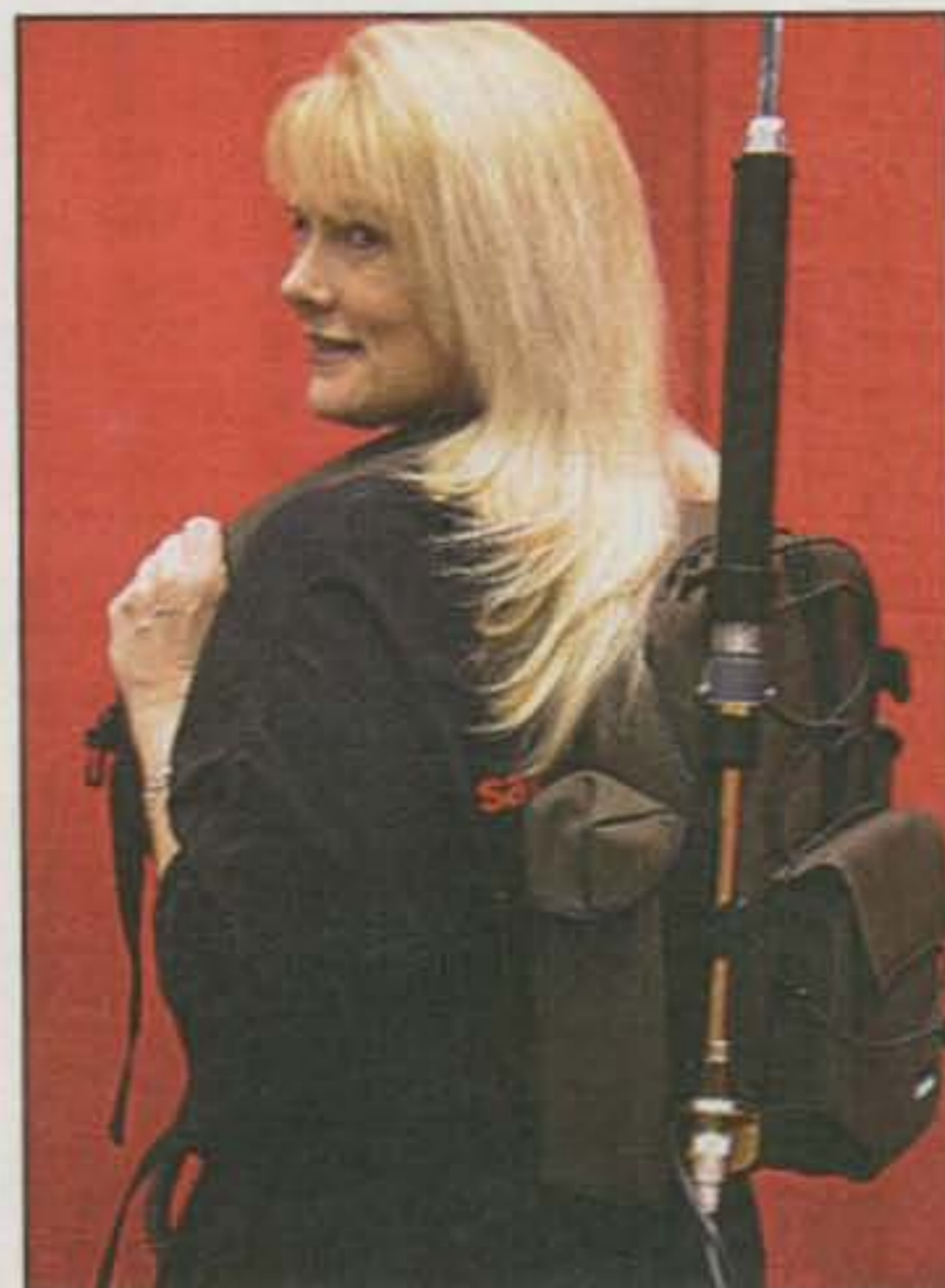
Photo 3— Rhonda Comer, KG4FVL, shows us the concept of operating pedestrian mobile with the IC-703. The rig is enclosed in its optional LC-156 backpack, fitted with a W6MMA multi-band MP-1 mini-antenna, and mated with a Heil "Traveler" headset with boom mic.
