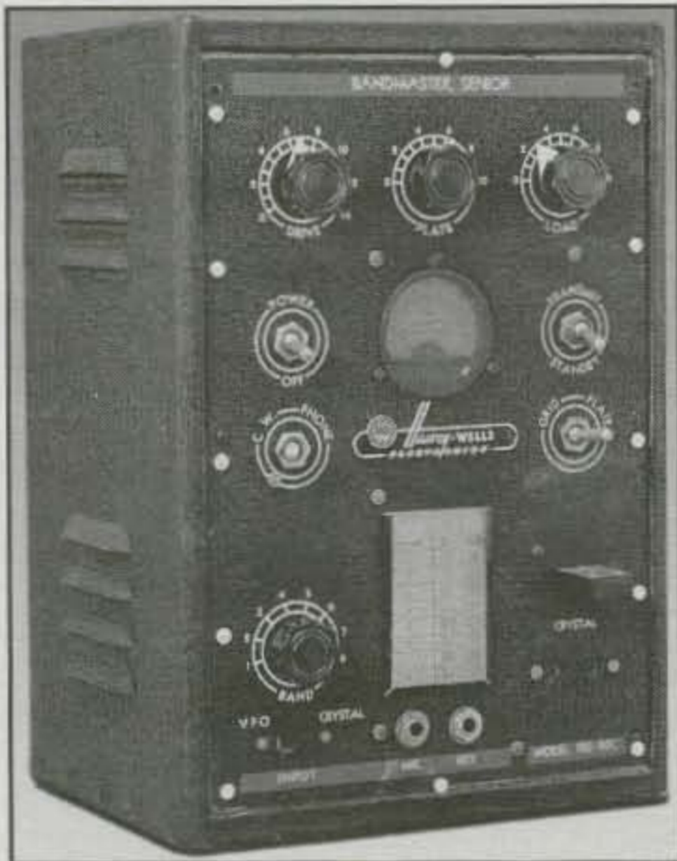
Photo 4— A favorite joke about the Harvey Wells Bandmaster was that the name was appropriate since harmonic suppression wasn't that great and it often seemed to transmit on all bands at once!
