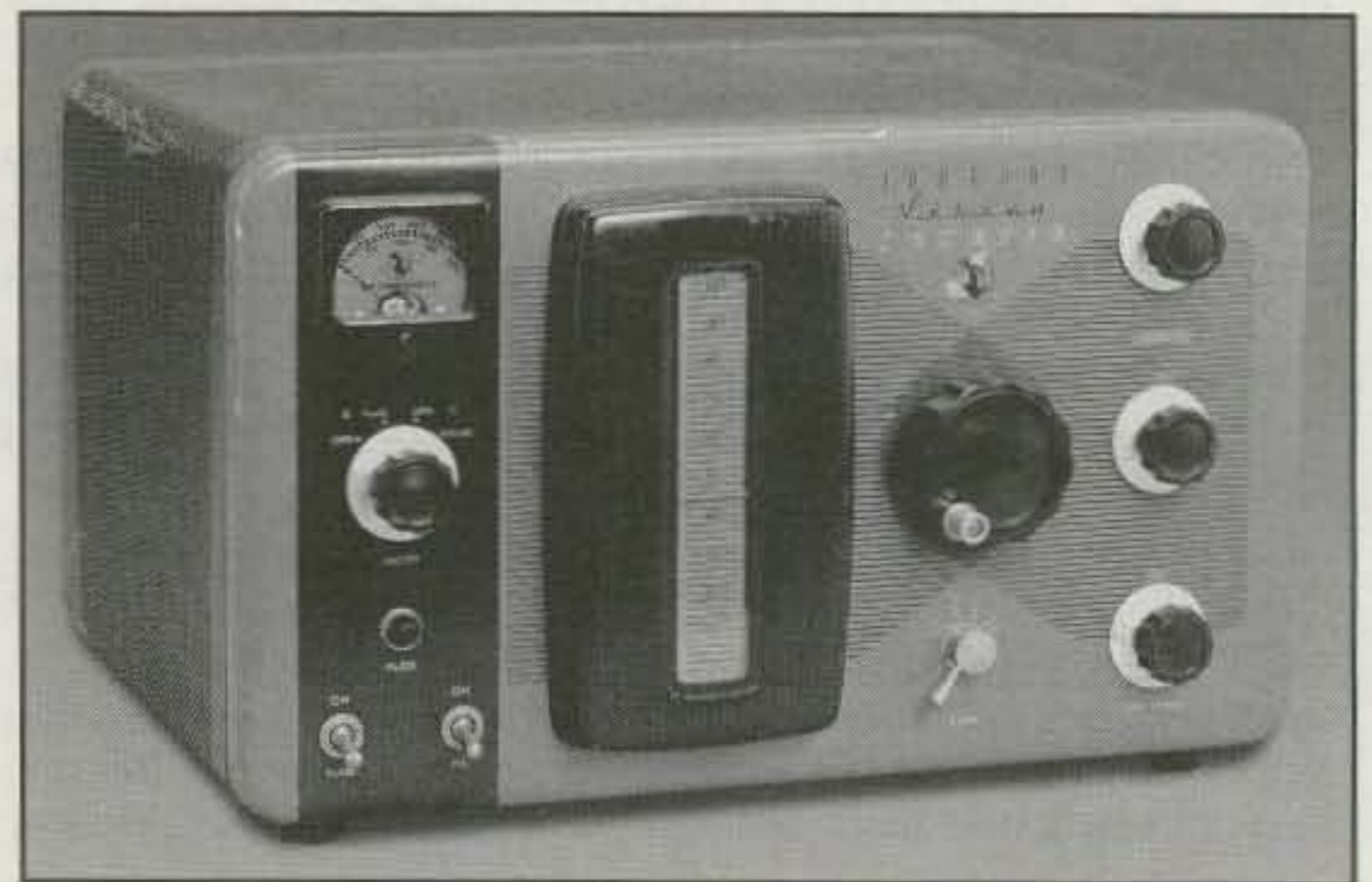
Photo 3—Courier was the name E.F. Johnson gave to its medium-power (300 watt) amplifier. If you wanted a full kilowatt, you had to go with the Thunderbolt, or maybe the Viking Desk Kilowatt.
