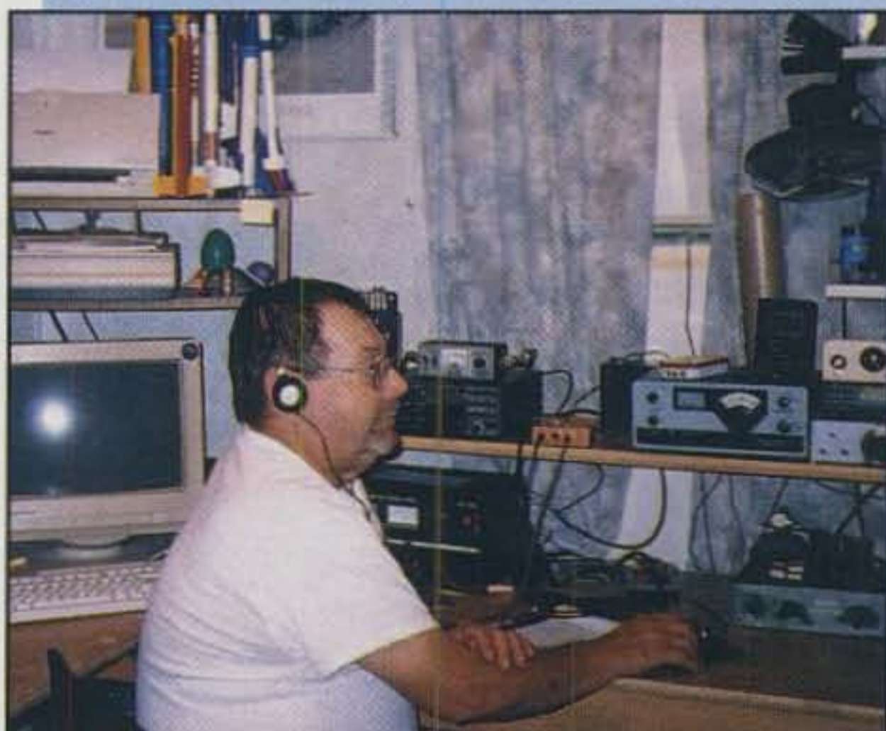
Photo A— Jerry Felts, NR5A, with his total QRP setup. Gear consists of an Elecraft K2 and Heathkit HW-8 plus NorCal 40 (top shelf) and a like-new Ameco 6V6 transmitter for nostalgic fun (on desk). The little 500 milliwatt Rock Mite used for our QSO is mounted in a homebrew PC-board case sitting between the K2 and HW-8.
