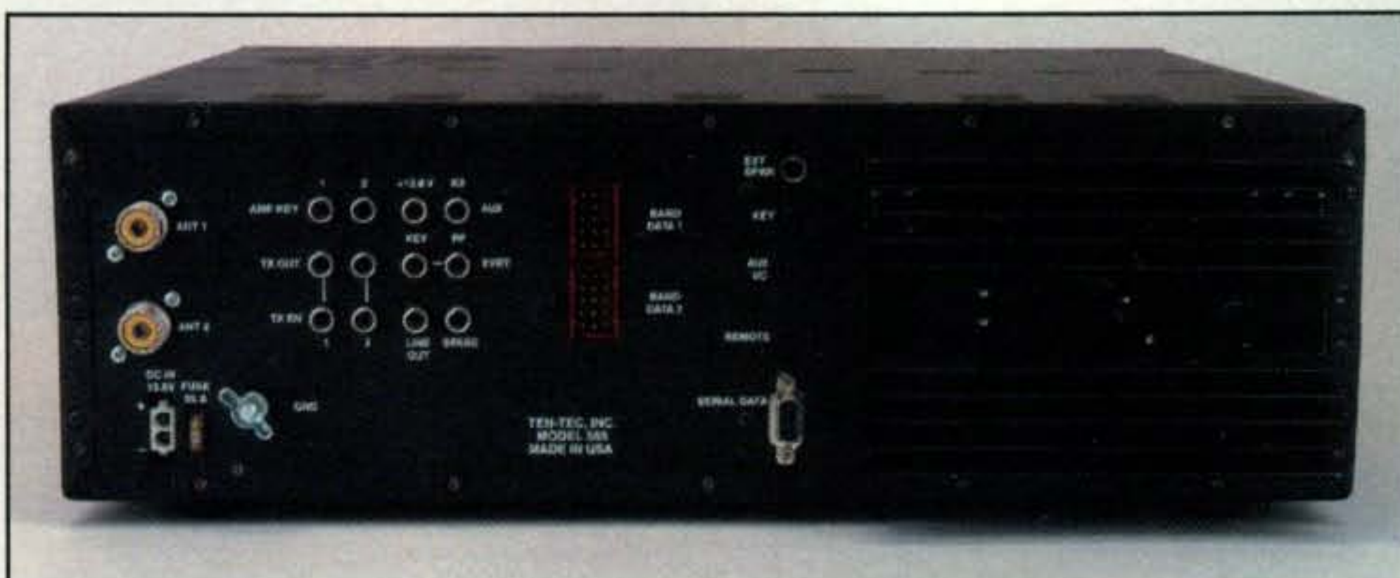
Rear view of the Orion. Note the dual output connectors, which allow users to not only switch antennas but also certain operating parameters with the push of a button on the front panel. (Ten-Tec photo)
