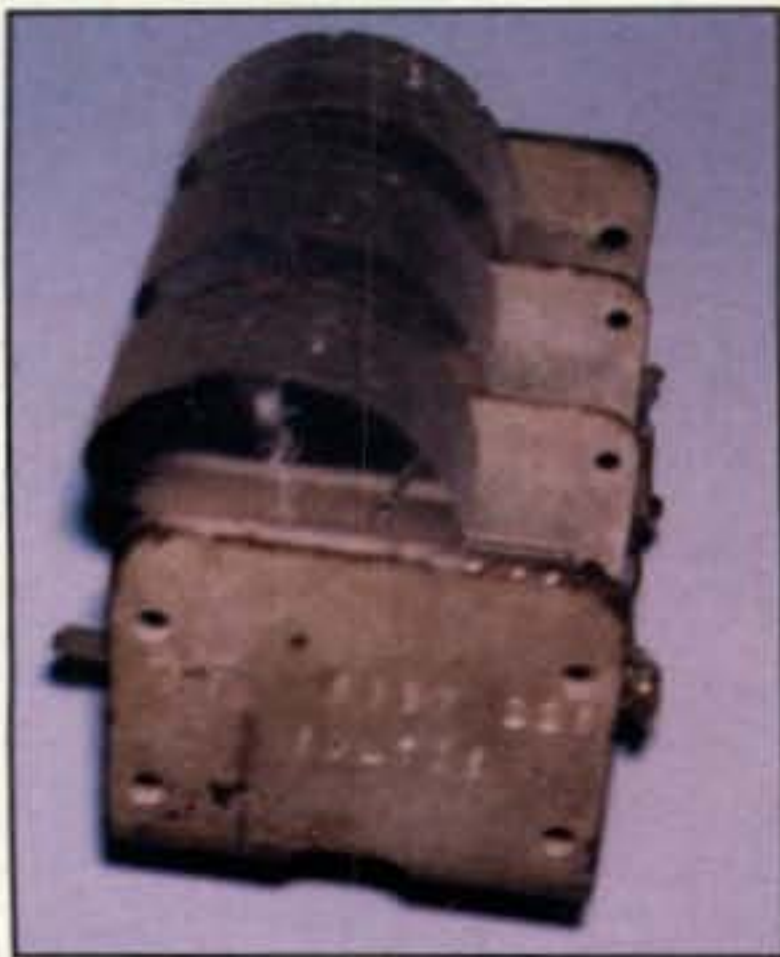
Photo B— Have you ever noticed how the rear rotor plates on some tuning capacitors are slotted? It permits slight bending in or out of various areas on the plate so tuning coincides with dial calibration marks.
