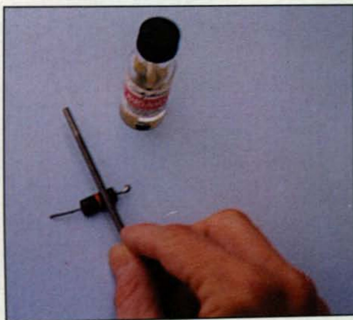
Photo A— Need a specific-value resistor not available in your junkbox? File one to fit using the simple procedure described in the text.
