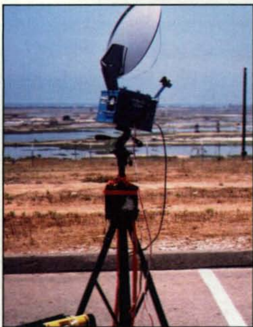
Photo A— Blue Morpheus looked really neat, but the enclosed chassis box restricted access to fix and modify the system, and there were many repairs and modifications needed. This was the "successful failure" rig mentioned in the December column.
