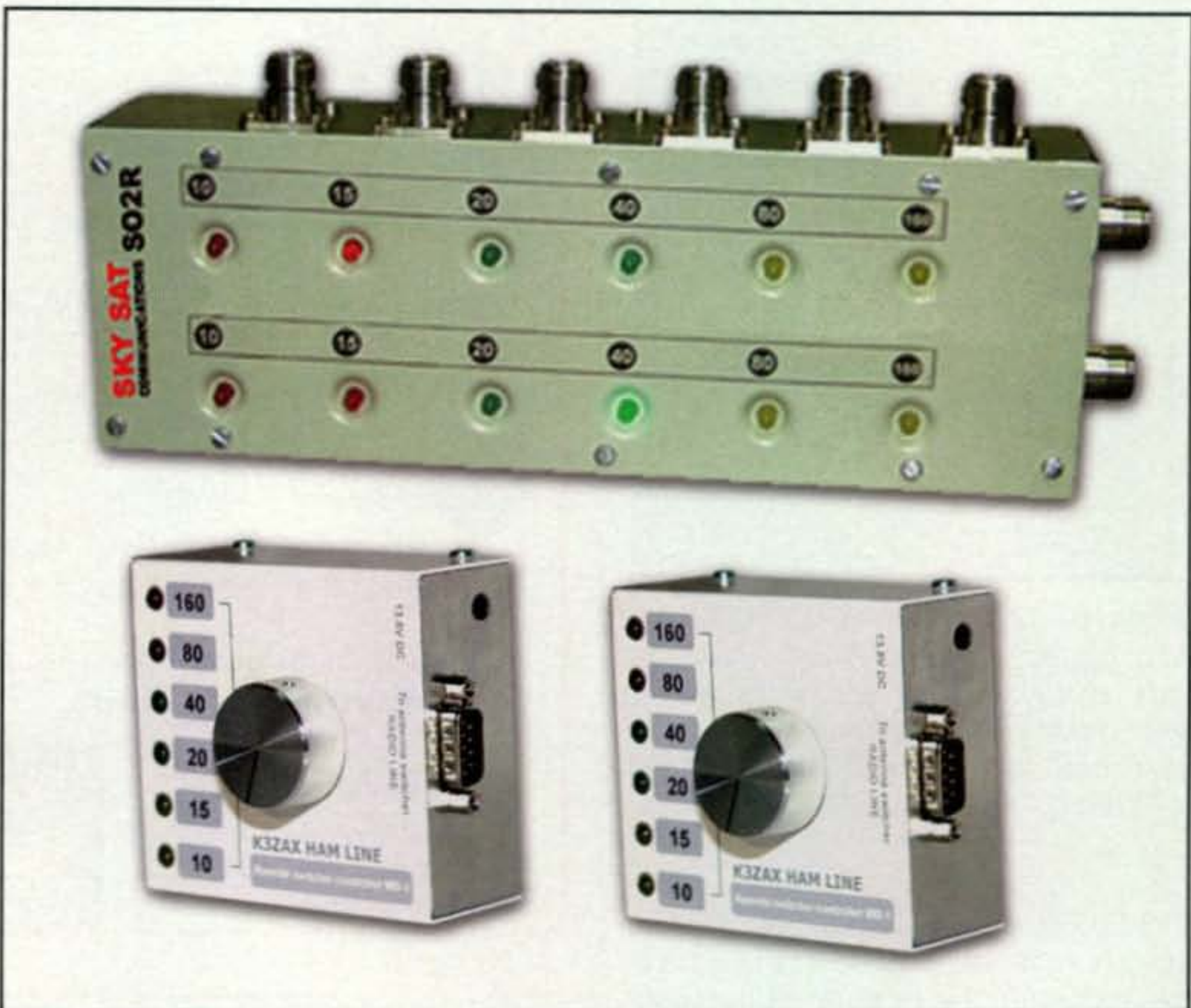
Photo C— The SO2R Antenna Switch with two MB-1 Controllers. The antenna switch has six inputs and two outputs or reverse; the unit can fully automate switching for a single operator and two transceivers. The prices noted in the column for the Remotely Controlled Antenna Switcher include the switcher itself and two controllers. A control cable is sold separately. (Photo courtesy Jovan Peric, KB9K)
