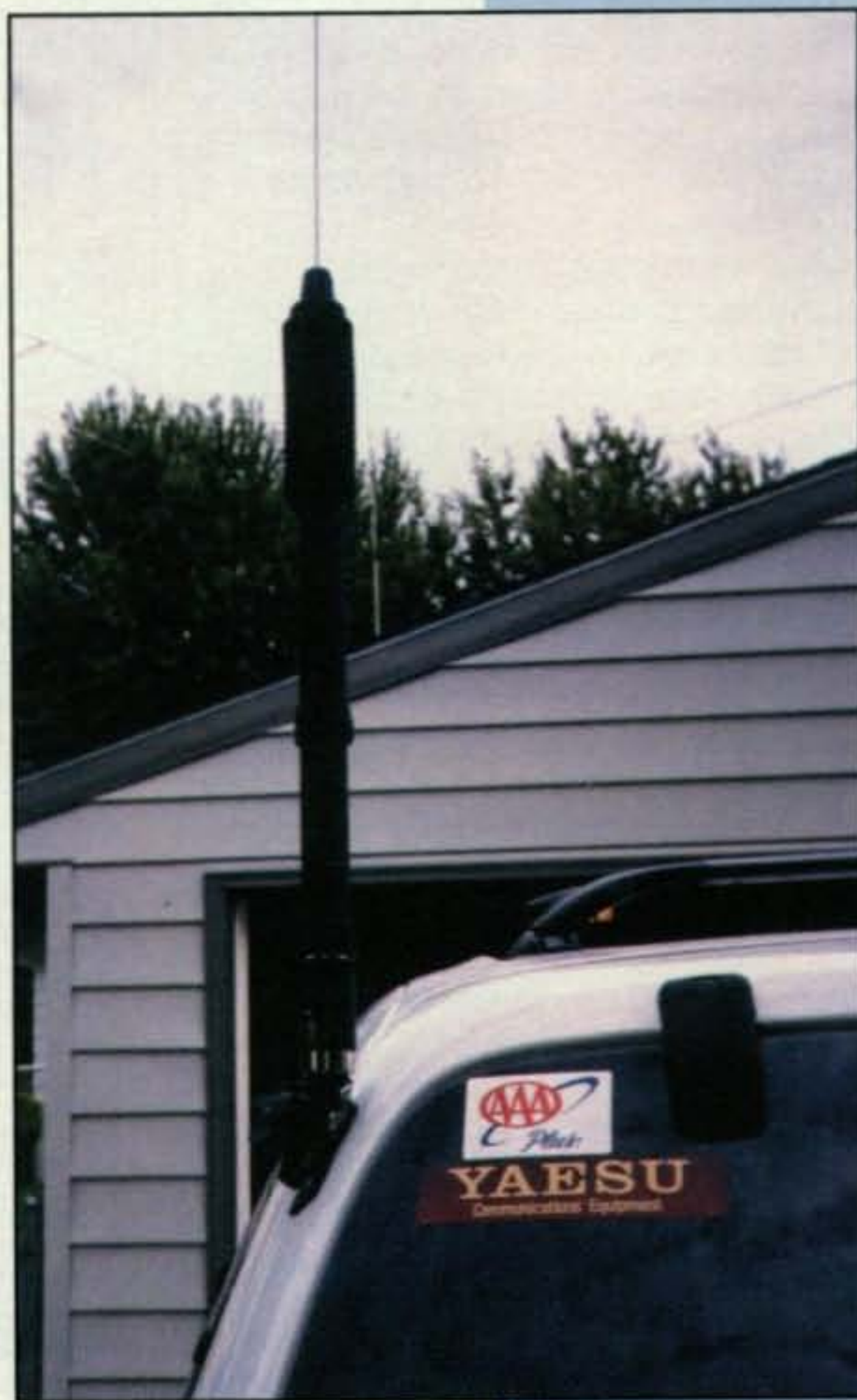
Photo 1—WØROB's motorized Yaesu ATAS-100. (WØROB photo)
