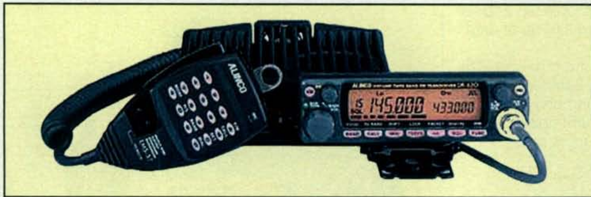
Alinco's new DR-620T dual-bander features more memories than previous models, plus alphanumeric and DCS along with CTCSS tones.
