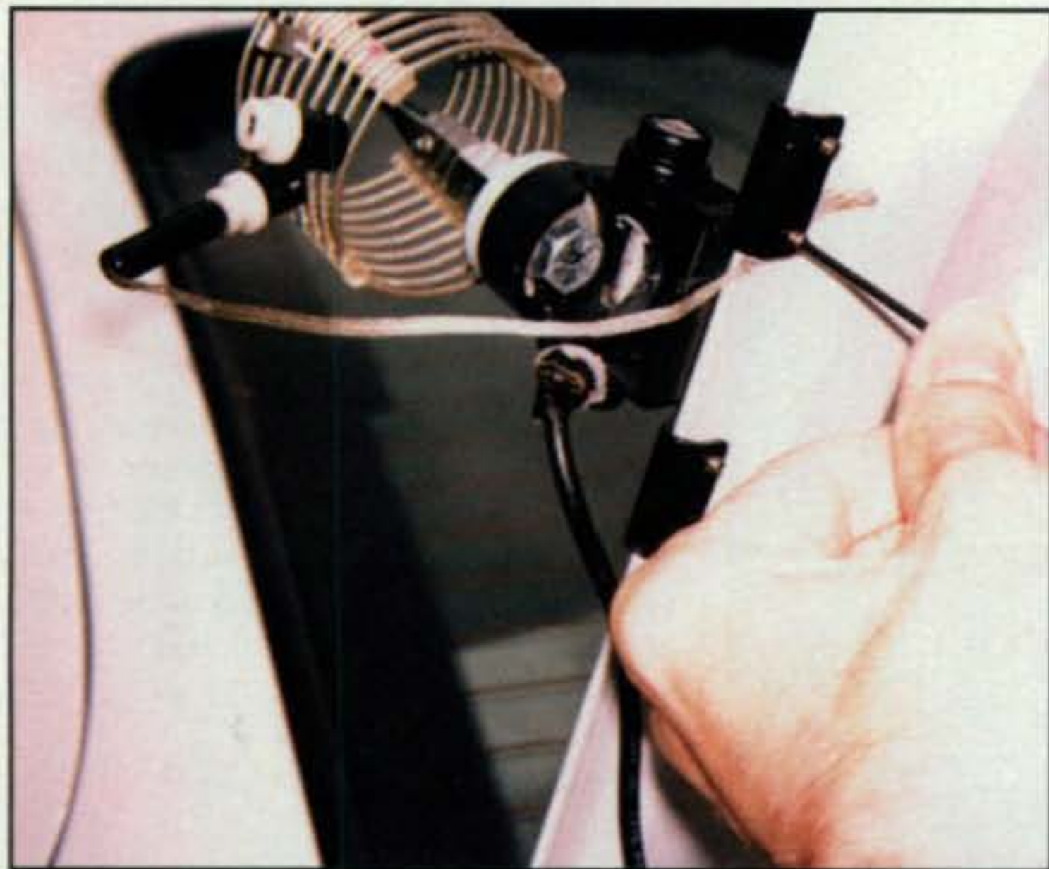
Photo 7— The main key to successful QRP mobiling is using the vehicle's metal frame as a solid ground. Here we scraped off 1/4 inch of paint so one of the mount's screws connects to ground. We then added a base matching coil and connected its ground strap to the mount's screws. A VOM check confirmed solid grounding.
