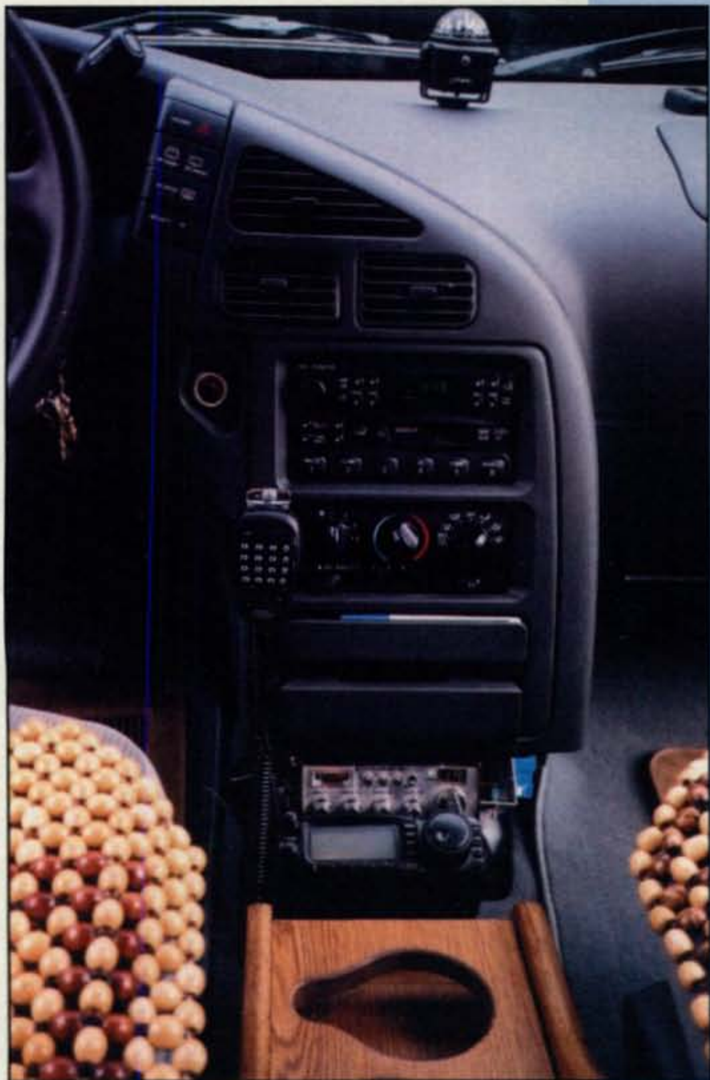
Photo 2— WØROB's FT-100 is nicely positioned clear of the airbag deployment zone and at the operator's fingertips. (WØROB photo)
