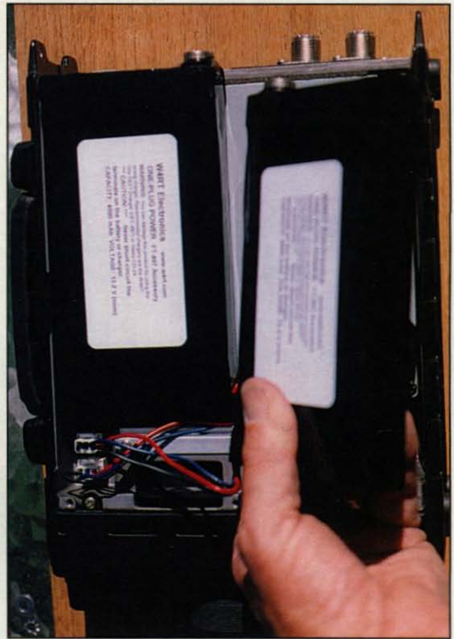
Two internal battery packs (4.5 amp/hours each) provide up to 9 amp/hours of portable operation for the Yaesu FT-897. They can be charged without being removed from inside the radio.
