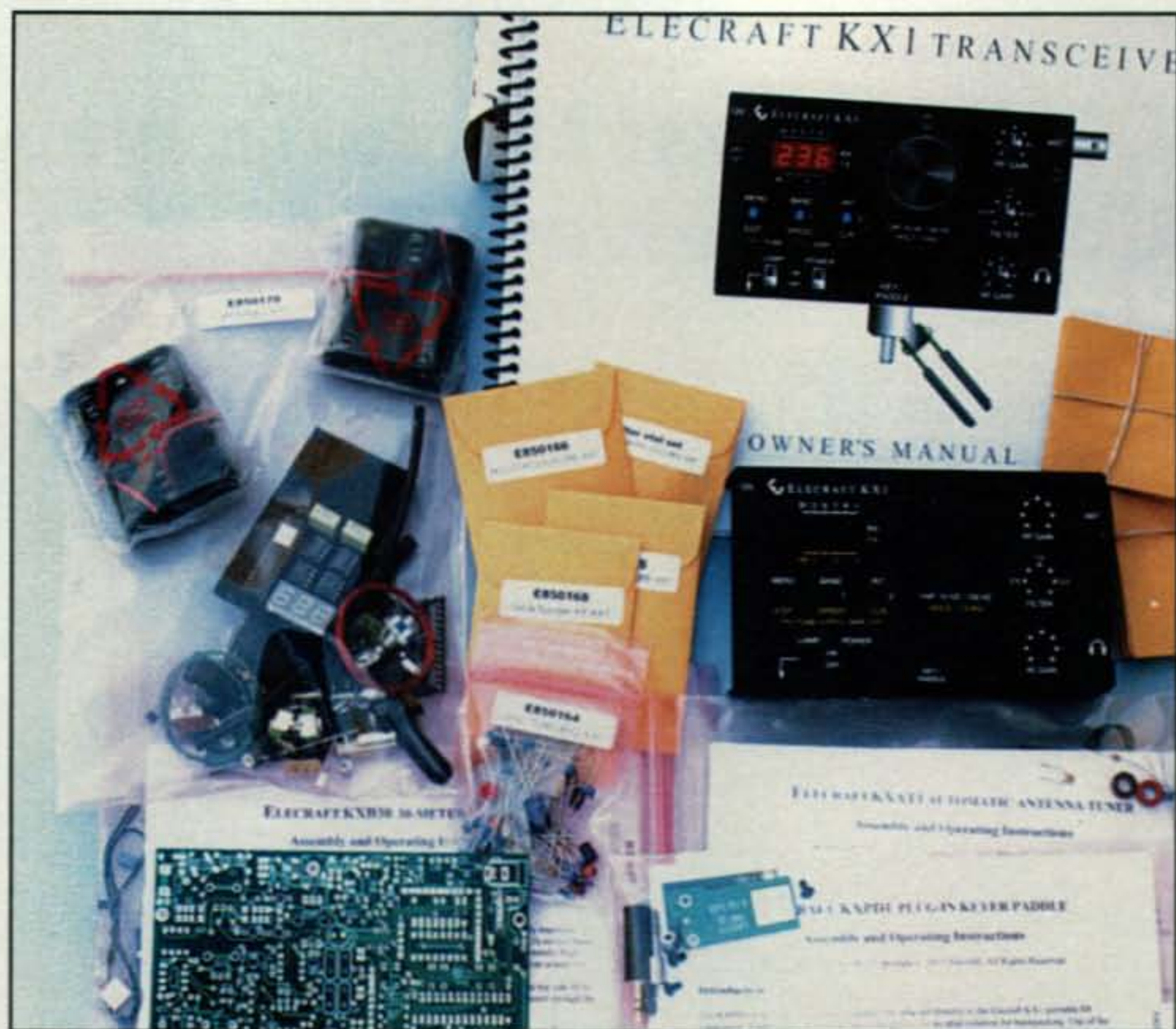
Photo 2— The full Elecraft KX1 kit as received, unpacked, and ready for assembly. Various components such as resistors, capacitors, and inductors are packaged in separate envelopes, while larger items such as transistors and ICs are in static-safe bags. The optional 30-meter board, antenna tuner, and paddle are also in separate bags.
