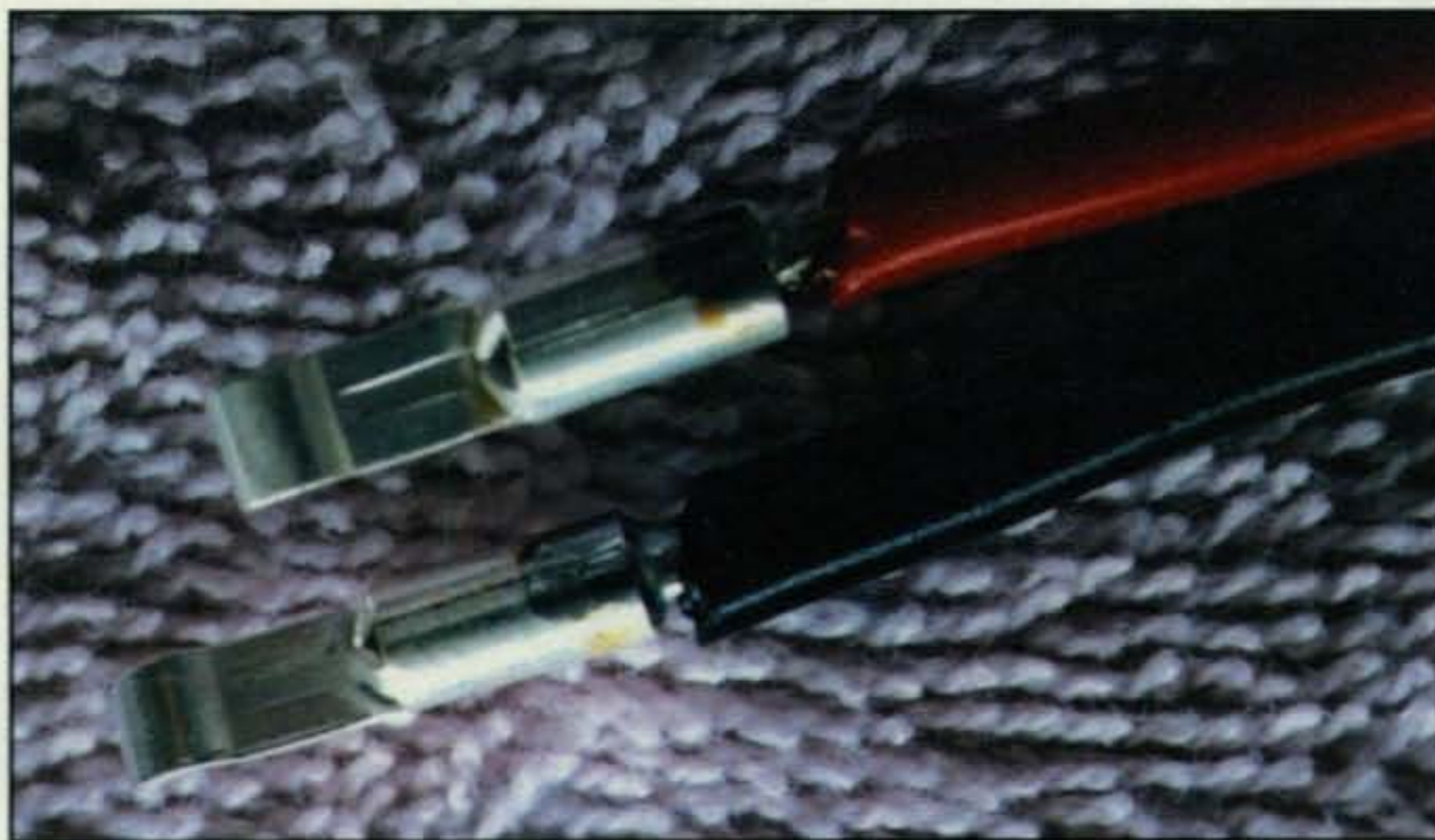
Photo 3— This is a close-up photo of what the wire-to-terminal joint should look like. Solder is wicked into the wire strands and has adhered to the terminal, without distorting the terminal or contact surfaces. There is no flux or excess solder on the sliding contact area.
