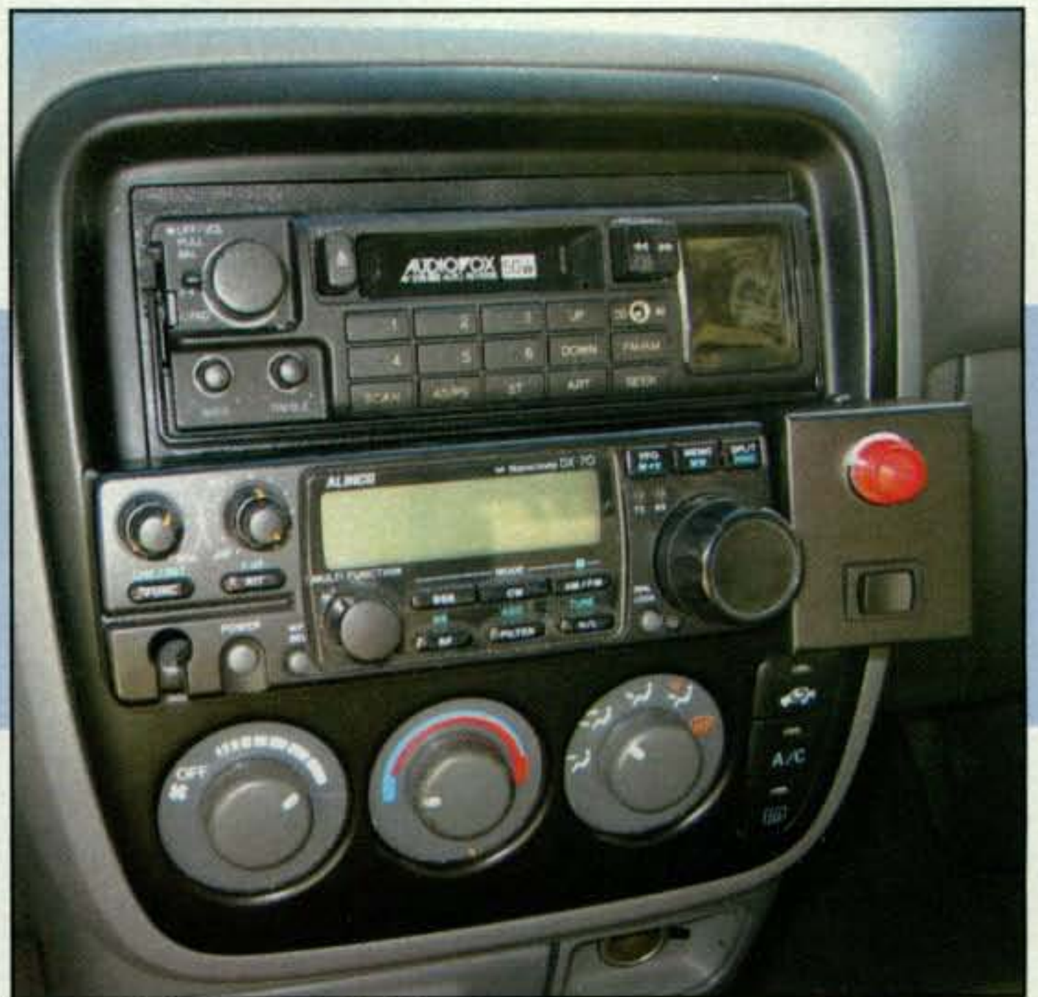
Photo 5— W6RH completed his High Sierra installation by placing the antenna control switch in the dash next to his Alinco DX-70 for a very professional look. (W6RH photo)
