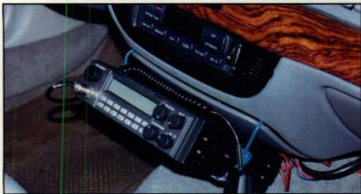
The Ranger RCI-5054DX is a single-band 6-meter FM mobile rig, one of very few such radios on the market today. (Individual radio photographs courtesy of their respective manufacturers)
