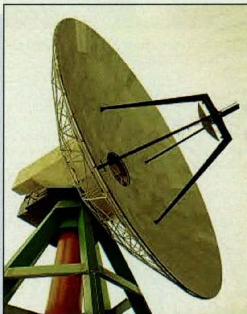
This 20-meter parabolic antenna in Bochum, Germany was used for the first amateur radio reception of the Mars Express spacecraft. This dish is to serve as AMSAT-DL command station for the P5A Mars Mission, which is scheduled for 2007. (AMSAT-DL photo)
