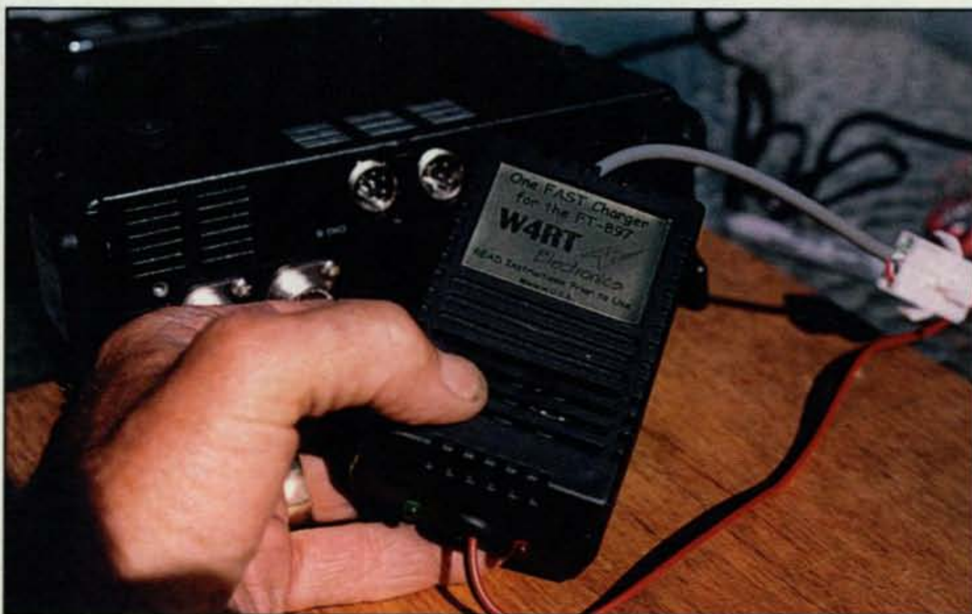
Be sure to keep the ventilation holes UP on the W4RT fast charger. The unit gets very warm after a few hours of charging, so you don't want to block ventilation.
