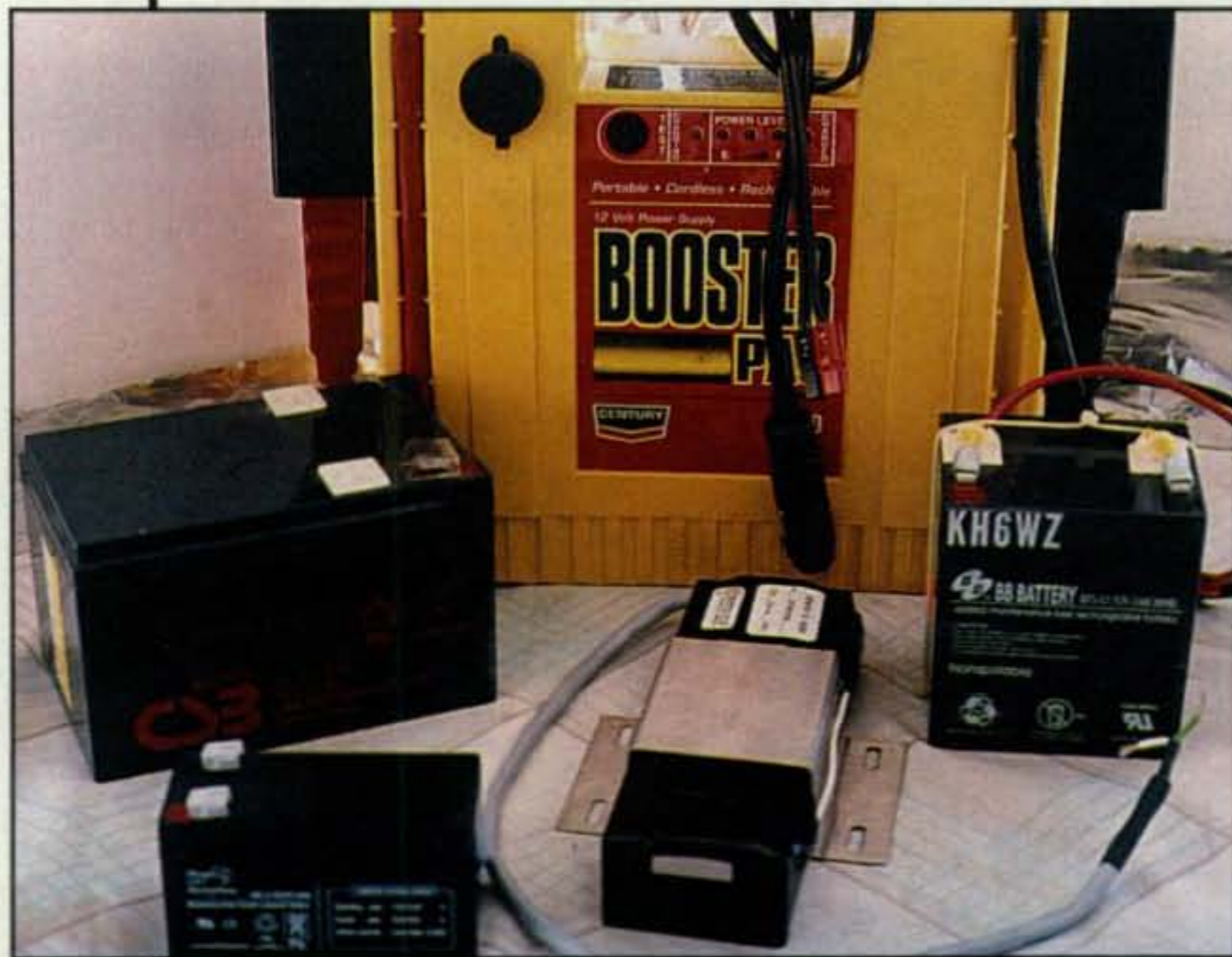
Photo 1— My growing family of 12-volt gel-cells. The big yellow box is disguised as an automotive emergency booster battery. Inside it is really just a 17-Ah gel-cell with an LED power/charge indicator. When looking for these units, get the heaviest ones you can find (bigger battery inside).
