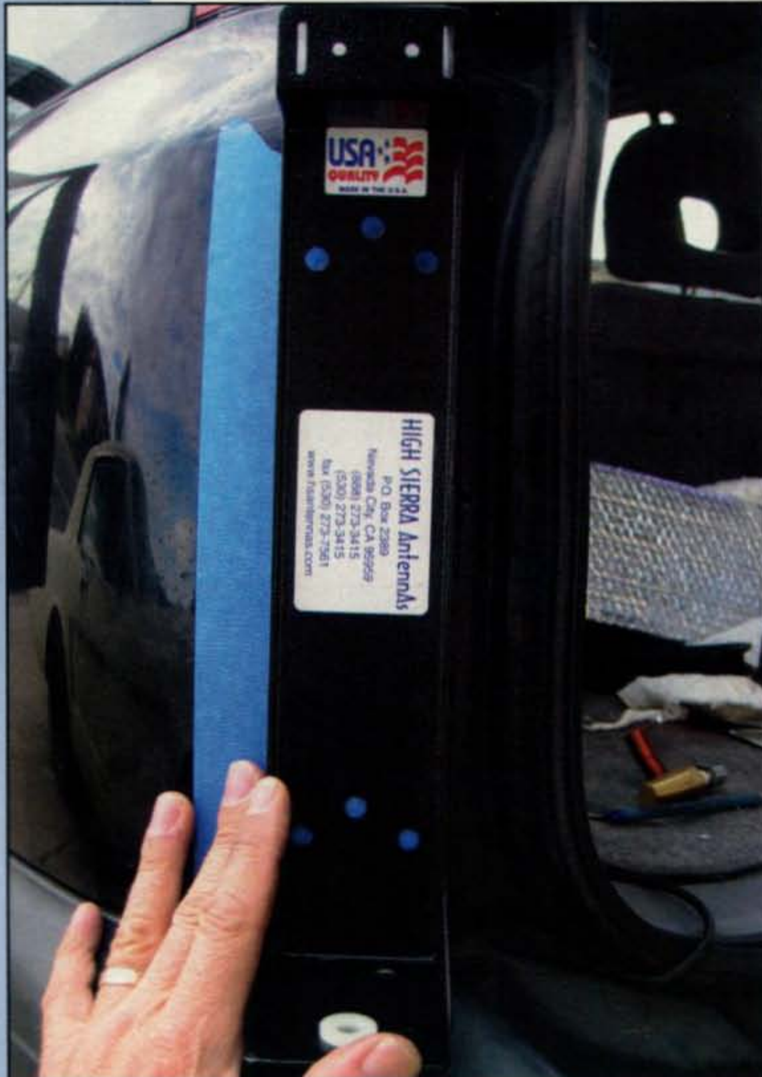
Photo 3— W6RH creates a template with tape prior to drilling holes in the car's body. (W6RH photo)
