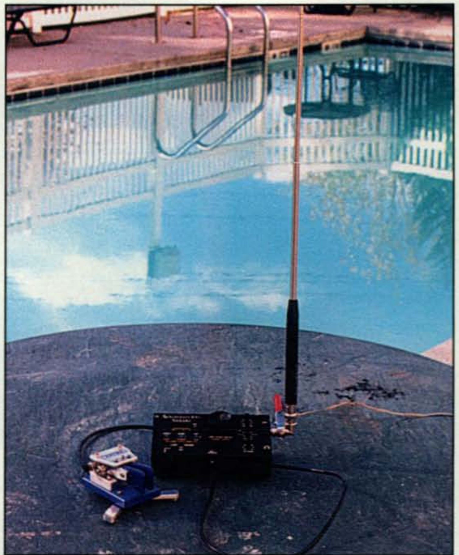
Photo 9— Poolside portable setup. Just plop down the rig, stretch out the counterpoise strap, and you are on the air in less than a minute. Try that with a big 100-watt rig. By the time you set up a power supply and run an antenna cable, I will have worked all the DX and gone parasailing!
