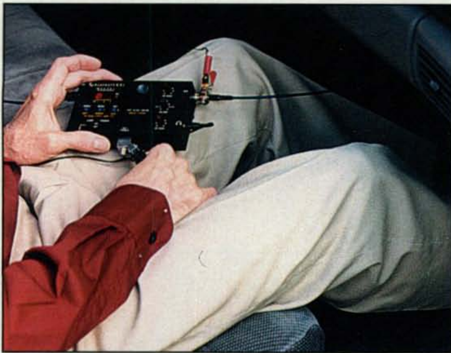
Photo 8— "Instant mobiling" in a rental car is easy. Just put the transceiver in your lap, let the XYL drive, and use a small earbud for good copy over road noise and screeching tires. Notice the separate ground strap clipped to the antenna plug; it routes directly to a body bolt under the seat and makes a big difference in performance.
