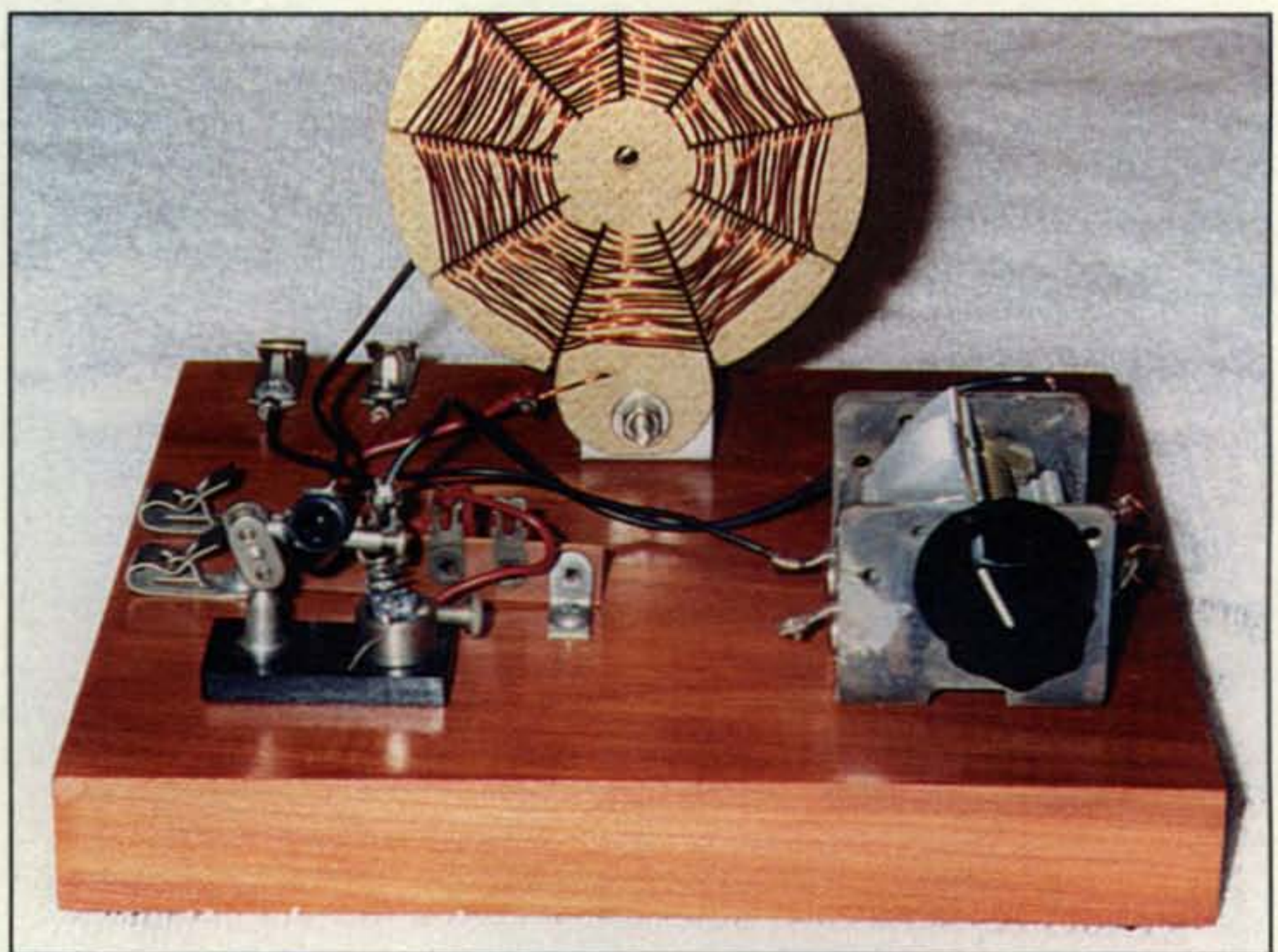
Photo D— This spider-web-coil-equipped crystal set was built by Walt Bullerwell, KF4YJQ, and tunes the AM broadcast band with slightly better than average selectivity. The little radio also uses an open-air galena and catwhisker-type detector like those employed during the era of spark. (Discussion in text.)
