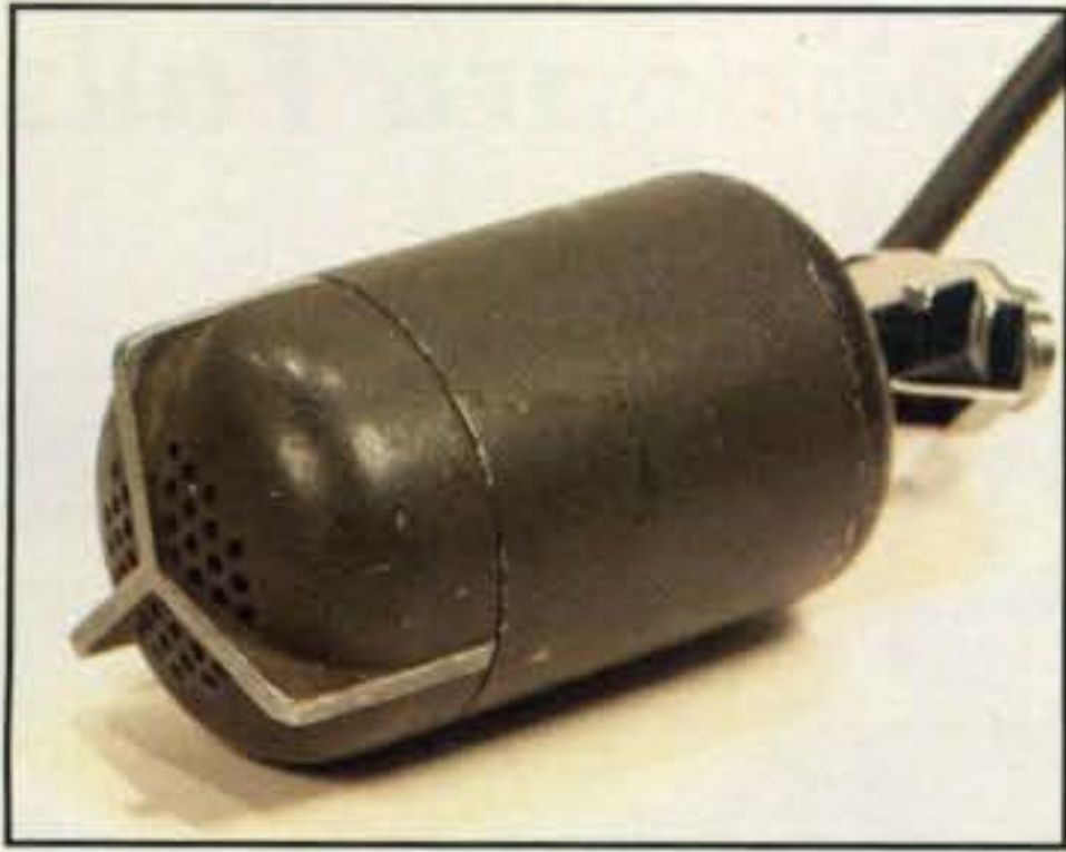
Photo 8— One look and you can understand how this Altec "Salt and Pepper" mic acquired its nickname. Every big-time newscaster of the 1940s had a Salt and Pepper mic. It surfaced in interviews, newsreels (remember those at the movies?), and more. Some folks attached them to stands (note rear mount) and some used them handheld style. (Photo courtesy K9EID)
