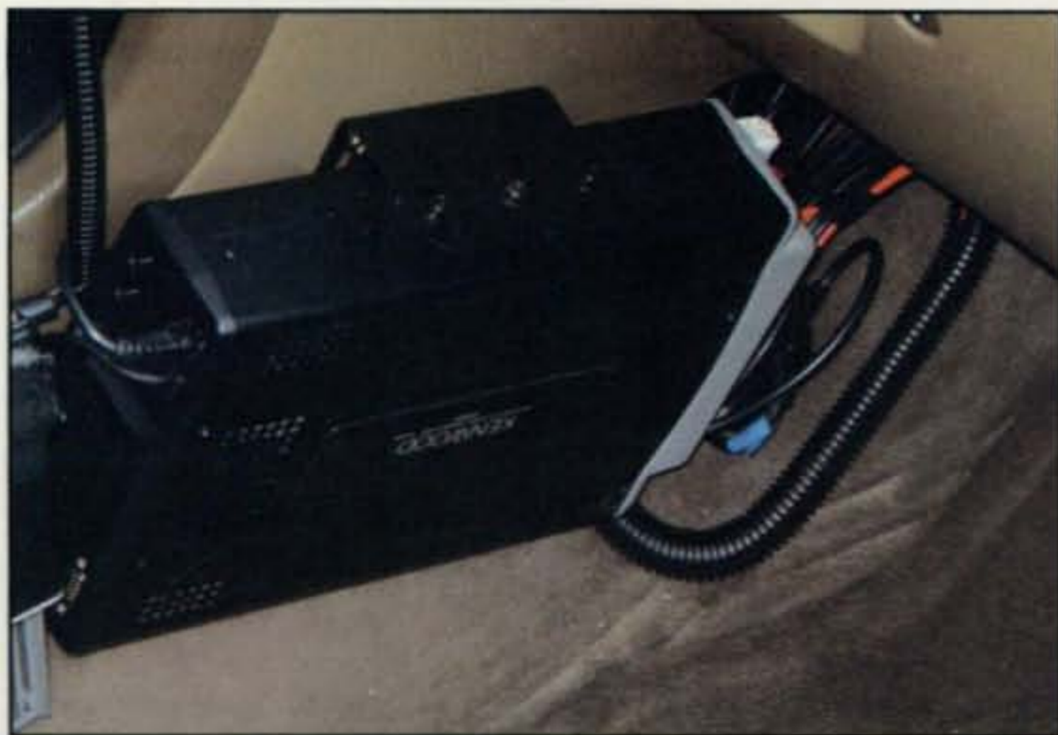
The radio body, mounted in the front passenger compartment. Note that the microphone plugs into the radio body, not the control head, so if you want to mount the radio body in the trunk, you'll need to get Kenwood's optional PG-4Z 4-meter panel extension kit, which will bring the access for your mic connector up into the passenger compartment. (N6FM photo)
