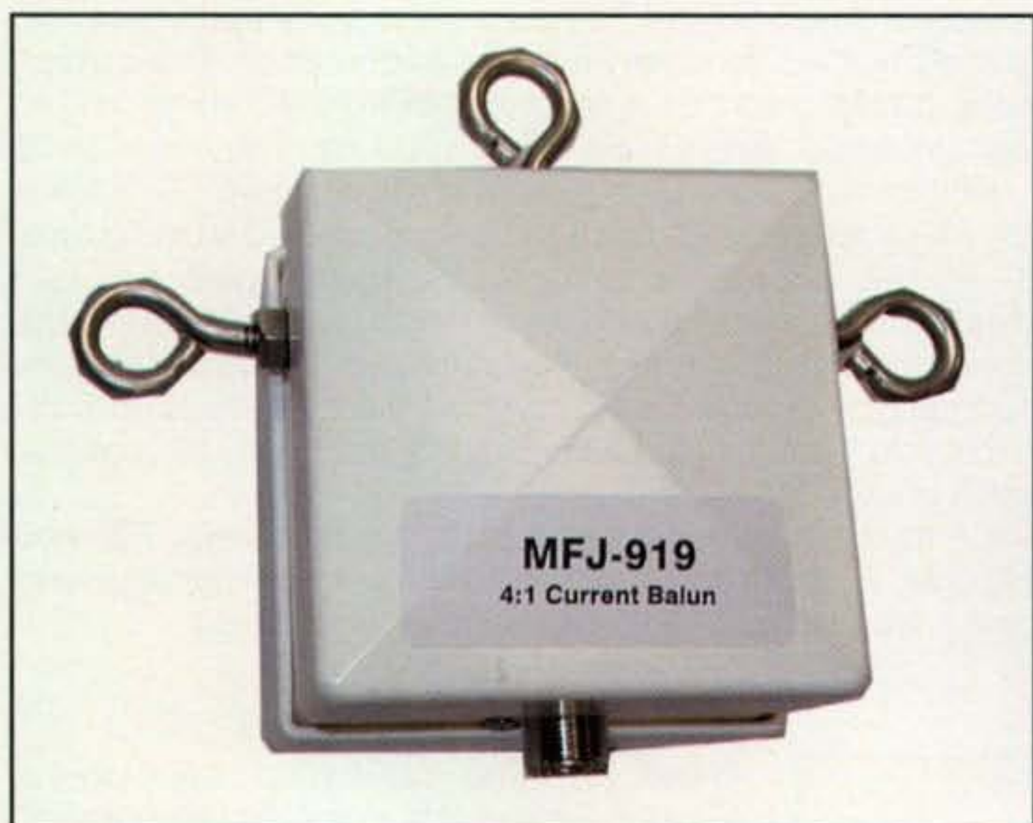
Photo F—The MFJ-919 4:1 Current Balun is a true current balun that doubles as an antenna center insulator, transforming 200 ohms to 50 ohms for convenient antenna feeding. The transmission-line transformer, using 100-ohm characteristic impedance transmission line, is said to provide a flat 160–10 meter response. (Photo courtesy MFJ Enterprises)
