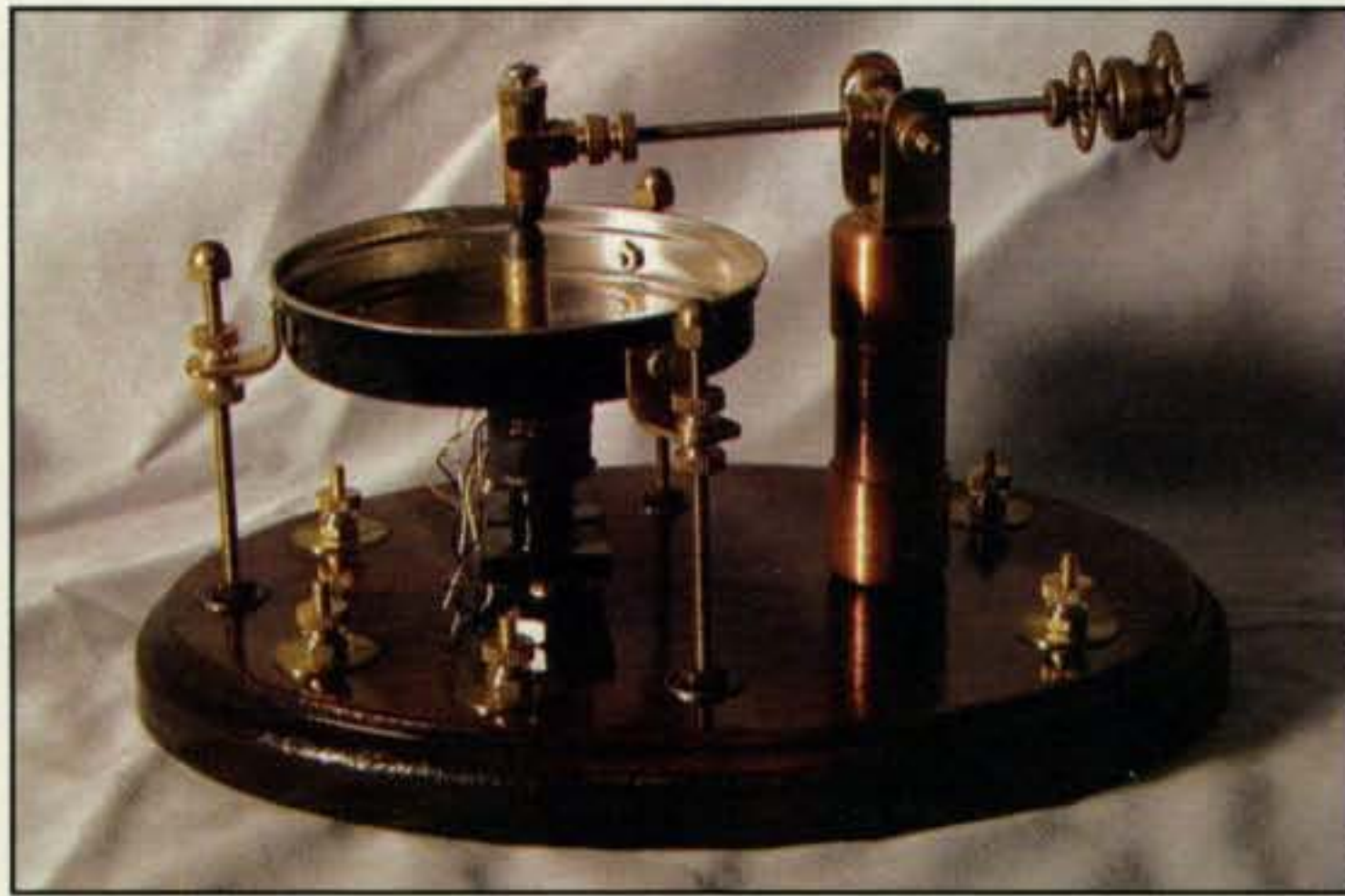
Photo H— Instruments of Amplification, by H. Peter Friedrichs, AC7ZL, shows you how to build amplifying components themselves! The extremely sensitive electromechanical amplifying instrument pictured here is called a "Balance Beam Amplifier," and it features carbon and graphite electrodes. Inspired by the Brown Amplifying Relay, it's capable of significant power gain. (Photo courtesy H. Peter Friedrichs)
