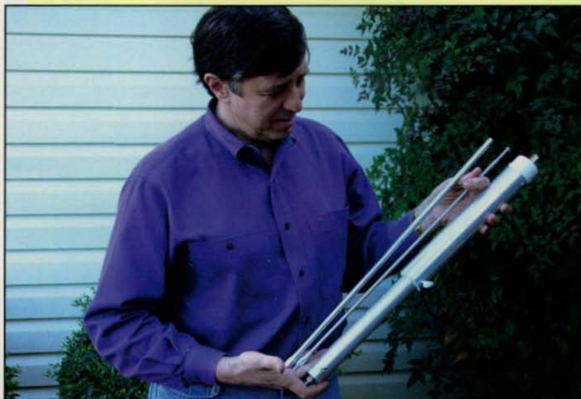
Photo 1— The author holding the disassembled MFJ-1664 antenna, including whip sections. Ease of assembly and disassembly makes the antenna convenient for portable operating. (Photos courtesy of the author)
