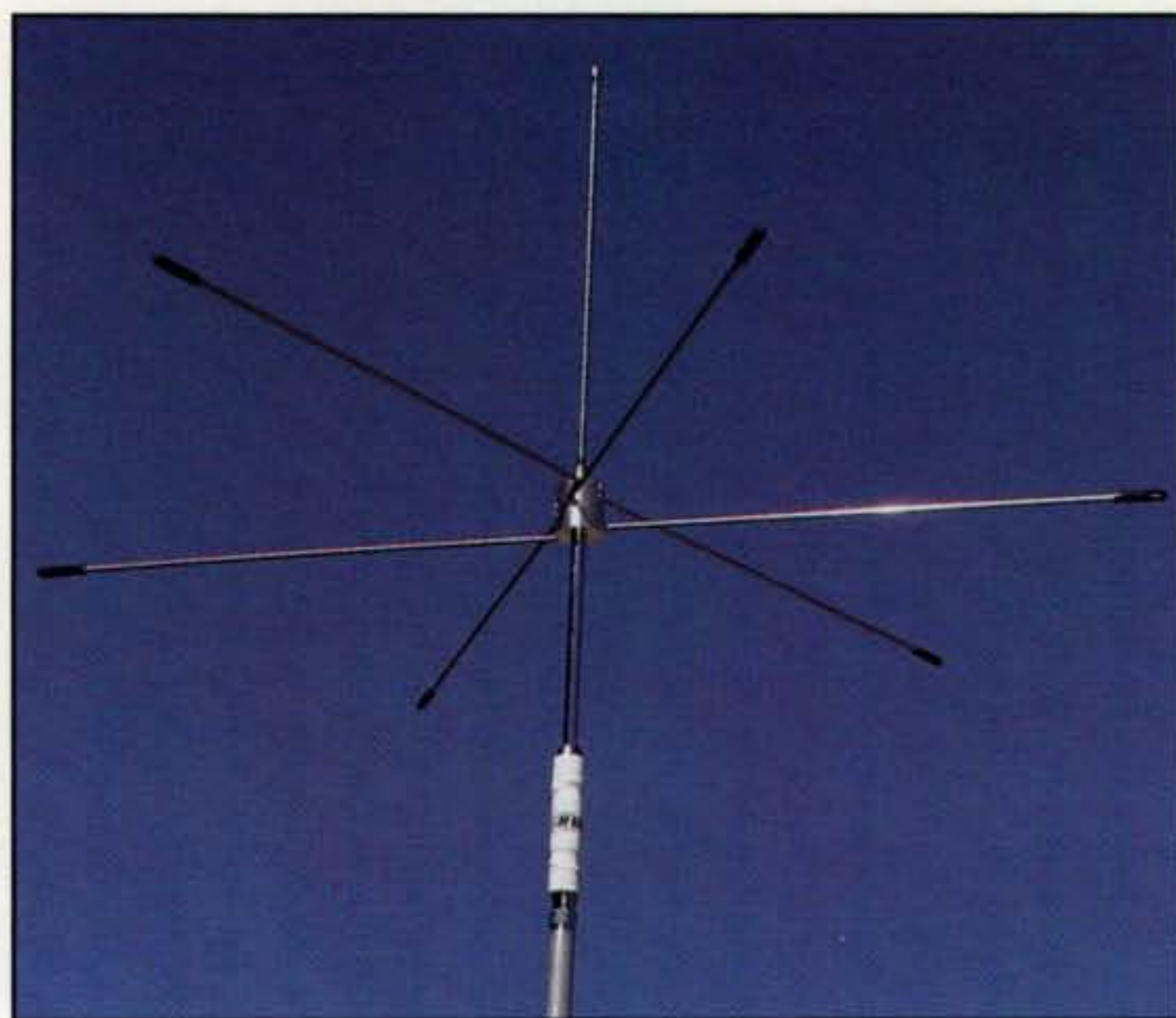
Photo G—DX Engineering offers a fully-adjustable capacity hat system, the Hot Rodz™, which can be applied to your Hustler mobile antenna and will allow you to run a significantly smaller loading coil. (Photo courtesy DX Engineering)
