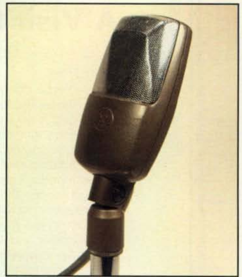
Photo 10— This marvelous-looking little gem is an RCA SK46 velocity mic. It is a high-gain PA-type microphone, and it was especially popular for complementing church and school sound systems during the 1950s. (Photo via K9EID)
