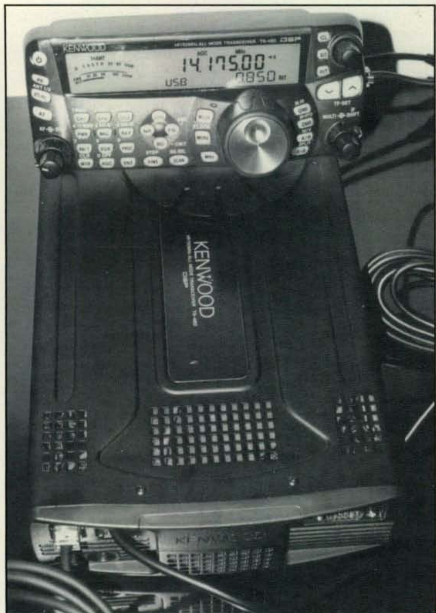
A rare meeting of the control head and radio body. Normally they are mounted separately and connected via a 13-foot cable (included with the rig). (WB6NOA photo)
