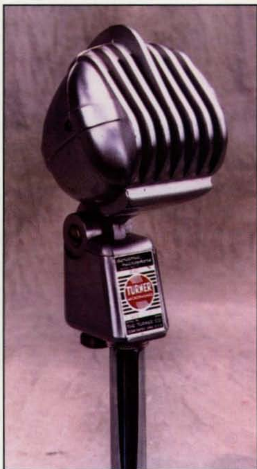
Photo 1— The simple elegance and neat "Deco" look that made Turner mics such as this model 33D popular during the 1950s and '60s still keep them irresistibly attractive today. This little gem would truly add class and flash to any amateur radio setup, especially if retro-fitted with a modern Heil element and red grill cloth. (Photo courtesy W2CQ, owner, and VE3NGW)
