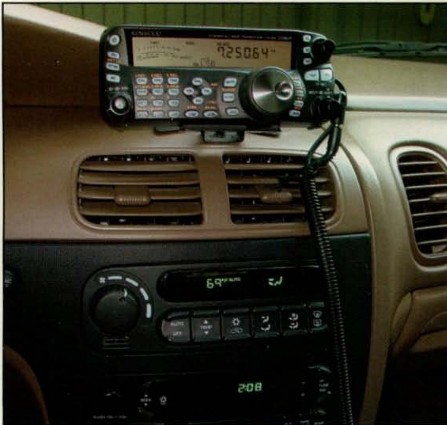
The control head of the TS-480 can be mounted just about anywhere on a dash-board for convenient and safe access while driving. (N6FM photo)
