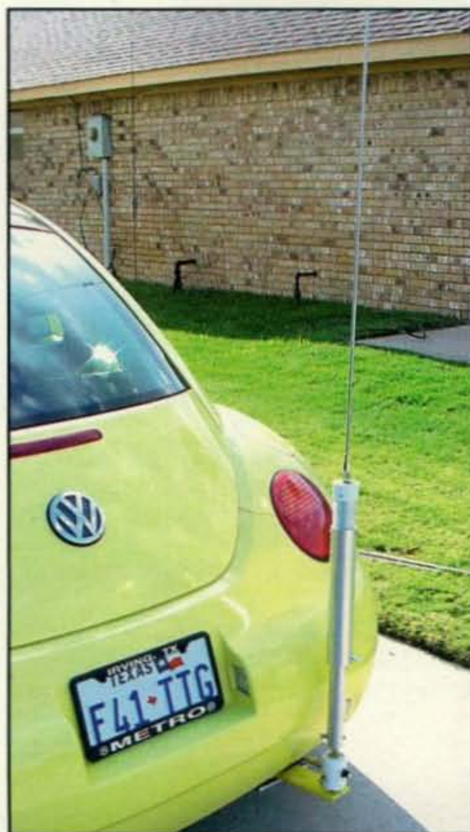
Photo 2— The MFJ-1664 mounted on the back of the author's VW New Beetle. The white piece at the bottom with the black switch is his variable capacitance switchbox for quickly changing base matching capacitors. (See "Base Matching" in the text for details.)
