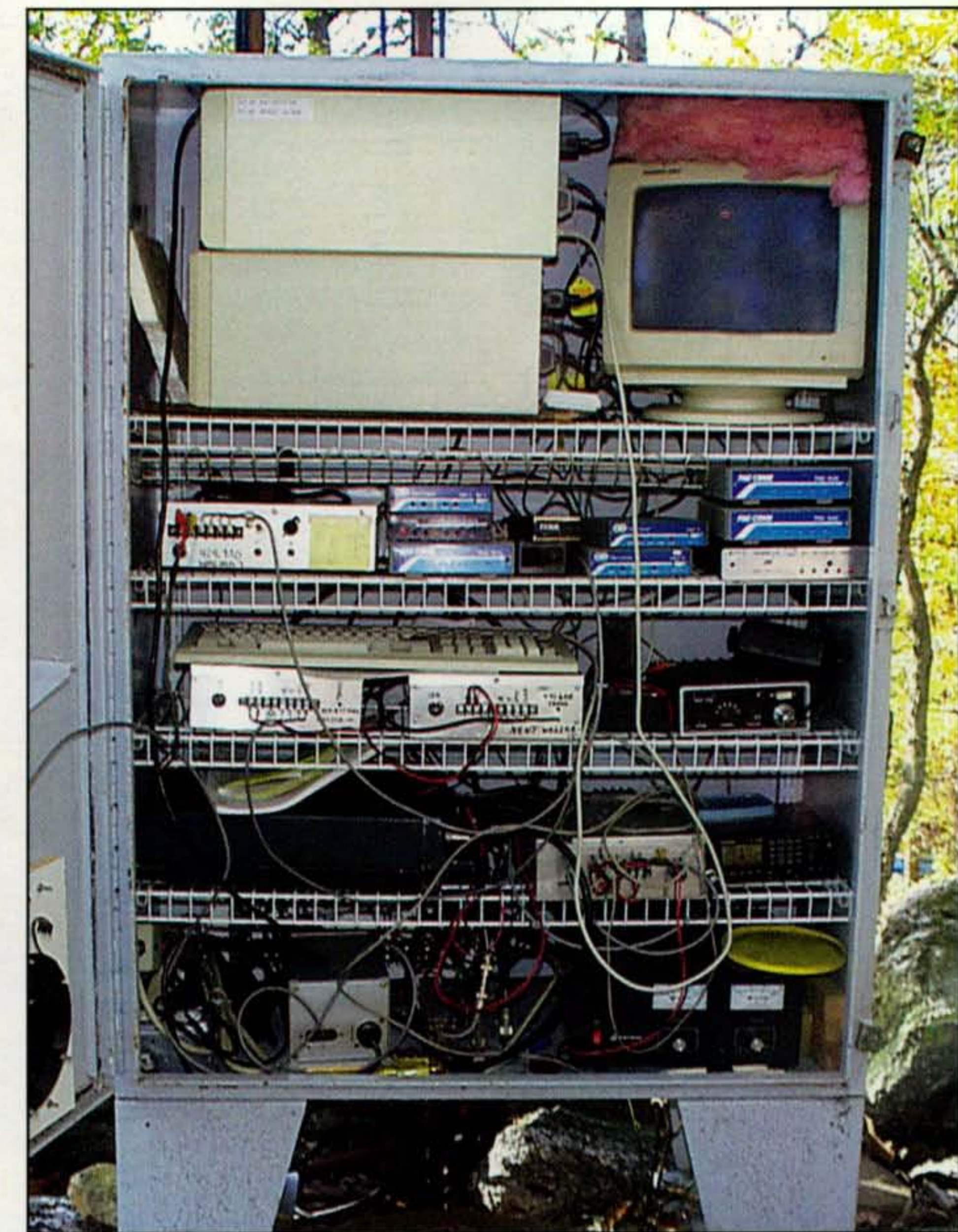
Photo 2— The WA2SNA packet network "node stack" circa 1996. Note the pile of TNCs, radios, and computers which ran this relatively large network site. The site has since been converted to FlexNet.
