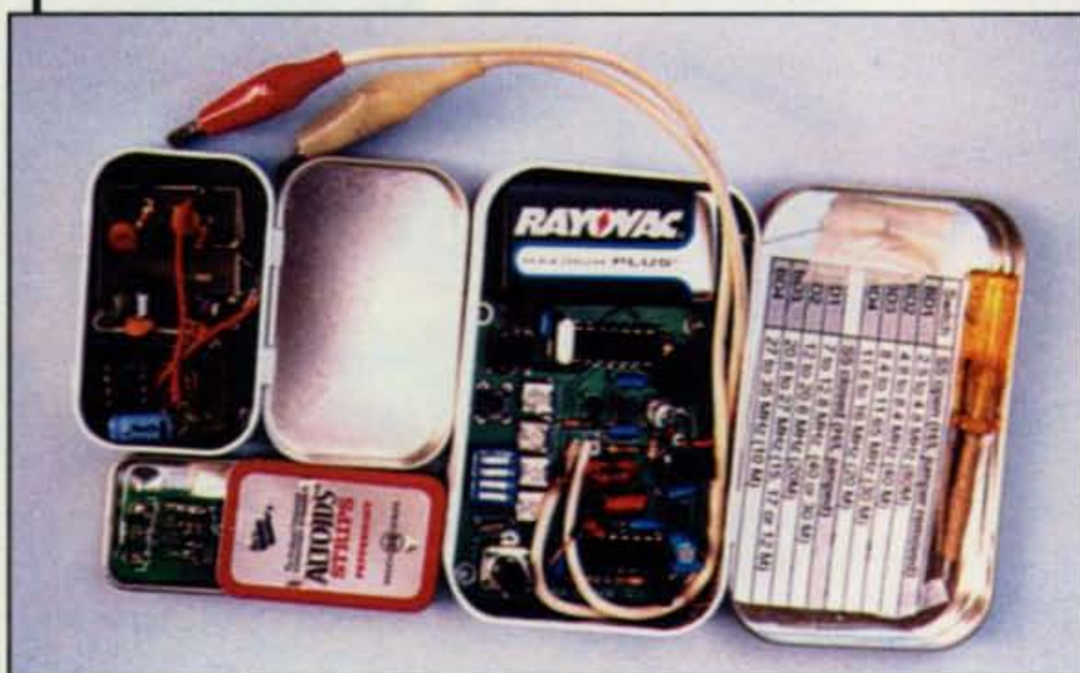
Photo A— Homebrewing and kit building are an integral part of the QRP experience, and the variety of projects is both captivating and endless. The "stairstep samples" shown here include an antenna SWR/resonant frequency tester from the Four States QRP group, my own mini-transceiver in a mini-Altoids tin, and a surface-mount Micronaut transmitter in a micro Altoids tin.
