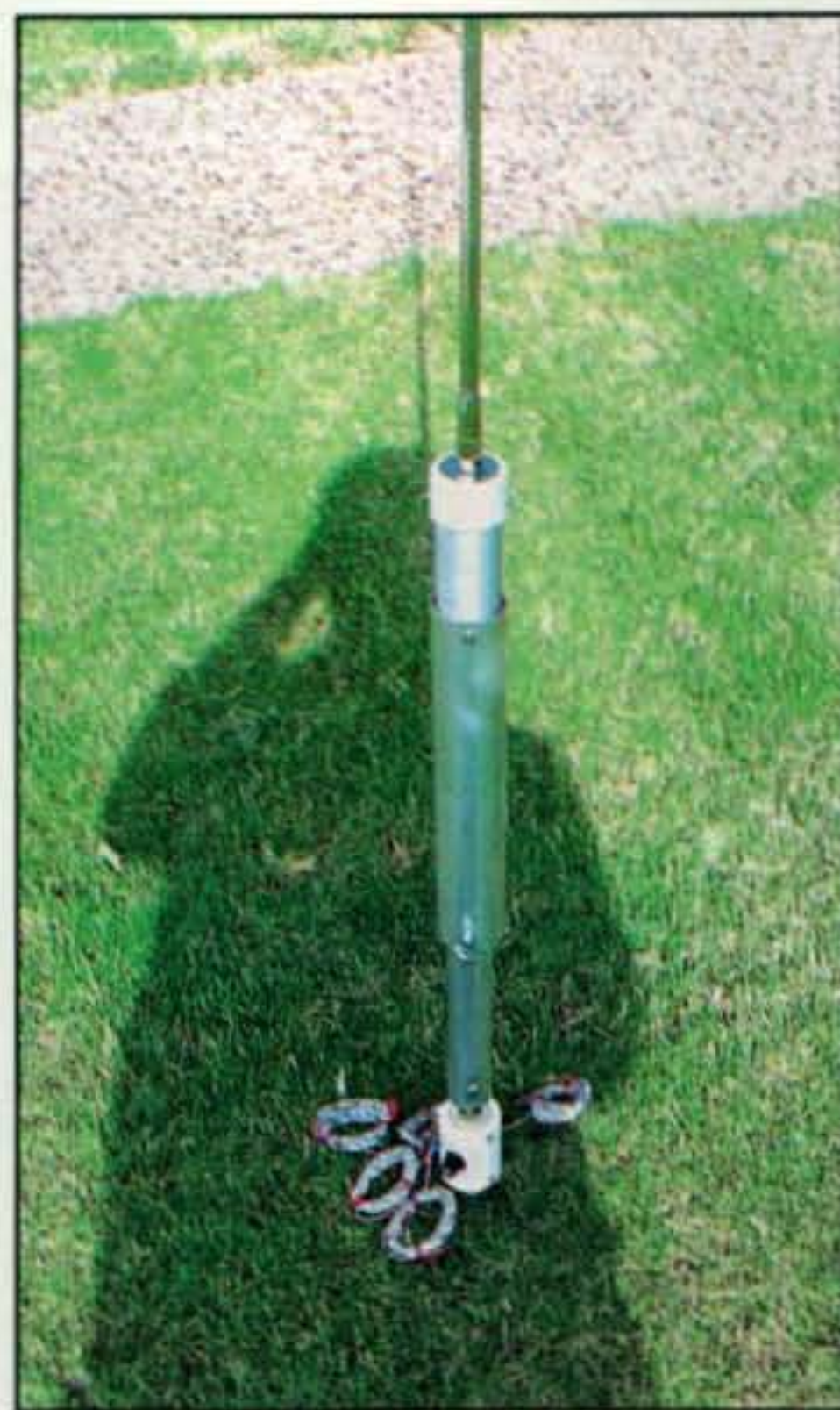
Photo 3— The MFJ-1664 also makes an excellent portable or temporary antenna when ground mounted with 16-foot wire radials.
