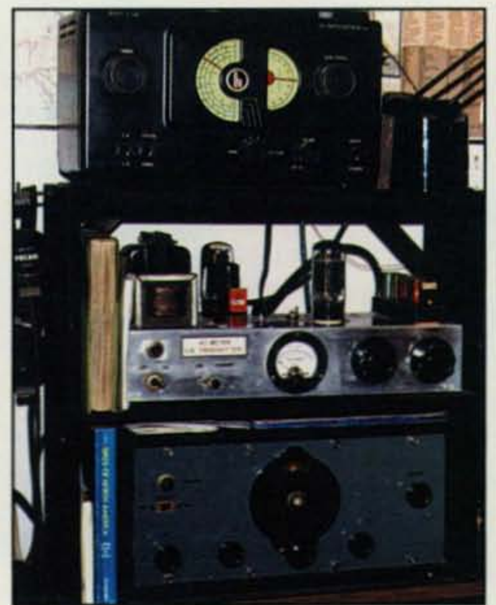
Photo E— Nostalgic QRP still romps! Bud Bearce, K5JGU, works QRP in style with the homebrew 5-watt transmitter and five-tube superhet receiver shown here. A classic Hallicrafters S-38 is used for backup and general short-wave listening. Bud answered one of my CQs and I never realized he was QRP until receiving his QSL and rig info.
