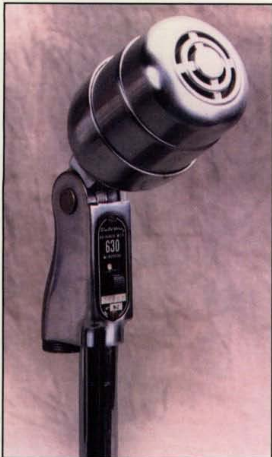
Photo 3— Another popular chrome-head mic during the early 1960s was this economically priced Electro Voice model 630. It featured a high-impedance and fairly wide-range dynamic element, it was designed mainly for PA use, and it also proved to be a good mic for SSB with new-era vacuum-tube transceivers such as the R. L. Drake TR-3 and National NCX-5. (Photo courtesy W2CQ and VE3NGW)
