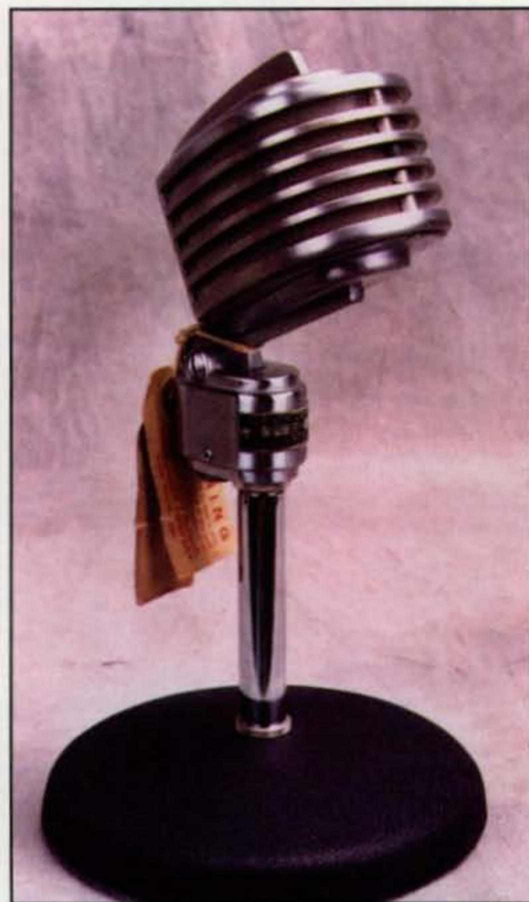
Photo 2— Bold, sweeping lines and the authoritative good looks of a real radio broadcast microphone make this vintage Turner model 34X a real attention grabber. It is equipped with a crystal element to mate with older vacuum-tube gear and was used as a prop in several '50s-era movies. Note original sales tags still intact on mic owned by W2CQ and photographed by VE3NGW.
