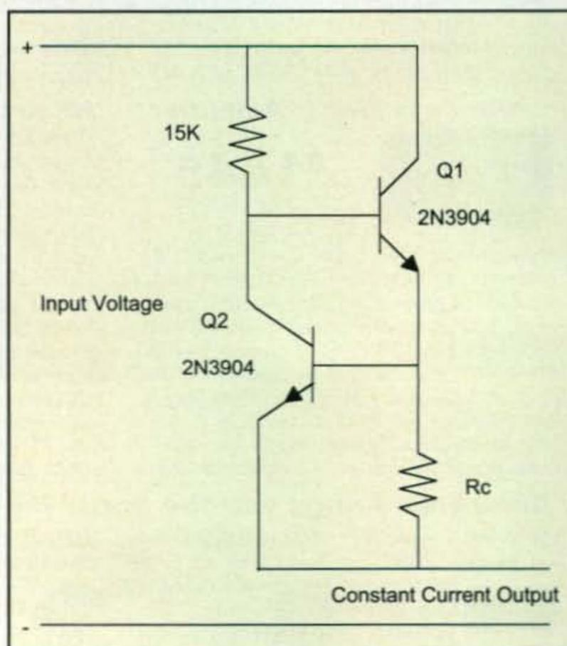
Fig. 3—Current-regulator circuit.
