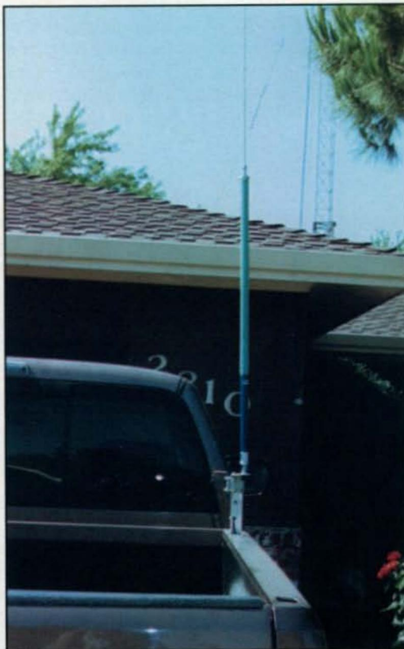
*Photo A— Check out this classic mobile antenna Mike Zane, N6ZW, mounted on his pickup truck. It is a 50-year-old, immaculately preserved Webster Band Spanner. It covers 75 through 10 meters and works like a manually tuned screwdriver-type antenna. Big-time radio glamour for sure! (Photo courtesy of N6ZW)*
