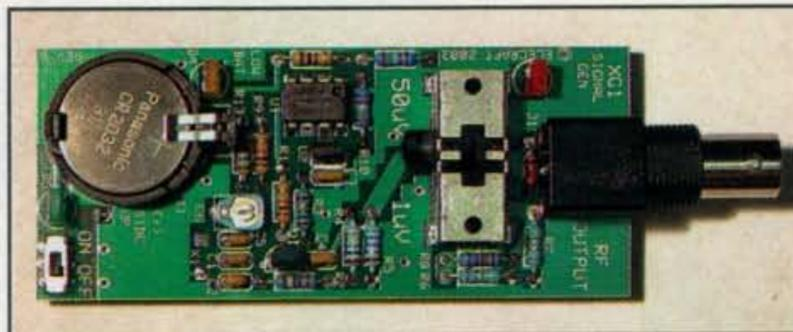
Photo A— One of the most important receiver-performance measurements is sensitivity. However, measuring sensitivity usually requires an expensive, lab-grade signal generator. Elecraft's new XG1 Receiver Test Oscillator is an inexpensive alternative. (Photo courtesy Elecraft)
