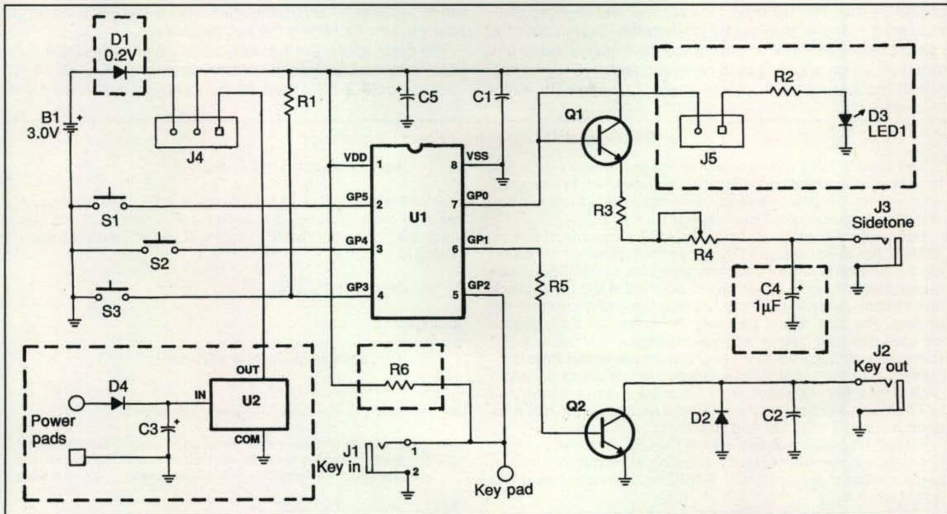
Fig. 1— Schematic of the W0XI Straight-Key Keyer. Note that the circuit calls for a 3-volt DC supply (2 AAA batteries), but it can also be set up to run off a 12-volt DC supply. (See text for details.)
