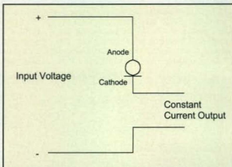
Fig. 2—The current-regulator diode circuit.
