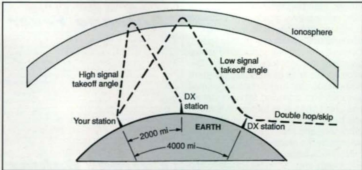
*Fig. 2— Comparison of high and low signal take-off angles from antennas. Notice the lower angle reflects lower on the horizon and first skip covers a longer distance. Signal(s) may continue to skip two or more times, but attenuation by each Earth and ionospheric reflection usually reduces signal strength.*
