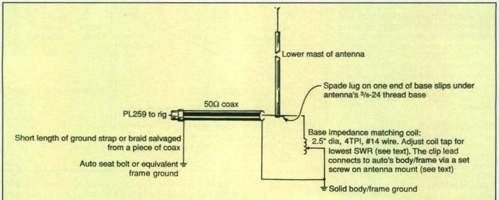
Fig. 3— Interconnection guide for putting together a top-notch HF mobile setup with antenna base impedance-matching coil and solid vehicle-frame ground system. (Discussion in text.)
