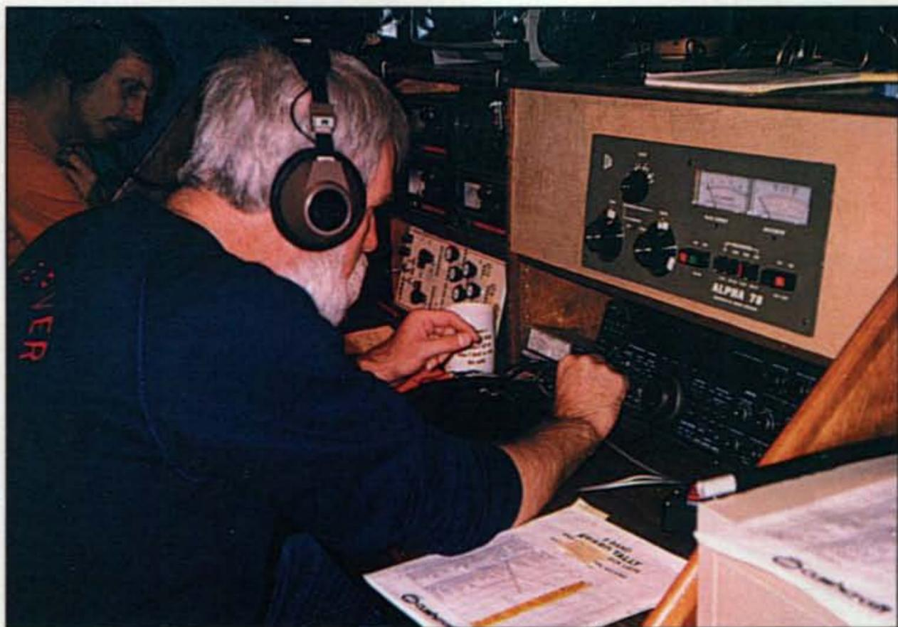
*Photo B— This is a typical "serious" HF contesting station. A custom console houses the equipment and accessories. This is one of three operating positions. Several operators can control multiple transceivers and antenna systems at the same time.*
