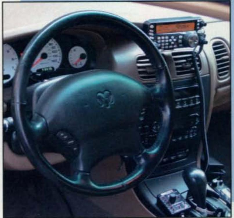
*Today's compact equipment allows hams to have a complete "shack on wheels" without occupying the whole car or looking unsightly. This is N6FM's very neat HF/VHF/UHF installation of a Kenwood TS-480 mobile HF rig (control head on dashboard, RF unit behind VHF rig), an Alinco DR-605T 2-meter/70-centimeter FM transceiver, a remote-control unit for his SGC 500-watt HF amplifier, and a Heil headset mic for safe operating while driving. (N6FM photo)*
