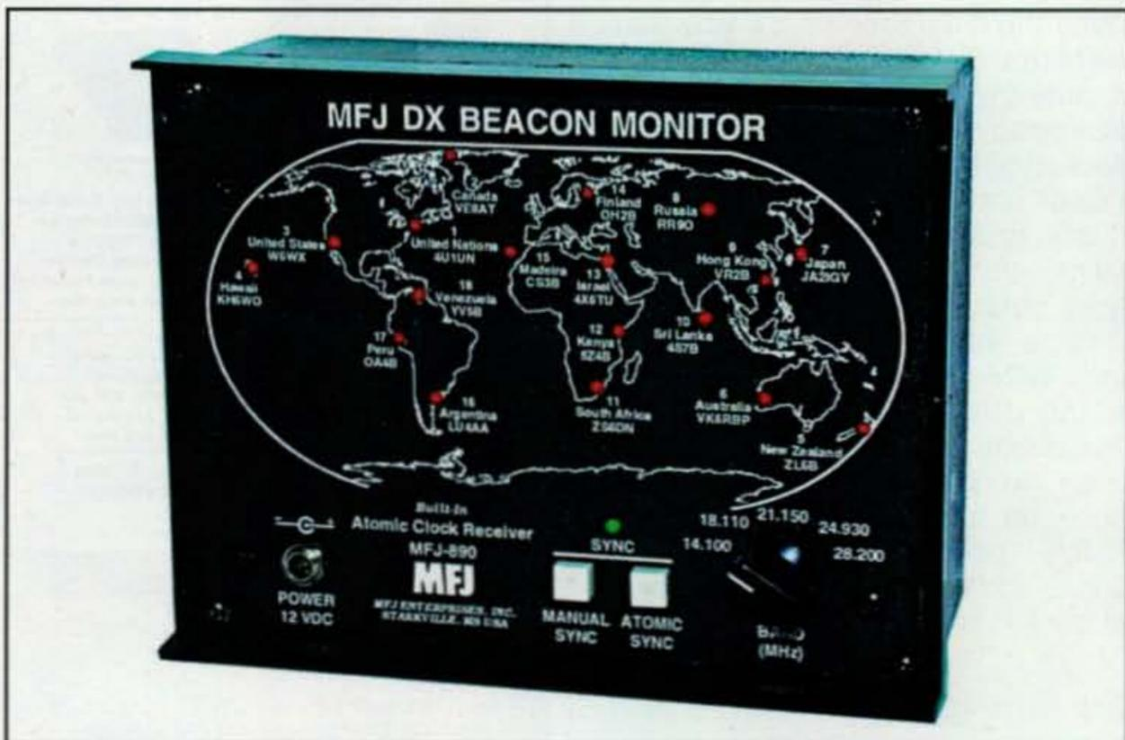
*Photo B— This MFJ DX Beacon Monitor uses atomic-clock-referenced signals from WWVB to precisely simulate timing of the NCDXF worldwide HF Beacon Network. With 18 LEDs it continuously displays on its map which network station is transmitting. Just tune your receiver to a beacon frequency and note which LED lights when you hear a beacon signal. (Photo courtesy MFJ Enterprises)*
