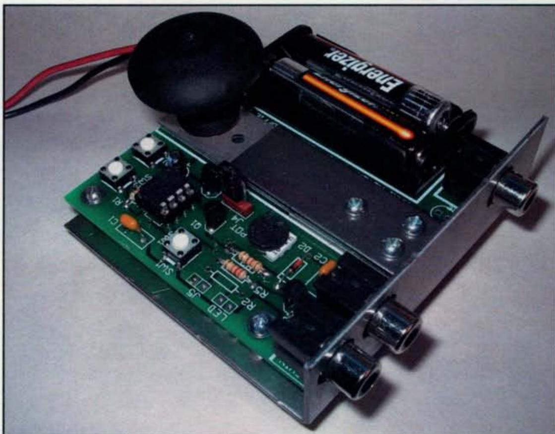
Photo A—The WØXI Straight-Key Keyer. It's shown from the rear so you can see the connectors. If you buy the complete kit, a case is included. (Photos courtesy of the author)
