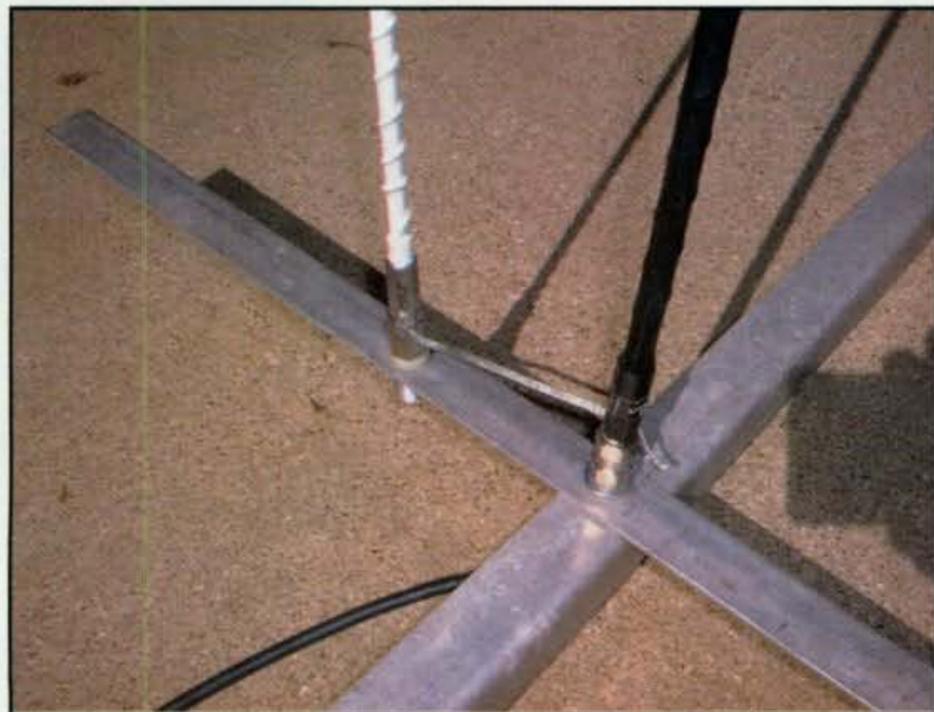
Photo C— Using two “stick” style antennas on your new ground plane. See text for details on using two antennas and just one feedline.
