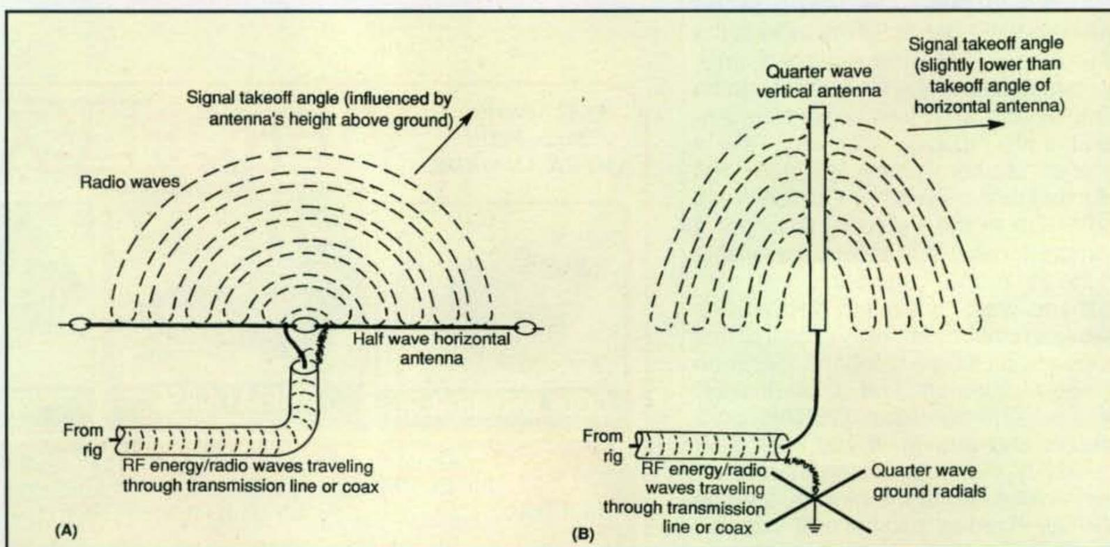
Fig. 1— The general concept of how radio waves generated by a transmitter or transceiver travel through a transmission line and are radiated into free space by an antenna. Some waves reflect off the ground and reinforce other waves to produce an overall signal take-off angle. This angle directly influences signal strength at a distant receiving point. (Discussion in text.)
