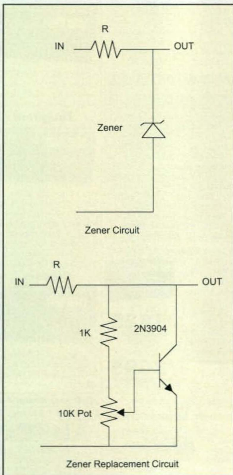
Fig. 1—A zener-diode replacement circuit.
