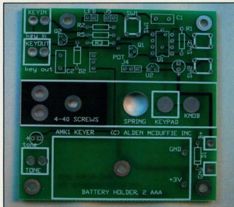
Photo B— The printed circuit board (PCB) for the Straight-Key Keyer. See notes on availability of complete kits or, for the junkbox enthusiast, only the PCB and programmed chip.
