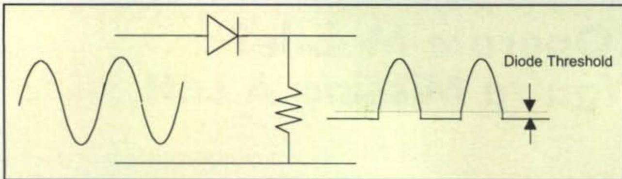
Fig. 4— Common half-wave rectifier.
