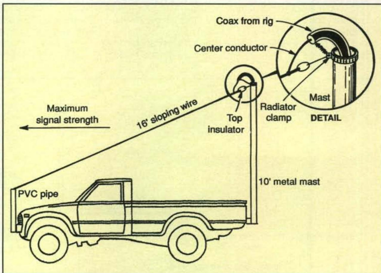
Fig. 2— Outline of the 20-meter mobile sloper devised by Budd Drummond, W3FF, for use on his pickup truck. Coax routes through the center of the 10-foot mast and the center conductor connects to a sloping wire at top. Coax shield connects to the mast, which is bolted to the frame. The sloper is full quarter-wave long and radiates an outstanding signal.
