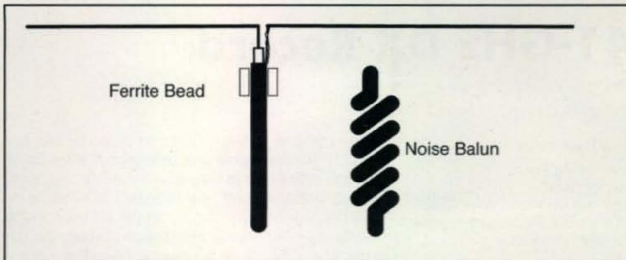
Fig. 3— Either a ferrite bead or a coaxial “noise balun” (see text) at the antenna feedpoint will create an effective RF choke to prevent RF energy from flowing back down the shield of the coaxial cable.
