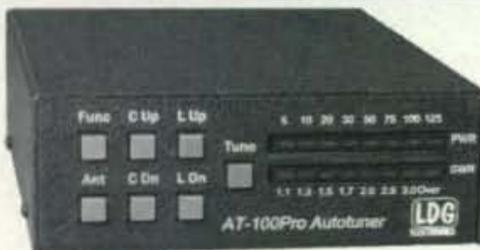
The **AT-100Pro** is a full featured, frequency sensing, memory autotuner designed for today's HF radios. It features dual antenna connectors with over 2000 memories for each. Latching relays reduce power consumption and hold the match even with DC power removed.
