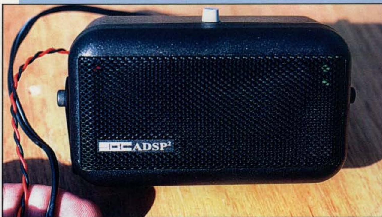
*The SGC ADSP<sup>2</sup> speaker offers two levels of noise reduction: One push of the top button drops the noise by 13 dB, best for SSB; pressing it a second time puts in 26 dB of DSP noise reduction, best for CW or data signals in a high-noise environment. A third push returns you to normal audio.*
