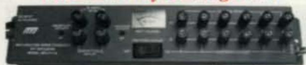
MFJ-1118 Power two HF and/or VHF rigs and six accessories from your main 12 VDC supply. Built-in 0-25 VDC voltmeter. Two pairs 35 amp 5-way binding posts, fused and RF bypassed for transceivers. Six pairs RF bypassed binding posts with master fuse, ON/OFF switch, and "ON" LED provide 15 Amps for accessories. 12½x2½x2½ in.
