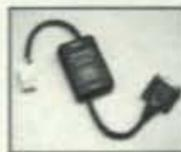
Intelligent Radio to LDG Autotuner Interface. Provides tuner control and DC power.
