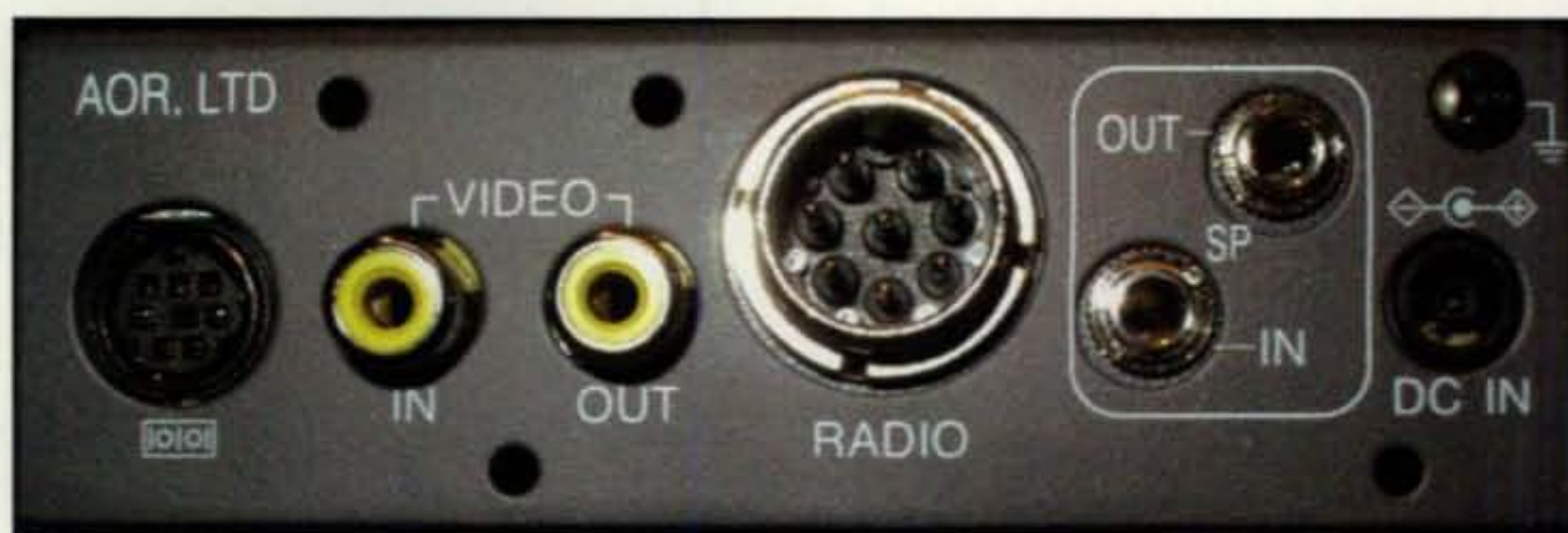
The rear panel of the 9800 has connectors for a computer serial cable (for text modes), video in and out (for digital video), the output cable to the transceiver mic connector, audio in and out, and DC power.
