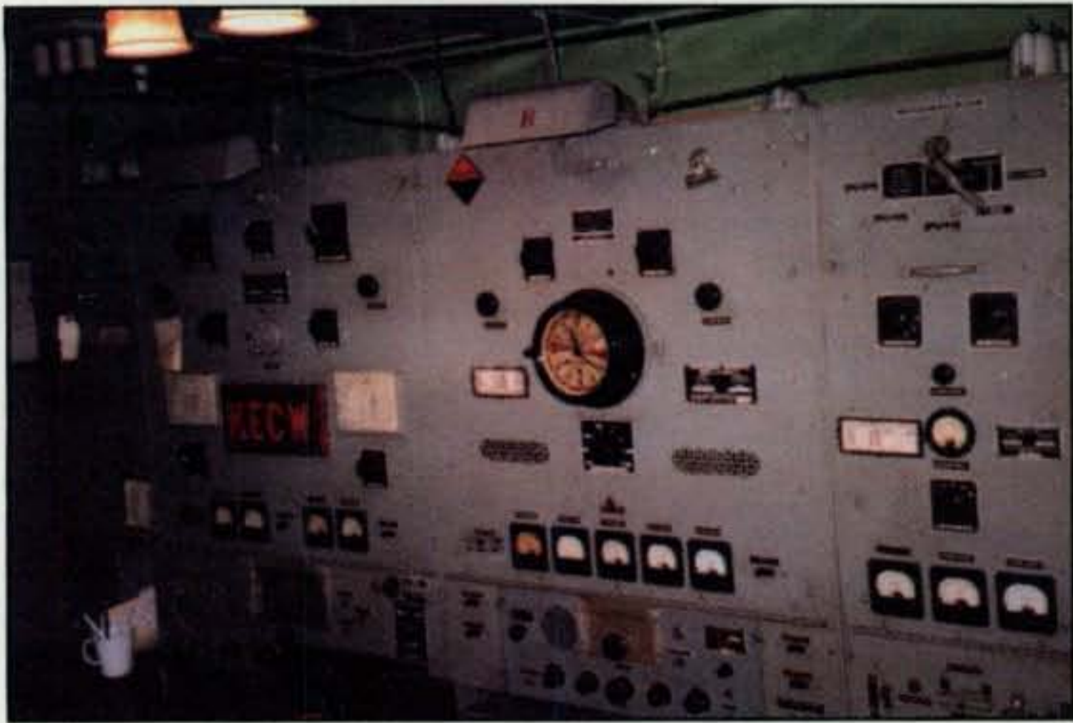
Photo F— The SS Lane Victory's original and beautifully restored radio room has three transmitters, three receivers, and a classic L F Auto Alarm system. Classy! (Photo courtesy KE6CJM)
