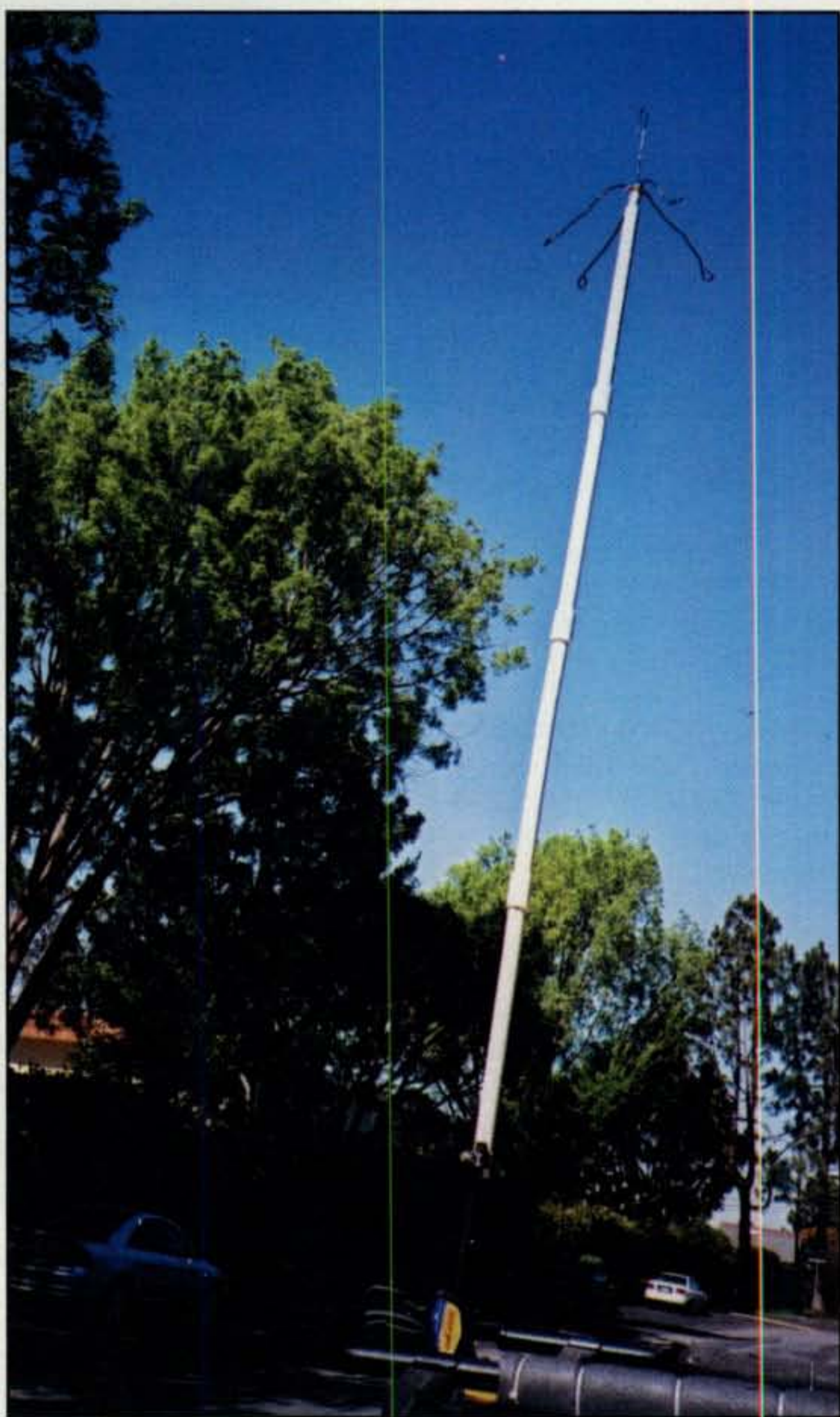
Photo C— The “squishy ground plane” is shown here unfolded and clamped to the multi-purpose rack on my vehicle. Mind the overhead clearance! For “man-pack portable” operations, the antenna can be lashed to a backpack frame. The number and lengths of pipe can be varied to adjust height.
