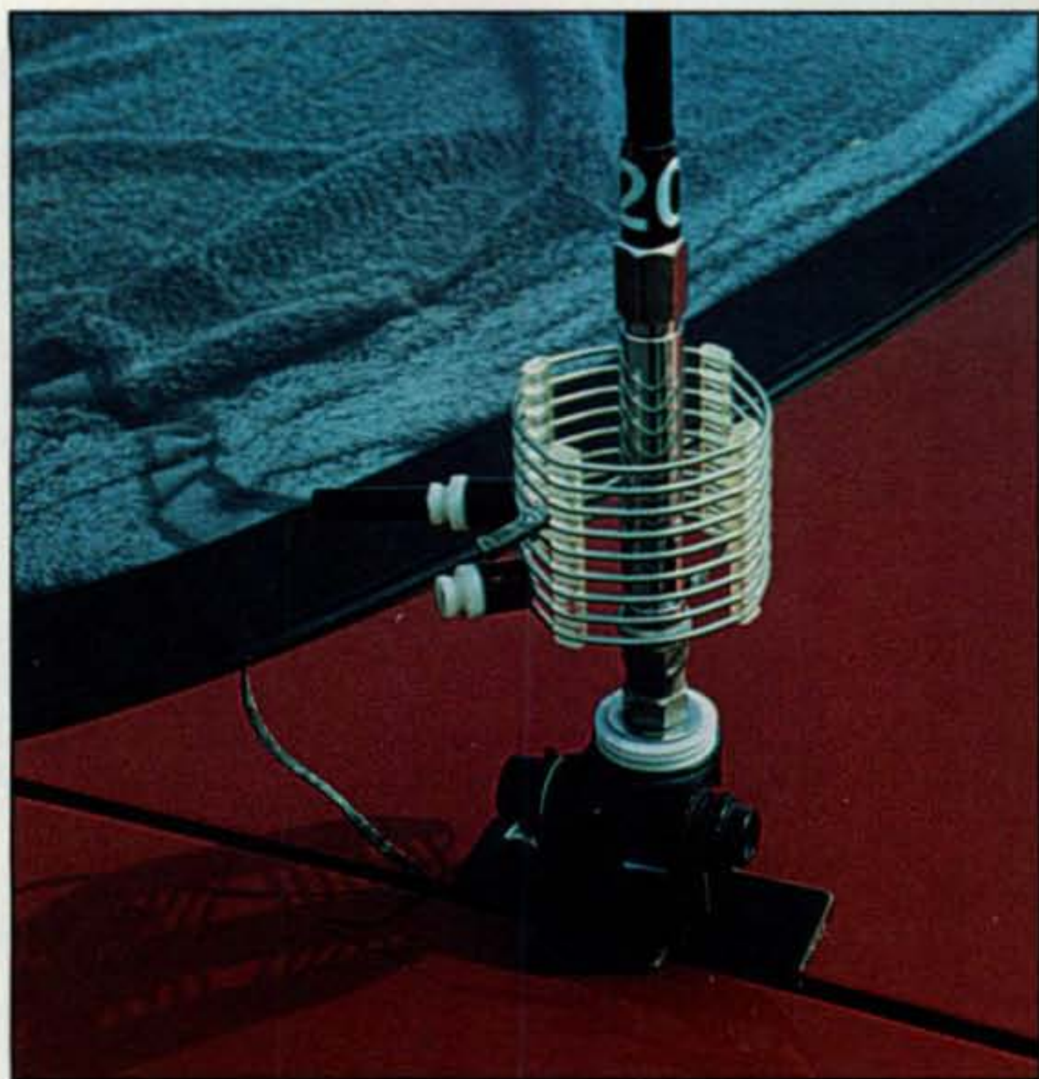
Photo C— Close-up view of the optional Iron Horse Quick Disconnect for easy band changing, plus the tapped base coil I added for impedance matching. (Discussion in text.)
