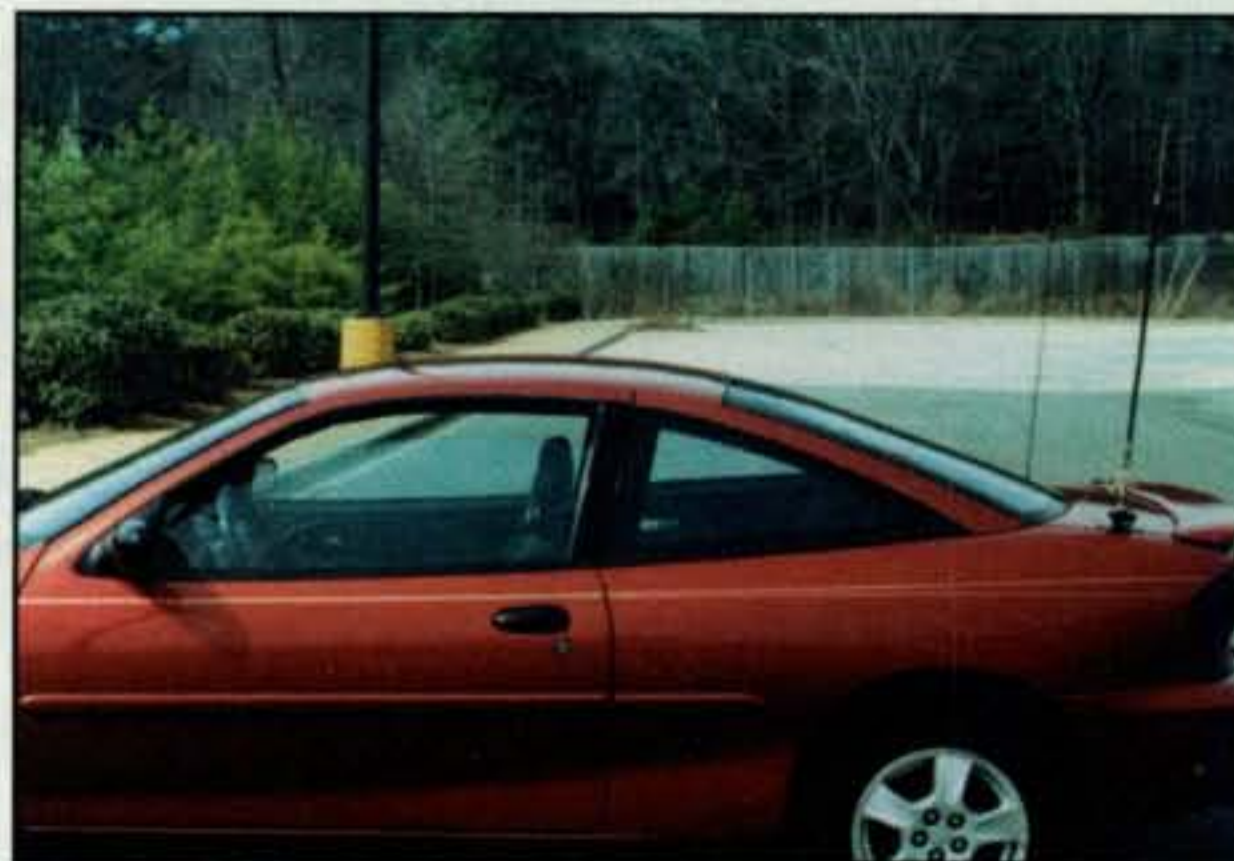
Photo B— Iron Horse's new half-size monoband HF antennas are ideal for low-profile mobiling with a regular trunk mount, and they are also handy for quick-mounting on hatchbacks of SUVs or Peugeots. (Details in text.)
