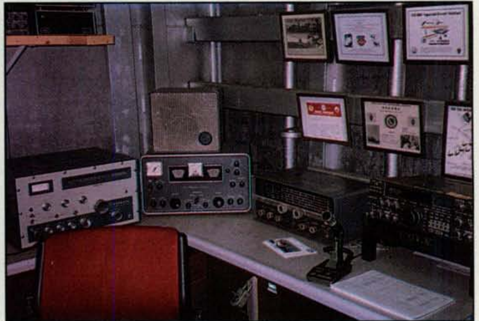
Photo G— The SS Lane Victory's ham shack sports a romantic blend of classic Heath, Hammarlund, and Hallicrafters gear, with a Kenwood TS-940 included for present-day flair. Now that's mobilizing in style! (Photo courtesy KE6CJM)
