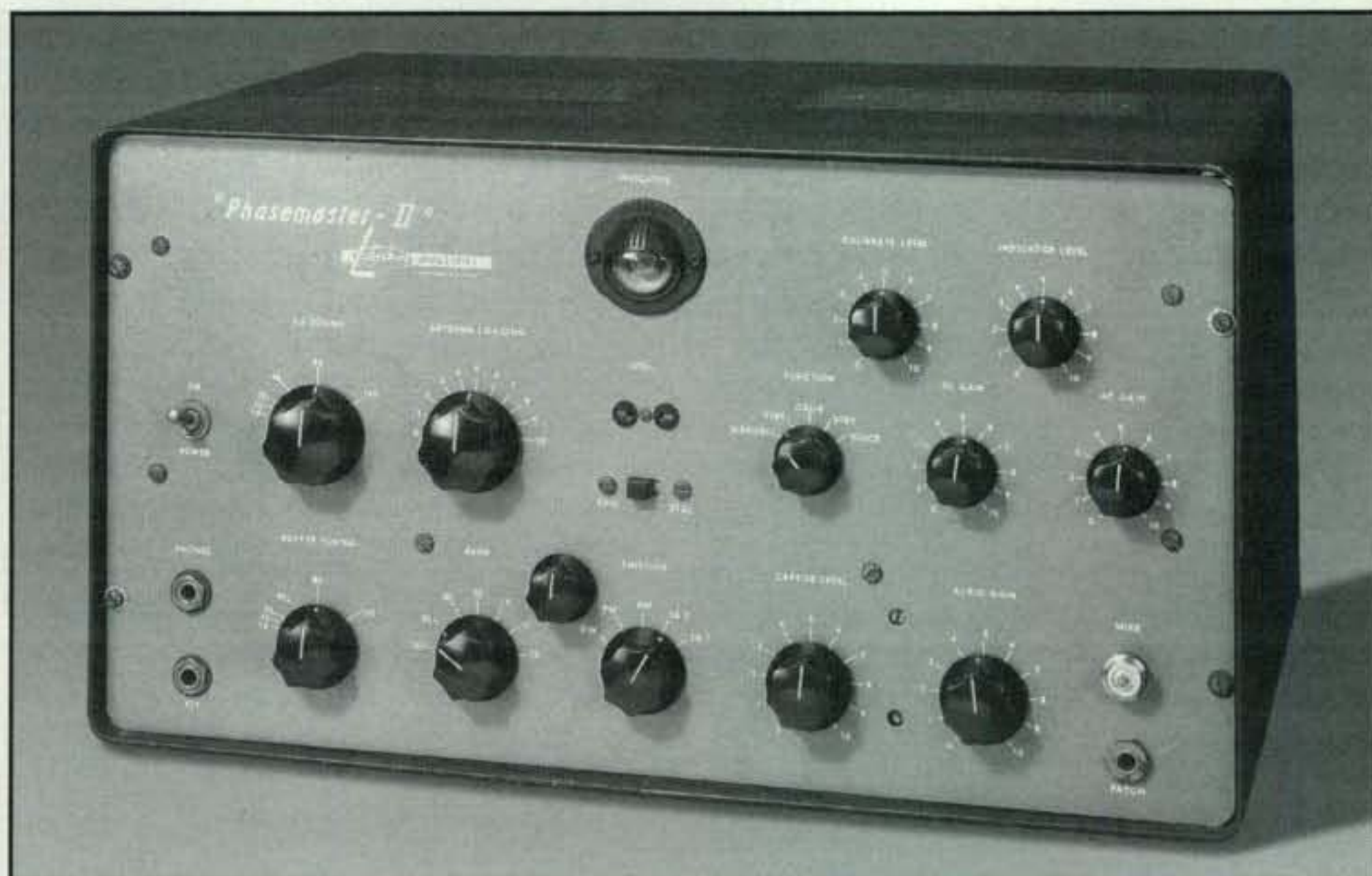
Photo B— Lakeshore Industries' Phasemaster II SSB/CW/AM transmitter sold for $279.50 in kit form or $329.50 factory-wired; 1955–57.
