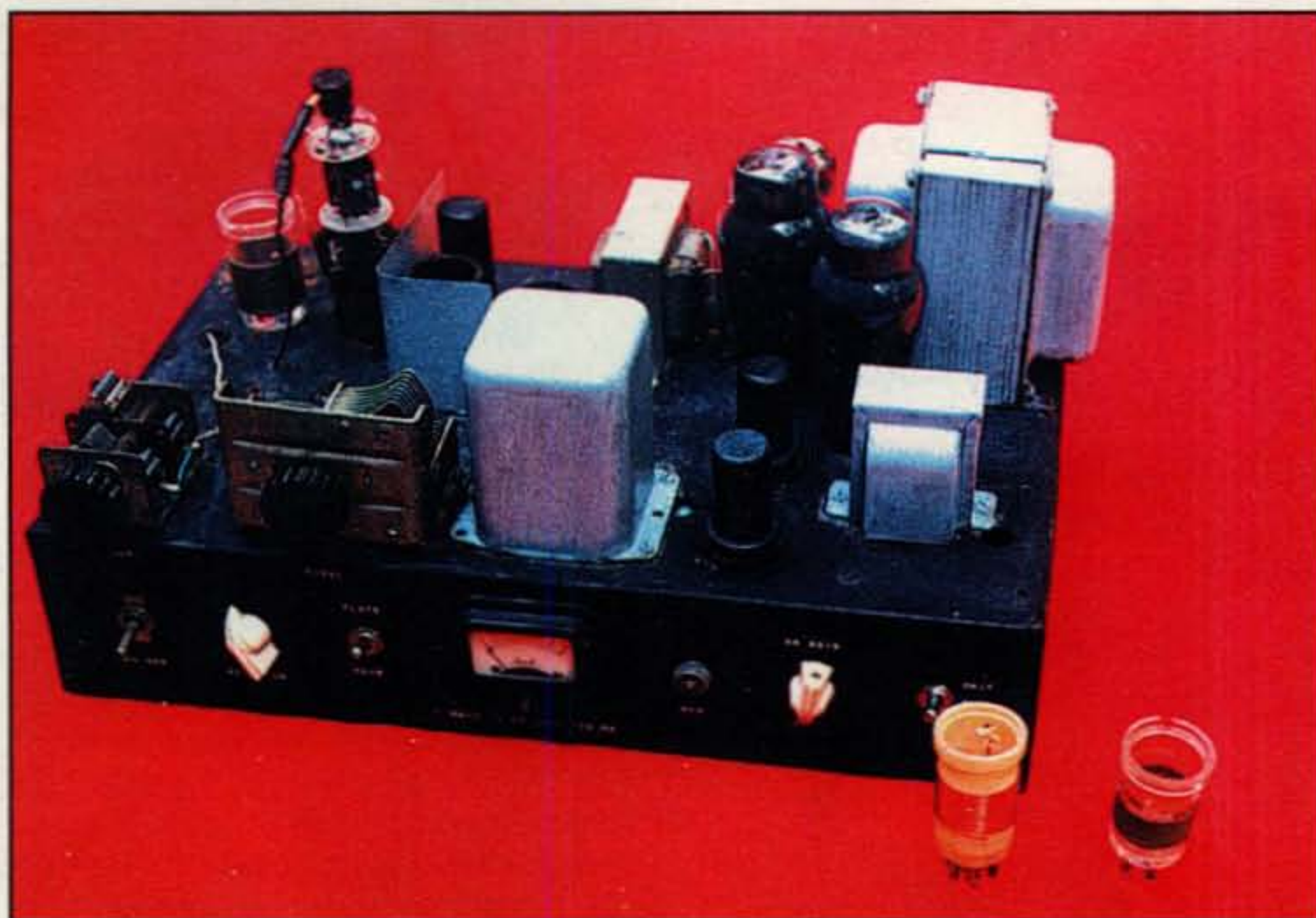
Photo B— A transmitter built by the author in the late 1950s from the innards of an old TV. Using plug-in coils, it put out 40 watts of AM or CW on 40, 80, and 160 meters.
