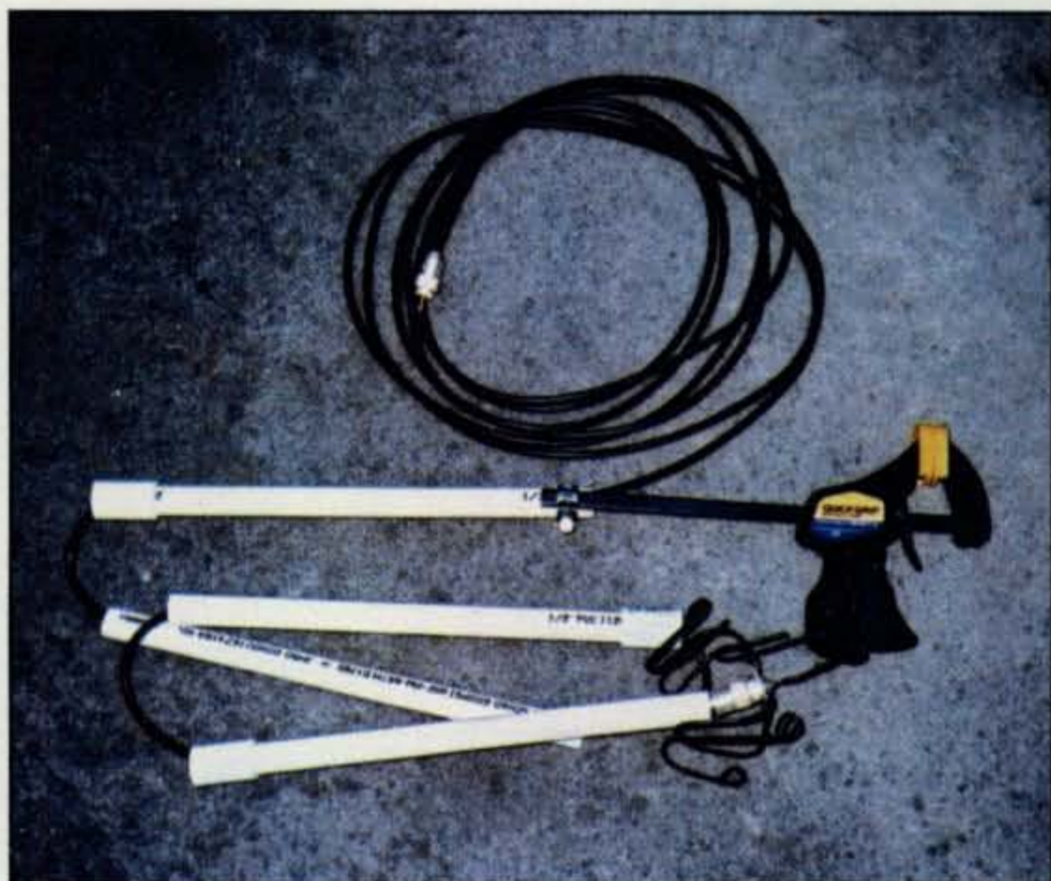
Photo B— The “squishy ground plane” is made of 12-gauge, insulated solid-copper wire and can be carefully crushed or folded into a little ball for transport. Here, half-inch PVC pipe with couplers and a QuickGrip® woodworker’s clamp complete the antenna.
