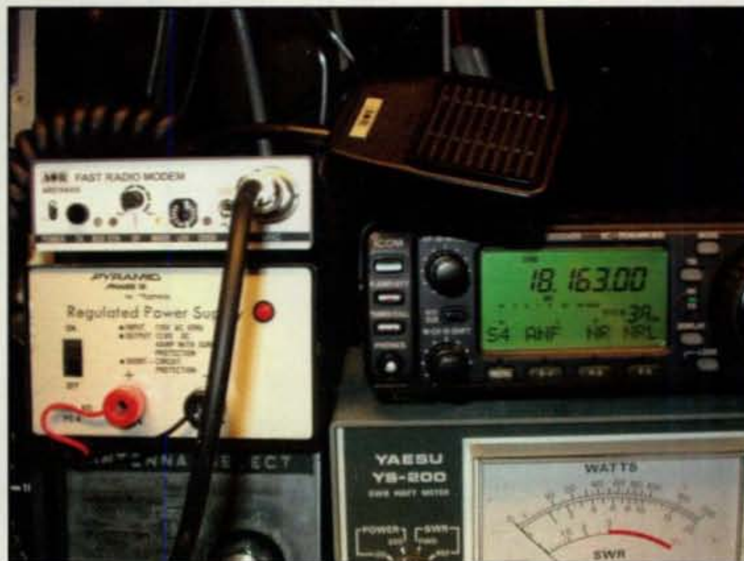
The ARD-9800 Fast Radio Modem hooked up to W2VU's borrowed (from N2IRZ) IC-706, along with the small power supply below for the 9800. It's essential to use a regulated, non-switching supply with the 9800.
