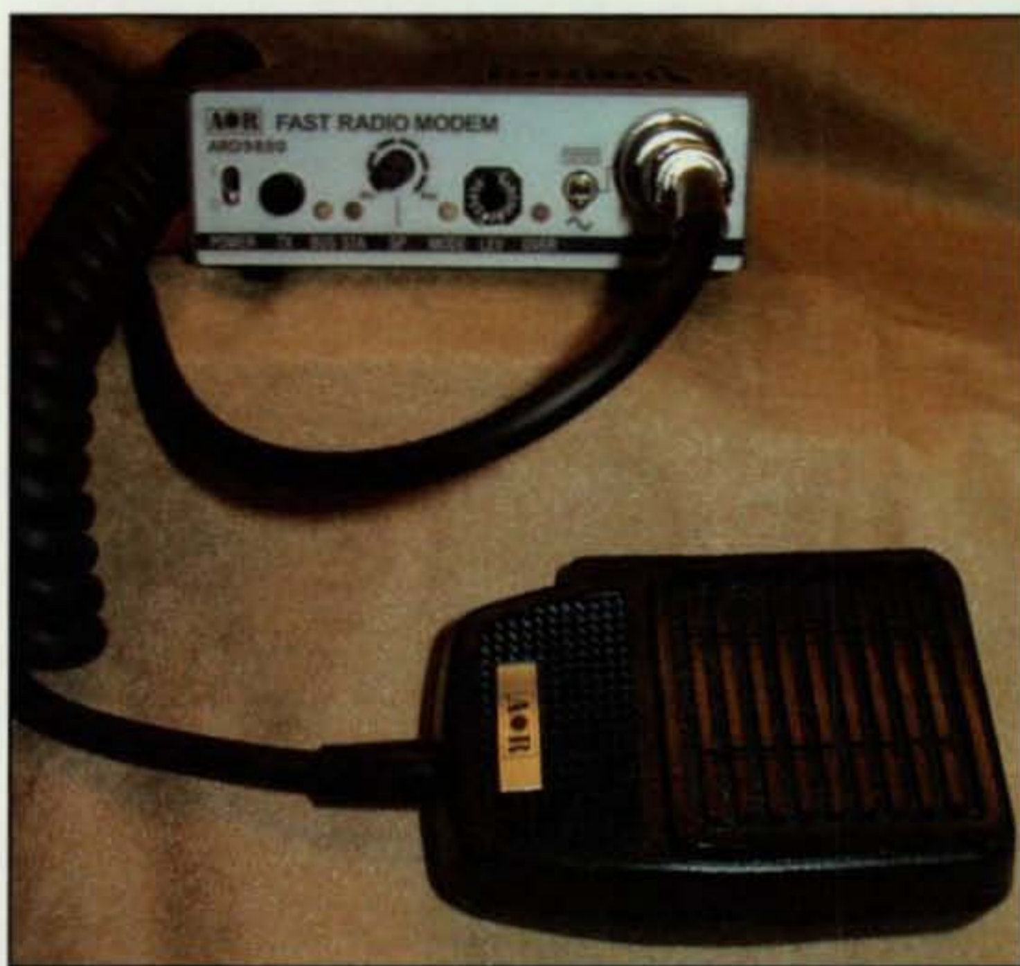
The ARD-9800 Fast Radio Modem from AOR is capable of producing and decoding digital voice, text, and photos. It can be used with virtually any HF SSB transceiver, using the mic in and speaker out connectors. (W2VU photos)
