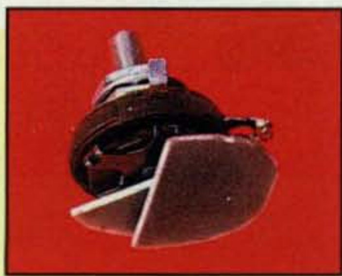
Photo C— A homebrew tuning capacitor made from a potentiometer and two pieces of PC-board material. See text and fig. 3 for details.
