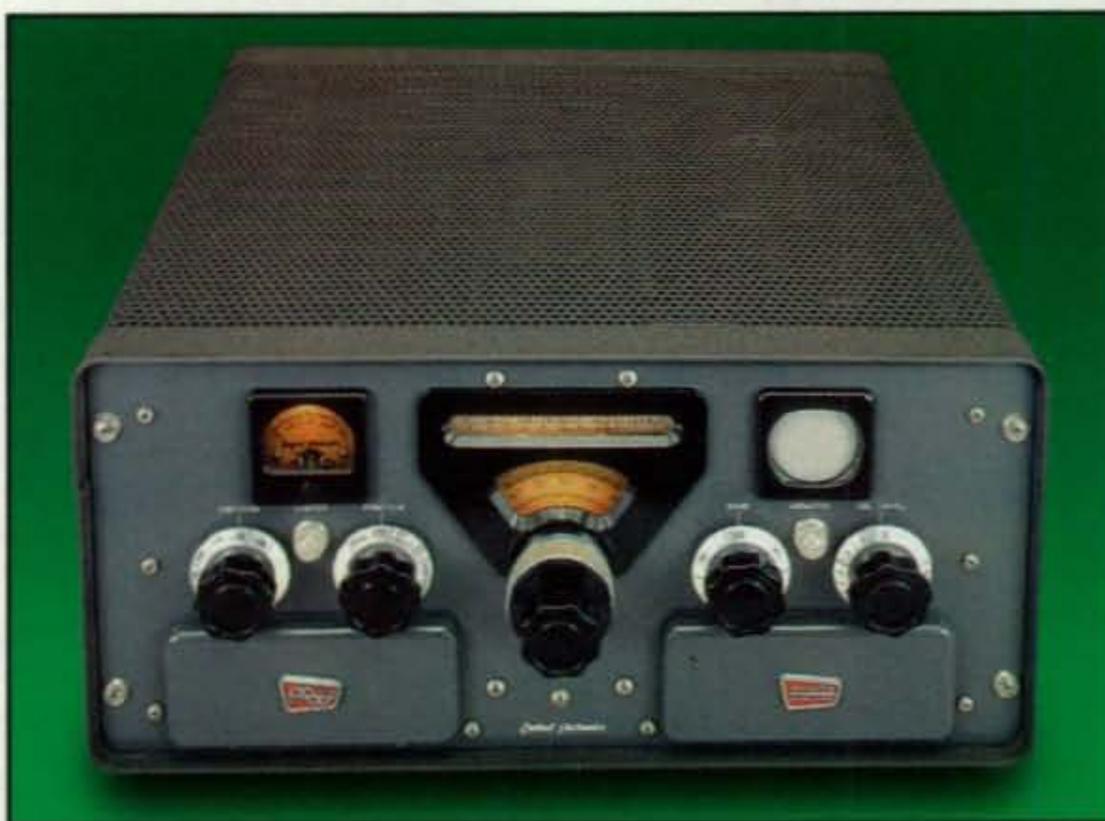
Photo A—The Central Electronics 200V phasing single-sideband transmitter was produced in 1961 and sold for $795. (Photos © Joe Veras, 2004, all rights reserved)
