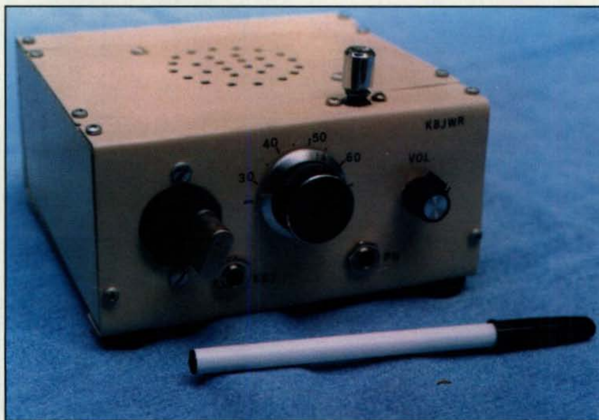
Photo A— The author's Phoenix QRP transceiver, built from the "ashes" of a dead TV set. (Photos by Michael Croke)
