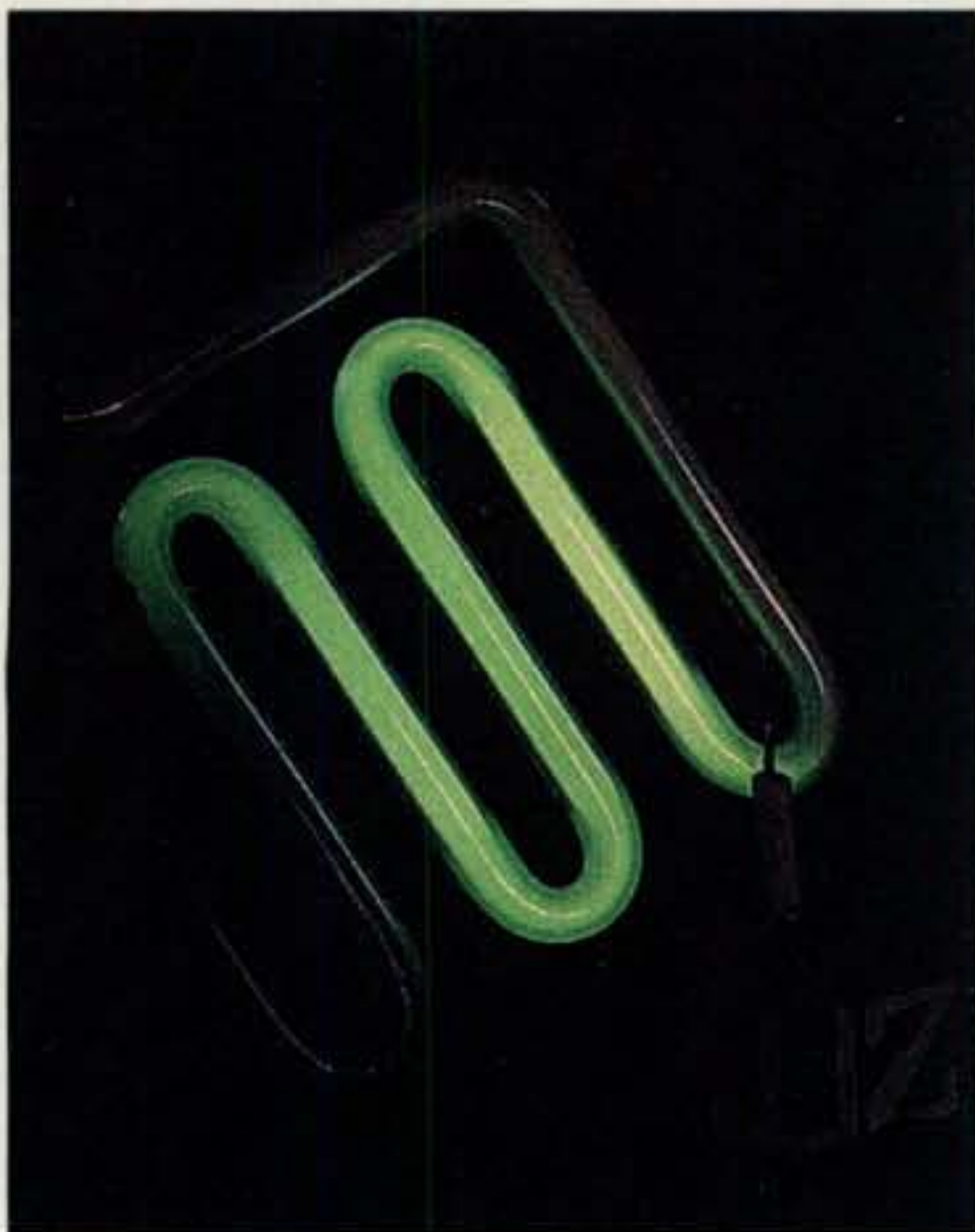
The little Tesla coil can still make a fluorescent tube glow without wires. This "squiggly" fluorescent tube was designed for backlighting some sort of display panel. I found it at a surplus store for five dollars. It has an interesting green color.
