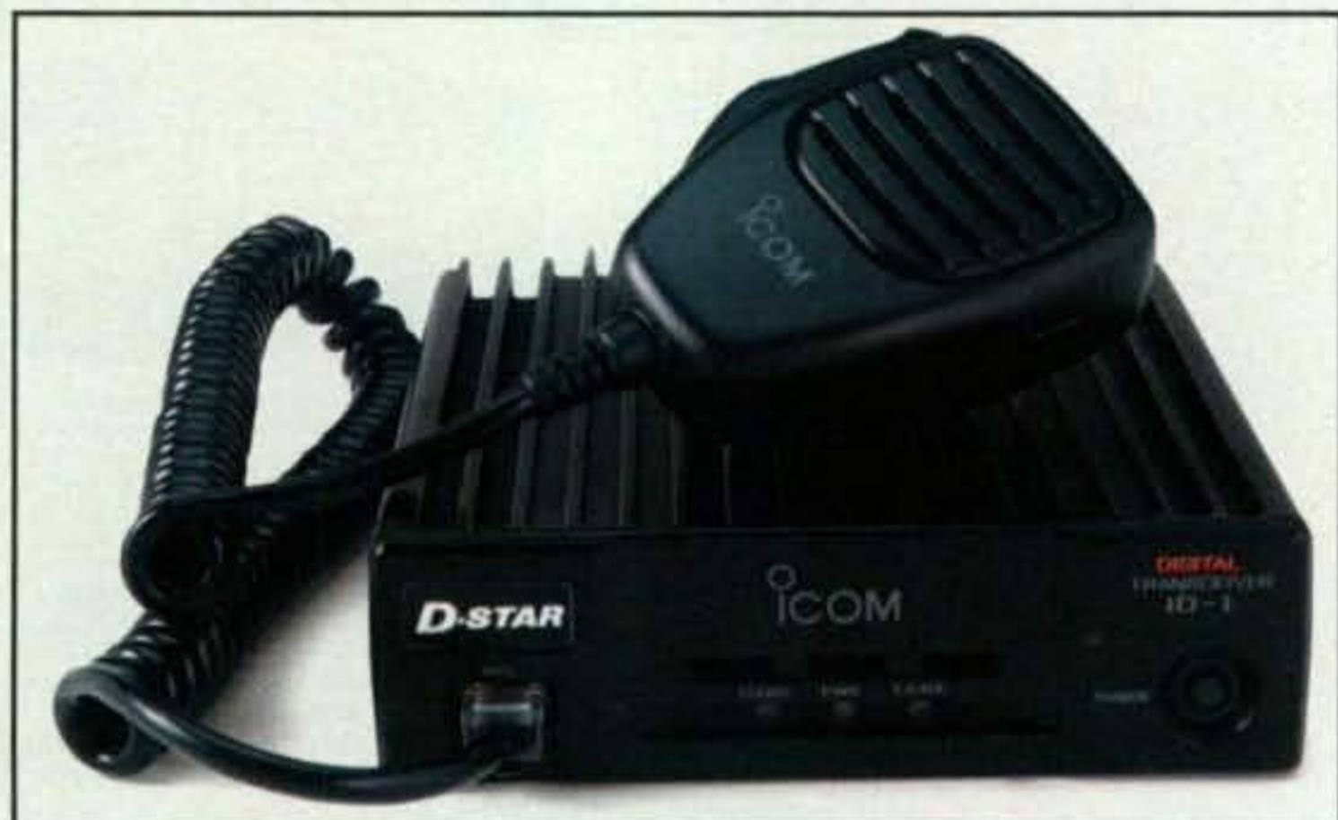
Photo H— Depicted here is ICOM's ID-1 Digital Transceiver, the "wireless" link in its groundbreaking EchoLink over D-STAR system described in the column text. The ID-1 transceiver is an important component of a complete D-STAR system. (Photo courtesy ICOM America)
