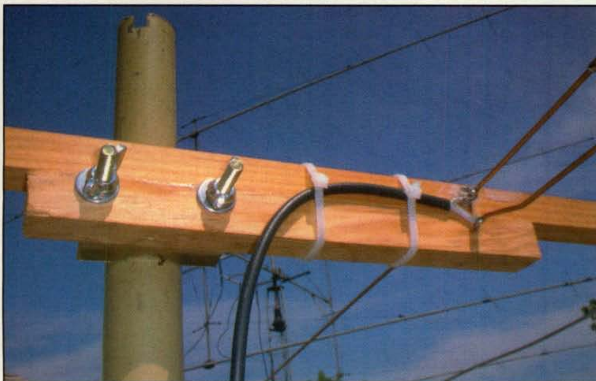
Photo C— The driven element and U-bolt on the 4-element Cheap Yagi.
