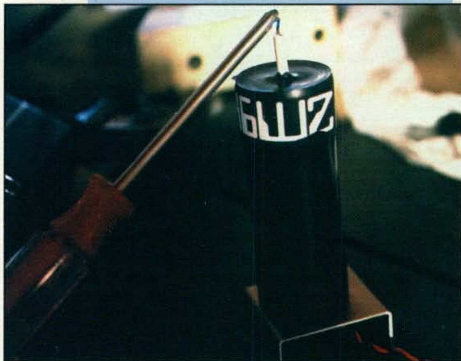
This simple and small Tesla coil was made from an inexpensive kit. Although very tiny, it can still produce a small Jacob's Ladder and it will deliver sparks and arcs if you get something close to the output terminal—including your fingers—so be careful. (Photos by the author)
