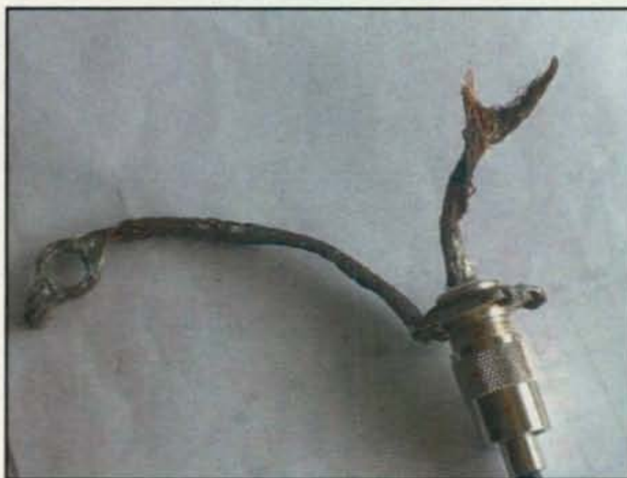
Damage caused by one of the turtles on Europa Island during the TO4E DXpedition. This was not one of those "easy" DXpeditions. (Photo courtesy of Dany, F5CW)
