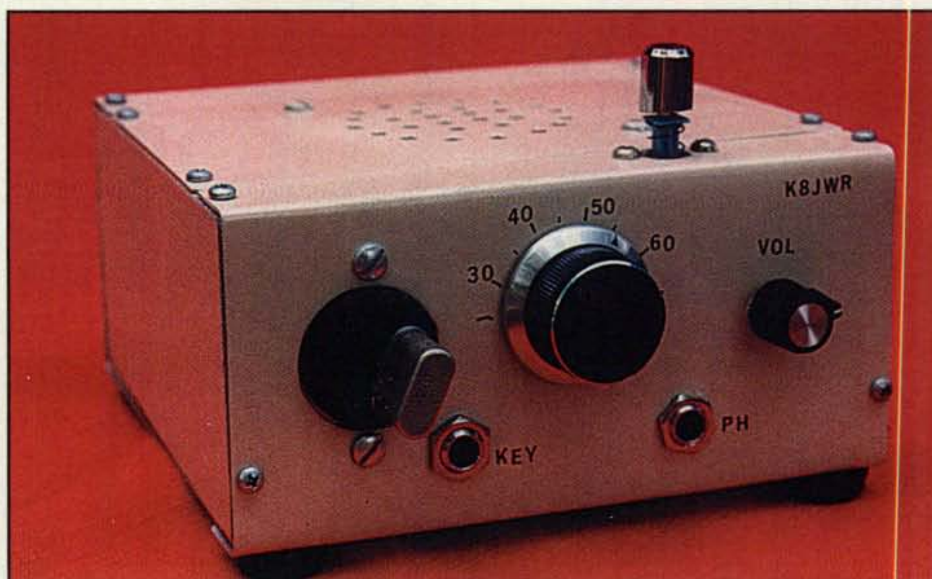
Photo E—The completed Phoenix transceiver. Note that the crystal is in one of four positions in the octal tube socket. Each provides a slight variation in frequency. See text and fig. 10 for details. (Photos by Michael Croke)
