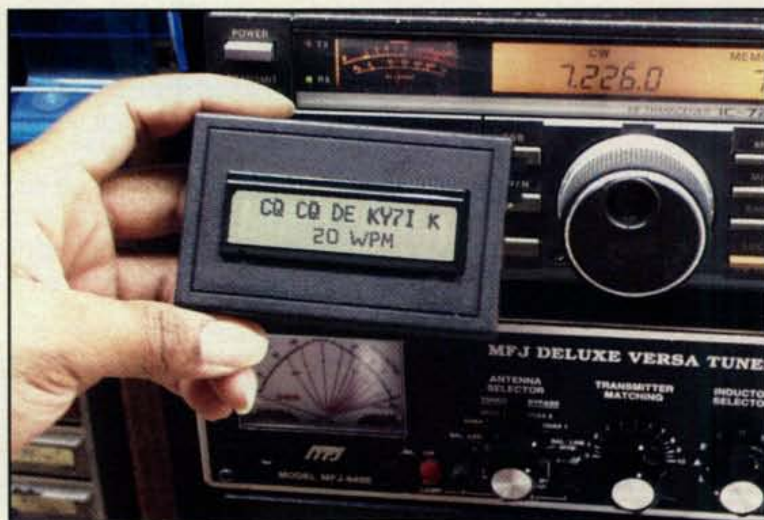
Photo E— If copying medium- or high-speed Morse code is your only handicap, try this MFJ-461 reader. Just place it near your rig's speaker and it displays received Morse on its LCD readout. Use it for a couple of months, and your code sending will also improve. (Photo courtesy MFJ Enterprises)
