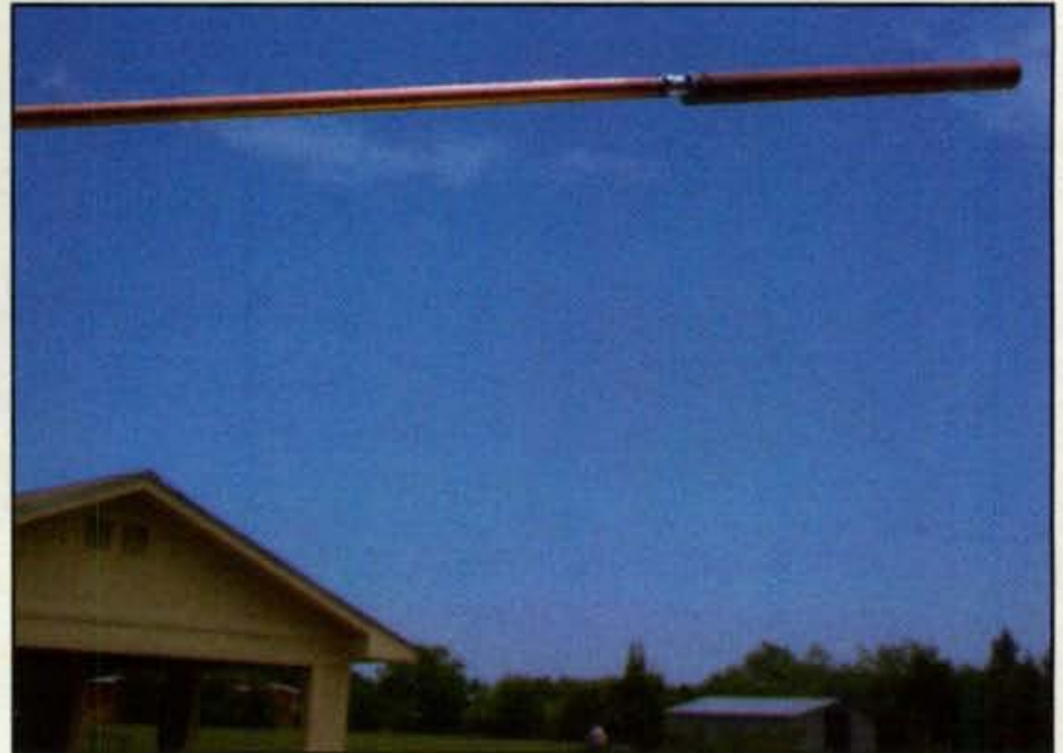
Photo E—Sliding tube on the driven element used in testing.
