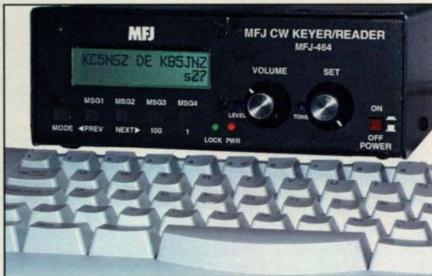
Photo D— Like to join the fun and DX action on CW, but have difficulty copying or sending code? Need help reading fast-sent Morse code? Check out the new MFJ-464 combination Morse code reader and programmable memory keyer from MFJ Enterprises. It connects to the key and earphone sockets of your rig and makes CW a cinch. (Photo courtesy MFJ Enterprises)
