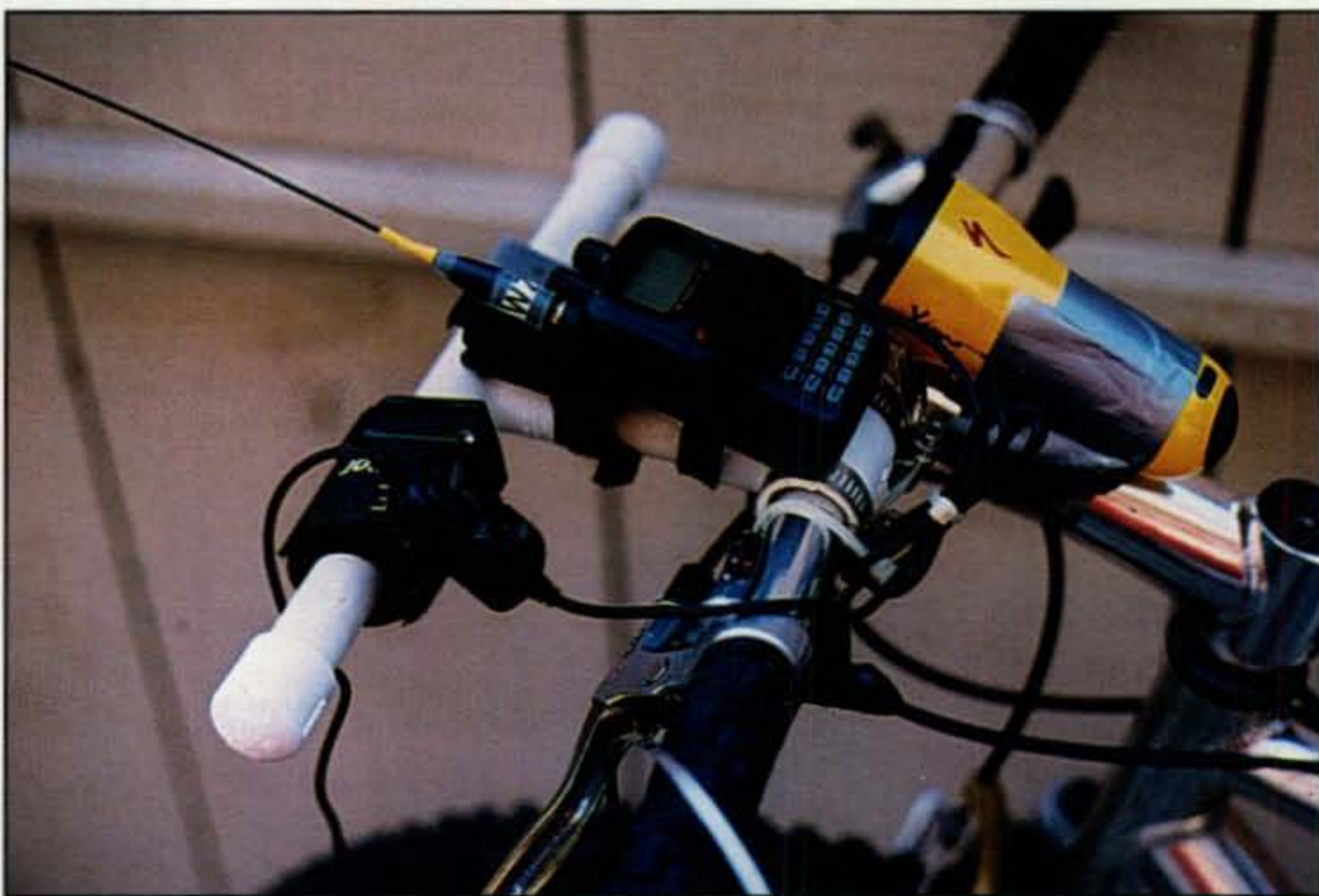
Photo C— The KH6WZ bicycle-mobile station consists of an HT attached to the handlebars with a PVC bracket. Scrap half-inch PVC pipe and parts are used to make the radio/GPS support bracket. Similar, but nicer, handlebar accessories are available at your local bike shop. Not shown is the small GPS unit that clamps on to the right of the HT. Make sure that no part of the setup gets in the way of safe bicycle operation.
