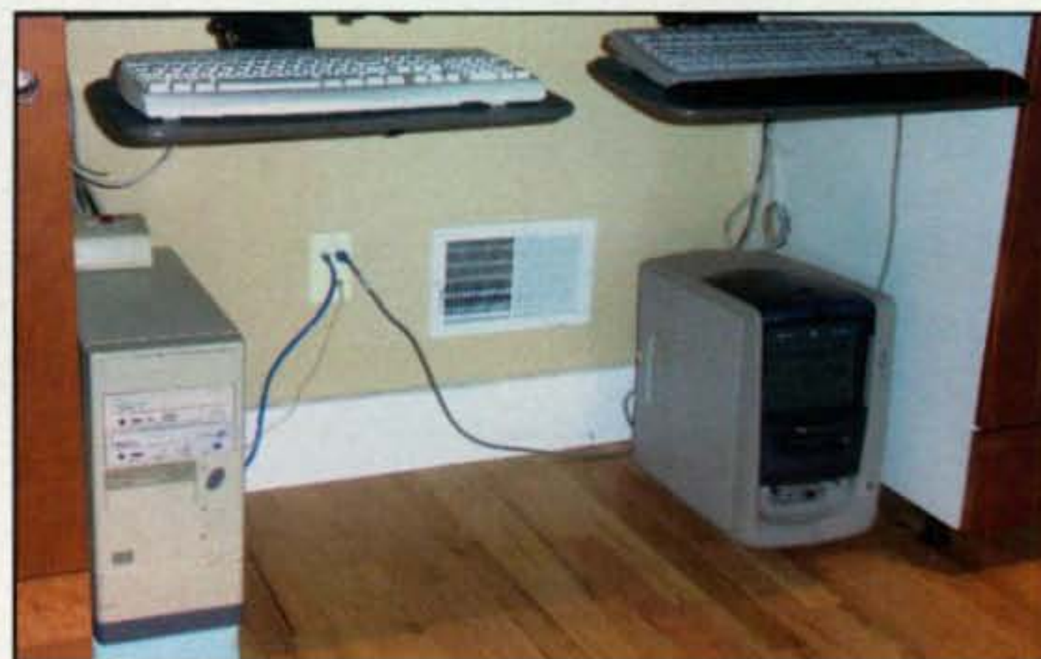
Fig. 5— My main computer setup—one for me, one for the kids. The cabinets hide supplies and printers, and servers for hard-disk storage and other functions are in the cellar. Note the neat look the wall plate provides for both Ethernet connections and a phone jack.
