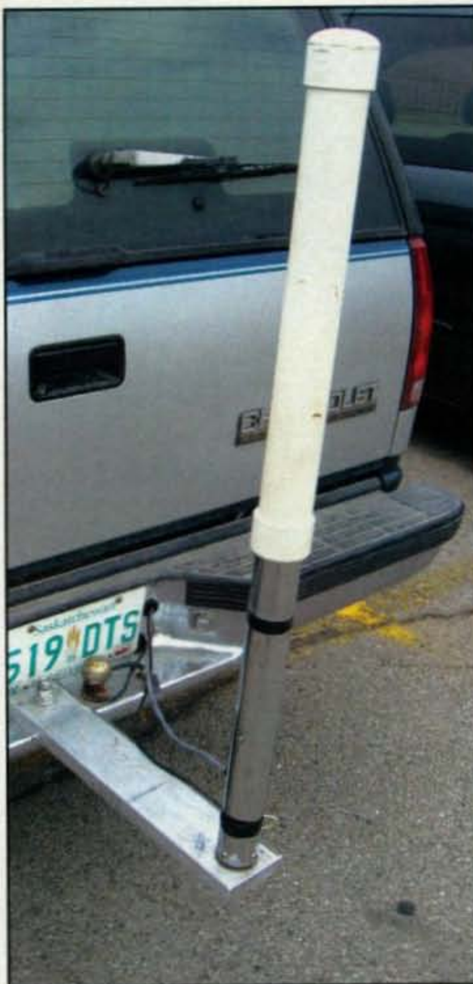
Photo 5– Sturdy is the word for this SUV “screwdriver” antenna mount
