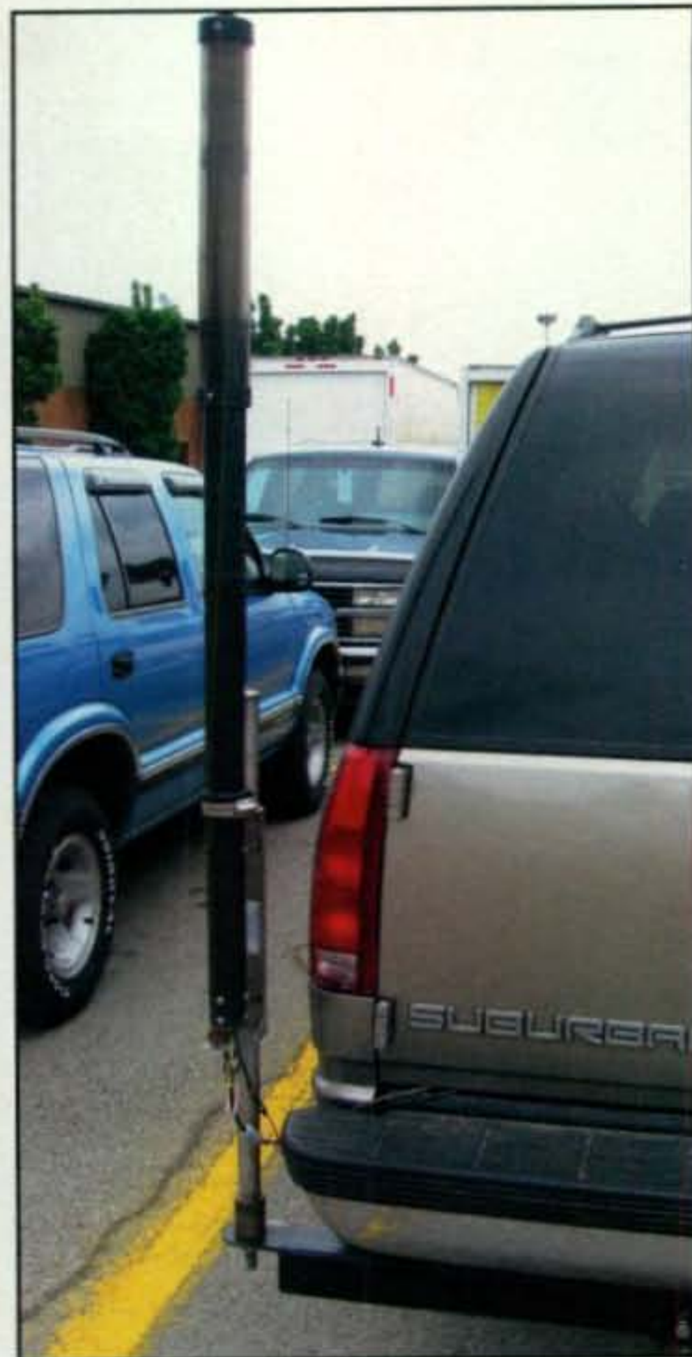
Photo 6– A big antenna requires a strong support system. This one is connected to a trailer hitch.
