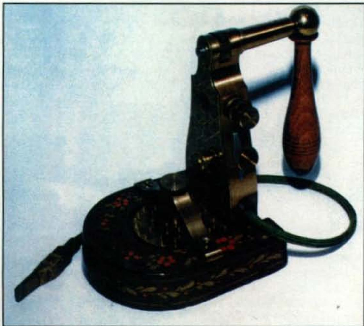
Photo 5—A number of unique items were devised to aid telegraphers with Carpal Tunnel Syndrome, but few are as wild and witty as this incredible Pump Handle Key. You pull down on its handle rather than pushing down on a knob to send Morse code, and it really works. A full key mechanism complete with gap and tension adjustments is mounted in the decorative case. (Photo courtesy K9WDY)
