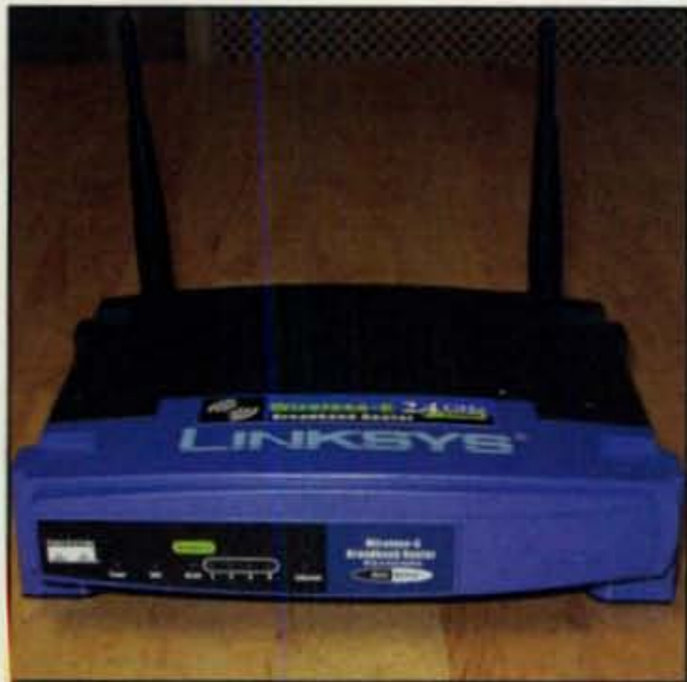
Fig. 6—A wireless router located at the CQ offices. The antennas can (and often must) be oriented to provide a good signal in the right places. It's a trial-and-error process to find the right "sweet spot," reminiscent of adjusting rabbit ears for your television. (Photo by Dick Ross, K2MGA)
