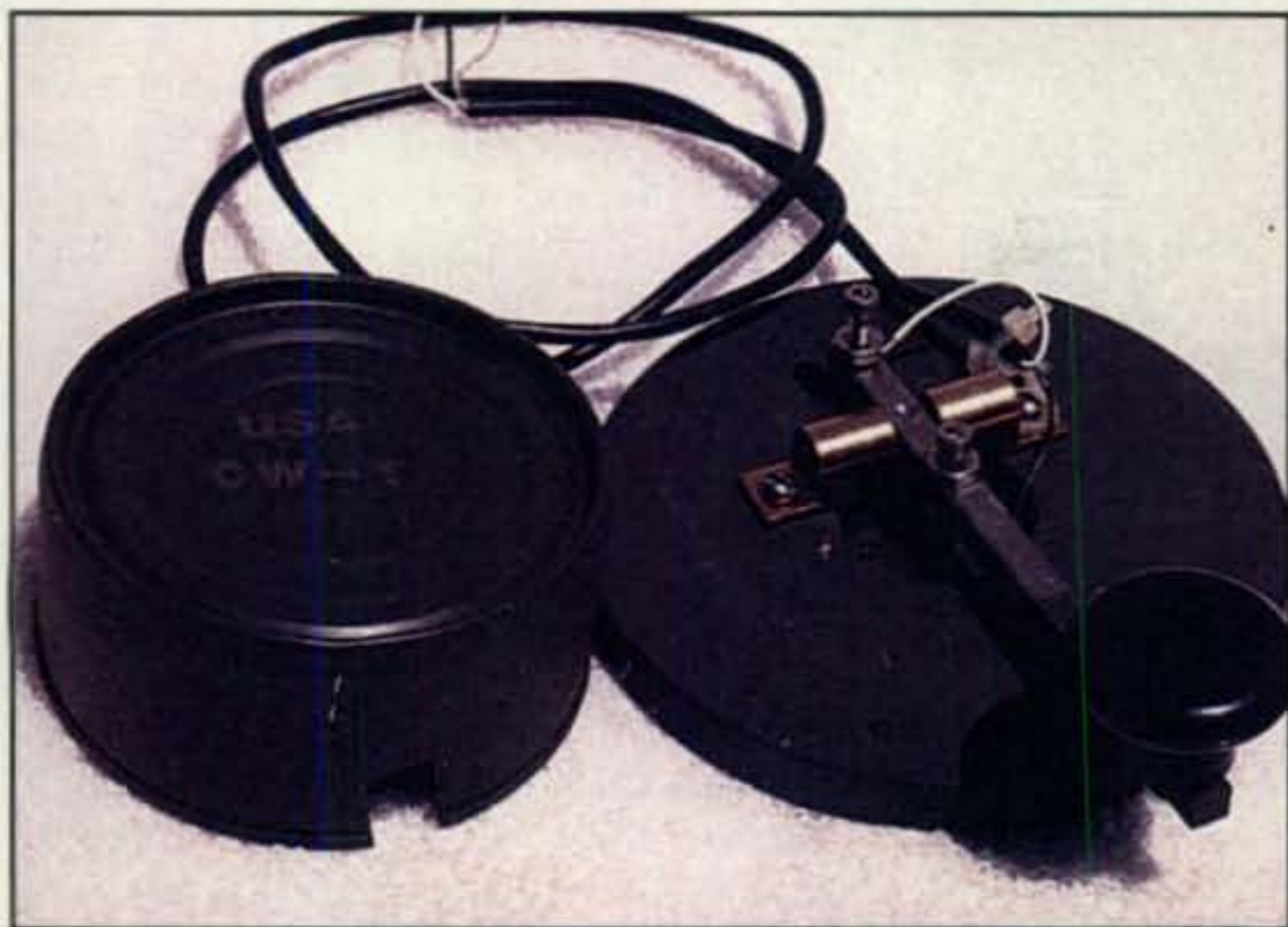
Photo 9— Under the can . . . err, top . . . we find another neat steel stock arm and door-latch pivot point. I have used this key on the air, and I must say it handles very well.
