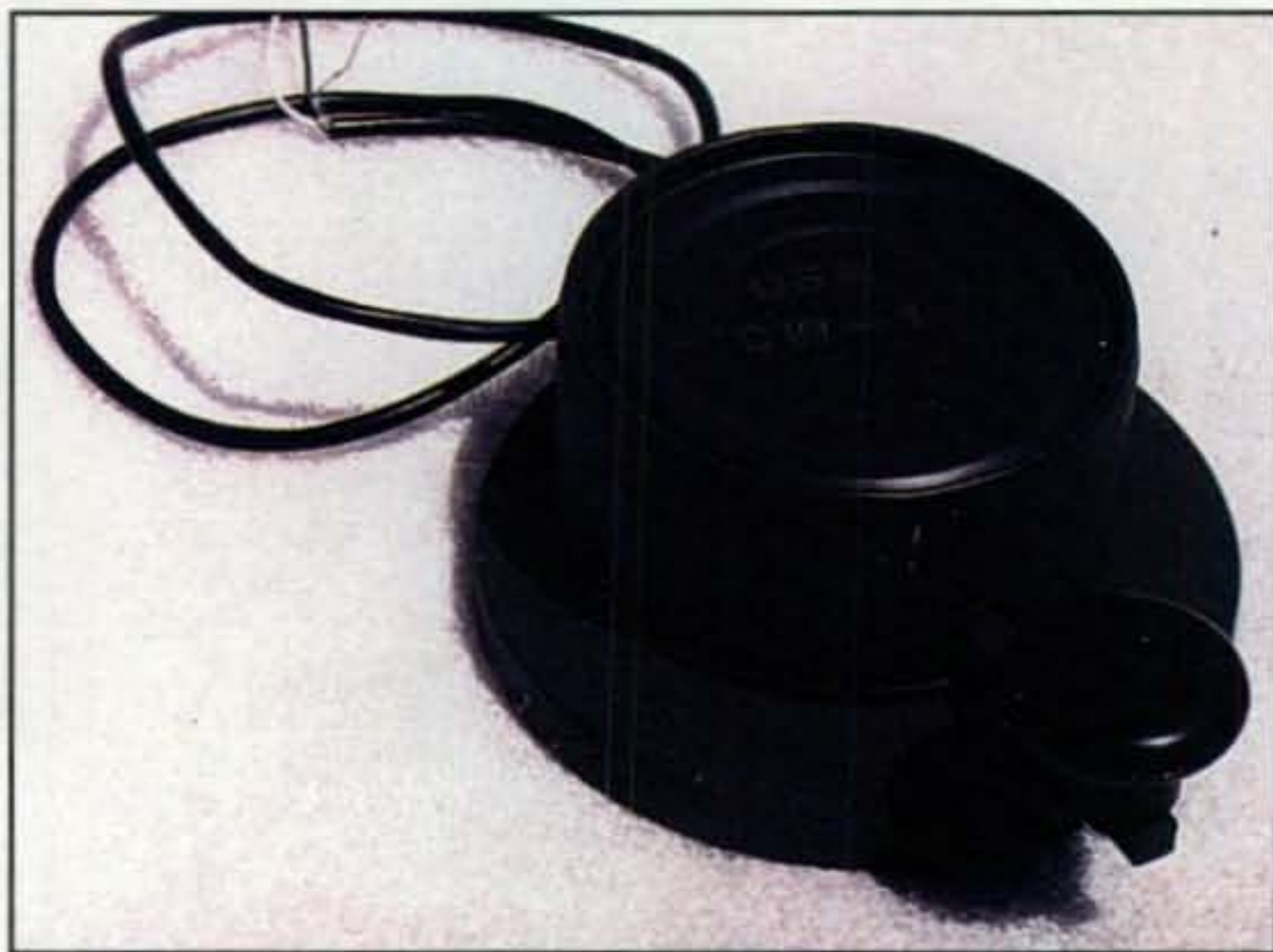
Photo 8— We are unsure if this KB4LJV-homebrewed item is a top-hat key or a can key (the cover is a cat-food can lined with hold-down magnets). Either way, it is a killer! Round keys rock!
