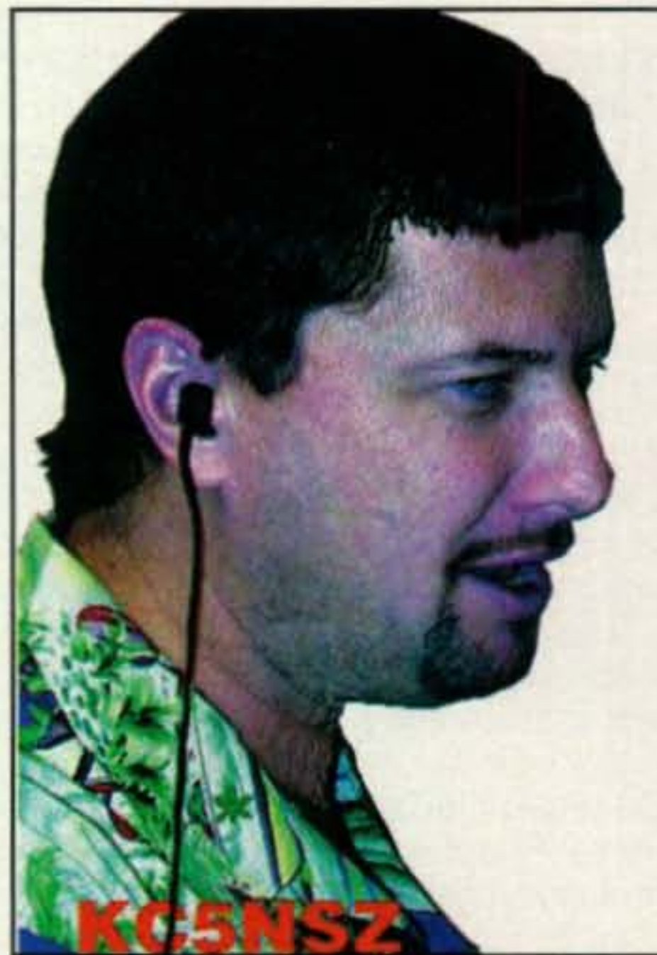
Photo D— The MFJ-283 Ear-Vibration Speaker Microphone is available for ICOM, Kenwood, and Yaesu radios; the speaker and microphone are both integrated into the earpiece. The "vibration pickup microphone" in the earpiece picks up the vibration of your ear bone when you speak. (Photo courtesy of MFJ Enterprises)
