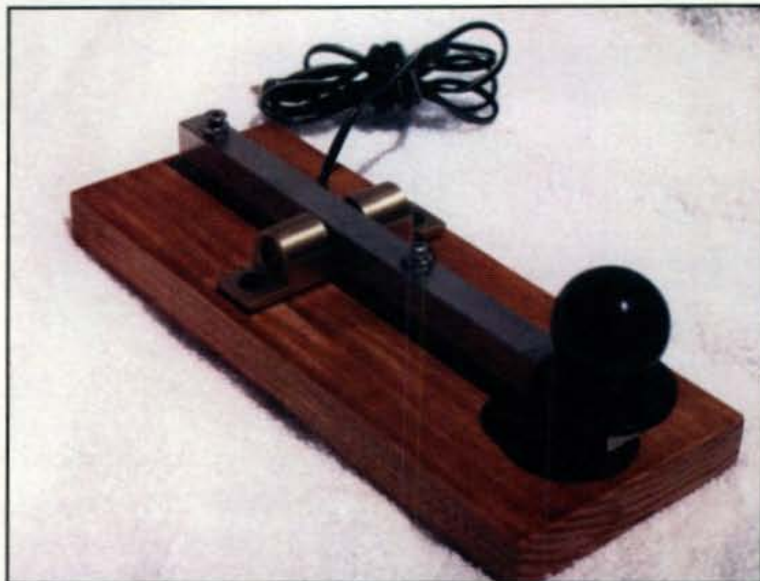
Photo 7— We call this intriguing little item a "door latch key." It was homebrewed by James Butler, KB4LJV, and uses a small door or cabinet latch for its main pivot point. The mating arm is half-inch steel stock fitted with screws for gap and tension adjustments plus a round ceramic cabinet pull with wood skirt for a knob. Clever!
