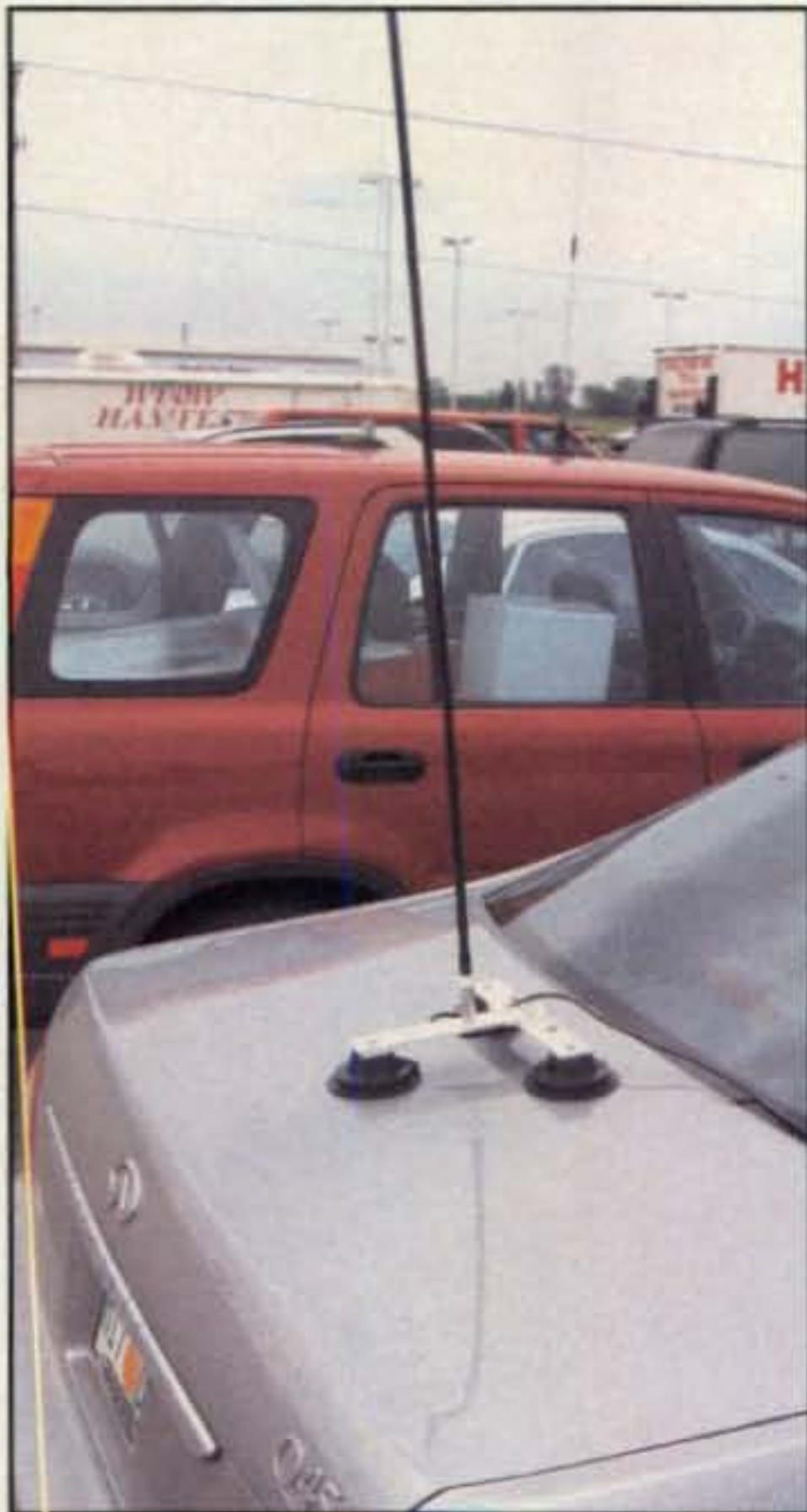
Photo 3— A simple mag-mount and "stick" antenna can get the job done!
