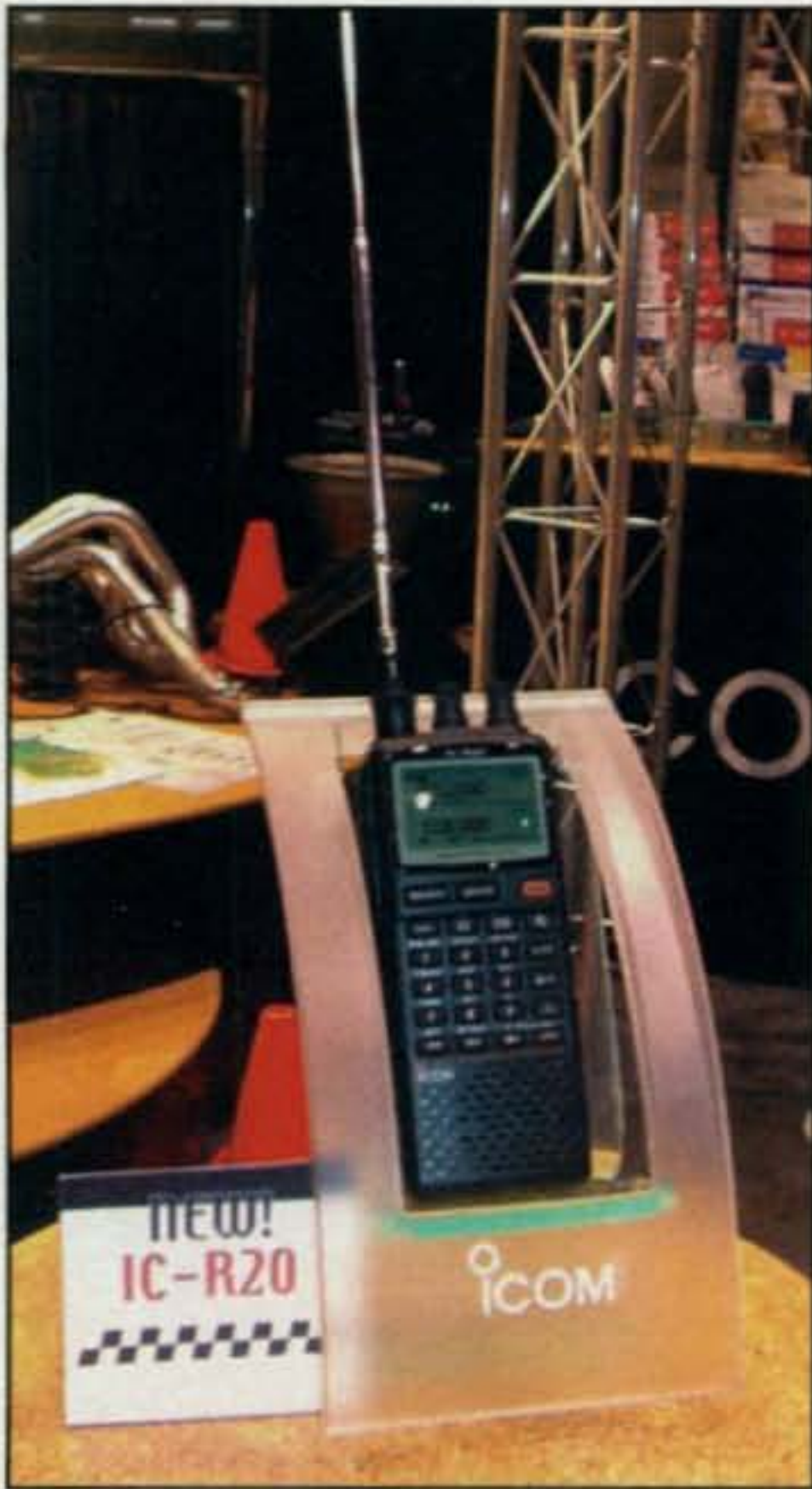
ICOM's new IC-R20 handheld receiver covers an amazing range of 150 kHz to 3305 MHz and even has a built-in four-hour digital recorder.
