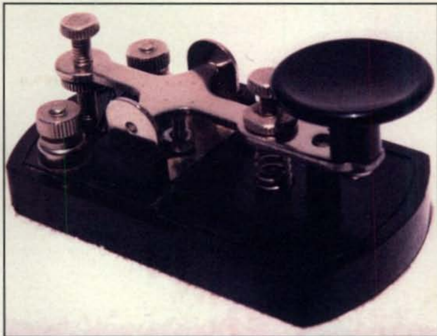
Photo 10— KB4LJV made this neat little treat from an inexpensive MFJ hand key. He cut the arm to the length of the base, moved the knob forward on the arm, and emerged with a clever QRP key for toss-'n-go use.
