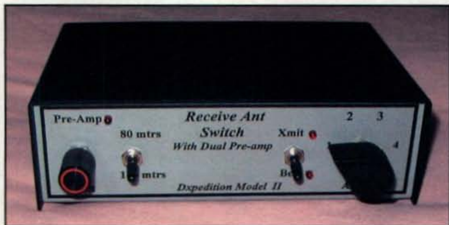
Photo G— Gary Nichols, KD9SV, and Radioware have announced a new version of their popular DXpedition Model Front End Saver (FES) with dual band 80/160-meter pre-amp. Using proven variable gain preamp and FES design, the Mark II fills the gap with radios without a separate receive antenna input. (Photo courtesy Radioware)
