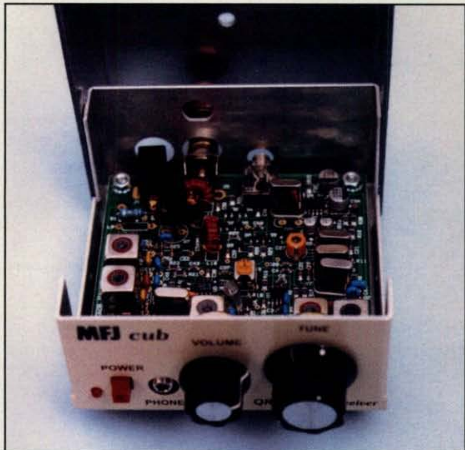
Photo B— The MFJ Cub QRP transceiver with its top cover raised for study. All of those tiny surface-mount parts you see are pre-installed on the PC board. You just install the “big components.” This little monobander is available in 80-, 40-, 30-, 20-, 17-, and 15-meter versions and tunes an approximate 50-kHz range on a selected band. Output is 2 watts standard, 4 watts with optional transistor.
