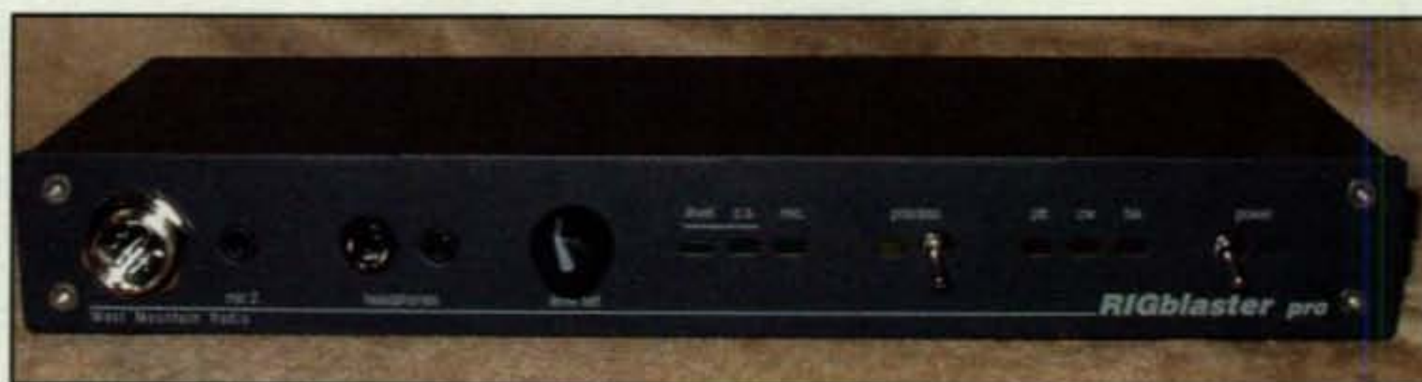
Photo 1—The front panel of the RIGblaster Pro has only three controls ... but that's all it needs.
