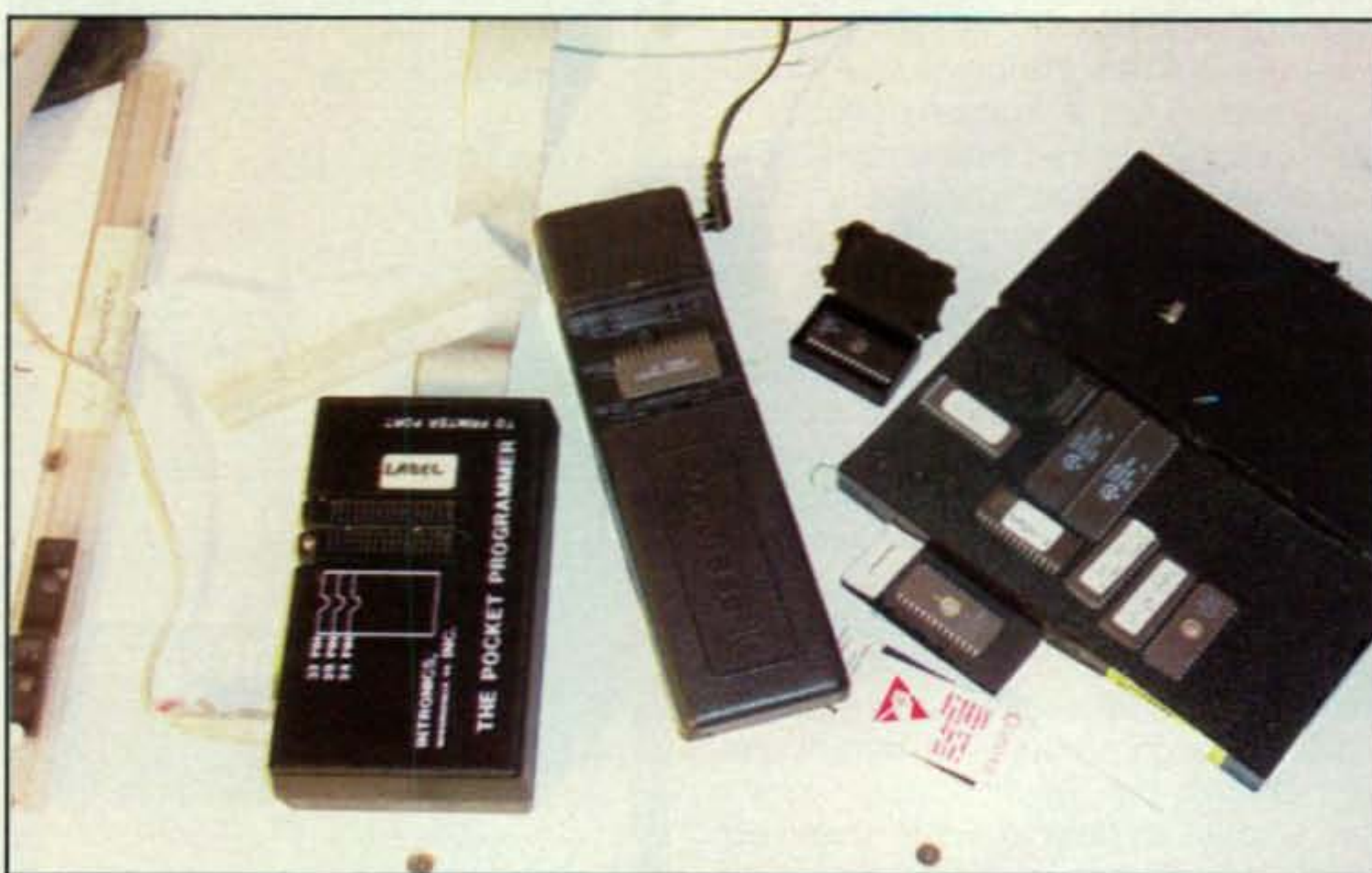
Fig. 5— My Intronics pocket programmer, still going strong after 15 years, next to an EPROM eraser and a few EPROMs. EPROMs are static-sensitive, so always store and handle them correctly.
