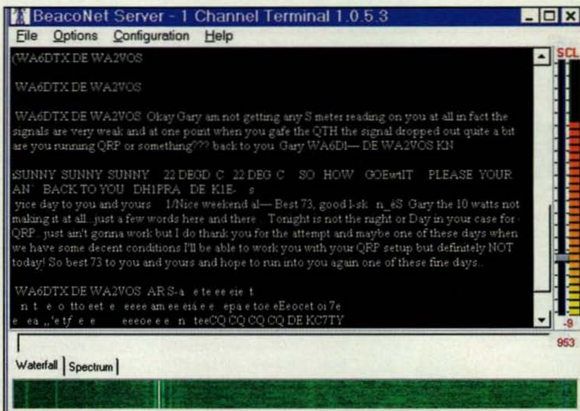
Fig. 1— Typical BeaconServer 1 (BS1) 14.070-MHz PSK-31 computer screen as text is being received and "read" in voice via CoolSpeech speech synthesis software.
