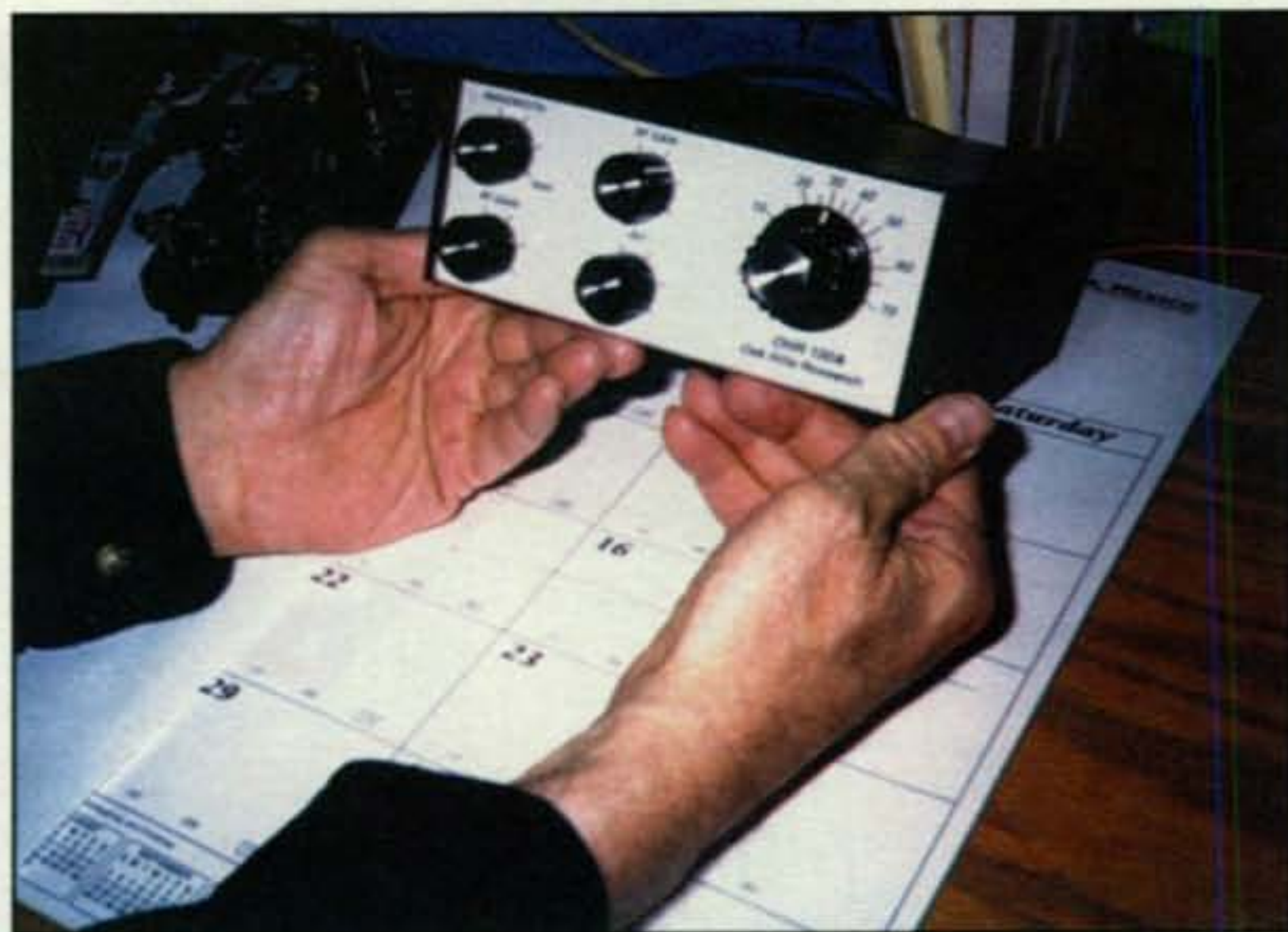
Photo A—The Oak Hills Research 100A QRP kit measures 2.5"H x 6"W x 6"D and pumps out a clean 5-watt signal. The monoband unit tunes an approximate 70-kHz range of 40, 30, 20, or 15 meters, and is generally considered an "intermediate level" project. The transceiver shown belongs to Tom, K4VIZ, and was photographed by Ed, N4ZUM.
