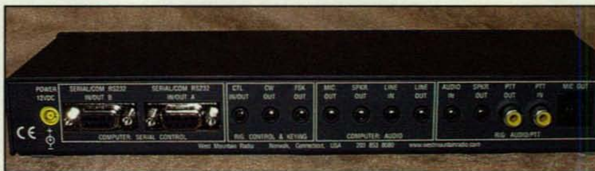
Photo 4- The rear panel of the RIGblaster pro is busy but clearly labeled.
