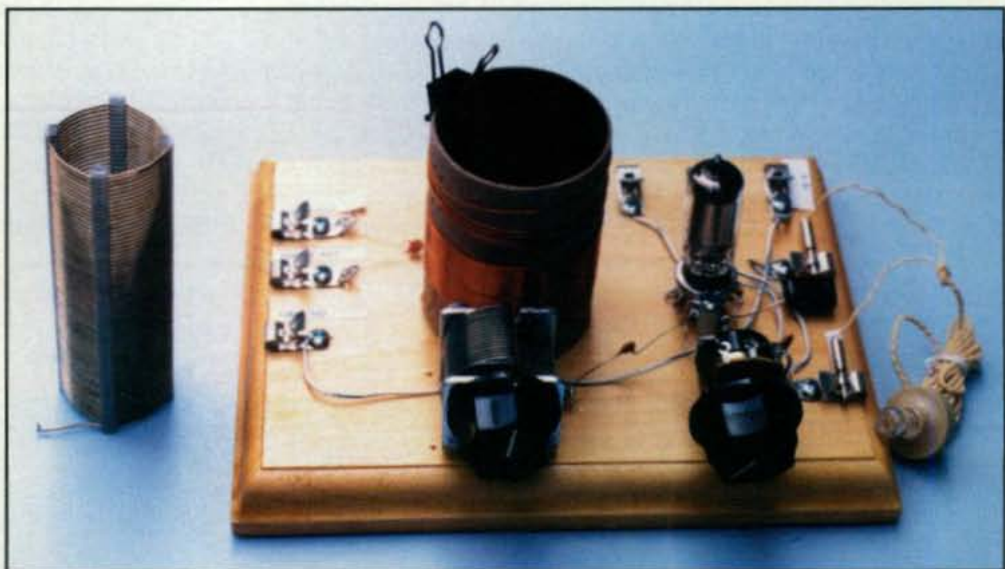
Photo E— The completed Bordon Radio Company One Tuber—well, almost. I was still dinking with coil turns for shortwave reception when shooting this photo. Note the cool decoupage plaque-type base! (Details in text.)
