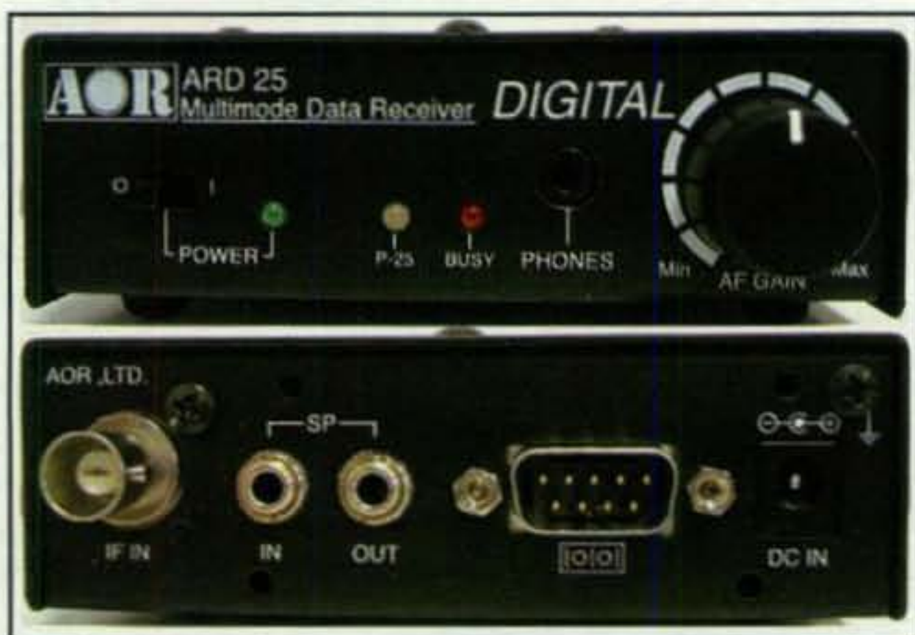
Photo D— AOR has created the ARD25 Multimode Data Receiver, an APCO25 Digital to Analog Conversion Unit, for use with receivers that have a 10.7-MHz IF output. The adapter processes the 10.7-MHz signal, converts the digital transmission, and sends it to the internal speaker or your station speaker. (Photo from the AOR USA website)
