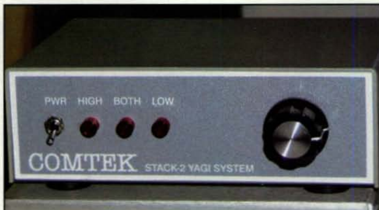
Photo E— One of Comtek's newest products is the STACK-2 2-High Stack Switch for tribanders, log periodics, or monobanders from 40 to 10 meters. You simply run two equal lengths of 50-ohm coax from the STACK-2 to each antenna and a three-conductor control line to enjoy increased performance in contests or chasing DX. (Photo from the Comtek website)
