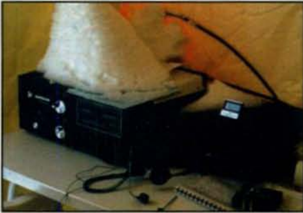
The shelters for the '94 Peter I operation failed to keep the snow from blowing in and covering up the Alpha amp.
