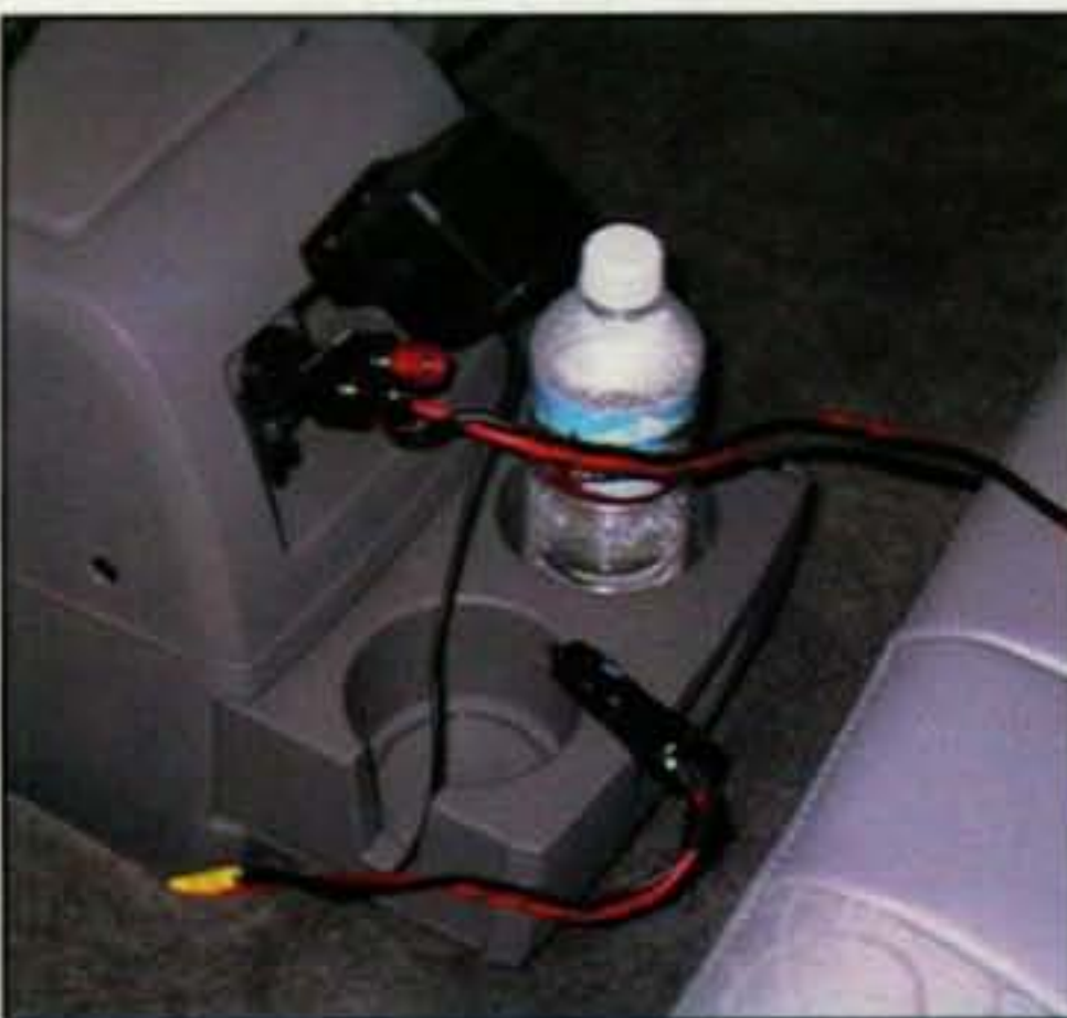
Photo E—This hefty power tap provides enough current to operate “tailgate portable.” Play it safe and check all current ratings prior to using a similar arrangement; specifications vary widely among vehicles.
