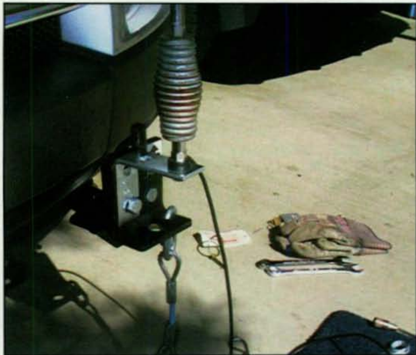
Photo C—Again, a simple design works in mating an antenna mount to the towbar of a small SUV that rides behind an RV. (W6AYJ photo)
