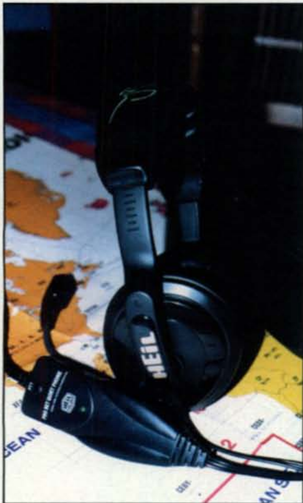
The "Quiet Phone" operates on two AA batteries and includes a boom mic with a famous Heil element (your choice of three elements).
