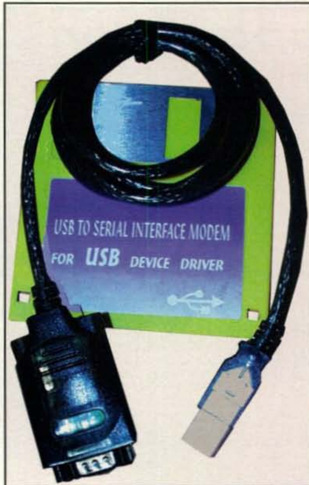
Photo C— The MFJ-5429 RS-232 to USB Adapter is a DB-9 male RS-232 serial port to USB 1.1 port adapter cable. You can use this handy gadget to connect serial port devices to a computer with no serial ports. (Photo courtesy MFJ Enterprises)
