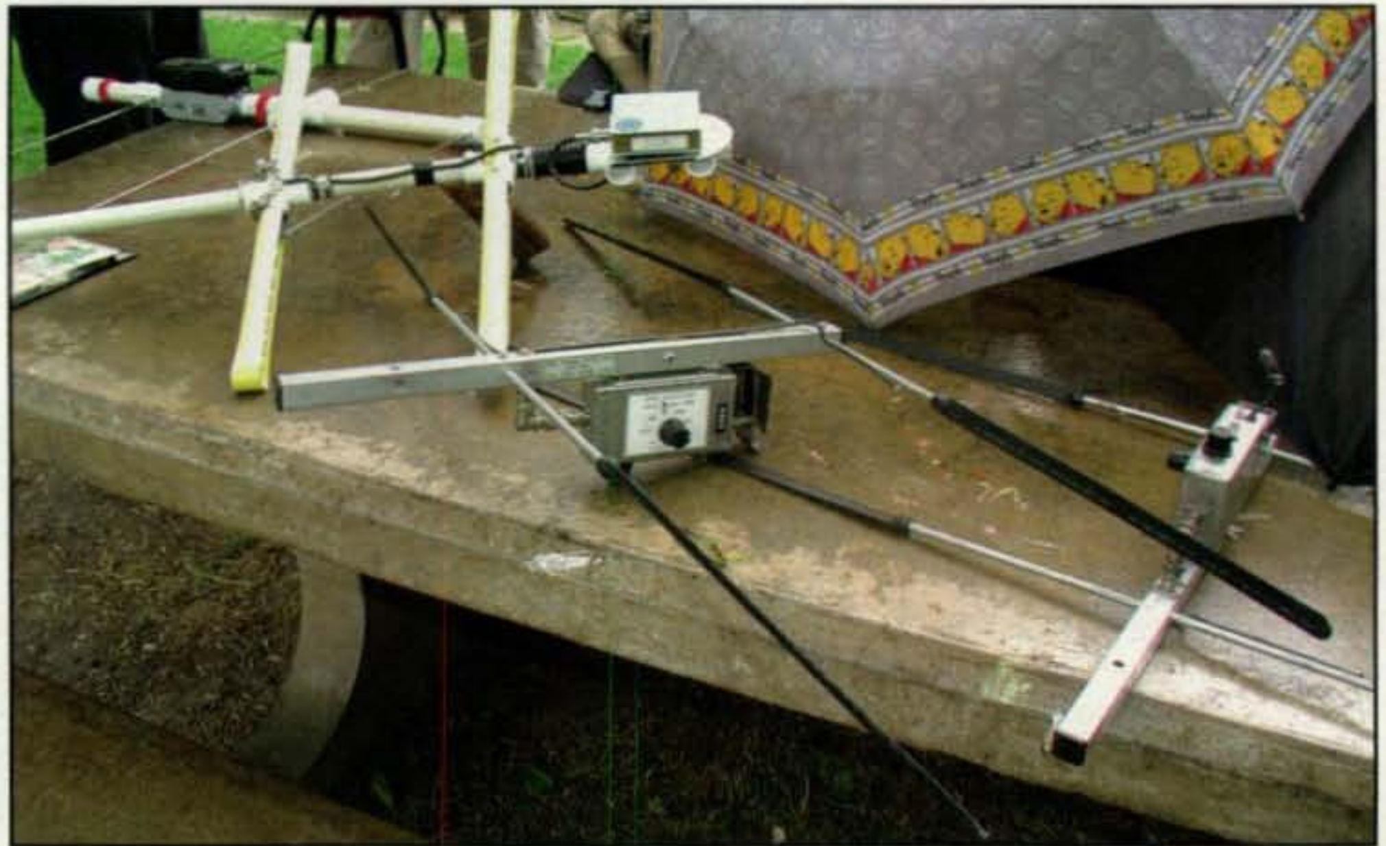
Photo 6— Here is some typical 2-meter ARDF gear (left to right): 3-element Yagi with attenuator and HT; 3-element tape-measure Yagi (elements folded) with VK3YNG Sniffer; 2-element Rod Graham Electronics HB9CV-style beam; and RX-1 2M ARDF receiver.
