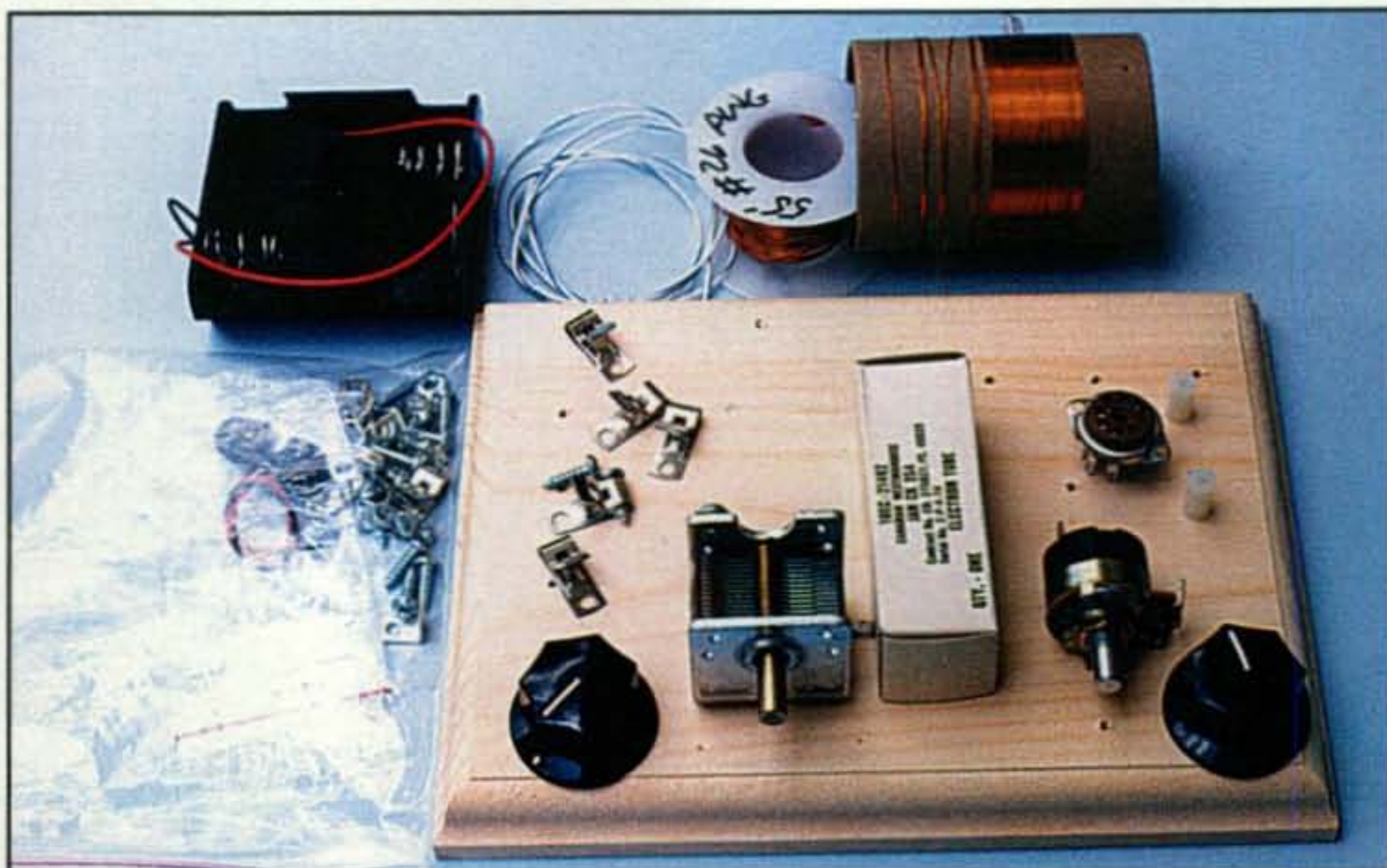
Photo D— The Bordon Radio Company One Tuber radio kit as received and unpacked prior to assembly, although I was overly impatient to start winding the coil before shooting this photo! Note pre-drilled holes to ensure quick success. Bordon also has some neat crystal set kits. Check them out at < www.xtalm.com >.
