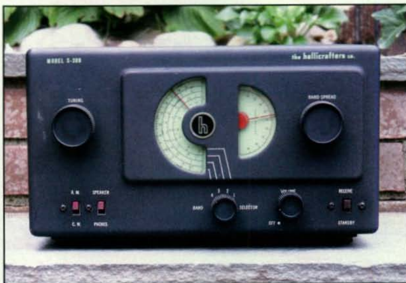
Photo A—The Hallicrafters S-38 receiver, a gem from the days of yesteryear. The S-38B, shown above, sported five tubes, four bands, and a black-wrinkle finish. Ah . . . the glow of the green dial. (Owned and photographed by Gail, K2RED)
