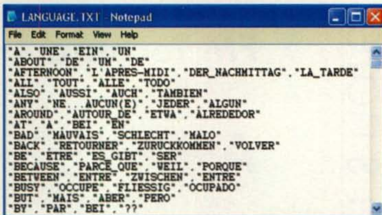
Fig. 5— The language text file can be edited or one can add languages/words to the program with a text editor.
