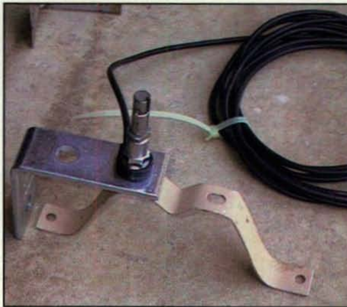
Photo B—This simple bracket can attach to the spare tire mount of a Honda CRV. (K6AWO photo)
