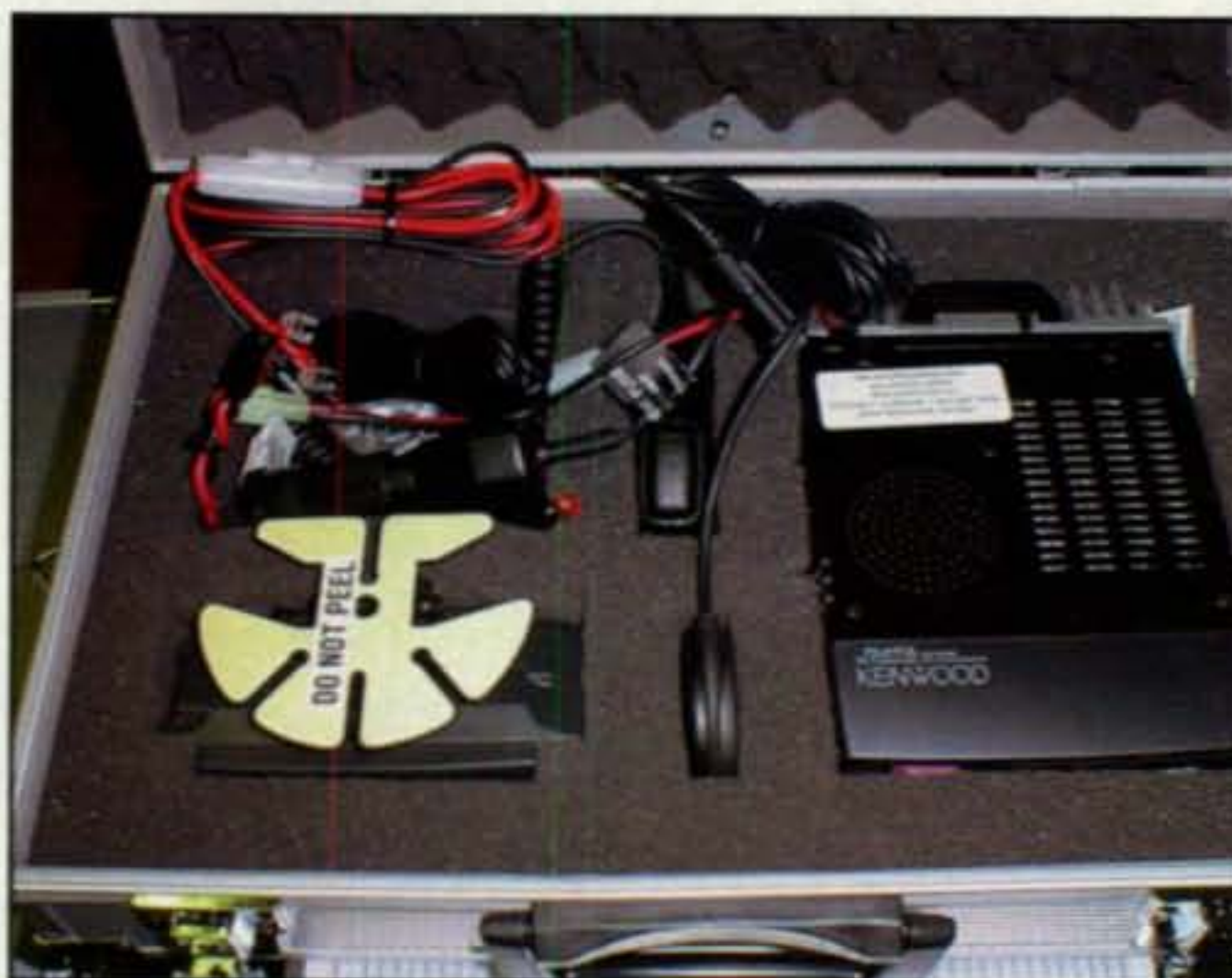
APRS unit packed to be shipped to the Salvation Army in Tampa. The kit's contents: the Kenwood TM-D700 main body on the right; in the center, the microphone on top and Garmin GPS 18PC GPS receiver below; on the left, power/interface cables and the D700 control head and mount. (Photo by Thomas Webb, WA9AFM)
