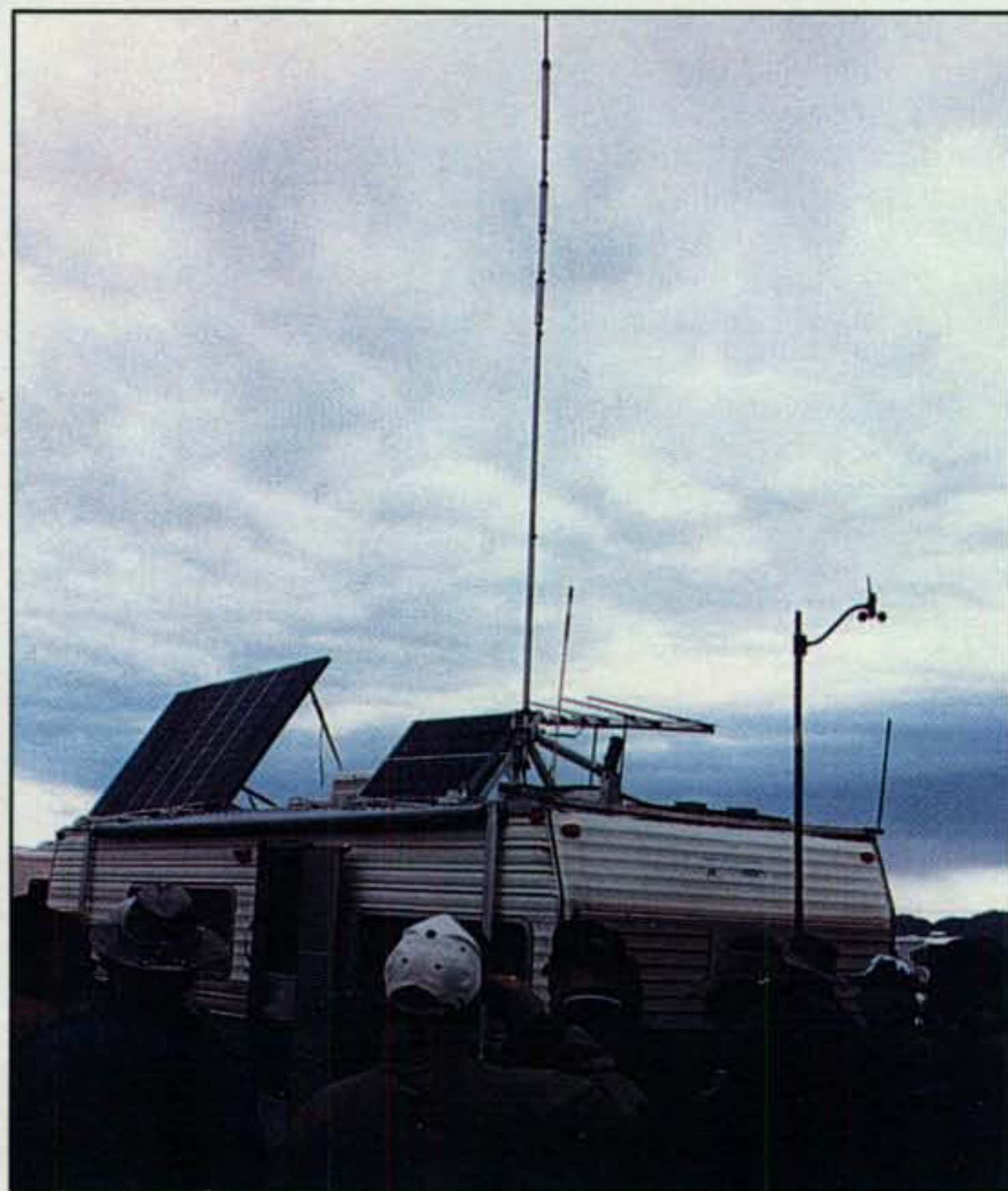
Photo D— Show-and-tell sessions included one on ways of using satellite TV antenna actuators to raise and lower ham antennas and solar panels, used to recharge RV/camper power systems.
