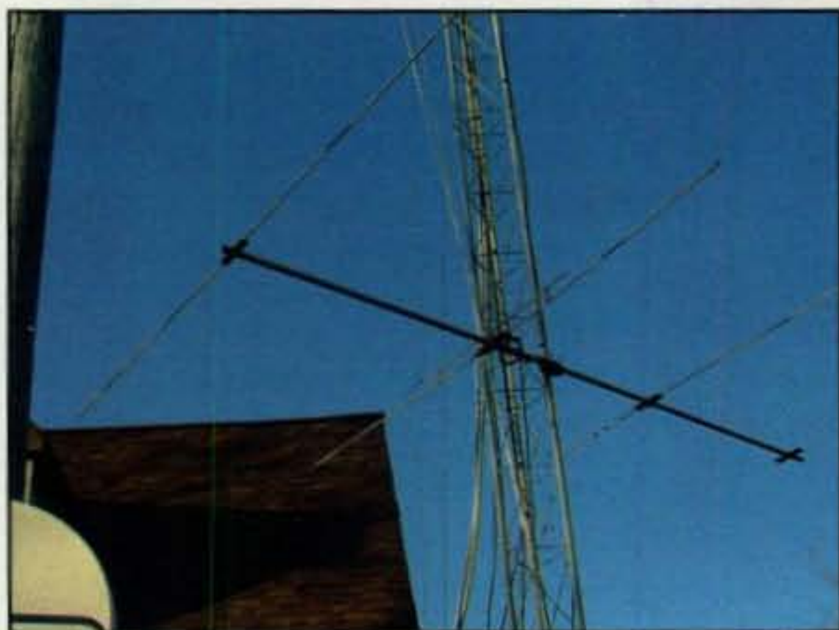
Photo A— A lobotomized 6-meter beam. Notice the missing front element. (Photo courtesy K0CQ)
