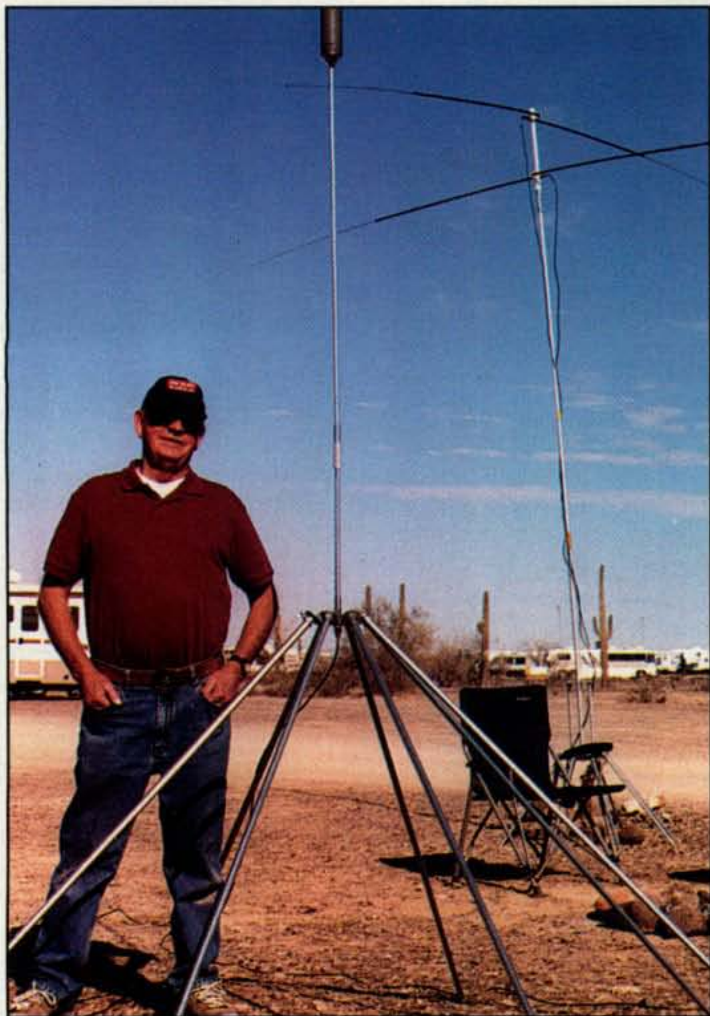
Photo F— Ron Nilson, KD6LA, shows off his "Oct-a-Pod" ground-plane base system for fixed use of mobile HF antennas. The eight legs also serve as radials and create a counterpoise.
