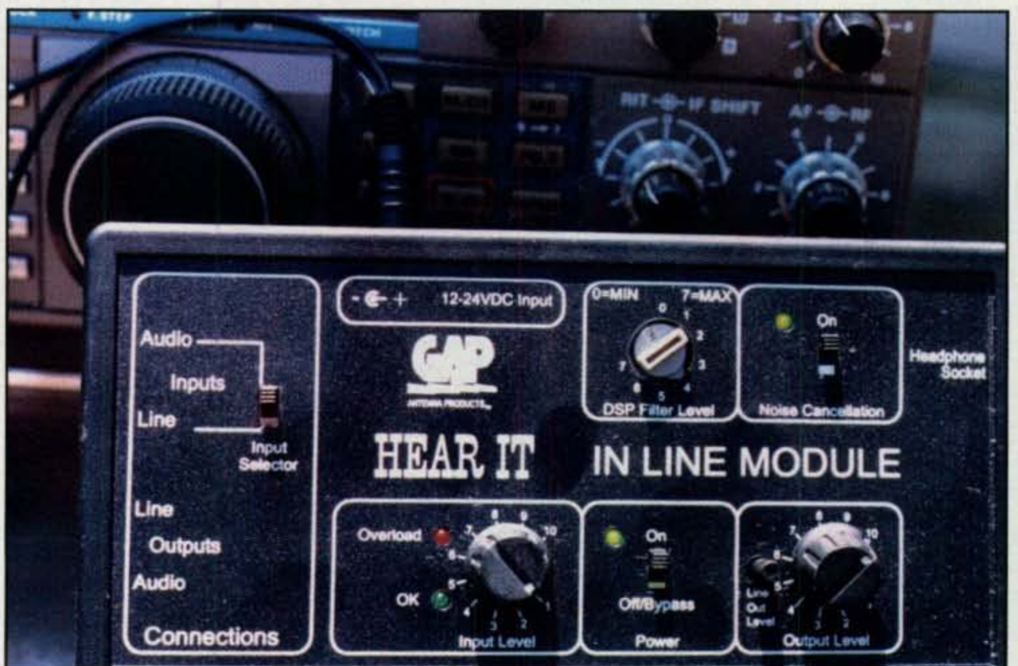
Photo C—The GAP "Hear It" inline module is intended to provide the same levels of DSP noise elimination for setups in which you don't want to replace your current speaker.
