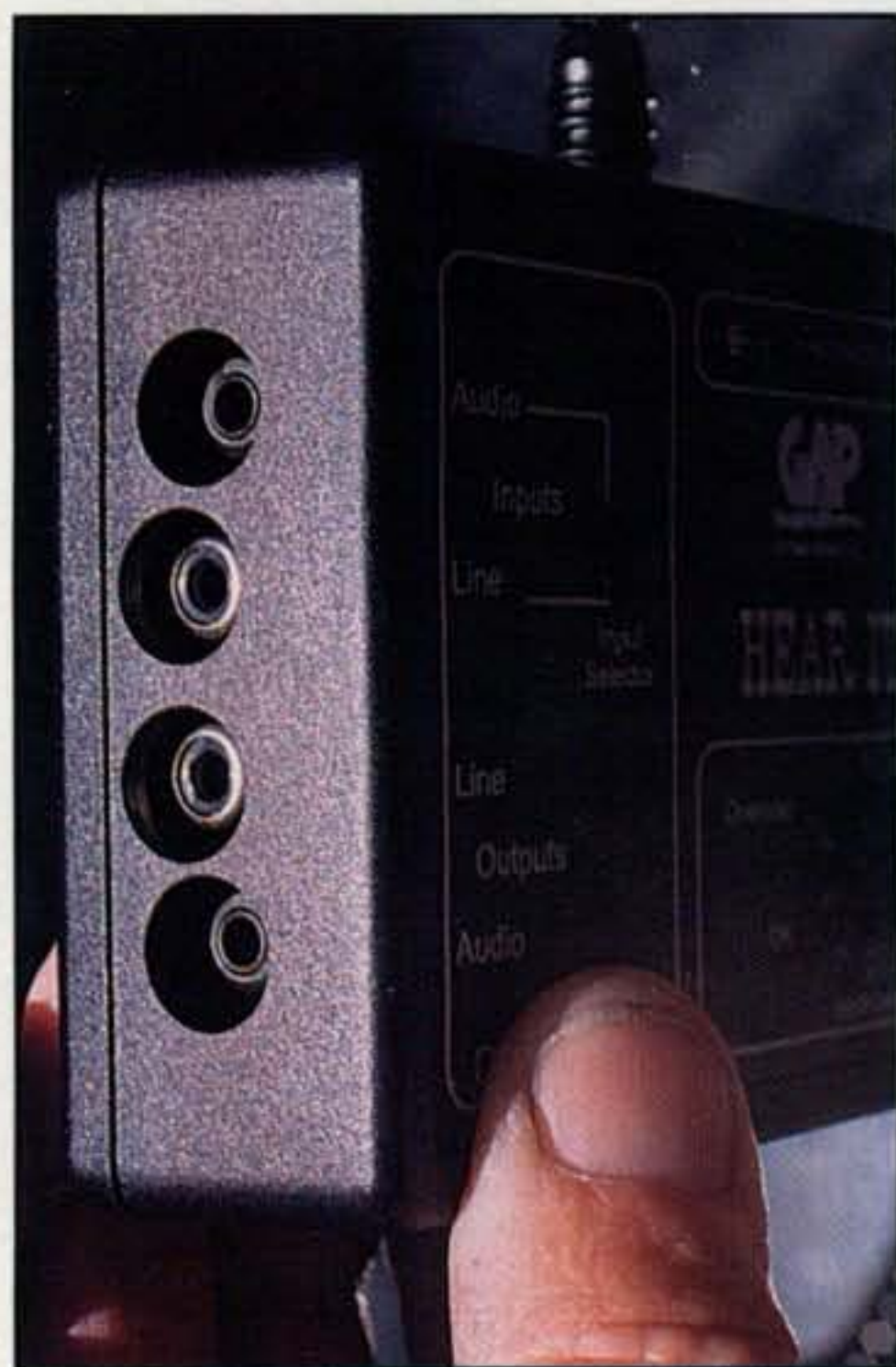
Photo D- Audio input and output cables plug into the side of the "Hear It" module. There are audio-level and line-level connections for both input and output.
