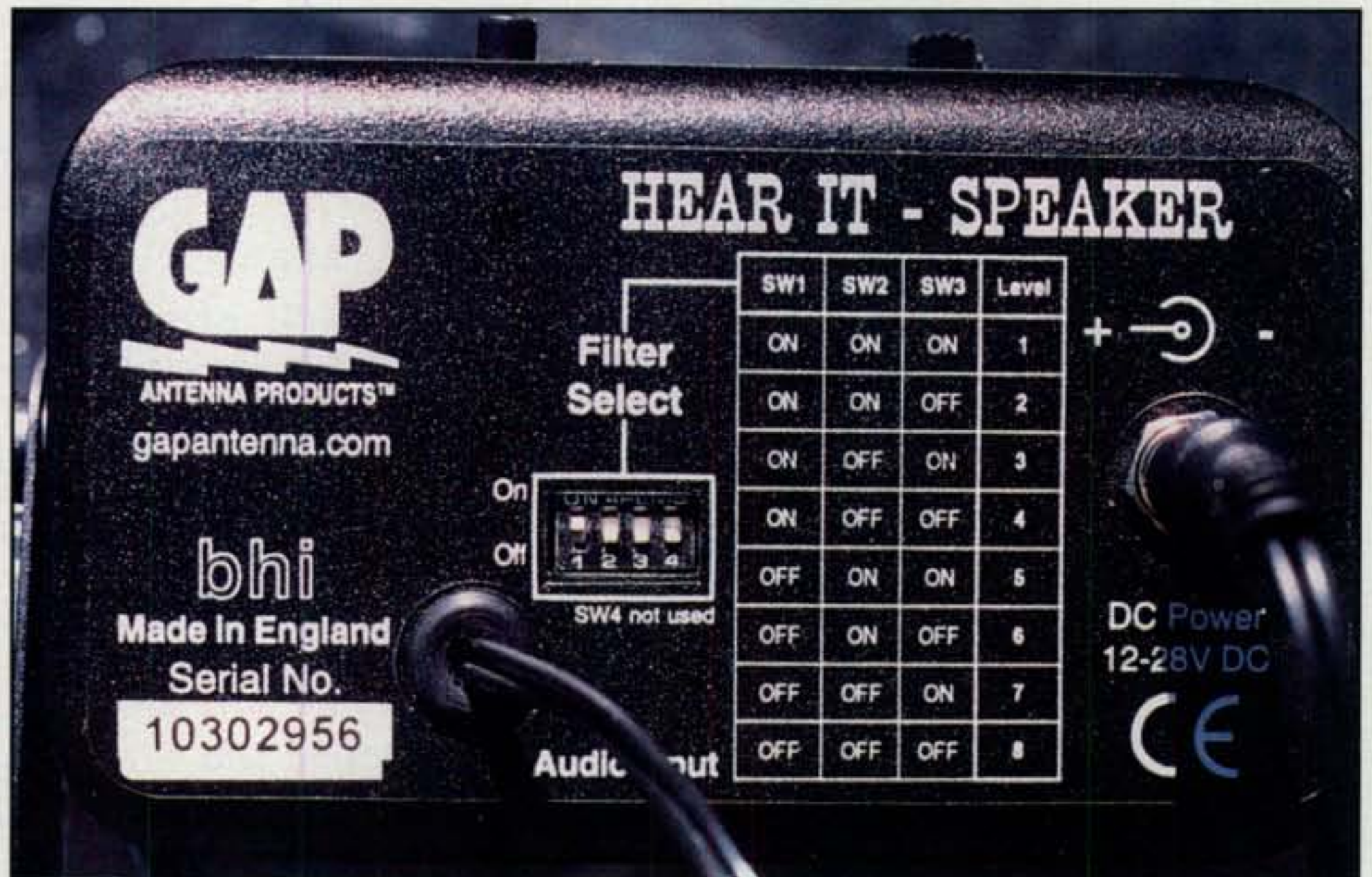
Photo B—DIP switches are used to control the DSP setting on the GAP "Hear It" speaker. Level 1 is minimum DSP, while level 8 is maximum.
