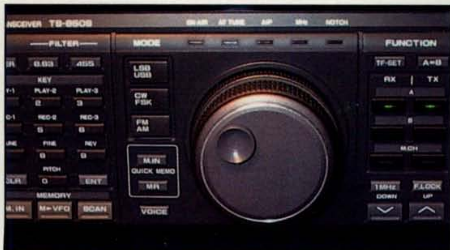
Photo C— The FingerDimple® is a precision add-on finger device to make a rotary dial spin easier for a rapid QSY. The self-sticking dimples come in black and gray, and they blend well with factory knobs. Here's a Kenwood TS-850S with a gray FingerDimple installed. (Photo courtesy Wayne Smith, K8FF)
