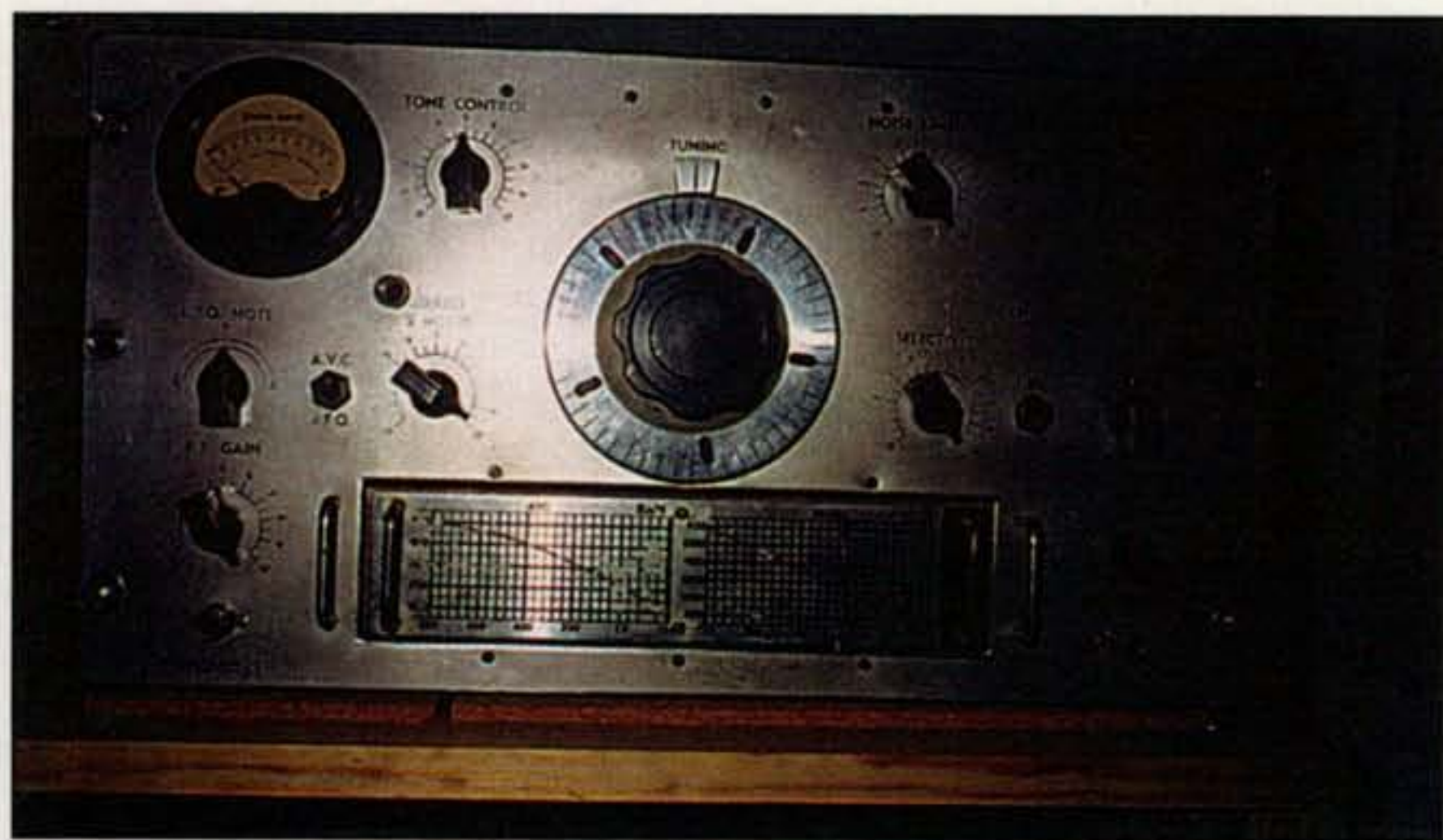
The Kingsley AR7. Like many other countries, Australia made its own version of the HRO receiver around World War II. This example is very original.
