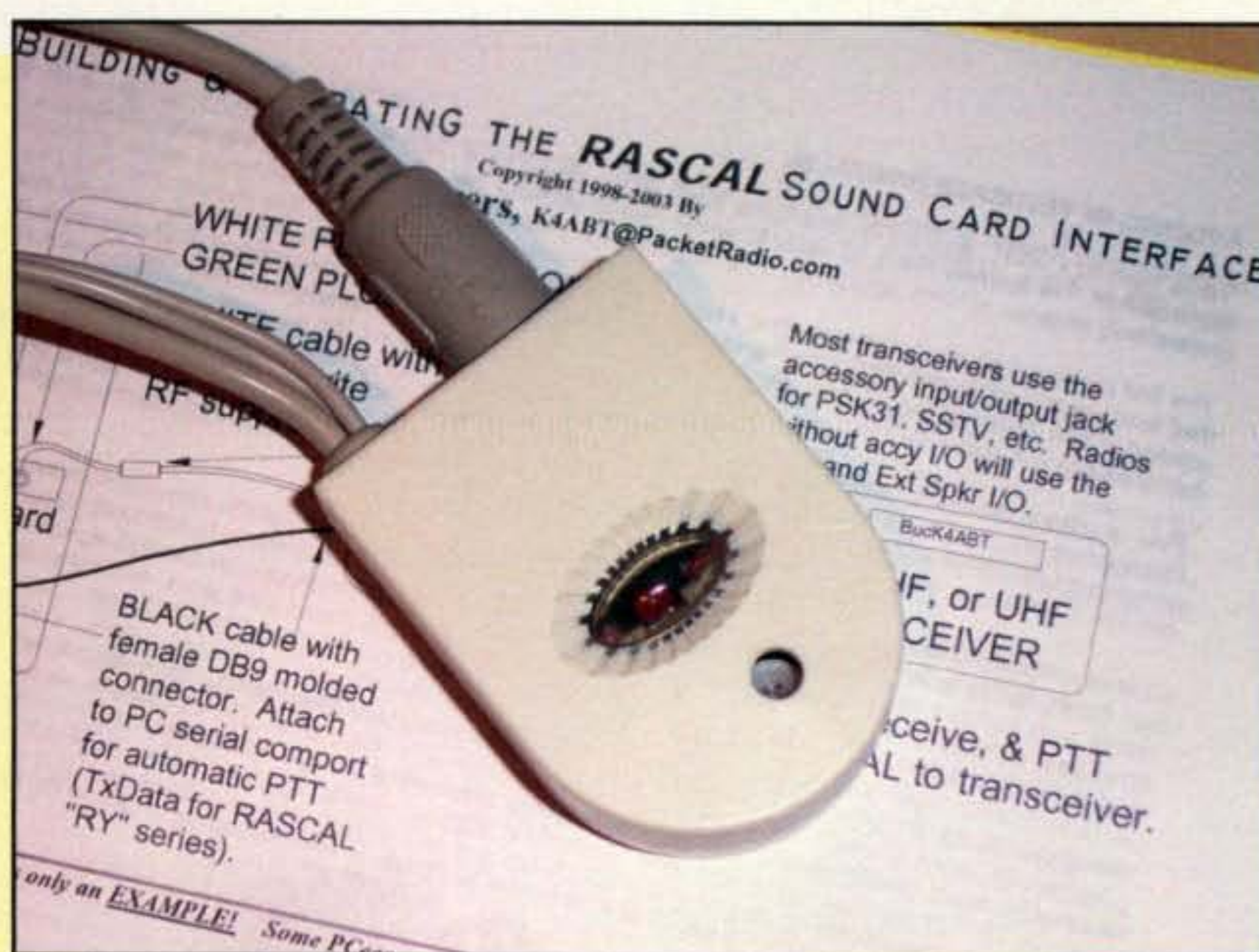
The K4ABT RASCAL sound-card interface. It is an inexpensive and relatively simple device, using good isolation transformers and ferrite beads to avoid feedback issues. Note the transmit audio level adjustment potentiometer inside the small hole. For more information, go to < www.packetradio.com >.
