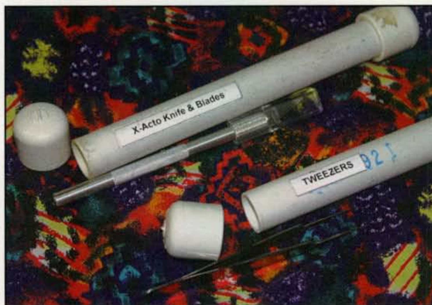
Photo 5— Pieces of scrap PVC pipe and a couple of caps ensure that small or dangerous tools are stored safely in your tool bag. The label serves two functions: It says what is inside the container, and the label is positioned on the left to indicate which end to open as an added safety precaution for sharp items that can poke or cut.
