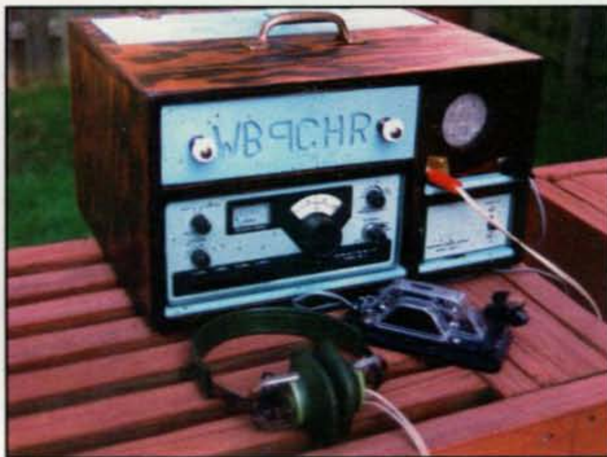
Photo 2— A classic QRP rig is the true sign of a QRP purist, and this restored-to-new and beautifully enclosed Heathkit HW8 station owned by N9IV is an example of that fact. The setup includes power supply, speaker, and a snazzy plastic-encased Hi-Mound key. (Photo by N9IV)
