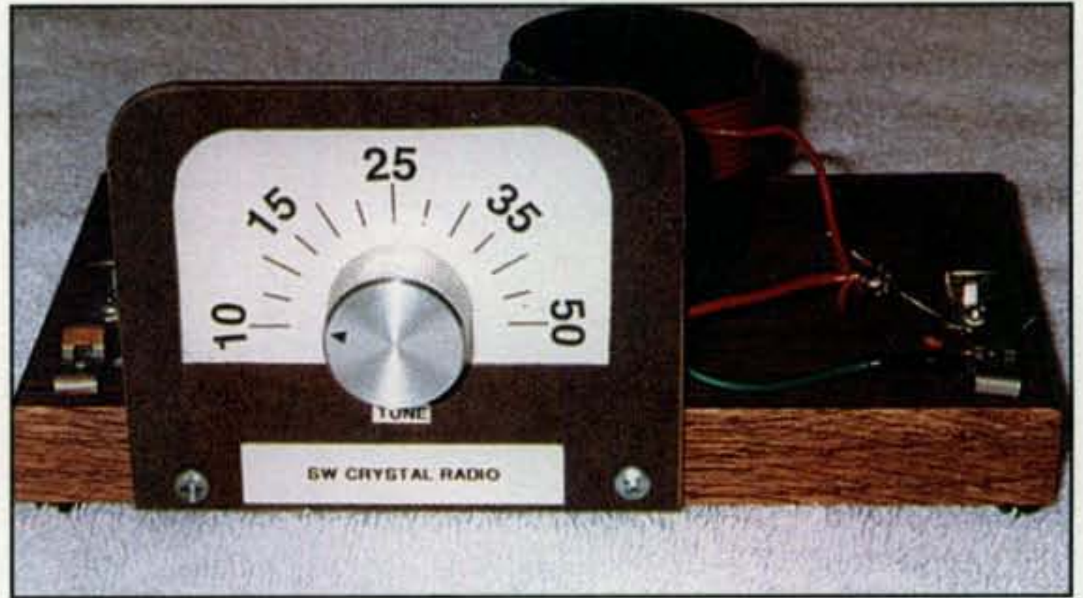
Photo A— This shortwave crystal set made by KF4YJQ uses a popular 1N34 glass-encased diode and double-tapped 7-turn coil to tune from the AM broadcast band to approximately 12 MHz. Circuit details are in fig. 1(B).
