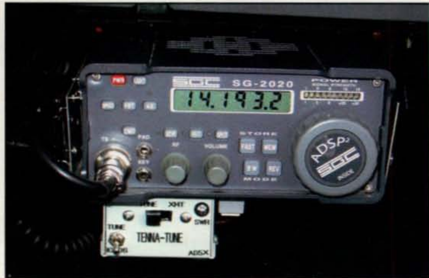
Photo 5— The SG-2020 mounted in the author's VW Beetle. The "TennaTune" box below it is the subject of a future article.
