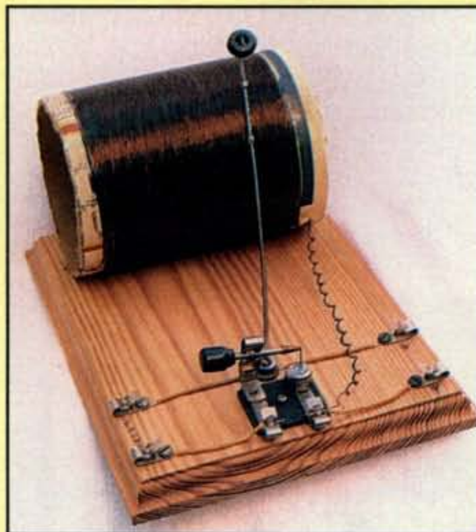
This quickly assembled crystal set uses a regular- or large-size oats box for the coil form and a genuine galena crystal in an authentic 1910 detector stand. It is a classic!
