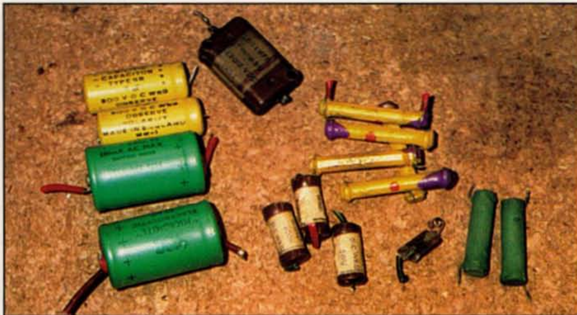
The majority of these components showed signs of overheating or age and thus were removed from the Panda Cub and replaced with modern equivalents.
