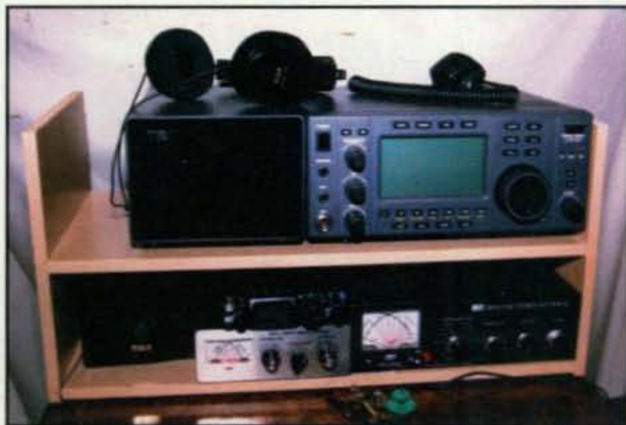
Photo 1— Answering that proverbial question "must I use QRP exclusively all the time to be considered a real QRPer?" is this modern setup of Russ Eberhart, N9IV. The station consists of a 5-watt Yaesu FT-817, a 100-watt Ten-Tec Jupiter for those times when QRP can't quite make the grade, two antenna tuners, and a neat WB9LPU prototype key with a green knob. (Photo courtesy N9IV)
