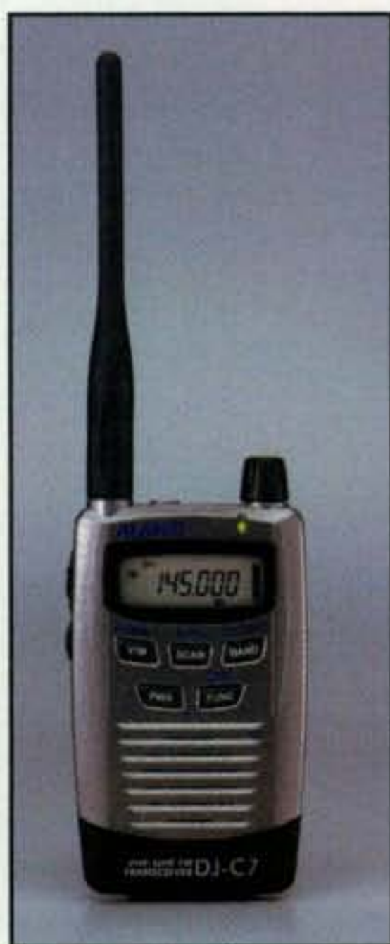
←Photo A— Alinco has introduced the DJ-C7T Pocket HT "Second Generation" Credit Card Size Dual Band Transceiver. The new 2m/70cm HT is a very small, pocket-size transceiver that succeeds the popular Alinco DJ-C5. This photo shows the front of the new mini HT. (Photo courtesy Alinco)
