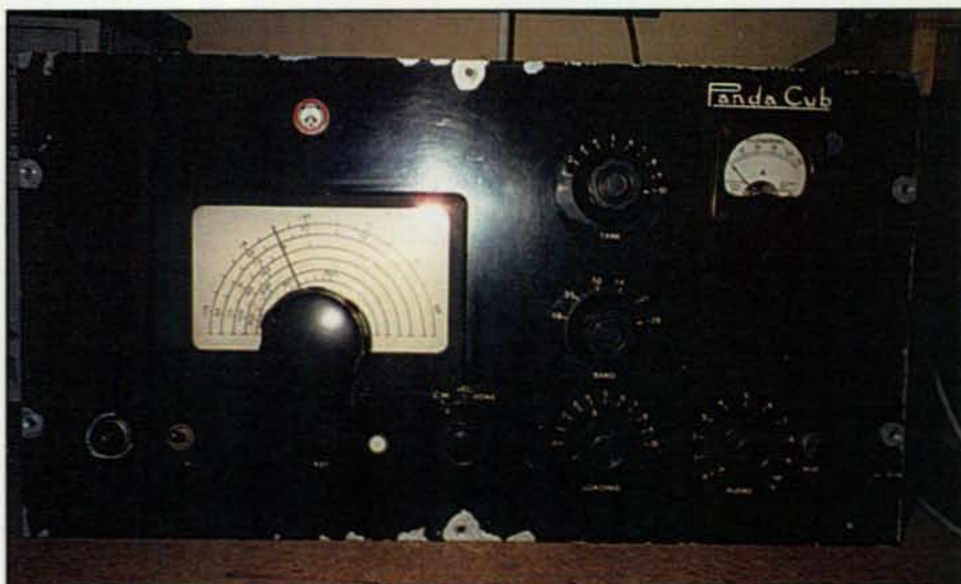
This Panda Cub 50W 1.8–28 MHz AM/CW transmitter is currently undergoing restoration at VK6VZ. It was designed by the legendary Louis Varney, G5RV, and commercially manufactured in the United Kingdom during the 1950s/60s from World War II surplus components.
