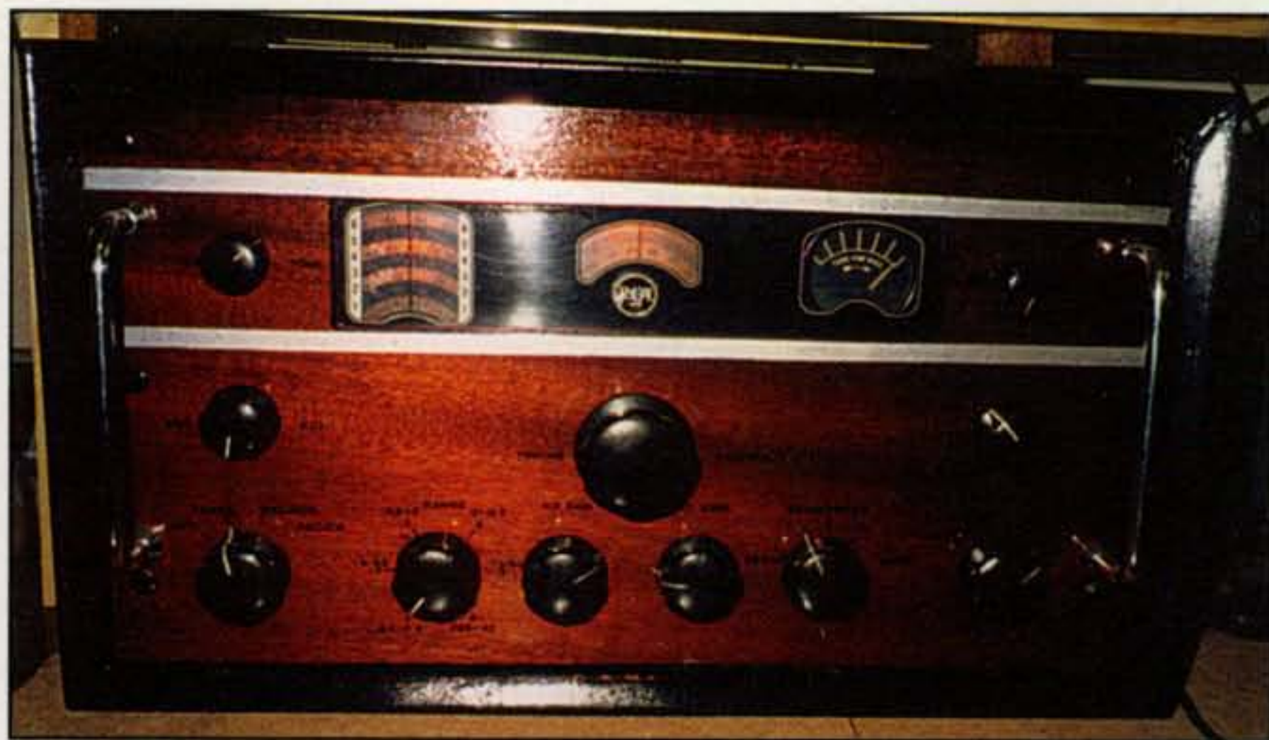
This RCA AR-88D receiver is far from being in original condition, with its first RF stage replaced with a miniature EF183 tube and its metal cabinet replaced by a wooden one made from West Australian jarrah. However, it works well and is a great conversation piece.
