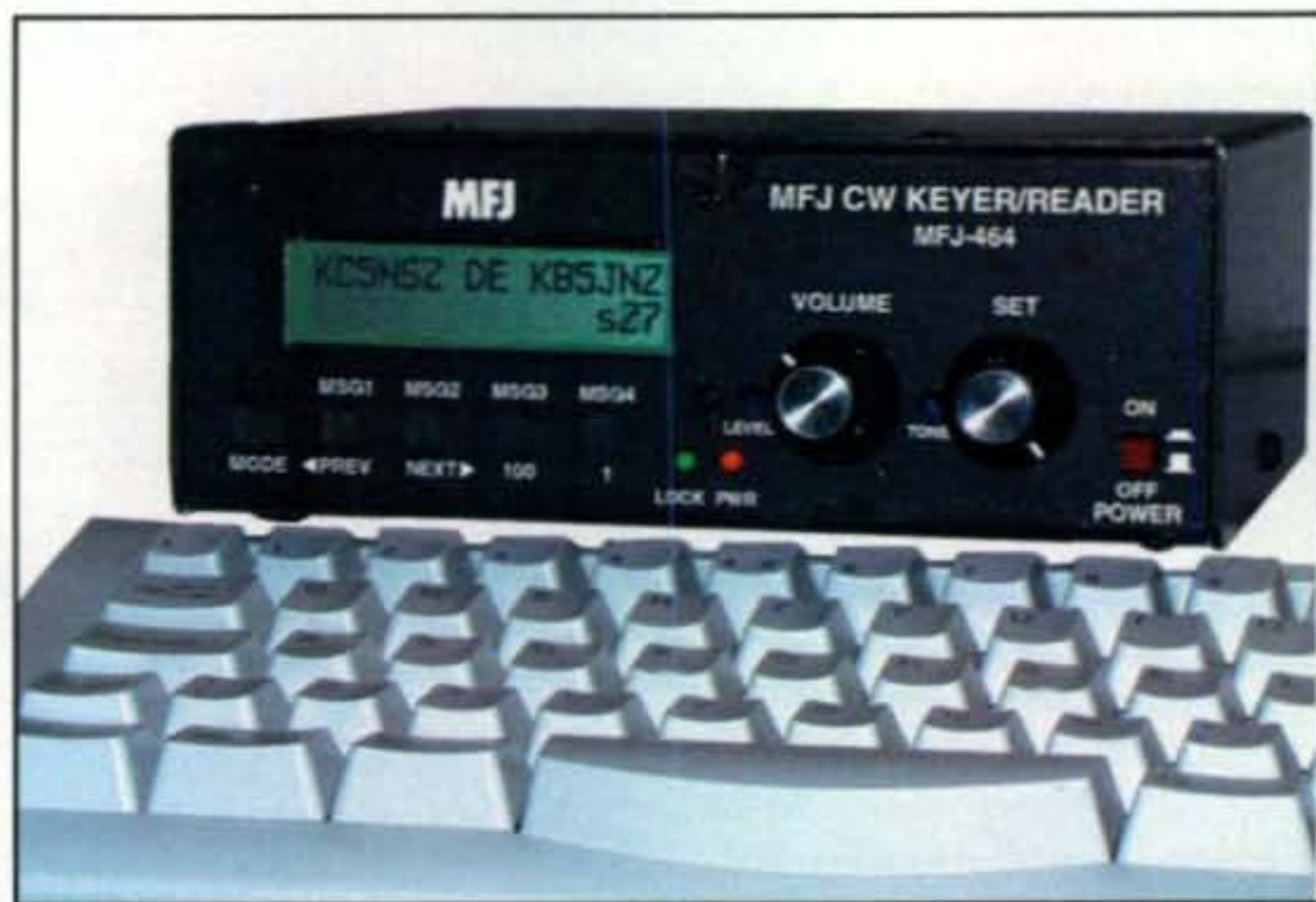
Photo B— Like to contact some really exotic DX working CW almost exclusively? Try an MFJ-464 combination Morse code reader and programmable keyer. It displays both incoming and outgoing code on its front readout and makes a neat CW aid.
