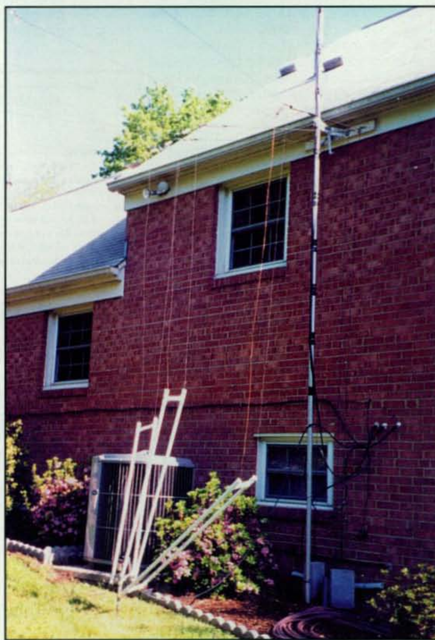
Photo A— Wide view of K4PRL's multiband inverted-L antenna array. The PVC separators "float" on the wires and are not connected to the base section. (Photos by the author)
