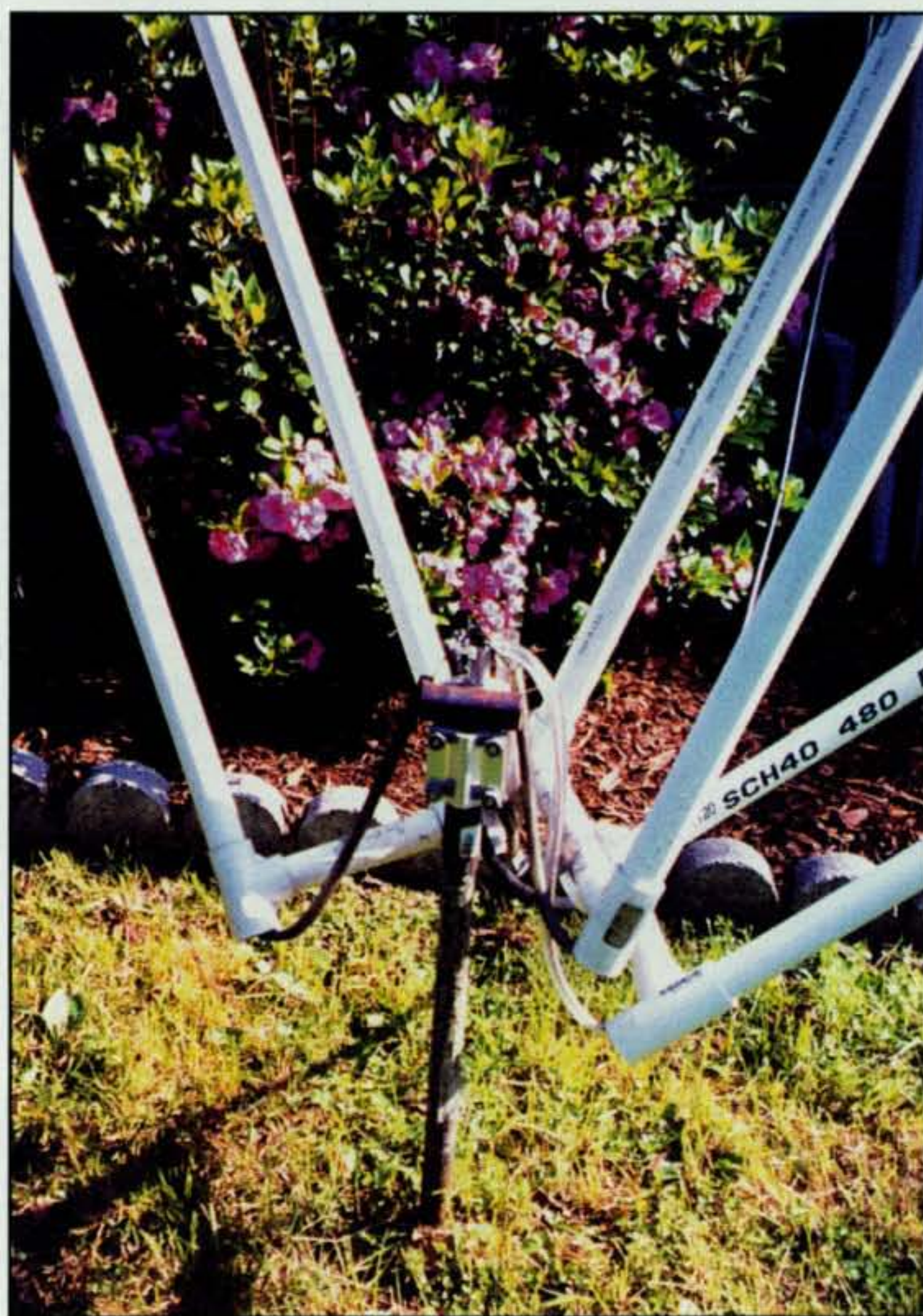
Photo B— Close-up of base section showing antenna wires coming through each of the PVC separators and meeting in the middle, where they're connected to a single piece of coaxial feedline going back to the shack.
