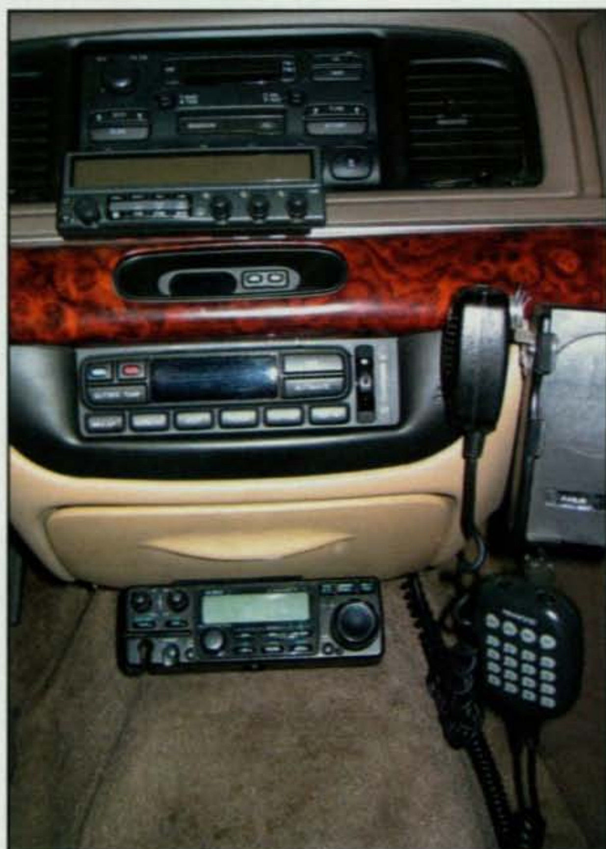
Multi-band capabilities in the author's Mercury Grand Marquis: Alinco DX-70TH control head attached to ashtray/cupholder for 6-meter +HF operations; and Kenwood TM-741A control head with 2m/222/440MHz modules just below the broadcast receiver. Microphones hang from the cell-phone holder, and all equipment is clear of airbag-deployment zones. The main transceiver units are mounted in the trunk and fed by fused wires connected directly to the car's battery.
