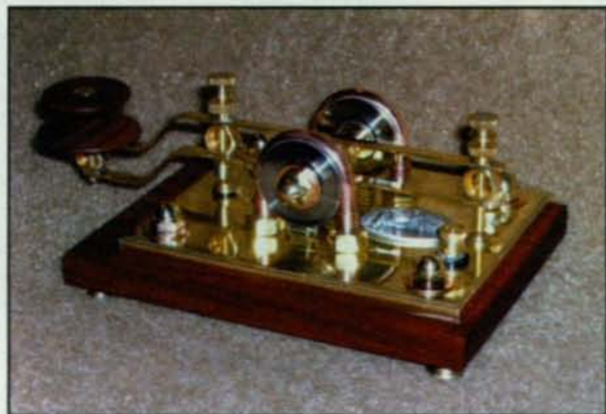
Photo 2—A reverse-angle view of the W1YBR Cliff Dweller key gives more insight to its unusual design. The key is supplied with two leaf-type springs for varying tension, and fitted with a pewter nameplate showing its serial number and the cliff-dwelling caveman log. (Photo courtesy of W1YBR)
