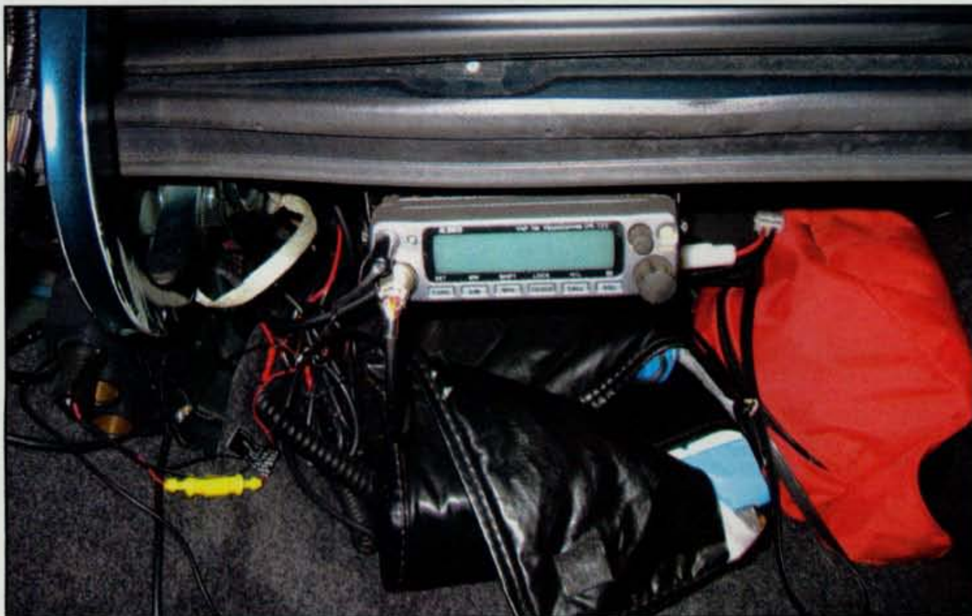
Alinco DR-135 2-meter transceiver mounted in the trunk for APRS operations. Not pictured is the GPS receiver, with the "stealth" antenna invisibly mounted beneath the fabric of the rear window shelf. Out of view, other transceiver units are securely mounted out of harm's way, against the rear seat support panel. Attention was given to air circulation for cooling.
