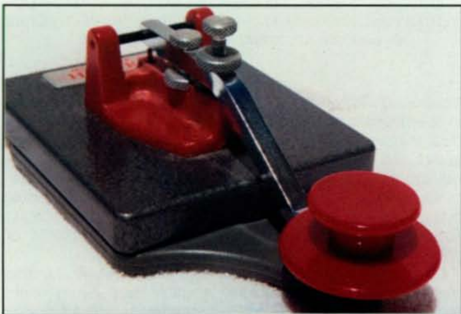
Photo 8— Ham Radio Center of St. Louis, Missouri produced this attractive Ham Key during the 1960s, and it is still popular today. The key sports a rear-pivoting arm fitted with a shiny red, navy-type knob and supported by a red plastic frame. Cool! (Key owned and photographed by James Butler, KB4LJV)
