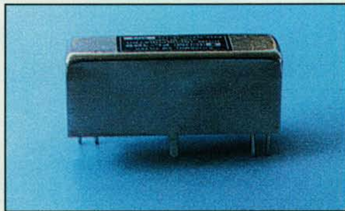
Photo A— A typical plug-in, optional crystal filter for an HF transceiver. These items are produced in various sizes, bandwidths, and IFs to mate with specific models of receivers or transceivers.
