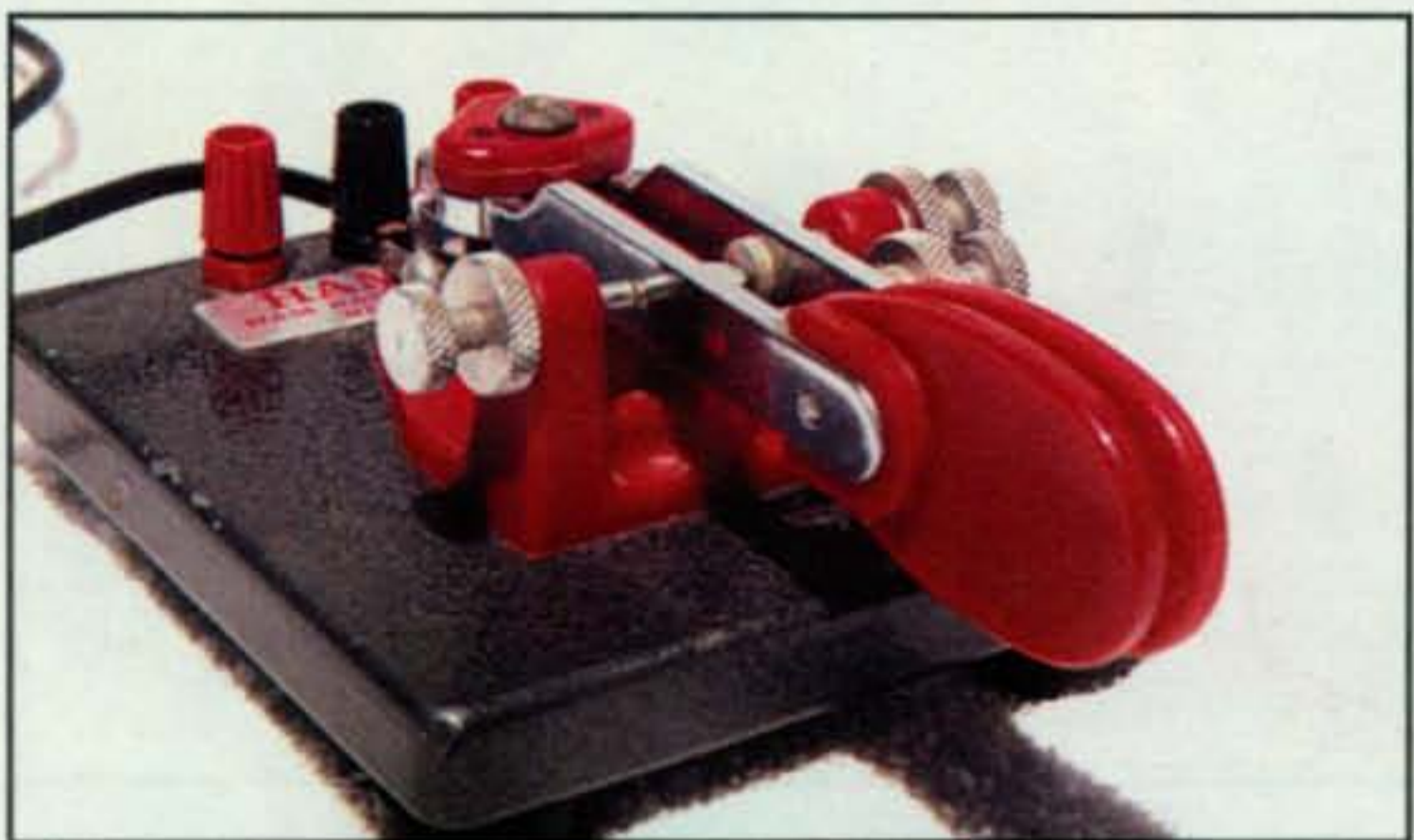
Photo 9— This matching twin-lever paddle was also produced by Ham Radio Center, and it too sports a bright-red plastic frame plus red fingerpieces. A single right-side adjustment sets tension, adjustments on each side set gap, and a ground contact/stop post is mounted between the levers. (Photo courtesy of WB4LJV)
