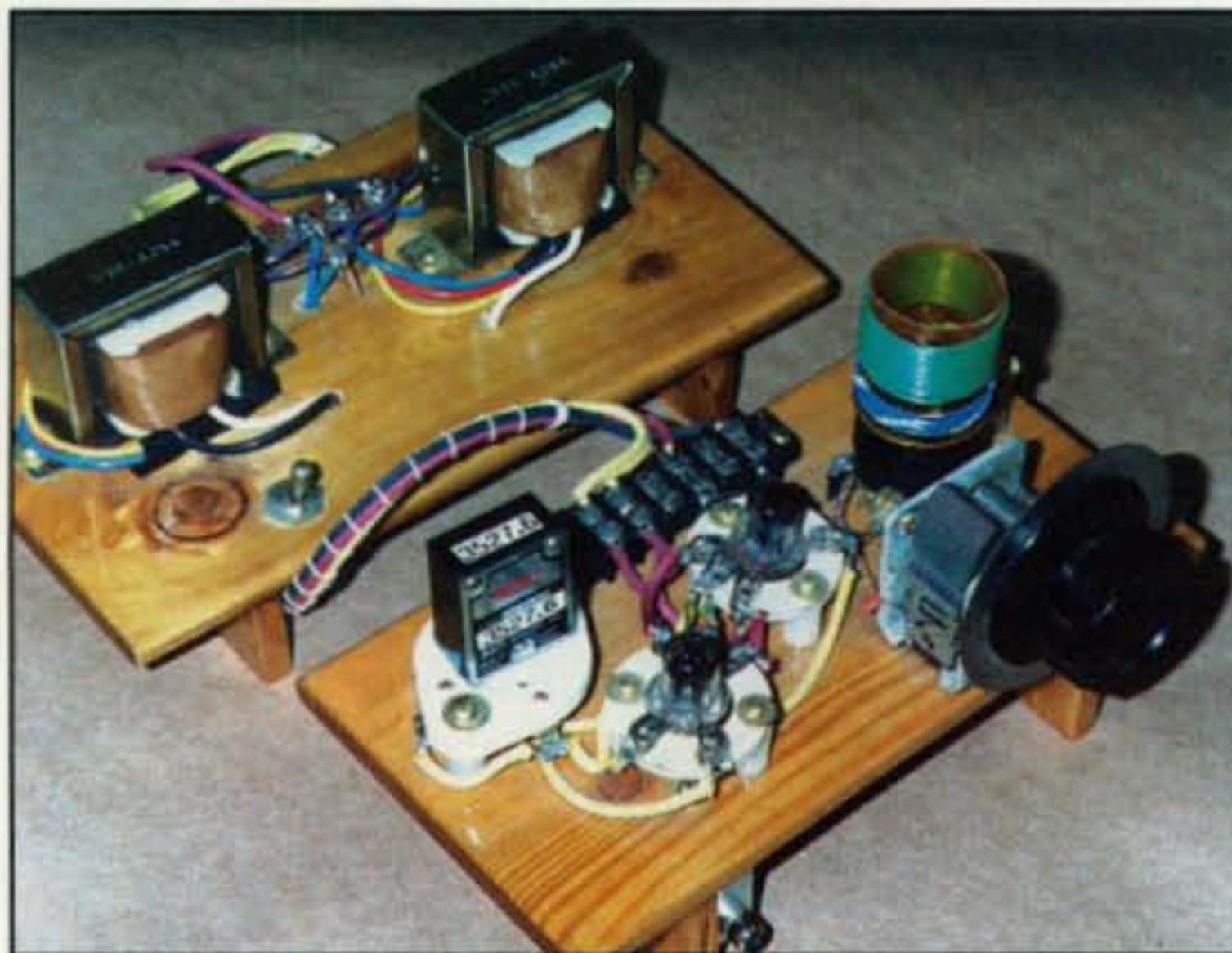
Photo E— This wood-base beauty was built by Mac Neill, W8ZNX, and uses dual 955 acorn tubes wired in parallel for real vintage QRP glamour. The power supply uses a pair of 6-volt filament transformers wired "back to back," and setup produces slightly over 1 watt output. Note the hand-laced cable and rare classic knob on the tuning capacitor. (Photo by W8ZNX)
