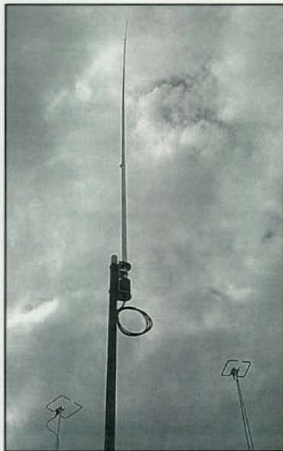
Photo A— The CHA250B mounted on the military mast. The antenna has a low wind foot print, and it almost seems to disappear into the air. This was the setup used for the A/B testing.
