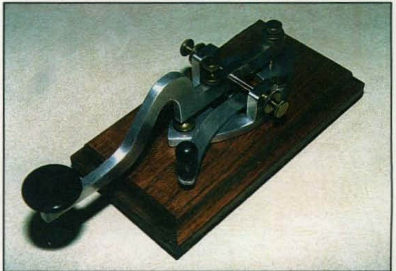
Photo 6— Using simple machine tools and salvaging adjustment screws from other keys, Ed, NS3E, homebrewed this well-detailed reproduction of a famous Phelps camelback key from the mid 1800s. Notice the teardrop-shape metal frame and smooth crafted arm with vintage trunion pin at the fulcrum. Nice! (Photo courtesy of NS3E)
