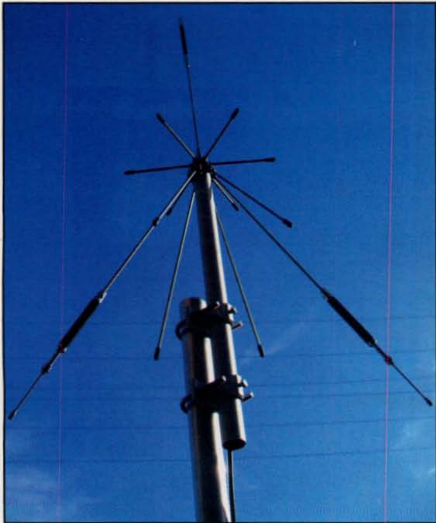
Photo E— The DS3000A discone in this photo can receive from 75 MHz to 3 GHz and can be mounted in confined areas. The DS3000A also can support transmitting on 144, 430, 904, and 1200 MHz, safely handling up to 50 watts. (Photo courtesy of AOR USA)
