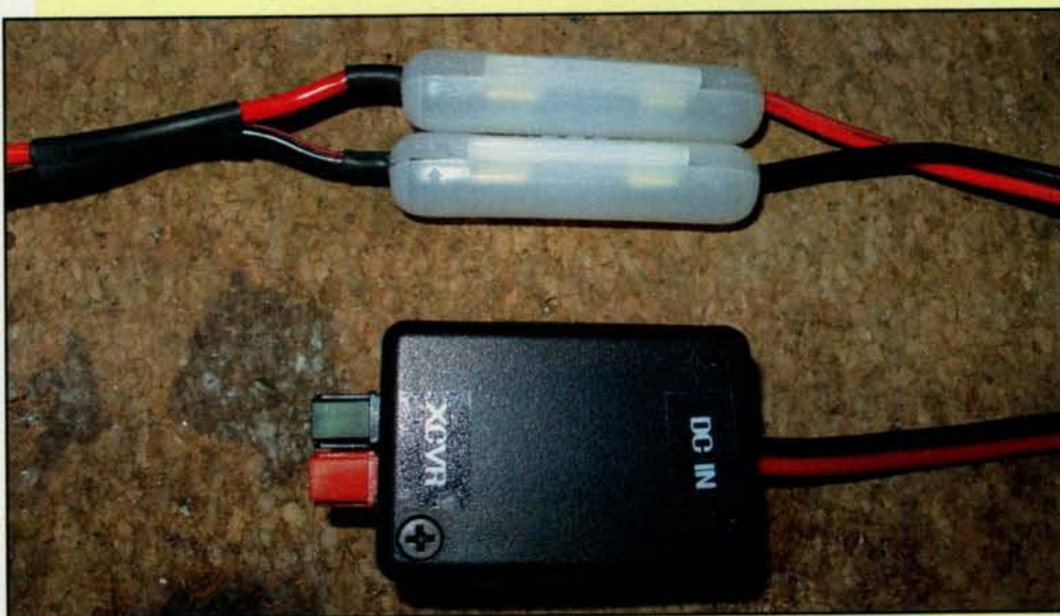
Photo B. Final assembly of the conditioner, compared with the original fuse-holder and fuse assembly.
