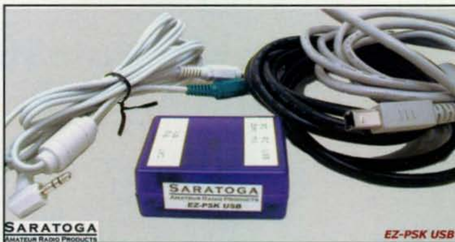
Photo C— Saratoga Amateur Radio Products offers the EZ-PSK USB™, a transceiver to sound card interface that uses the computer's USB port. The new product is for the user who wants to connect to the computer's USB port rather than its serial port. (Photo courtesy of Saratoga Amateur Radio Products)
