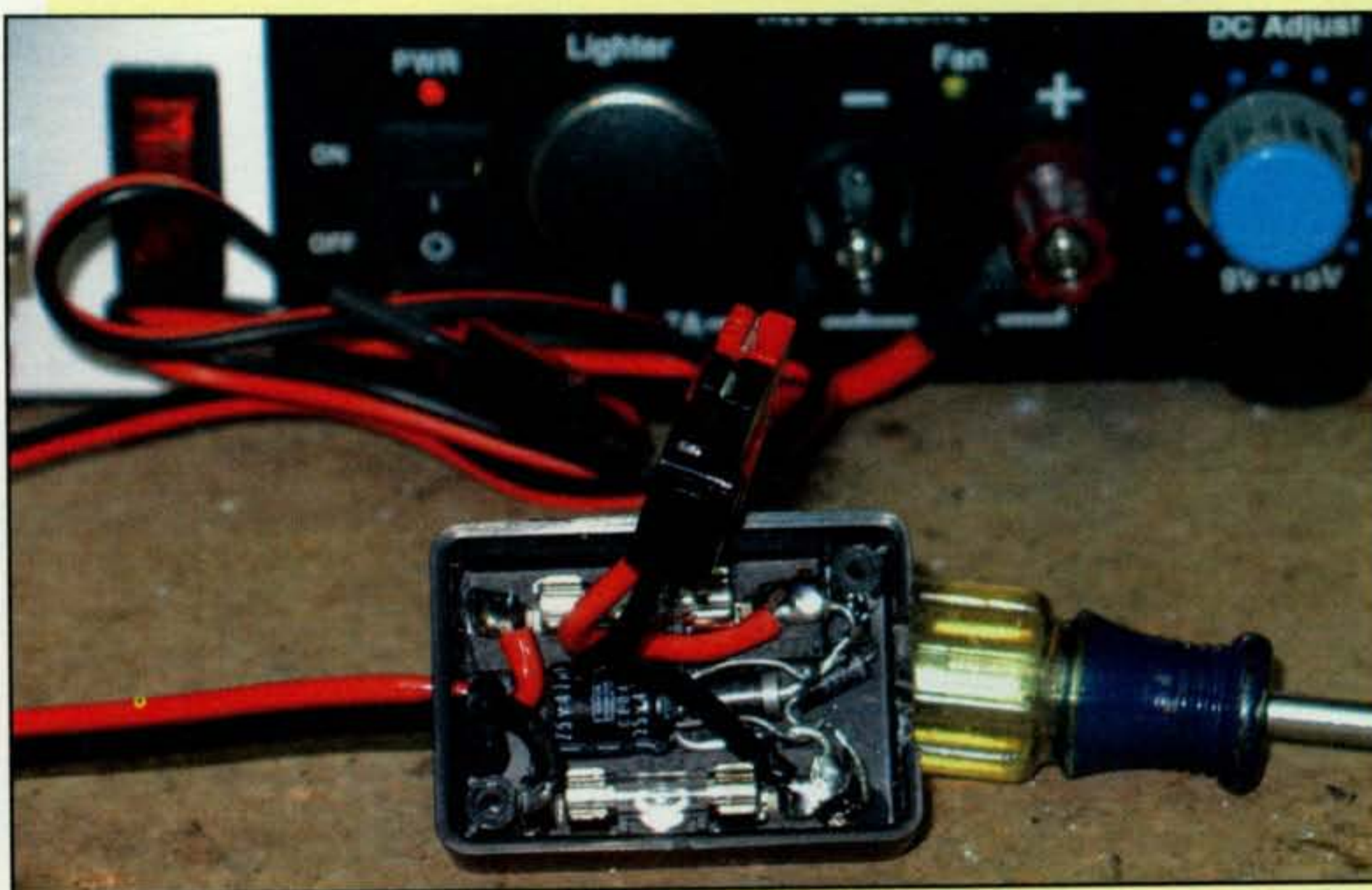
Photo A. Internal wiring of the voltage conditioner. The Anderson PowerPole has been pushed aside to allow you to see better.
