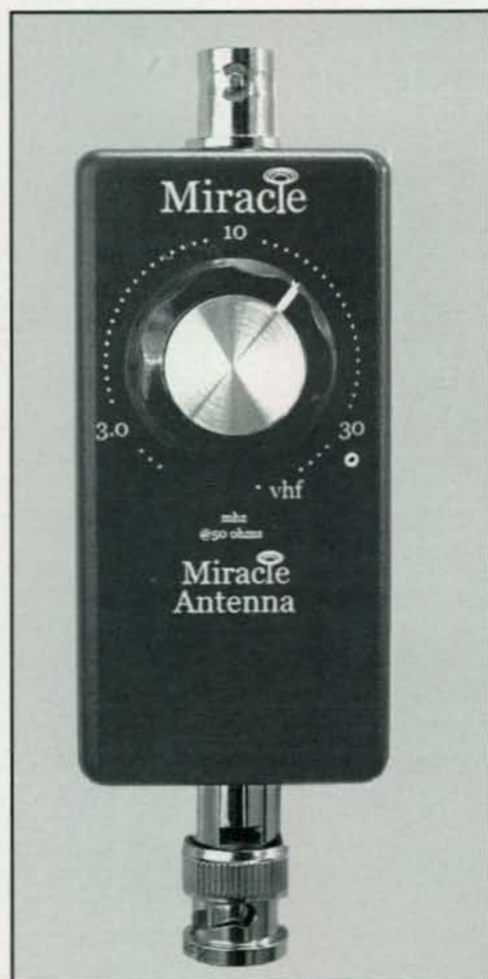
Photo G— Miracle Antenna also offers the Ducker family of portable antenna devices. The Duckers, available in PL (PL-259) and IL (inline) versions, permit transmitting with a short whip throughout the entire HF range for portable operations. (Photo courtesy of Miracle Antenna)
