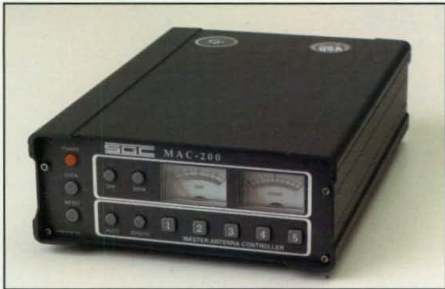
Photo D— SGC's recently announced MAC-200 Automatic Antenna Controller/Tuner covers 1.8 to 60 MHz and handles up to 200 watts. The item differs from a regular auto tuner, as it tunes dipoles, beams, and verticals plus single random-length wires and balanced or ladder-line-fed antennas such as multiband doublets and Zepps. (Discussion in text.)
