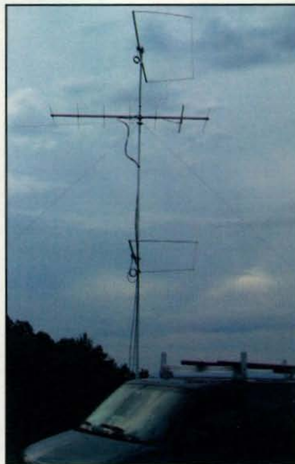
The 21-foot fiberglass Wonder Pole with two 6-meter Moxon rectangle antennas and a 7-element 2-meter Yagi. The antennas are rotated "Armstrong-style" out the vehicle's window for a quick fix on direction. (Photo by Clarke, K1JX)
