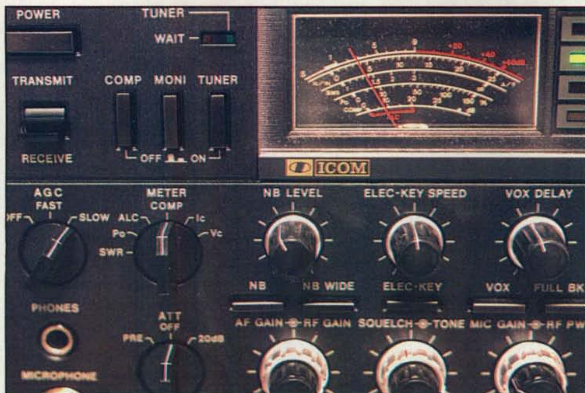
Photo A— Most mid-range to high-end HF transceivers include a very effective noise blanker with front-panel level adjustment. The older ICOM IC-761 shown here also sports both wide and narrow noise blankers. Wide blankers were originally designed to minimize “Woodpecker” or over-the-horizon radar noise, but they also help minimize raspy BPL-type noise.
