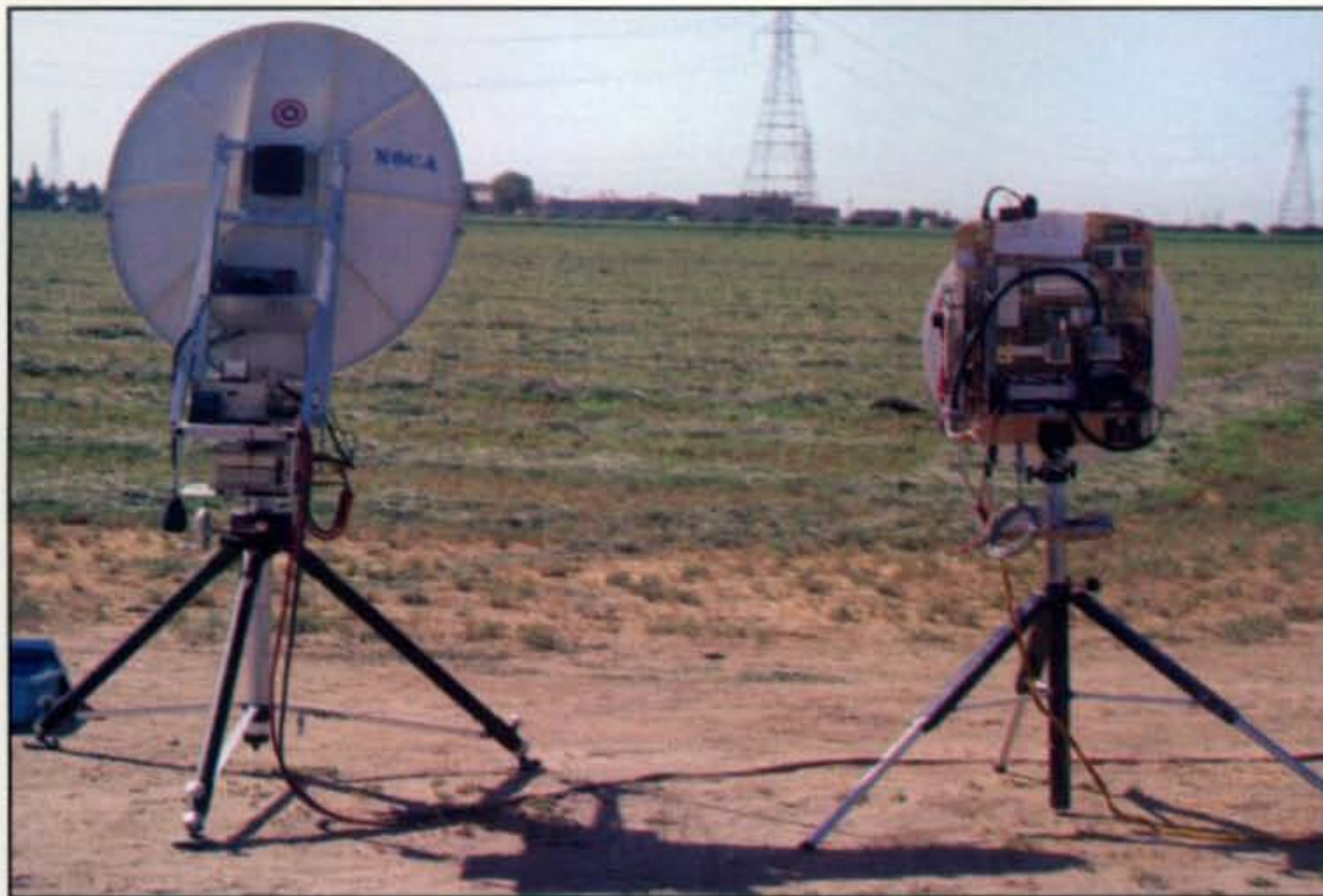
Photo B— Chip Angle's rig (on left) has much more receive and transmit capability than mine. Notice the difference in the size of the dish antennas. The CW mode increased the useful communications range over SSB.
