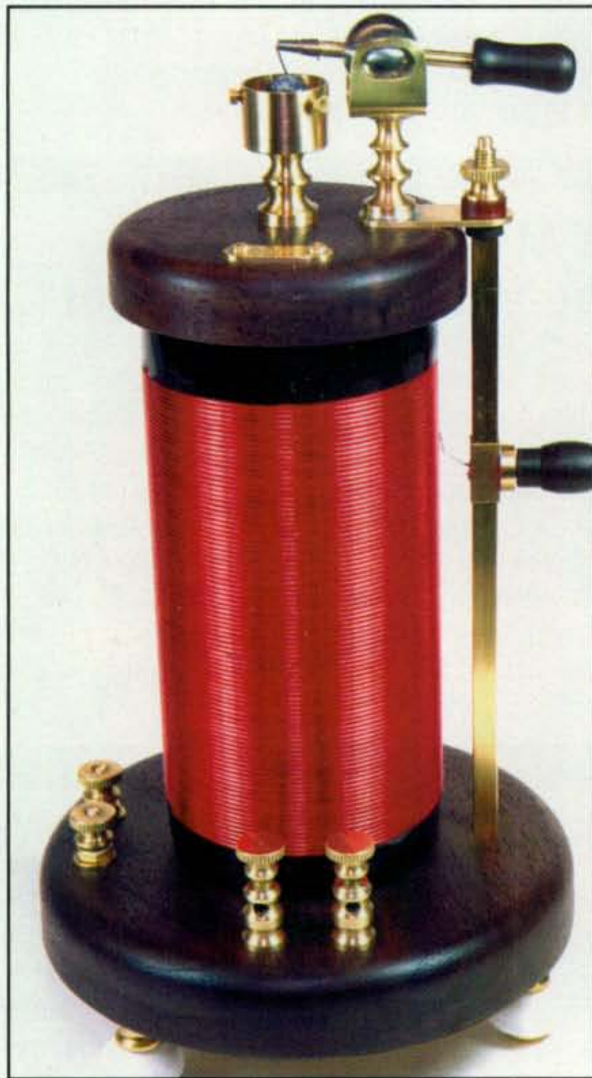
Photo A— This dazzling little crystal set, made by Jerry Clement, VE6AB, sports a 5-inch-tall coil form with home-fabricated locking slider, walnut end caps, plus a machined-from-scratch catwhisker and galena crystal stand. Jerry wound that perfect 100-turn coil on a lathe and daughter Jen Clement shot this stunning photo. Awesome, isn't it?
