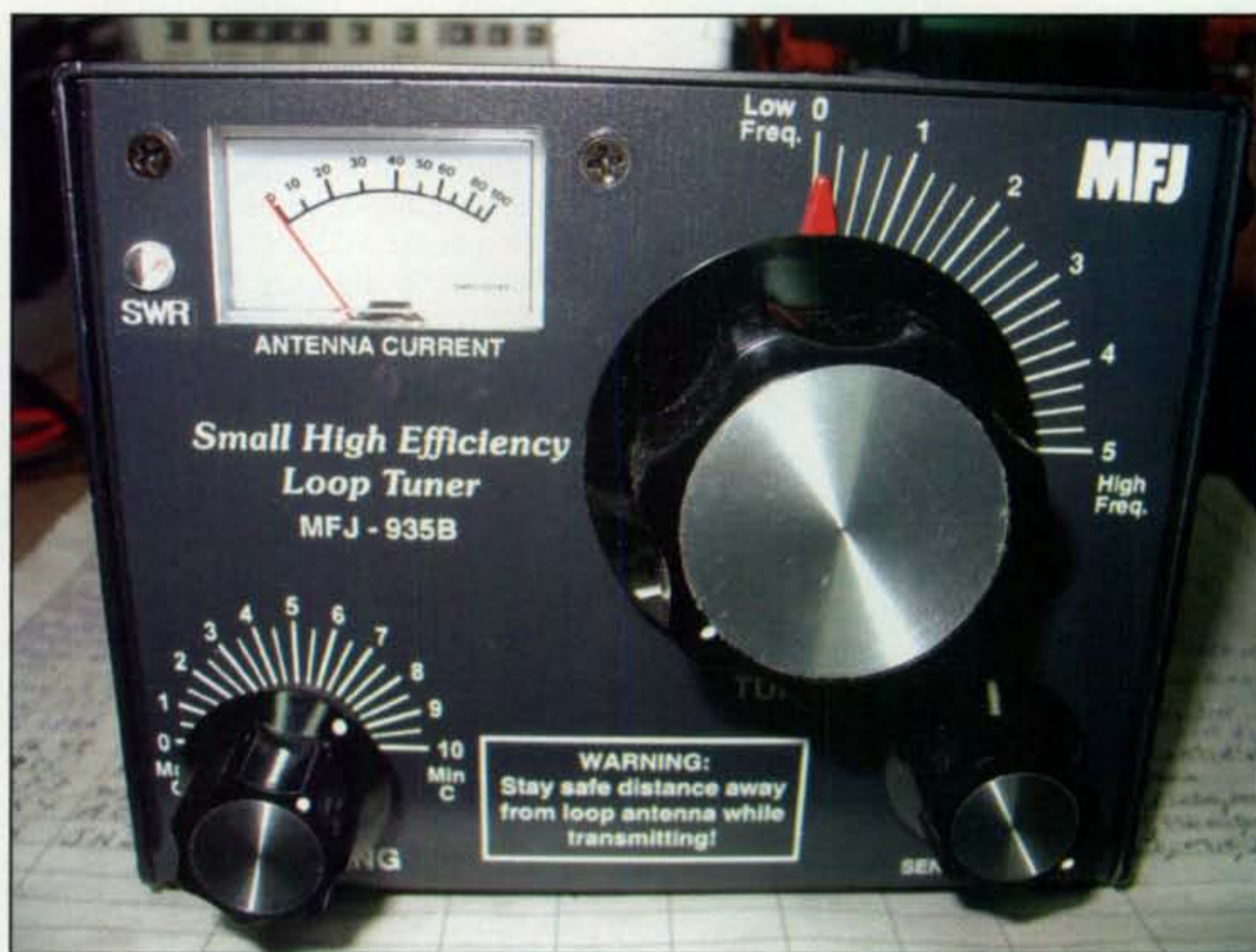
Photo A— The MFJ-935B is one three models of similar loop antenna tuners introduced this year by MFJ. This photo shows the 935 with my SWR LED added (see sidebar for details).
