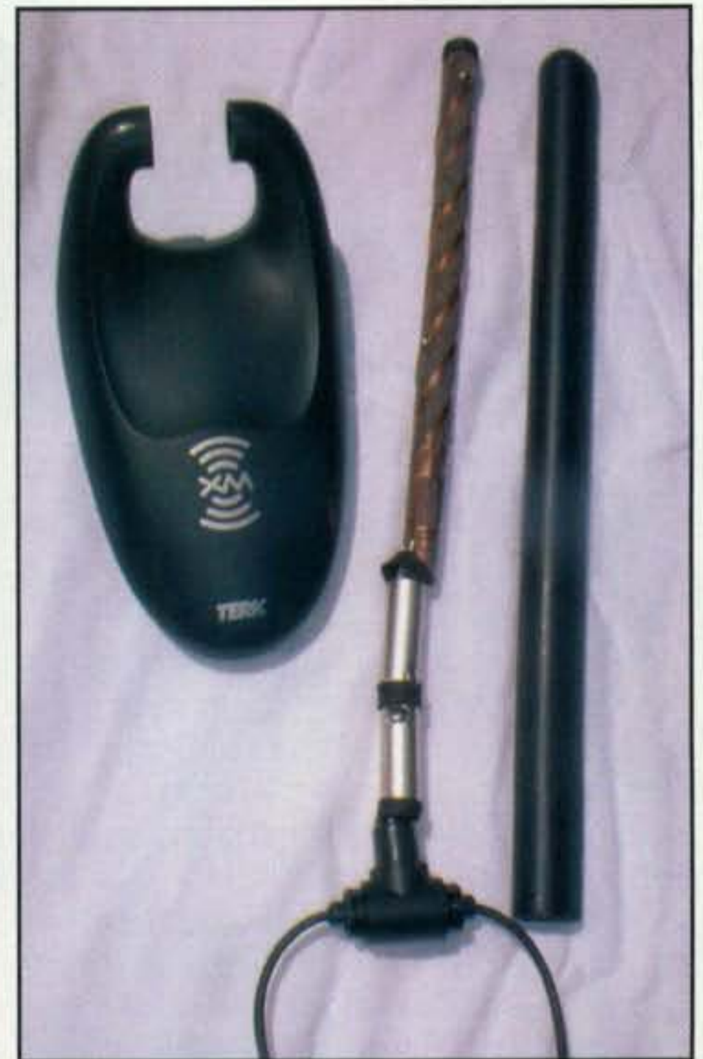
Photo D— An XM satellite antenna I picked up at a fleamarket and took apart to see how it works. Actually, there are two antennas, a quadrifilar spiral for satellite reception and a dipole for terrestrial reception.
