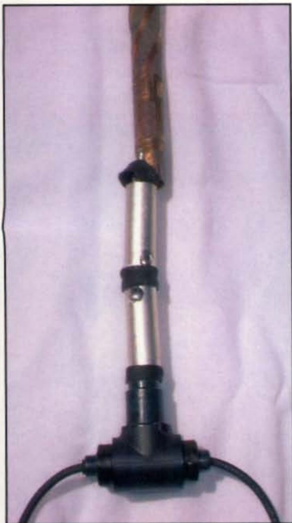
Photo E— The dipole part of the XM antenna, used to pick up terrestrial rebroadcasts of programs for reception in urban areas where satellite signals have trouble getting through.
