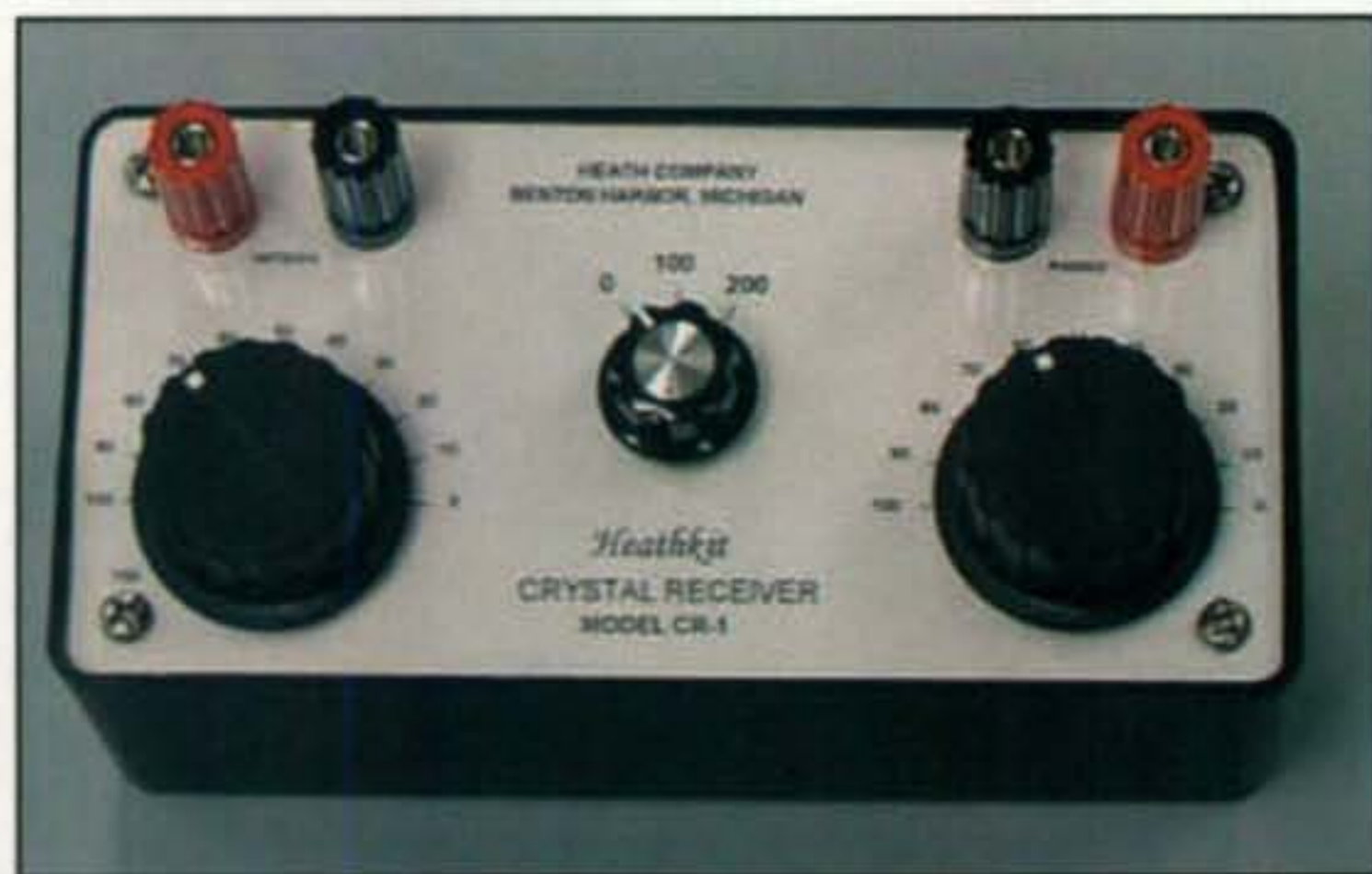
Photo D—W4LF-built "retro replica" of Heathkit's 1950s-style CR1 Crystal Set. The little gem has become a rare collectable, but thanks to its use of conventional and readily available parts, homebrewing a copy is relatively easy.
