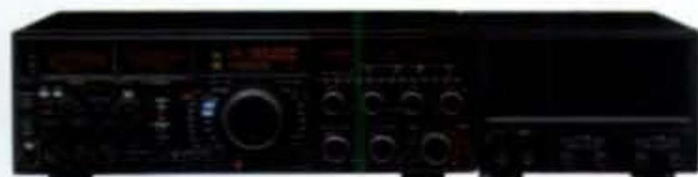
FT DX 9000MP 400 W Special Order Version Two Pairs of Meters, plus LCD Window; Data Management Unit and Flash Memory Slot Built In. Main/Sub Receiver VRF, plus Full Dual Receive Capability. External 50 V/24 A Switching Regulator Power Supply and Speaker with Audio Filters. Display color (Umber or Light Blue) may be selected at the time of purchase. Modification from 400 to 200 W not possible.
