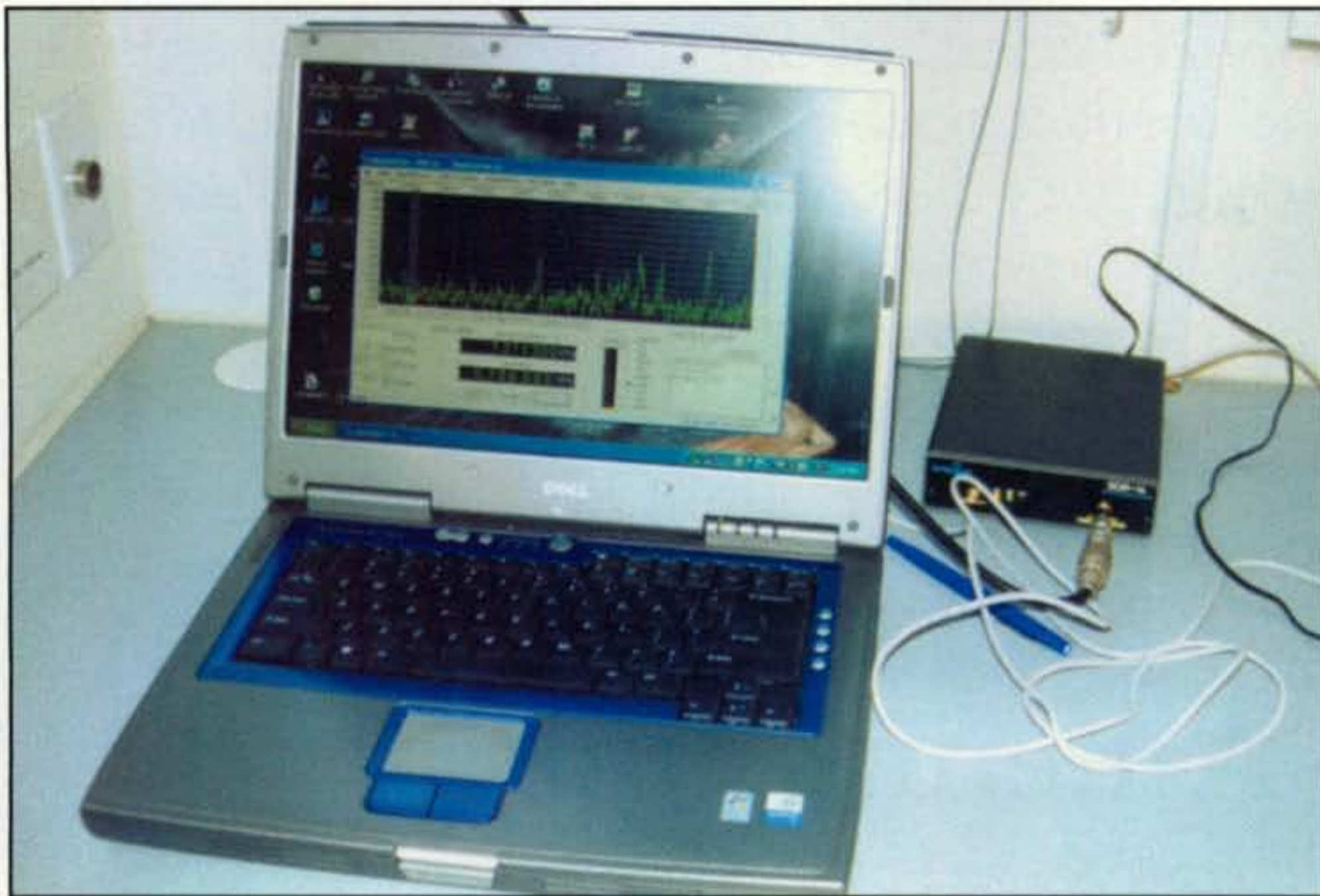
The RFSpace SDR-14, at right rear, is a software-defined radio receiver that outputs spectrum-usage information for a visual display on a computer screen rather than audio to a speaker or headphones. In this photo, students in a licensing course are watching activity on 20 meters.
