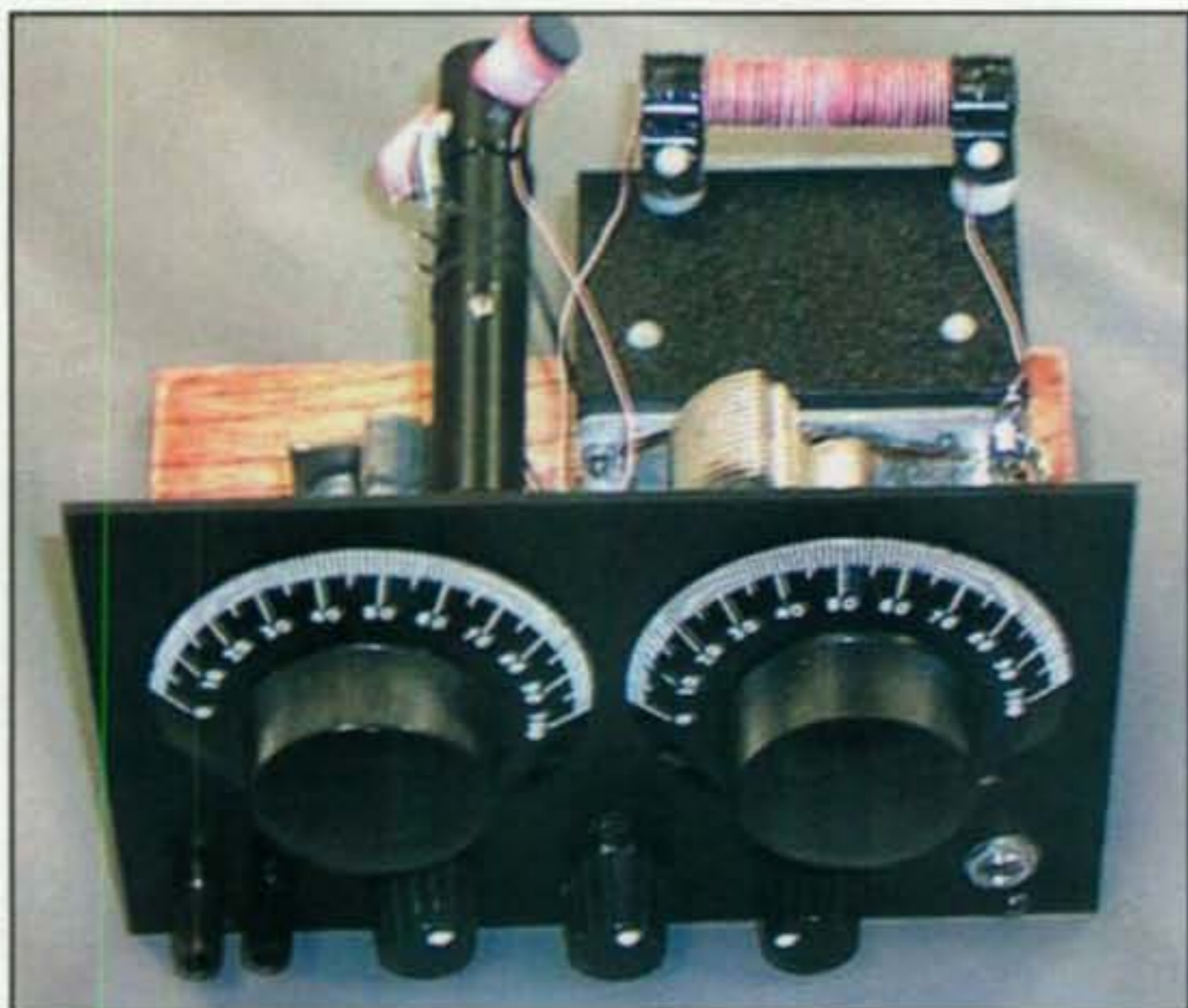
Photo B—Classic National Velvet venier knobs give this high-performance crystal set built by Jim Frederick, W4LF, a real radio look. The little set is exceptionally sensitive and selective, thanks to Jim's "Hobbydyne" circuit shown in fig. 2.
