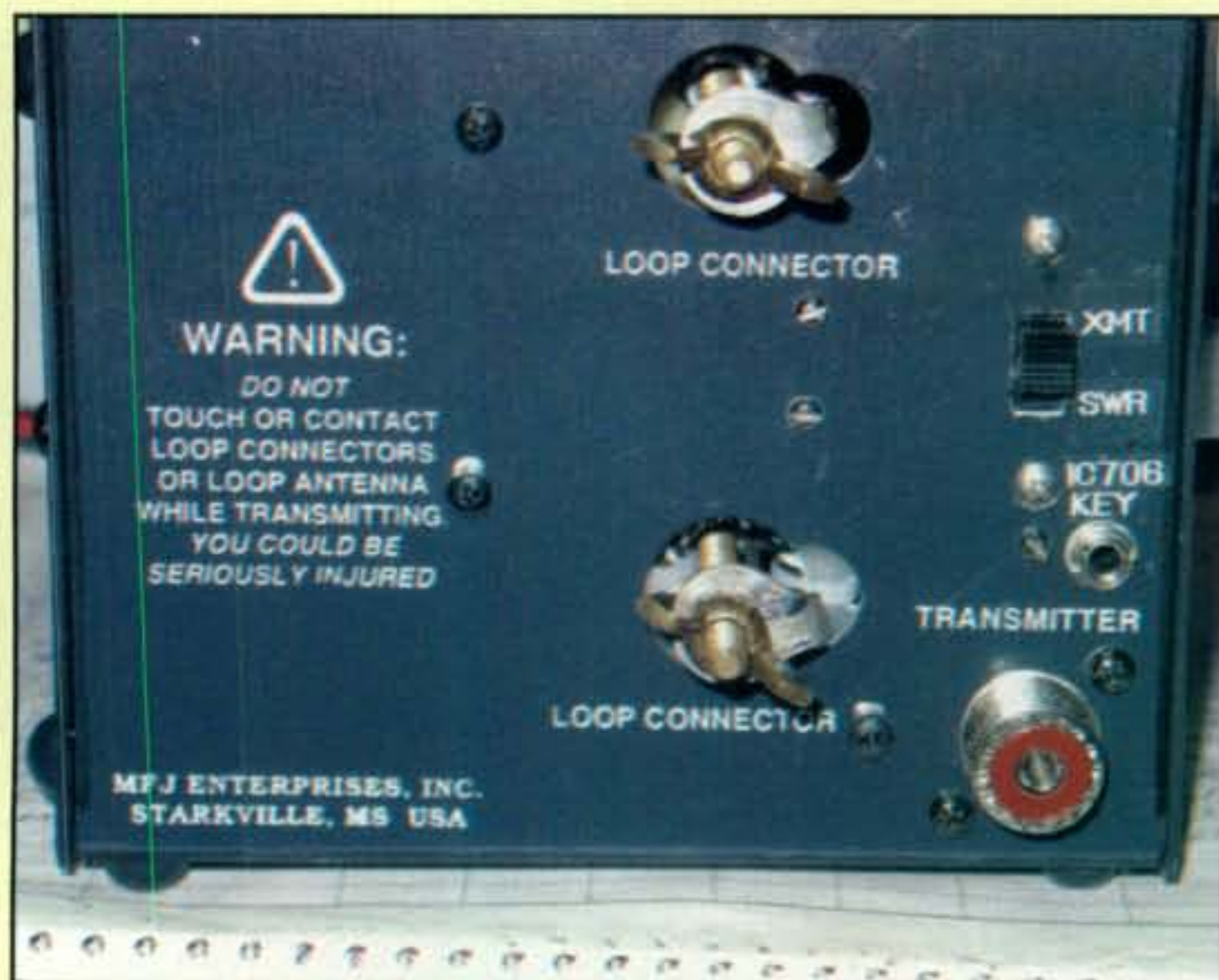
Photo D—Rear view of the MFJ-935B showing added switch and socket for the Tenna-Tune interface.
