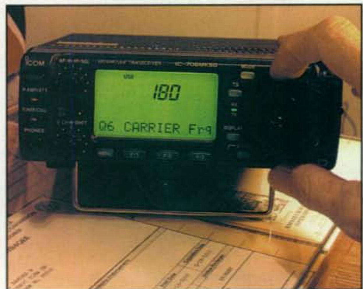
Photo B— Response on some transceivers is adjusted by shifting the transmit-carrier oscillator's frequency, as on this ICOM IC-706. Here we have set the carrier frequency plus 180 Hz of center frequency to emphasize highs and give the audio a bright, clear sound.
