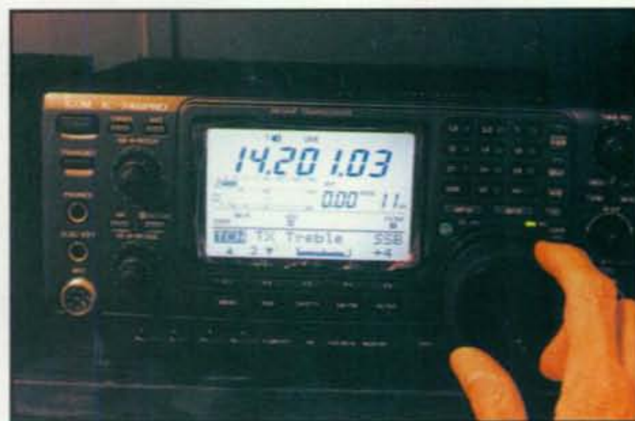
Photo A— Precisely adjusting a transceiver's equalizer for great transmit audio can be a bit challenging, but it is always worth the effort. Here we are setting the transmit treble response on an ICOM IC-746Pro while listening to results on an external receiver with a wide passband and high-fidelity earphones. (Discussion in text.)
