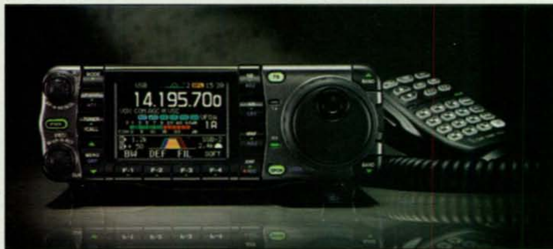
The ICOM IC-7000 mobile radio is an HF rig that also includes the 50-, 144-, and 430-MHz VHF/UHF bands.
