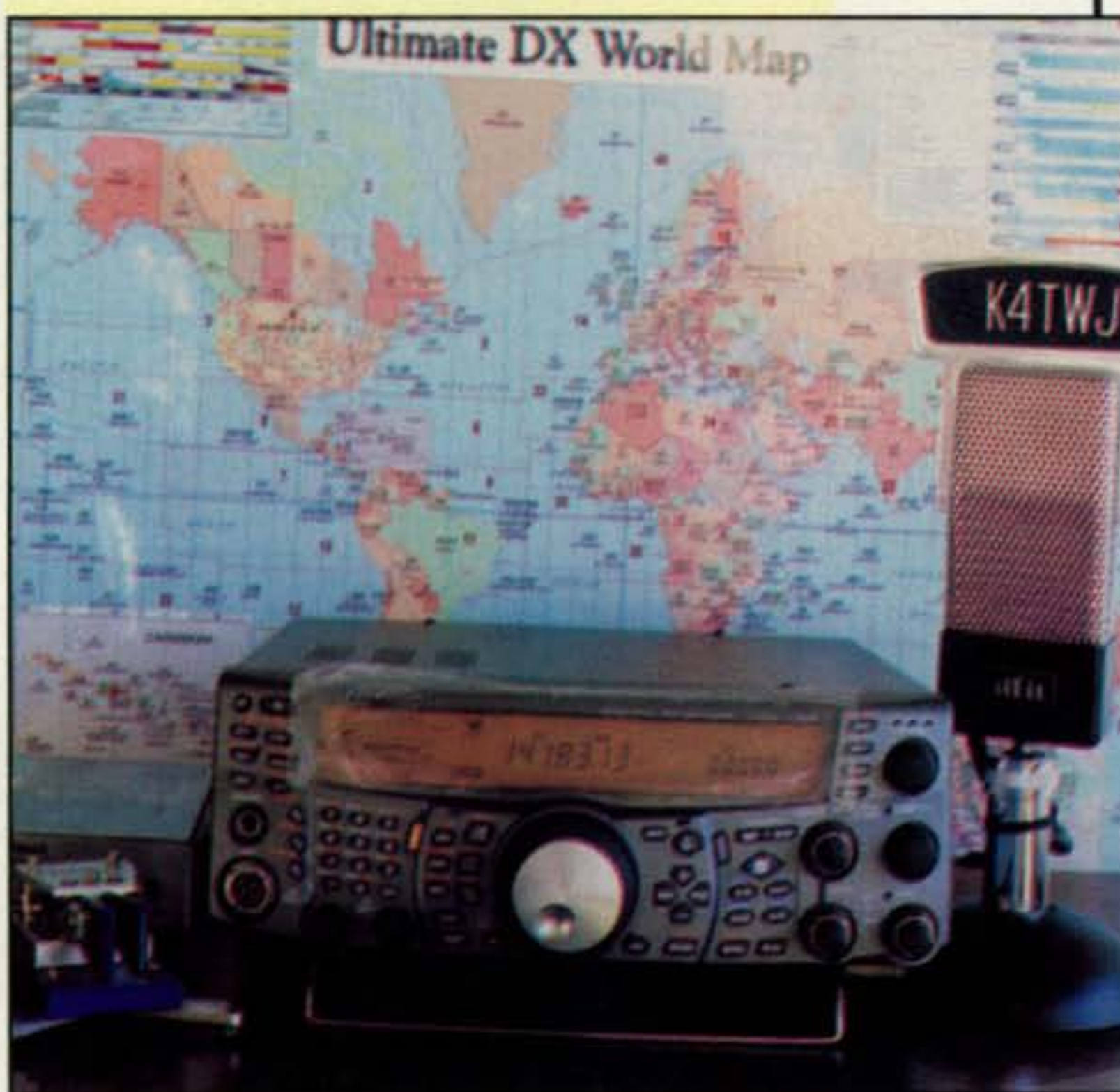
Photo 1—An HF setup need not be large and lavish for successful DXing, but it should encourage a good mindset. A world map marked with time zones and prefixes of various countries supports that mindset and makes a good operating asset to boot. With regard to a rig, a midsize, mid-priced transceiver such as this Kenwood TS-2000 is an excellent choice.
