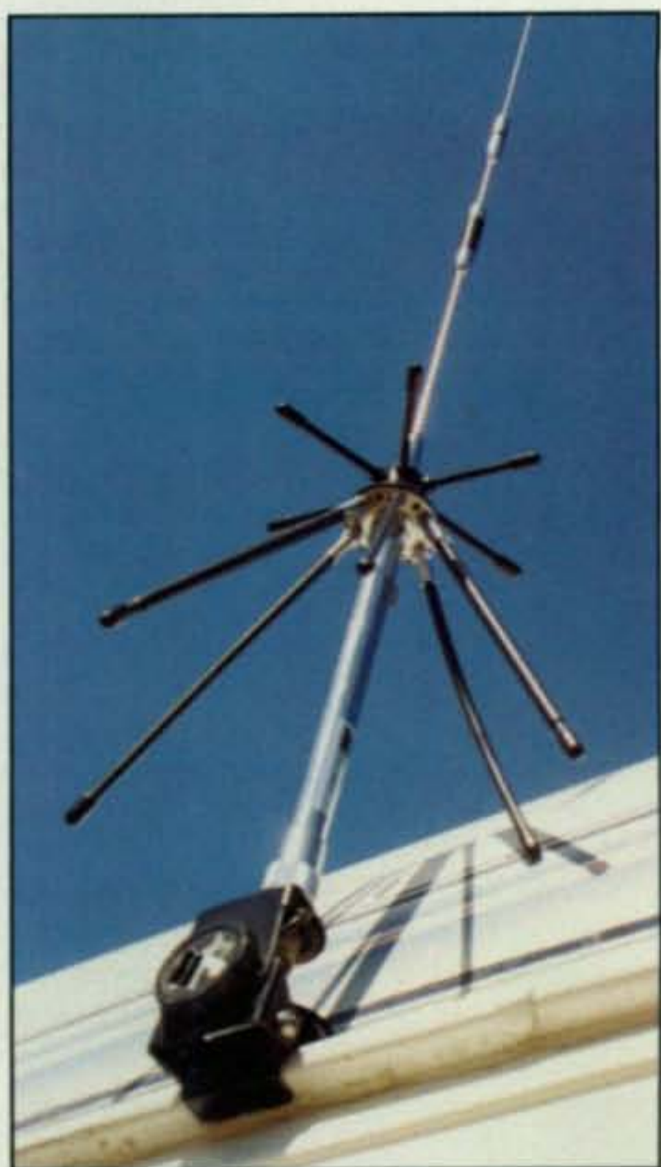
Photo F— WB6NOA got good results with the discone mounted on his van, compared with single-band antennas for the ham bands it covers. (See text for details.)
