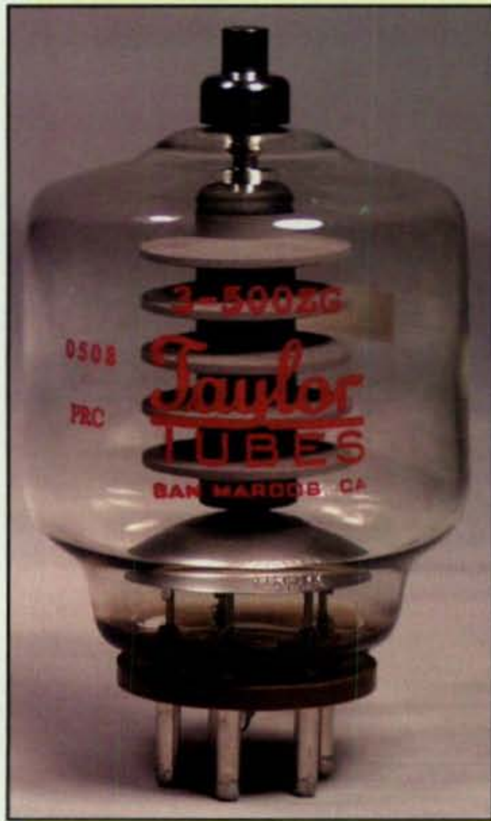
Photo B— Our column's main stars proudly stand up for an encore. On the left is the ever-popular glass-envelope 3-500Z (5"L x 3.5"D), and on the right is the world-famous 3CX-1500A7 (3.51"L x 3.38"D). (Photo courtesy Richard Stubbs, KC5NSZ of MFJ Enterprises)
