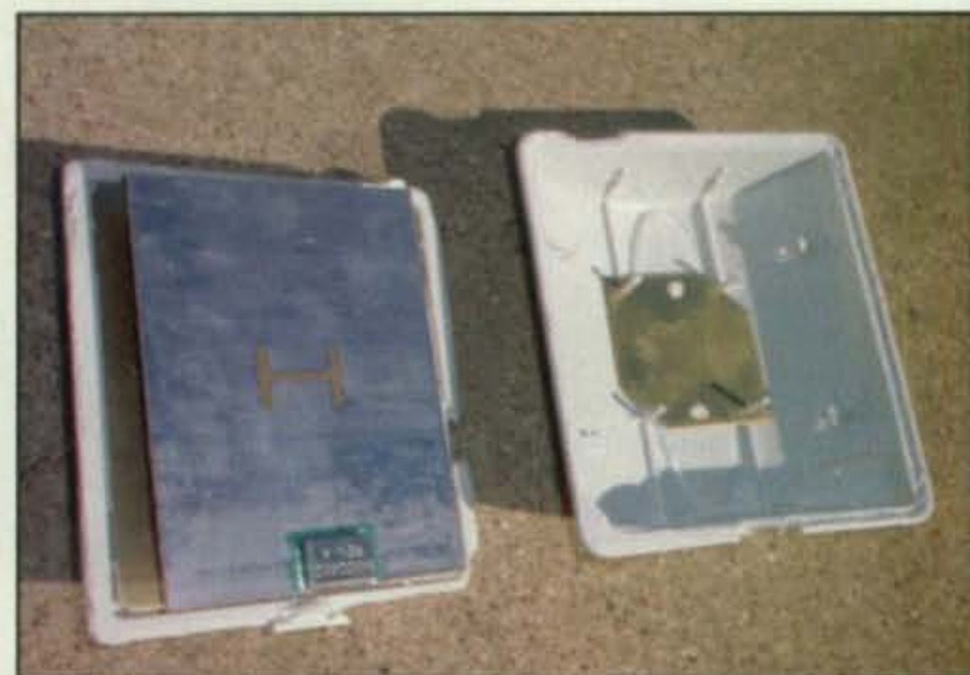
Photo B— The 2.32-GHz circularly polarized patch and slot inside the Sirius antenna.
