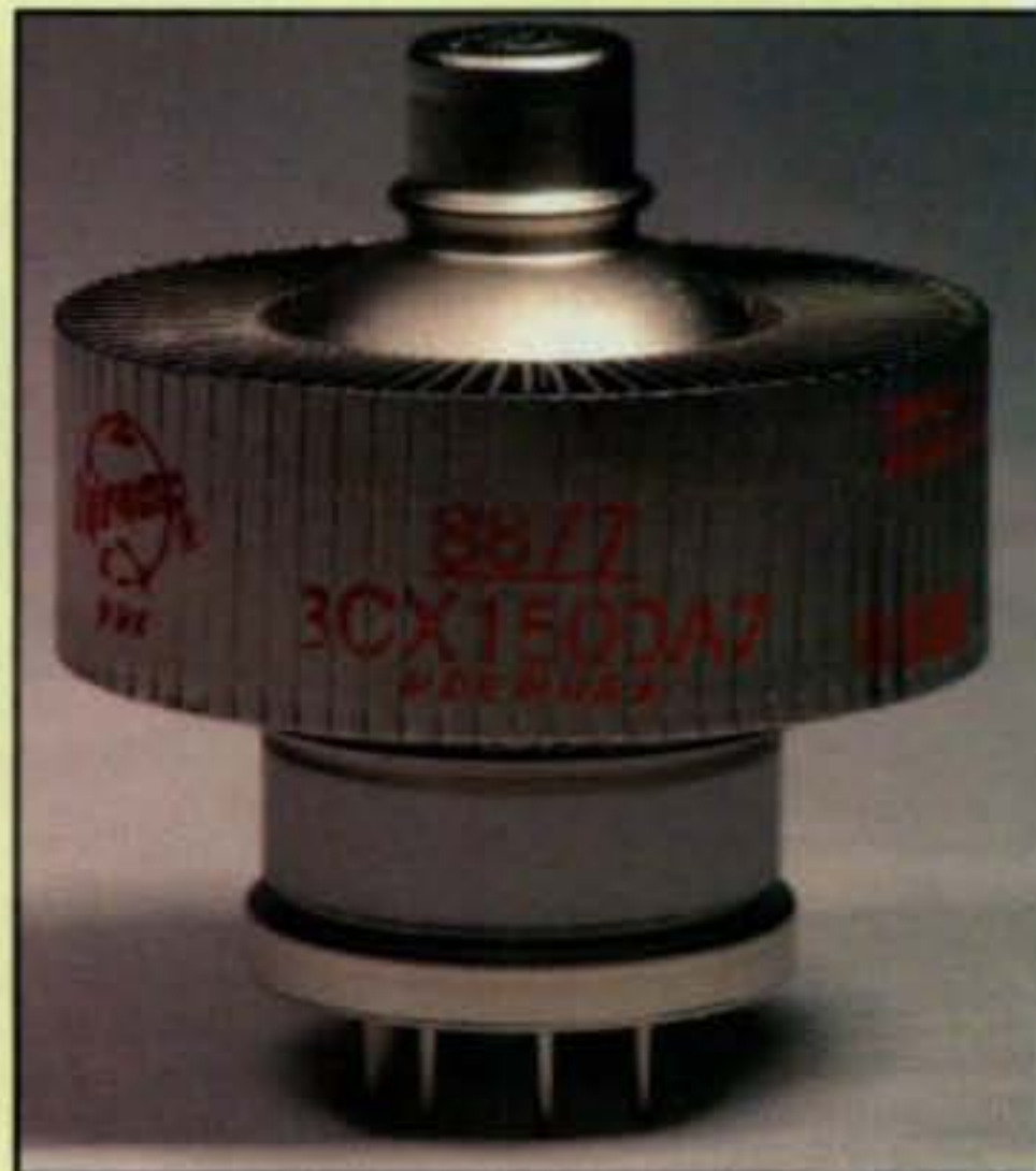
Photo B— Our column's main stars proudly stand up for an encore. On the left is the ever-popular glass-envelope 3-500Z (5"L x 3.5"D), and on the right is the world-famous 3CX-1500A7 (3.51"L x 3.38"D). (Photo courtesy Richard Stubbs, KC5NSZ of MFJ Enterprises)
