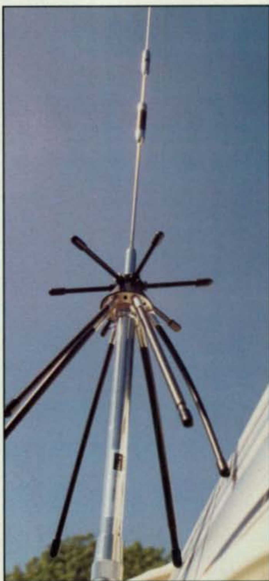
Photo E— The Diamond D220 discone antenna is smaller than many similar antennas and is designed for mobile as well as fixed-station use. It covers 100-1600 MHz on receive, with transmit capabilities on 2 meters, 70 centimeters, 900 MHz, and 1200 MHz.
