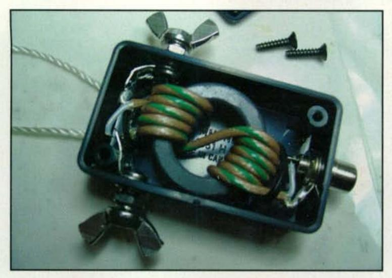
Photo D– The balun (see text) performs double duty, helping minimize RF "bites" in areas with poor or no ground, and providing a center support and feedline connection point for the antenna.
