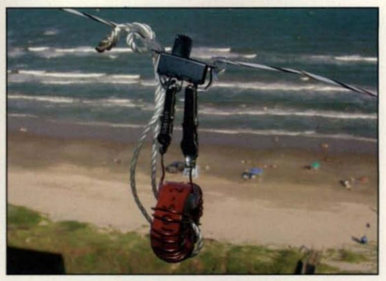
Photo G-With the 40-meter coil in place, the antenna is ready to "rock" on 7 MHz. Changing bands simply requires unclipping the coil.
