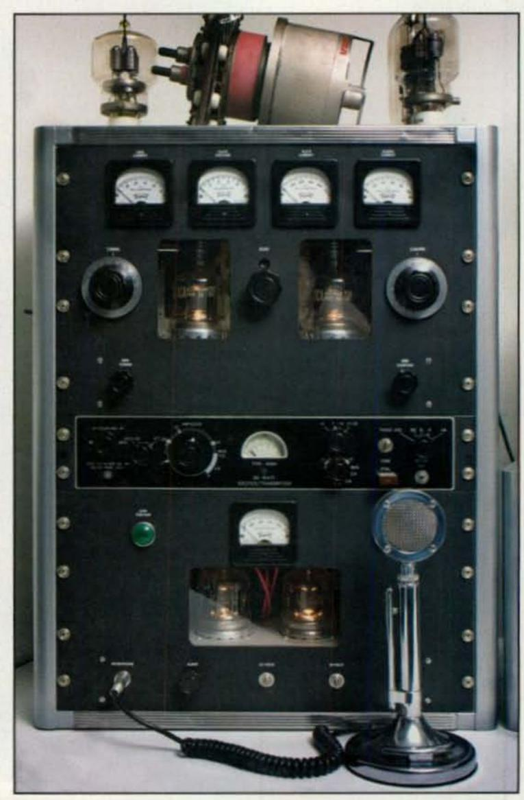
Photo 3— This desktop AM transmitter runs 500 watts with a pair of 4-125As. The tubes on top are for decoration only!
