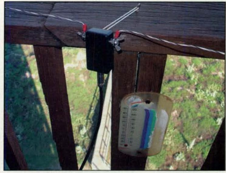
Photo I—This is a close-up of the feedpoint, showing the balun string wrapped around a stray nail to provide center support, and the RG-174 coax feeding the rig.
