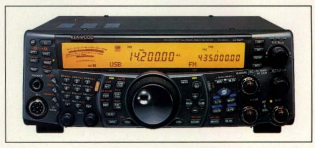
Photo C— A mid-size transceiver may easily represent the best overall mix of special operating features, portability, and cost. This Kenwood TS-2000, for example, is factory supplied with a full IF-level DSP filter system, digital AGC, automatic antenna tuner, plus other "big rig" features. It is also satellite ready and equipped for deluxe remote-controlled "Sky Command" HF operation using a handheld talkie as discussed in the text. (Photo courtesy of Kenwood U.S.A.)
