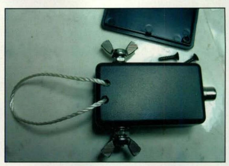
Photo E- A loop of nylon cord through the back of the balun box makes it easy to hang up this antenna just about anywhere.
