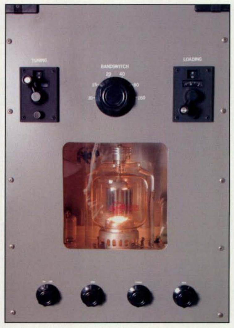
Photo 5– Front-panel detail of the 4-1000 transmitter's RF deck. The viewing window for the tube is a signature Howard design feature.
