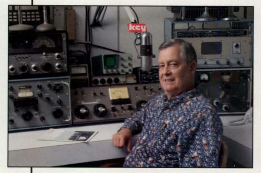
Photo 1- The main AM operating position at WA4KCY. Equipment includes several very desirable classic receivers, a Gates broadcast audio mixer, and even a vintage Conelrad monitor. (Photos © Joe Veras, 2006, all rights reserved)
