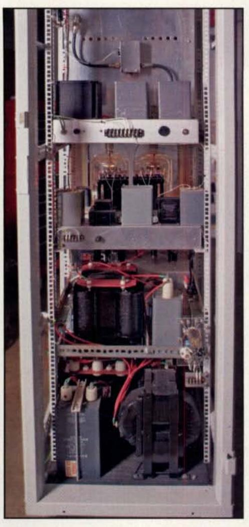
Photo 6- The business end of the 4-1000 rig. The RF deck is behind the cover at the top.
