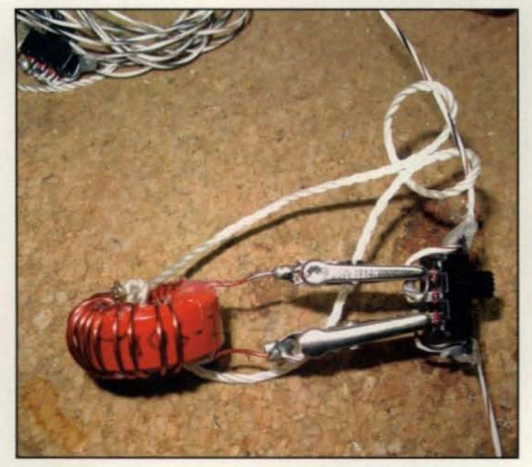
Photo F— Putting a 20-meter antenna on 30 and 40 meters requires the addition of loading coils, clipped across the 10-meter switch. This photo shows the 30-meter coil.
