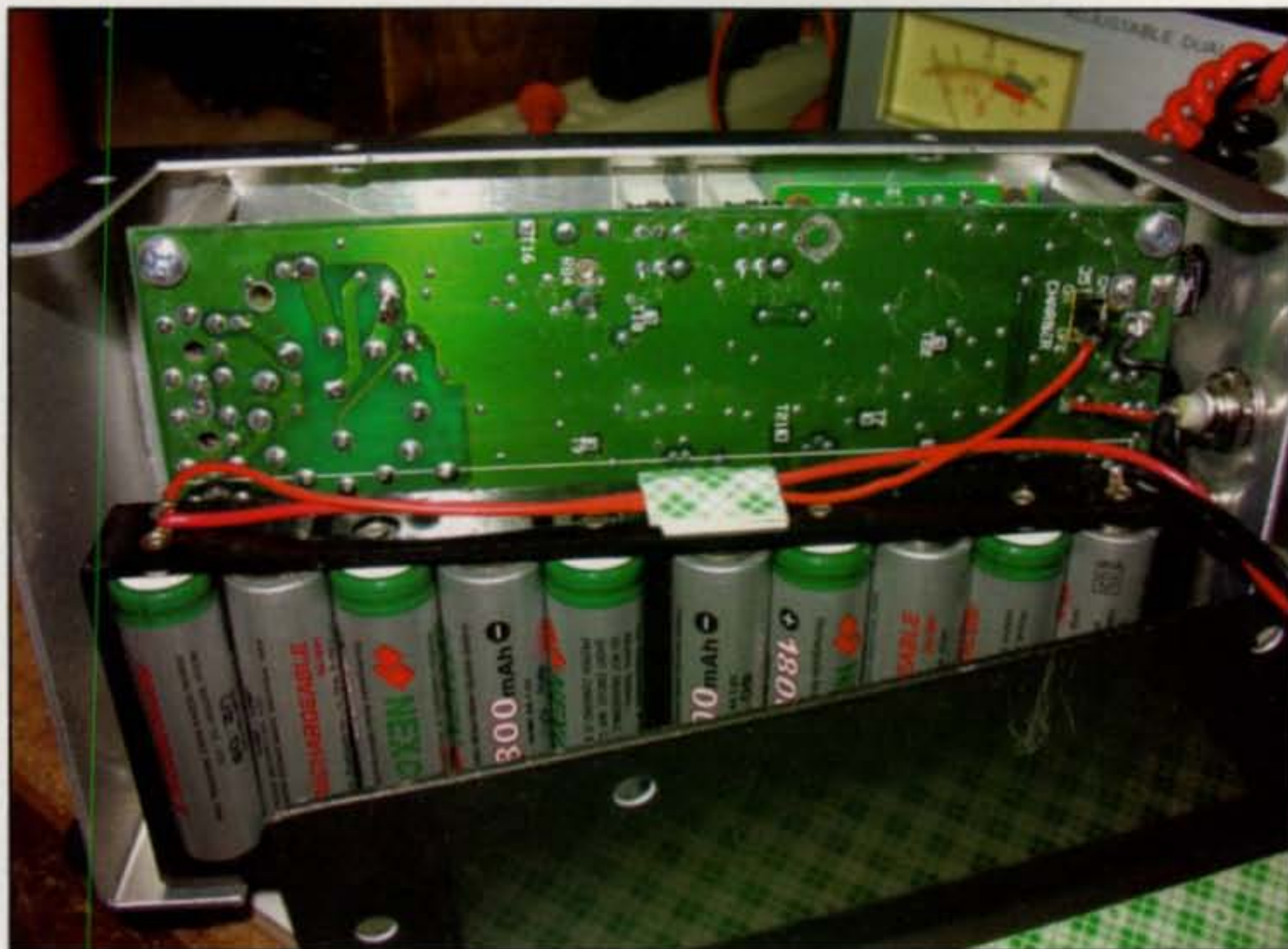
Photo D— Wire routing between the battery pack and the fast-charge jack.
