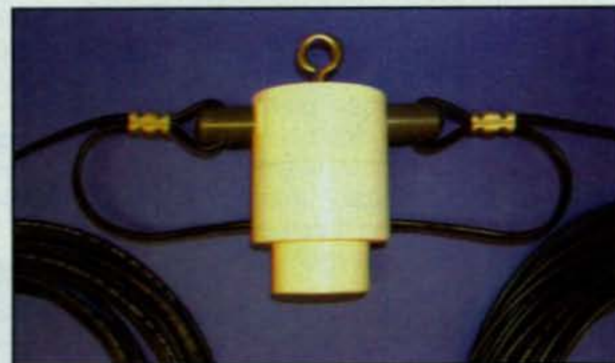
Photo C— The custom designed, integral 6:1 balun used in the Alpha Delta Model DX-OCF multiband antenna is permanently potted in a special epoxy potting compound for moisture- and corrosion-free operation. (Photo courtesy of Alpha Delta Communications)
