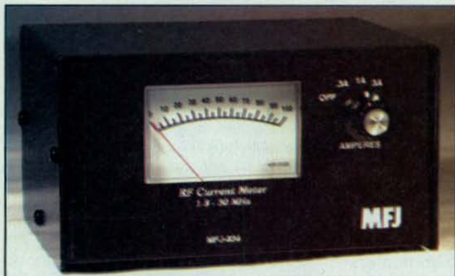
Photo G—The MFJ-834 Coax In-Line Calibrated RF Ammeter can be connected between your antenna and tuner/transmitter/amplifier to measure antenna feedline current in three calibrated ranges. You can use the MFJ-834 to determine the best antenna tuner settings and to compare various tuners. (Photo courtesy of MFJ)
