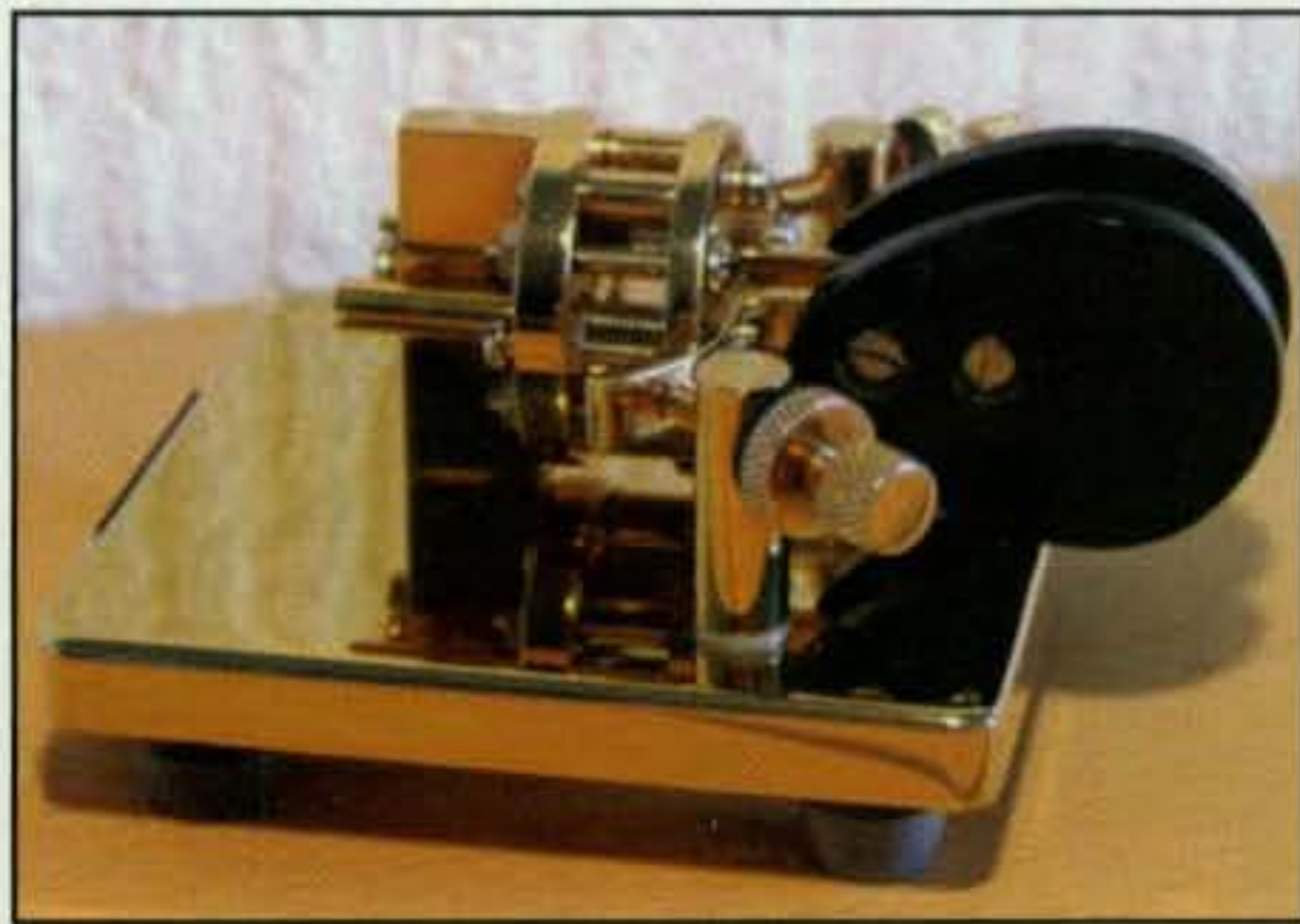
Photo 1— G4ZPY's world-famous keys and paddles vividly reflect the glitz and glamour side of amateur radio telegraphy. Shown here is his popular "VHS" high-speed iambic paddle. It sports a high-luster 3-inch brass base, brass and chrome mechanism with fine adjustments, silver-to-silver contacts, and custom fingerpieces. Nice! (Photo courtesy of Gordon Crowhurst, G4ZPY)
