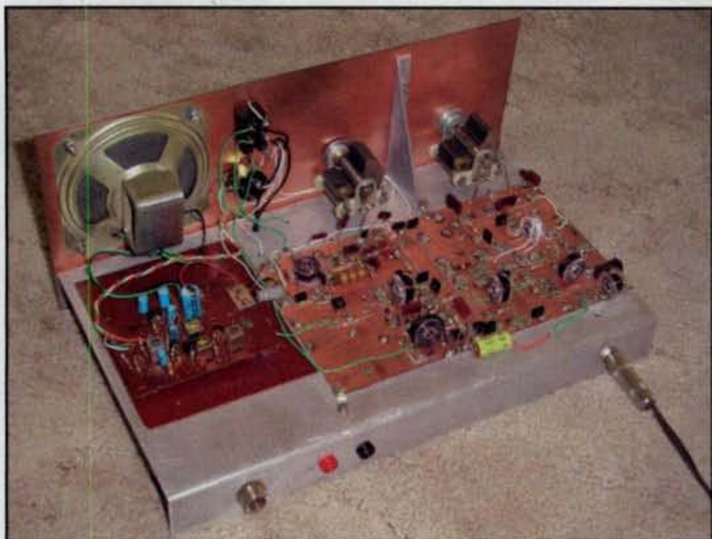
Small pieces of PC-board material hot-glued to the unetched PC-board base provide all the necessary connections for the various components.
