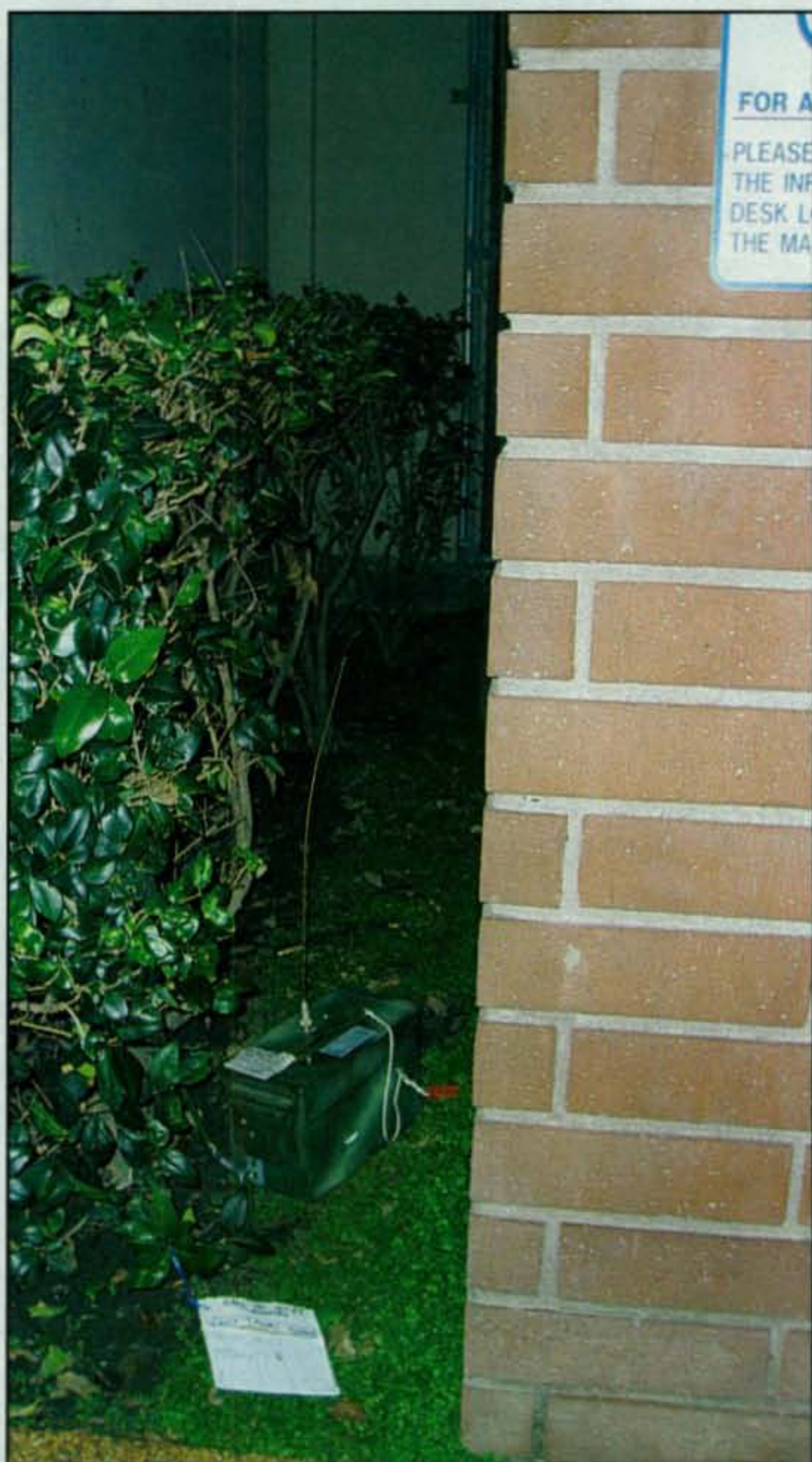
Surplus ammunition boxes make great waterproof enclosures for unattended fox transmitters (and decoys, too). With room inside for a handie-talkie, controller/timer, and a big battery, they are suitable for both mobile and on-foot transmitter hunts. (Photo by Joe Moell, KØOV)
