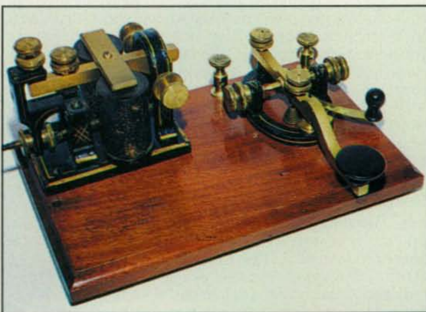
Photo 13— Check out this extra-classy KOB made by Jerome Redding. It features a rare Camelback key and a compact sounder, both with custom pinstriping and a beautifully finished wood base. Nice!
