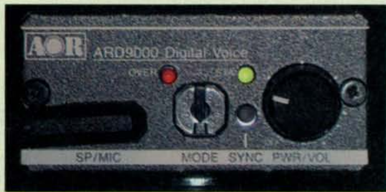
In digital mode—the default startup mode—the LED glows green in receive and flashes when a digital signal is being received.
