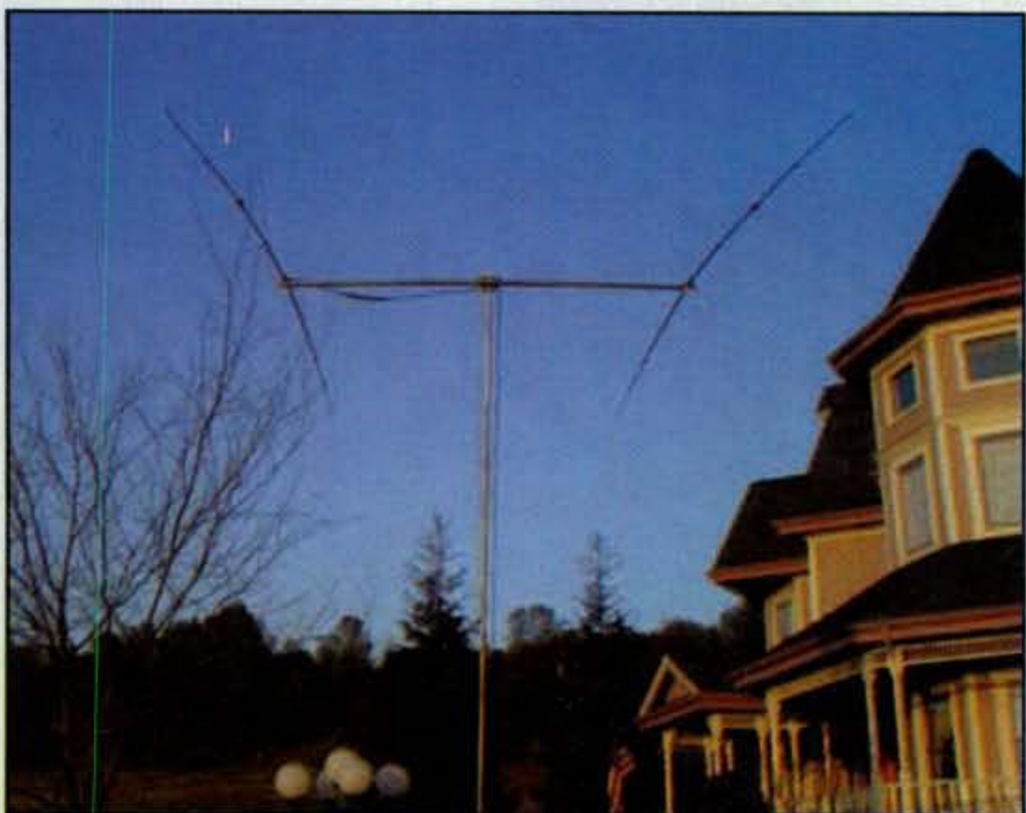
Photo F— The Super Antenna two-element Minibeam assembled and ready for action on 20 meters. The boom is 84 inches long and tip-to-tip element length is approximately 210 inches. It is a neat medium-gain antenna one person can handle/erect and remove without assistance. It is the perfect answer for low-profile hamming.
