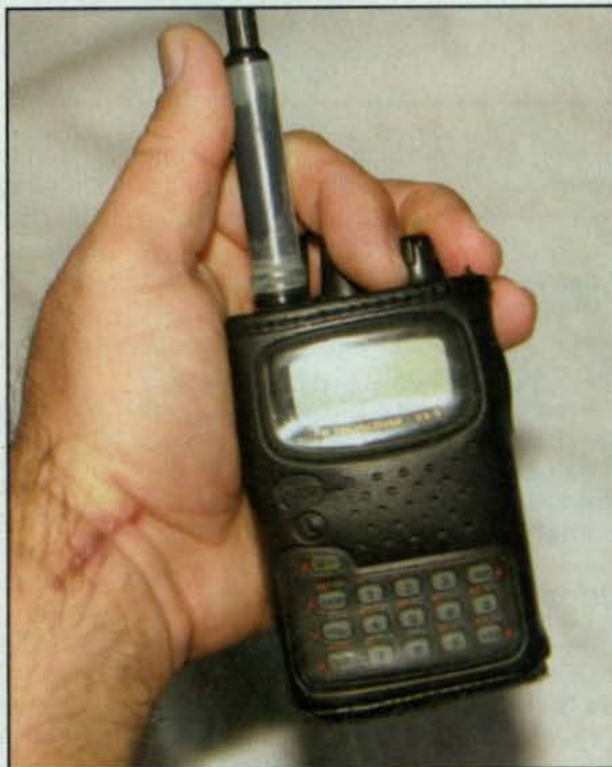
Photo 3— When using an extended, gain-type antenna on your HT, remember to "cradle" the radio in your hand to prevent damage to the antenna connector.
