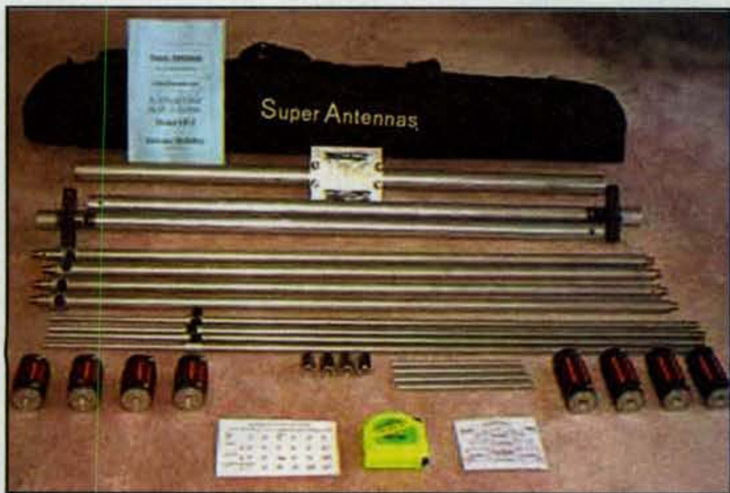
Photo E— The Super Antennas' two-element Minibeam laid out and ready for quick on-the-spot assembly. Everything—including loading coils, balun, boom-to-mast plate, and even a tape measure—stores in that 36-inch-long shoulder-strap bag. The antenna goes together in approximately 20 minutes and can be set for 20-, 17-, 15-, 12-, 10-, or 6-meter operation. (Details in text.)
