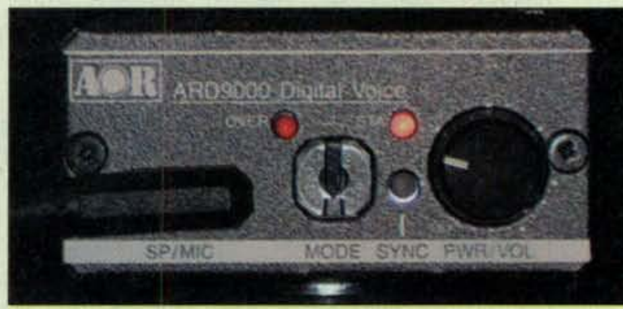
In analog transmit, the LED glows red.
