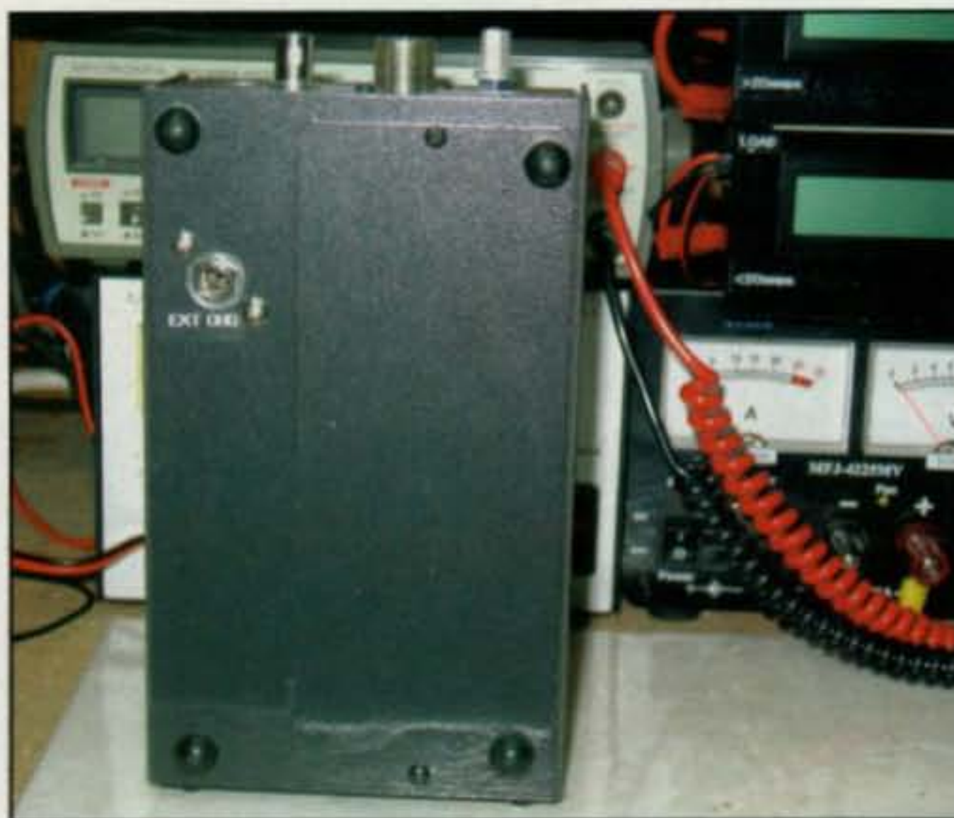
Photo B— The location of the charging jack on my 259B. Note clearance around the jack to permit mounting as described in text.
