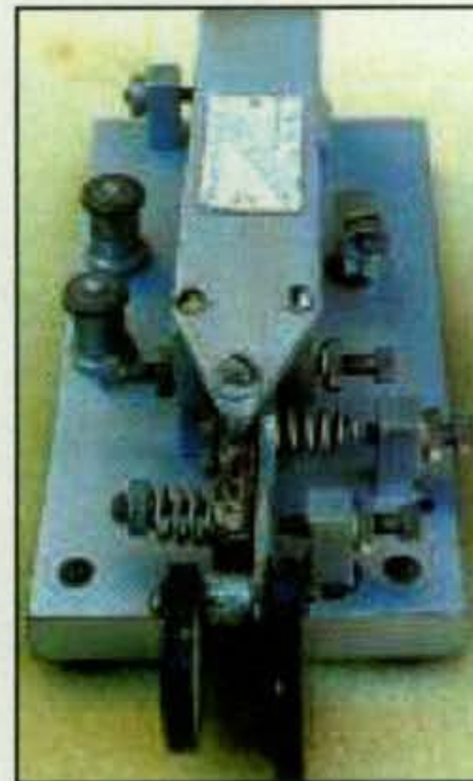
Photo 7— Here it is! The first and probably only available picture of the rare and elusive Ingram Master Key made in Perth, Australia. What a doll it is, with a metal nameplate atop its protective top shroud plus all the traditional bug adjustments. Look carefully and you will also notice this is a left-handed model. (Photo courtesy of Ron McMullen of Australia)
