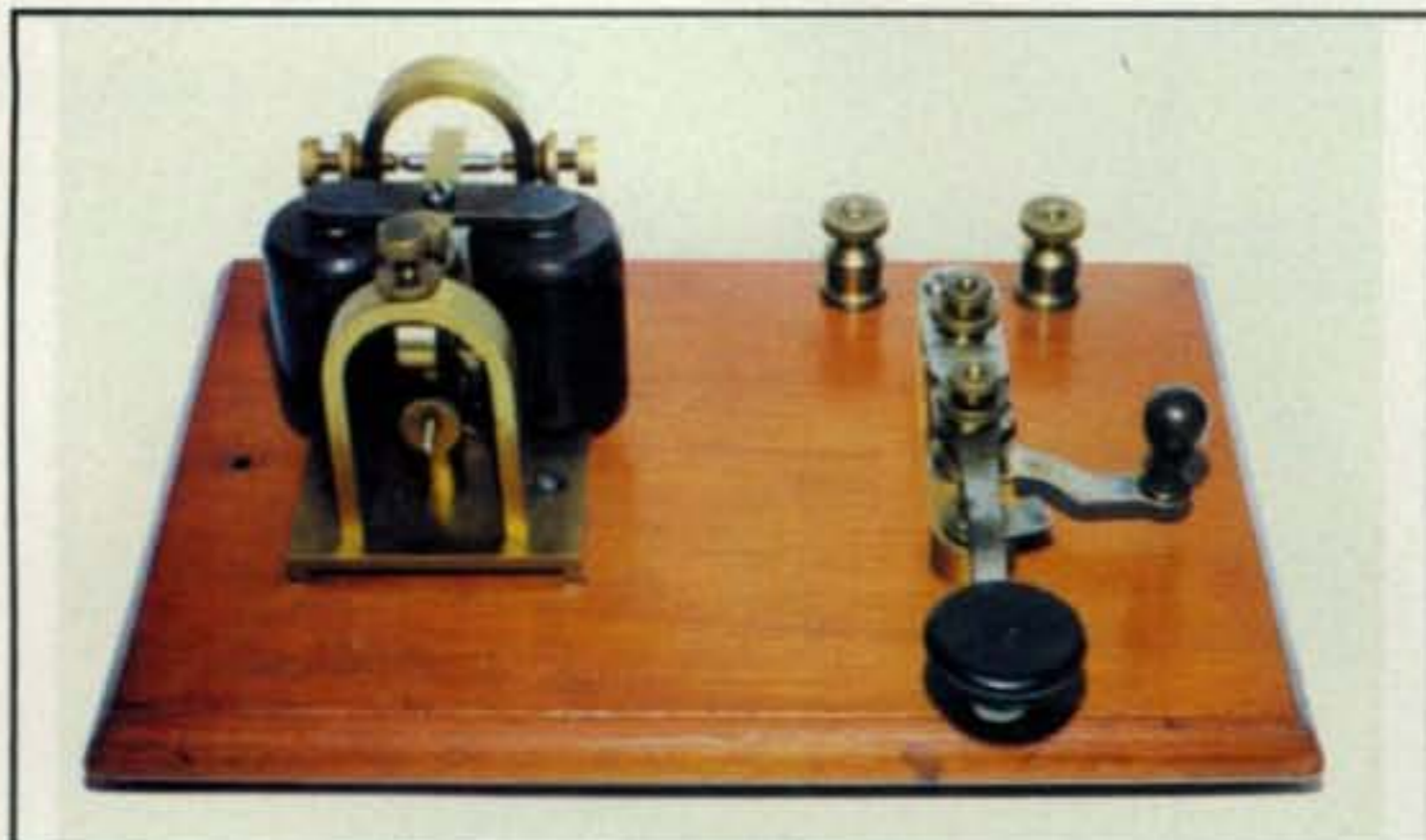
Photo 11— A KOB, or Key with sounder On Base, is another important part of a key collection. KOBs served as portable telegraph setups one could carry between jobs or use for in-field work when required. The one shown here sports an unusual Steiner key and was probably made during the late 1800s. (Photo courtesy of key collector extraordinaire K9WDY)
