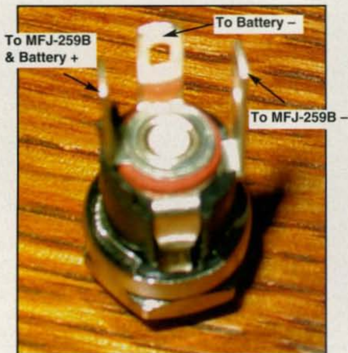
Photo A— The fast-charge jack and connections of the three necessary wires.
