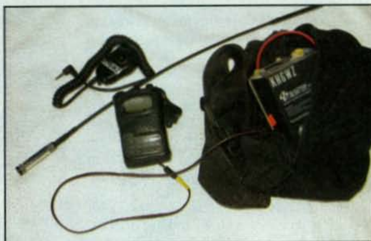
Photo 2— To extend operating time, I equip my little Yaesu VX-5 dual-band HT with an external gel-cell carried in a small fanny sack. The fanny sack also includes several essential items, such as snacks, medications, a spare speaker-mic, and a small flashlight.
