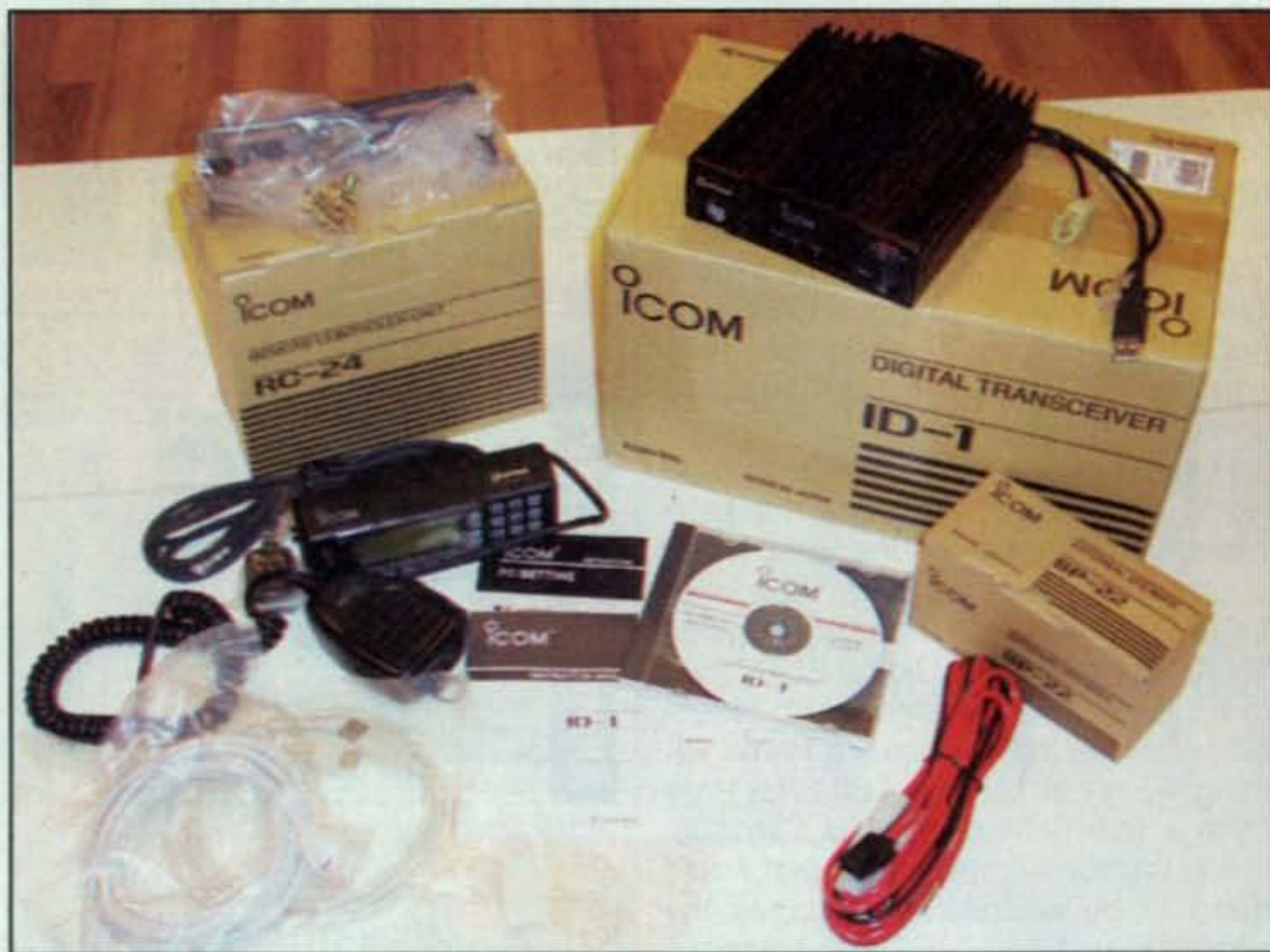
Photo 2— When you open the box of an ICOM ID-1 D-Star Transceiver, there's some stuff you might not expect, such as Ethernet and USB patch cables and a CD-ROM for programming the radio. As W2VU said in February's issue, "This ain't your father's radio." I can't wait to get it on the air.
