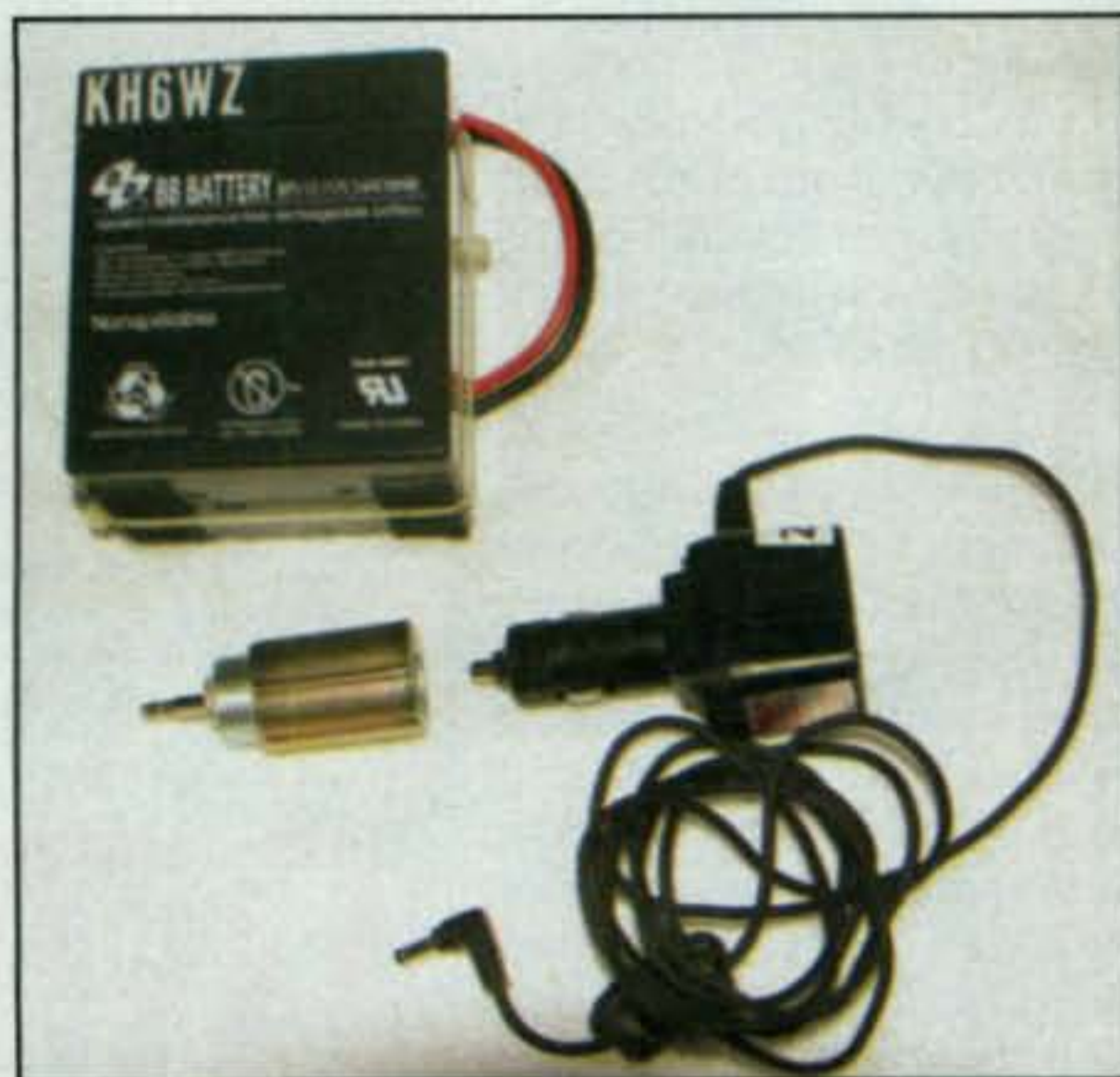
Photo 1— An easy way to make an external battery pack for your HT is to use the manufacturer's accessory cigarette-lighter cord, a lighter socket, some wire, and a small rechargeable lead-acid gel-cell. (Photos by the author unless otherwise noted)
