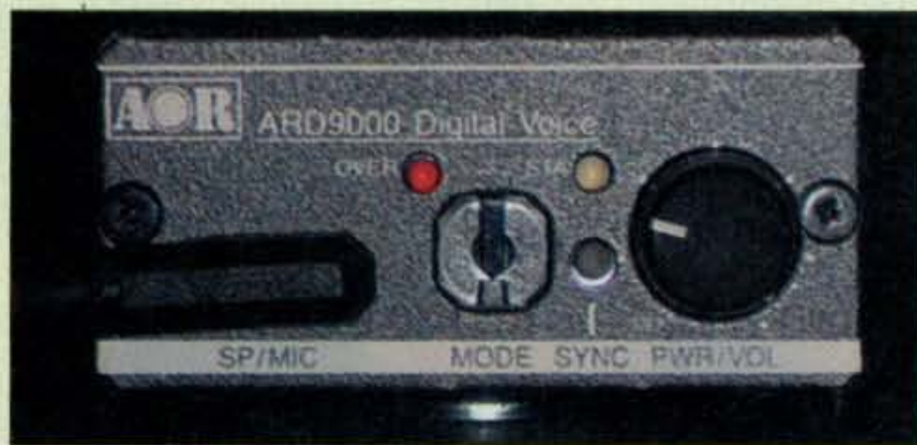
In analog receive mode, the LED marked "STA" is not lit.
