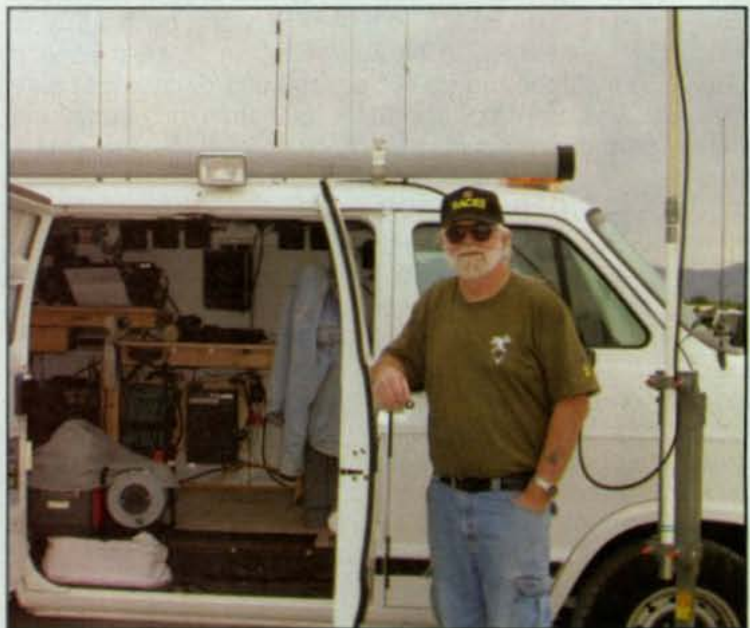
Photo 8— Peter Shores, AD6TN, manned the portable communications command post in the city of Pahrump, NV, the mid-point of the race. Peter's communications van is equipped to operate on the HF to UHF ham bands as well as business (Land Mobile Radio) frequencies. Large antennas are mounted on masts to boost radio performance in both transmit and receive.
