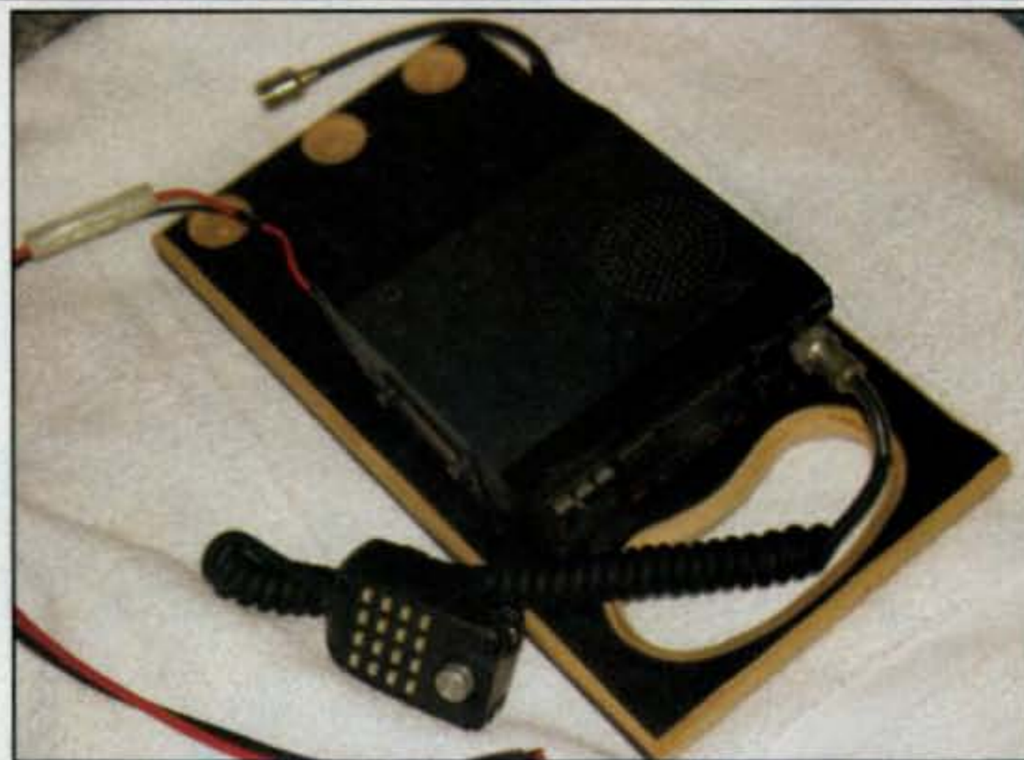
Photo 4— This "portable-mobile" station can be removed and installed into another vehicle in less than five minutes. The scrap-wood board has a comfortable handle to make it easy to carry. A magnet-mount antenna is used on the vehicle roof or the trunk lid to complete the station.
