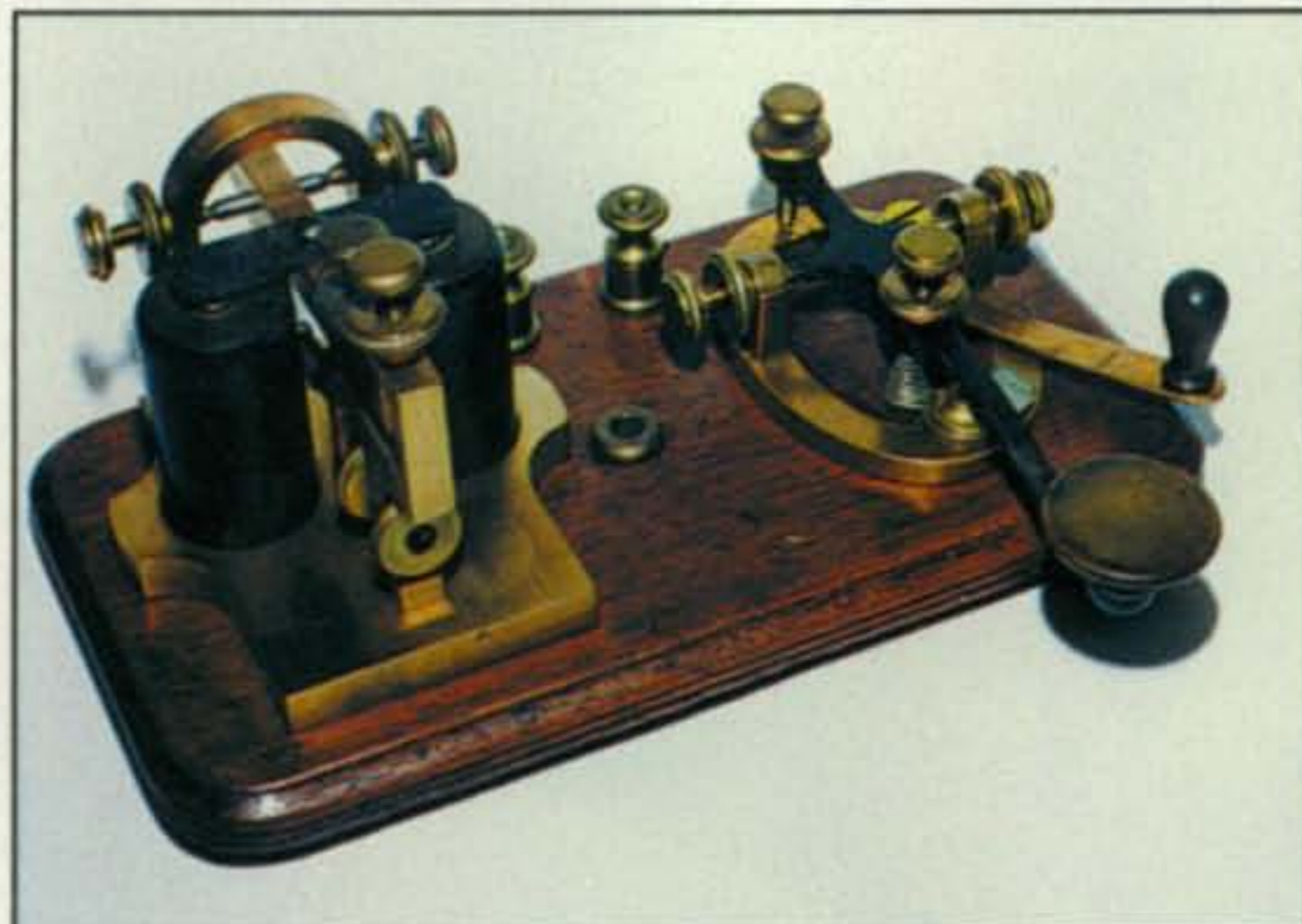
Photo 12— This neat KOB was made during the early 1900s by the Altoona Shops of places unknown, but it is still a piece of fascinating telegraphic history. (Photo courtesy of K9WDY)
