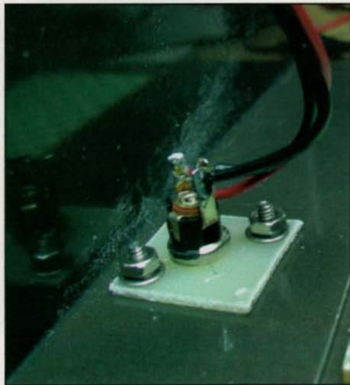
Photo C— Here's the jack with wires soldered on and mounted on a piece of insulating printed circuit board.
