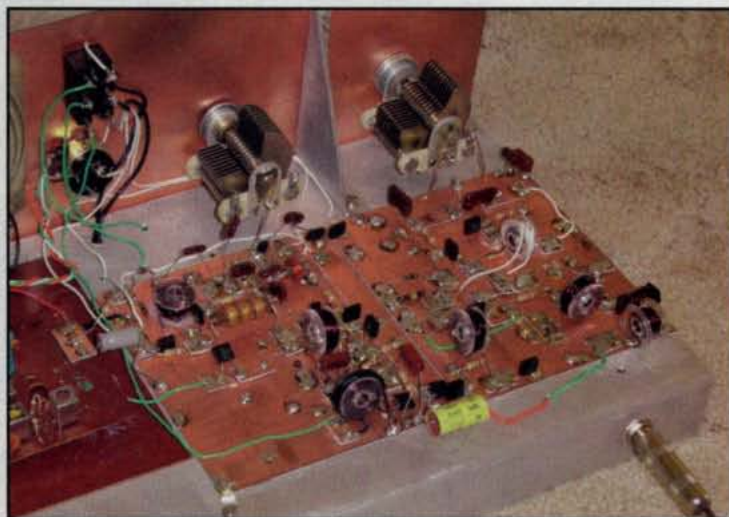
Rear/interior view of the transceiver. Most of the parts were salvaged from an old AM broadcast radio. Note the angled piece of aluminum between the variable capacitors, which provides structural stability essential to the stability of the VFO circuit.
