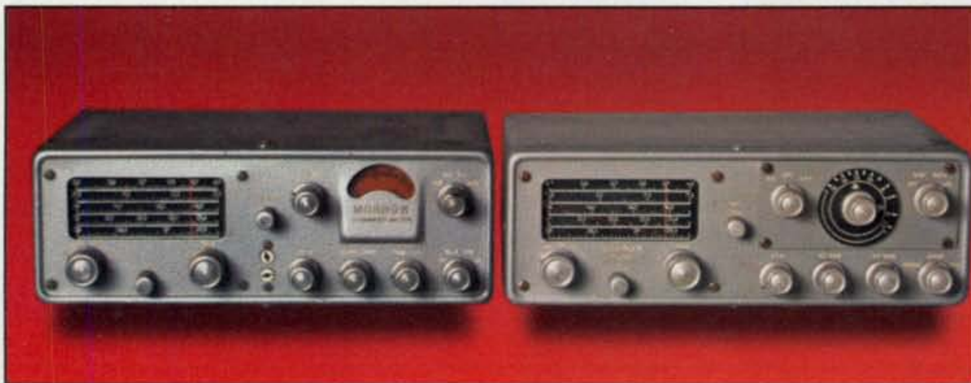
Photo 4— Morrow made a series of matching mobile transmitters and receivers that could also be configured for use as a home station. (The MB-560 transmitter is on left, the Falcon receiver on the right.)
