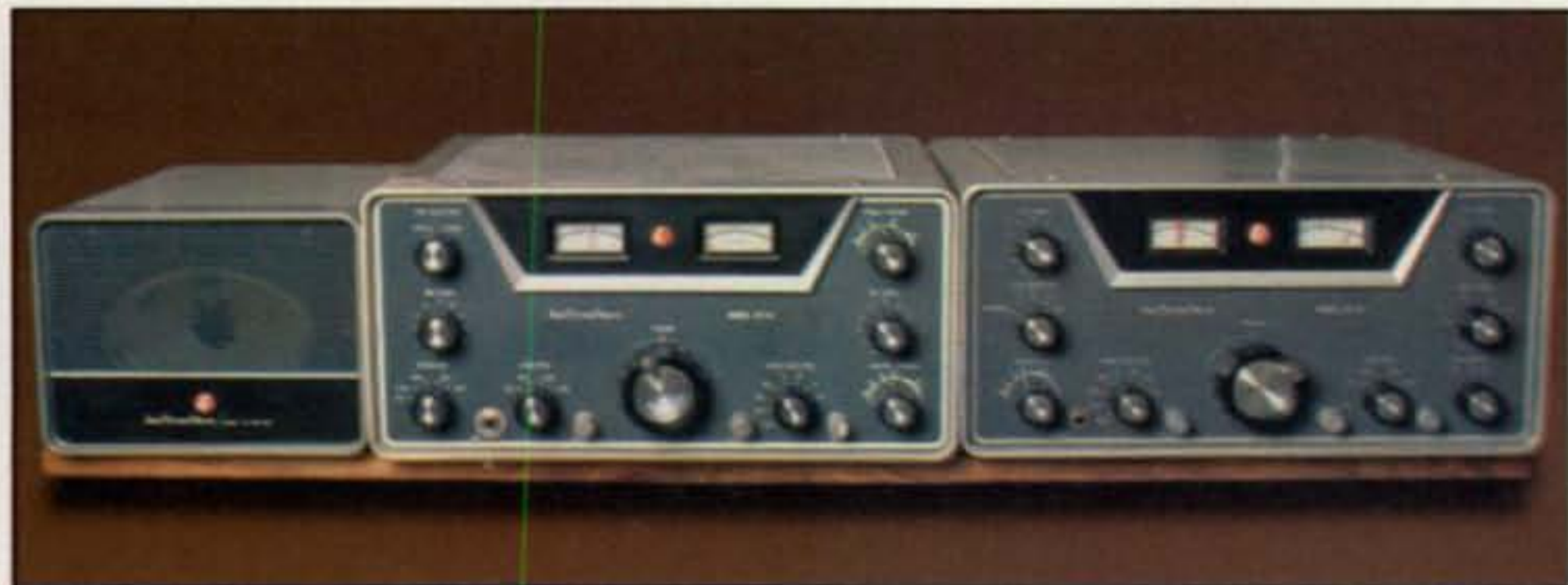
Photo 5- The SX-117 receiver and HT-44 transmitter from Hallicrafters could be slaved together for transceive operation. The unit on the left is the PS-150-120 AC power supply.
