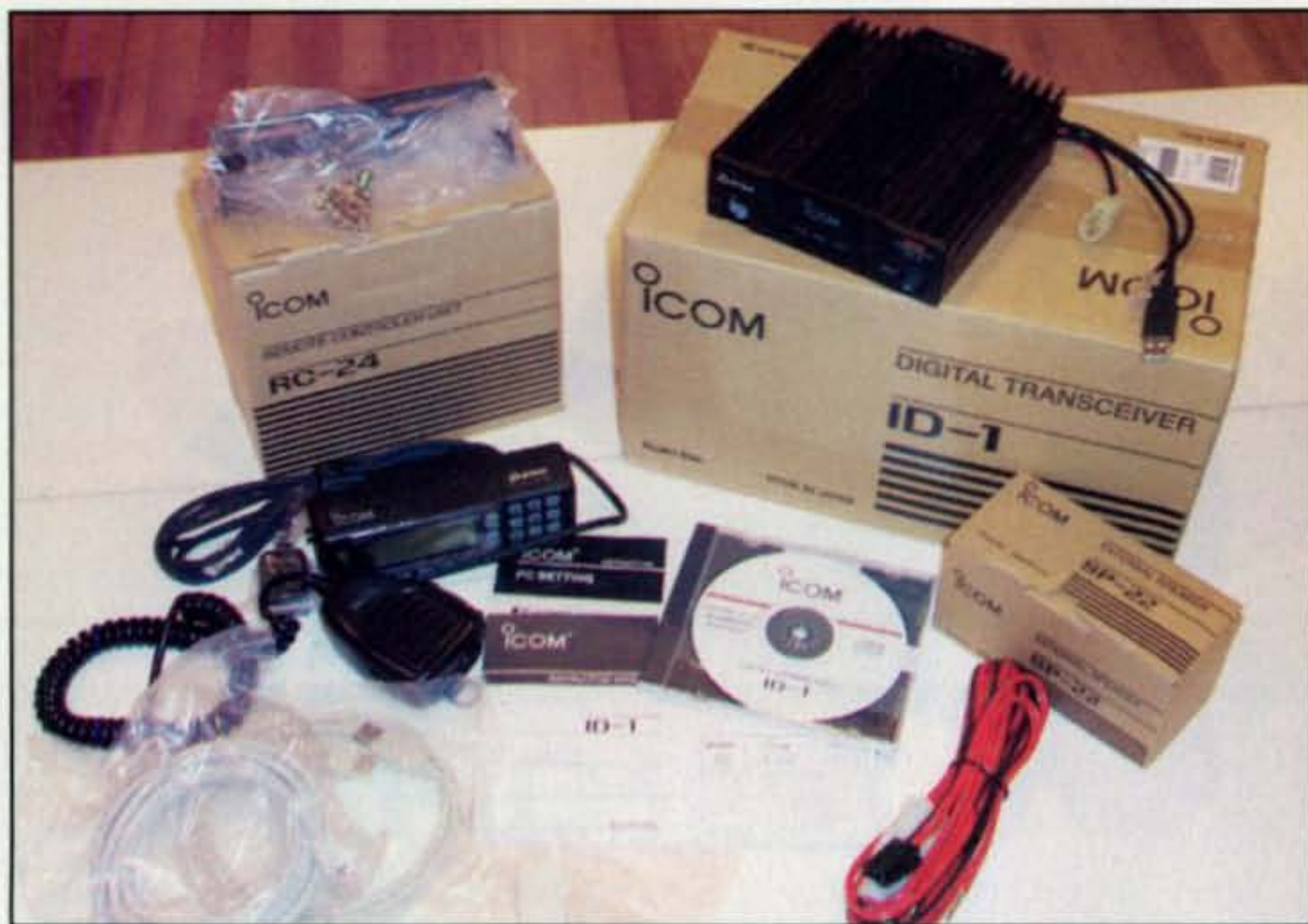
Photo C— The contents of the ID-1 package. Note the USB and ethernet cables, along with the CD-ROM. Take a few minutes to read the manual. This is one of those rare cases where you'll need it.
