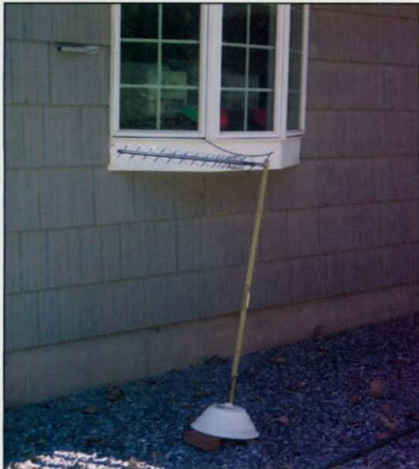
Photo B— My 17-element loop Yagi for 1.2 GHz. Note the computer (seen in photo A) visible through the window. The feedline is only about 7 feet, since it's RG-58. Also note the fancy antenna-positioning system, which uses a stick jammed into the base as a rotator brake.
