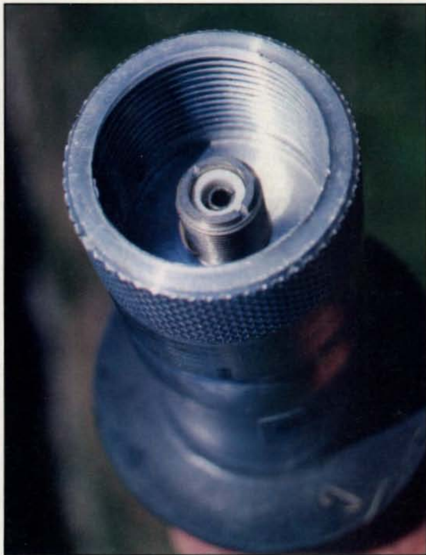
Photo B— The GAM verticals screw onto a standard 1 1/4-inch pipe fitting. Run your coax up the pipe and connect it to the SO-239 connector at the antenna base before attaching the antenna to the pipe.
