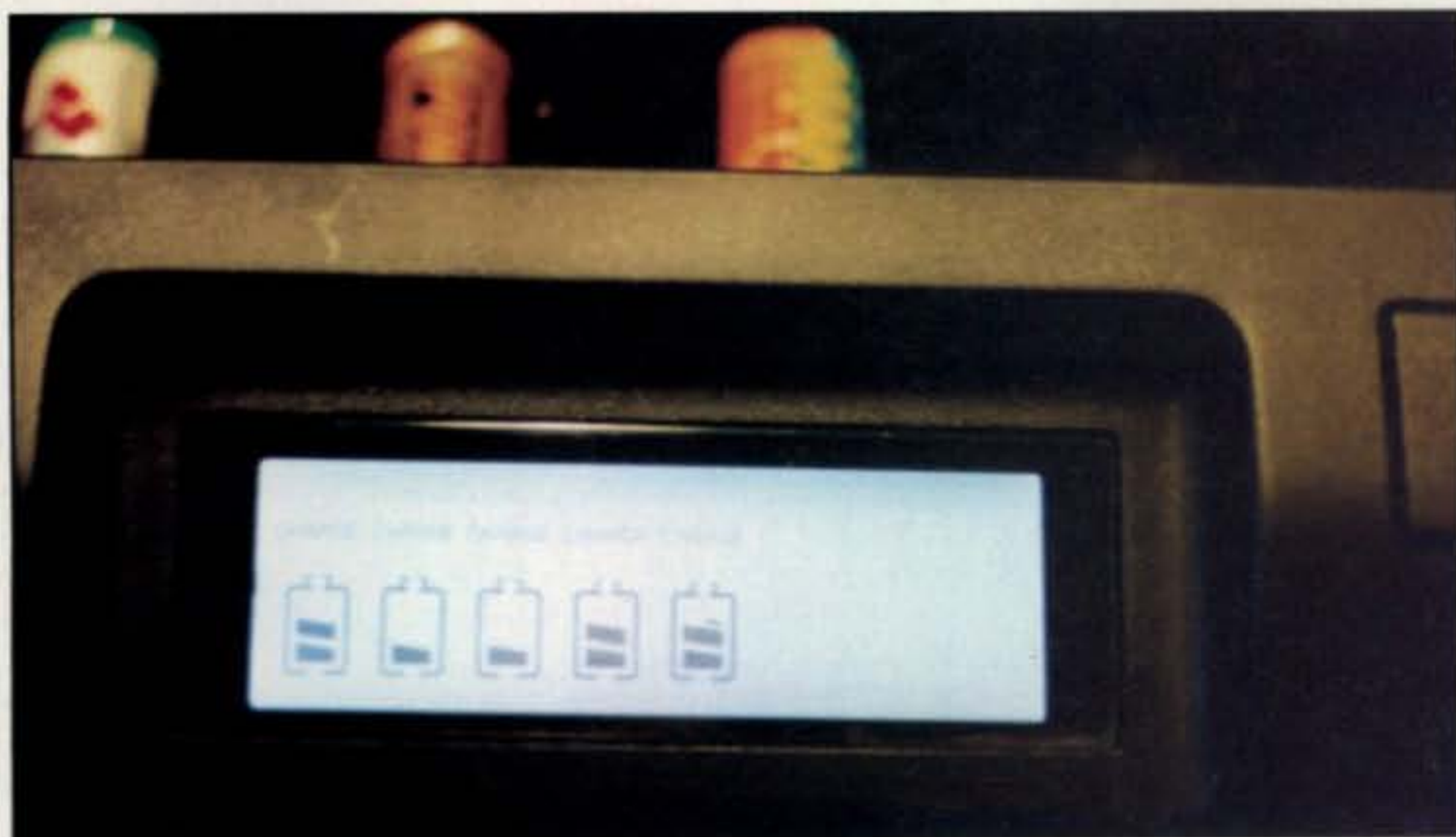
Photo B— The LCD display screen on the charger indicates the status of each cell being charged. It's best viewed at about a 45-degree angle and is hard to photograph clearly. See text and fig. 1 for details on what the different indicators mean.
