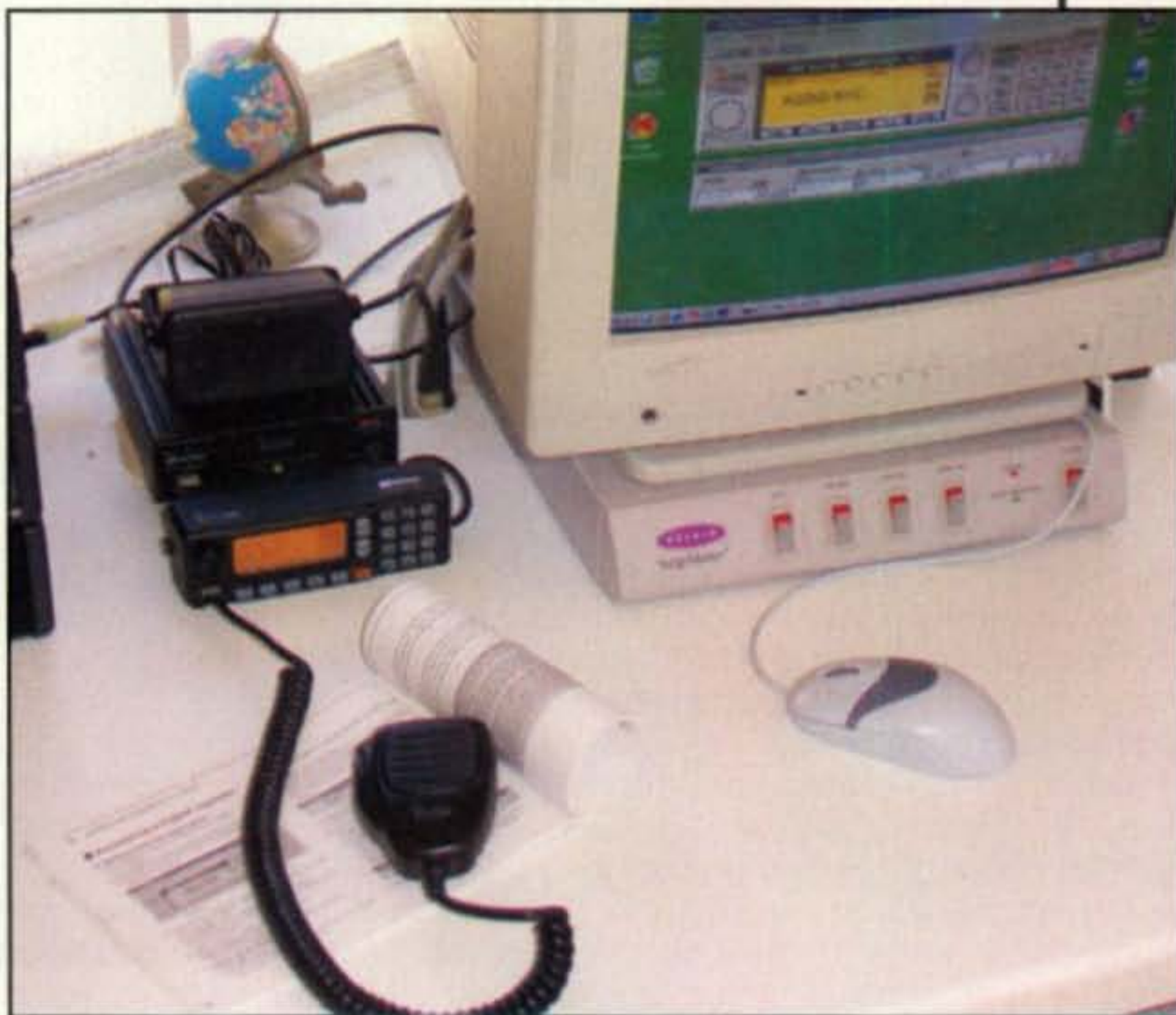
Photo A— The ID-1 1.2-GHz digital transceiver next to my computer. While the computer isn't essential to operating the ID-1, it comes in handy during setup. Since my commute is only a few miles, I operate mostly from home.
