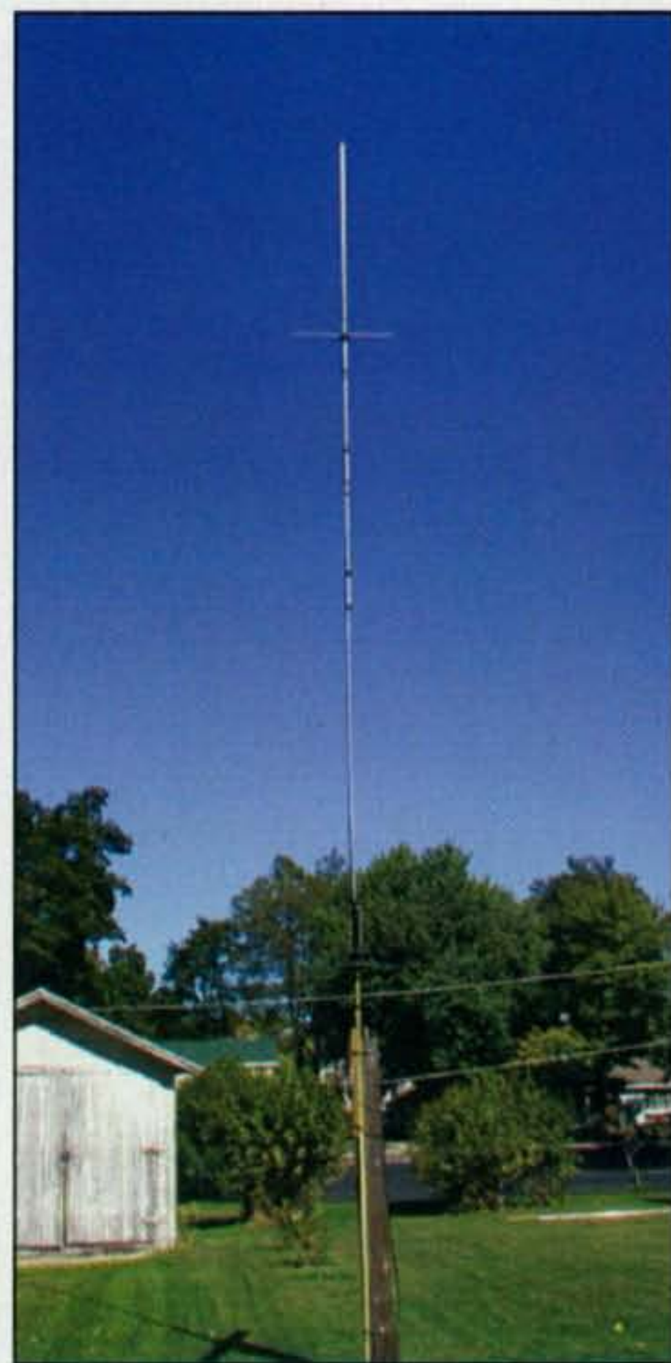
Photo A—The Hustler/Hamstick Combo antenna mounted on a test pole in the author's yard. The horizontal elements are difficult to see, but they're there.
