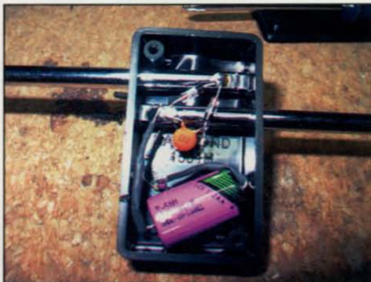
Photo B— The actual inside-wiring view of the simple RF detector.
