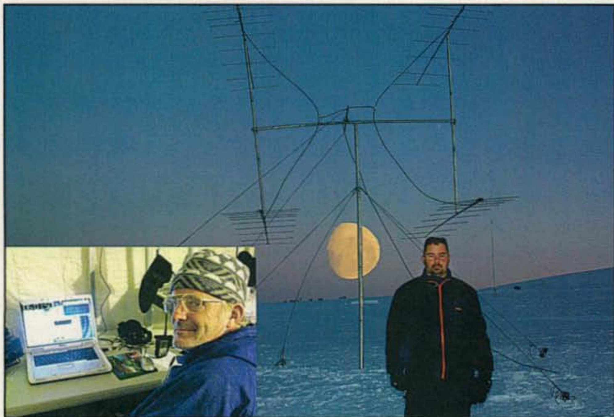
EME, or moonbounce, added a new dimension to the 3Y0X operation, with 113 contacts made off the moon. Here W0RUN is at the EME operating position (inset), while PA5M stands outside with the 2-meter EME antenna array, plus, of course, the moon.
