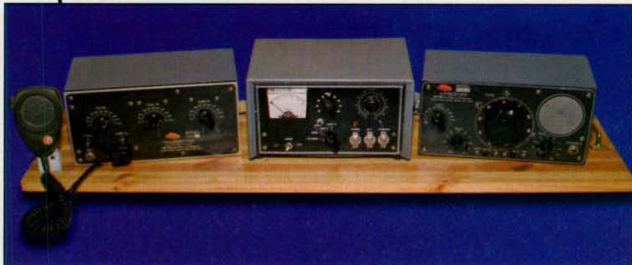
Photo 1— Although he was better known for his elaborate receivers of the 1920s and '30s, McMurdo Silver sold a line of basic ham equipment in the late 1940s. The Model 701 transmitter is on the left, the Model 802 receiver on the right, and the homebrew power supply, center (Photos © Joe Veras, 2006, all rights reserved)
