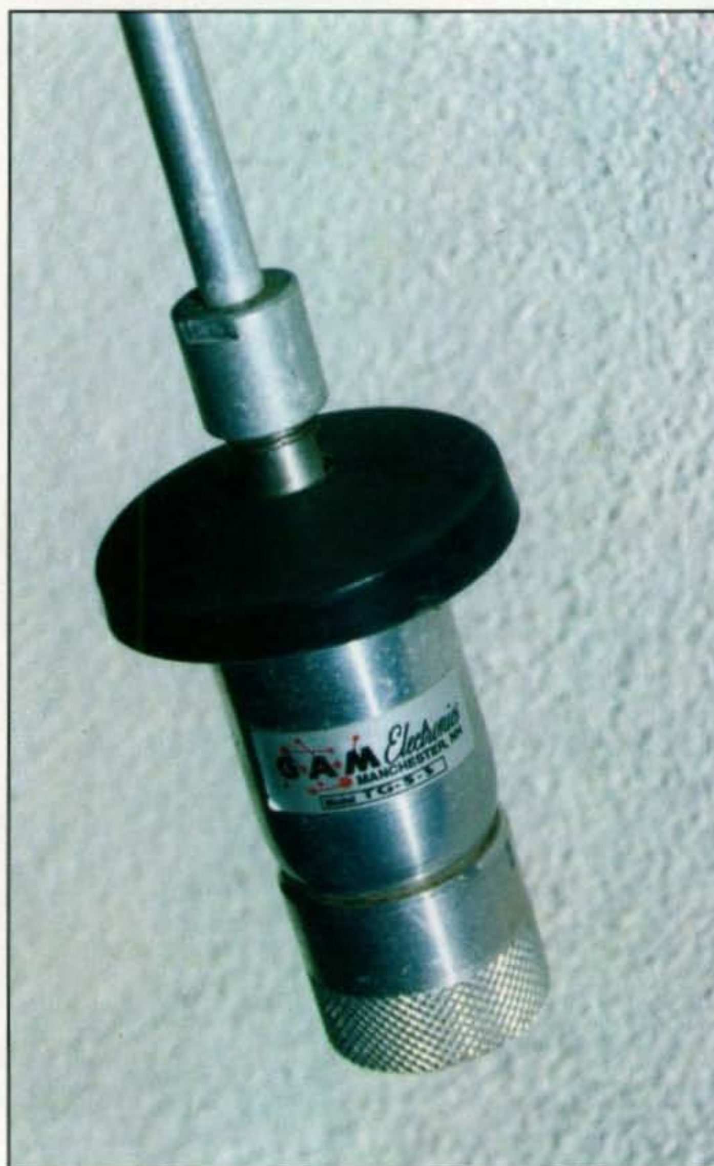
Photo A— GAM VHF antennas are easily recognized by their distinctive shunt-fed matching network at the base.
