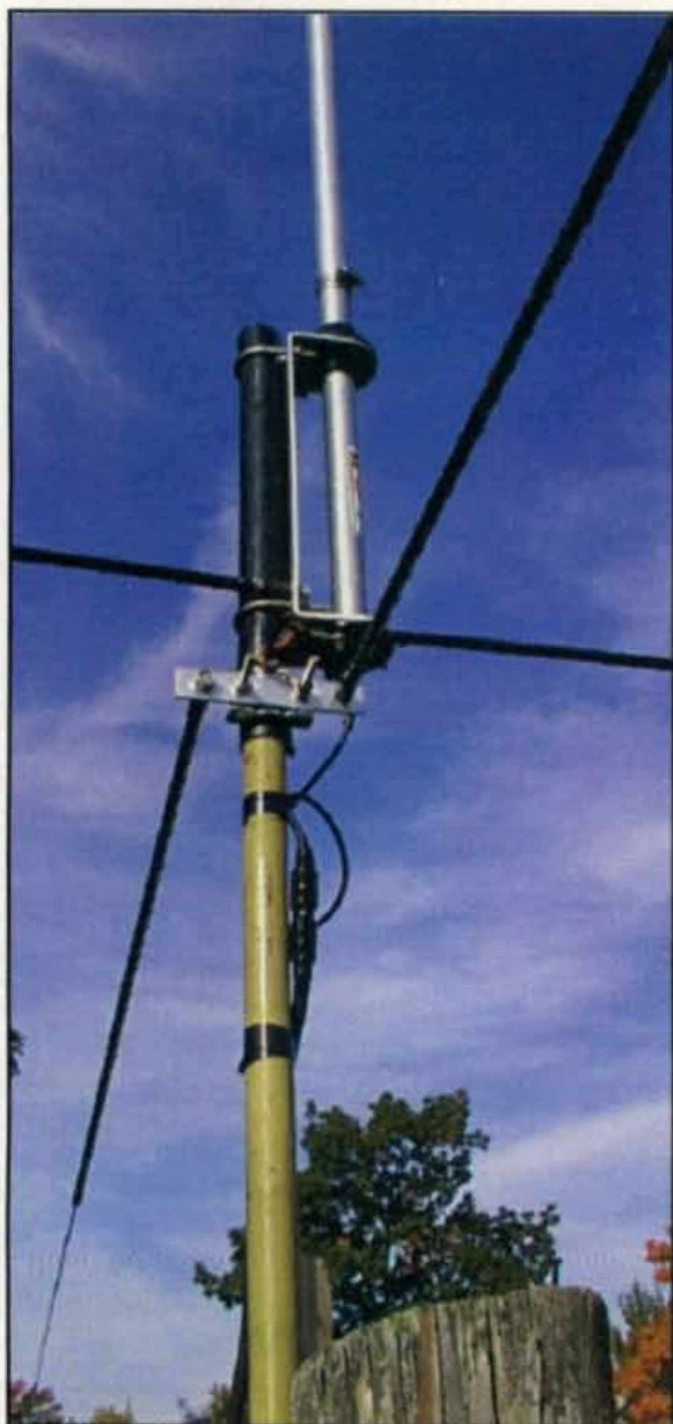
Photo B— A closer look at the base of the antenna clearly shows the Hamstick whips—each tuned for a different band—used as horizontal elements. Note the PVC tubing over the top of the mast to electrically isolate the antenna from the mast.
