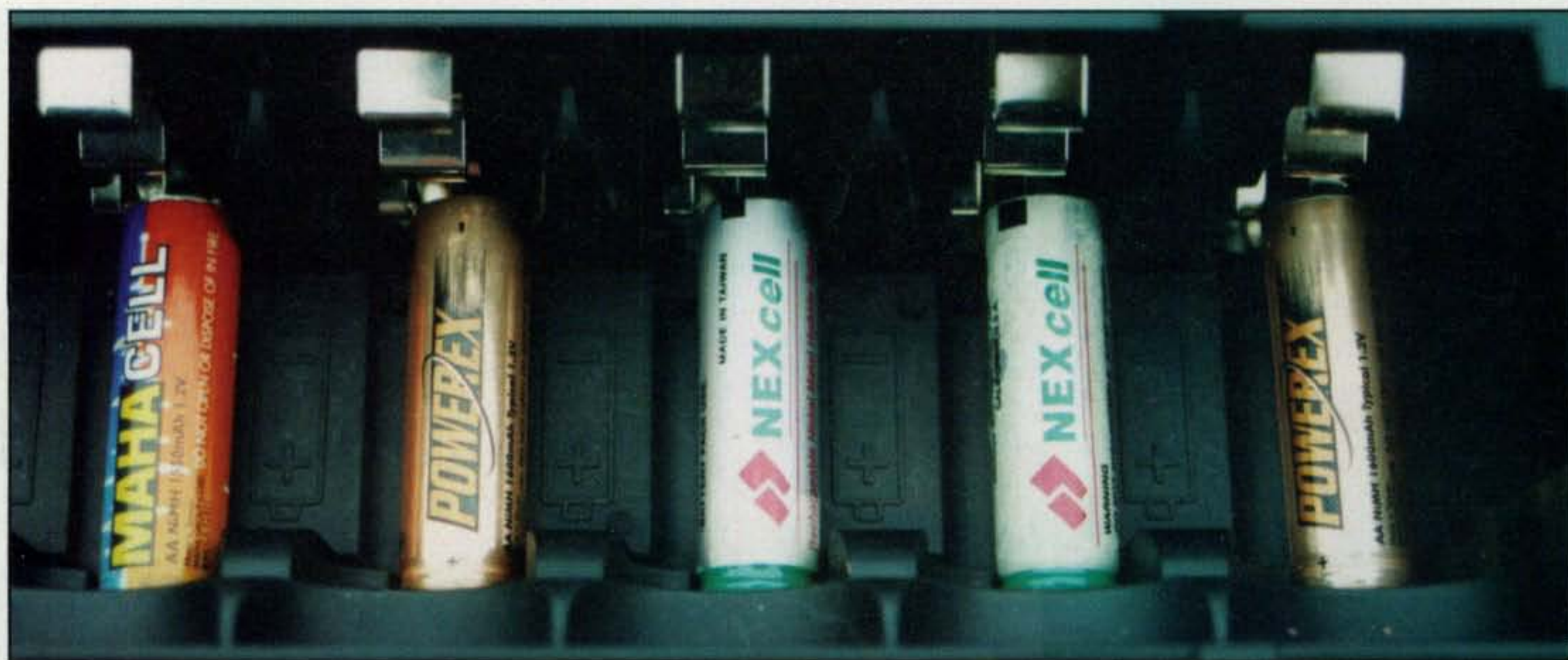
Photo A— The MAHA multi-cell-size charger will accept up to eight batteries to be charged at once. While only AA cells are seen here, the charger will also accept AAA, C, and D cells, and you may charge different sizes at the same time. See text for precautions.
