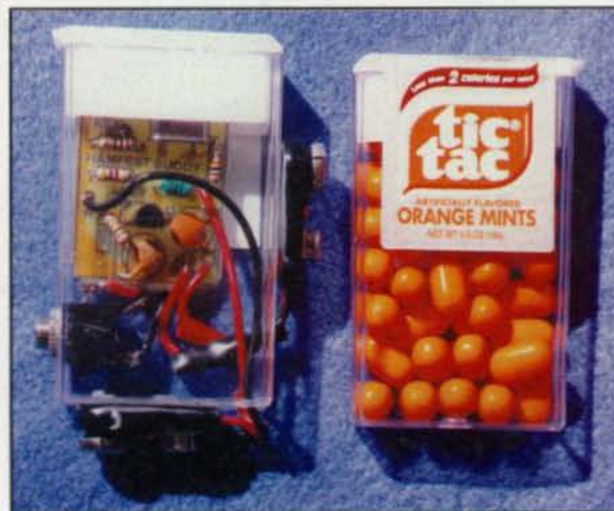
Photo B— Check out this snazzy Hamfest Buddy Larry Johnson, WB4LKI, installed in a tic tac® box. Key socket is on left, antenna connector is on the right, 9-volt battery clip is on the bottom, and VXO frequency switch is accessible through a flip door on top. Ponder how Larry installed the PC board in the box without bunched up wires, and then read the answer in the text. (Photo via WB4LKI)
