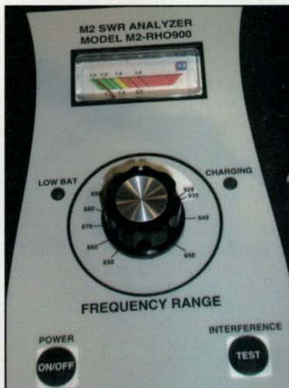
Photo N— The RH0900 SWR analyzer from M 2 is a specialized unit for 850–950 MHz, useful for the 900 MHz amateur band as well as cellphone antennas.
