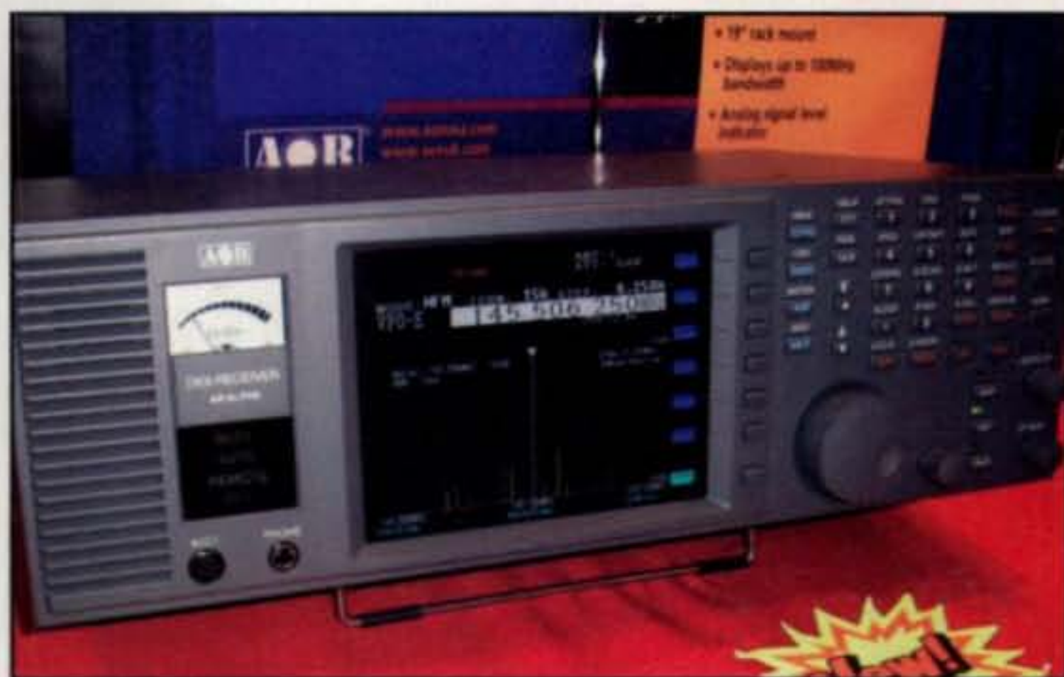
Photo D—The AOR AR-Alpha receiver covers 10 kHz to 3.3 GHz and will even function as a TV.
