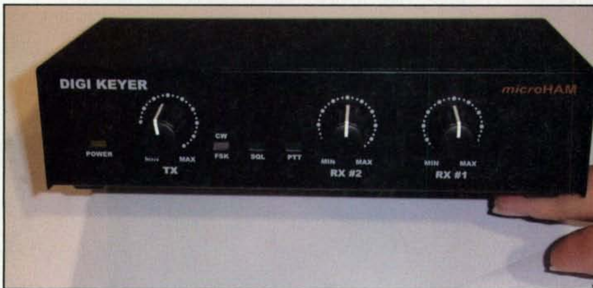
Photo R— The microHAM DigiKeyer contains its own sound chip, so you can operate digital modes without relying on your computer sound card.
