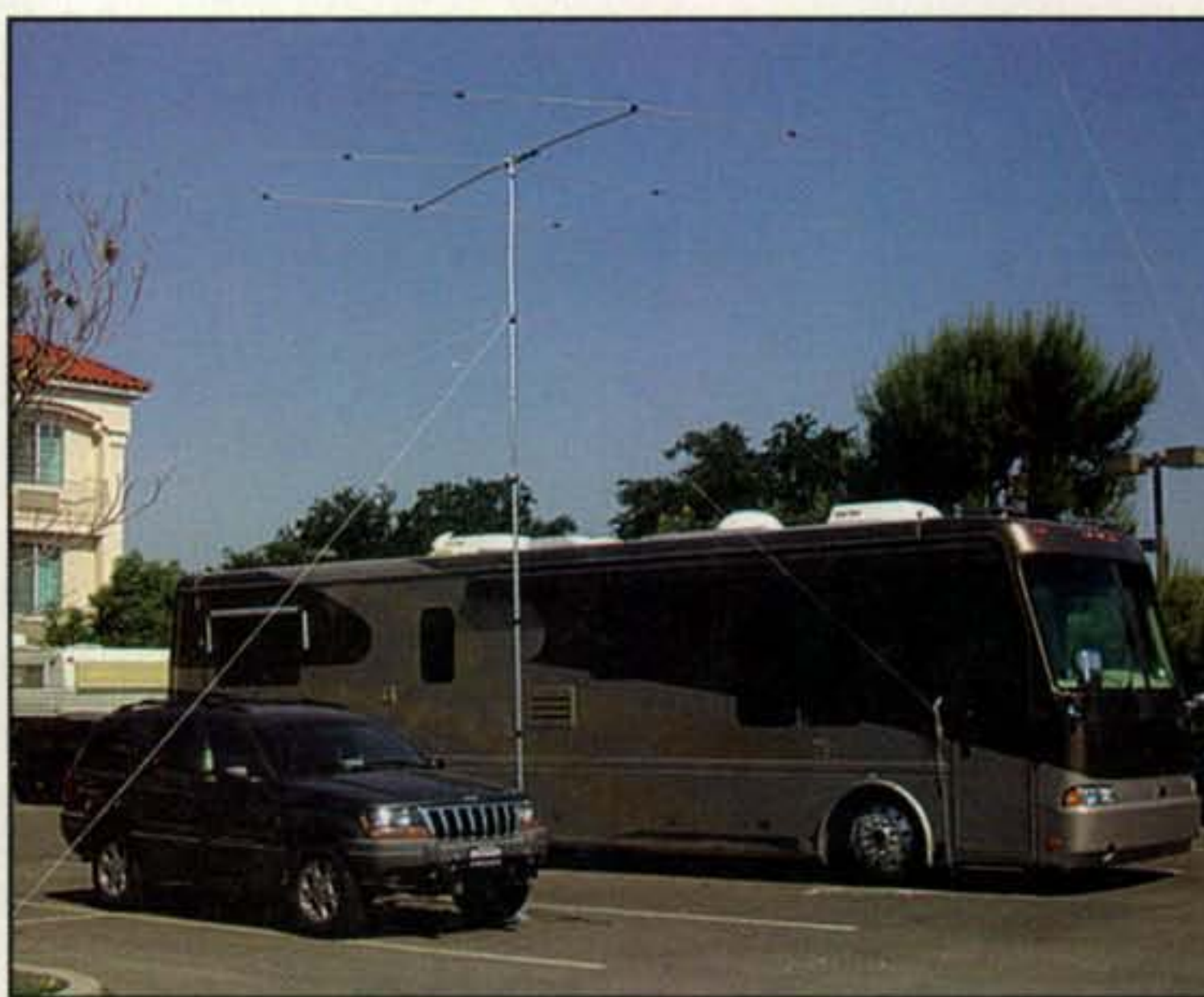
Photo D— This new three-element Super Antennas mini beam is a traveler's delight. It easily fits in an auto's trunk or on a rear seat; can be configured for operation on 20, 17, 15, 12, 10, or 6 meters; and assembly time is only 10 or 15 minutes. Being heard from the boonies is a cinch with this antenna! (Photo via W6MMA)
