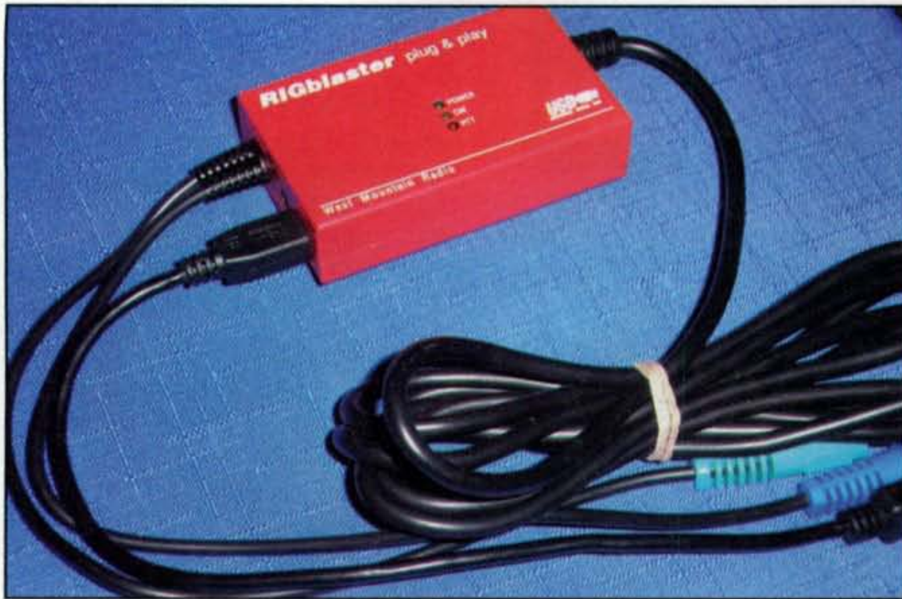
Photo Q— The RIGblaster Plug & Play from West Mountain Radio will let you run digital modes with a minimum of fuss, using your USB-equipped computer and just about any transceiver.
