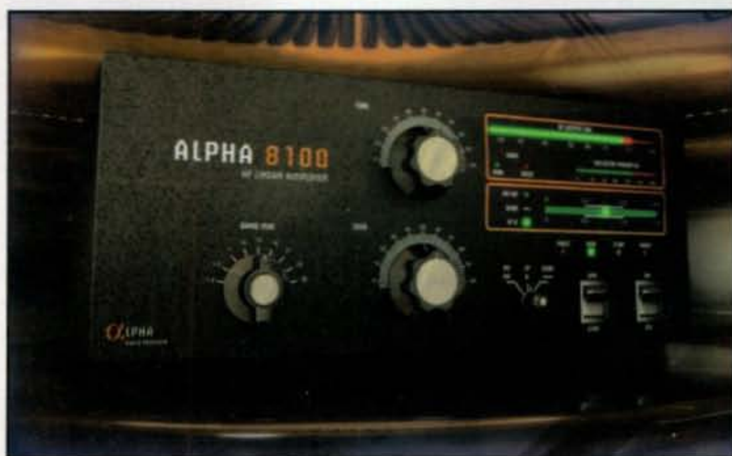
Photo G— Alpha's new 8100 amplifier continues to rely on tubes in the final, a pair of 4CX800 tetrodes.
