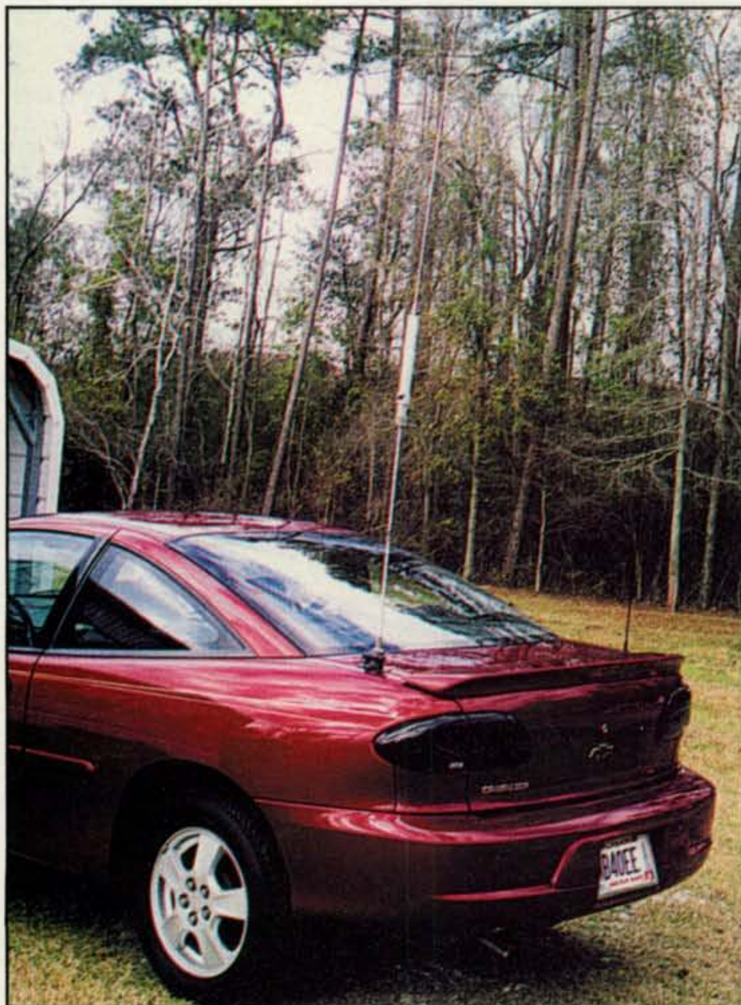
Photo C— Here is the new Super Antenna standing tall on the trunk of XYL WB4OEE's Chevy Cavalier. Look closely and you can see the two base masts are coupled together to raise the coil above the roofline, and the sliding aluminum sleeve is positioned above the coil so it acts as a capacity hat. Combined, both measures ensure radiation of an impressive mobile signal.
