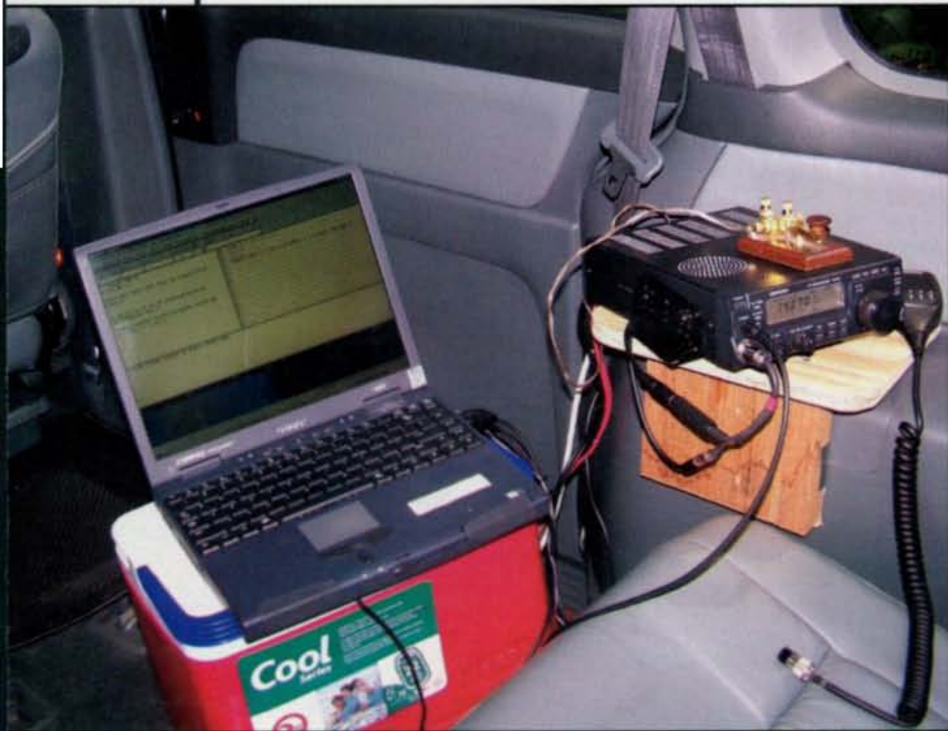
Photo A—Ed's setup ready for operating PSK-31 mobile with his Kenwood TS-50 transceiver, Compaq laptop computer, and Electronic Devices, Inc. interface. Numerous U.S. and DX contacts were made while traveling freeways and byways. (Photo via K4YFR)
