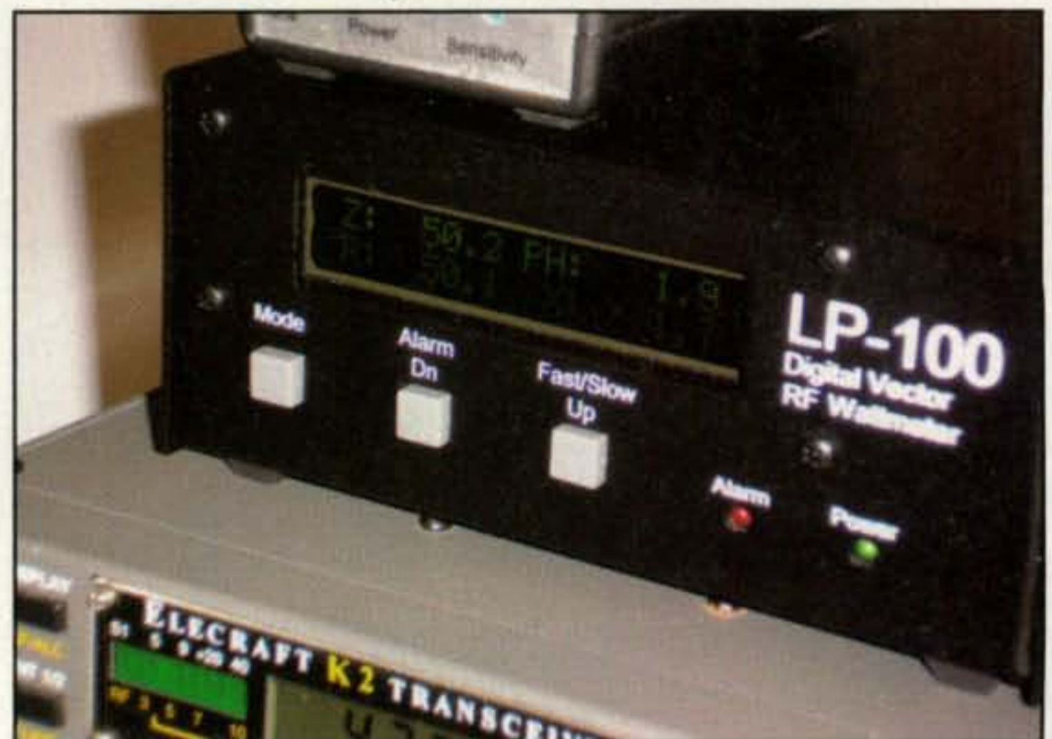
Photo L— Telepost's LP-100 digital vector wattmeter displays not only power and SWR but impedance (Z), resistance (R), reactance (X), and phase angle (P).
