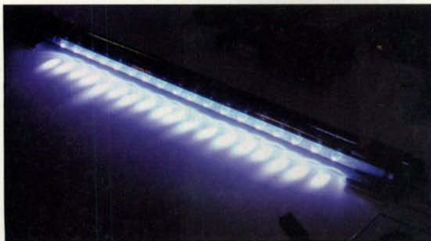
Photo U— West Mountain Radio's PWRbrite light uses bright white LEDs and can be rotate in its mounting clips for maximum flexibility.
