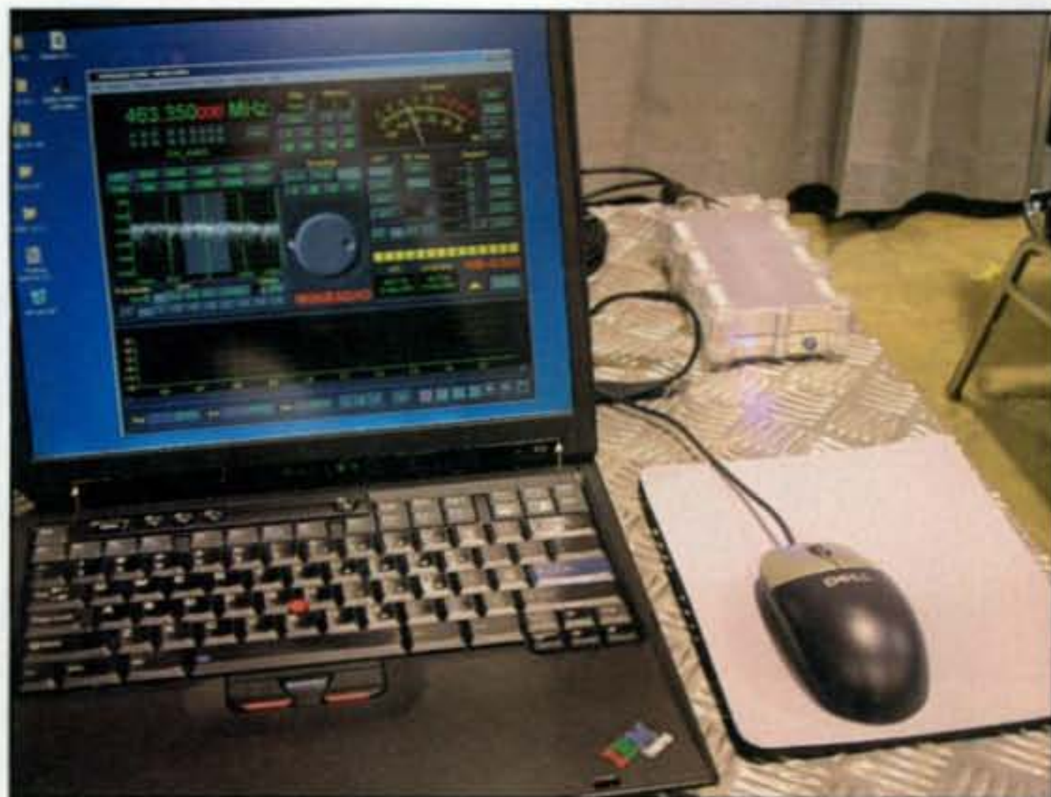
Photo E— WinRadio's new WR-G305 software-defined radio is available either as an external unit (seen here at right rear) or built onto a PCI card that installs inside a computer.
