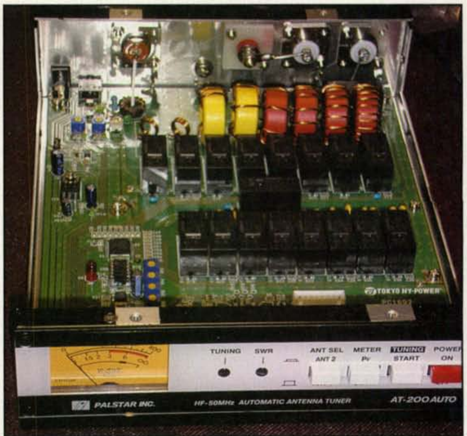
Photo K— The Palstar AT-200 AUTO is, as its name suggests, a 200-watt automatic antenna tuner. It has a built-in SWR meter and provision for two antennas.
