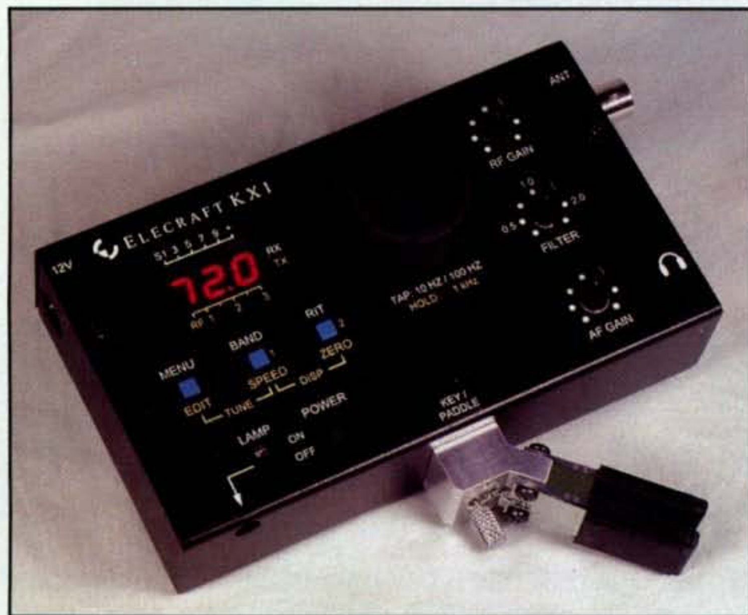
Photo C— The Elecraft KX1 Ultra-Portable CW Transceiver Kit is a backpacker's dream. Addition of the KXB3080 option kit allows four-band coverage; new firmware adds a scanning feature. (Photo courtesy of Elecraft)
