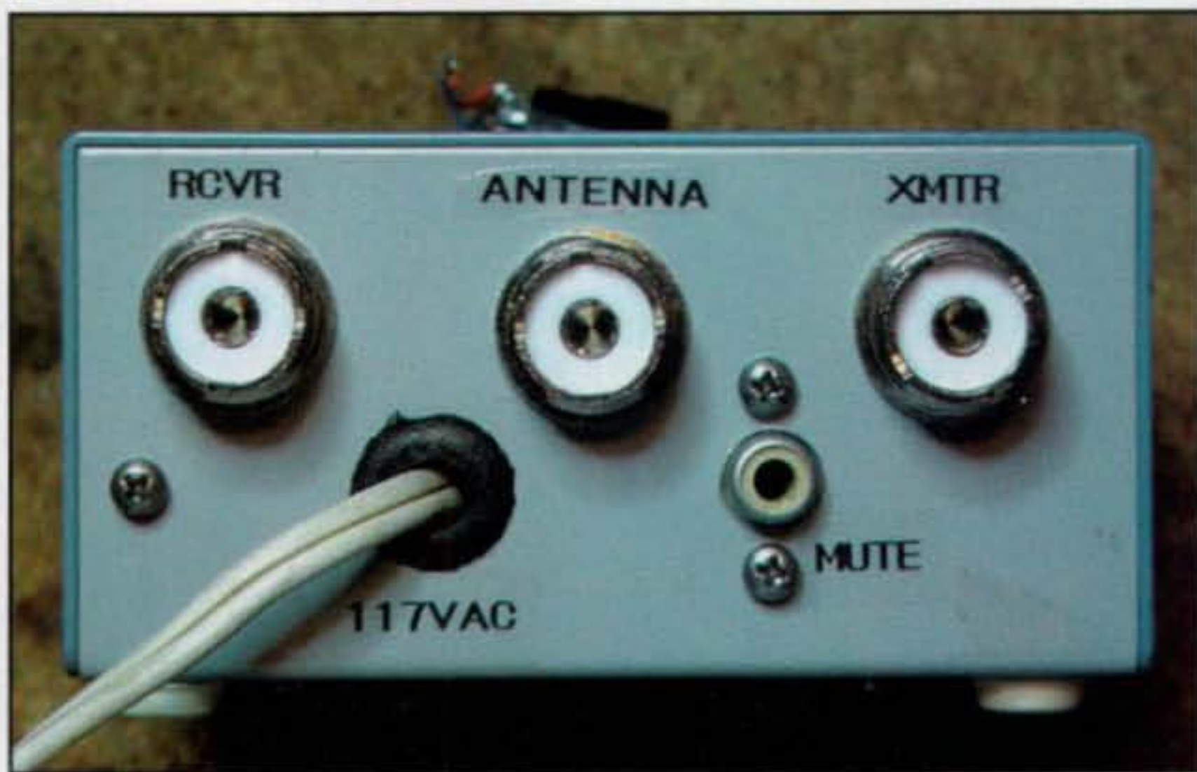
Photo A— This inexpensive T/R switch solves antenna-switching and receiver-muting problems for your vintage ham radio station.
