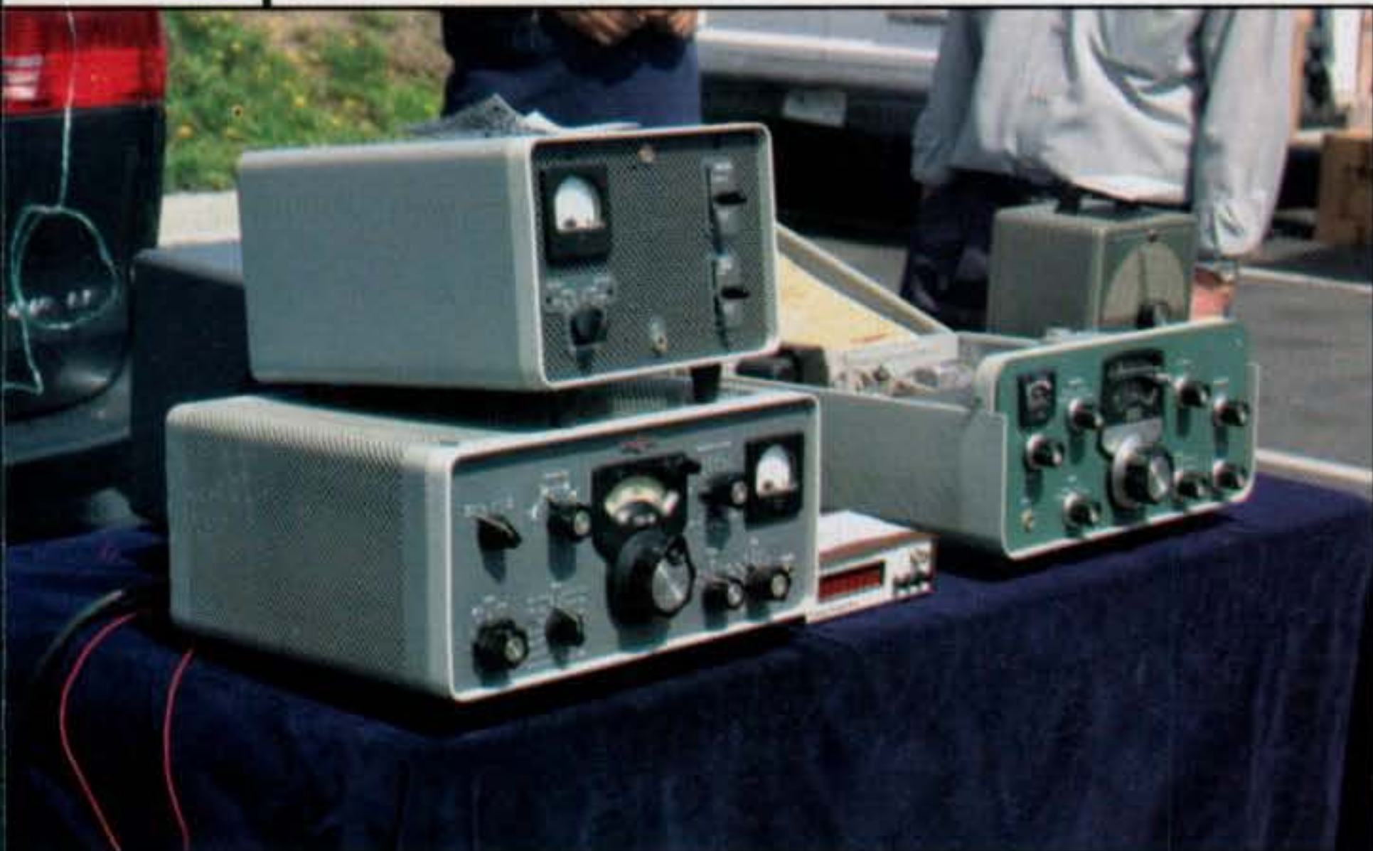
Photo 1— Here is some very nice-looking vintage ham gear for sale. On the left is a classic Collins receiver from the 1960s and a Heathkit transmitter from the same era. Both units use vacuum tubes. The small unit on top of the Collins receiver is a station console, a unit used to “interface” a microphone to the transmitter, and includes an SWR and RF power meter.
