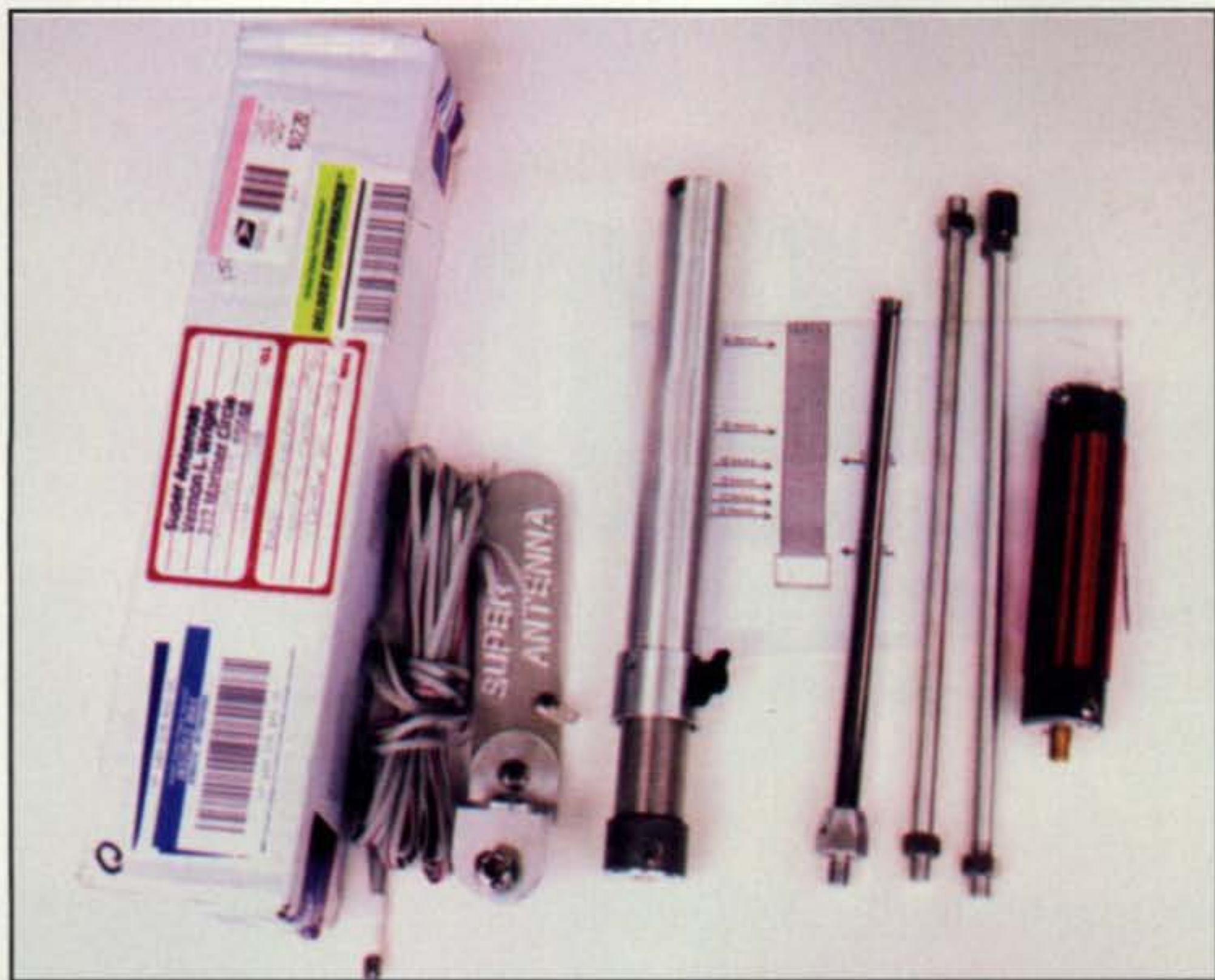
Photo B— Check out this new multiband mobile and portable antenna from Super Antennas, friends. It covers 40 through 10 meters (plus 80/75 and 60 meters with optional coil on right) and is supplied with universal clamp-on mount, adjustable coil, retractable whip, radial wire for non metal supports, and double-base masts with threaded coupler. The antenna has a clean, brushed-aluminum look, works great, and it all fits in the 14-inch-long mailing box.
