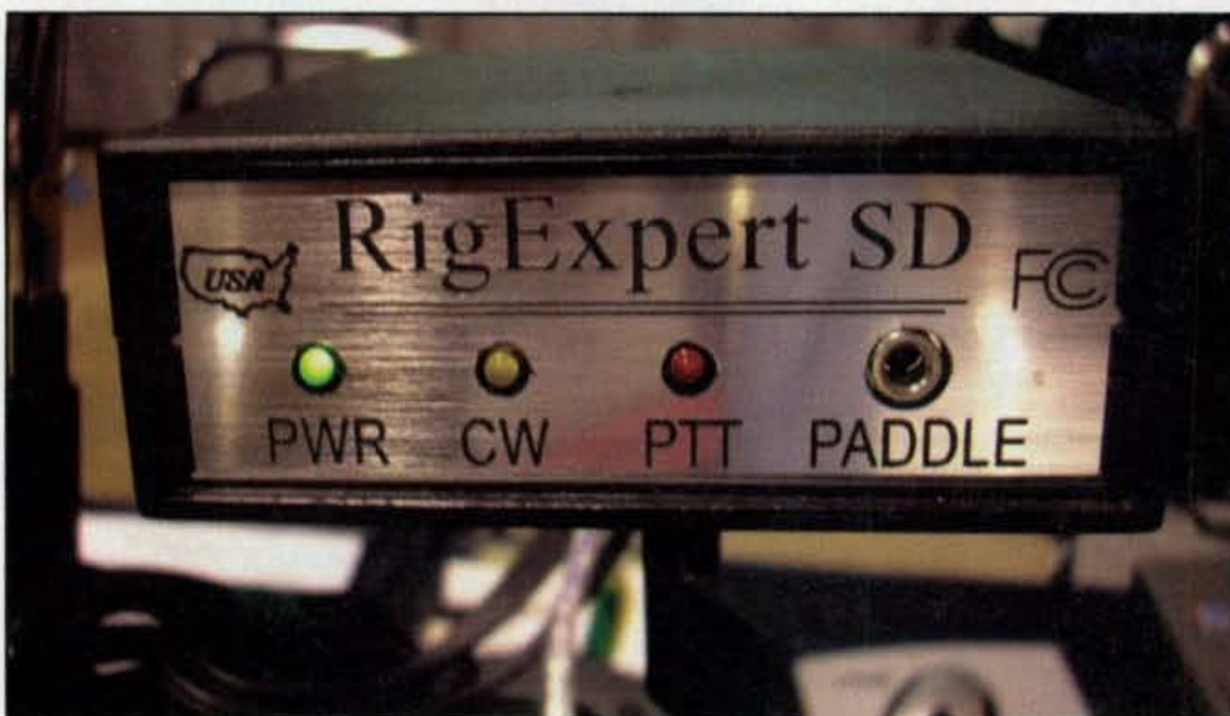
Photo S— The Rig Expert SD is another digital-mode interface with its own sound card built in, and runs everything on a single USB line to your computer and the line-in on your rig.
