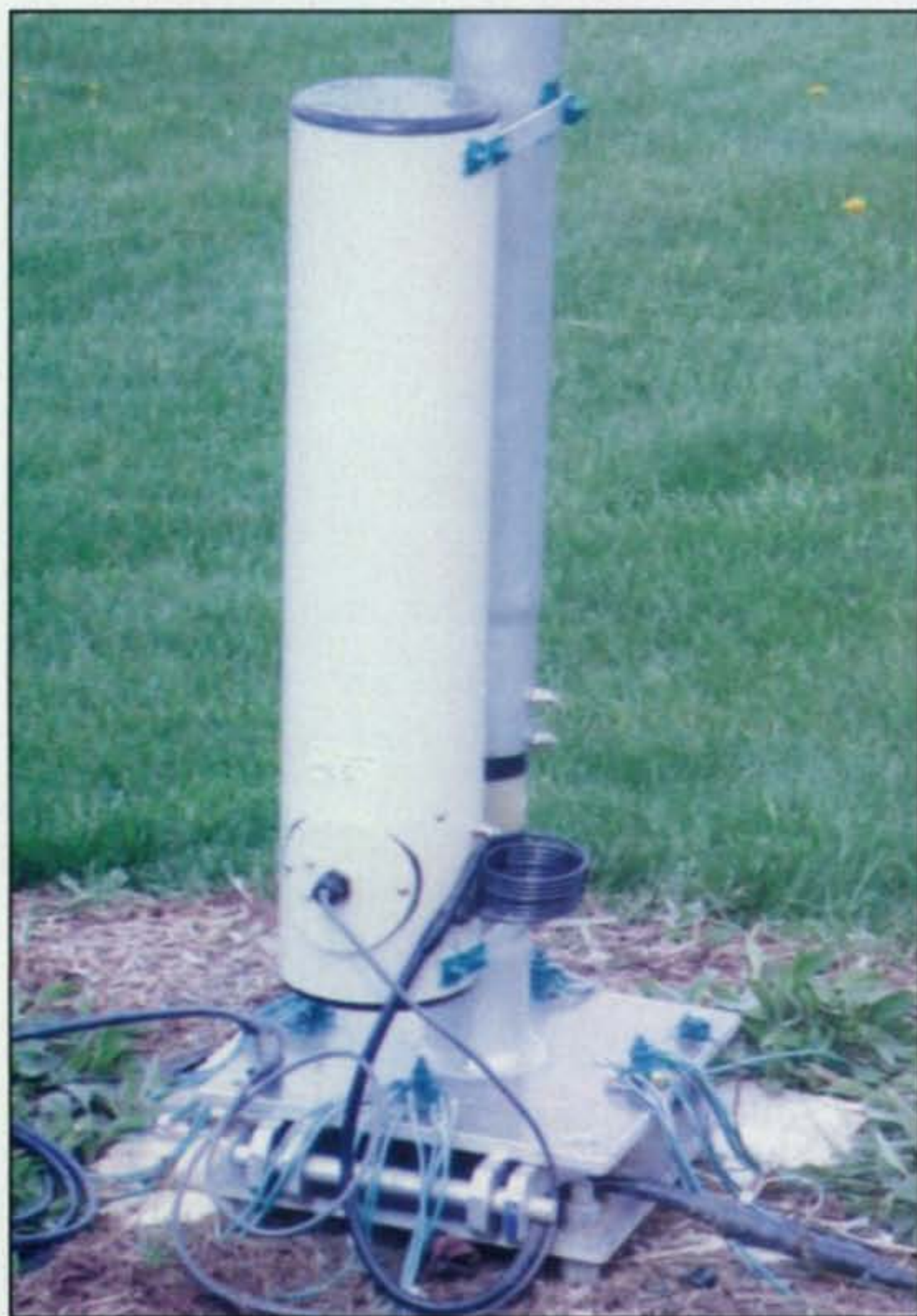
Photo 3— Here an optional 40-meter base coil has been added to the Force 12 antenna. Installation was halted at this particular point, so you can see the radial wires and transmission line connecting to the base plate.
