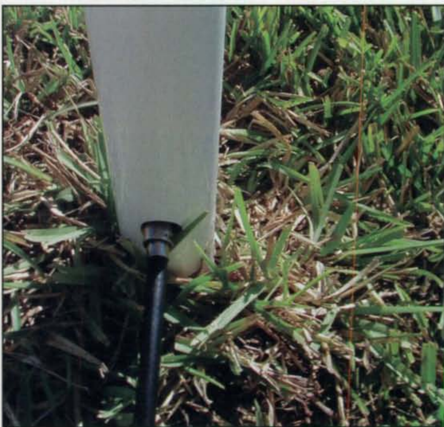
Photo 5— Base/feed-point view of IAC's SB-40 flagpole vertical showing the recessed socket accepting PL-259. The antenna fits onto a support mast you preinstall in the ground. Associated radials are buried just deep enough to avoid damage by wild weed eaters. (Photo courtesy of IAC Antenna Corporation)
