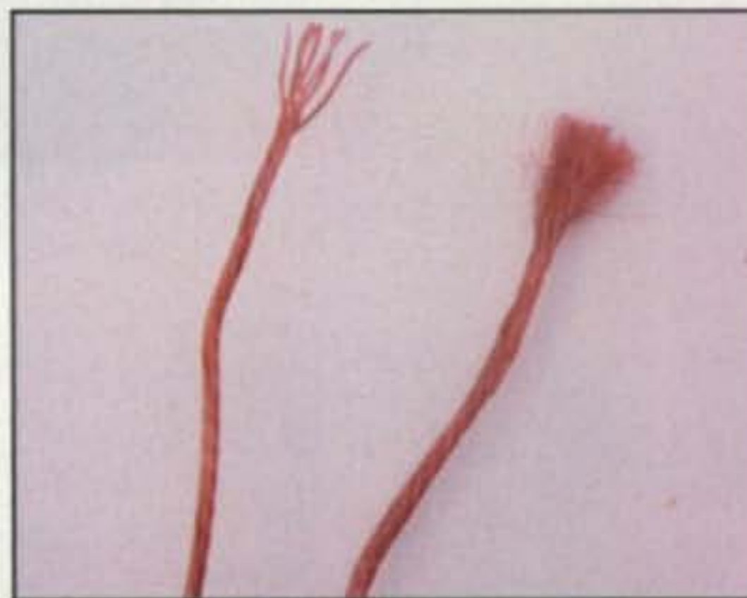
Photo 2— Notice the difference between 7-strand hard copper wire on the left and Flexweave 168-strand hard copper wire on the right. Numerous strands of finer wire make Flexweave as strong as copper wire, but as flexible as string. It is available from <www.radioworks.com>.
