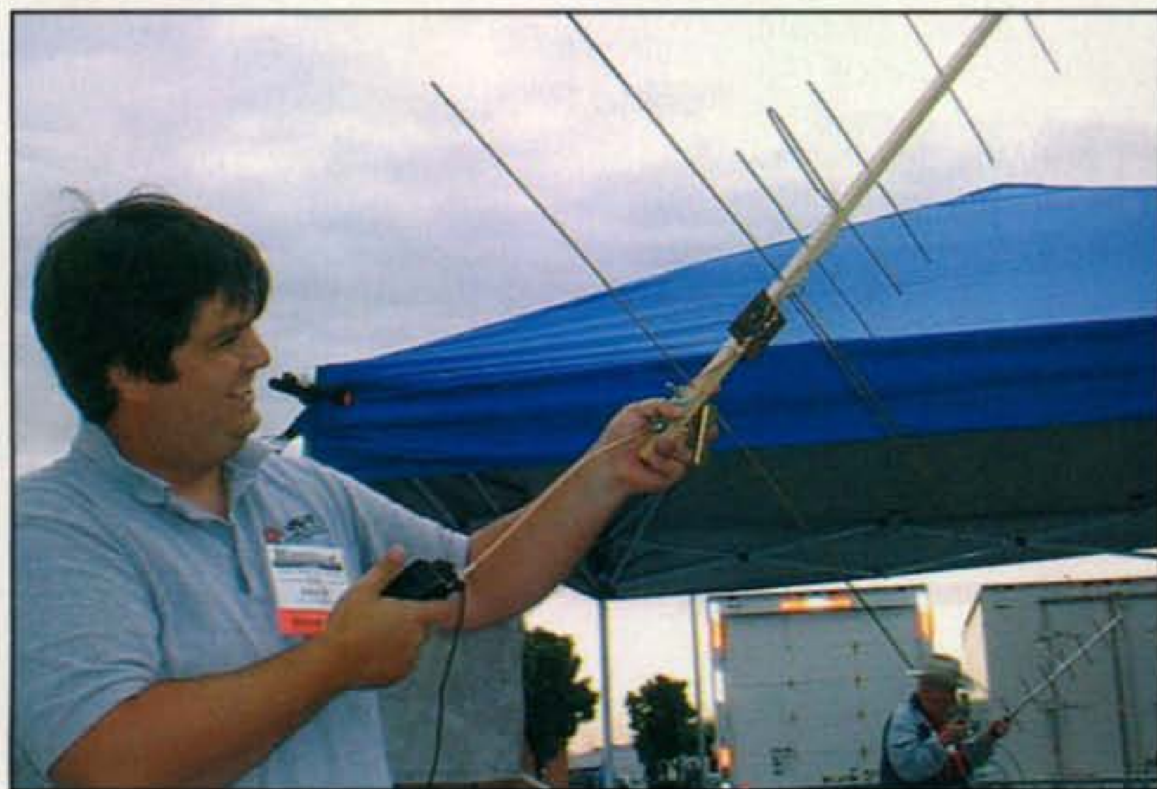
Photo B— Drew, KO4MA, using the Cheap LEO Yagi during a Dayton demonstration. In the background you can see CQ VHF Satellite Editor Keith Pugh, W5IU, using his Arrow commercial antenna. The Cheap LEO Yagi was at least as effective.
