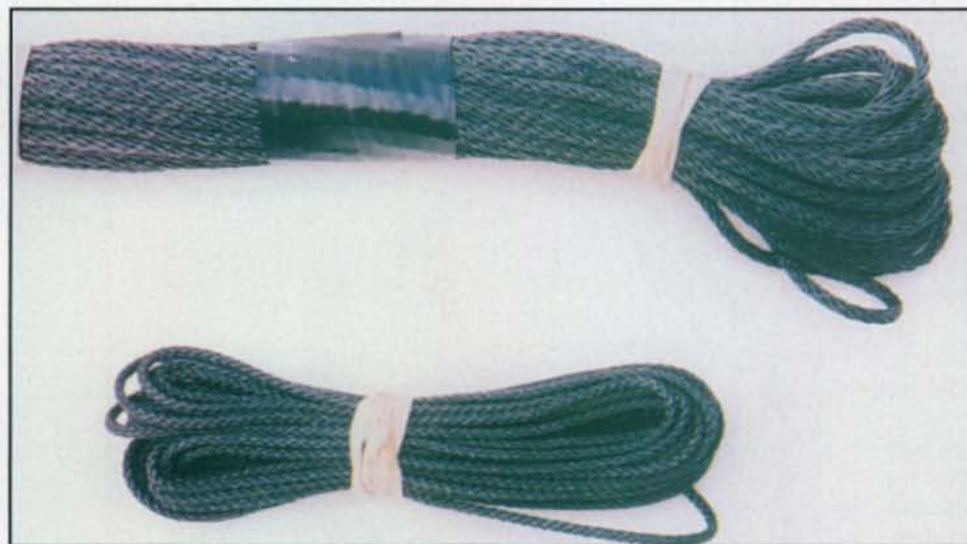
Photo 4— The rope used to support an antenna is just as important as the type of wire selected. Samples shown here are Dacron® (top), which exhibits good UV immunity and also tends to stretch rather than break when snapped by wind, and Kevlar® (bottom), which is stronger, tougher, and does not stretch. Both types are significantly better than any generic-type rope. Samples shown courtesy of The Radio Works.
