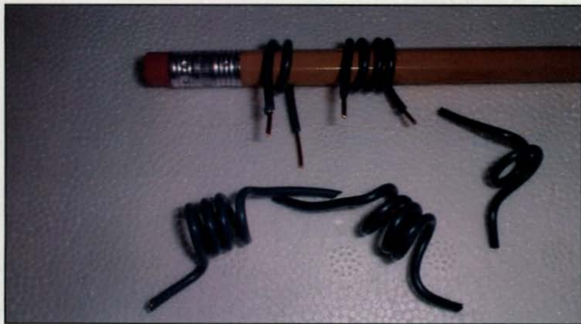
Photo F— Winding the band splitter coils.
