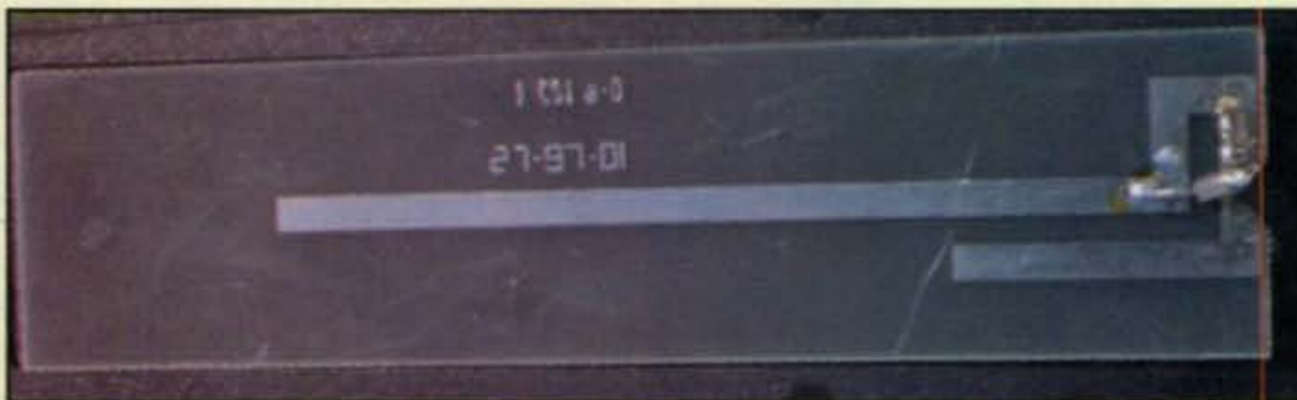
Photo H— Close-up of the PCB J-pole antenna, the first time I've ever seen a J-pole etched onto a PC board.
