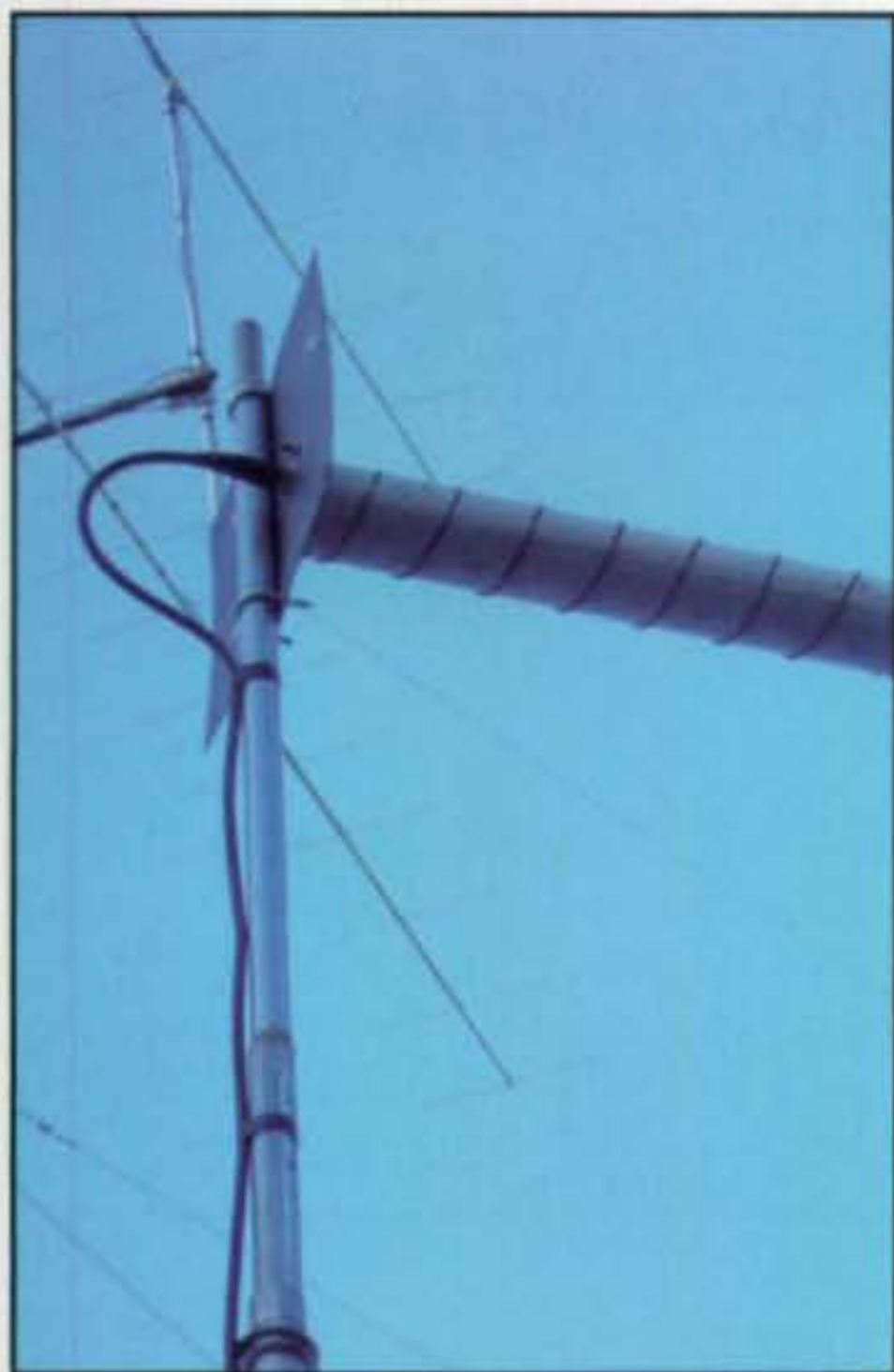
The collinear antenna used for cell-phone communications.
