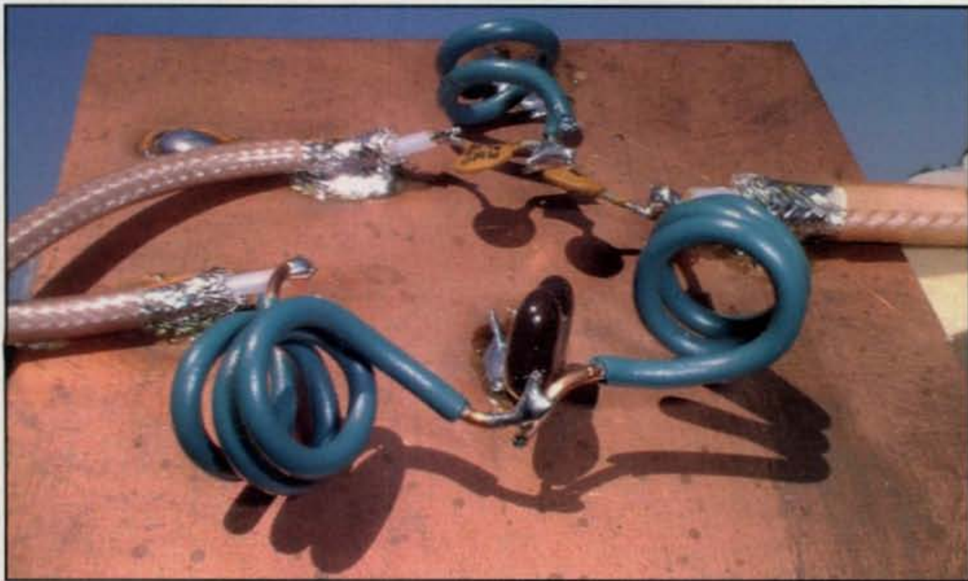
Photo E— 145/435 MHz band splitter.
