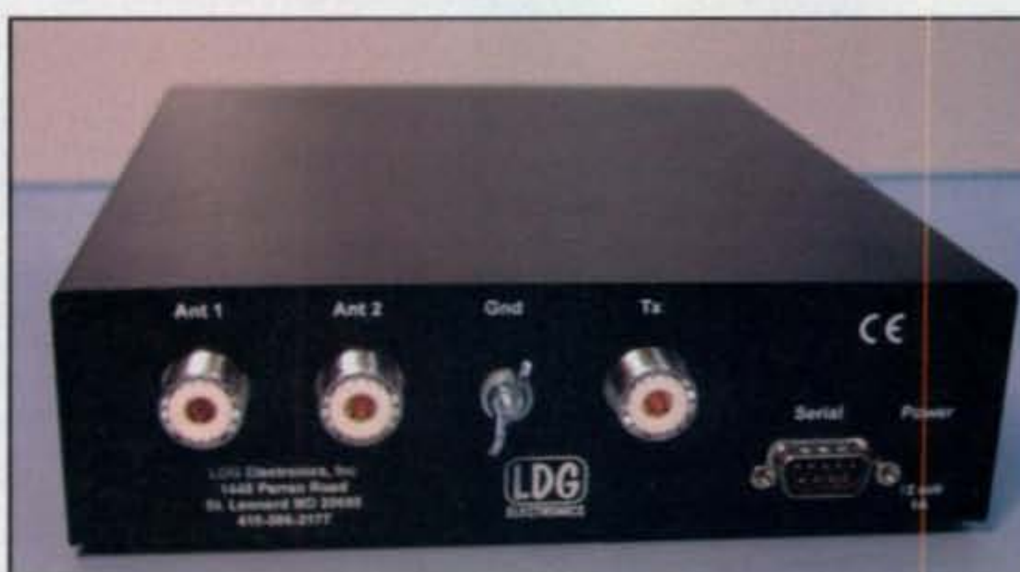
Photo D—You can install the AT-200PC Automatic Antenna Tuner out of the way, on the floor, or even in another room, interfacing to your PC via a serial or USB cable. The rear view is shown here. (Photo courtesy of LDG Electronics)
