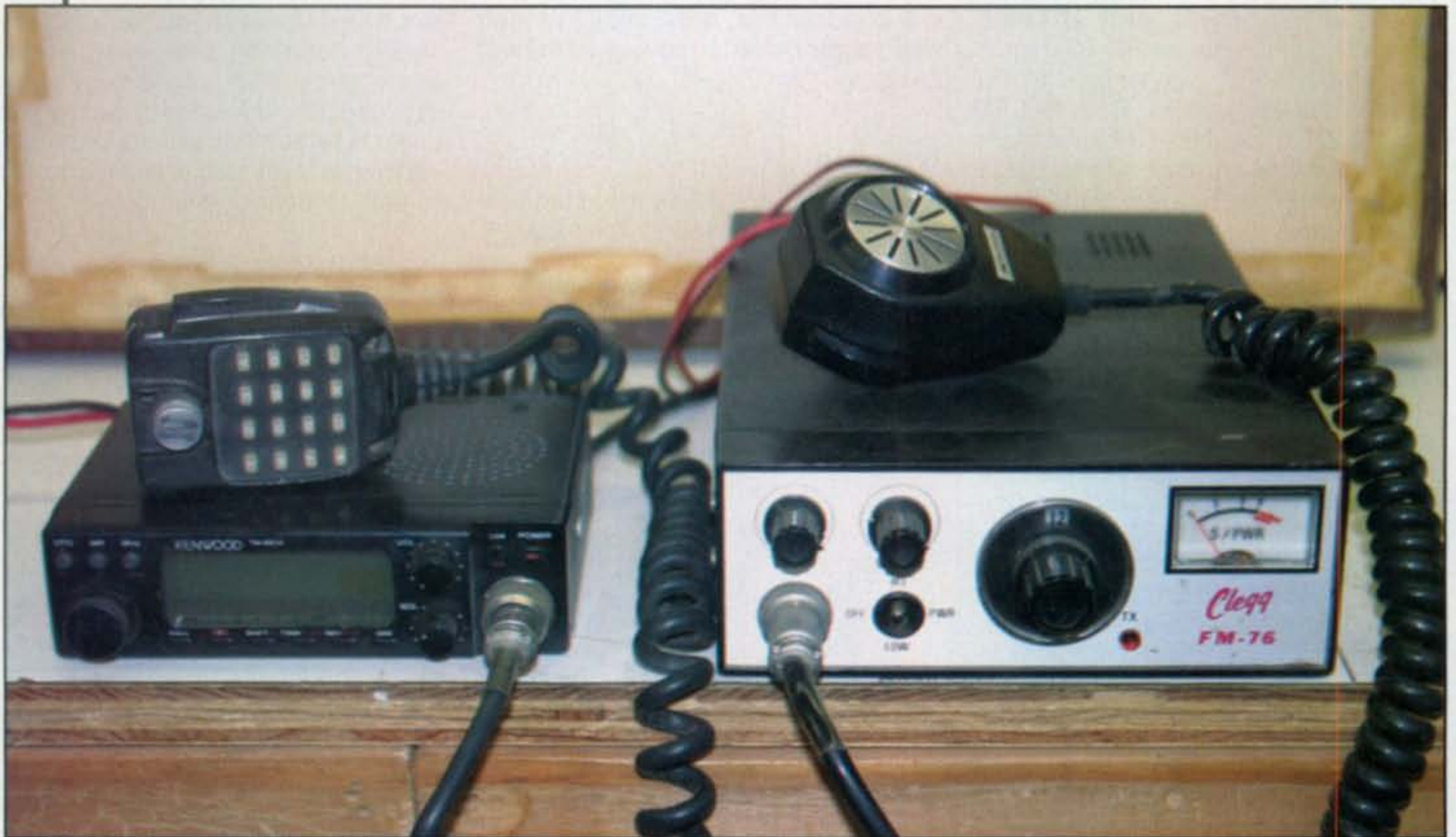
Photo A— The 220-MHz FM rig on the left has microprocessor-control, lots of memory channels, and multiple-function keys and knobs—sometimes good, sometimes bad. On the right, the 220-MHz FM rig from the 1970s is an example of a perhaps long-forgotten concept: A radio that "just works"—not much more than a power switch, a volume control, a squelch control, and a tuning knob. Would you really want one of those today?
