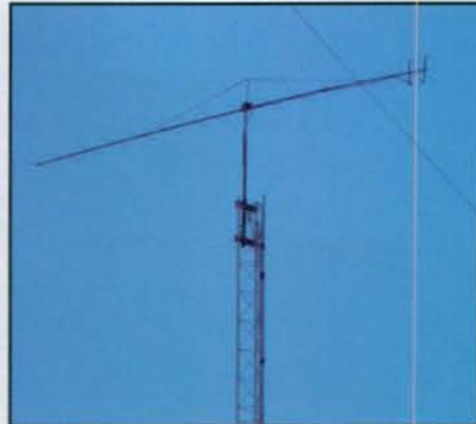
The 222-MHz quagi antenna on a 30-foot boom.
