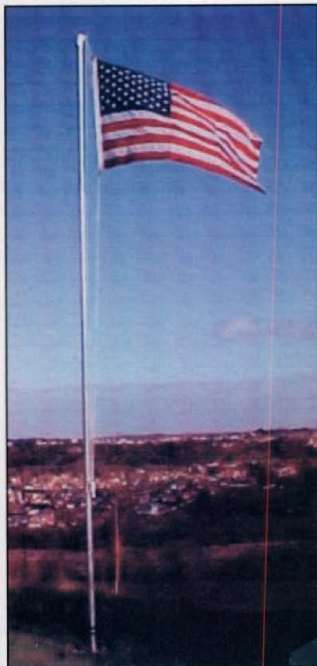
Photo 1— What's tall, delightful to see, and heard around the world? A Force 12 flagpole antenna, of course. It is an authentic metal flagpole that works 20 meters without a tuner and other bands with a tuner. Antenna is 16 feet tall and additional 4-foot sections to make custom flagpoles are available as options. Install the antenna so it has a good view of distant horizons in desired directions, and it will work out like a champ. More details at < www.force12inc.com >.
