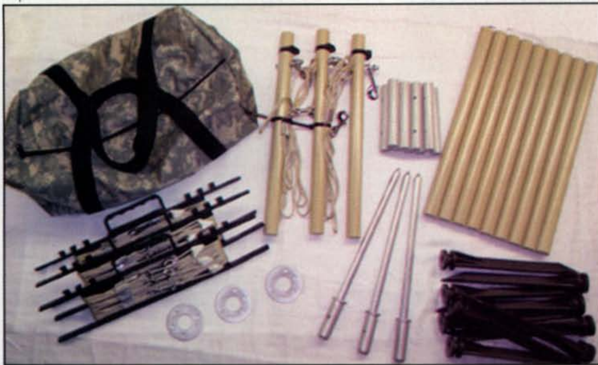
Photo F— The three-pole B & W Manpack Mast System will hold the antenna at a height of 6 ft. in a flattop configuration. Mast pole sections are a very short 18 inches and are rapidly field assembled with an inner joiner piece by pushing them together. (Photo courtesy B & W)
