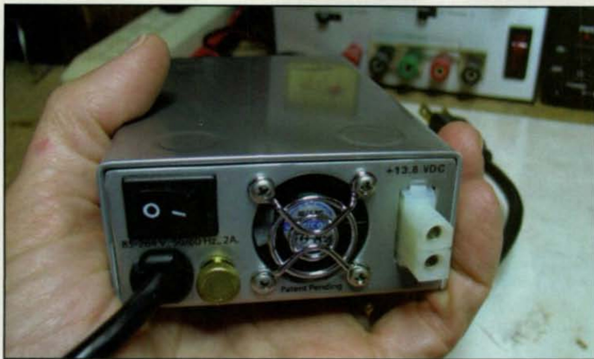
Photo B— Back side showing the 20-amp Molex DC output connector. Gamma provides a matching plug (also available from RadioShack).
