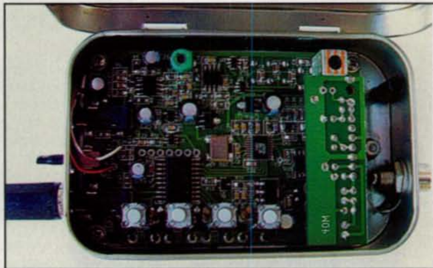
Photo I— Interior view of the digitally tuned and band-selectable transceiver shown in photo G. The four pushbuttons in the lower area are up/down tuning, RIT, and menu selections. Have you ever seen such a remarkable example of home brewing in surface mount? (Photo courtesy of N9JXY)
