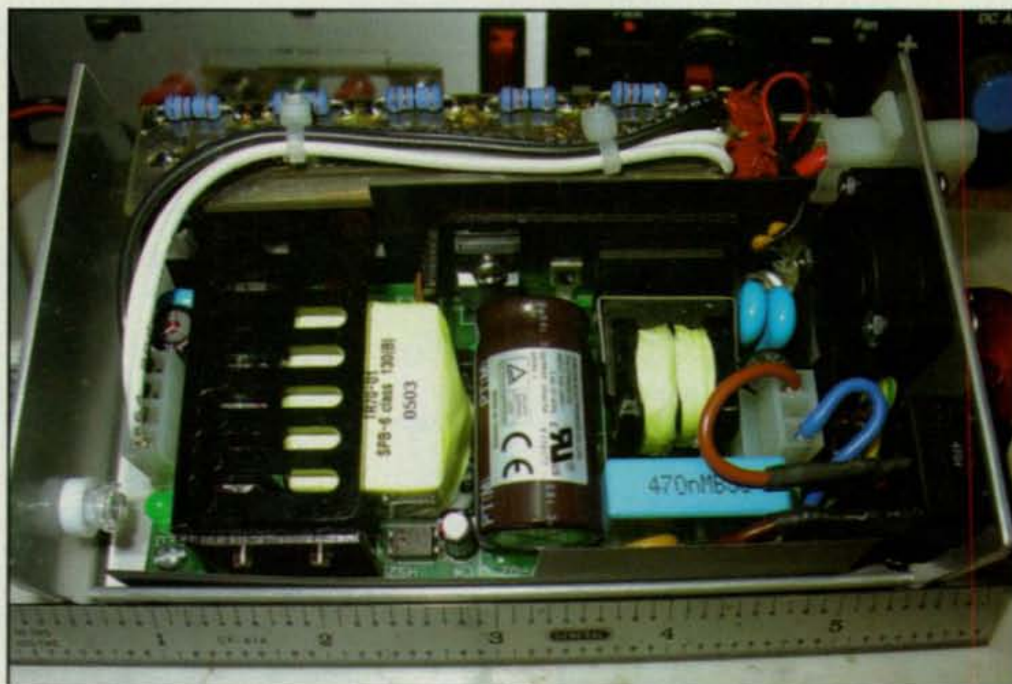
Photo C— Inside view showing the 5-amp switching power supply in the front and the capacitor bank assembly along the back.
