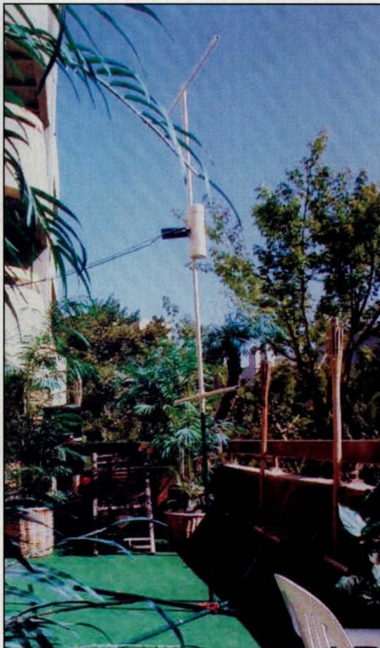
Photo 3— This clever installation of a Force 12 Sigma Five vertical dipole sitting on its optional garden trellis mount should inspire your creative ingenuity on disguised yard art-type antennas (Just tell the neighbors it is a night roost with foot warmer for migratory birds!) The antenna stands 9 feet tall (less mount) and works 20, 17, 15, 12, and 10 meters with a typical SWR below 1.5:1. Nice! (Photo courtesy of Force 12)
