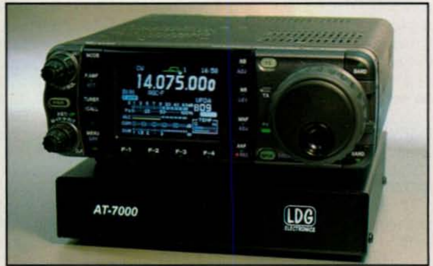
Photo C— The LDG Electronics AT-7000 Automatic Tuner is said to be a perfect "match" for the IC-7000 transceiver. It fits under the radio and comes with everything you need for plug-and-play operation. (Photo courtesy of LDG)
