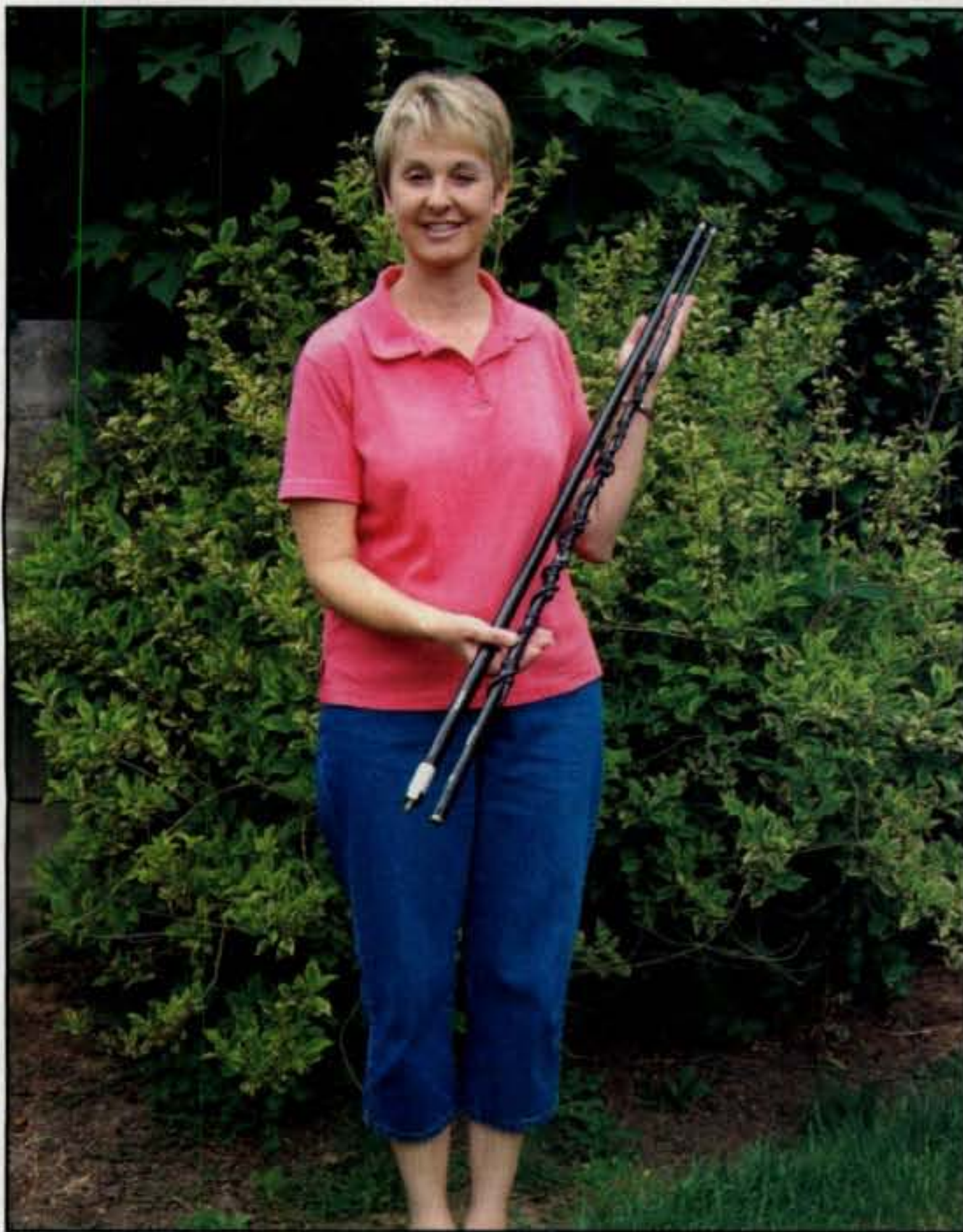
Photo 2—Shan Burns, XYL of Outbacker North America manager Jim, WB4ILP, shows us the versatile Outbacker Outreach made by Terlin Aerials and imported to the U.S. by Outbacker North America. It is 12 feet tall (less optional "outpost" mount), unscrews to 4-foot sections for quick storage, and works 160–10 meters. It could even double as a super mobile antenna for stationary operation. (Photo courtesy of Outbacker North America)
