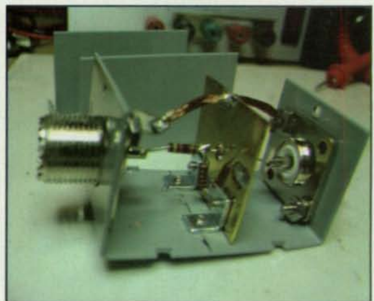
Photo B— 30-dB attenuator construction.
