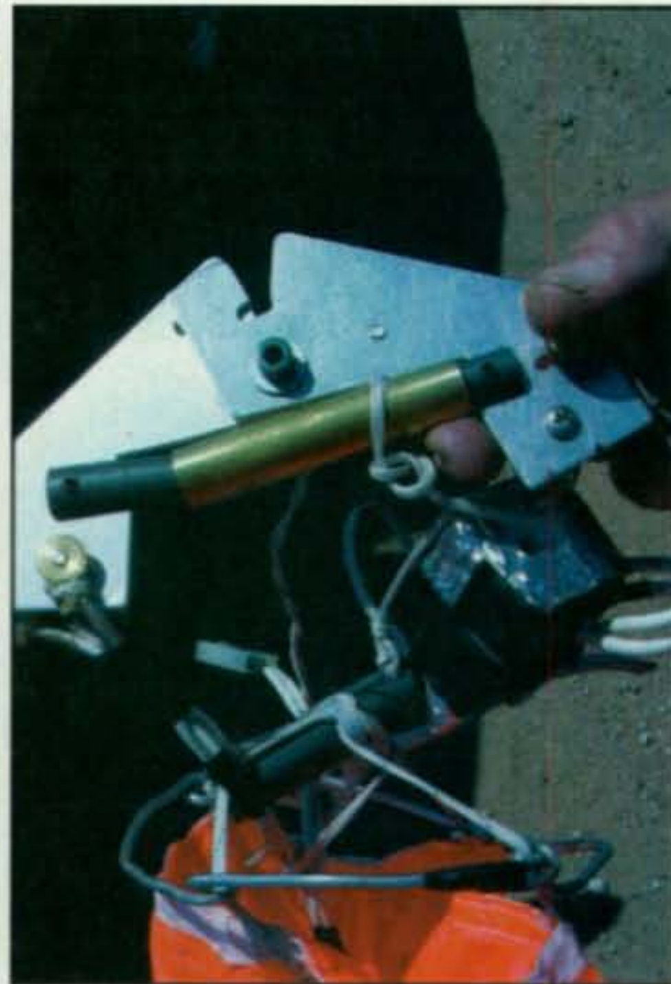
Mike Manes, W5VSI, demonstrated how his recovered homebrew cutdown device worked in releasing the exploded balloon from the payload. This device was the subject of Mike's presentation on Friday. (N6CL photo)
