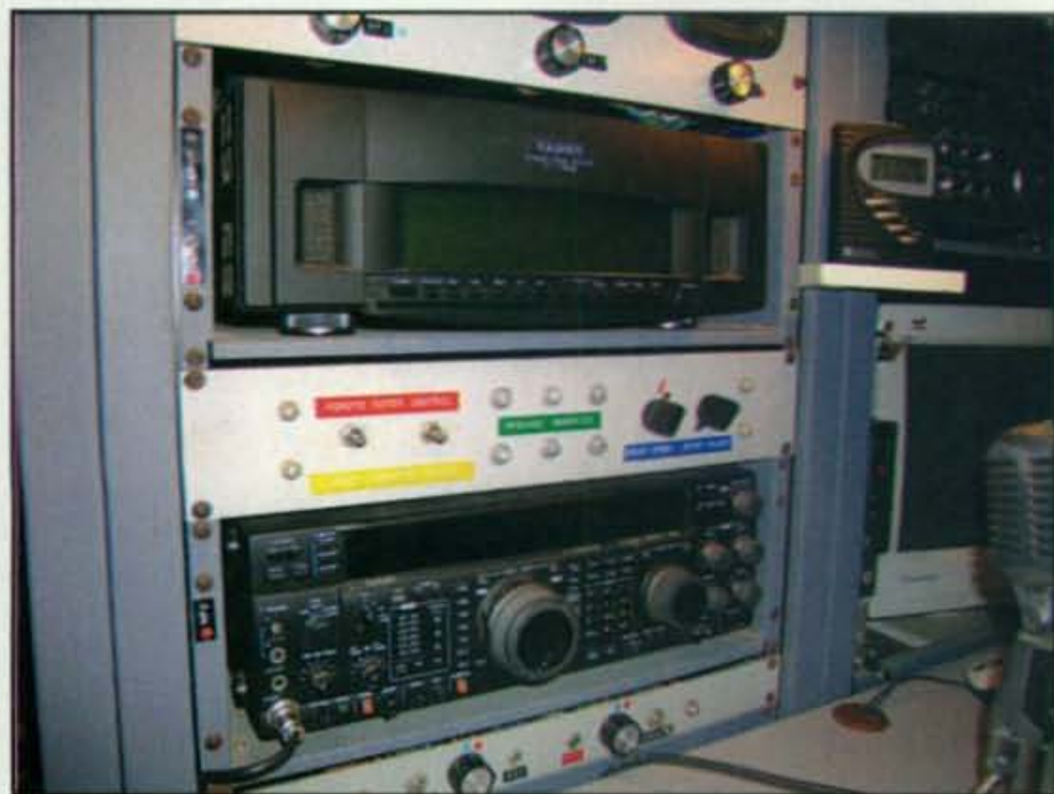
Photo B— Special shelves may be installed to hold equipment that was not designed for rack mounting, such as the author's Yaesu gear and the two computer monitors seen in photo A.
