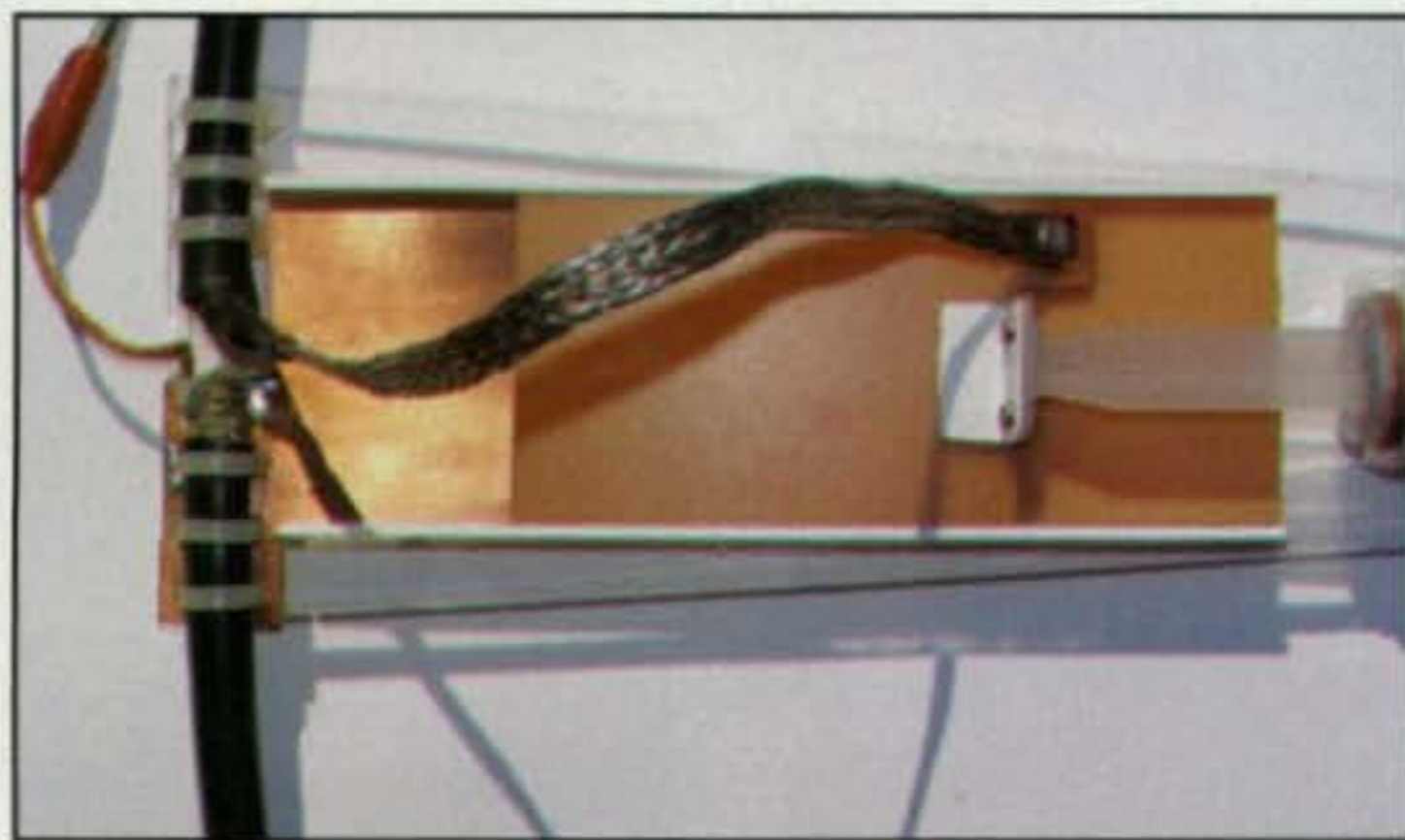
Photo D— The homebrew 5–50 pFd tuning capacitor at the top of the loop antenna is made by sandwiching two pieces of copper-clad PC-board material in plastic "U"-channel guides available from hobby stores
