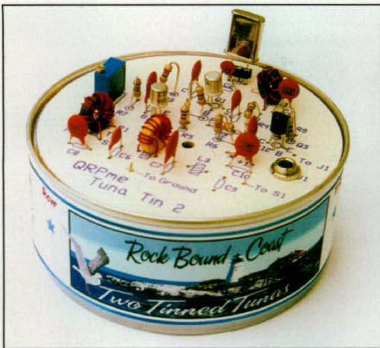
Photo 4—The completed Tuna Tin 2 is a novel conversation piece. My first contact with it was a station in New Jersey, which is not shabby for 350 mw. Where else could one find such fun for less than 20 bucks?
