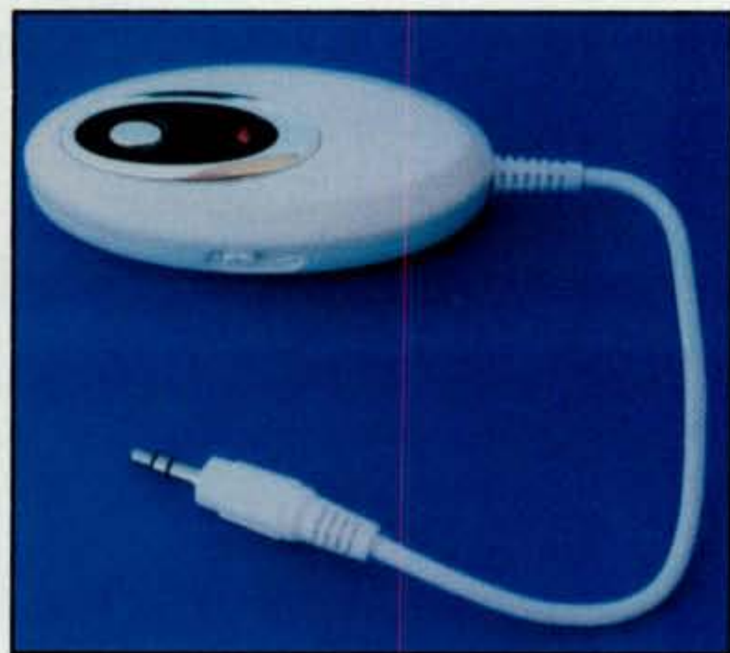
Photo 8— This little gizmo is a miniature 88-MHz FM-band transmitter with an approximate 200-foot range. Its general purpose is interfacing a portable CD player with a car's FM radio, and it also works terrific for routing your ham rig's audio through the car radio. Just plug it into the rig's earphone socket and tune it in on the radio. It is available from www.HamRadioFun.com .
