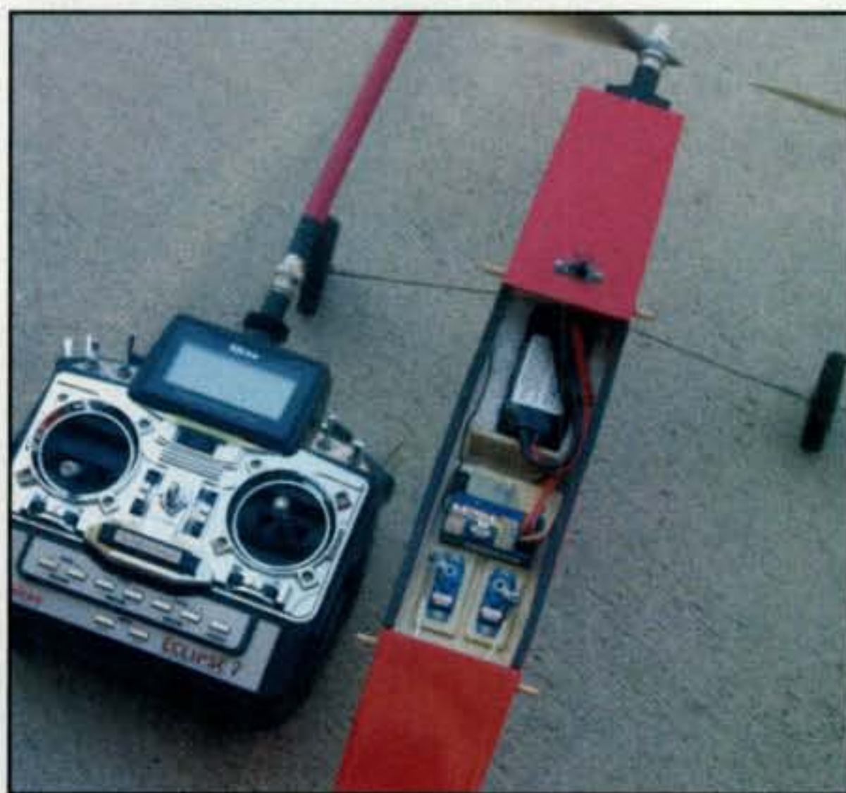
Photo 2—An RC "station" consists of a transmitter (left) and a receiver (right). The receiver, battery pack, and associated servo units are inside the model built and flown by Larry Frakes, KG6EG. The battery is just below the power switch, and the receiver is the small object in the middle. Two servos are visible below the receiver. Radio pulses (modulation) are used to command the servos to control the various functions on the model craft.
