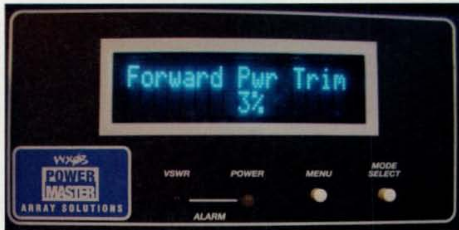
Photo F—Forward and reverse trim values recorded on the coupler are set in this and the next menu screen.
