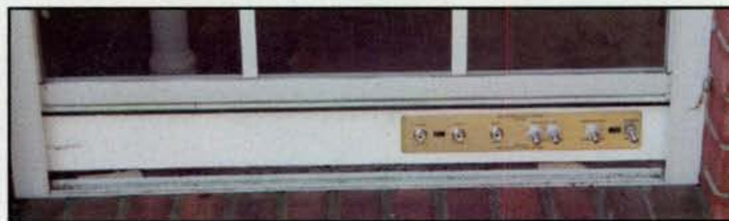
Photo E— The weather-proof MFJ-4602 Antenna Feedthrough Panel from MFJ Enterprises brings three coax-fed HF/VHF/UHF antennas, balanced lines, random-wire antennas, and ground wires into your shack without the need for drilling through walls. (Photo courtesy of MFJ Enterprises)
