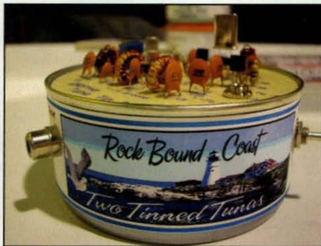
The Two Tinned Tunas kit by Rex Harper, W1REX. In addition to the cool label, Rex managed to get an antique canning machine that lets him pack virtually all of the parts for the kit, including the mini-CD instruction manual, inside the flip-top tuna can!
