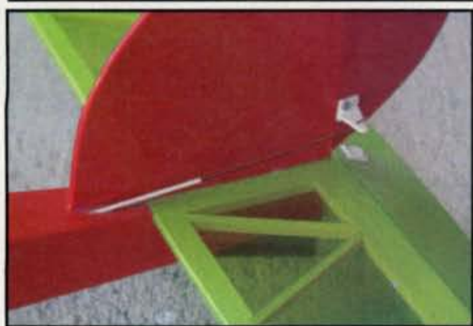
Photo 3— The receiver commands various control surfaces with servos and linkages, like the airplane rudder.
