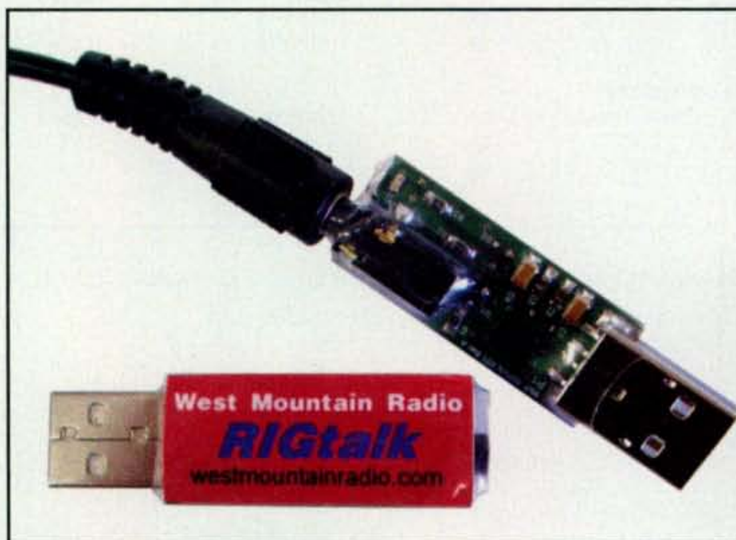
Photo C— The RIGtalk USB Rig Control Interface from West Mountain Radio plugs into your computer's USB port, and it allows software control of programming of compatible transceivers. (Photo from the West Mountain Radio website)
