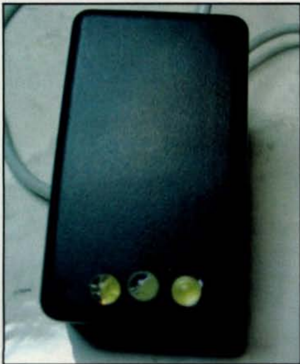
Photo B— The three LEDs extend through the box.
