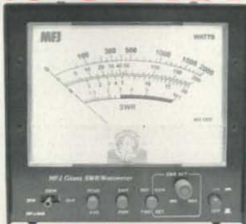
MFJ-868 Has 20/200/2000 Watt ranges for accurate QRP or QRO operation.
