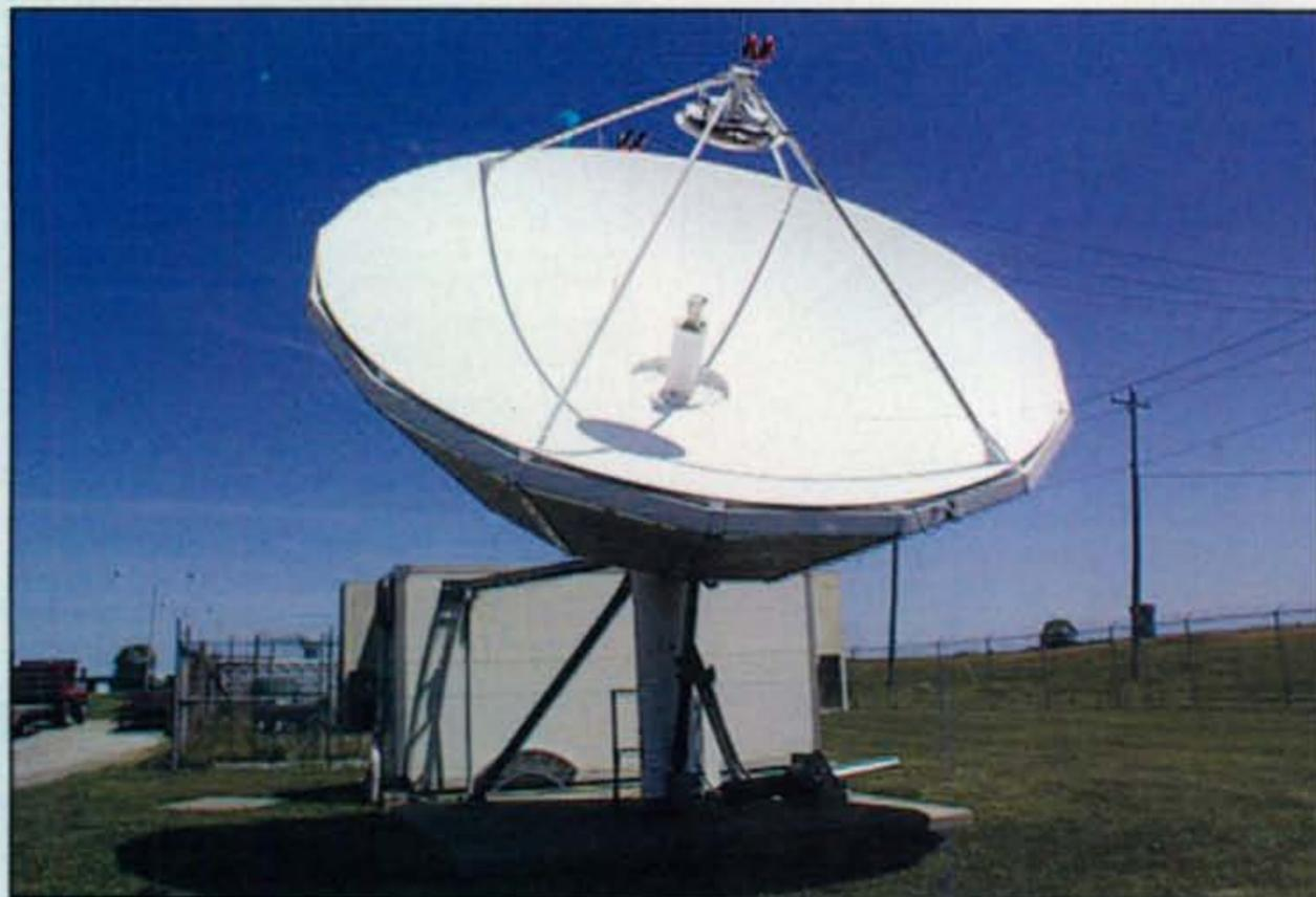
*Photo A— WC8VOA's EME dish, Model KXK 7.2M (24') Ku-band satellite antenna by Vertex/RSI, 54 dB gain in 0.28-degree beamwidth. It had been abandoned in November 1995 at the Bethany VOA. (Photo courtesy of the WC8VOA website: <[www.wc8voa.com](http://www.wc8voa.com)>)*
