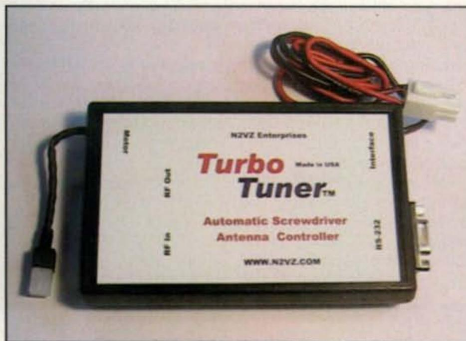
Photo I— The Turbo Tuner from N2VZ Enterprises is an automated screwdriver controller that affords one-button tuning for screwdriver antennas, using your radio's tune button. (Photo courtesy of N2VZ Enterprises)
