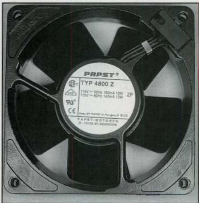
Photo A— Square-frame fans are exceptionally quiet, efficient, and popular for cooling everything from power supplies to linear amplifiers. This particular fan is used in an Ameritron AL-80A linear amplifier. It is positioned in the unit's mid section so it draws air across power-supply filter capacitors and blows it across the 3-500Z tube. (Photo courtesy of MFJ Enterprises)
