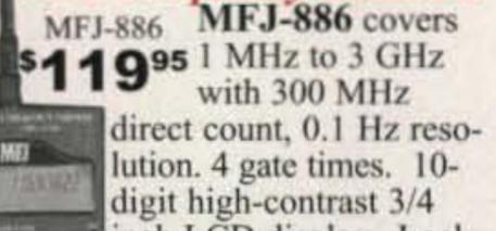
MFJ-886 covers 1 MHz to 3 GHz with 300 MHz direct count, 0.1 Hz resolution. 4 gate times. 10-digit high-contrast 3/4 inch LCD display. Lock display button. Bargraph shows RF field strength. Includes rechargeable Ni-Cad batteries, charger, telescopic antenna. Black anodized aluminum. 2 1/4" x 2 1/4" x 1 1/4" in. MFJ-888, like MFJ-886, but covers 10 Hz-3 GHz. Measures frequency/period, has 50/1M Ohm input, auto hold, LED backlight, beeper. 2 3/4" x 4 1/4" x 1 1/4" in.
