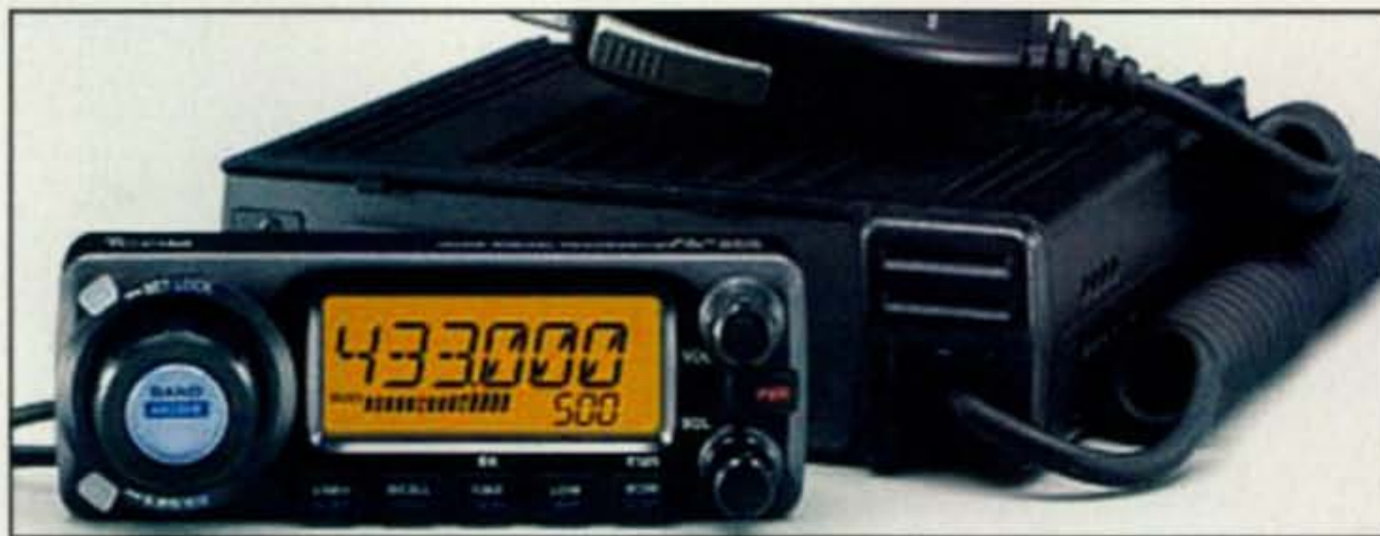
ICOM's IC-800 is a dual-band (2m/70cm) D-STAR-ready transceiver that offers traditional analog voice as well as the digital voice and data features of D-STAR. (Photo courtesy of ICOM America)
