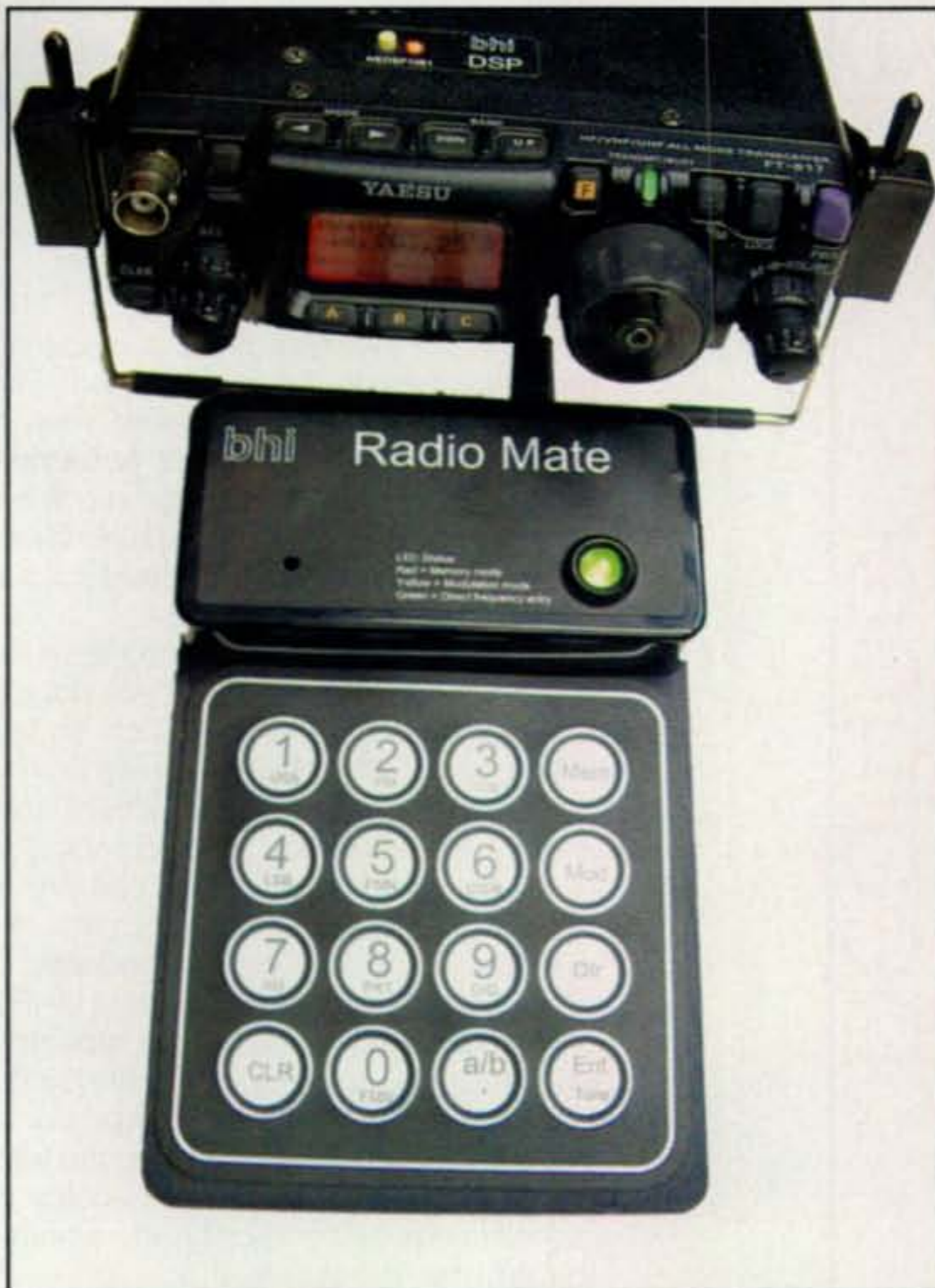
Photo I— Check out this new Radio Mate from W4RT Electronics. It plugs into a rear socket on the FT-817 and produces direct selection of bands/frequencies, modes, and any of its built-in 20 memories. It's a blast for contesting and laid-back QSOing as well. Details at < www.w4rt.com >.
