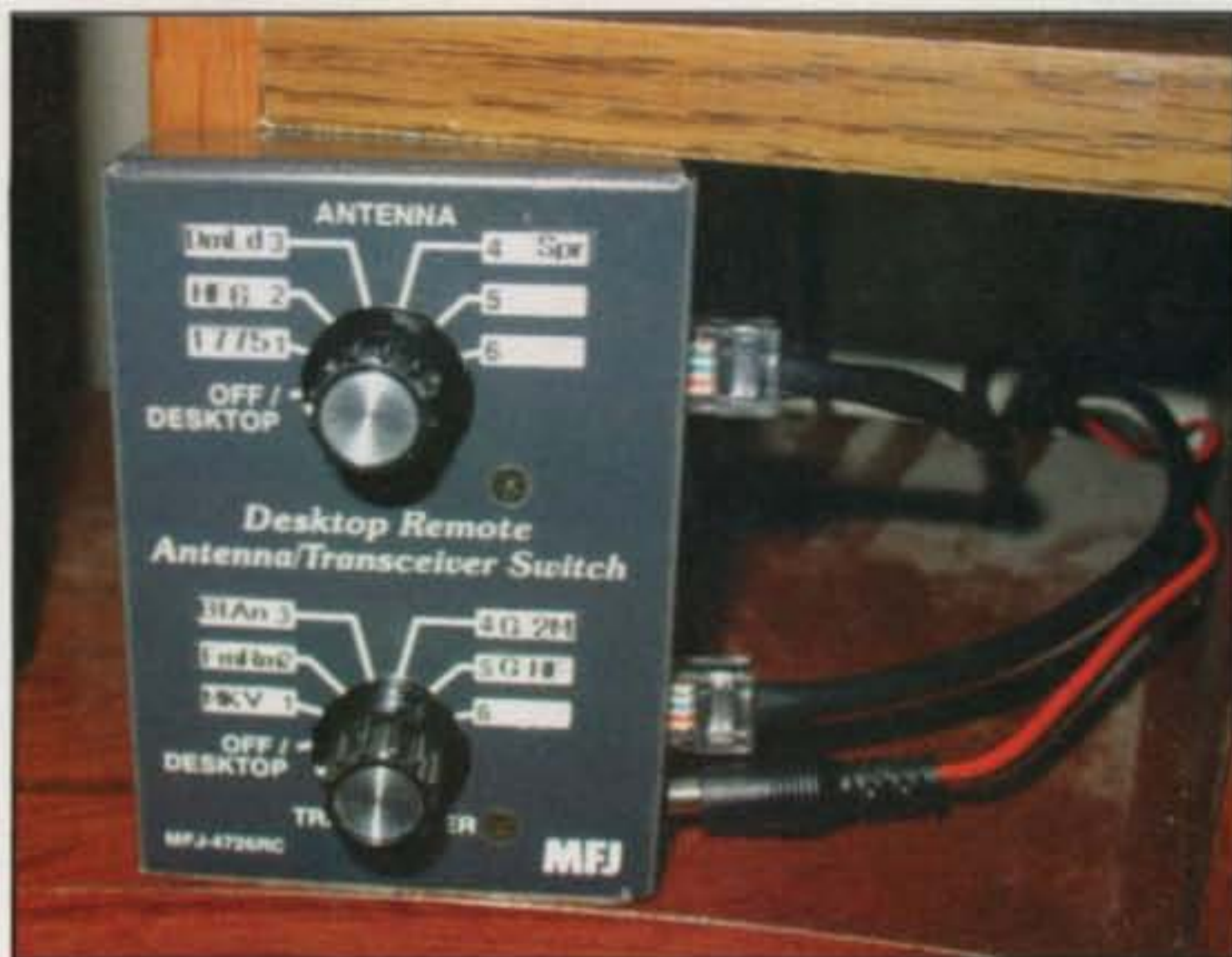
Photo B— Close-up of the MFJ-4726RC. This optional remote-control unit allows you to mount all of your feedlines out of the way (see photo C) and just have the control unit on your desk.
