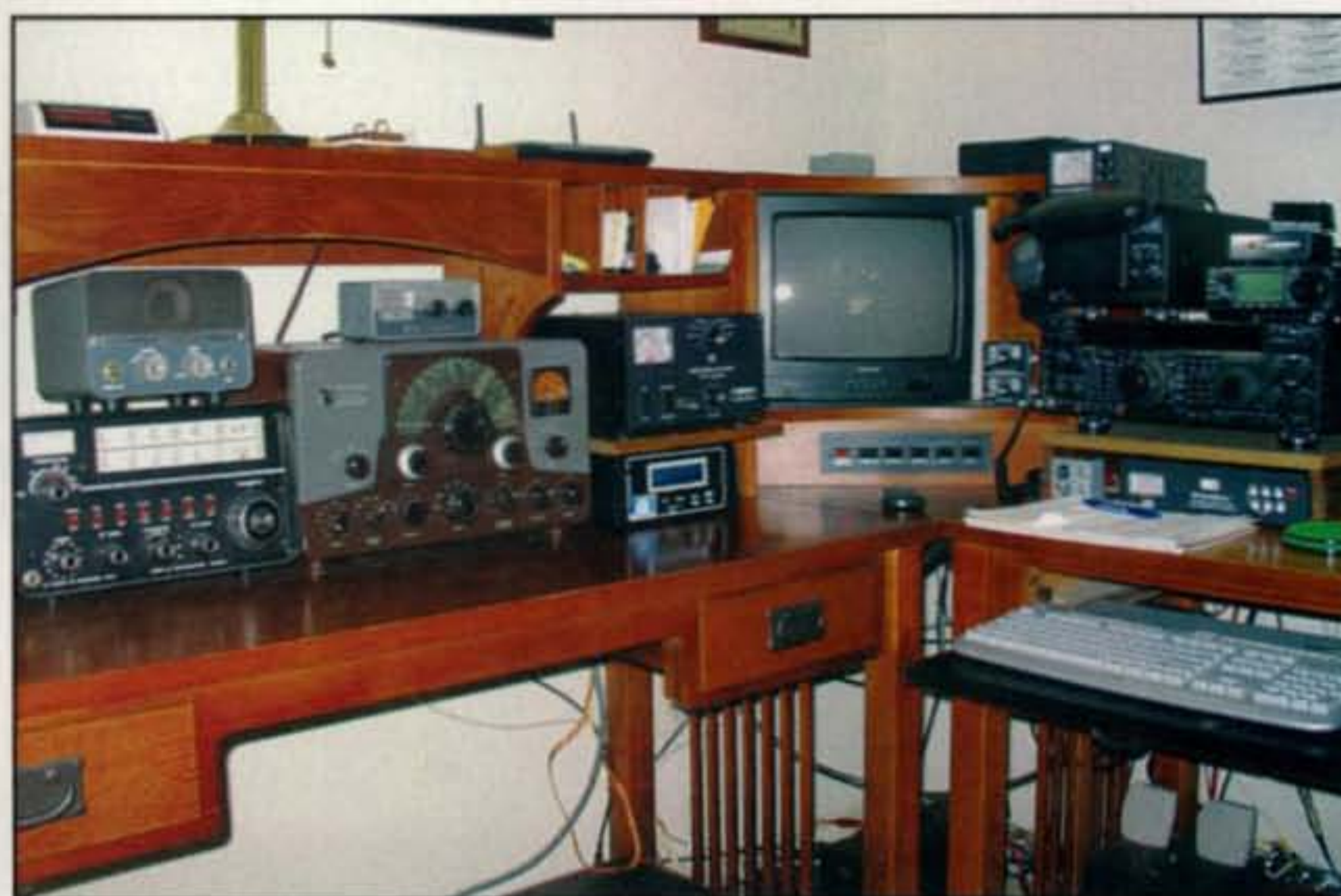
Photo D— The author's multiple radio station. Using a switch such as the MFJ-4726 makes it a snap to connect whichever radio he wants to use to whichever antenna he wants to use.
