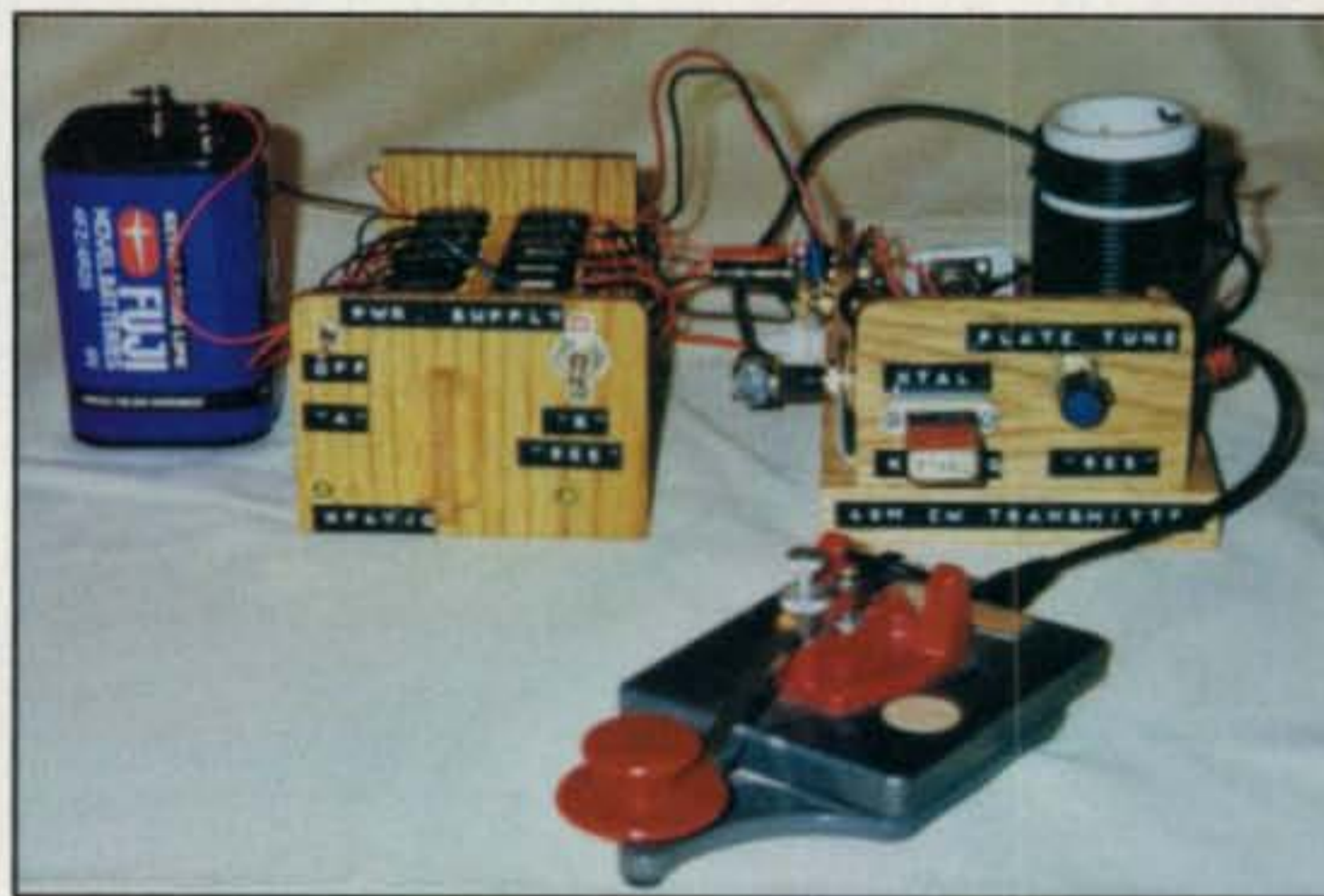
Photo F— A delightful blend of milliwatt magic and nostalgia are immediately apparent in this wood-framed 955 Acorn Tube transmitter and its battery supply built by Walt Bullerwell, KF4YJQ. Running 100 milliwatts on 40 meters with the rig, Walt worked stations around the country immediately after assembly. (Photo courtesy of KF4YJQ)
