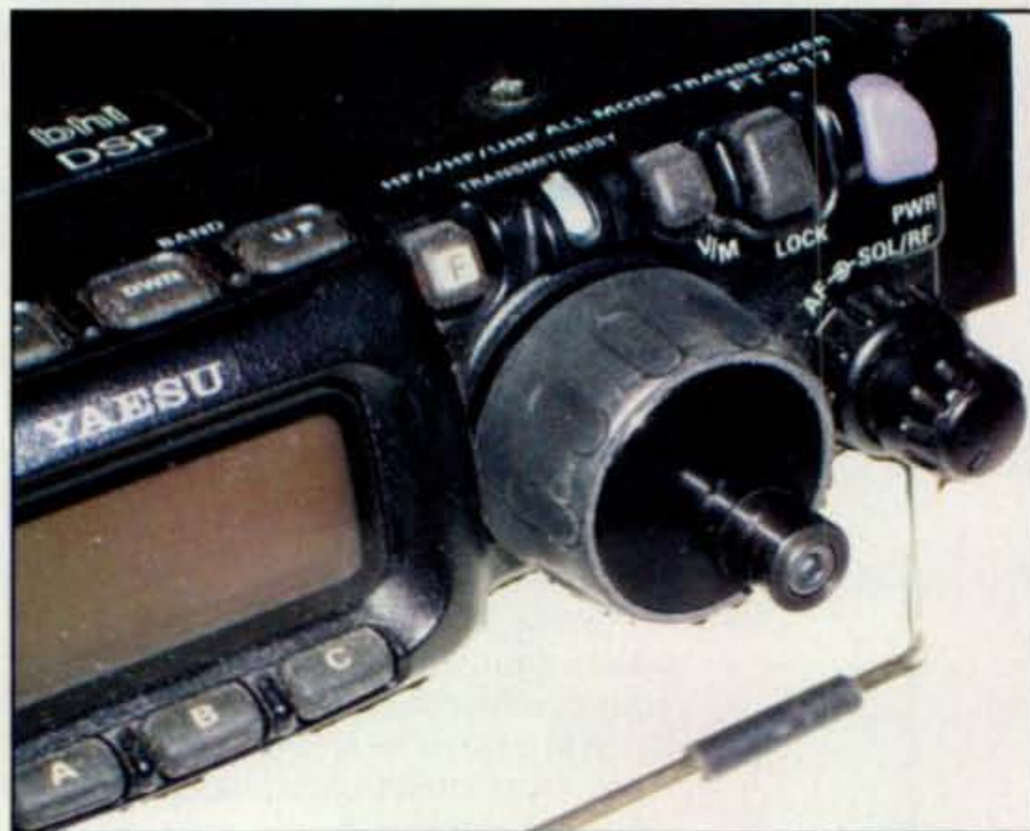
Photo J— Another special item available from W4RT Electronics is this K8FF Kranker Knob. It quickly swaps with the FT-817's stock knob and makes band tuning both delightful and accurate. Nice! (Photo courtesy of Barry Johnson, W4WB)
