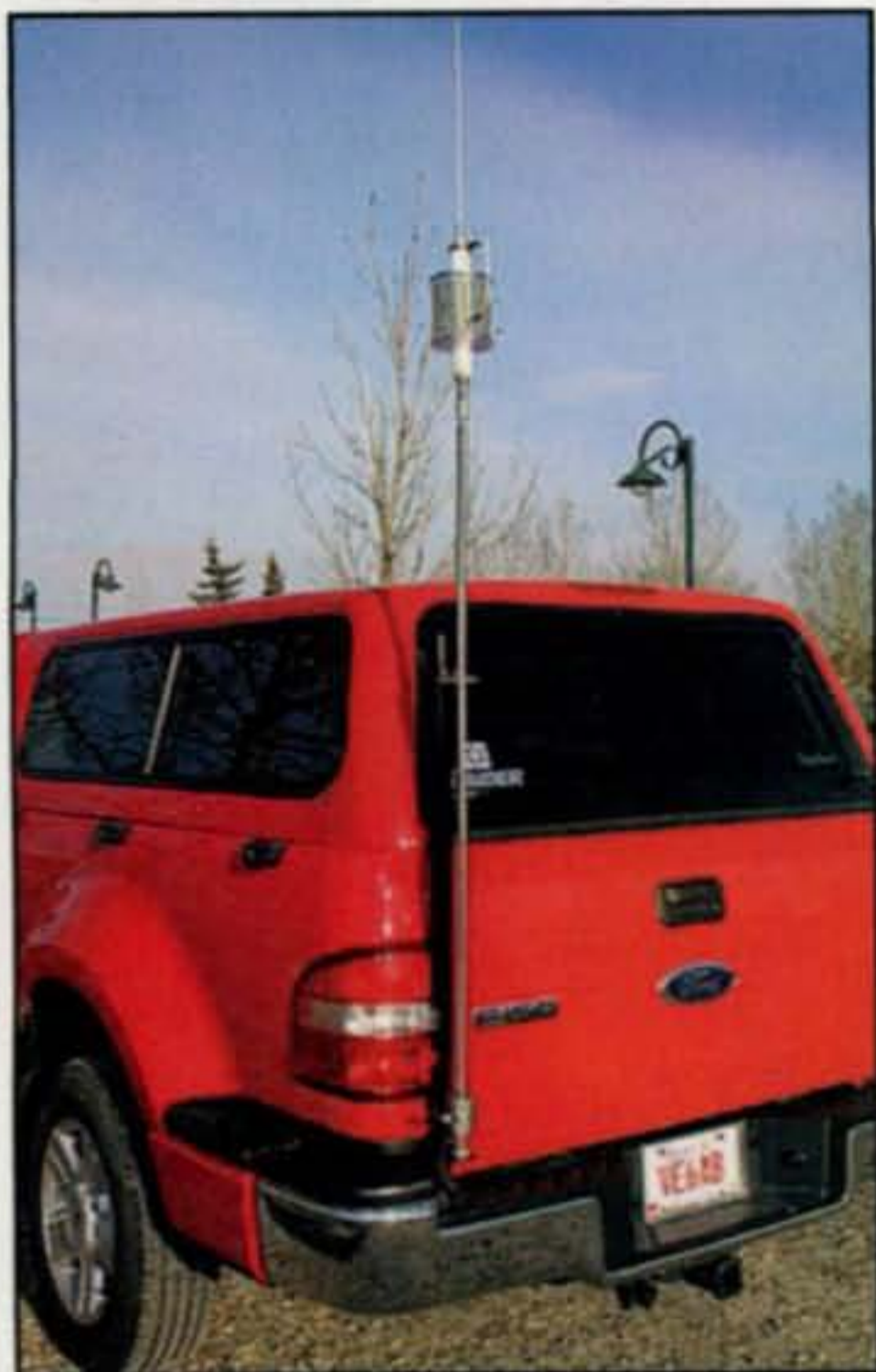
Photo D— VE6AB's Bugcatcher is securely mounted; cross Yagis can also be placed on the mount for mobile satellite work! (VE6AB photo)
