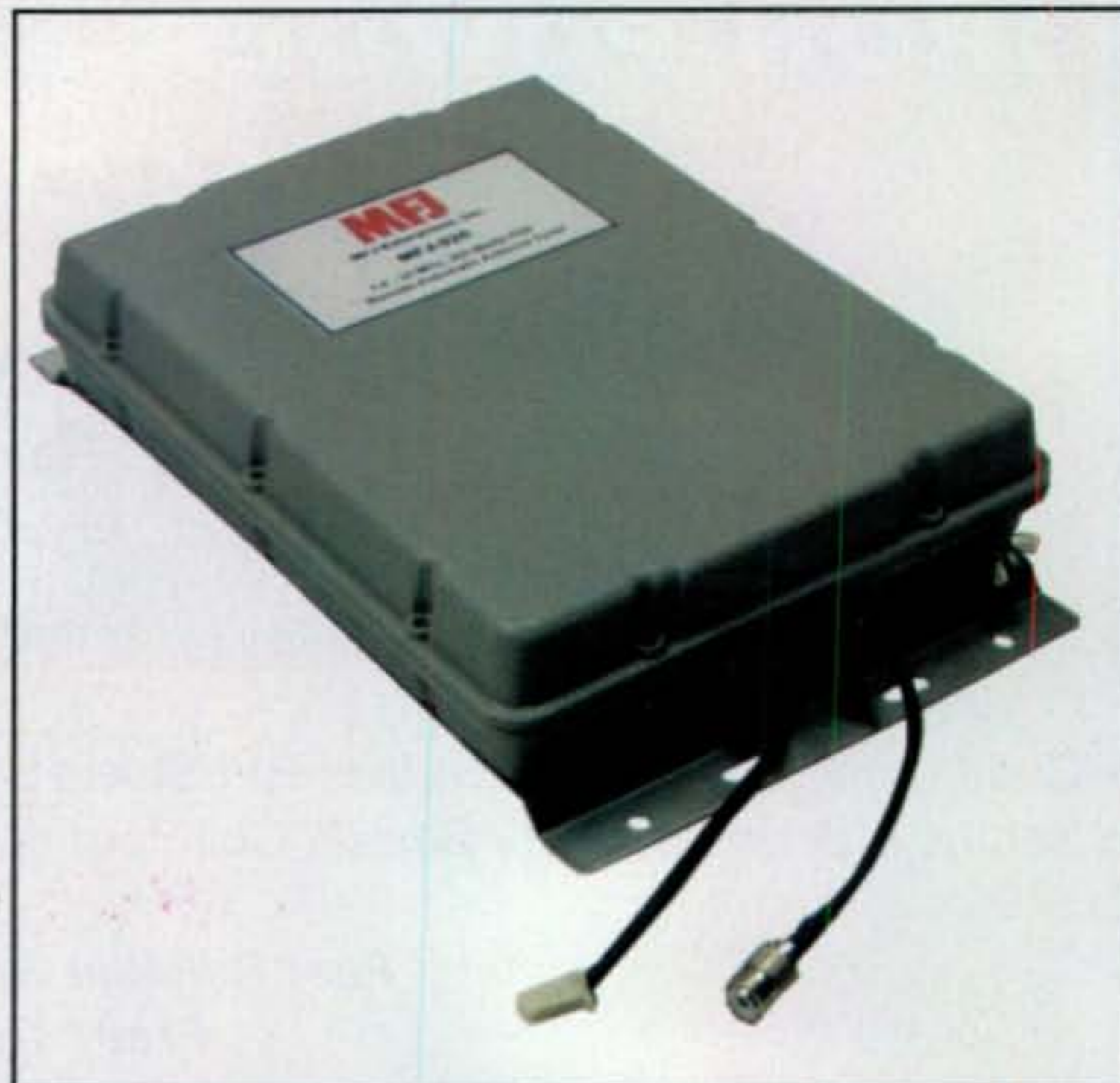
Photo C— The MFJ-926 Remote Automatic Antenna Tuner is weather-sealed for marine use or for use outside at the base of your ham station antenna. The tuner covers the entire HF band from 1.6 to 30 MHz and handles 200 watts PEP. (Photo courtesy of MFJ)
