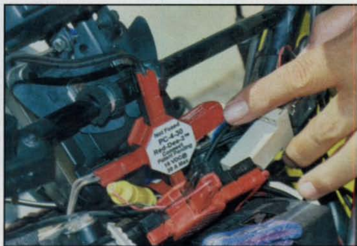
Photo D—Anderson Power Pole connectors make for easy power hookups and—with the plugs used as a standard by club members—easy swapping of radios as well.
