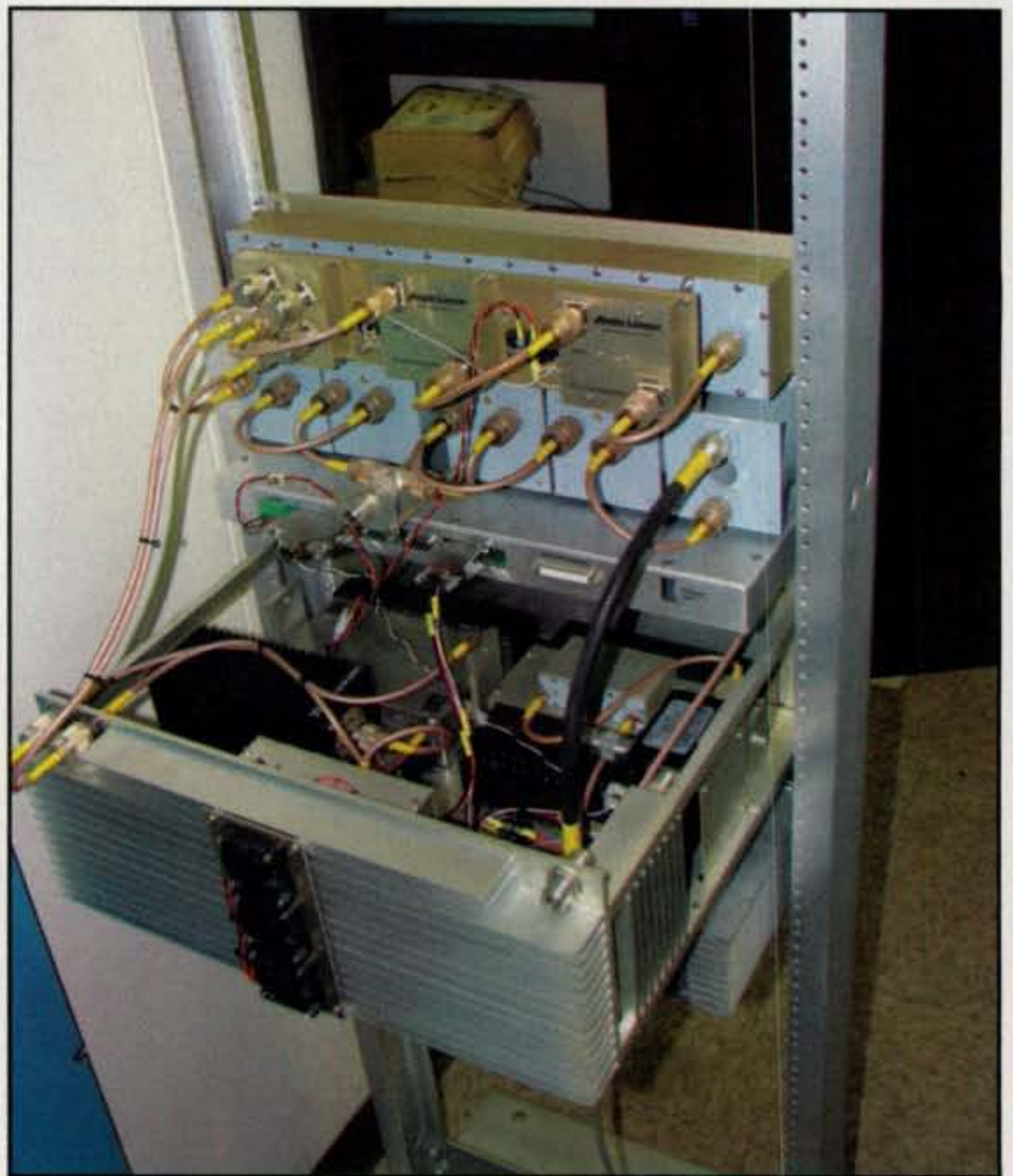
Photo B— The N6CA 900-MHz repeater is a sophisticated machine that receives low-power signals and retransmits them with high power and a tall antenna system, extending communications range to the system users. (Photo by Glenn Allen, KE6HPZ)
