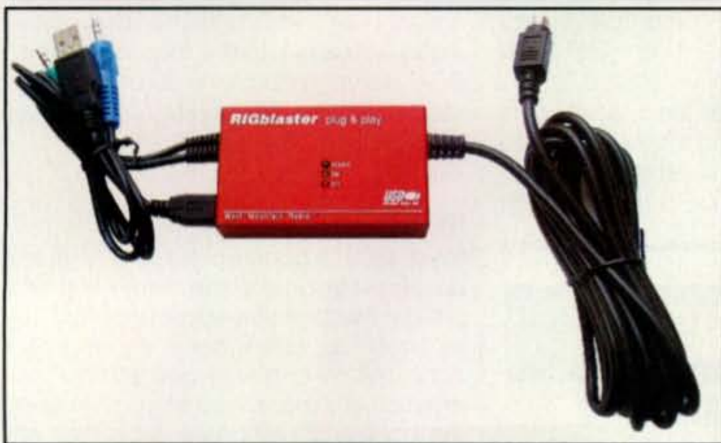
Photo B— The RIGblaster Plug & Play sound-card interface from West Mountain Radio. Truly plug & play, it connects to your radio's data or aux port and gets you on the air in record time. With RS-232 serial ports going the way of spark modulation, a USB interface might be your only choice. (Photo from West Mountain Radio's website)
