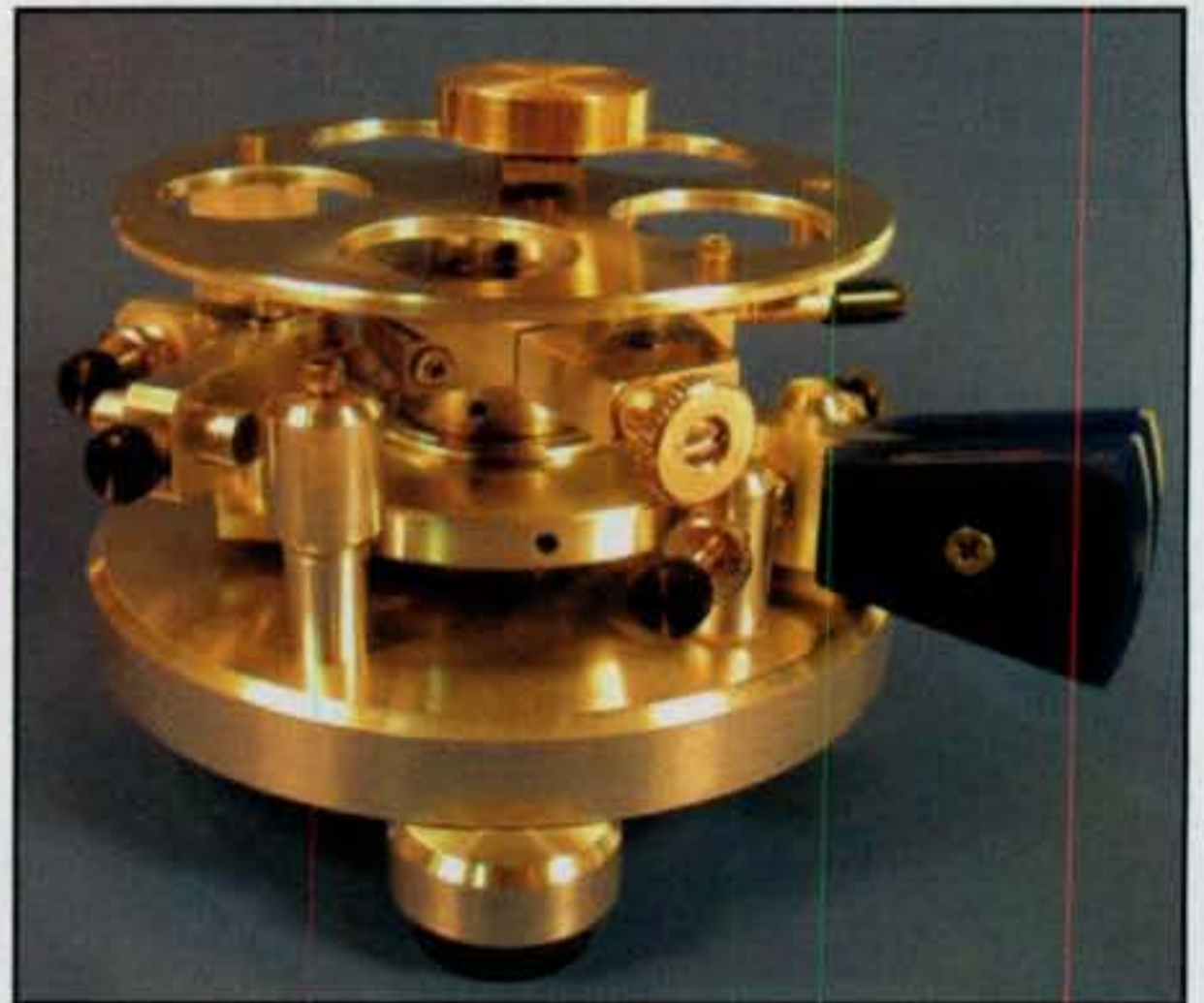
Photo A— QRPers are well known for their creativity, and this round-framed bug designed and built by Richard Meiss, WB9LPU, vividly shows that fact. The bug's three-tier mechanism moves on a center pillar/spindle and operates completely by magnetic action. This thing truly takes bug-transmitted QRP to a new level! (Photo courtesy of WB9LPU)
