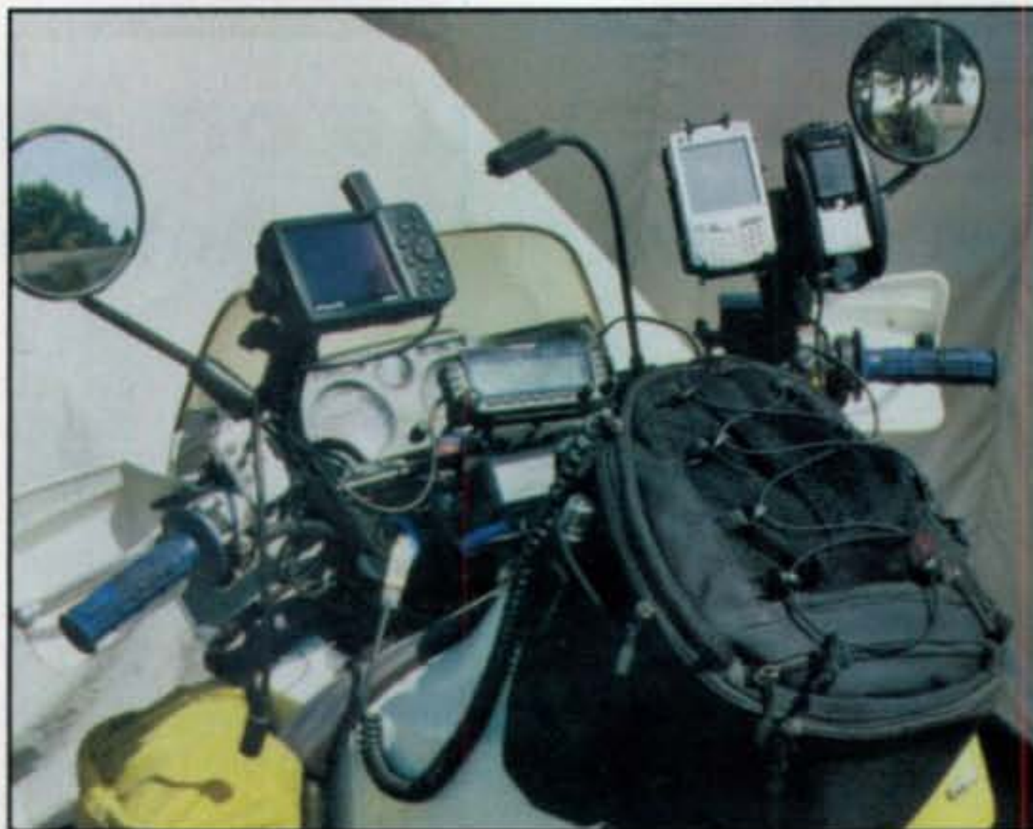
Photo B—Radios and other devices, such as GPS receivers and personal digital assistants, are mounted to be safe yet in easy view.
