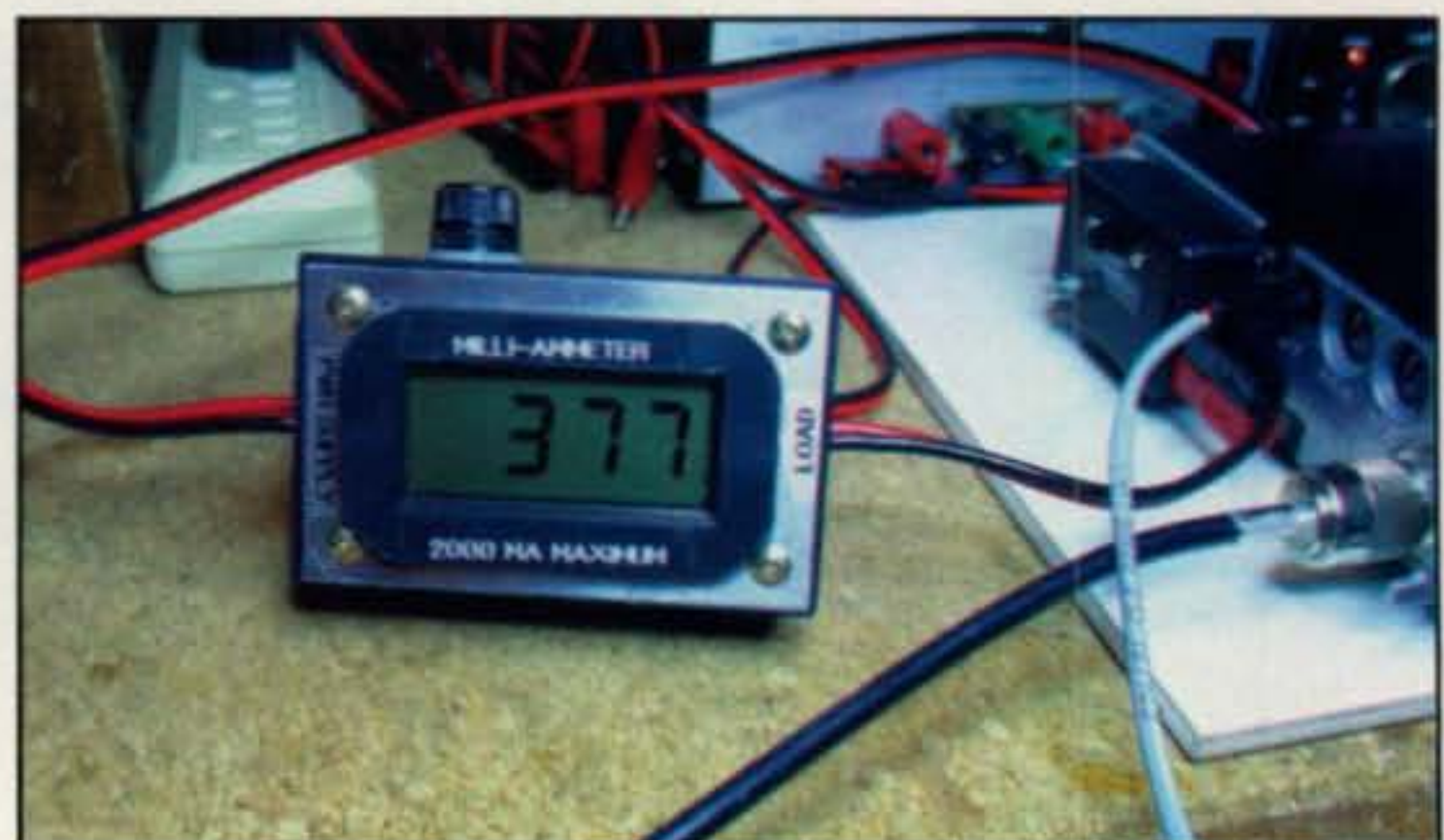
Photo E— Measuring the Yaesu FT-817 receive current (milliamps).
