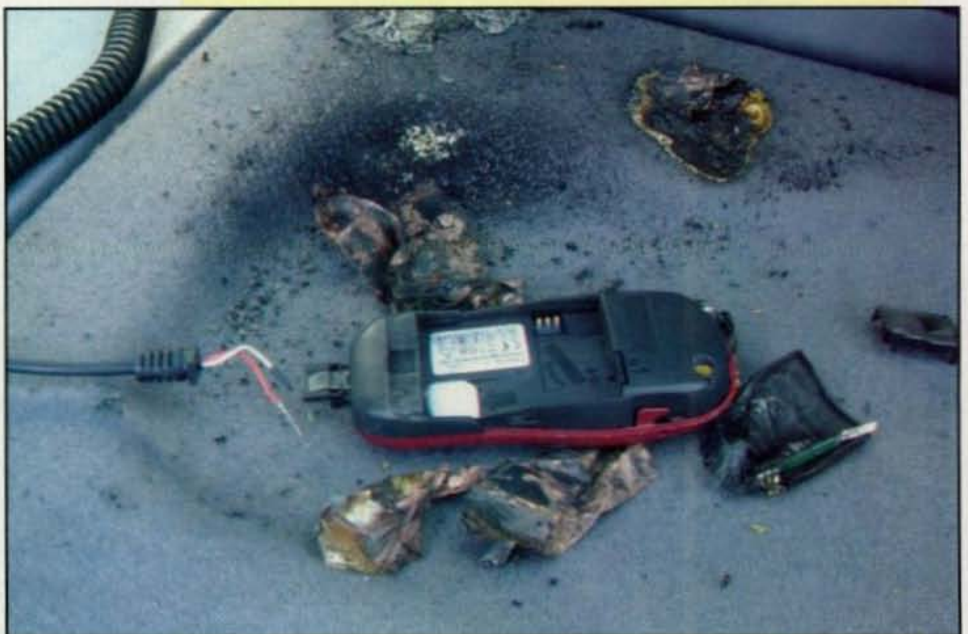
Photo A— A cell phone with a no-brand battery that "vented with flame" while charging in the back of a car.
