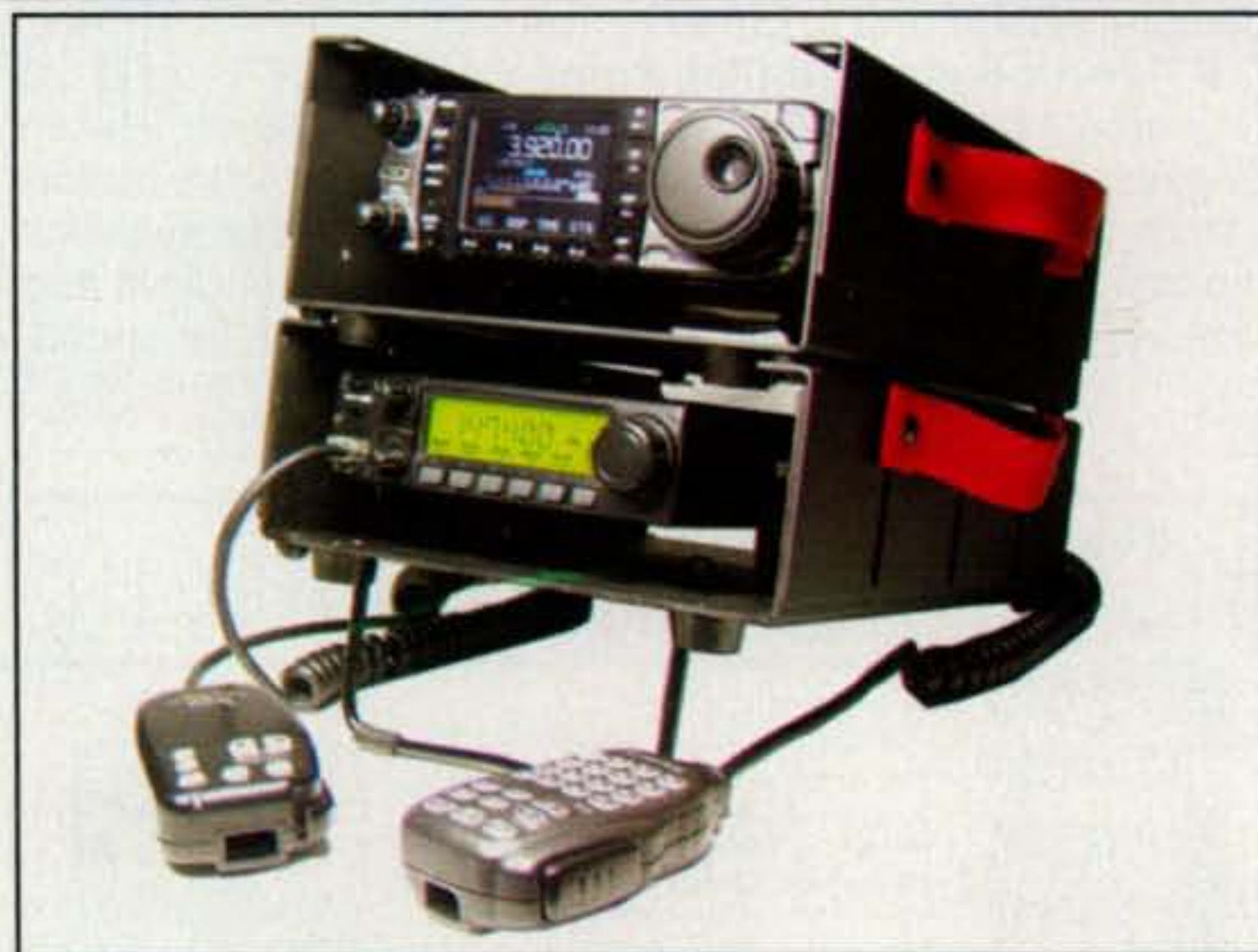
Photo E— You can stack or use side-by-side multiple Tactical Radio Carriers (TRC-1s). Shown here are two stacked TRC-1s that can provide an impromptu communications center boasting a variety of electronics equipment. (Photo courtesy Tac-Comm)
