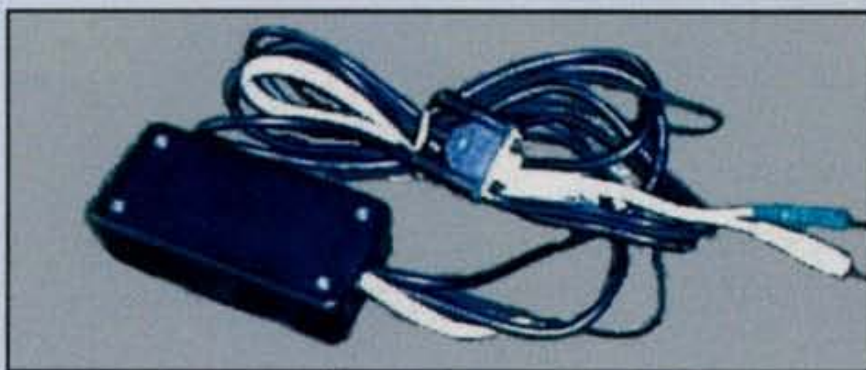
Fig. 4—A variety of commercial interface boxes are also available to connect your computer to your radio.
