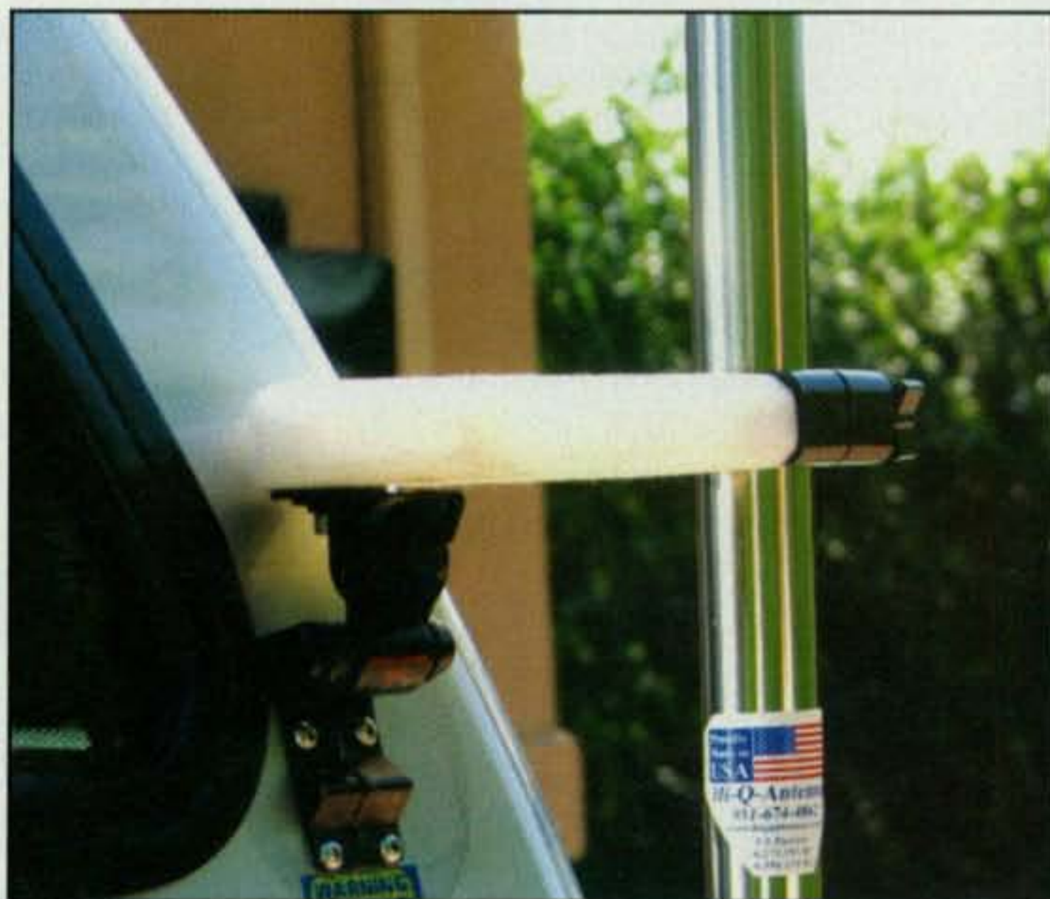
Photo E— Extra support comes from a nylon brace on the outside of the vehicle.
