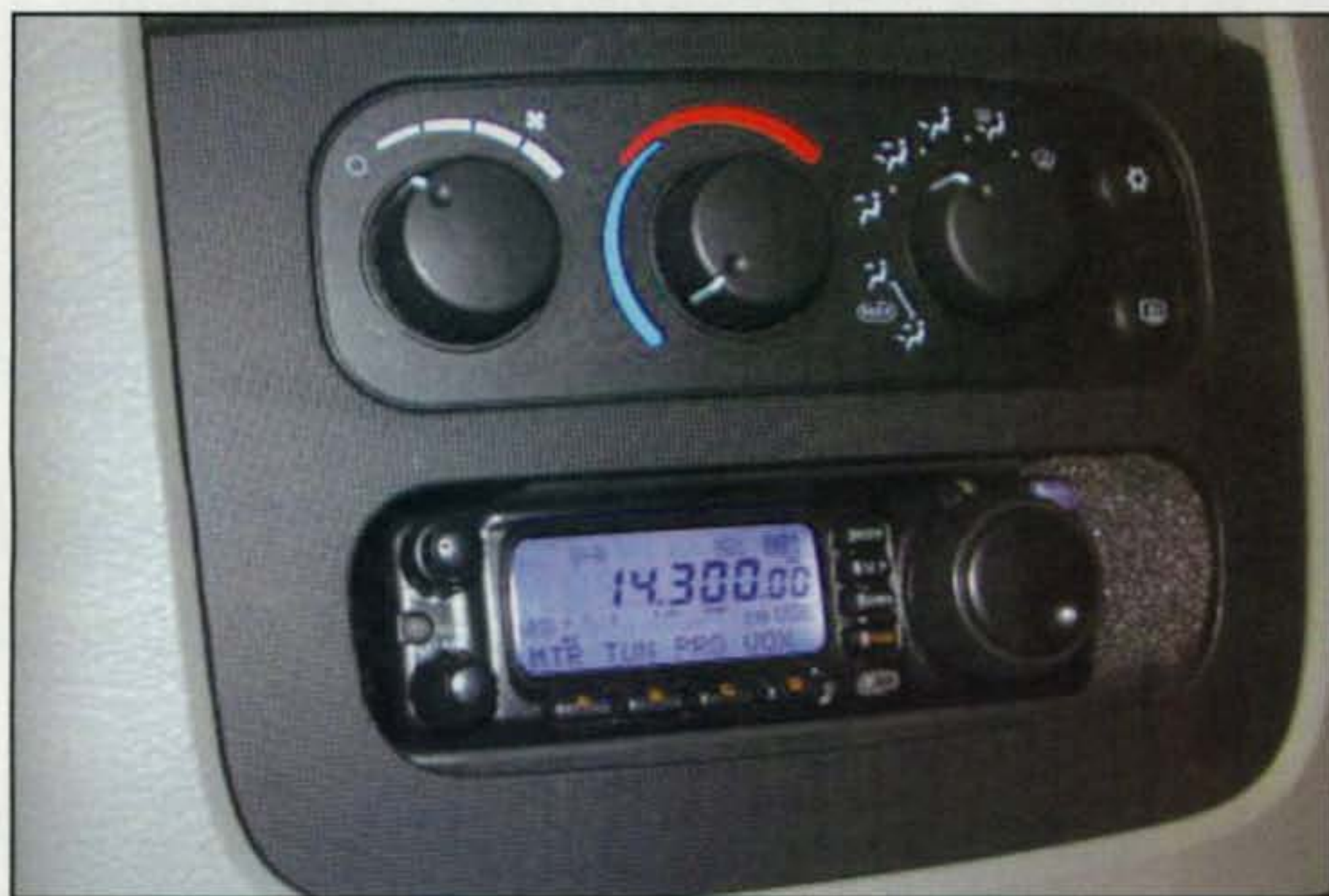
Photo A— In today's cramped, crowded cars it's much easier to safely install a remote-control head than an entire radio. (All photos by Kari Arave, KF7DP)
