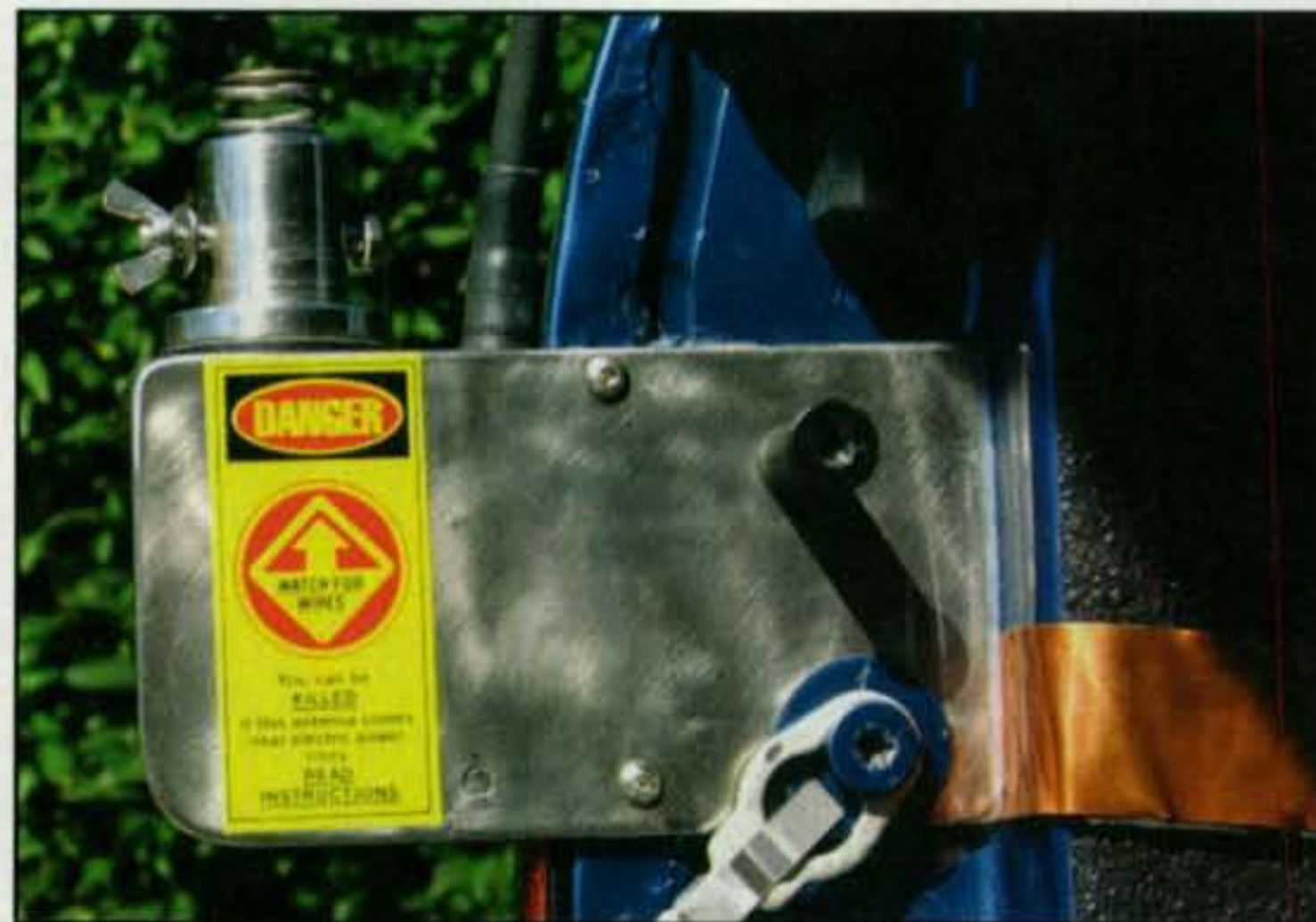
Photo D— Detail of the mount installation. The author drilled holes in the plate to match existing holes in the truck.
