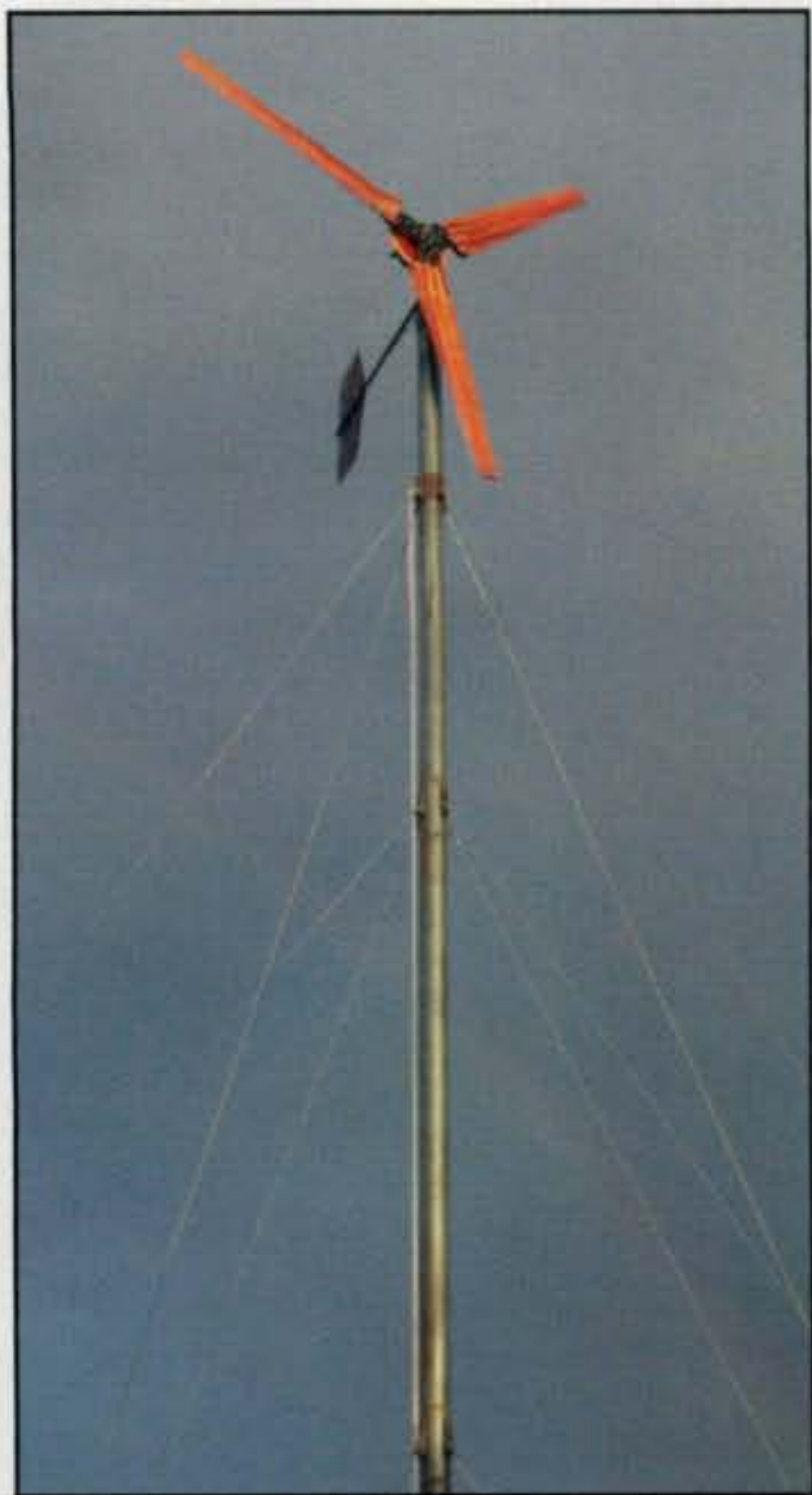
Photo 4— Wind turbines are an effective and/or progressive form of alternative energy and work well for powering your ham gear, backing up a solar energy system. Large wind turbines can even power an entire house. Just ask Dan Bartmann, KC0VSU. He lives 11 miles from commercial power lines, builds and sells plans and parts, plus offers free advice for making this 20-foot model wind turbine, which powers his house and workshop. Details in text and at < www.otherpower.com >.
