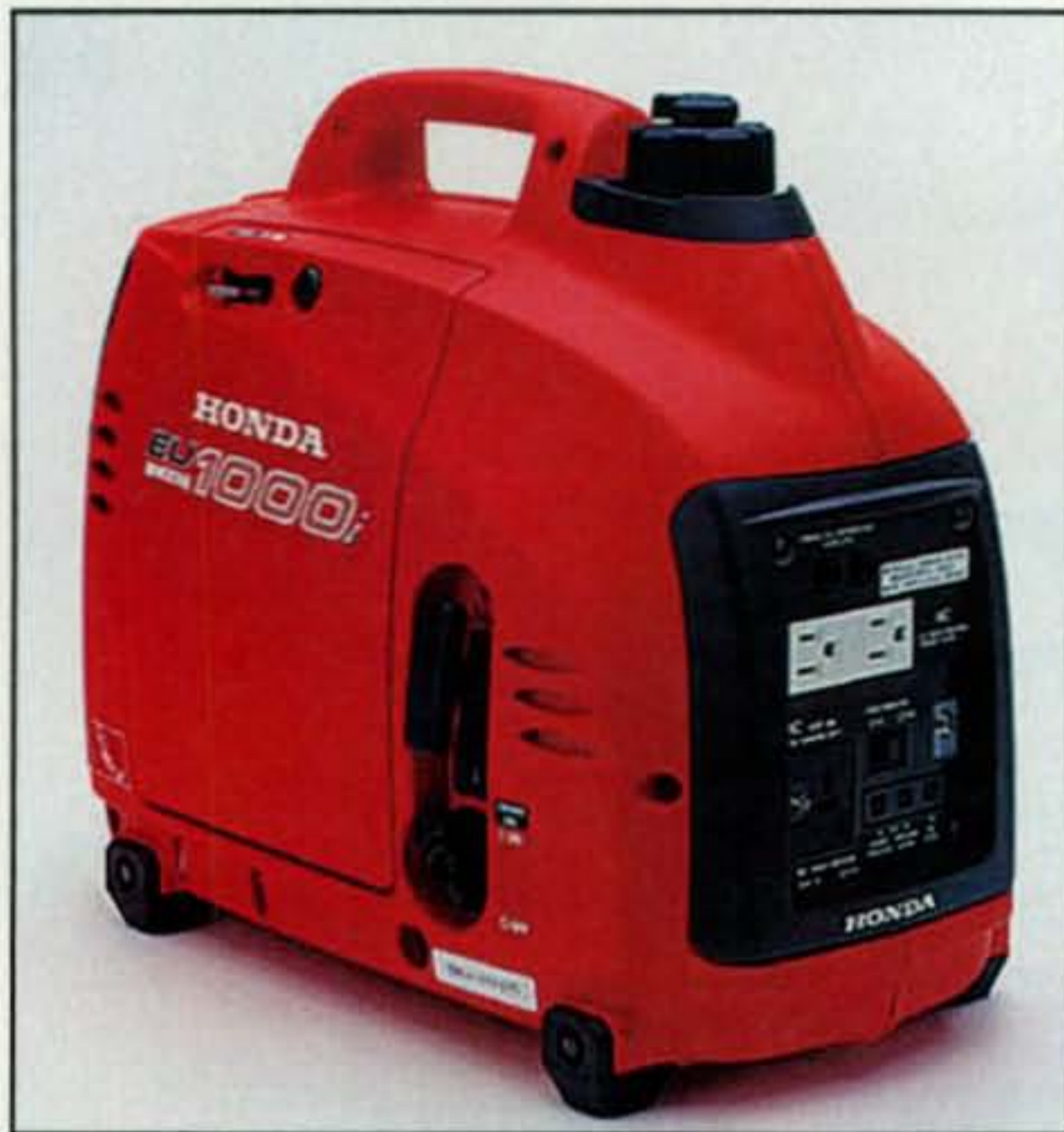
Photo 2— Portable gasoline-engine-driven generators in the 1000-to 4000-watt range are made by several well-known manufacturers and are quite popular sources of power during short-term emergencies. They are also handy for backing up a solar- and/or wind-powered system. Never attempt directly connecting one to your home's existing wiring. Use a separate and fused extension cord for safety. The generator shown is available from < www.mayberrys.com >.
