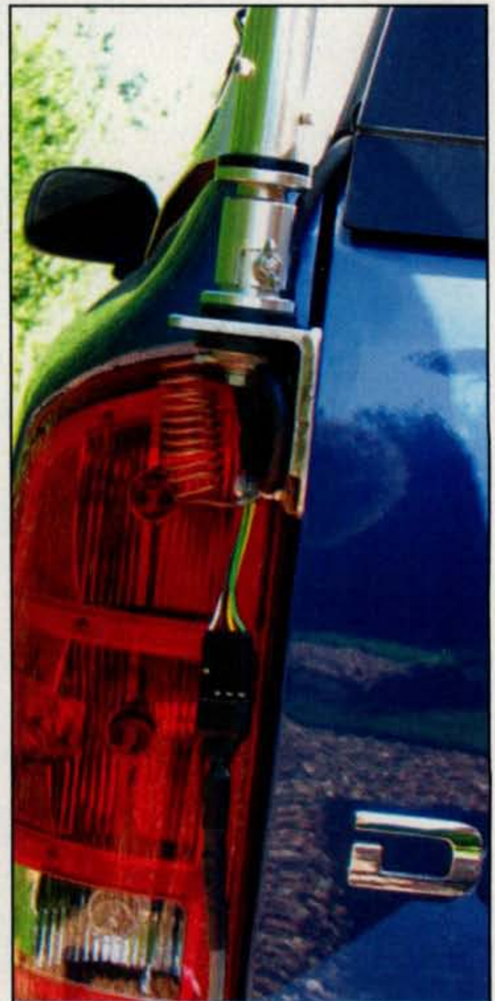
Photo C— The author mounted his mobile HF antenna just above his left tail light. It attaches inside the tail gate (see photo D).
