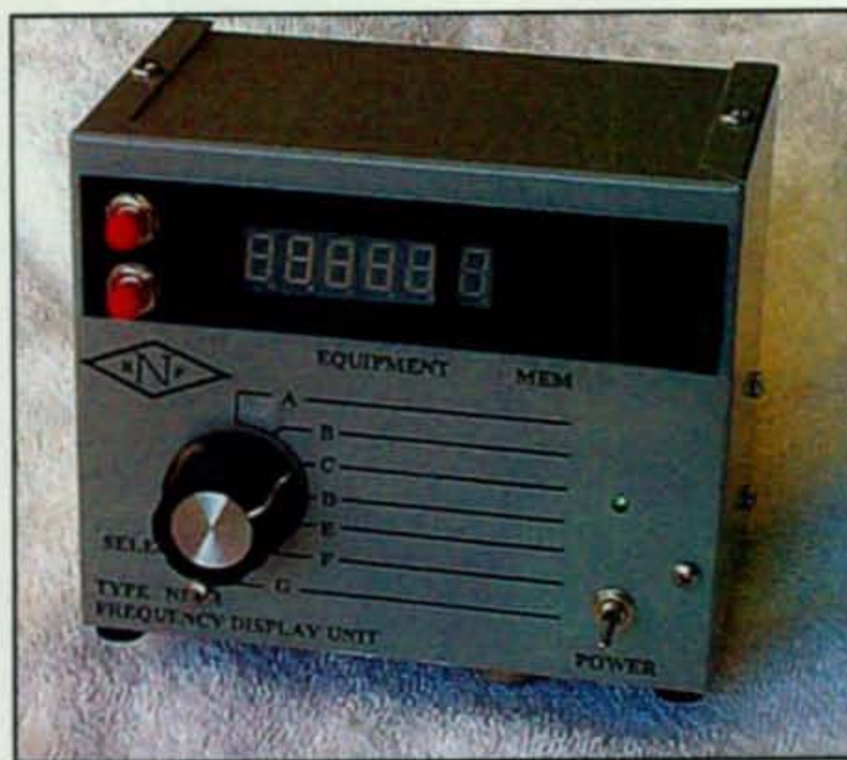
Photo A— The National RF NFD-1 Frequency Display is designed for use with vintage/classic communications equipment to display the received or transmitted radio frequency. Details? They are found within this month's column. (Photo from the National RF website)
