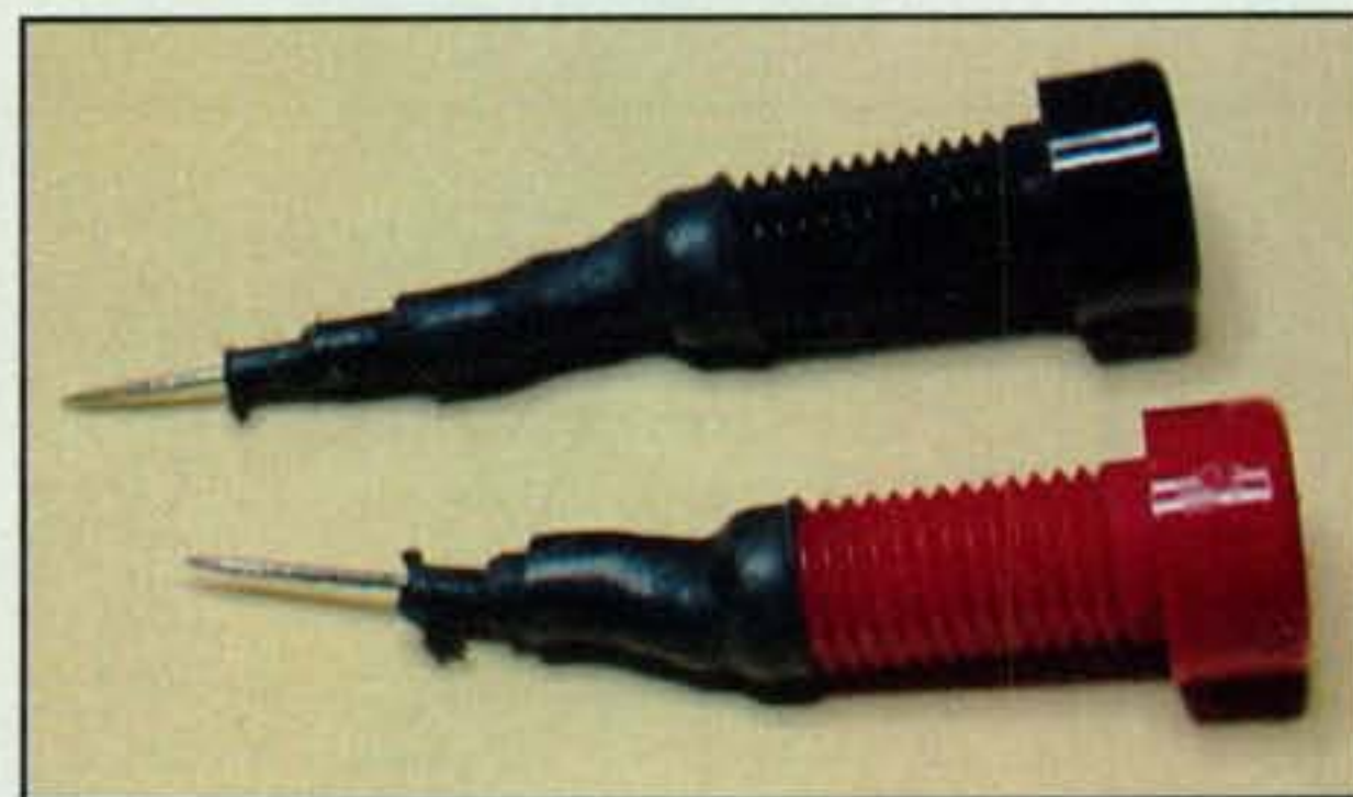
Photo B— The finished tip probes make it much easier to reach a multimeter cable into the tight confines of a circuit board than the standard banana plugs that come with most meters.
