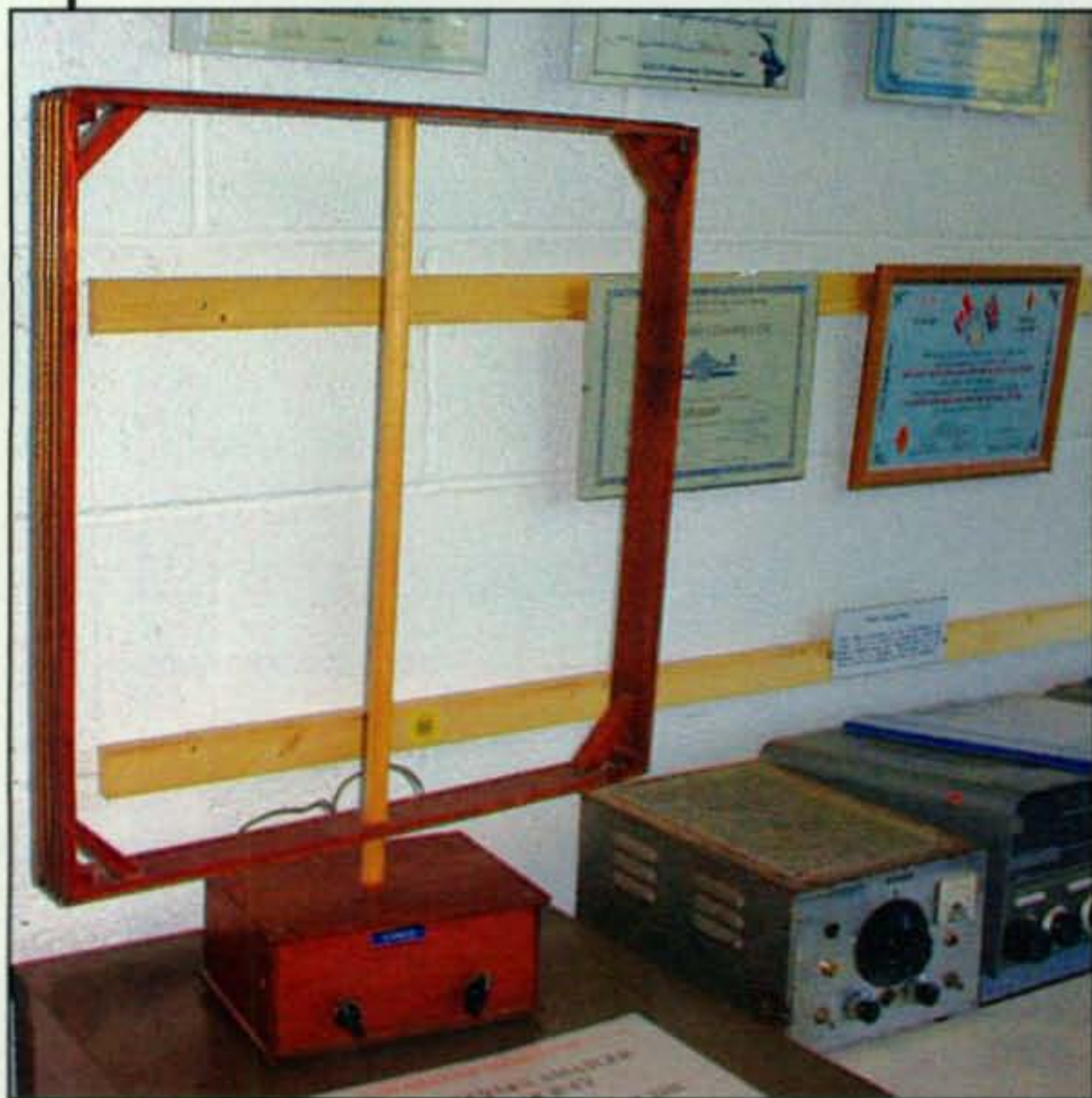
Photo A— Receive loop antenna at the Bletchley Park Cryptography Museum in the UK.
