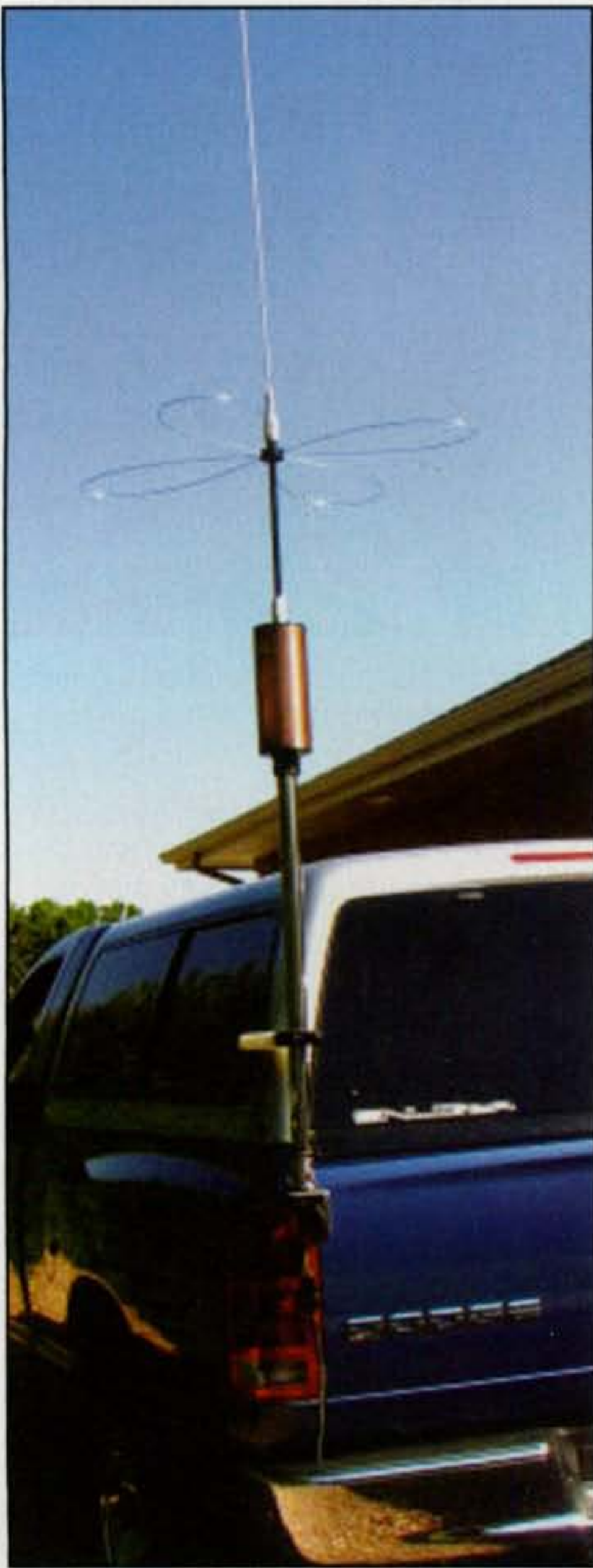
Photo B— Installing a mobile antenna means finding a balance between keeping it low enough for a safe and secure installation and high enough that the loading coil is clear of the roof.
